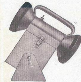
•TYPE T&T 2-WAY with one red and one white light. Beam and red reflectors. Uses two No. 6 or telephone type dry cells. 1/5th mile range. Focusing knob. Sturdy rustproof steel case.
