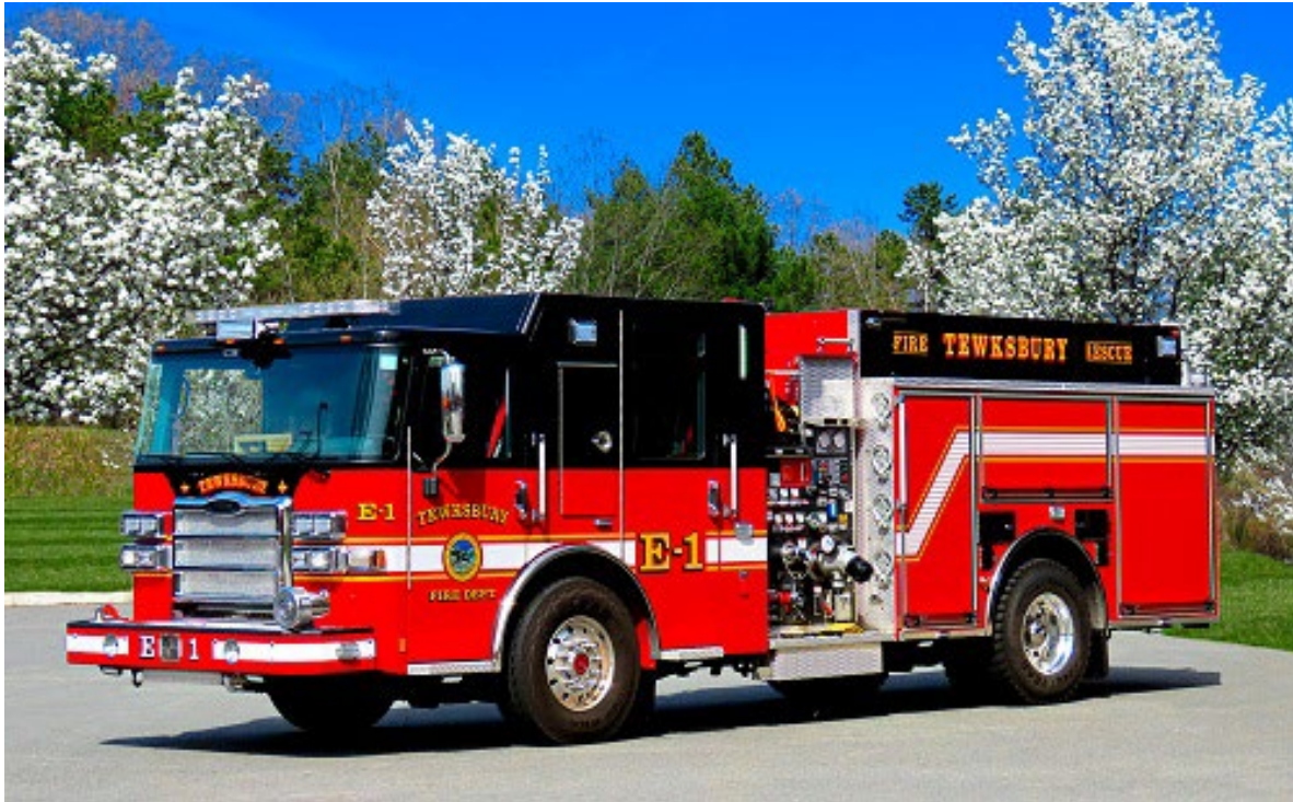
Tewksbury Engine 1 2023 Pierce Enforcer 1500/1000/20 gallons foam.
