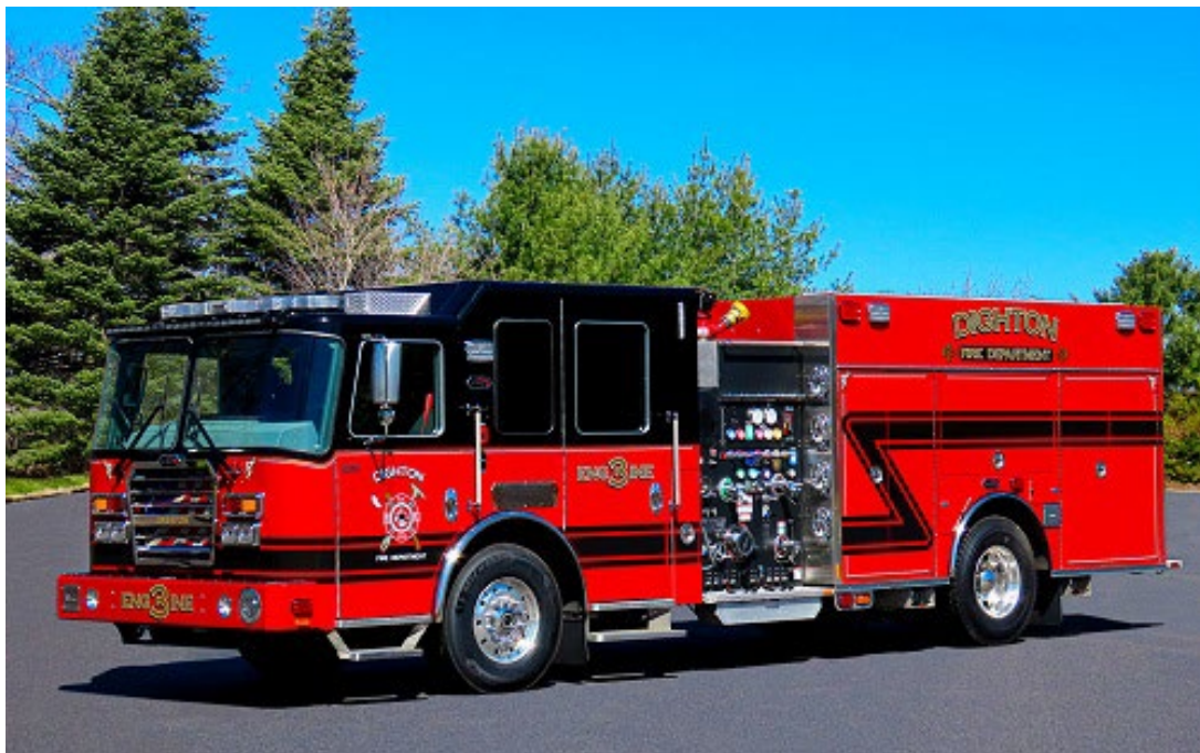
Dighton Engine 3 2024 KME Predator model 1500/1000/ 30 gallons Class A foam. All three pumps and the rescue are built by KME.
