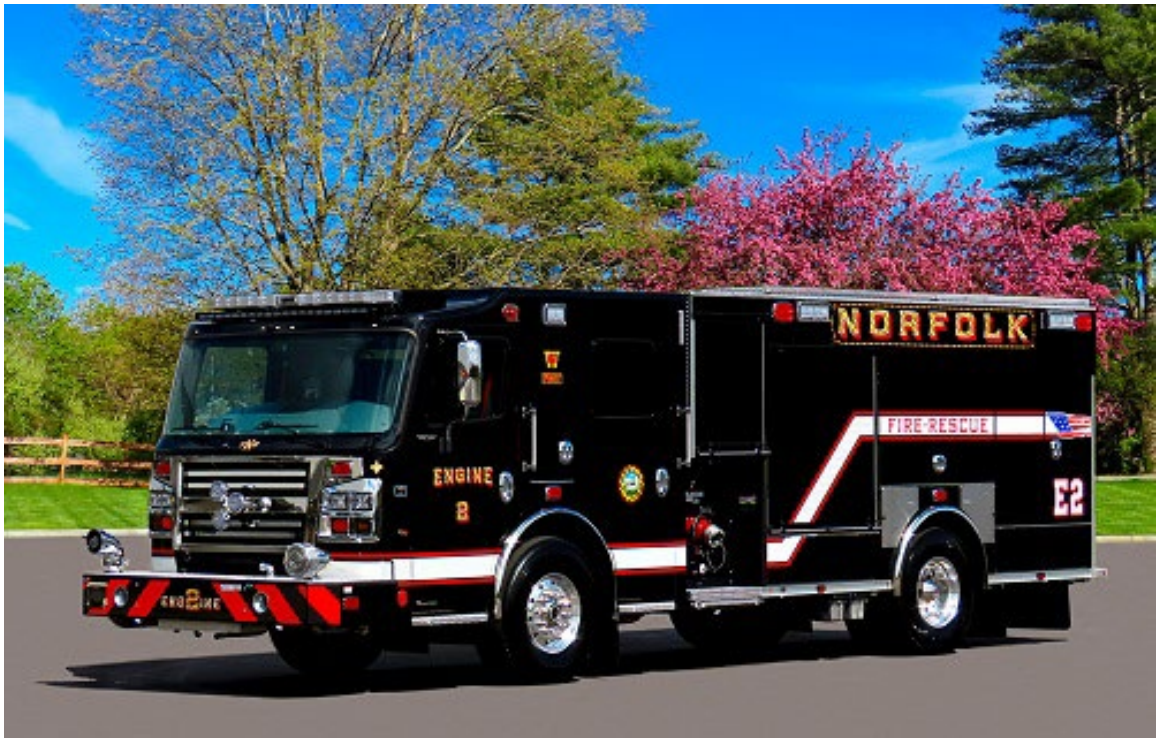
Norfolk Engine 2 2024 Rosenbauer Commander MP3 1500/1000/30 gallons of foam.
