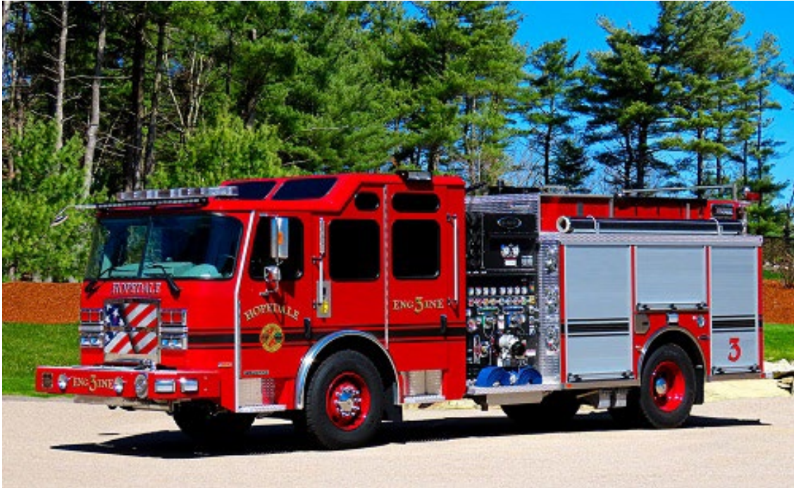
Hopedale Engine 3 2024 Emergency-One Typhoon 1500/750/30 gallons foam.
