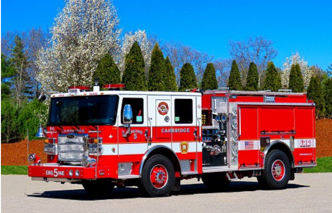
And Cambridge Engine 5 both are 2024 Pierce Enforcer models equipped with a 1250 pump and 500 gallon tank. All front line pumps and spares are Pierce built, along with all their ladder companies!
