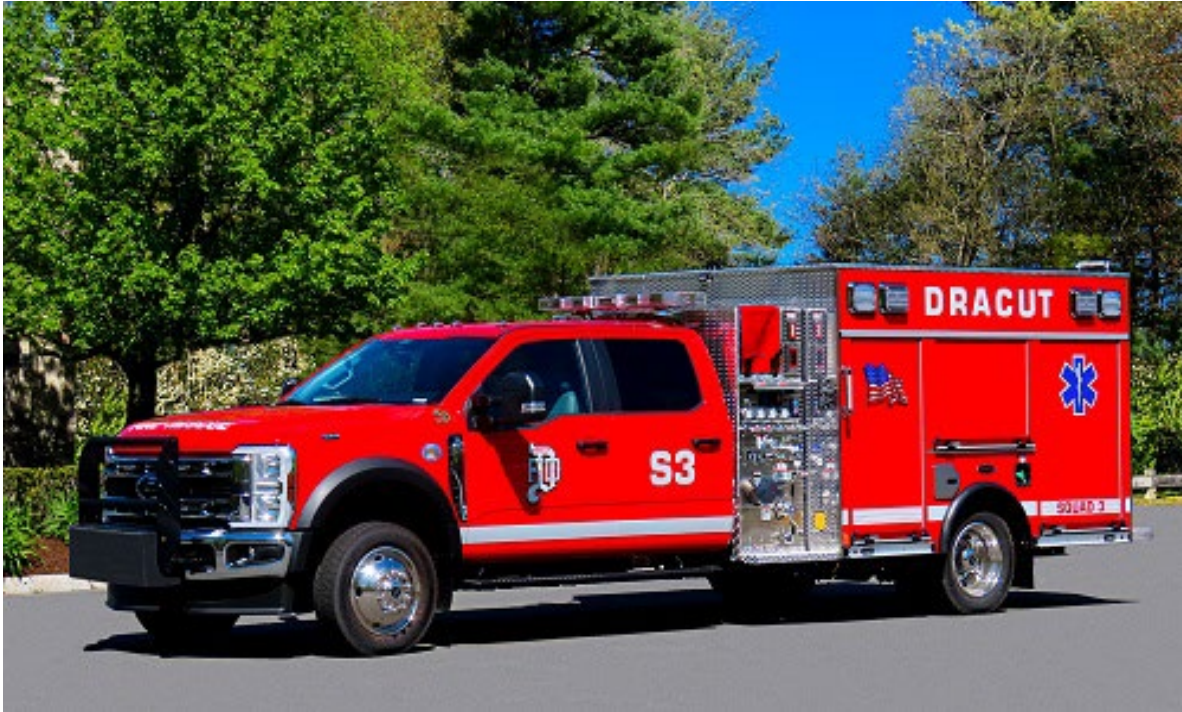
Dracut Squad 3 2024 Ford F-550/Emergency-One 4x4 equipped with a 1250 gpm pump, 300 gallon tank and 20 gallons of foam.
