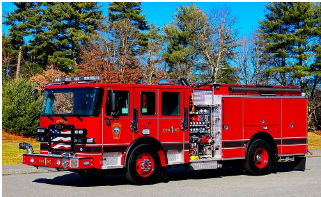
Hopkinton Engine 1 and Engine 2 both received 2024 Pierce Enforcer models 1500/750/20 gallons of foam.
