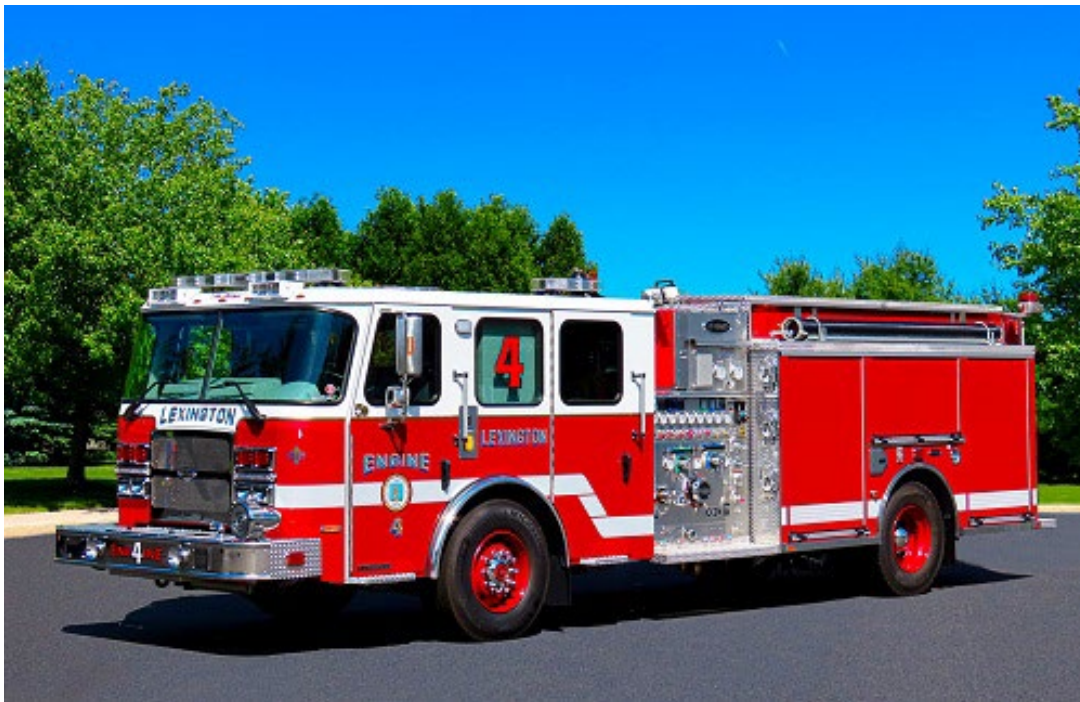
Lexington Engine 4 assigned to East Lexington is a 2024 Emergency-One Typhoon model with a 1250 gpm pump with a 500 gallon tank and 30 gallons of Class A Foam. Another Departments whose frontline and spare pumps and the aerial ladder are all Emergency-Ones.
