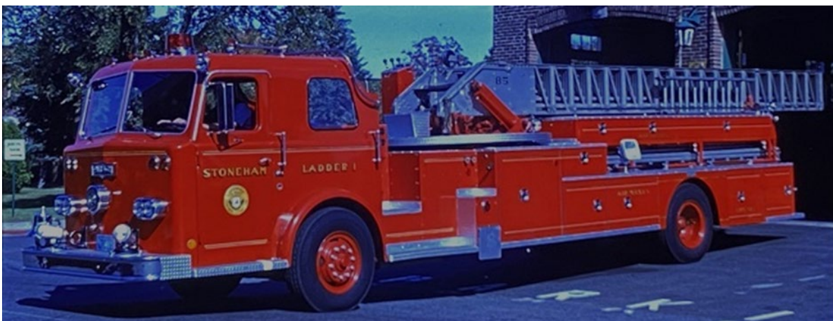
Ladder #1 running a 1969 Pirsch enclosed Custom Cab Service Aerial with 85' Stick. Common at the time for many suburban ladder trucks, Ladder #1 also had a 250 GPM pump and a 200-gallon water tank. While the specific staffing on that day is not available, at the time the Ladder ran with 2-3 firefighters and no officer.
