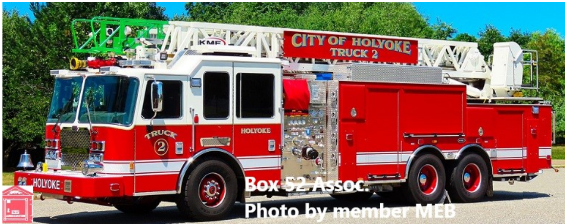
Holyoke Truck 2 – 2020 KME Severe Service 1500/500 103' RMA
