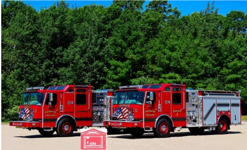
Franklin Engines 1 and 2 2021 E-One Typhoons 1500/750/30A
