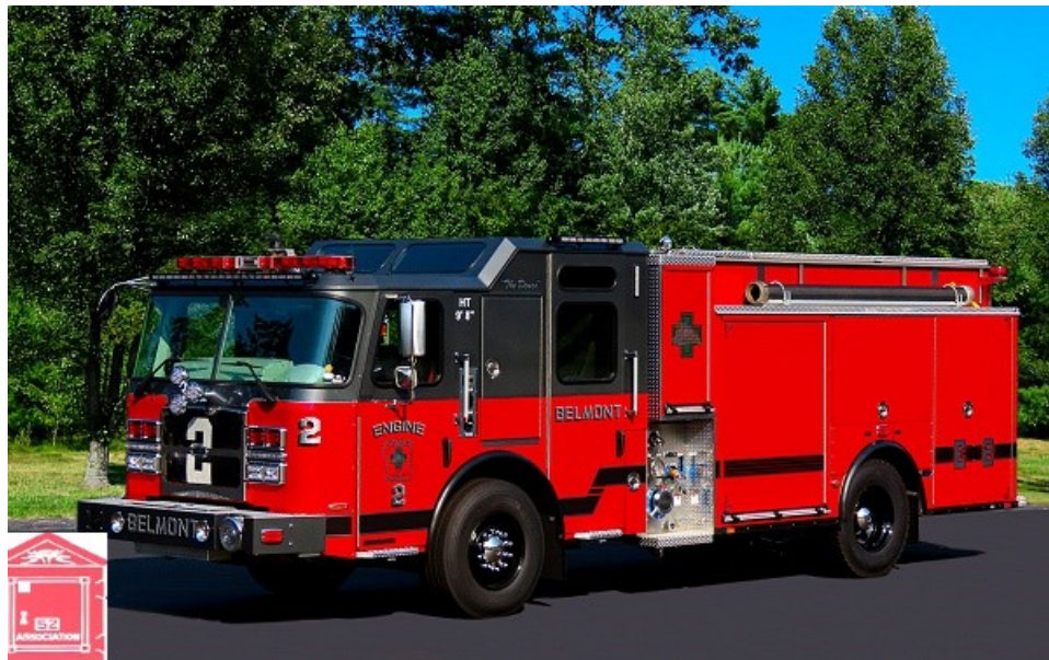
Belmont Engine 2 2021 E-One Typhoon e-MAX 1500/510/20 class B foam
