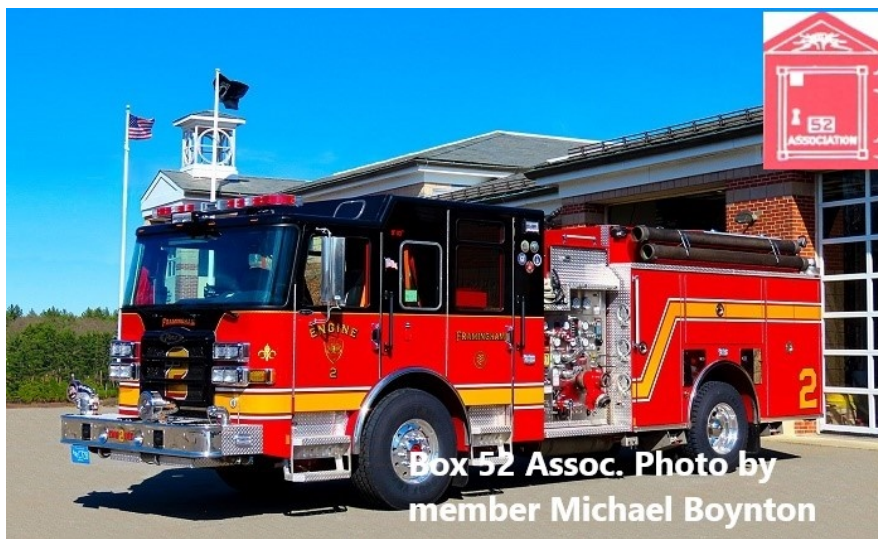
Framingham Engine 2 2020 Pierce Enforcer 1500/750/100 gallons class B foam.
