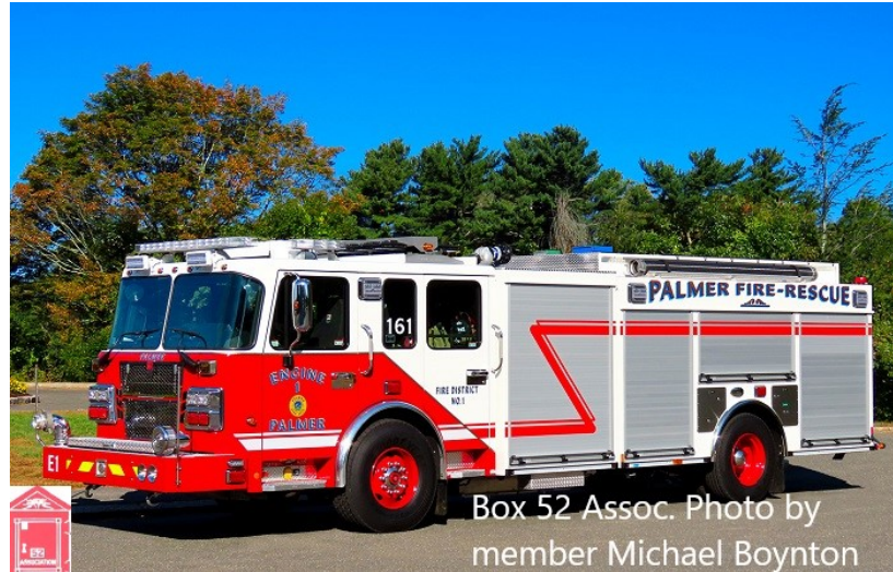
Palmer Engine 1 2020 Spartan/Smeal "Sirius" 1500/1000/20 gallons class A foam.
