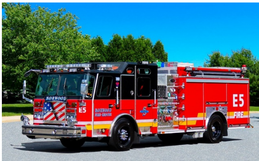
Norwood Engine 5 2020 Emergency-One Cyclone II 1500/730/50 gallons class A foam.
