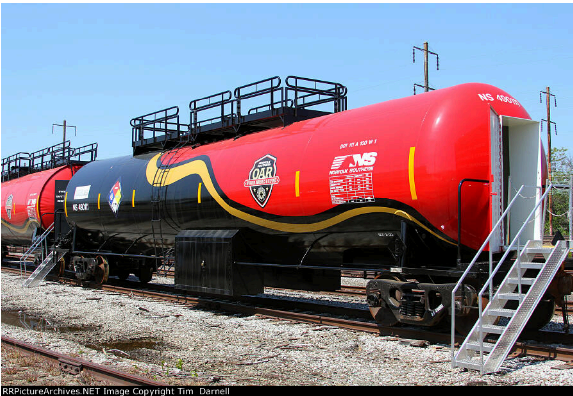
NS OAR Tank Car 490111 set up for a class. The car is designed to carry 30,194 gallon capacity. Photo courtesy of Tim Darnell. RRPicturesArchives.Net
