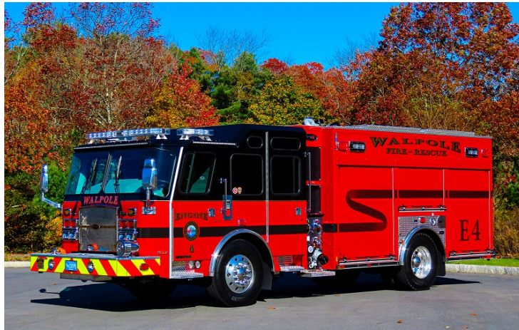
Walpole – Engine 4 - 2019 E-One Typhoon eMax 1500/500/30F. The Department has also taken delivery of a new 2019 E-One Cyclone 2000/270/30A 100 foot rear mounted tower for Tower 1.
