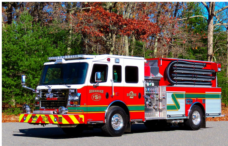
Sherborn – Engine 2 – 2019 Rosenbauer Commander 2000/500/30F w/ 5,000' of 5" LDH. Also received for Engine 6 – 2019 Freightliner/Rosenbauer Timberwolf AWD 1250/1000/30F
