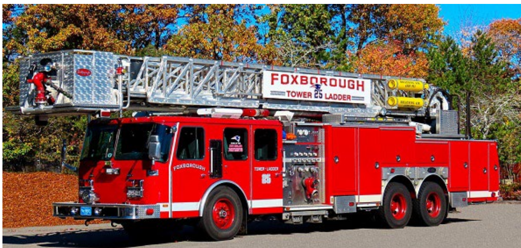
Foxborough Tower Ladder 25 2001 Emergency-One Hurricane 1500/300/95 foot RM. Former Naperville, IL. Truck 5. Obtained 2023.
