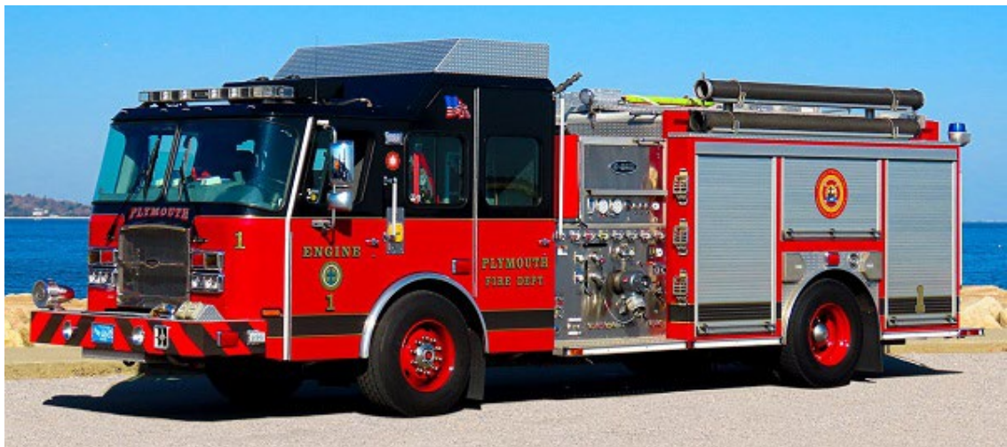
Plymouth Engine 1 2011 Emergency-One Cyclone 1500/750/30 foam. Rehabbed by Greenwood Fire Apparatus 2023.
