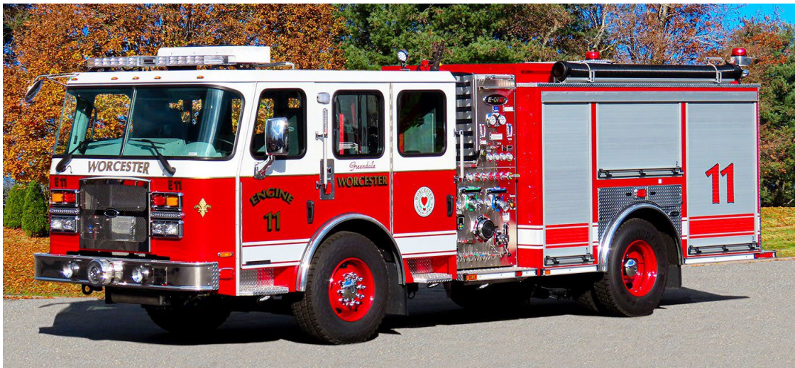
Worcester Engine Companies 11 and 13 received 2023 Emergency-One Typhoon's equipped with 1500 gpm pump, 500 gallon tanks and 30 gallons of class B foam.
