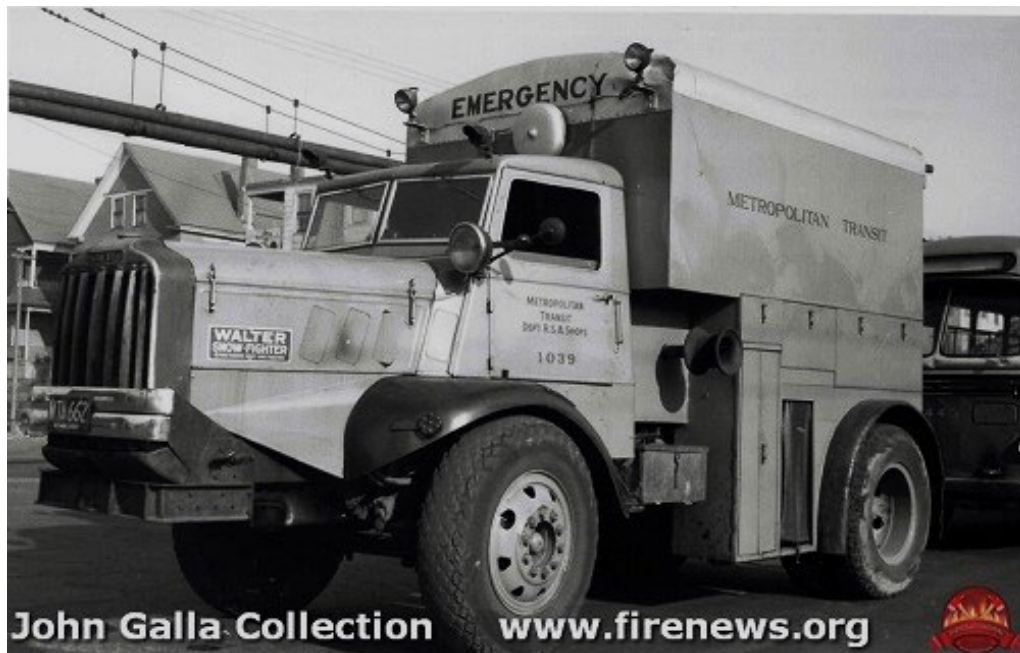
Walter Emergency Truck equipped for towing. Note large emergency bell above the cab.
