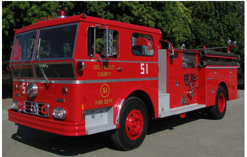
Engine 51 in all her glory! 1971 Ward La France Ambassador Model equipped with a 1,250 pump and a 500 gallon tank. Photo by Member M. Boynton
