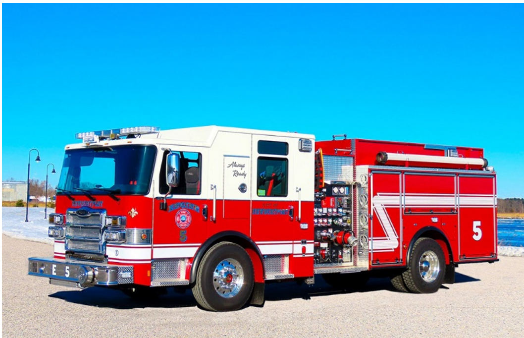
Newburyport Engine 5 has been assigned this 1019 Pierce Enforcer rated at 1500 gpm with a 750 gallon water tank and 30 gallons of Class A Foam.
