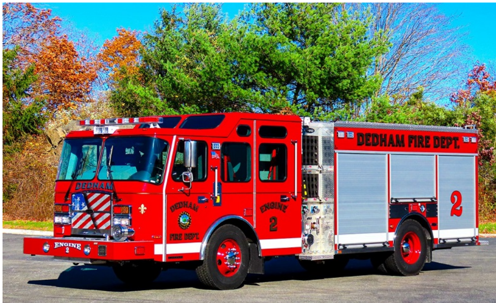
Dedham Engine 2 operates with this handsome 2020 Emergency-One Typhoon eMax equipped with a 1500 gpm pump, 750 gallon tank and 30 gallons of Class A foam.
