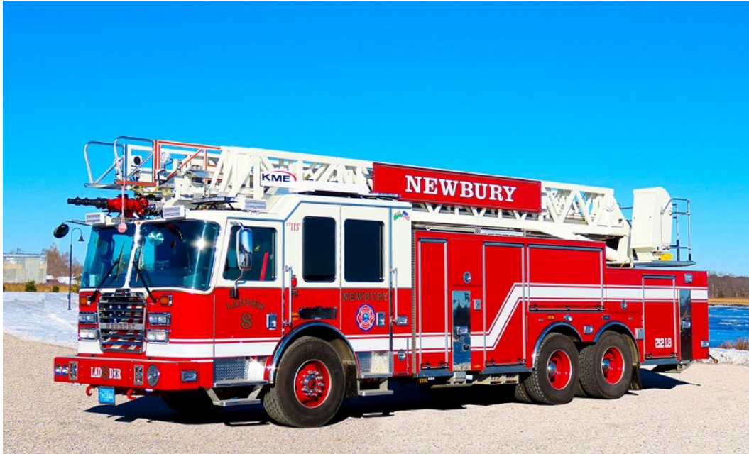
Newbury Ladder 8 is a 2019 KME Panther Tuff Truck with a 103 foot rear mounted aerial.
