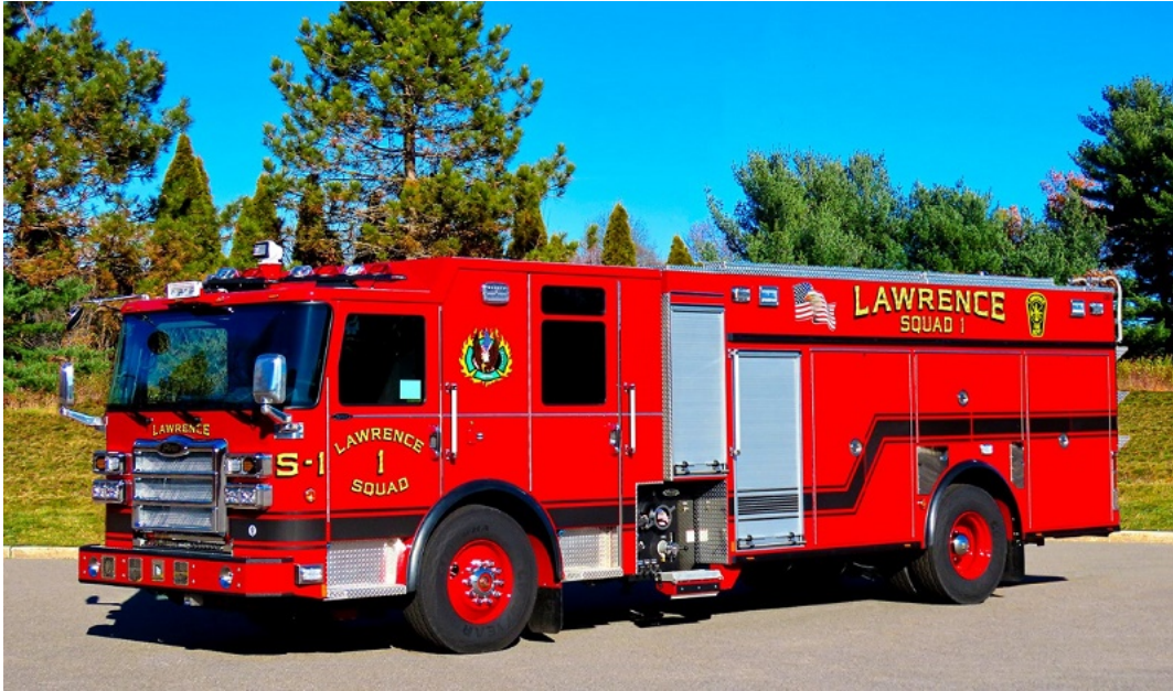
Lawrence has placed Squad 1 in service with this 2020 Pierce Enforcer PUC with a 1500 gpm pump and a 750 gallon tank.
