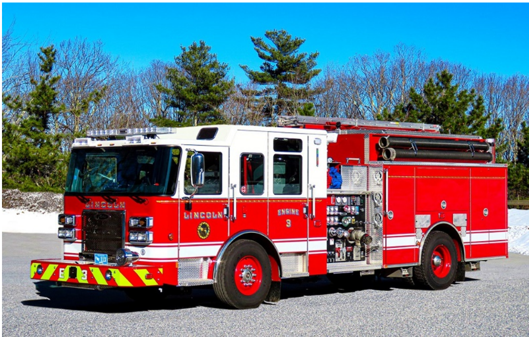
Lincoln Engine 3 is now equipped with a 2019 Pierce Saber pumper rated at 2000 gpm carrying 750 gallons of water and 20 gallons of Class A Foam.
