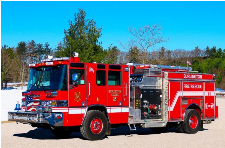
Burlington Engine 2 has placed in service a 2019 Pierce Quantum pump 1500/500/30 Class A Foam.
