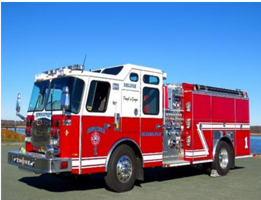
Newburyport – Engine 1 the “ Deluge ” & Engine 2 the “ Mechanic ” 2015 E-One Typhoons 1250/500/30F
