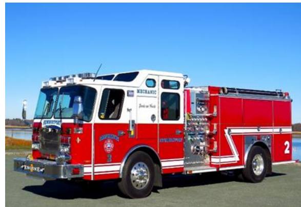
Newburyport – Engine 1 the “ Deluge ” & Engine 2 the “ Mechanic ” 2015 E-One Typhoons 1250/500/30F
