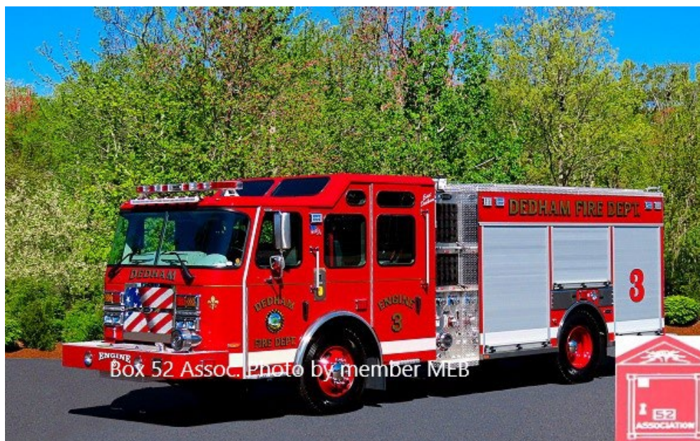
Dedham – Engine 3 – 2022 E-One Typhoon eMAX 1500/750/30A
