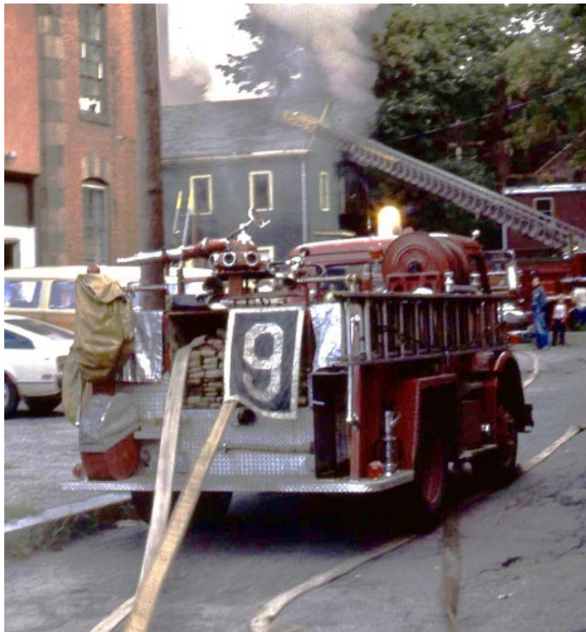
E9 wagon laying in from the pump. The wagons had two beds of 750 feet of 2 1/2 hose on each side.
