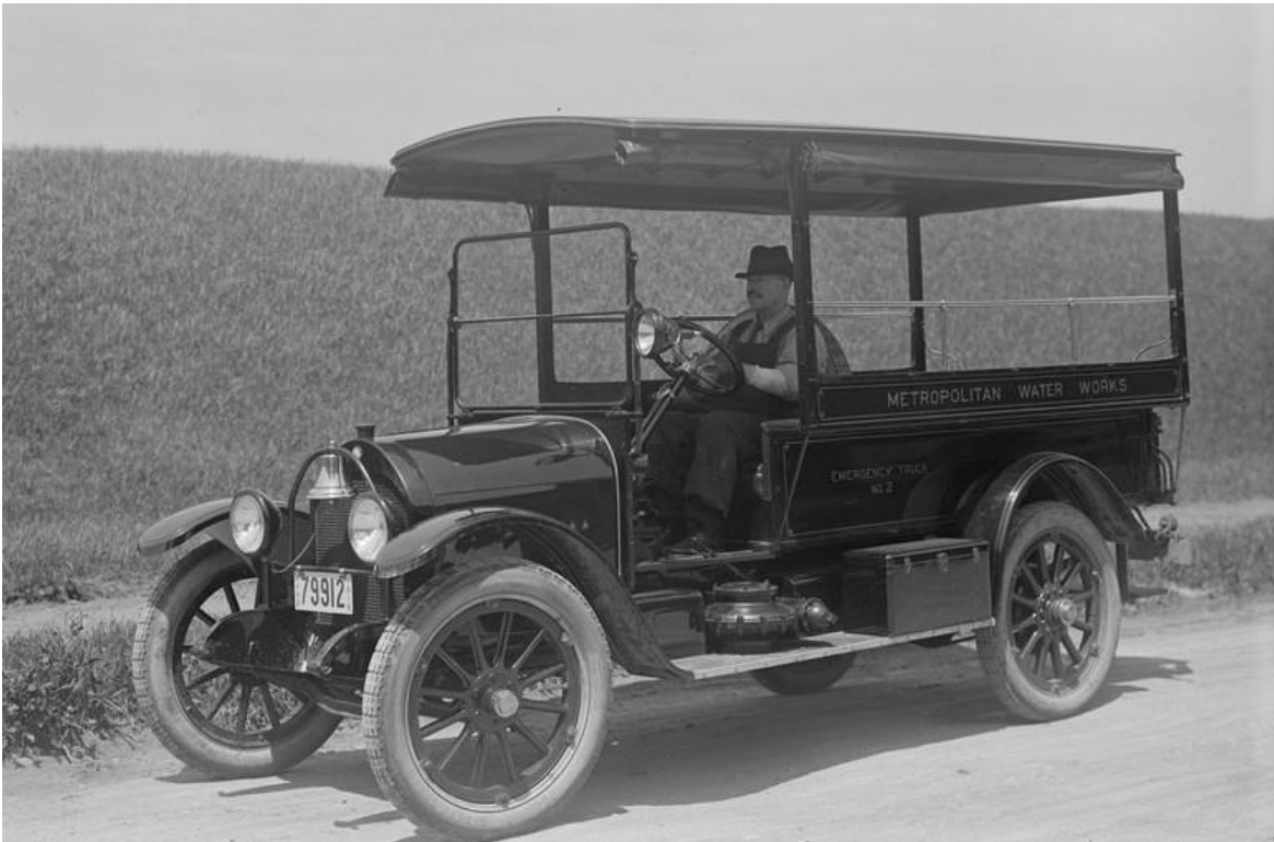
Truck 2 showing the automatic valve under driver. Circa July 1916
