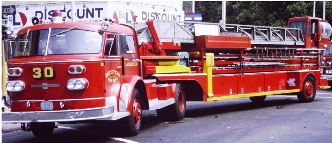
Ladder 30 1970 ALF 100 Ft. TDA. Photo by Member F. San Severino
