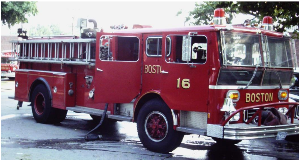
Engine 16's 1976 Ward La France pump with enclosed cab and the familiar plexi-glass covering. Photo by Member F. San Severino
