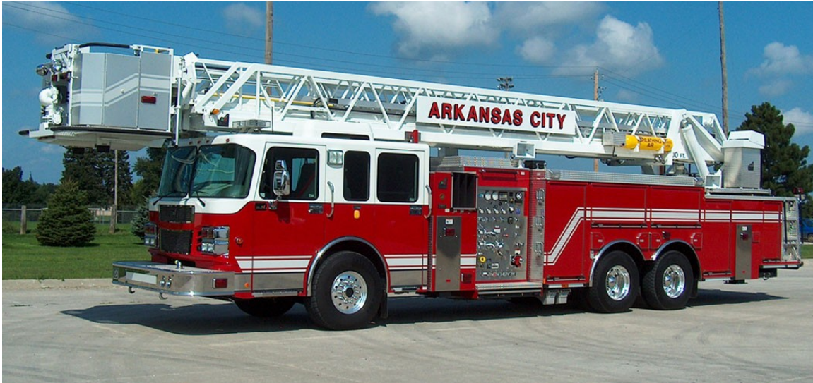
Ark. City 2006 Smeal 100 ft. Tower with a 2000 gpm pump. Photo courtesy of Smeal Fire Apparatus.
