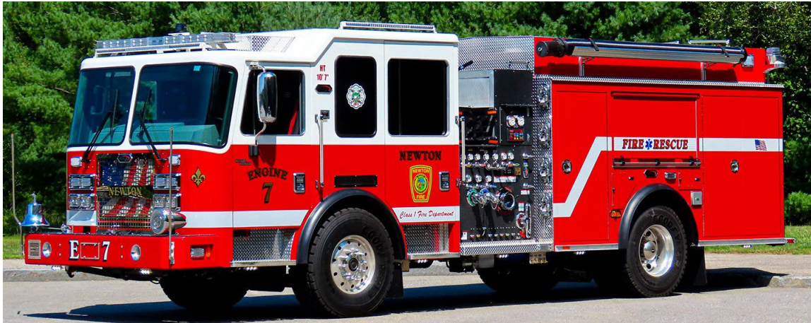
Engine 7 – 2025 KME Severe Service 1500/750
