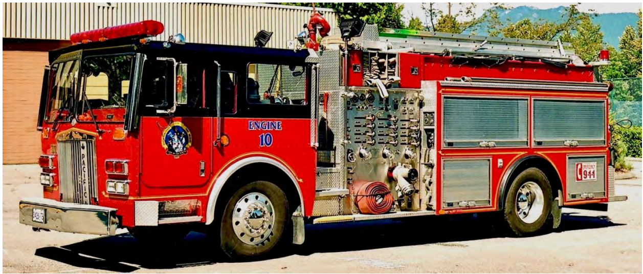
City of North Vancouver E 10, a 1989 Pacific PFC410: 1750igpmp ump/300gwt/45gft
