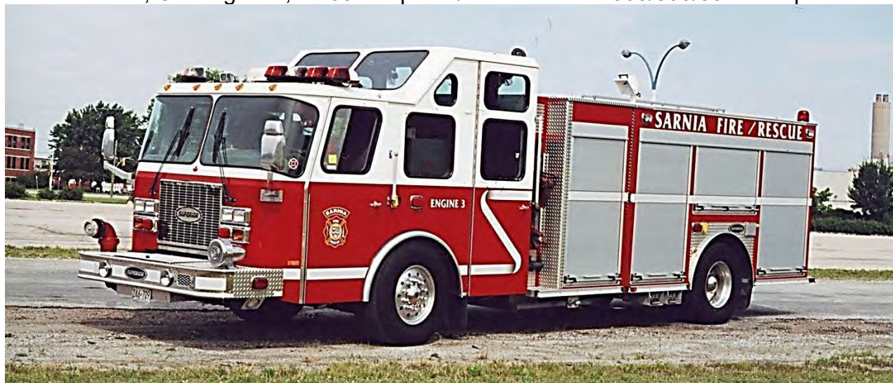
Sarnia, ON Engine 3, 1999 Superior/E-One Cyclone II Rescue Pumper 1500/500/20A/30B.
