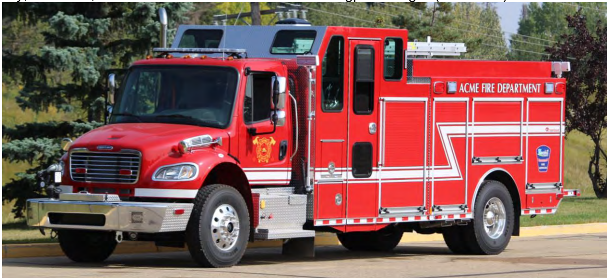
Acme, AB now has a 2020 Freightliner M2 106/Rosenbauer TME, 1100igpm/900gwt/20gft.
