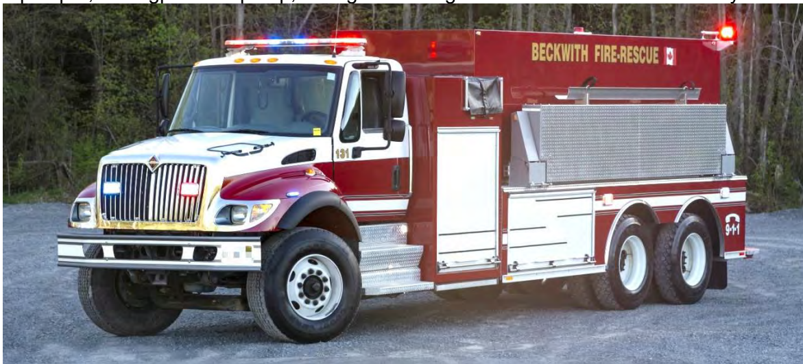
Beckwith Twp., ON 131 is a 2020 Battleshell remount of a Carl Thibault pumper/tanker on a 2003 International 7400 chassis with a 1250igpm pump (Chassis and pump ex-Arnprior Fire Department) (Battleshell Industries photos)
