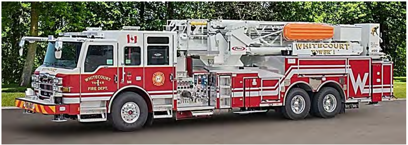
Whitecourt, AB, a 2020 Pierce Velocity 1665igpm/230gwt/20gft Ascendant 100' tower. (Pierce photo)
