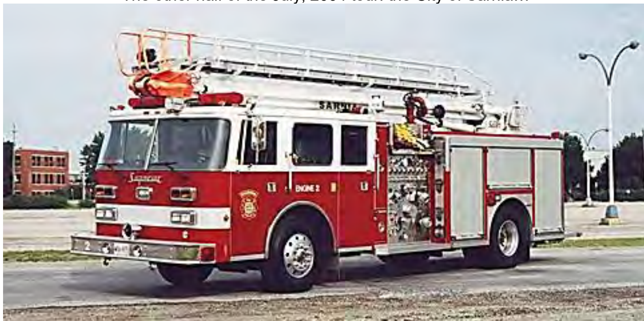
Sarnia, ON Engine 2, a 1992 Superior/Pierce Arrow 1500/500/50' TeleSquirt
