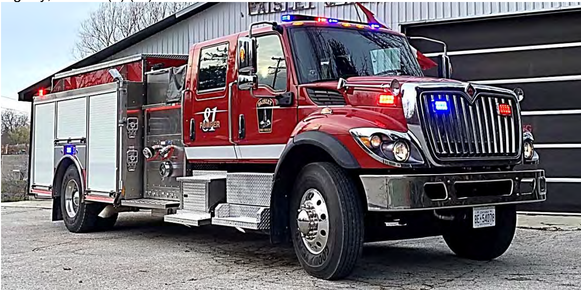
Paisley, ON P.81, a 2020 International HV607 / HME Ahrens-Fox 1250igpm(W)/833gwt (DEV)
