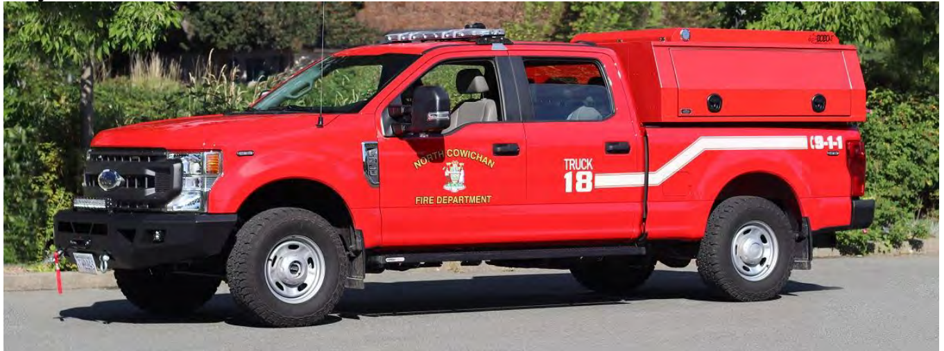
North Cowichan, BC Truck 18, a 2020 Ford F-350 / Express Custom skid, 18HP pump/150igwt.
