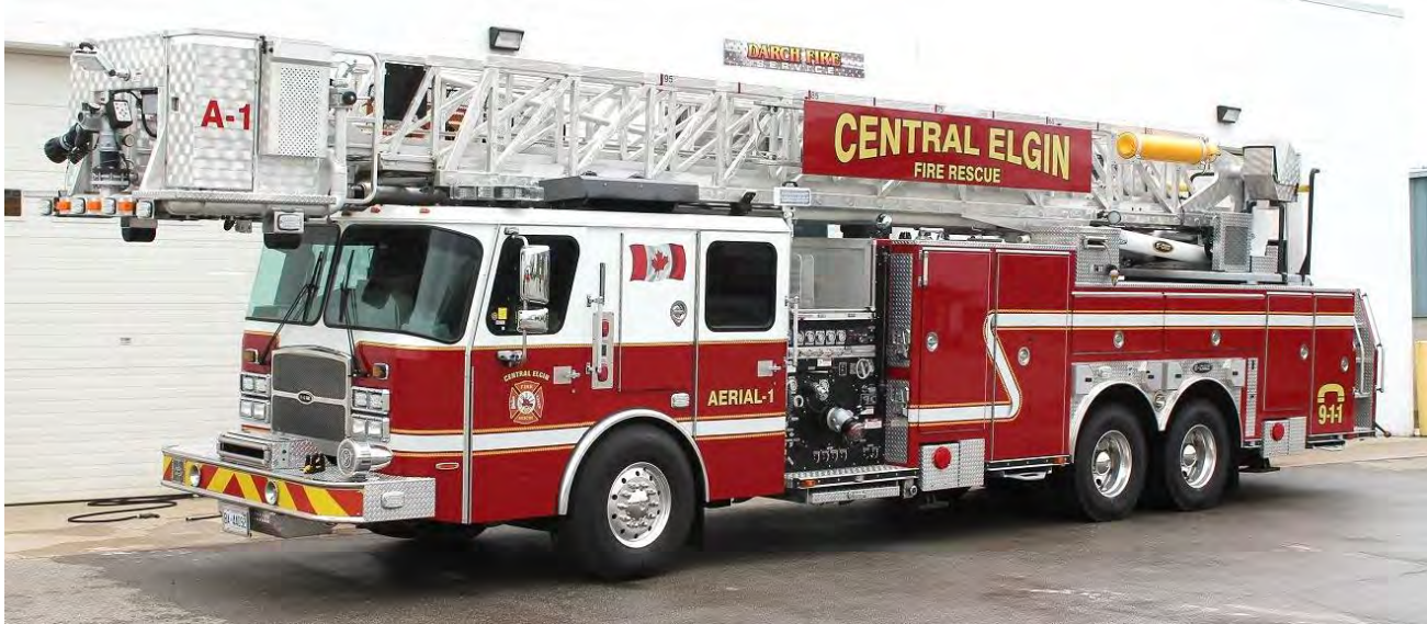
Central Elgin bought this 2014 E-One Cyclone II 95' tower from Brindlee Mountain late last year. It features a 1750gpm Hale pump and a 500gwt. It is assigned as Aerial 1 in Port Stanley. (Gary Dinkel photo)
