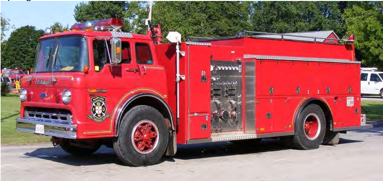
Engine 4 (Shwoob) 1987 Ford C/Thibault pumper, 840igpm/800gwt. (SN#T88-102)
