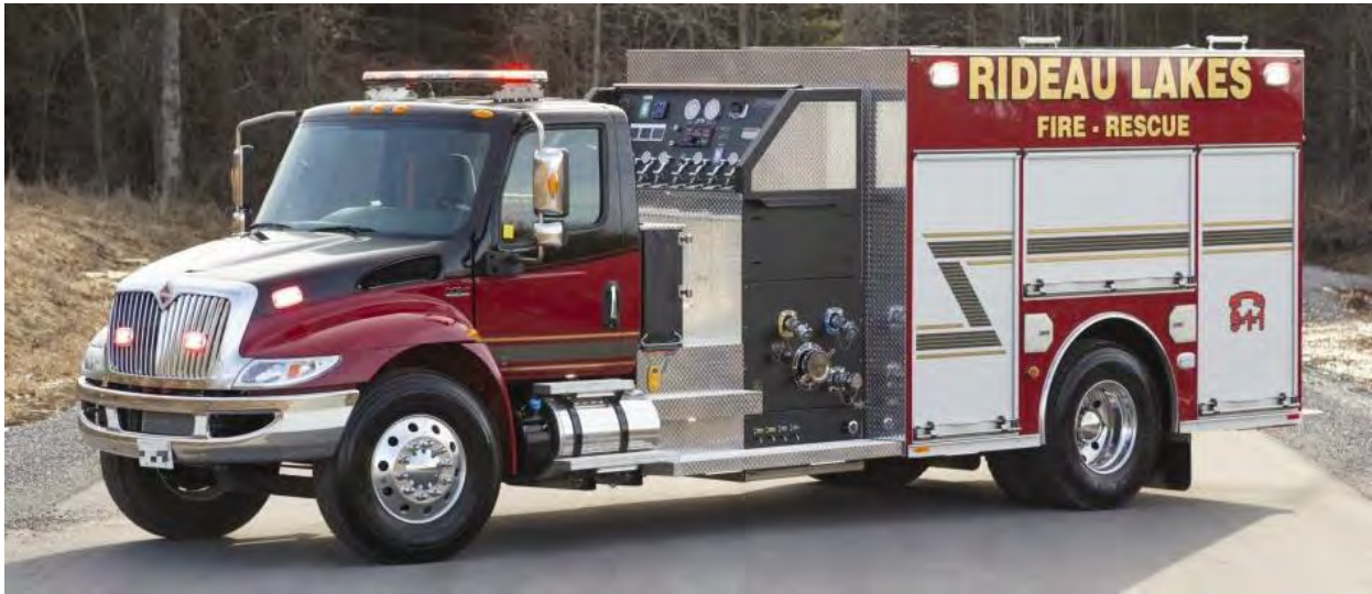
Earlier this year, Rideau Lakes, ON acquired this 2019 International MV607/ Battleshell pumper, 1050igpm Hale pump, 1000gwt and 35gft with a FoamPro 2001 foam system.
