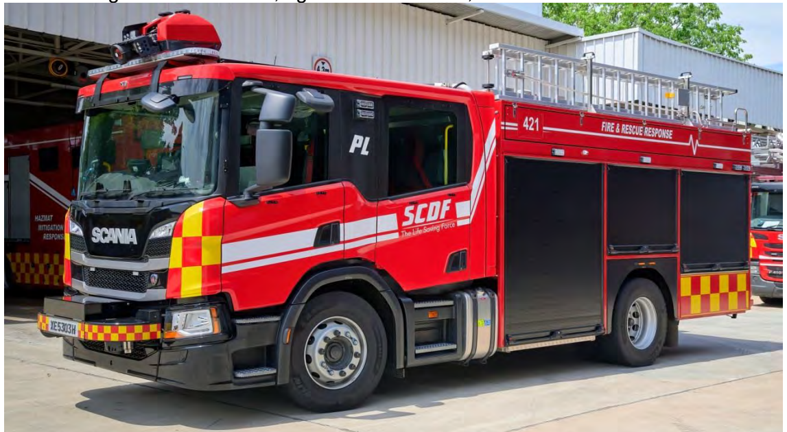
This is a 5 th generation pump-ladder. PL421 also runs from Tuas Fire Station. Built on a Scania P320 chassis by Rosenbauer, it has a 4000LPM pump, 2400GFT, and 1200LFT. (Kenneth Lai photos)
