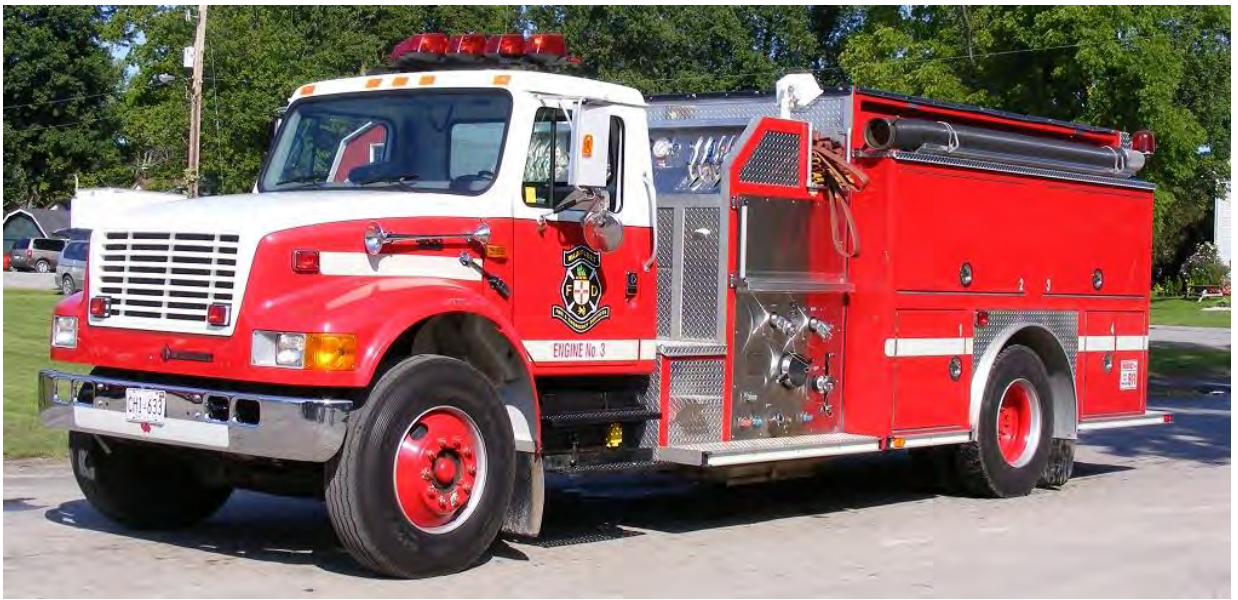
Engine 3 - 1999 International / Superior pumper, 1050igpm/900gwt. (SN#SE 1957)
