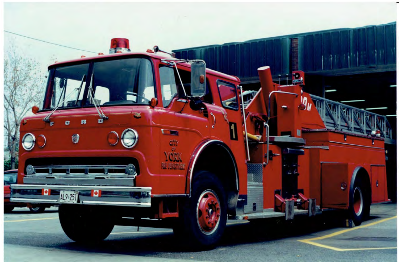
Aerial No. 1, at Station 1, ran this 1974 Ford/Pierreville 100' aerial, it had a 100 IGPM pump and 100 GWT. (Photos courtesy Ken Walton)
