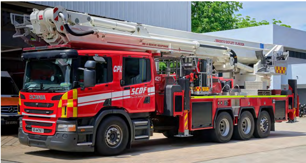
CPL 421 is a Scania P410/Bronto Skylift FL60XR (195') tower with a 4000LPM pump.
