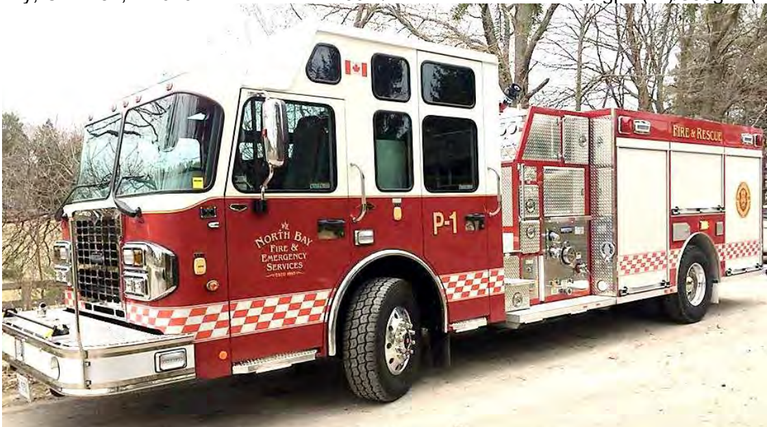
North Bay Pump 1, a 2020 Spartan Metro Star / Metalfab 1250igpm/800gwt/20gft
