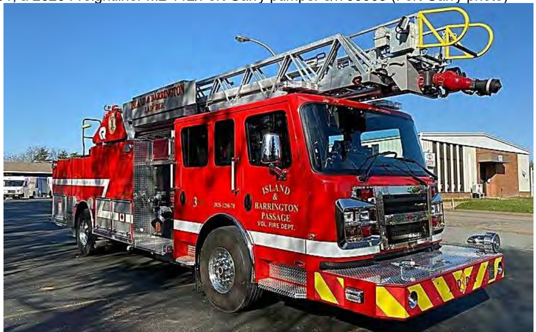
Island & Barrington Passage, NS Ladder 3, a 2020 Rosenbauer Warrior 1250/400/20F/78' Viper aerial.
