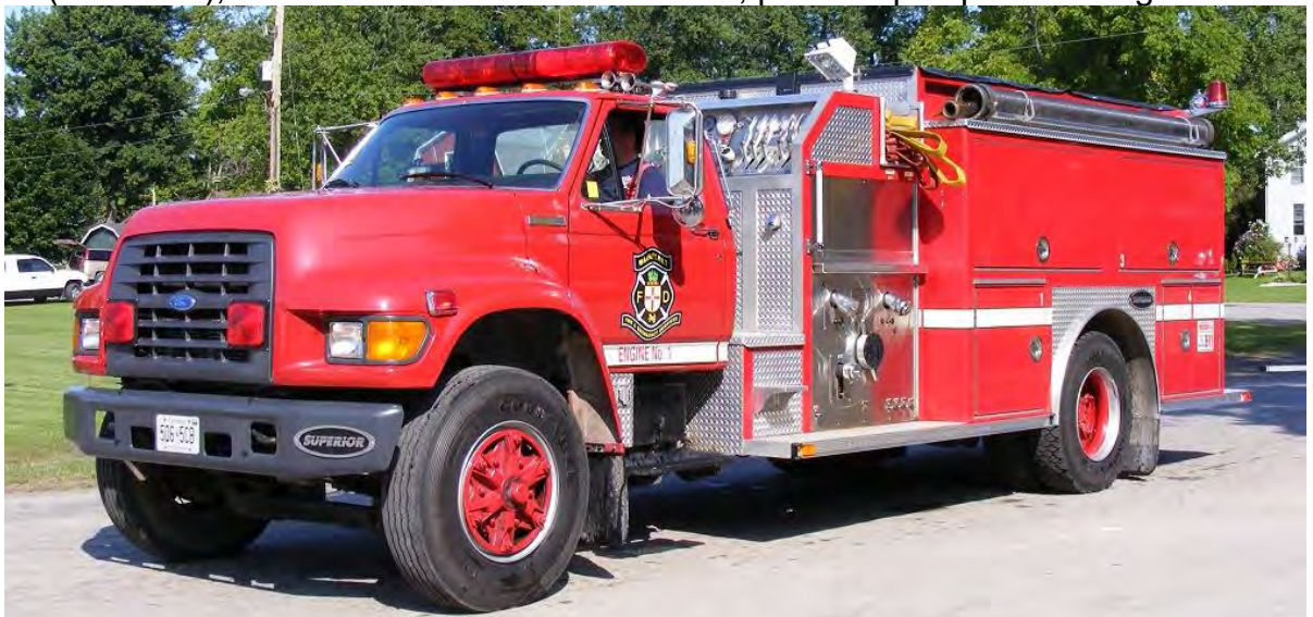
Engine 1 (Winger), a 1996 Ford F-800 / Superior pumper 1050igpm/1000gwt. (SN#SE 1700)
