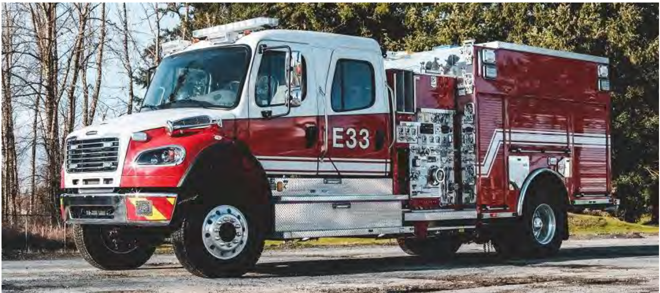
West Kelowna, BC E.33 West Kelowna, BC Engines 33 and 34 are both 2019 Freightliner M2-106 4x4/Smeal pumpers with 1050igpm pumps, 800gwts and 40gfts.
