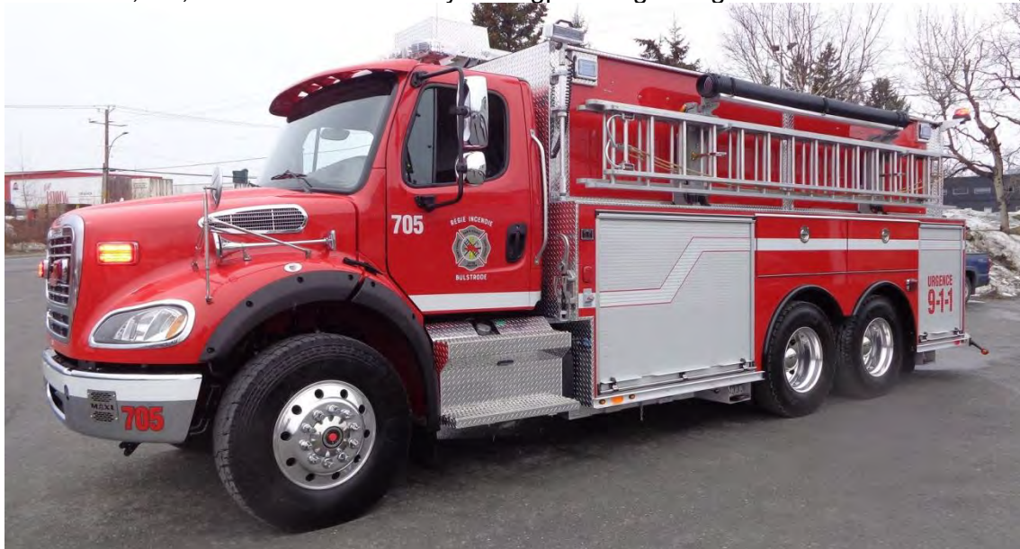
Bulstrode, QC Unité 705, a 2020 Freightliner M2 112/Maxi Métal pumper/tanker, 1050/2500/40.
