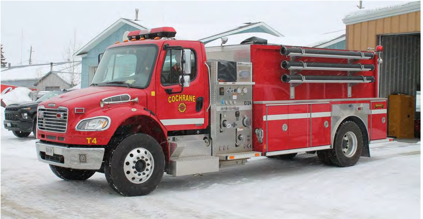
Tanker 4 a 2008 Freightliner M2 106 / E-One tanker, 420igpm/1540gwt
