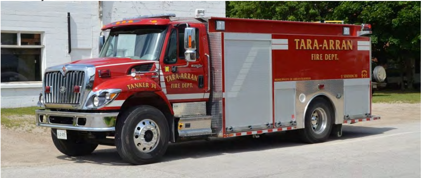
Tara-Arran, ON Tanker 74, a 2010 International 7400/Dependable with a portable pump and 1800igwt.
