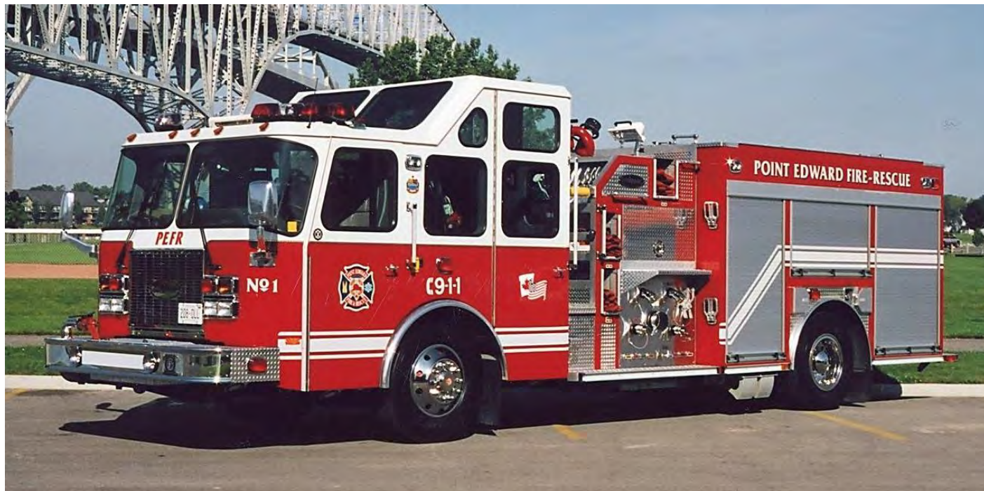
Point Edward, ON Pumper #1, a 2002 Spartan/Superior 1500igpm/500gwt/50gwt SN SE2821
