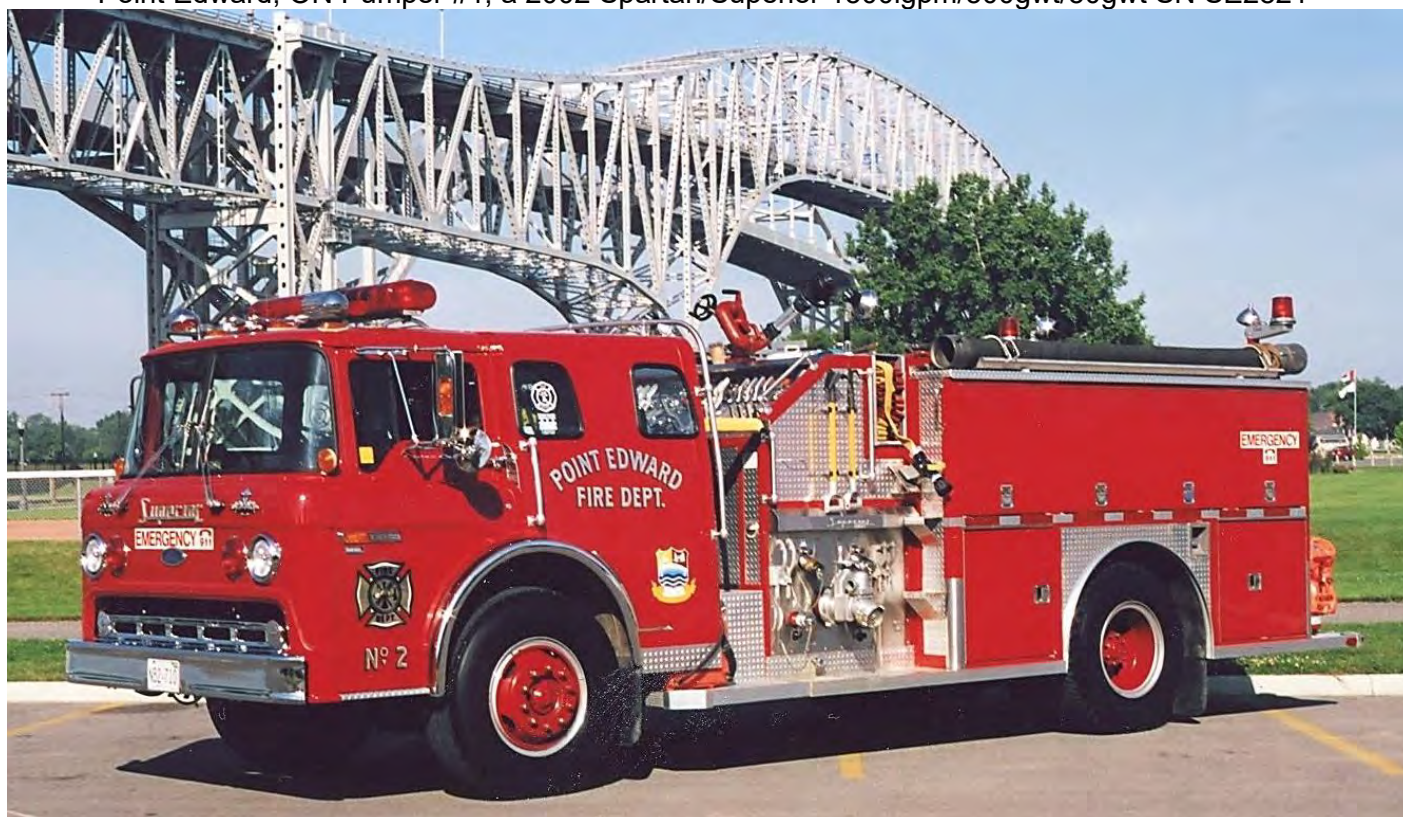
Point Edward, ON Pumper #2, a 1987 Superior/Ford 8000 1050igpm/700gwt. (Larry Ward photos)
