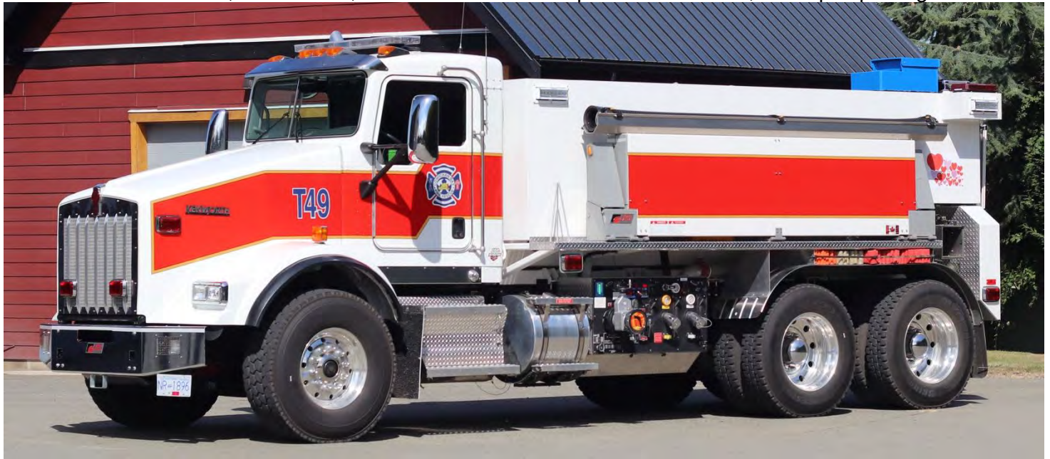
Cowichan Bay, BC Tender 49, a 2020 Kenworth T800/Fort Garry pumper-tanker, 1050igpmPTO/2500gwt. (Shane MacKichan photos)
