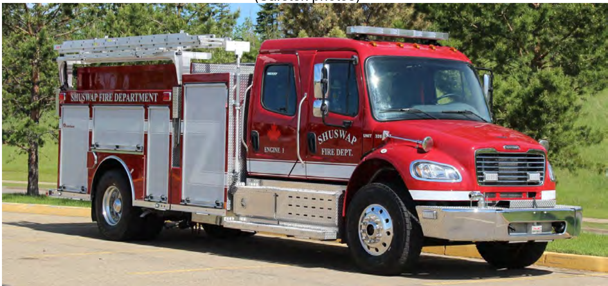
Shuswap, BC (Sorrento) P.1, 2020 Freightliner M2 106 / Rosenbauer 1050igpm/1000gwt/20gft E.1 (RMP)
