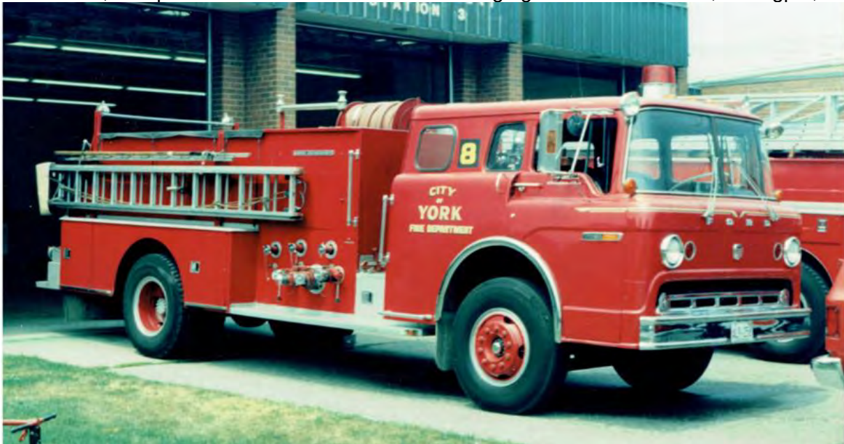
At the time, Pumper 3 had this 1973 Ford C-900 / King pumper, 1050 IGPM 500.
