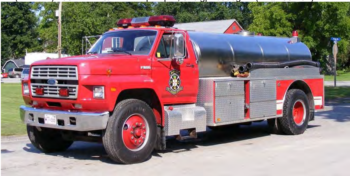
Tanker 1 (Wainfleet), a 1990 Ford F-800/Smeal tanker, portable pump and 1500gwt.
