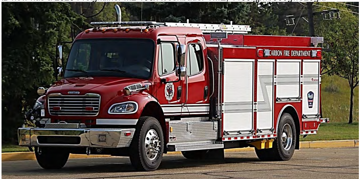
Carbon, also in Kneehill County, AB received a 2020 Freightliner M2 106/Rosenbauer rig, with an 1100igpm pump, 900gwt and 20gft. (Photos courtesy Rocky Mountain Phoenix)
