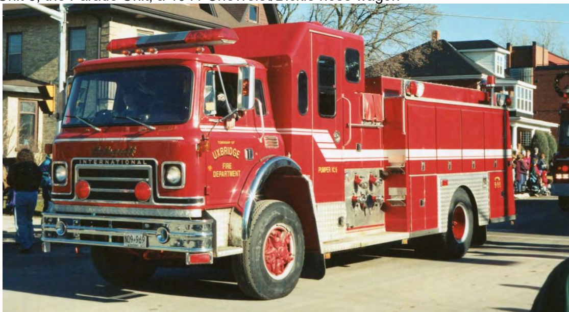
Uxbridge Unit 6, a 1987 International CO1950B/Thibault, 840igpm pump/750gwt
