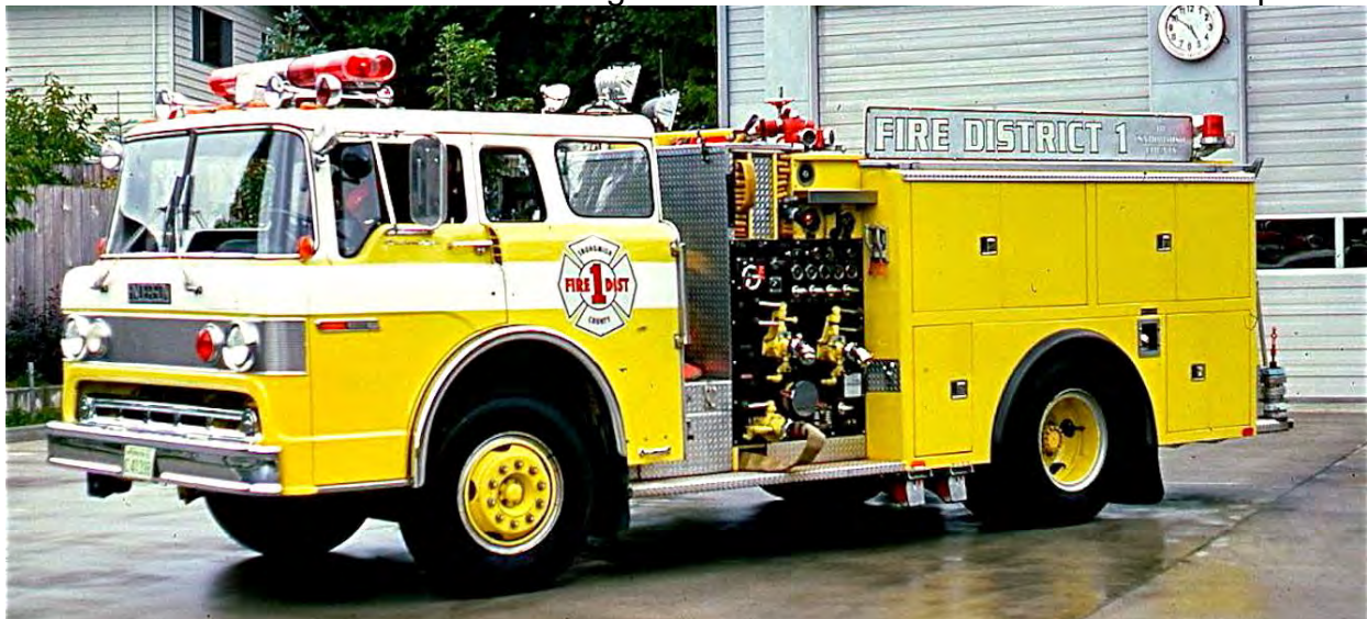
Snohomish County Fire District 1 in Washington State (1 of 2 built) 1982 build using a fire department supplied 1974 Ford C chassis, 840igpm/500gwt.
