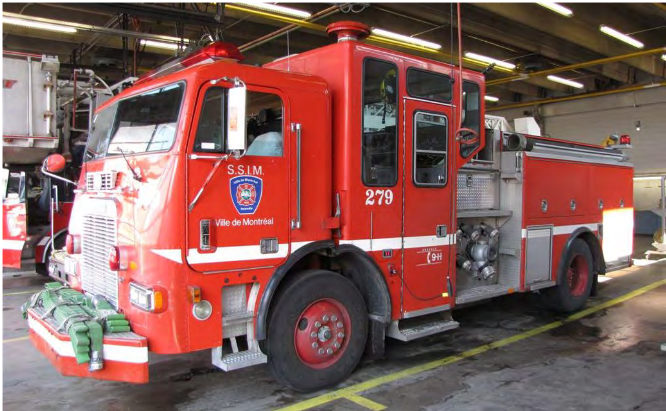
Autopompe 279, a 1992 Freightliner FLL6342S / Anderson pumper, 1050igpm/500gwt.
