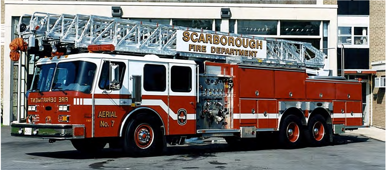
Scarborough, ON Aerial 7, a 1990 E One Hurricane quint, 1050igpm pump, 160gwt and 110' stick.
