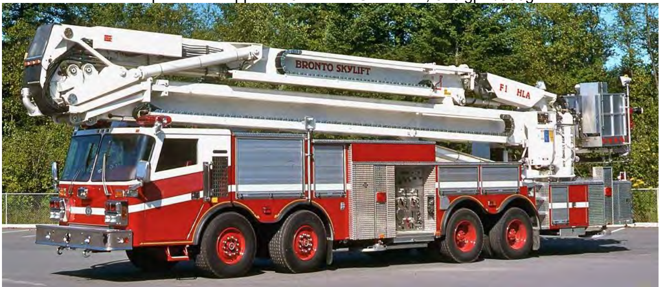
During 1994 AE supplied this Simon Duplex D9681 truck with 1050 GPM pump and 50 M Bronto to the Island Nation of Guam. No water or foam on this truck though.
