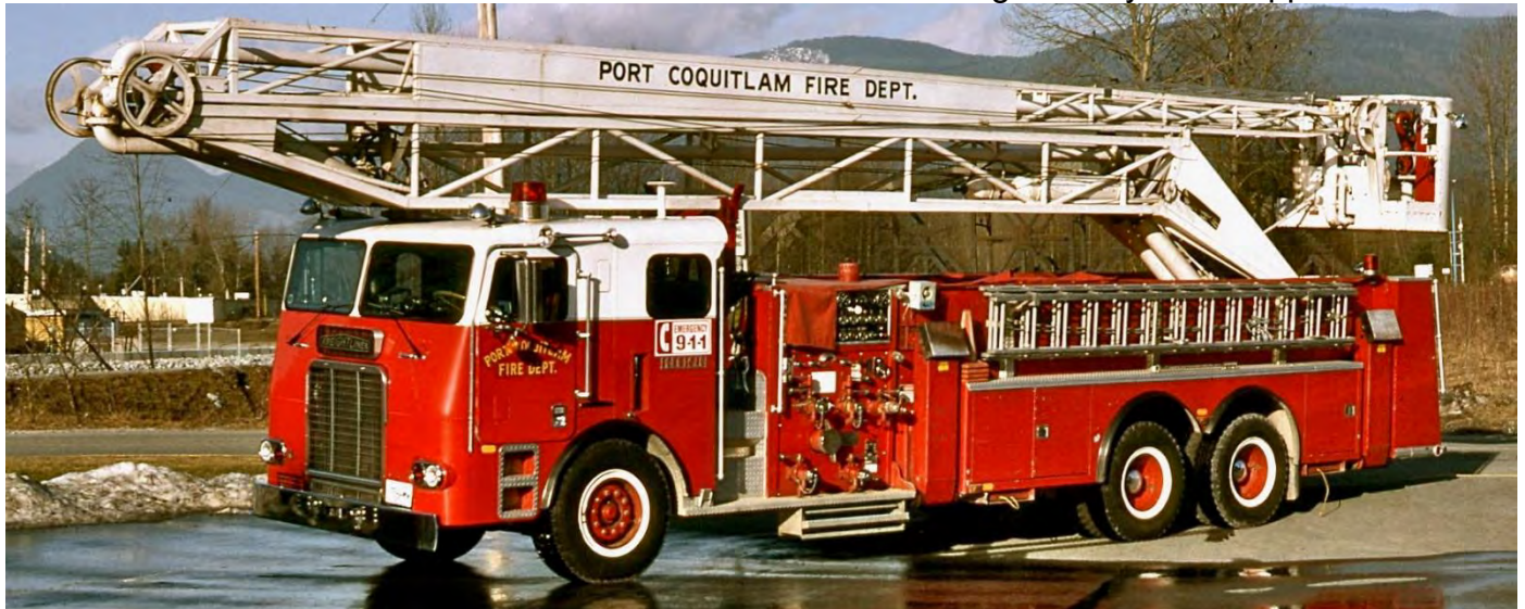
80' High Ranger platform for Port Coquitlam on a 1980 Freightliner FLL chassis that included a 1050 pump and 250 gallon water tank.
