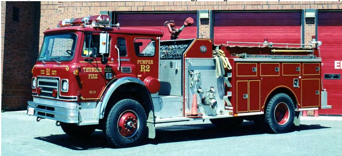
Thunder Bay ON Pumper R2, a 1985 Anderson Int'l CO1950B 1050igpm/500gwt, the first apparatus sold in Ontario. (Dave Stewardson photo)
