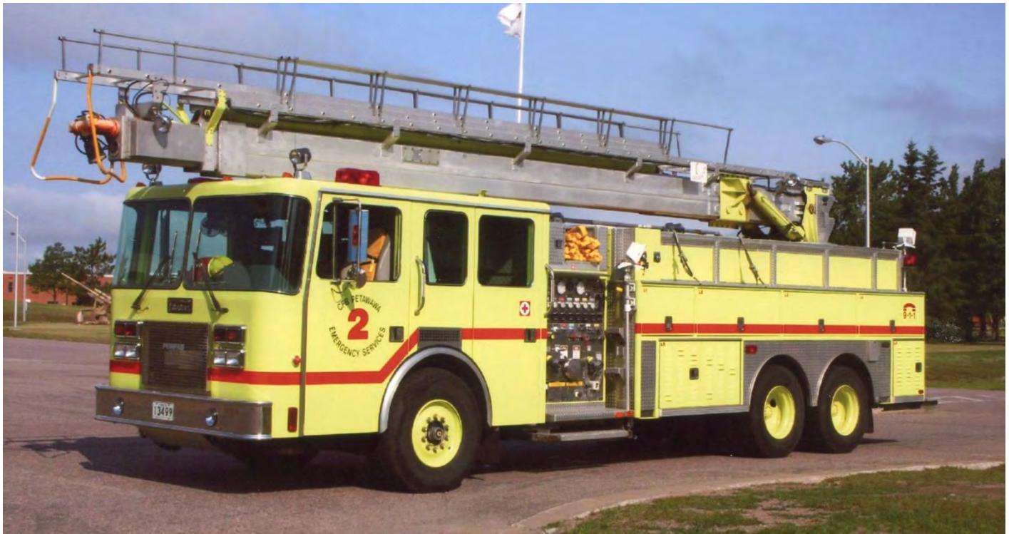
Assigned to Station 1, this old Red 2, a 1996 Pemfab T964/Tibotrac quint, equipped with a 1050igpm pump, a , 500gwt and a 75' aerial.
