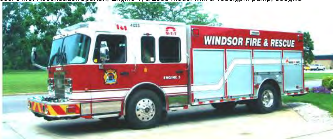
Engine 3 (now Engine 2), a 2010 Rosenbauer/Spartan, 1050igpm/600gwt.
