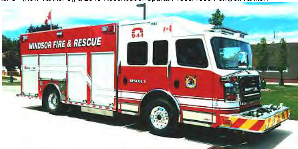
Rescue 3, a 2017 Rosenbauer/Commander 500/500 Rescue/Pumper.
