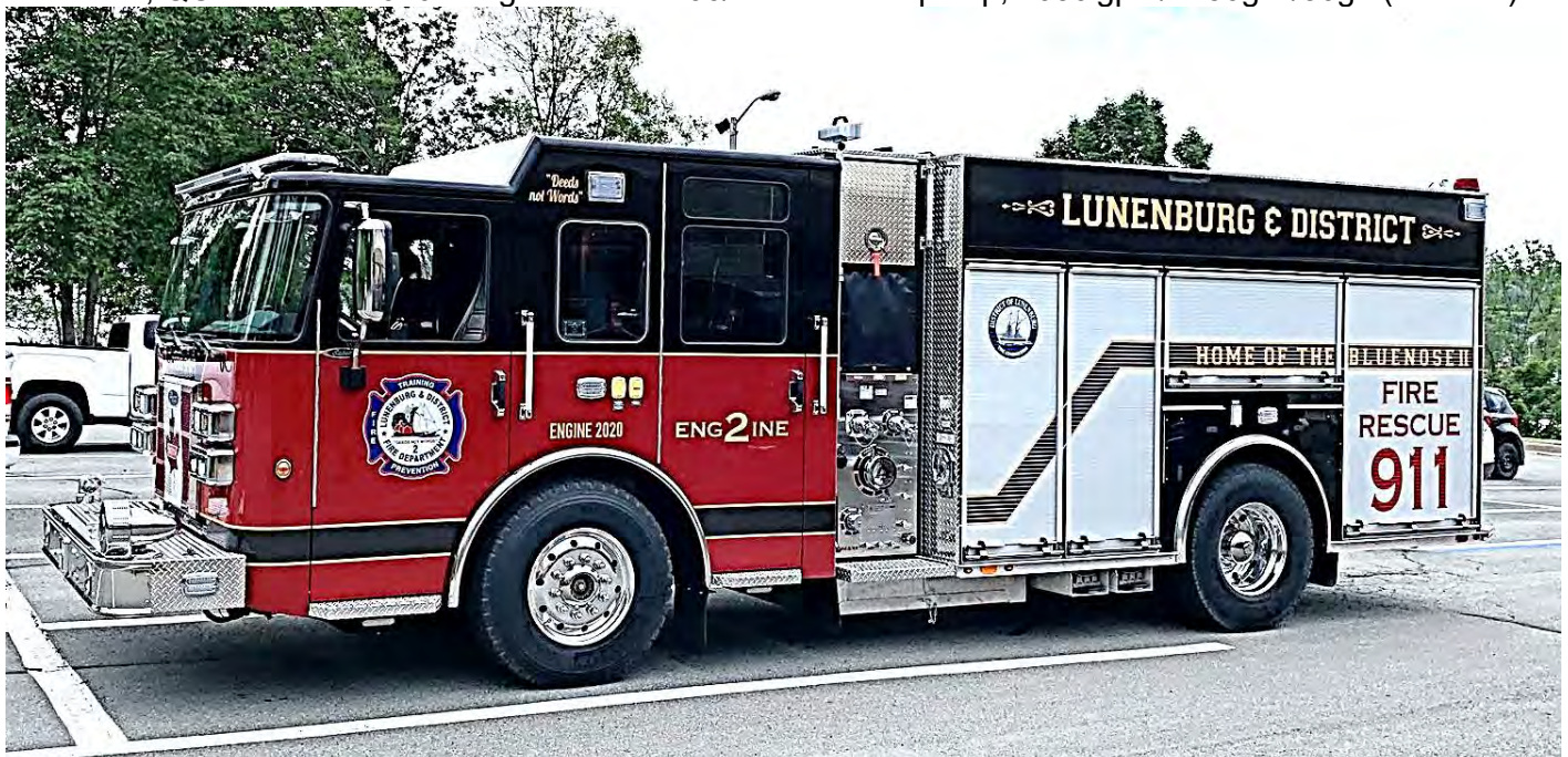
Lunenburg, NS Engine 2, a 2020 Pierce Maxi-Saber, 1500gpm pump, 1500gwt (Will Brooks photo)
