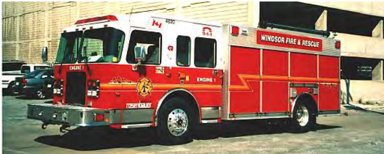
Windsor's first Rosenbauer/Spartan, Engine 1, a 2003 model with a 1050igpm pump, 500gwt.
