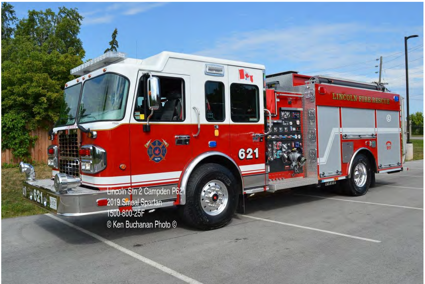
Delivered last year, this is Lincoln, ON Pump 621 in Campden. The 2019 Spartan Metro Star/Smeal pumper has a 1500igpm pump, 800gwt and 25gft. (Ken Buchanan photo)
