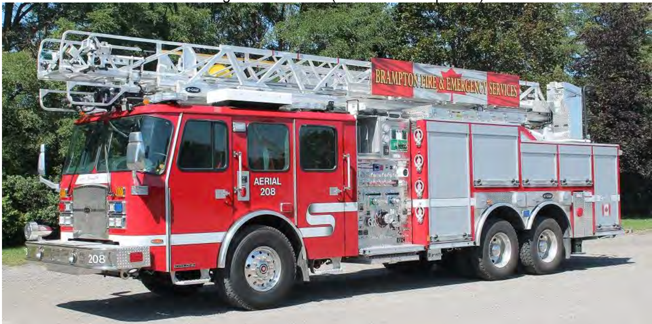
Brampton's new Aerial 208, a 2020 E-One Cyclone, 1103igpm/400gwt/17gft/78' s/n 142512 (Gary Dinkel photo)
