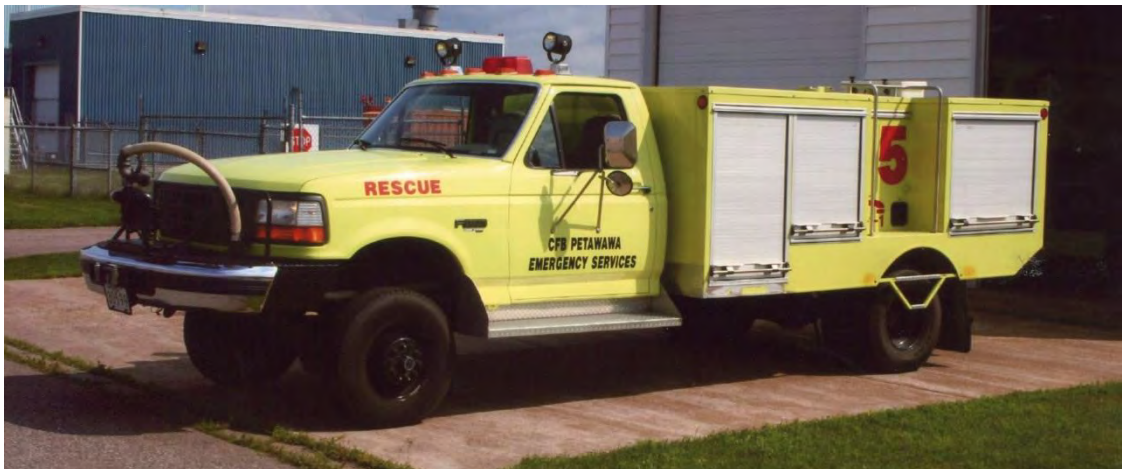
Rescue 5, a 1997 Ford F450/Davtair rapid response with a 250igpm pump, 225gwt and 15gft with 200lbs PK.
