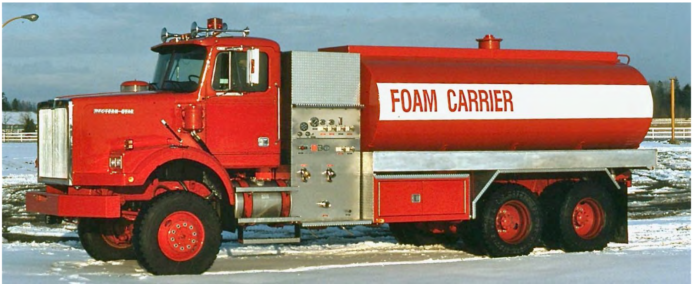
1This is a 1994 Western Star Bulk Foam carrier that was sent to Kuwait It had a 500 GPM transfer pump and 3000 gallon foam tank.
