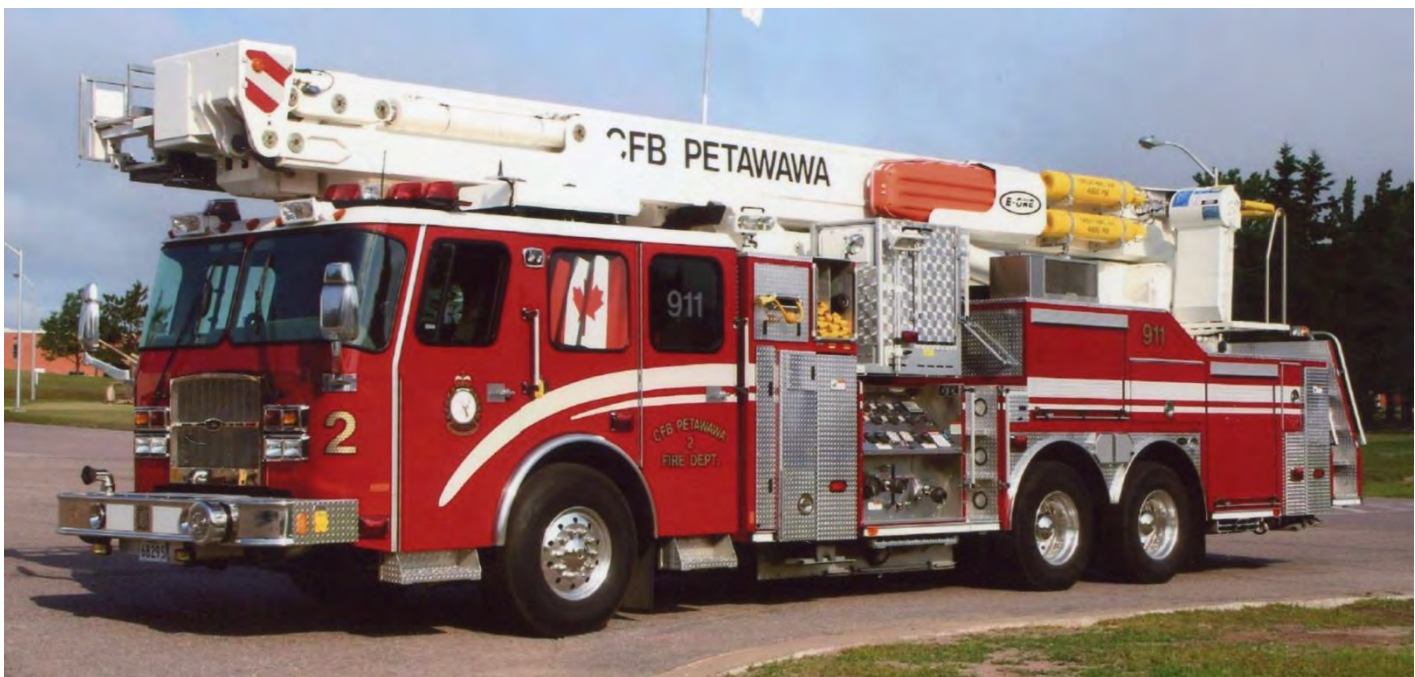
The new Red 2, still in service, a 2006 E-One Cyclone II/Bronto with a 1750igpm pump, 3500gwt, 45gft and 114' tower. This is the typical aerial device now in use at most DND facilities. (Dean Nickerson photos)
