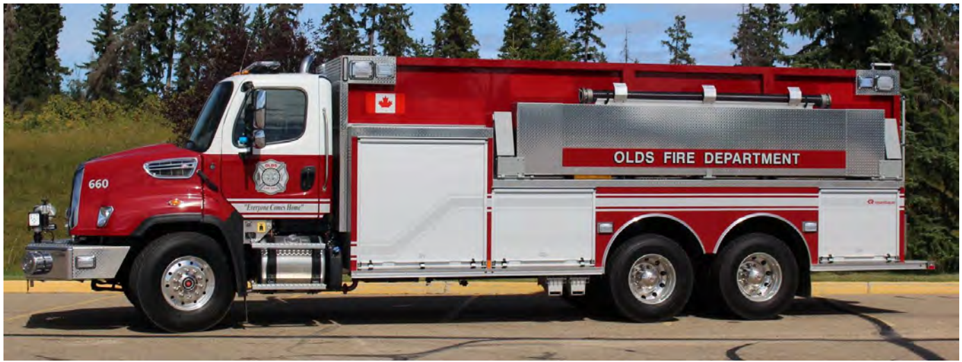
Olds, AB Tender 660, a 2020 Freightliner 108SD/ Rosenbauer tanker, 625igpm/3260gwt. (Olds FD photo)
