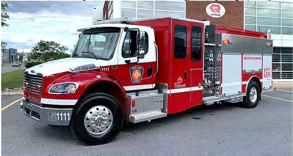
Prévost, QC 1111 is a 2020 Freightliner M2 106/Rosenbauer pump, 1050igpm/1250gwt/30gft (Aerofeu)
