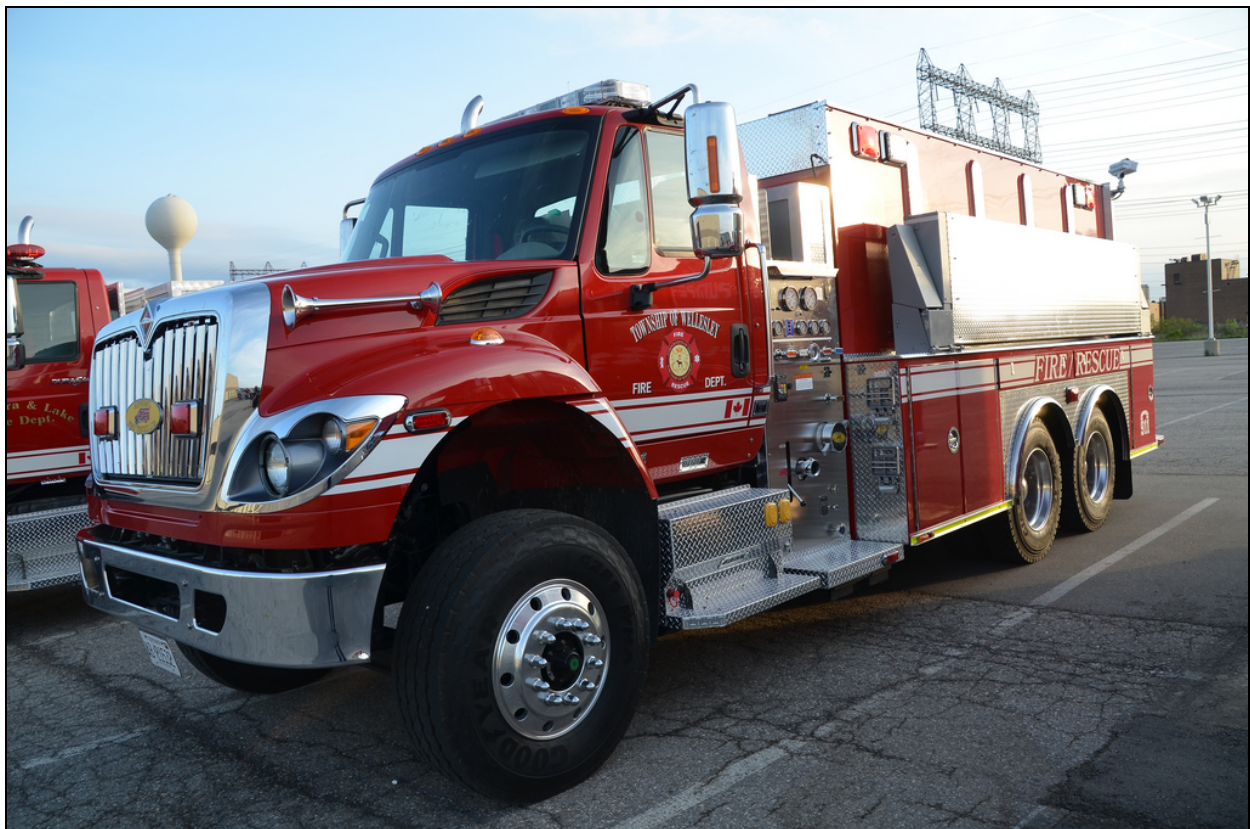
Delivered last year: St. Mary' tanker, a 2012 Freightliner M2/Rosenbauer with a 420igpm pump and 1800gwt, (SN#2102012) and Wellesley Twp. Tanker 3, a 2500 gallon job from Asphodel on a 2012 IHC 7500 chassis. Tanker 1 (Linwood), bought in 2010, is the same. (Larry Thorne photos)
