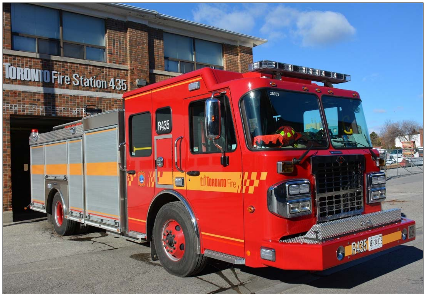
One of 12 new Spartan ERV pumps delivered to Toronto, 11 of which are rescue-pumps. All are on 2013 Spartan Metro Star chassis with 2000gpm pumps with 500gwt. (Larry Thorne photo)
