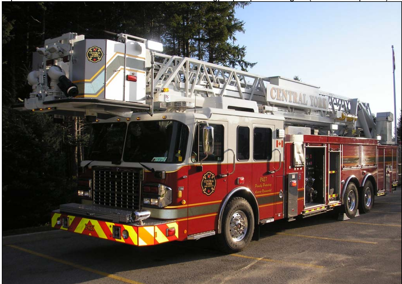
Two of several Smeal units acquired by Central York Fire, these aerials are A436, a 2012 Spartan Gladiator/Smeal 105' rear-mount with a 2000gpm pump and 300gwt, and Platform 427, a 2013 Spartan Gladiator/Smeal 100' rear-mount with a 2000gpm pump and 300gwt. (Rod Bruton photos)
