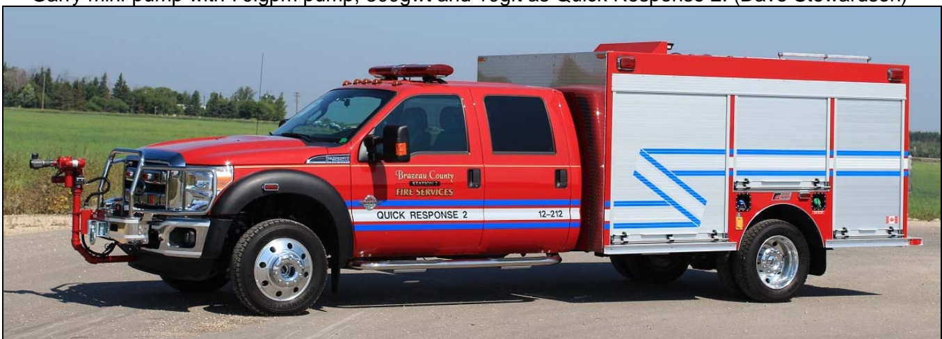
Above is Otter Point's all white 2013 Hub/Spartan Metro Star pump, with a 1050igpm pump, 1025gwt, and twin 25gfts, delivered in July. Below, Brazeau County is now running this 2013 Ford F550/Fort Garry mini-pump with 70igpm pump, 300gwt and 10gft as Quick Response 2. (Dave Stewardson)
