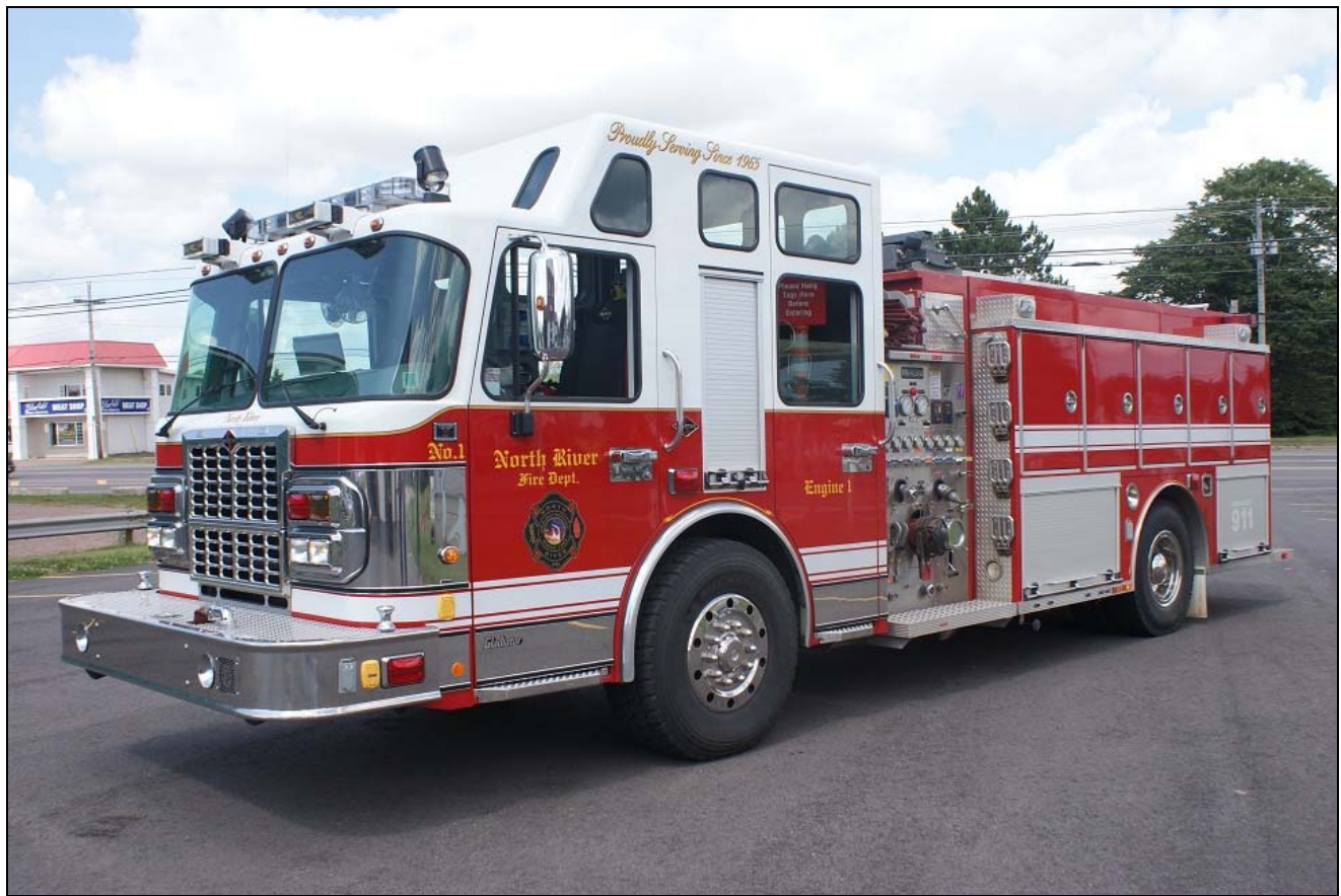
From the PEI Tour are North River Pumper 1, a 2010 Spartan Gladiator/Metalfab with 1250igpm /1000gwt/2x30gft , and TRU 2, a 1996 Spartan/Tri Star Tactical Response unit. (Ken Buchanan)
