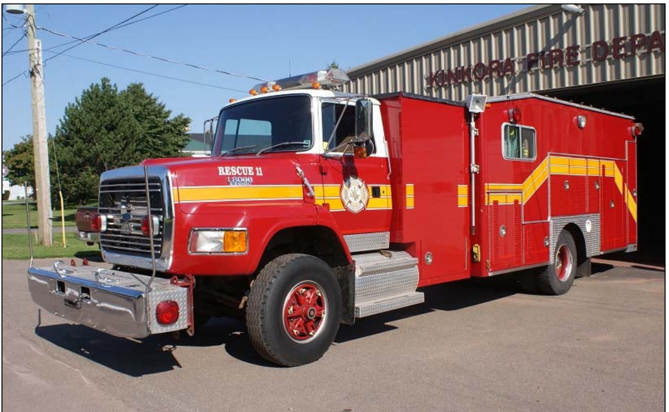
Some of the unique or unusual apparatus found on PEI, this pair in Kinkora. Rescue 11 is a 1990 Ford L8000/Dependable rig, originally purchased by Ancaster. Tanker 9 is a 1989 IHC/Hub product with an 840igpm pump and 2500gwt, formerly with Yarmouth #2 in Ontario. (Ken Buchanan photos)
