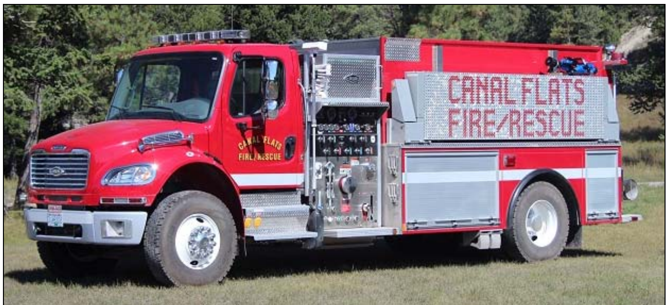
Canal Flats, BC runs this 2011 Freightliner M2/Hub pump with an 840igpm, a 1600gwt and foam as P.1, also a rescue on a 1990 Chevrolet Silverado chassis with a box from the Beasley FD added later.
