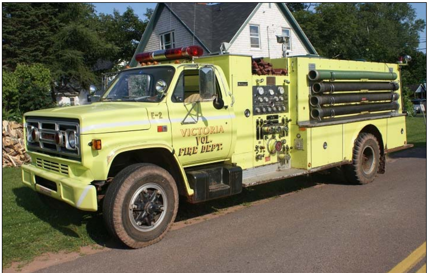
Victoria's 1996 GMC/Remco ex-ambulance, resplendent in black. Below is Victoria Engine 2, a 1983 GMC/Middlesex pumper/tanker with a 1000gpm pump and 1500gwt. (Ken Buchanan photo)
