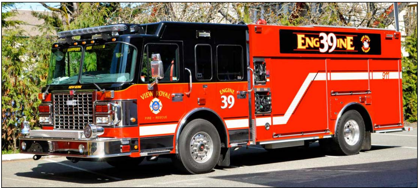
This is View Royal, BC Engine 39, a 2012 Spartan/Smeal pumper with a 1522igpm pump, 600gwt and 25gft. It features black over red graphics. (Terry Yip photo)
