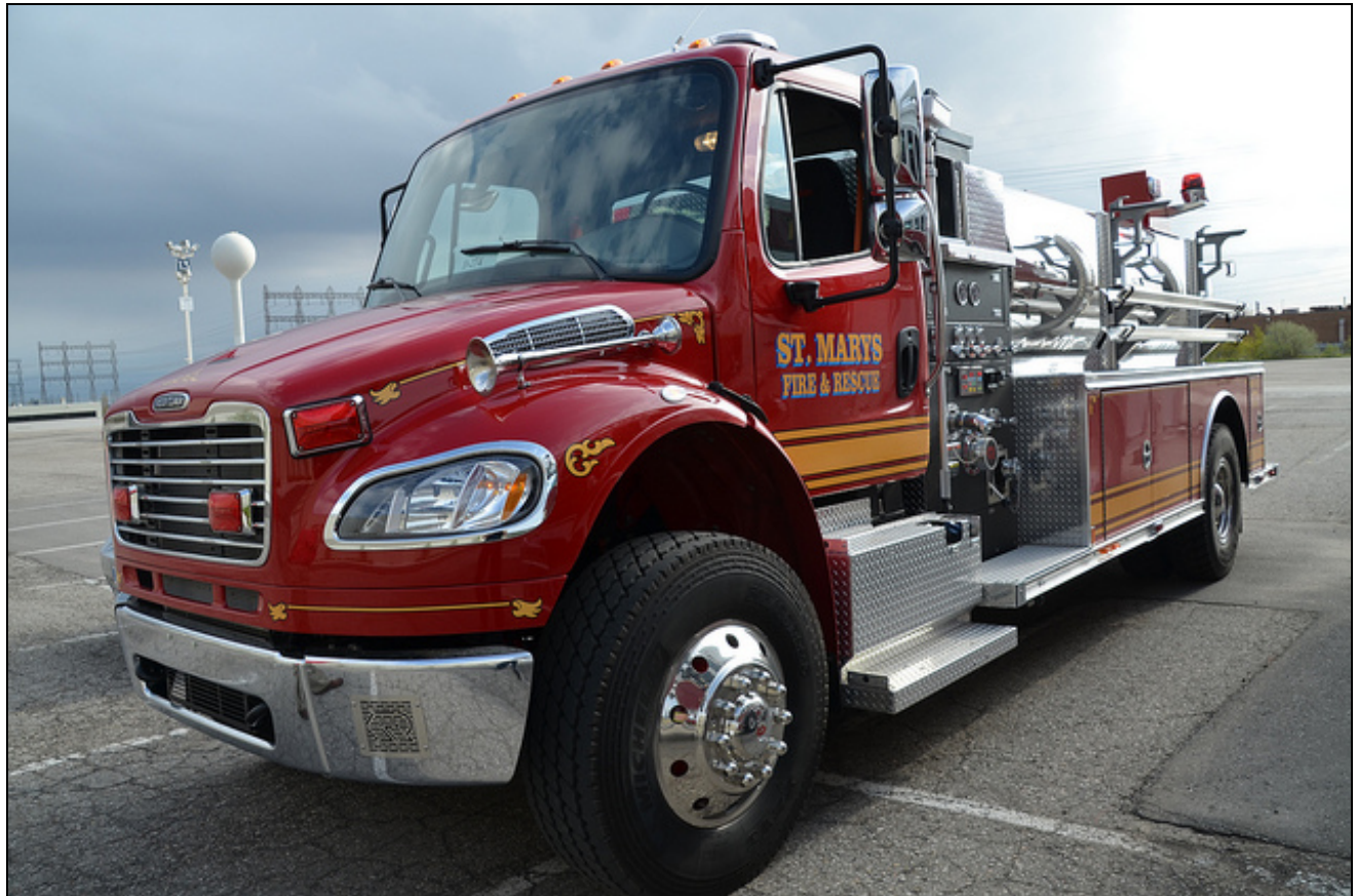
Delivered last year: St. Mary' tanker, a 2012 Freightliner M2/Rosenbauer with a 420igpm pump and 1800gwt, (SN#2102012) and Wellesley Twp. Tanker 3, a 2500 gallon job from Asphodel on a 2012 IHC 7500 chassis. Tanker 1 (Linwood), bought in 2010, is the same. (Larry Thorne photos)
