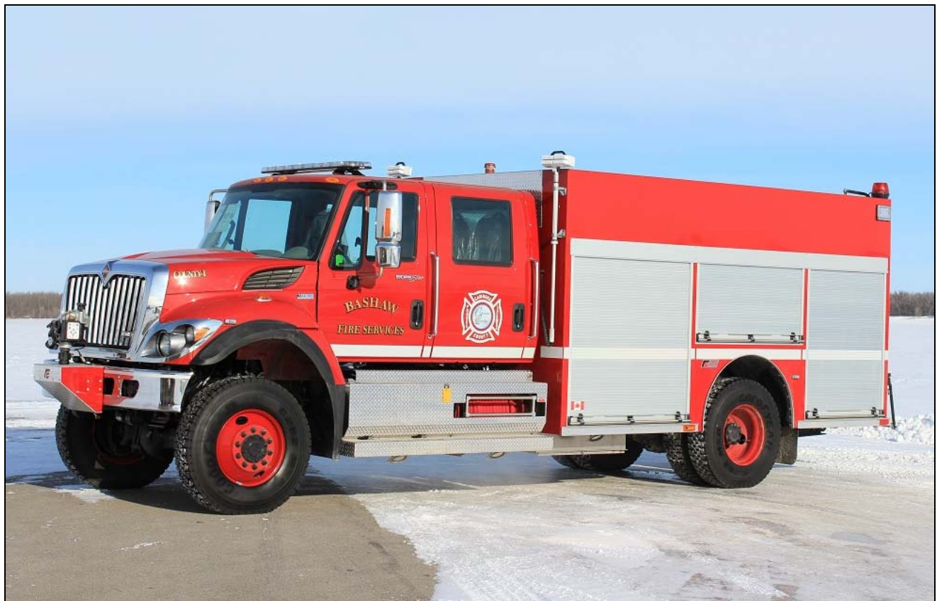
A pair from Fort Garry, above is Bashaw, AB's 2013 IHC 4400 4x4/Fort Garry Duster pumper with 1050igpm pump, 800gwt & 25gft (s/n M390), below is Gillam, MB's 2013 Freightliner M2 4x4/Fort Garry Terminator, with 1050igpm pump, 1000gwt & 25gft (s/n M451) (Dave Stewardson photos)
