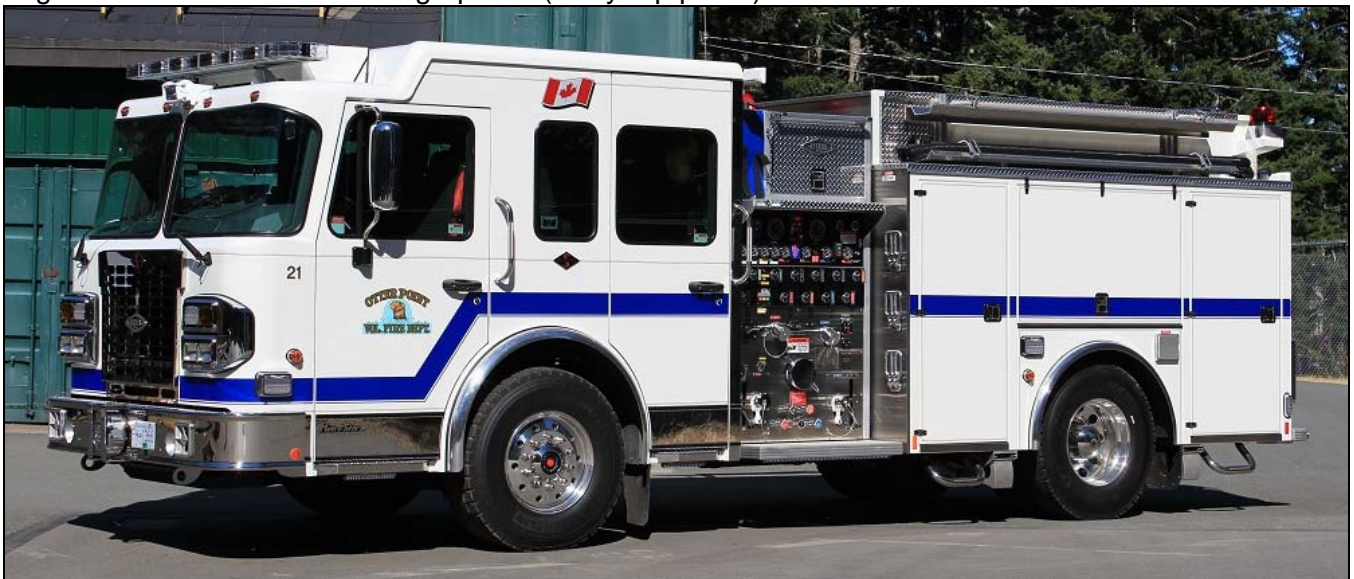
Above is Otter Point's all white 2013 Hub/Spartan Metro Star pump, with a 1050igpm pump, 1025gwt, and twin 25gfts, delivered in July. Below, Brazeau County is now running this 2013 Ford F550/Fort Garry mini-pump with 70igpm pump, 300gwt and 10gft as Quick Response 2. (Dave Stewardson)
