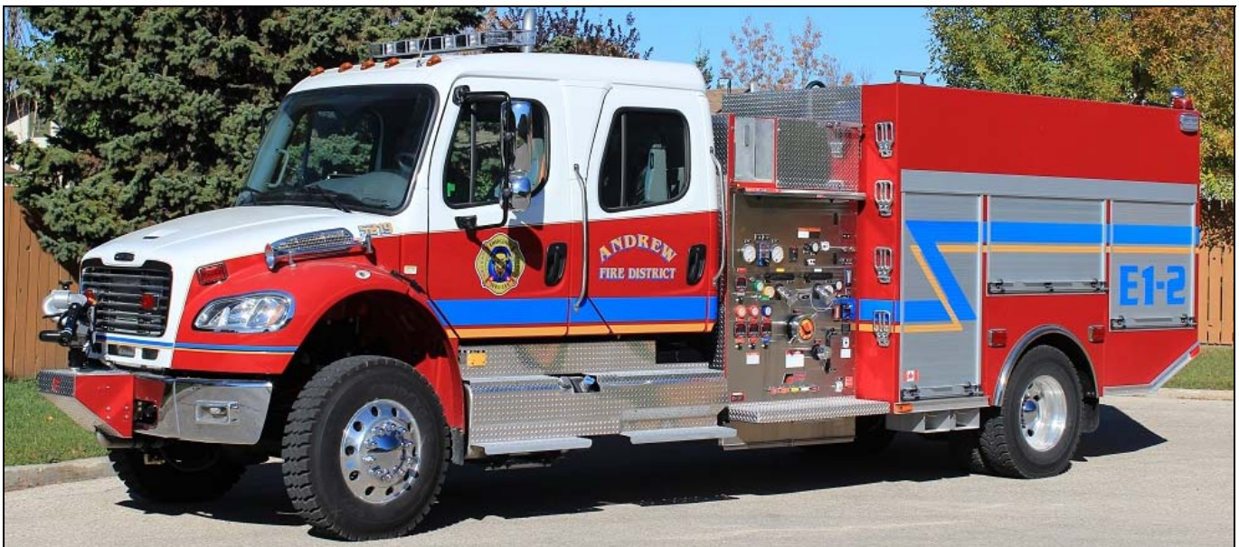
Three from the roundup: Andrew, MB E1-2, a 2013 Freightliner M2 4x4/ Fort Garry pumper with 1050igpm, 500gwt & 25gft, and Inuvik, NWT P1, a 2013 IHC 4400/Fort Garry1050igpm/1500gwt/50gft pumper.
