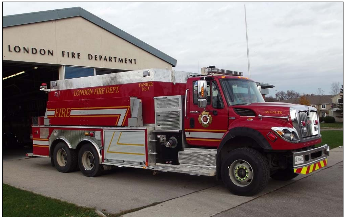
London's latest acquisition from Carl Thibault , a 2500 gallon tanker on a 2013 IHC 7600 chassis equipped with a 500igpm pump. (Rick Loiselle photo)
