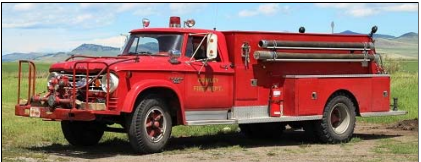
Cowley, AB ran this 1965 Dodge D600/Saskatoon pumper with a front-mount 500igpm pump and 300gwt. (John Bowerman photo)
