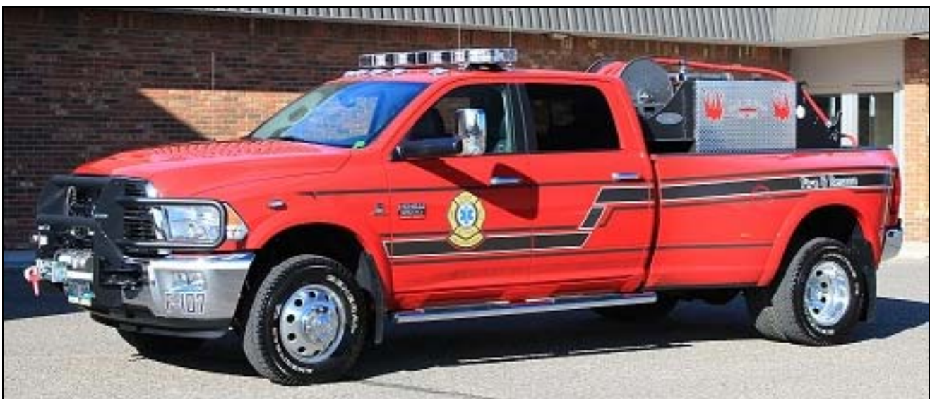
East St. Paul, MB 107, a 2012 Dodge Ram 3500/Acres 4x4 brush unit with a portable pump and 250gwt and 5gft. (All photos Dave Stewardson)
