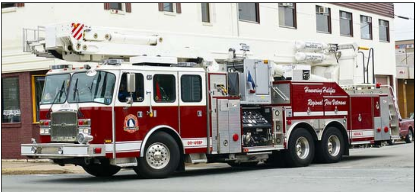
Halifax Aerial 1, a 2009 E-One Cyclone II Bronto 114 tower with a 1750igpm pump and 400gwt.
