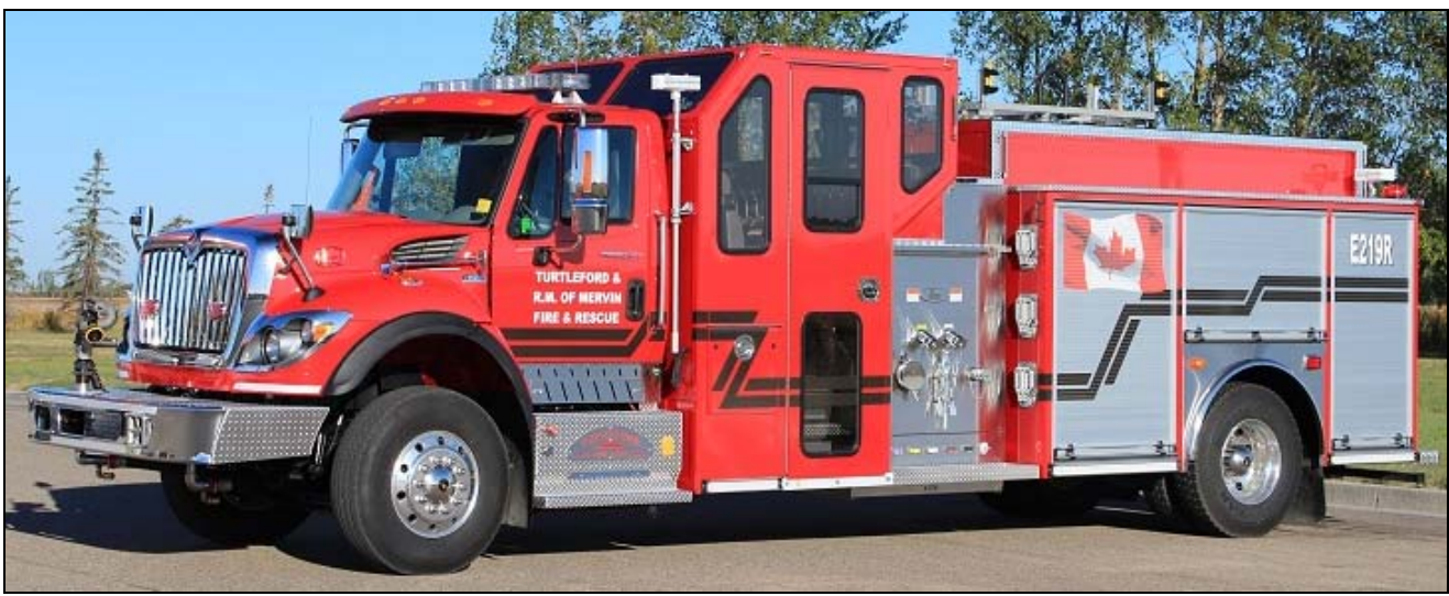
Turtleford, SK Engine 219R, a 2012 IHC/Acres pumper-tanker with 1050igpm, 1000gwt & 25gft.
