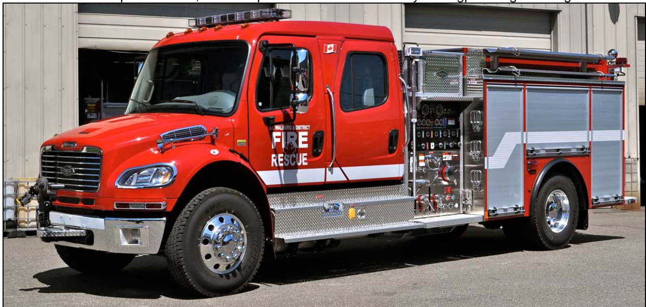
St. Walberg, SK has this 2012 Freightliner M2/Hub pumper featuring an 840igpm pump. 800gwt, 25gft and Foam Pro 1600 FS. (All photos by Terry Yip).
