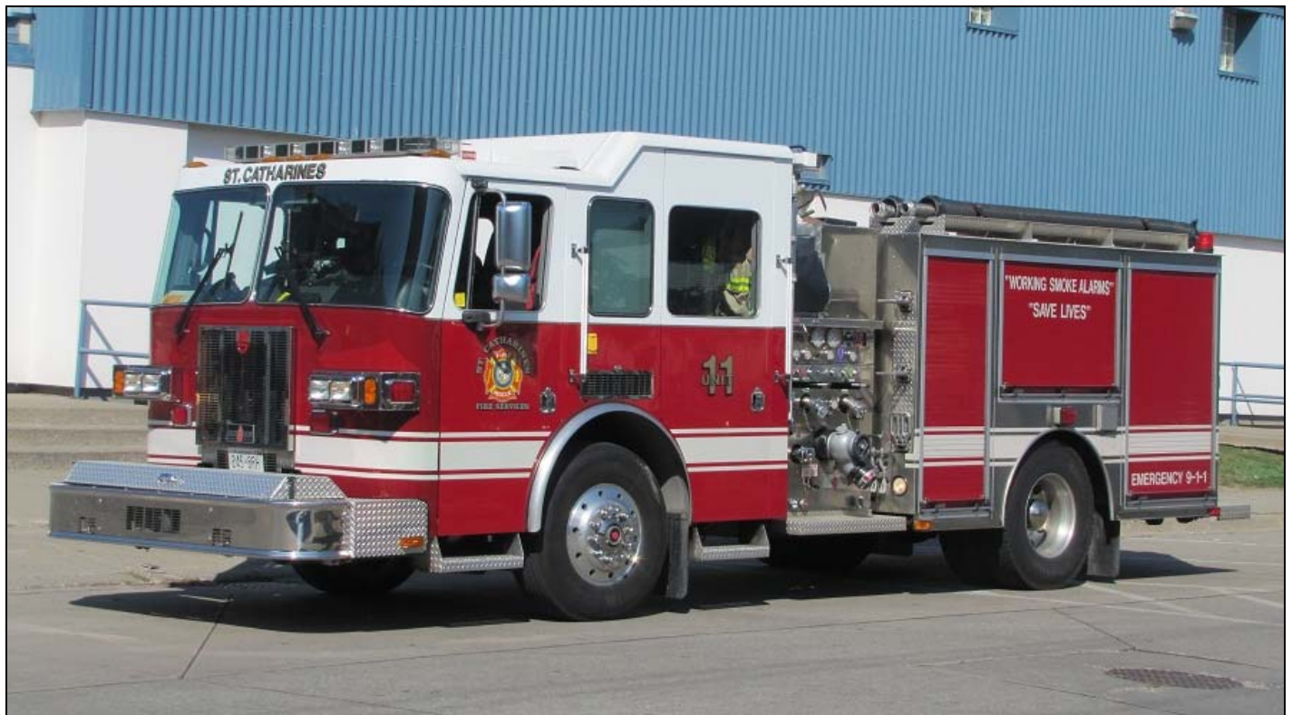
St. Catharines Unit 11 runs as Pump 4, it's a 2005 Sutphen Shield pumper with a 1250igpm pump, 600gwt and 20gft. (Desmond Brett photo)
