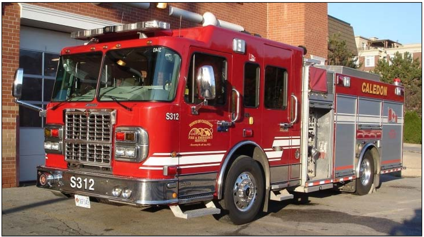
From the tour last fall, this shot is Caledon's Squad 312, assigned to the Bolton hall. Staffed by the CFD's only full time crew, the rescue pump is a 2009 Spartan Gladiator/DEV 1050igpm, 600gwt and 25gft.
