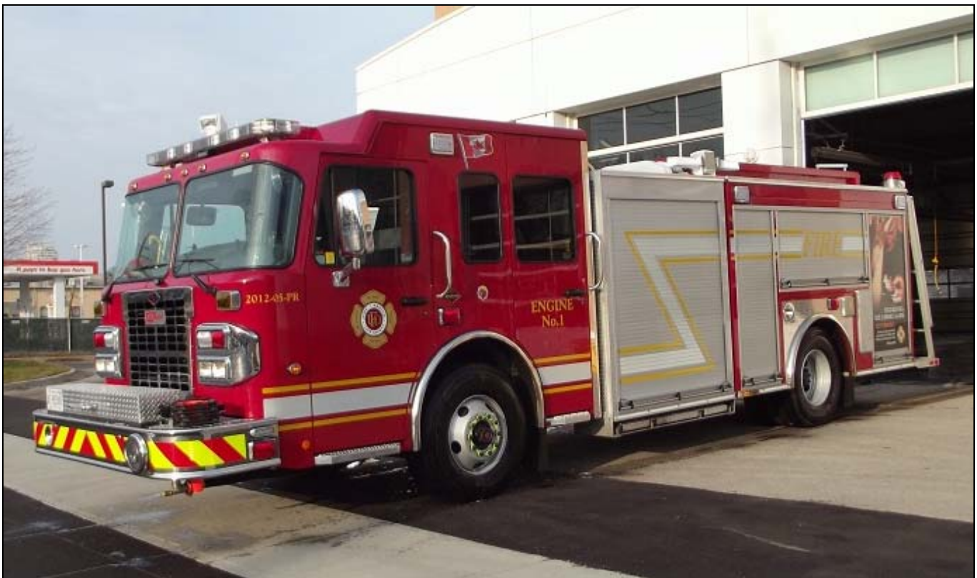
One of a pair delivered to the Forest City, this is Engine 1, a 2012 Spartan Carl Thibault 1250/500 pumper. The other pump went to Engine 14 and E14's 2010 Carl Thibault went to Station 4. (Rick Loiselle)
