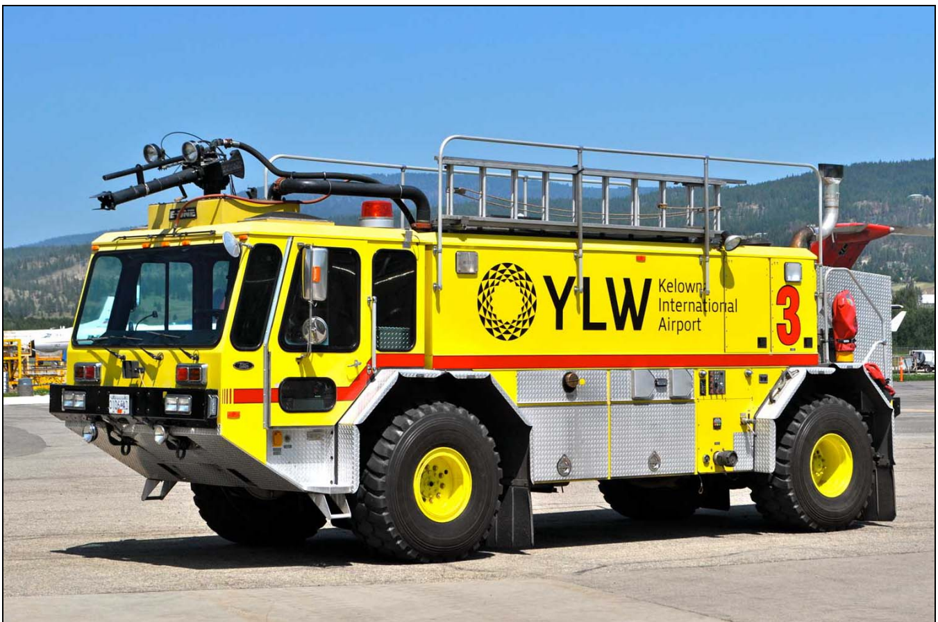
Kelowna Airport Red 3, a 1995 E-1 Titan crash truck equipped with a 1250igpm pump, 1585gwt, 200gft, and 500 lbs dry chemical. It is one of a pair at the airport. (Terry Yip)
