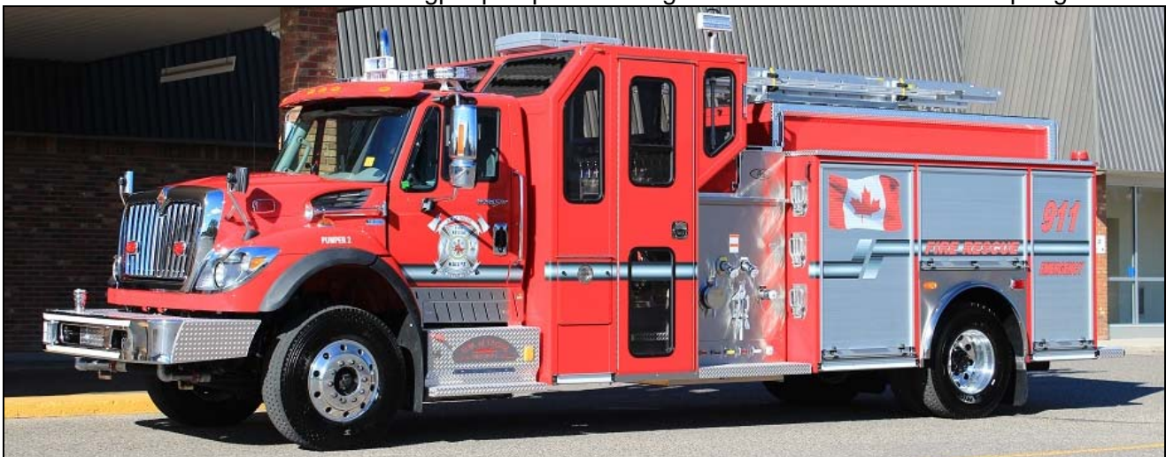
The Rural Municipality of Tache Pumper 2, stationed in Landmark. It is a 2012 IHC 7400/Acres 1050 igpm pumper with a 1000gwt and 25gft also received in the fall. (Dave Stewardson photos).
