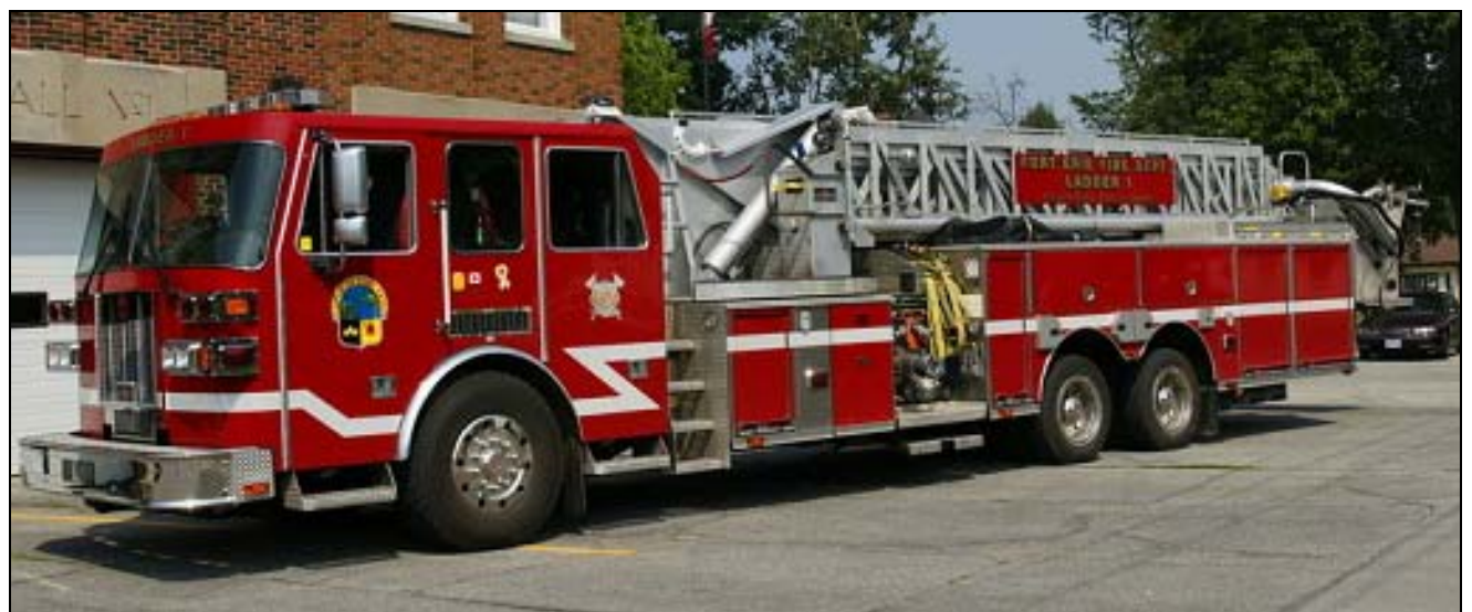
Ladder 1 is a 2006 Sutphen 95' Aerial Tower with a 1250igpm pump and 300 gwt. A similar rig just went into service at Ladder 4.
