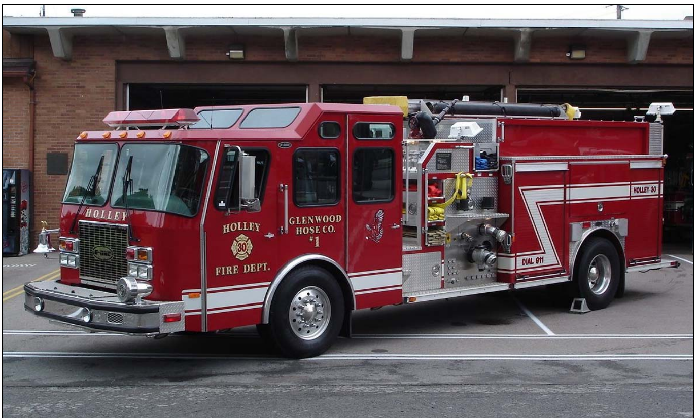
The Glenwood Hose Co. #1 in Holley, NY runs this 2006 Emergency One 1250gpm pumper with a 1000gwt. (Bob Rupert photos)
