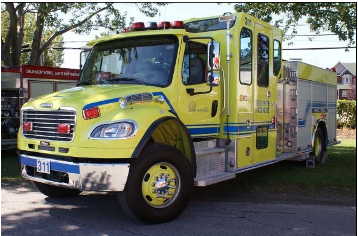
A fast-disappearing breed, the yellow fire truck: this example belongs to Mirabel, QC. P.311 is a Maxi-Metal product on a 2008 Freightliner M2 chassis, with 1250igpm pump and 700gwt. (Bertrand Campo)
