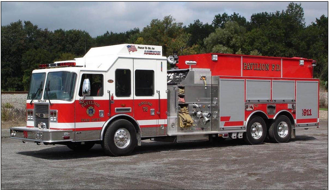
Pavilion, NY Engine 76s very long 2006 KME Predator which has a 1500gpm pump and 3000gwt.
