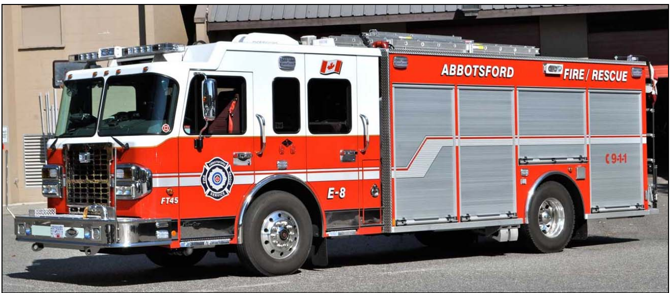
Abbotsford E. 8, a 2012 Spartan Metro Star/Hub 1750igpm/400gwt pump with a Foam Pro 2002 FS.
