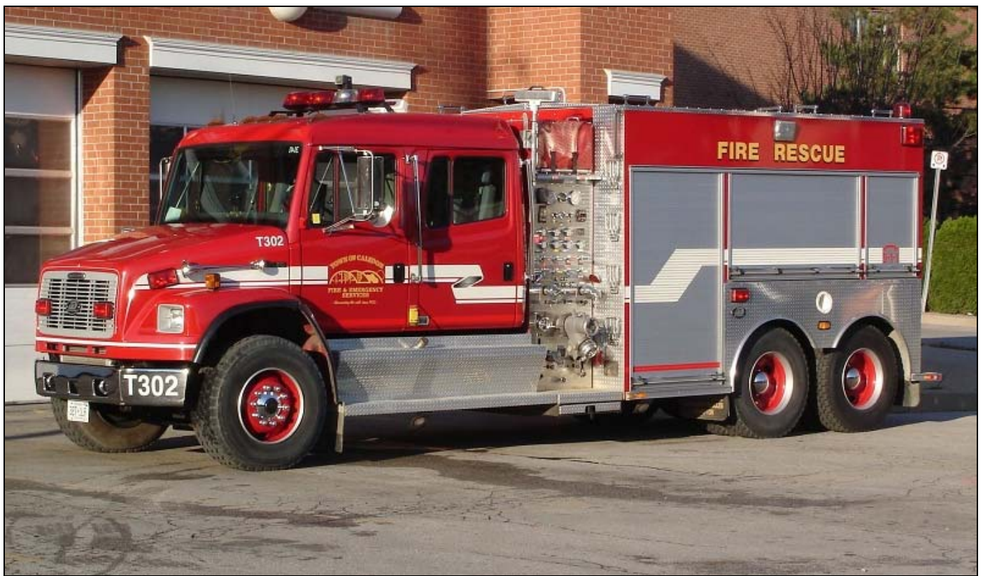
Also running from Bolton is Tanker 302, another Dependable product, built on a 2002 Freightliner FL-80 chassis. It sports a 425igpm pump, 2000gwt and 25gft. (Bob Rupert photos)
