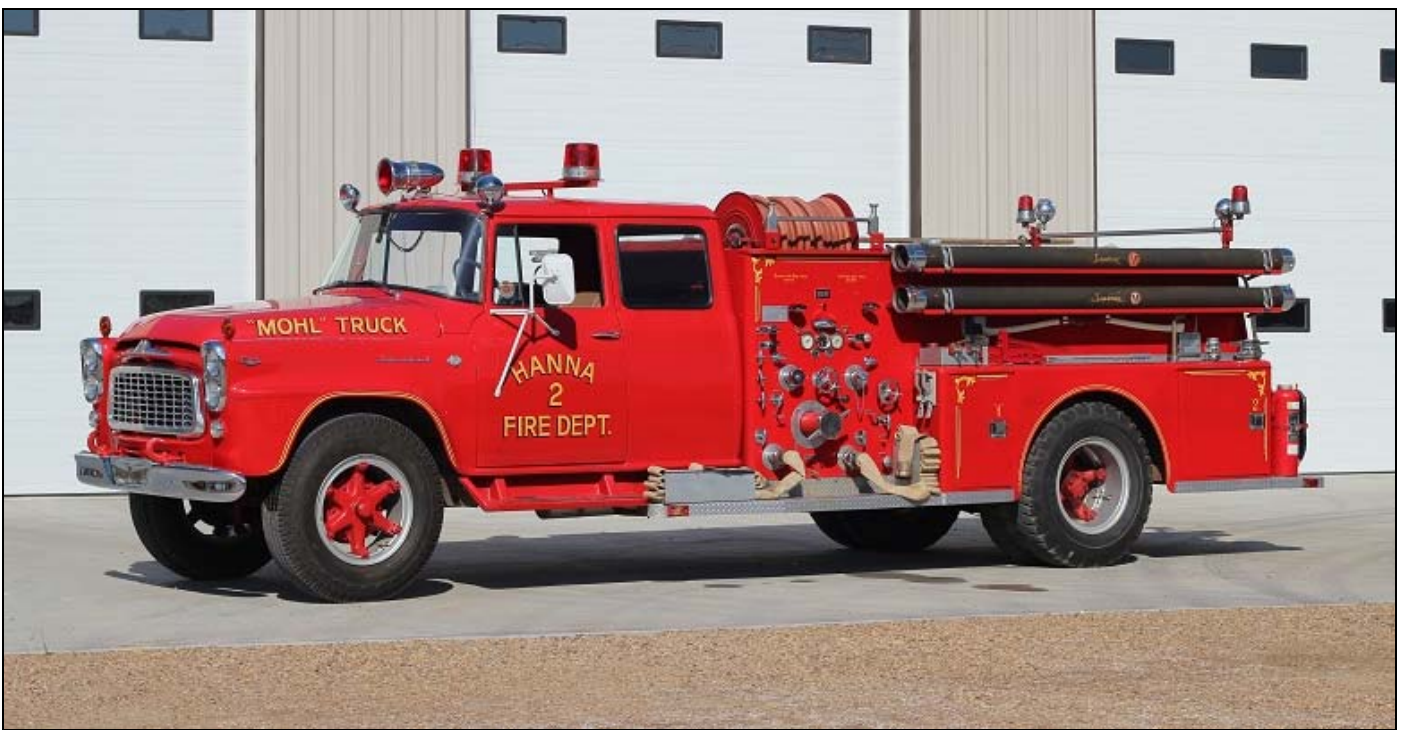
A couple of classic commercial based rigs from yesteryear, the first being this 1960 IHC B-170 "Extended Cab" / LaFrance Pump with a 625IGPM pump and 600GWT. The truck belongs to the Hanna, AB Fire Dept and is one of two vehicles going into the department museum, part of their new hall opened last year. "Mohl" on the hood honours a past fire chief. (John Bowerman photo)
