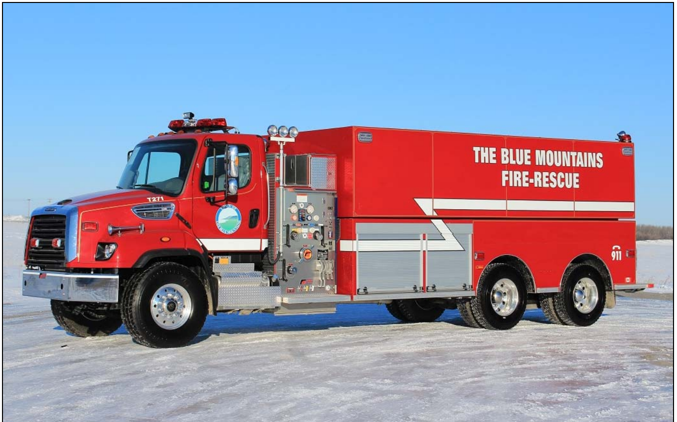
Just delivered to Blue Mountains, Tanker 271 is a massive 2012 Freightliner FL114SD/Fort Garry product with 1050igpm pump and 3000gwt, SN M392.
