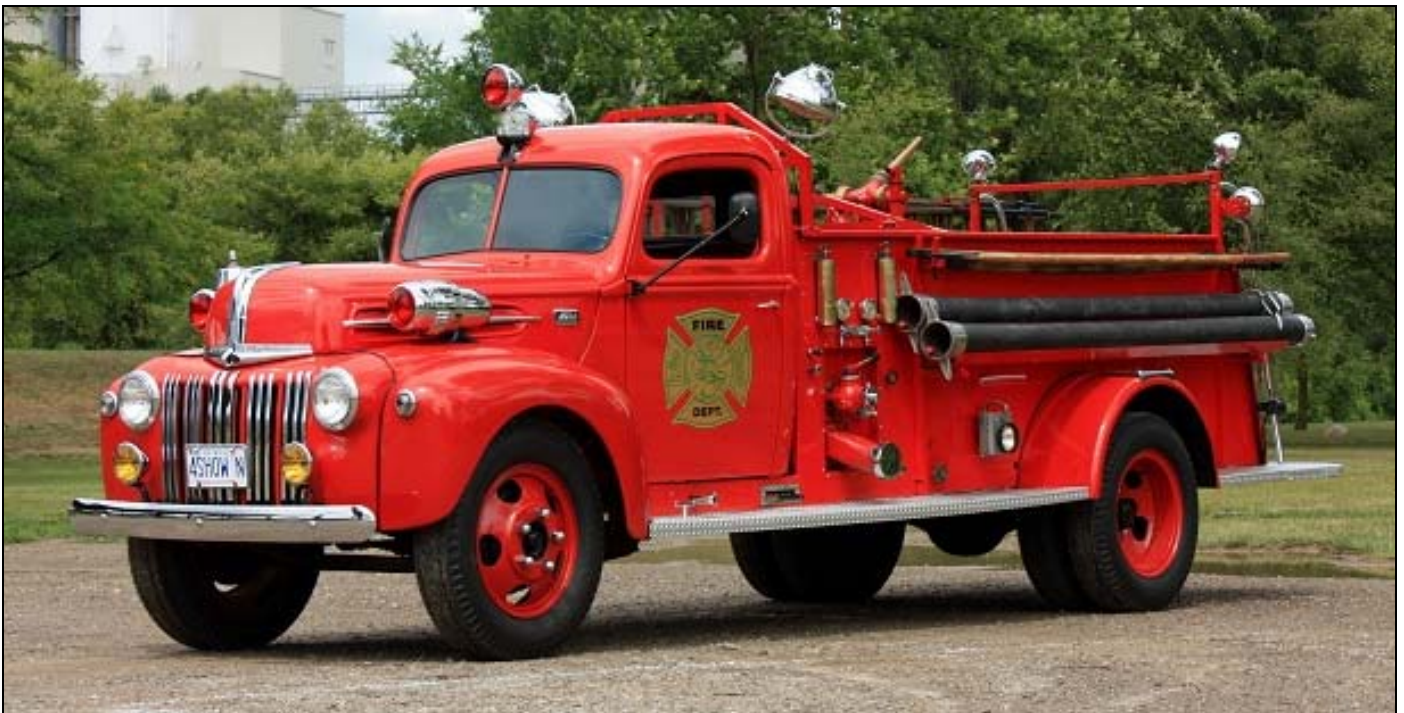
This oldie was in service with the St. Clair Shores, ON Fire Dept. Owned by Steve & Mary Irvine, Yarmouth Centre, it was photographed at the Franenmuth Muster last year. It is a 1942 Ford/General pumper with a 425ipgpm pump and 250gwt. (Herb Galloway photo)
