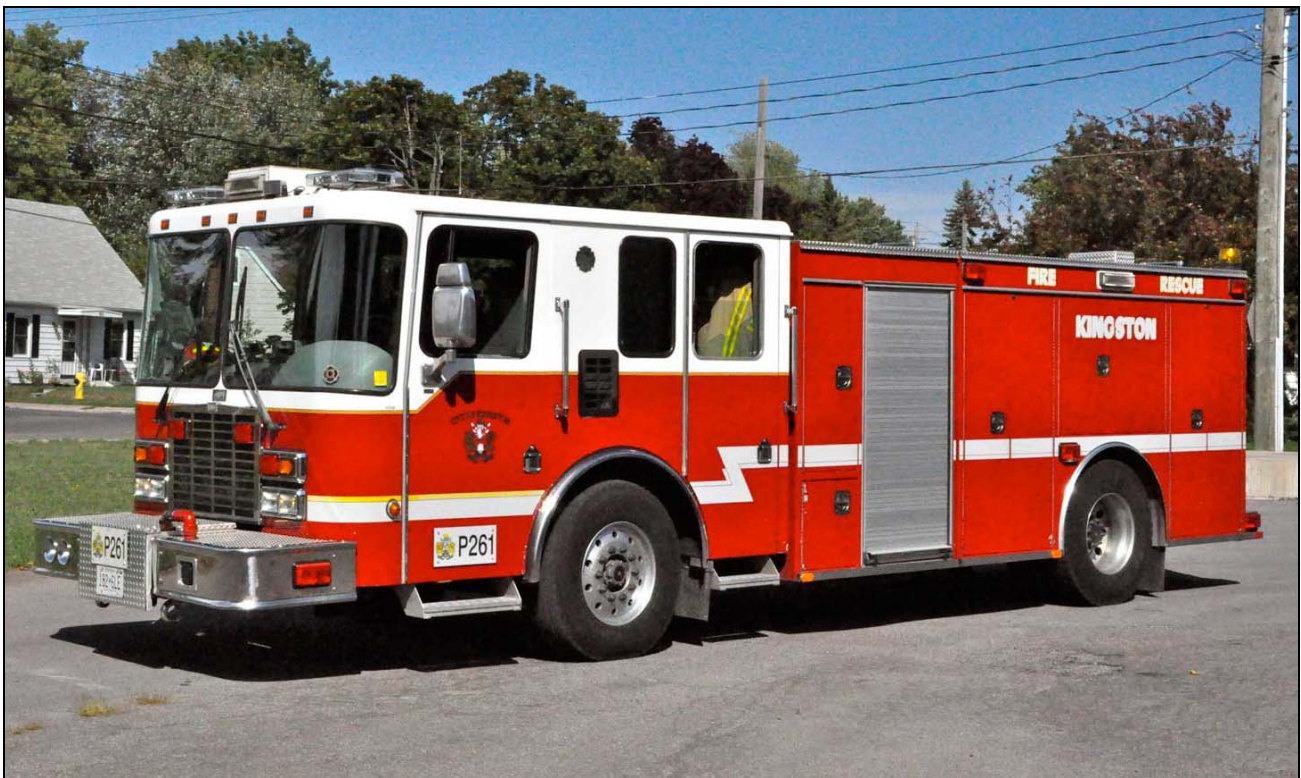
An interesting pair of rigs from Kingston, Pump 261 is a 2002 HME/Almonte 1050igpm with a 400gwt and 40gft. Roll Off 271 is a 2008 IHC chassis equipped to transport pods and was shot while carrying the Tech Rescue box. (Above: Terry Yip, below: Neil McCarten photo)
