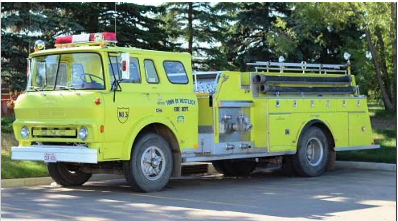
Westlock, AB still has this 1976 GMC T6500/Superior Super Vision pumper on its roster, although retired. The canopy cab rig has an 840igpm pump. It carries serial number SE87. (John Bowerman photo)
