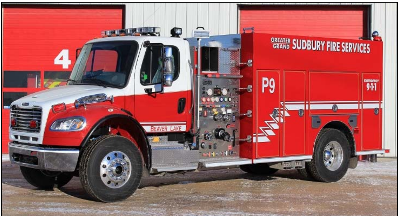
Sudbury's newest, a 2012 Freightliner M2/Fort Garry pumper-tanker with a 1050igpm pump, 1000gwt and 25gft, SN 393. It's also equipped with a Foam Pro 1600 foam system. Pumper 9 is assigned to Beaver Lake. P25, just received, is identical; it went to Red Deer Lake. (Dave Stewardson photos)
