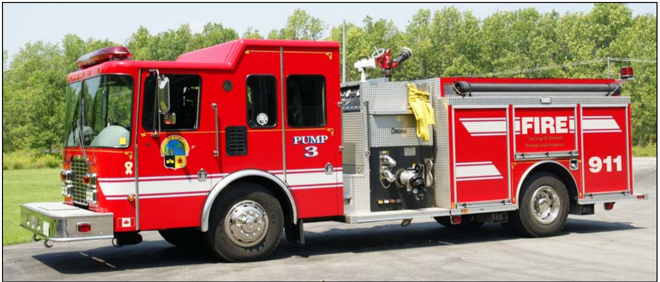
Three from Fort Erie, first up is Pump 3, a 2002 HME 1871/Central States product with a 1050igpm pump and 700gwt. (All photos by Jon Lasiuk)
