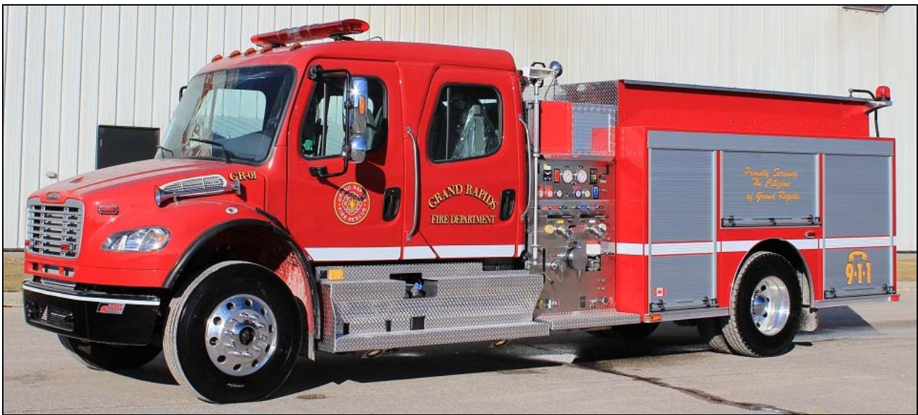
Three from Manitoba: Grand Rapids received this 2012 Freightliner M2/Fort Garry pumper last fall; it has a 1050igpm pump, 800gwt and 25gft. SN M374.
