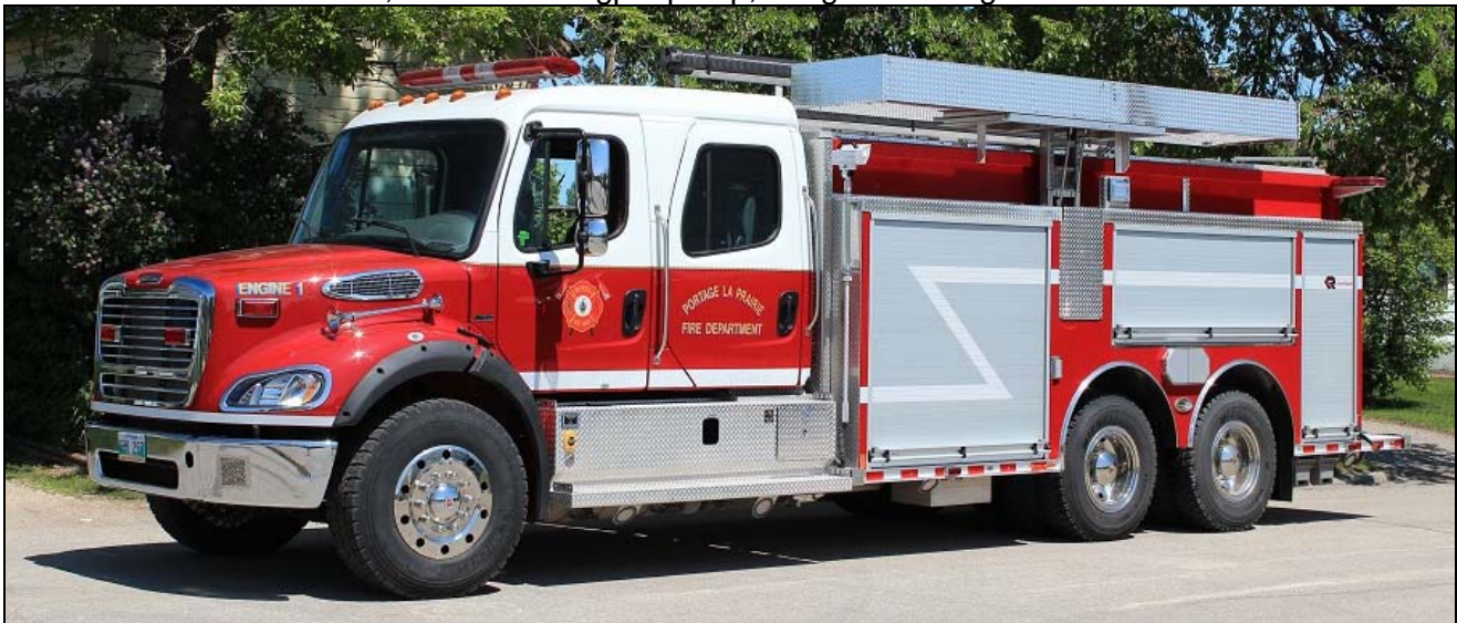
This big tandem-axle pumper-tanker runs as Engine 1 in Portage La Prairie, it's a 2012 Freightliner M2/Rosenbauer with a 1050igpm pump and 2000gwt and was delivered in the spring.
