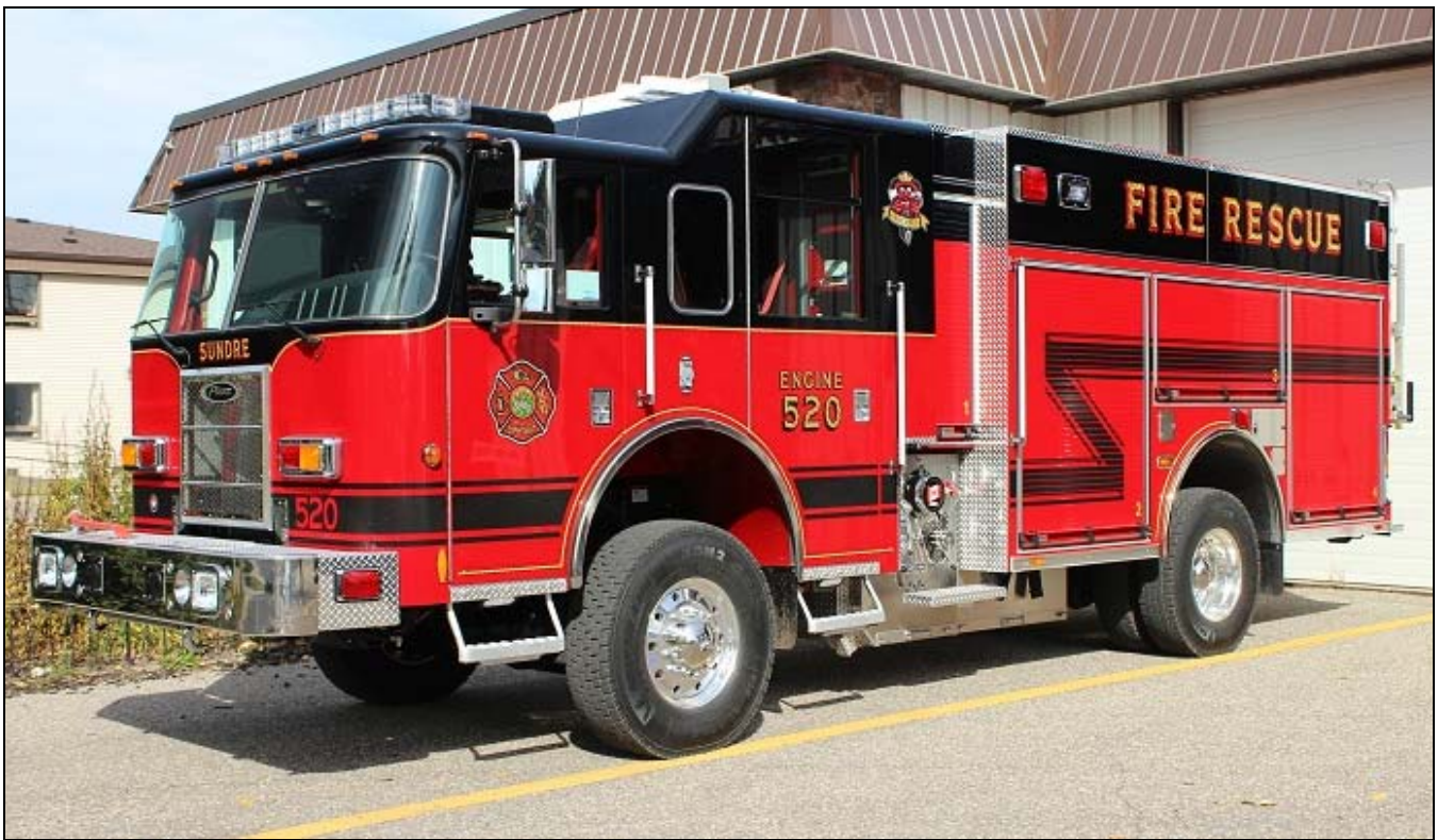
Sundre, AB Engine 520, a 2012 Pierce Saber PUC 4x4 pumper with 1250igpm pump, 800gwt and 25gft. It also has a Husky 3 foam system. (John Bowerman photo)
