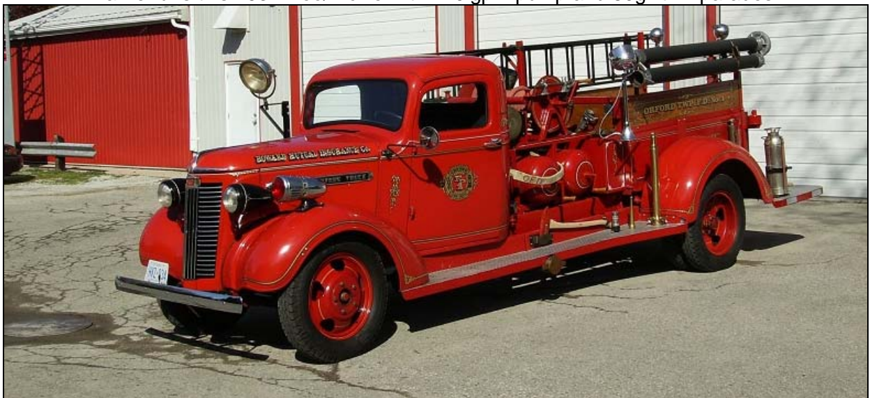
Another Chatham-Kent station, No.10 in Highgate, still has this former Orford Township 1938 GMC/General rig, it has a 225igpm pump and twin 40gwt. (Neil McCarten photos)
