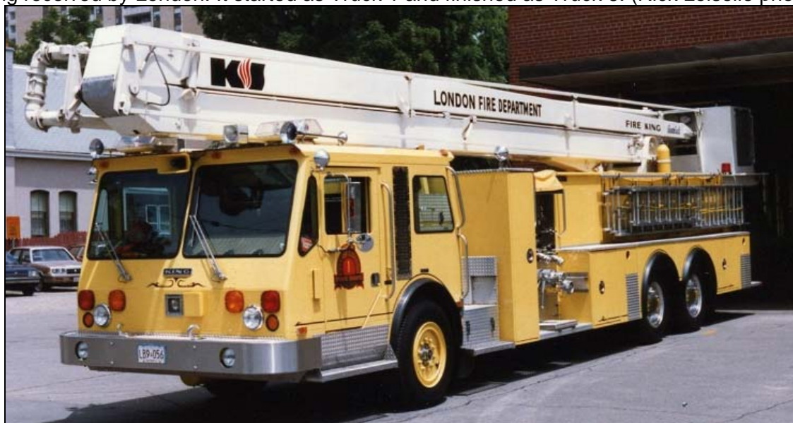
Below, LFD's 1985 King CM-1 snorkel, with a 1050igpm pump, 300gwt and 85' booms transplanted from the 1971 Ford/King Seagrave rig. It is probably the last rig delivered by King, certainly the last King received by London. It started as Truck 1 and finished as Truck 6. (Rick Loiselle photos)
