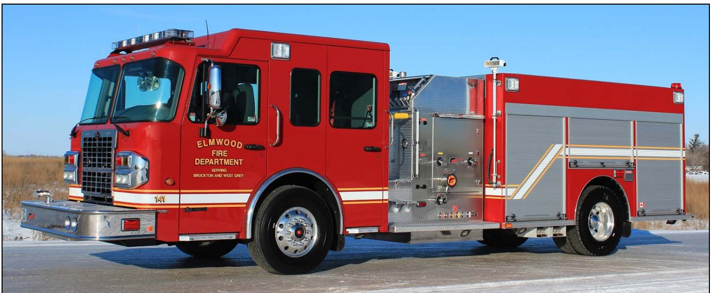
Elmwood just got this 2014 Spartan MS-X/Fort Garry 1050(H)igpm, 800gwt, 20gft pumper for P.141 s/n M562. (Dave Stewardson photos)
