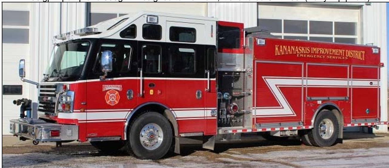
Newly received in the Kananaskis Improvement District in Alberta, this 2015 Rosenbauer pumper has a 1261igpm pump, 461gwt and 40ft. SN 16462. (John Bowerman photo)
