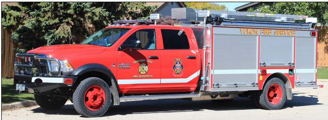
Starting out west: Yukon Fire Service put this 2014 Dodge 5500 4x4/Fort Garry mini into Dawson, it has a 675igpm Waterous pump, 275gwt, 20gft and a 140cfm CAFS. (Dave Stewardson photo)
