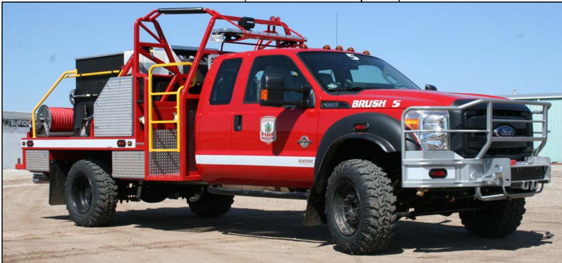
Saskatoon, SK Brush 5, a 2013 Ford F-550 4x4/Blanchat 150gpm/300gwt (Blanchat photo)
