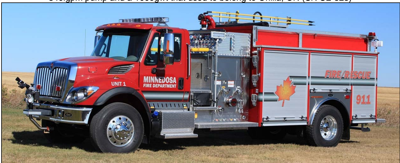
Minnedosa, MB Unit 1 is a 2015 IHC 7400/Acres pumper/tanker equipped with a 1050igpm pump, 1000gwt and 25gft. s/n 151002133 (Dave Stewardson photos)
