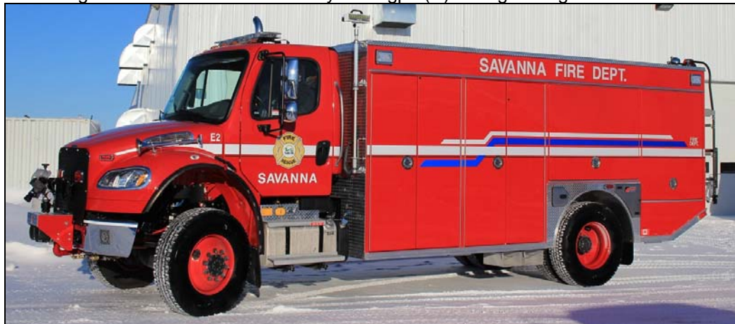
Savanna E.2 2015 Freightliner M2-106 4x4/Fort Garry 1050igpm(D)/1000gwt /25gft s/n M649
