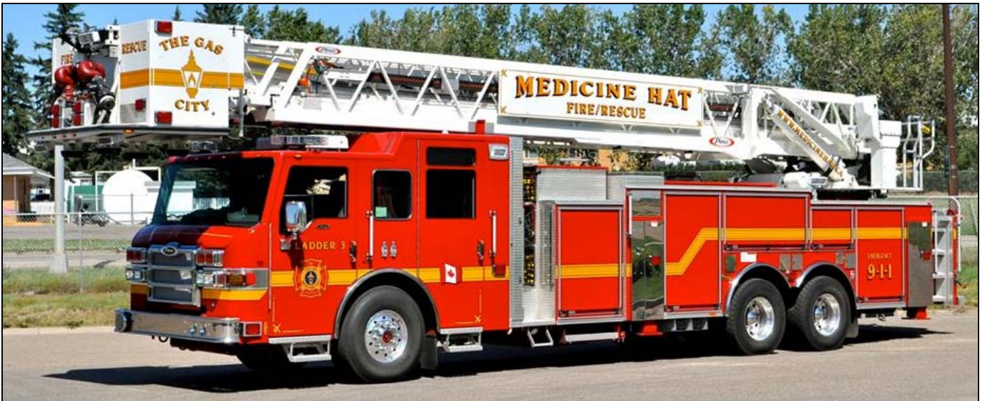
Medicine Hat, AB Ladder 3 is assigned this 2010 Pierce Velocity 100' tower ladder, with a 1750igpm pump, 250gwt and 25gft. SN 23422. (Terry Yip photo)
