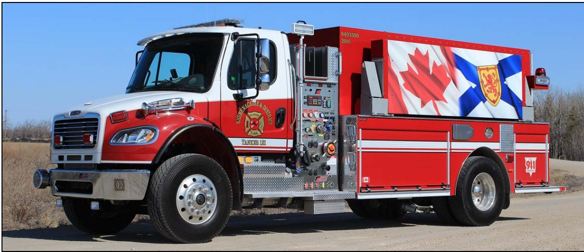
Shubenacadie, NS received this 2015 Freightliner M2-106/Fort Garry pumper-tanker in the spring. Tanker 121 has a 840igpm pump, 1500gwt and 25gft. SN M555. (Dave Stewardson)
