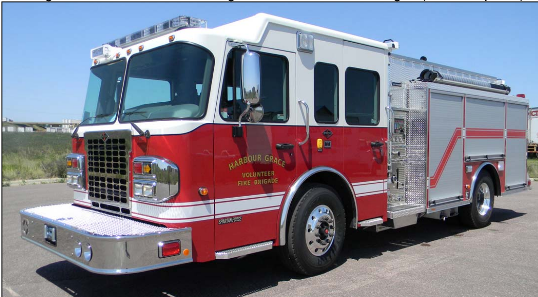
This 2012 Spartan Force/Spartan ERV pumper went to Harbour Grace, NL. Pumper 5 has a 1500gpm pump, 1000gwt and 30gft. ( Dependable Emergency Vehicles)
