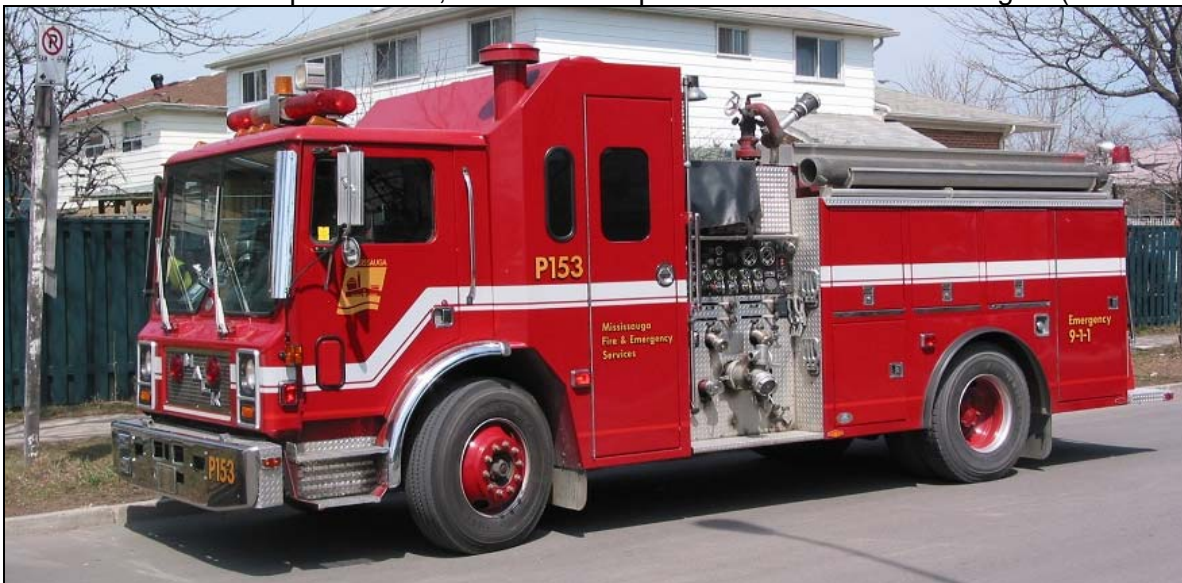
Mississauga had a brief alliance with Mack in the late 80's, including this 1989 MR chassised Superior. Seen here as a spare, it was originally Pump 112, with a 1250igpm pump and 500gwt. s/n SE915. (D. Brett photo)
