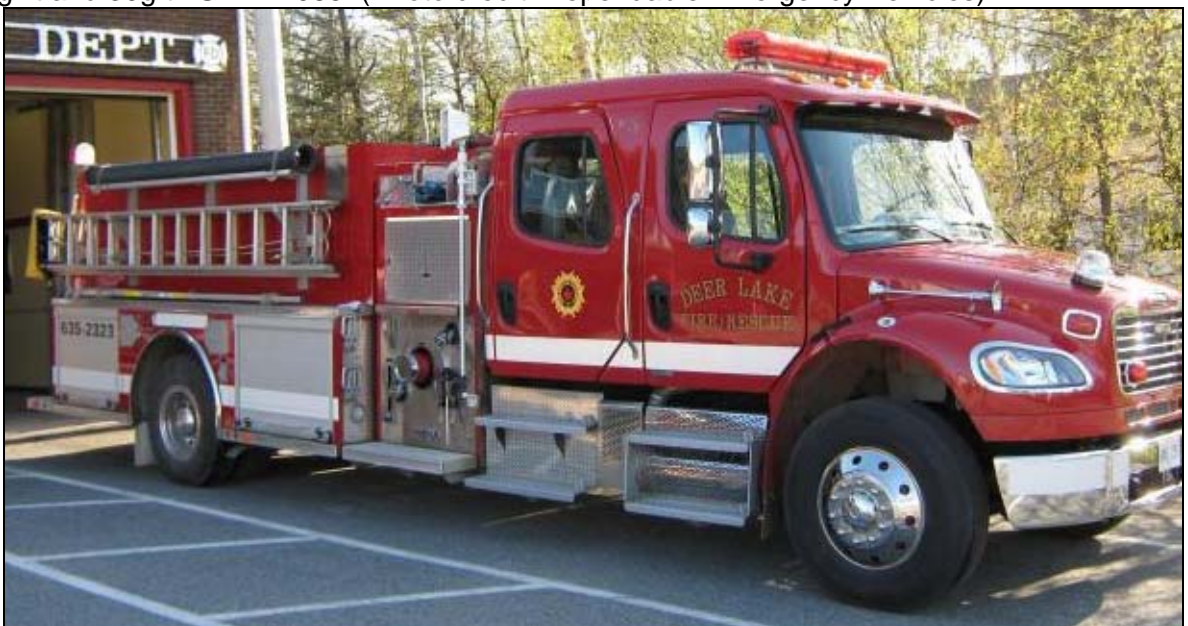
Deer Lake, NL Pump 5, a 2009 Freightliner M2/Metalfab, 1050igpm, 800gwt & 30gft. (Metalfab photo)
