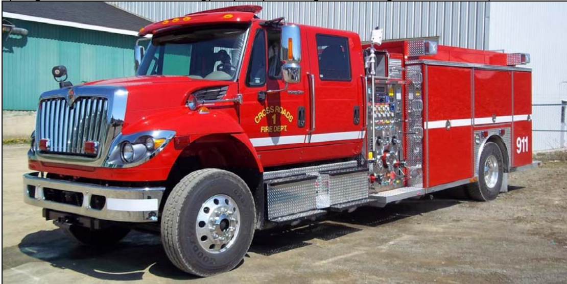
Crossroads, PEI's 2013 IHC 7400/Metalfab pumper has a Hale 1250igpm pump, 800gwt and 20gft. It's also has a 5KW PTO generator and twin 500w light. (Metalfab photo)
