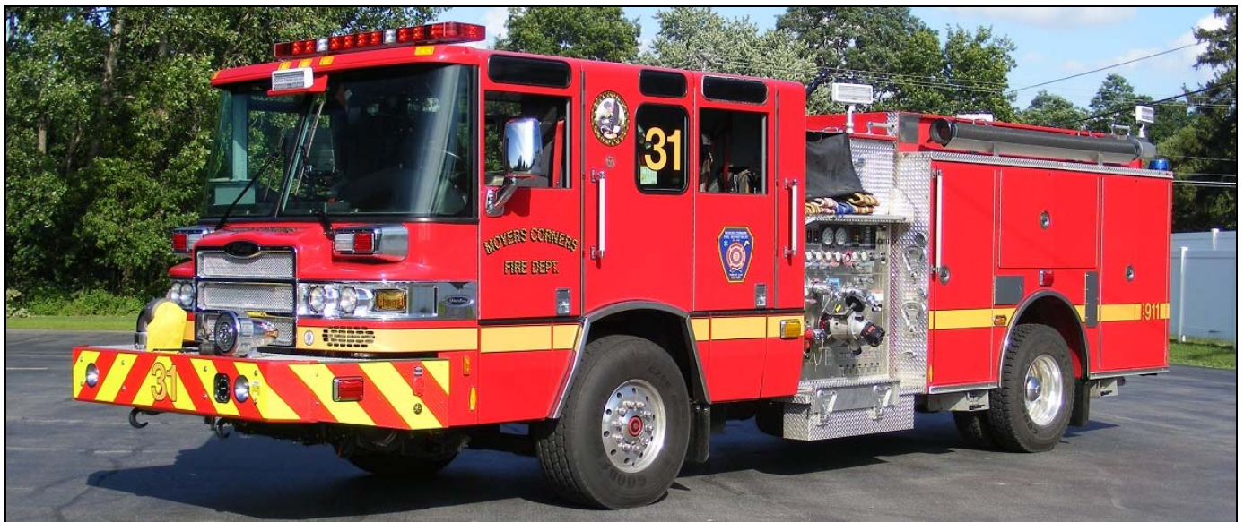
Moyers Corners, NY Engine 31 is 2013 Pierce Quantum with a 1500gpm pump and 1000gwt.
