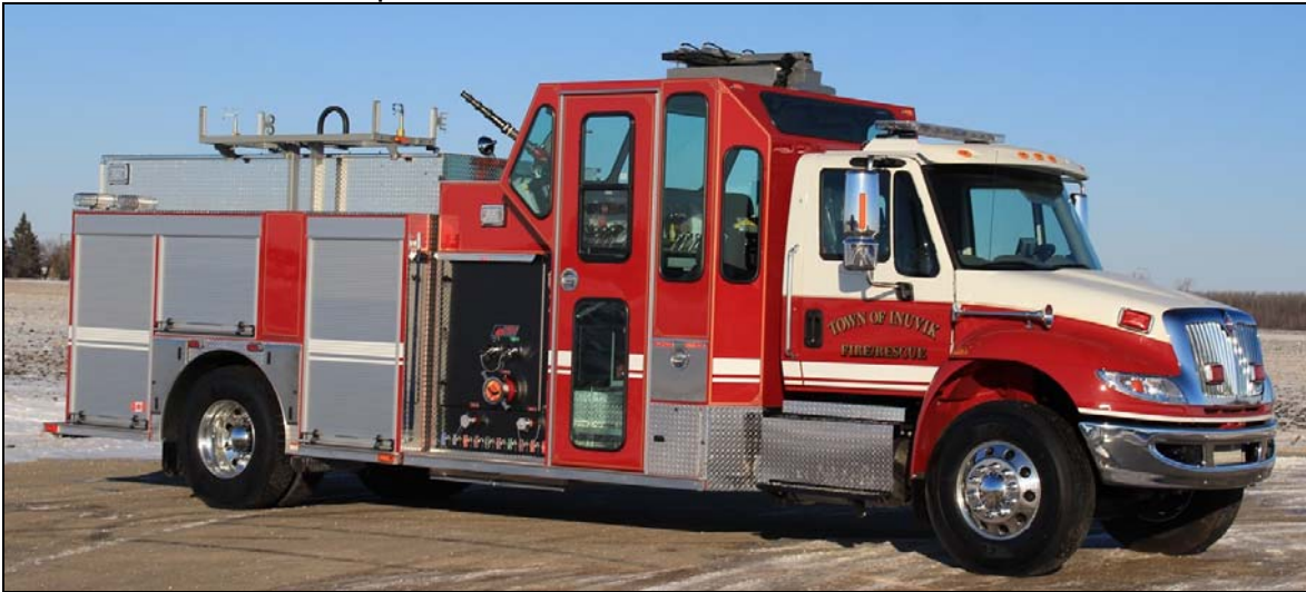
Inuvik, NWT recently received this 2015 IHC 4400/Fort Garry 1050igpm Darley pump, a 1000gwt, 25gft and a CAFS. s/n M644. (Dave Stewardson photo)
