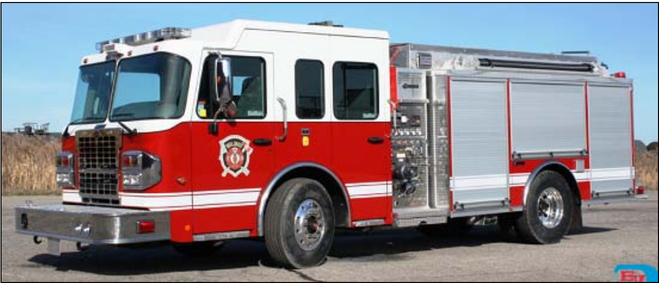
Wilmot Twp. 2015 Spartan Metro Star-X/Spartan ERV/Dependable 1500gpm/1000gwt) (ex-demo) (Photo credit: Dependable Emergency Vehicles)
