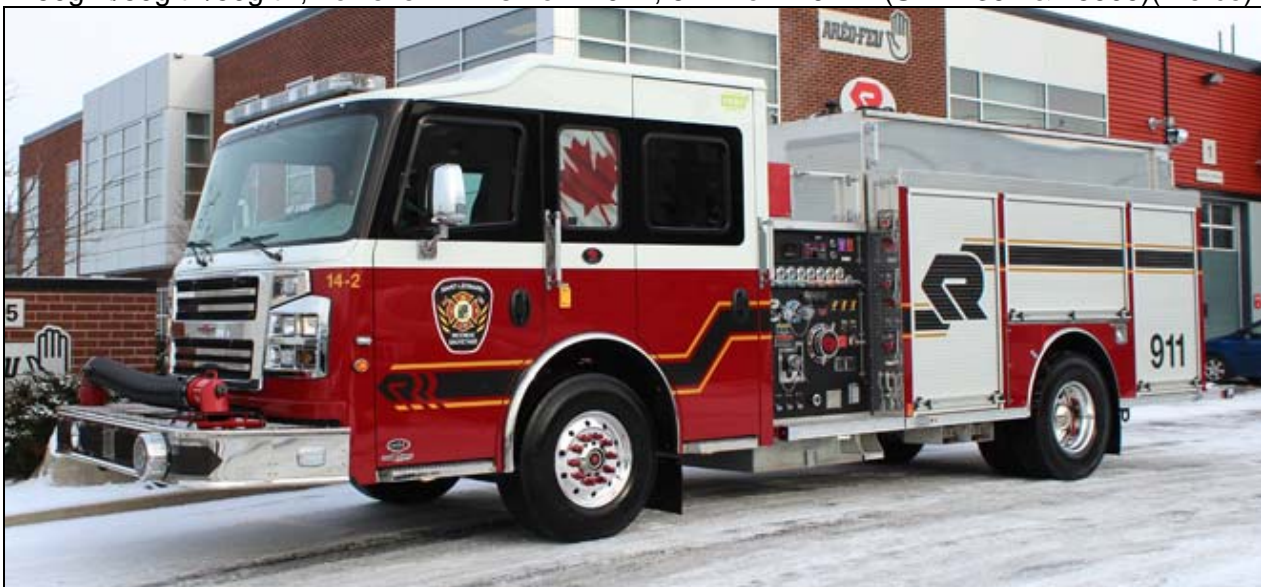
St. Leonard, NB took delivery of this 2014 Rosenbauer Commander pumper a couple of years ago. Autopompe 2 sports a 1250igpm pump, 1250gwt and 30gft. (Aerofeu photo)
