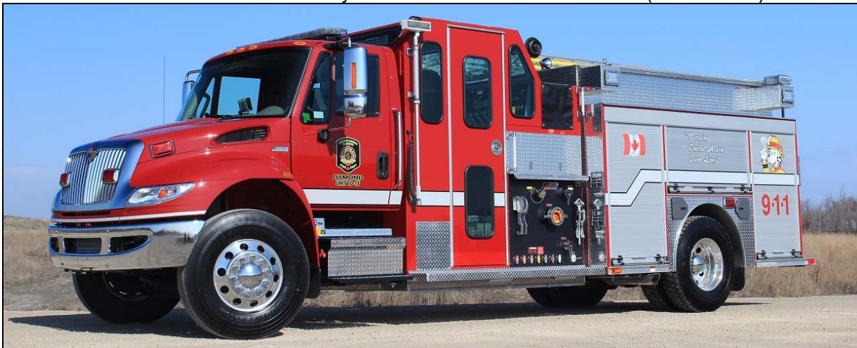
Temiskaming Shores 10-15 2015 IHC 4400/Fort Garry 1050igpm(W)/800gwt /25gft s/n #M609 (Dave Stewardson photo)
