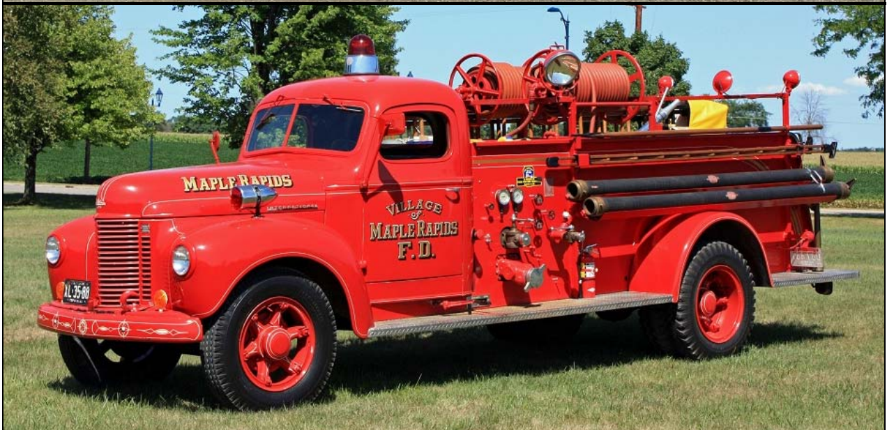
Once serving Maple Rapids, MI, this 1945 IHC KB/American pumper has a 500gpm pump and 300gwt. It is now privately owned and appeared at the Frankenmuth Muster. (Herb Galloway photo)
