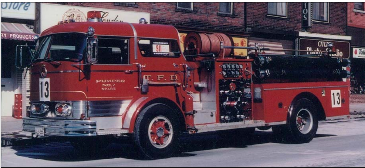
Two views of the C-95 Macks, both had 1050igpm pumps and 125gwts. Spare No. 7 (acting as P.13) is the ex-Swansea 1965 model, below is Pumper 12, delivered in 1962. (Neil McCarten photos)
