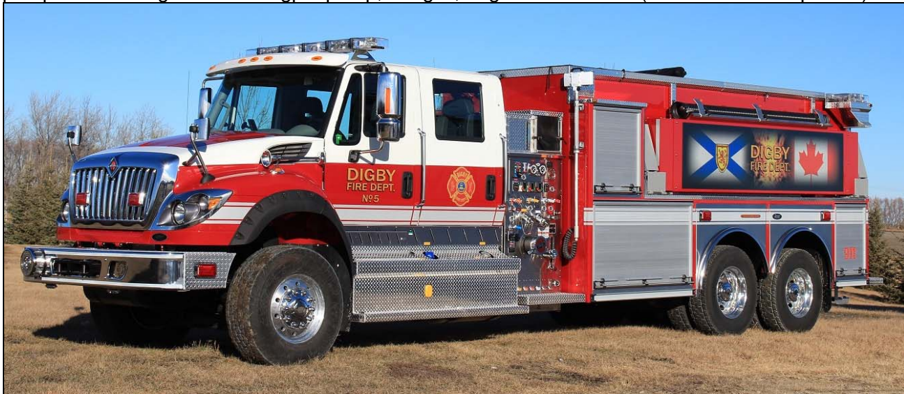
Digby, NS got this 2015 IHC 7600/Acres pumper/tanker in November. Unit 5 sports a 1250gpm pump and a 2500gwt, SN 151130134. (Dave Stewardson photo)
