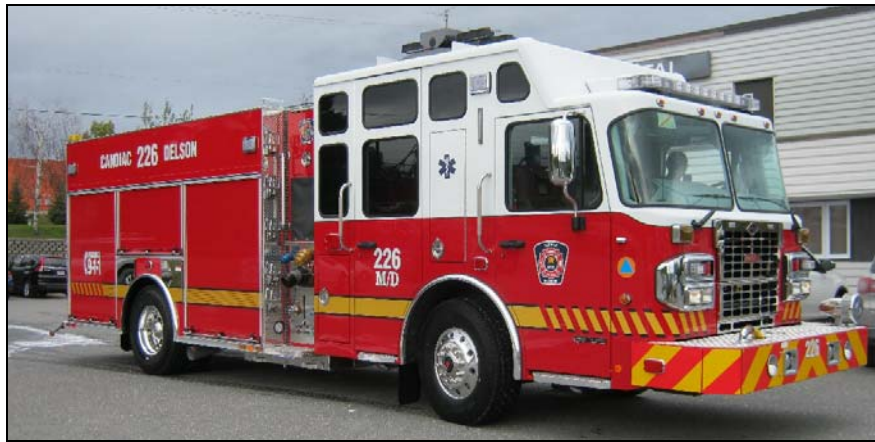
Candiac-Delson, QC, a 2015 Spartan Metro Star/Maxi Metal 1500gpm/700gwt/50gft (Maxi Metal photo)
