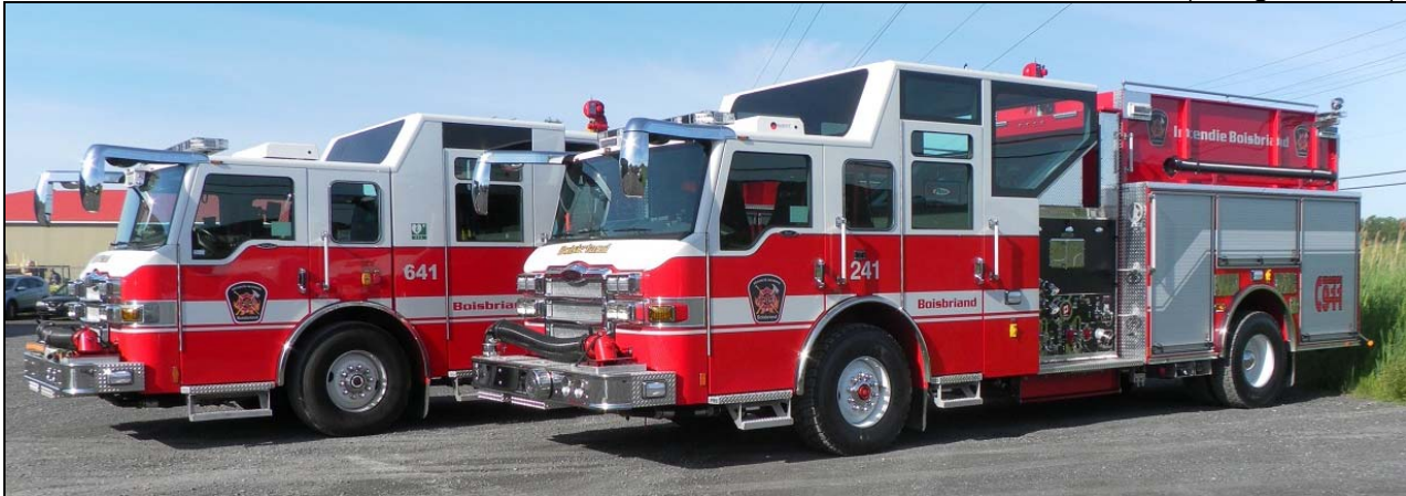
Boisbriand, QC Units 241 and 641, both are Pierce Velocity TME pumper/tankers, 1250igpm/1250gwt/50gftA/50gftB, however 241 is from 2014, 641 from 2012. (SN 27394 & 25909)(Pierce)
