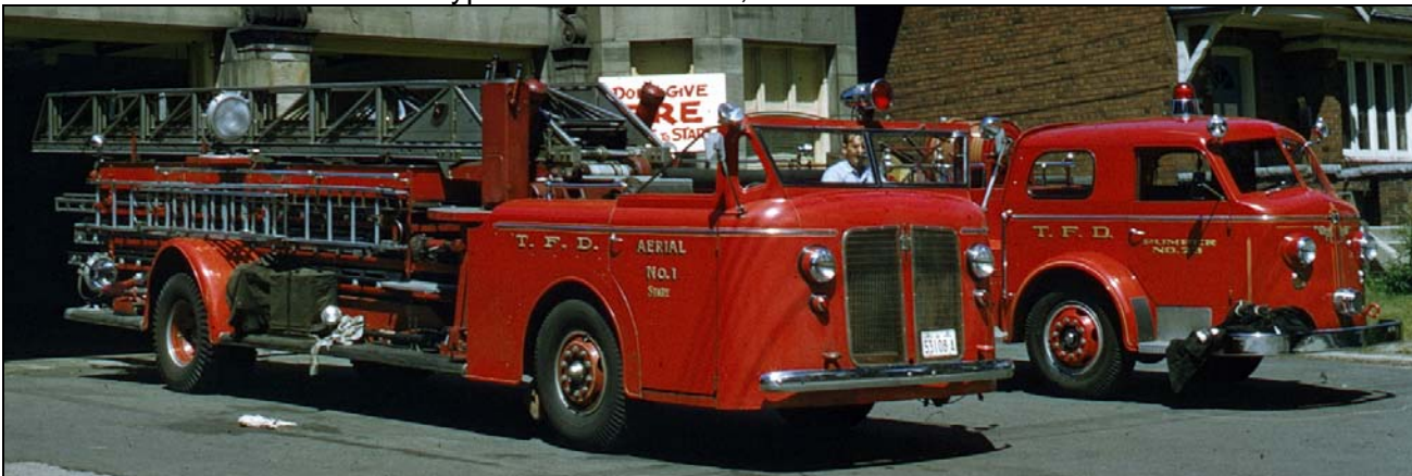
Toronto's first steel aerial, a 1942 ALF JOX 100', then running as a spare, seen at Station 23 along with their 1953 ALF 700 series pumper (840igpm,125gwt). Note the pumper's unusual siren placement.
