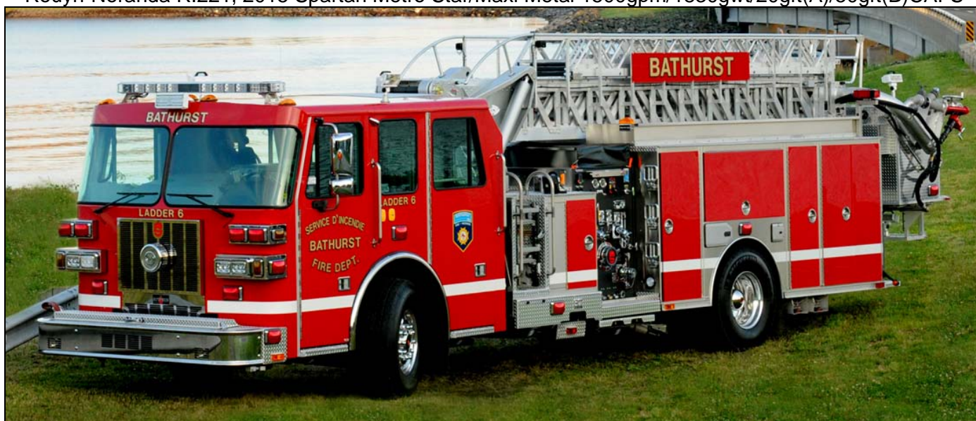
Ladder 6 in Bathurst, NB, a 2014 Sutphen SP70, 1250igpm/400gwt/70' tower. (Bathurst Fire Dept.)
