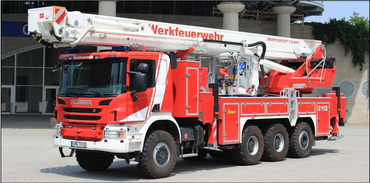
A Zeigler/Bronto 52m platform on a Scania chassis, destined for a works brigade in Germany.
