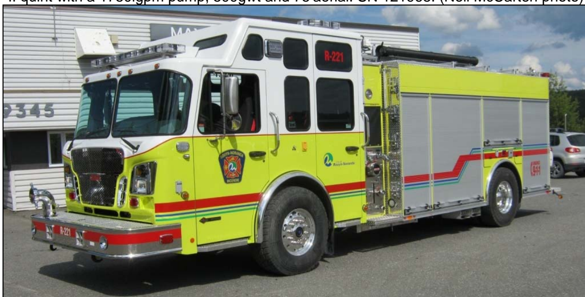
Rouyn-Noranda R.221, 2015 Spartan Metro Star/Maxi Metal 1500gpm/1830gwt/20gft(A)/50gft(B)/CAFS
