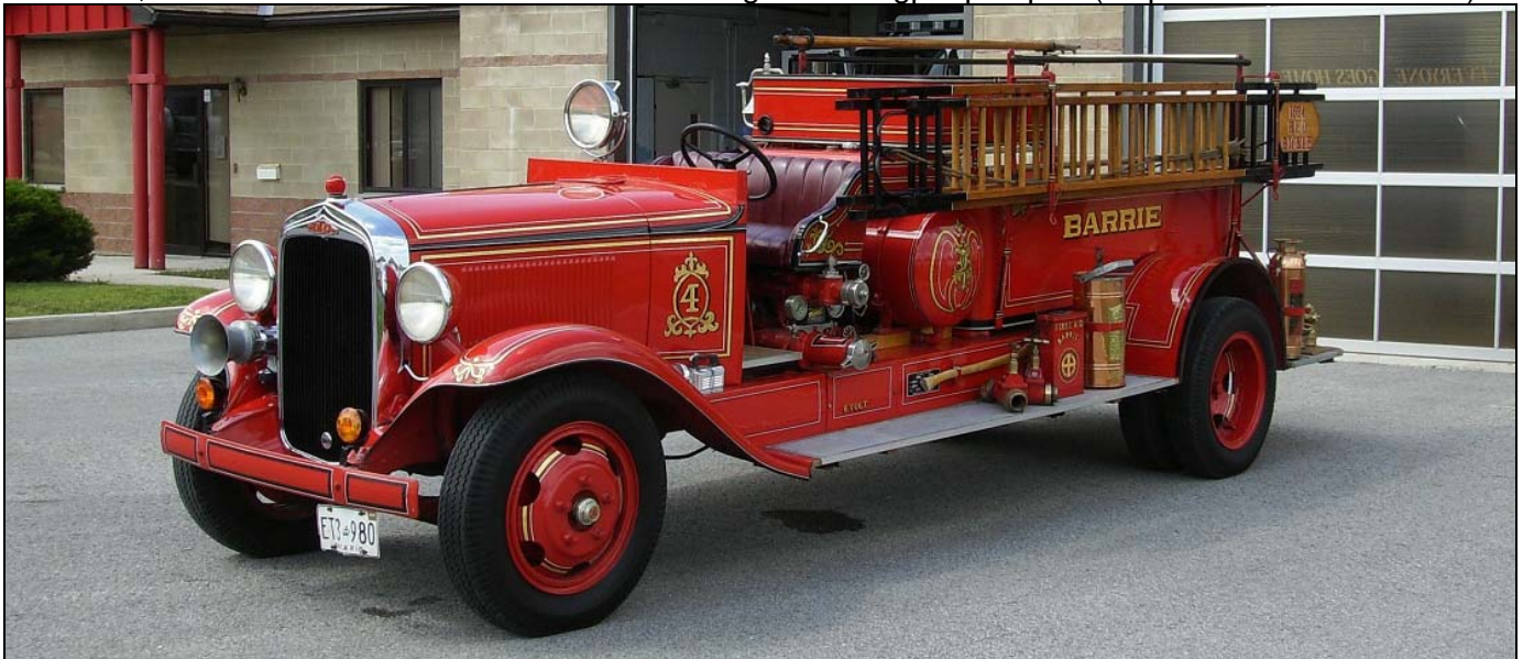
Still serving as a parade unit in Barrie, Unit 4 is a 1934 Reo/Bickle triple-combination, 400igpm & 80gtw.
