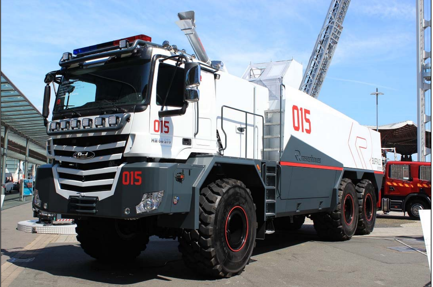
The Rosenbauer Buffalo Extreme off-road rig is a fully customizable 3-axle tanker with up to 33,000L on board. It carries an N65 6500LPM pump and 6000LPM monitor. This unit was built on a 2015 Paul Heavy Mover 68-570 6x6 chassis with a top speed of 65kph, it is intended for mining and fuel complexes.
