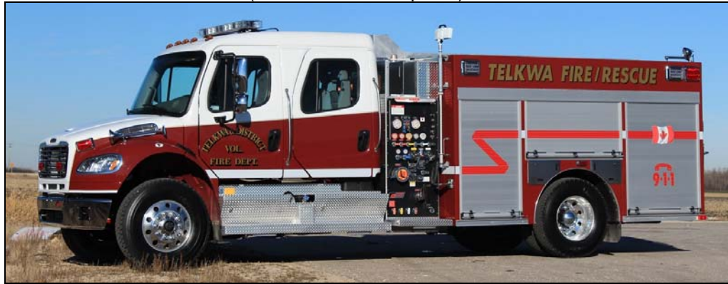
Telkwa, BC 2015 Freightliner M2-106/Fort Garry 1050igpm/300gwt/25gft s/n M639
