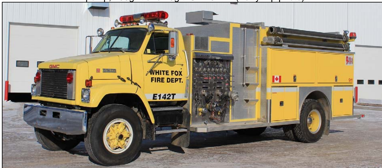
White Fox, SK still runs this 1987 GMC Brigadier 8000/Superior pumper-tanker. It has an 840igpm pump and a 1000gwt that used to belong to Orillia, ON (SN SE 823)
