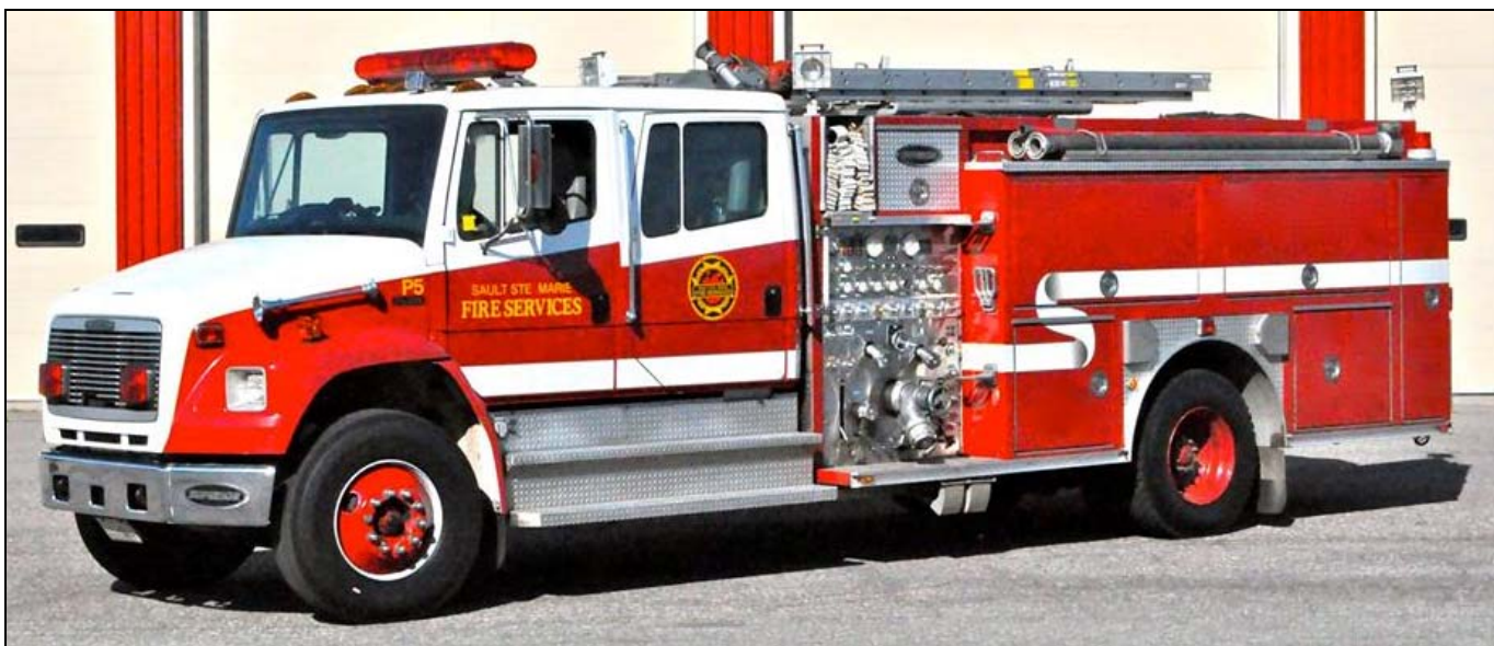
Sault Ste. Marie, ON P.5 1995 Freightliner FL106 / Superior pumper 1050igpm pump, 800gwt.
