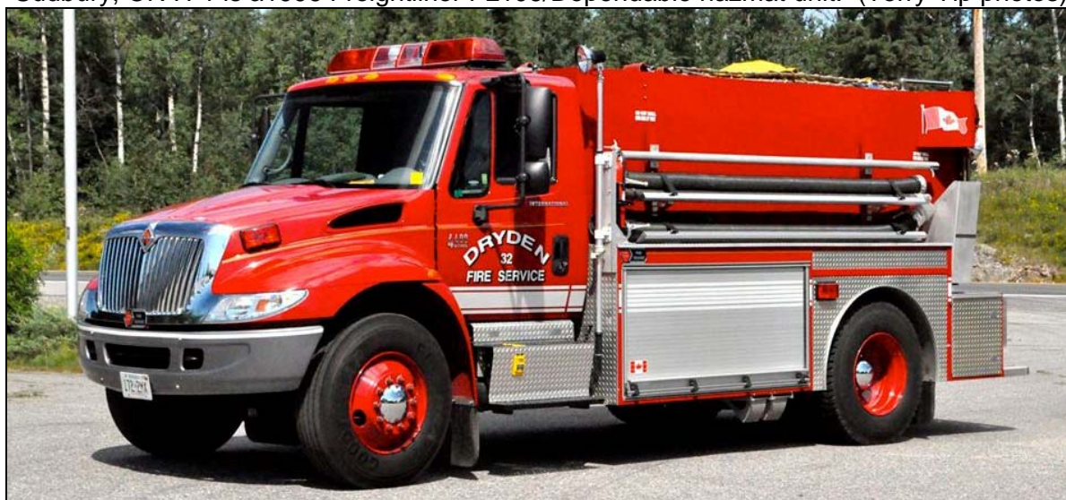
Dryden, ON Tanker 32, a 2004 International 4400/Fort Garry tanker, 550igpm pump, 1500gwt.
