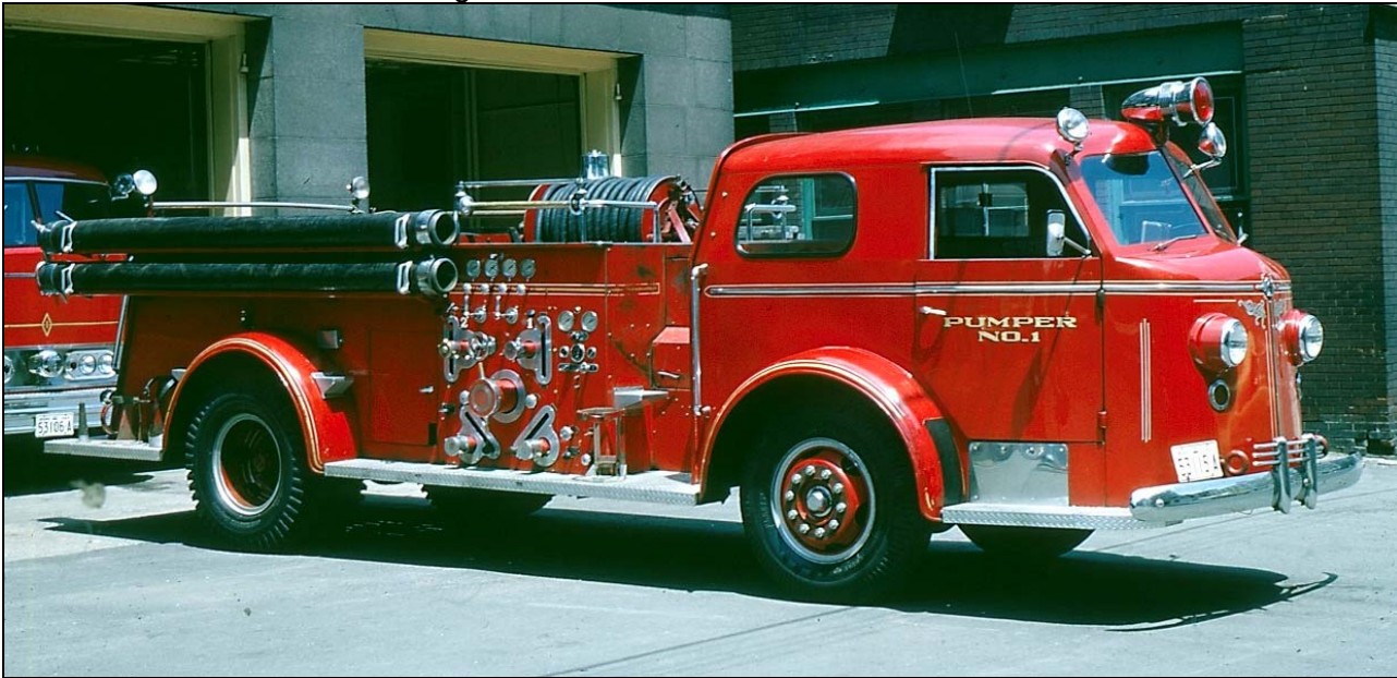
Pumper 1's 1948 ALF 700 series pump on the tarmac at Adelaide St., its replacement, a 1961 Mack, can be seen behind it. It had an 840igpm pump and 125gwt. (All photos Harold McMann)
