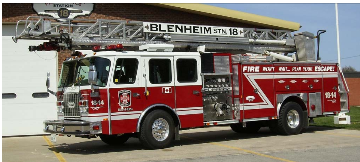
From Ontario, Chatham-Kent Aerial 18-14, assigned to Blenheim. It is a 2000 E-One Cyclone II quint with a 1750igpm pump, 500gwt and 75'aerial. SN 121968. (Neil McCarten photo)
