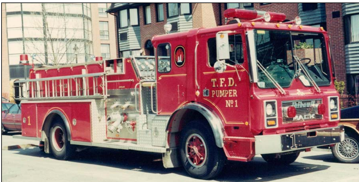
More Toronto Macks...This 1986 Mack/Thibault ran from Adelaide St. HQ with a matching 100' aerial. It had a 1050igpm pump and 300gwt. (Desmond Brett photos)
