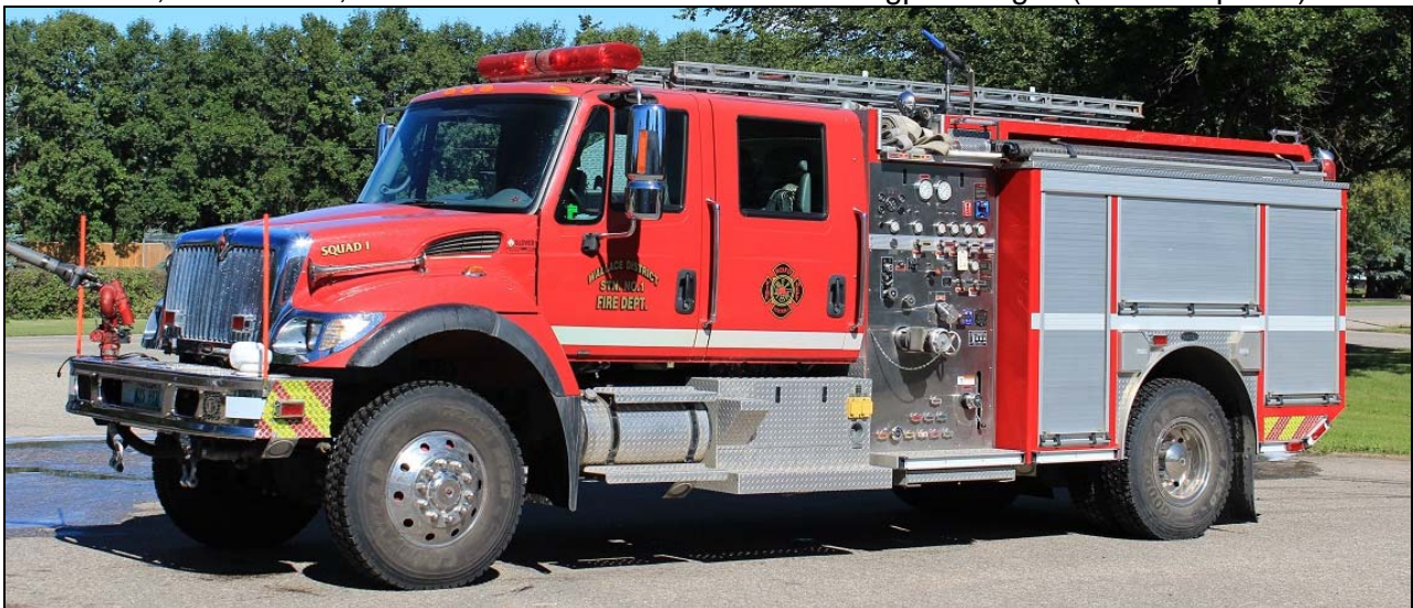
Viridien, MB has this 2006 IHC 7400/E-One pumper running as Squad 1. It has a 325igpm pump, an 800gwt, and 50gft.s/n SE 3492 (Dave Stewardson photo)
