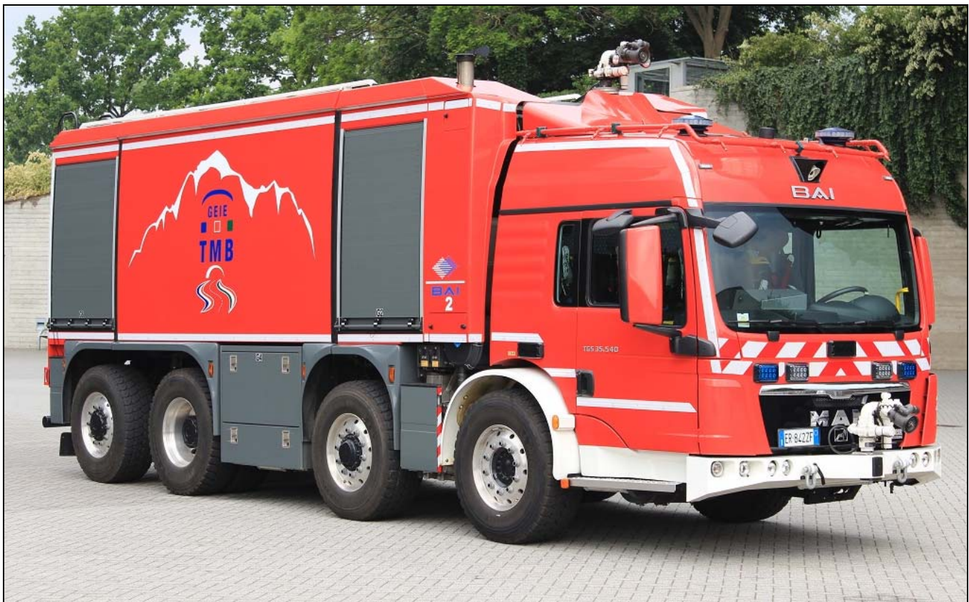
Above is a BAI Proteus Tunnel Rescue vehicle on a 2015 MAN chassis, built for the Mont Blanc Tunnel Co. (TMB). It has three driving axles and three steering axles for maneuverability. Below, a Polish built Wiss command unit on a 2014 Renault D12 chassis. Unit 303W98 is in service in Warsaw.
