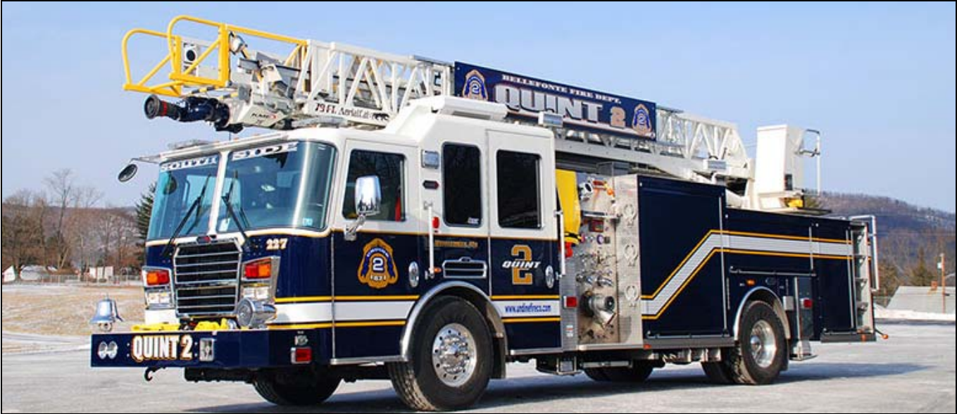
This is Bellefonte, PA Quint 2, run by the Undine Fire Co. #2. All four of the company's rigs are done in this striking colour scheme, including an immaculate Mack/Baker Aerialscope. Q.2 is a 2014 KME Aerialcat, 2000gpm pump, 500gwt, 79' stick. SN 8506. (KME delivery photos)
