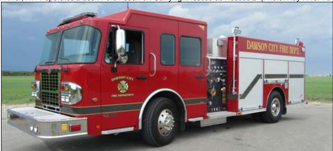
Dawson City, YT runs this 2015 Spartan Metro Star/Fort Garry engine equipped with a 1050igpm pump and 800gwt. SN 4260 (Fort Garry Fire Apparatus photo)
