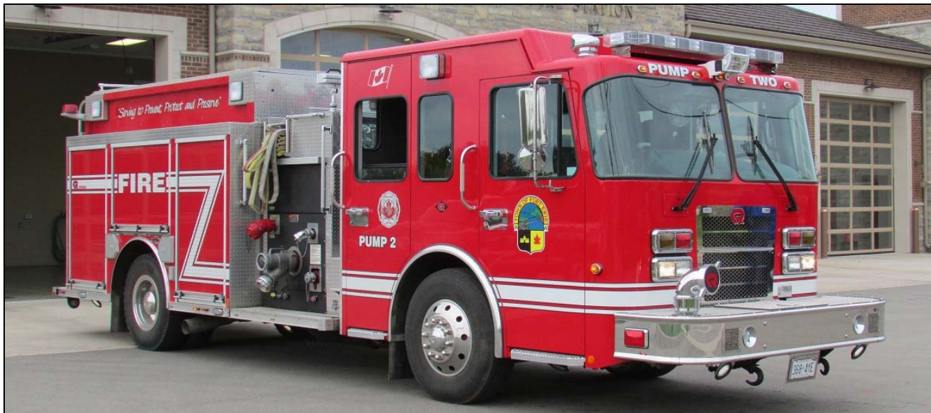
Fort Erie Pump 2 is a 2009 Spartan Metro Star/Rosenbauer product, with a 1050igpm pump, 840gwt and 20gft. (Desmond Brett photo)
