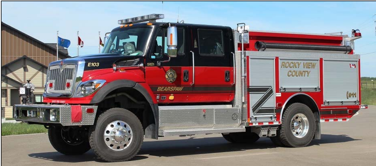
Rocky View, AB E.103, 2015 IHC 7400 4x4/Rosenbauer 840igpm/600gwt/30gft s/n 16443 (John Bowerman photo)
