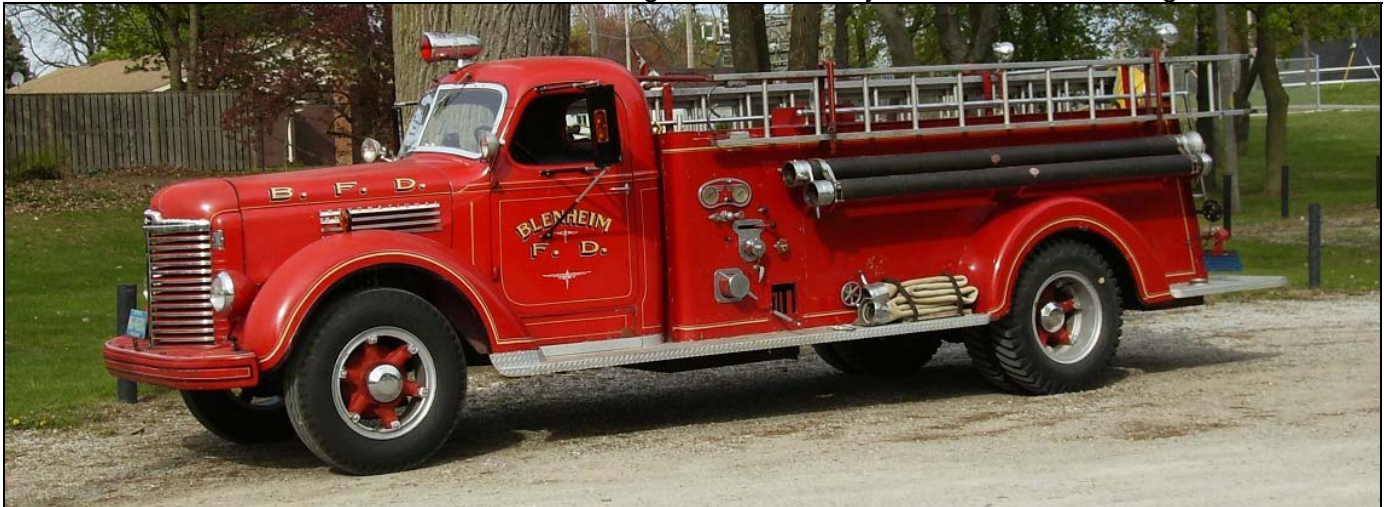
Blenheim, ON used to run this 1946 IHC/Bickle-Seagrave 450igpm pumper. (All photos: Neil McCarten)
