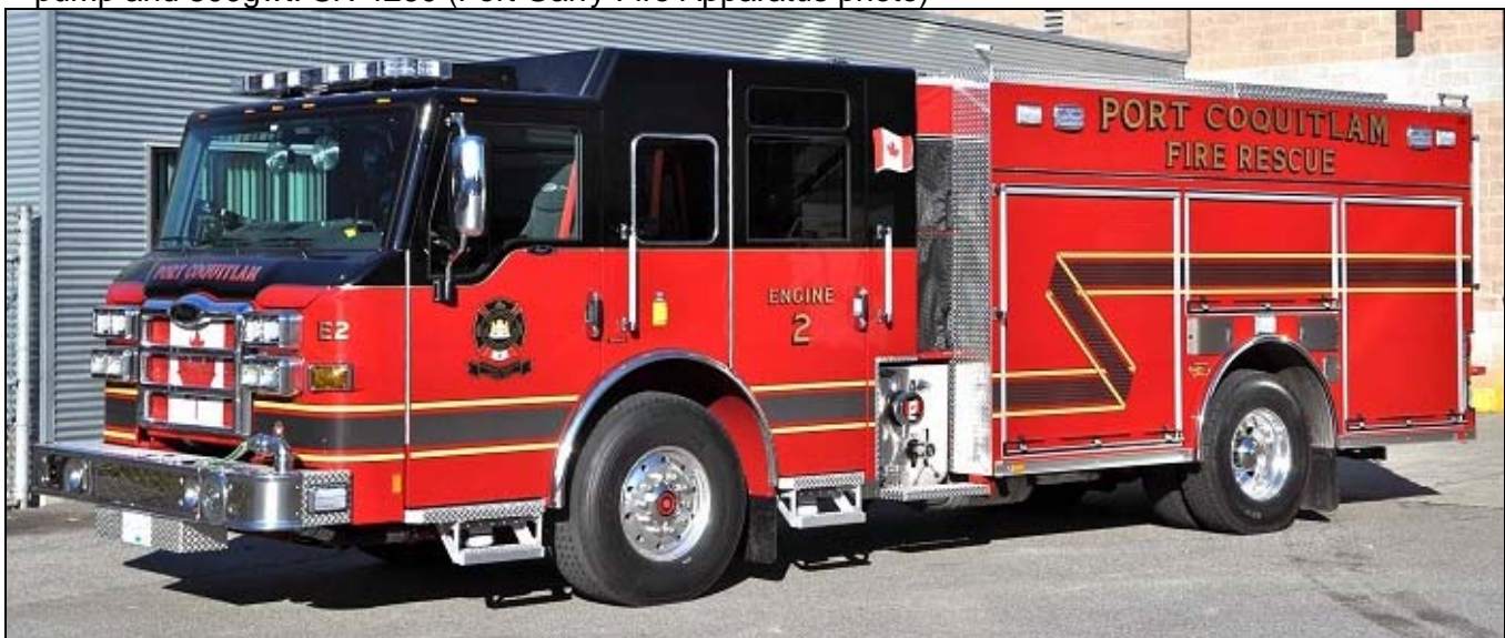
Port Coquitlam, BC Engine 2, a 2014 Pierce Impel PUC with a 1250igpm pump, 420gwt and 25gft. SN 27569 (Terry Yip photo)
