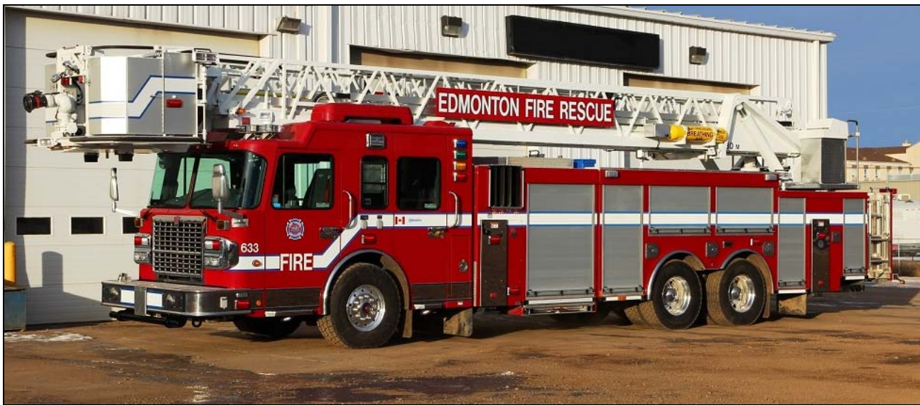
One of two units recently put into service in Edmonton, shop no. 633 is a 2015 Spartan Metro Star/Smeal 100' tower. They have 1500igpm pumps, 250gwts and /2x25gfts, the 2 nd rig is 634.
