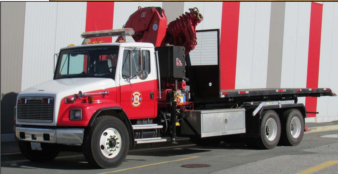
This is a Dedicated Fire Protection Unit, at the Vancouver, BC training centre. It's a 2000 Freightliner FL80 flatbed equipped with an Amco Veba Legend 63' crane for carrying pods. Body work done by VFD shops and Highway Products. (Desmond Brett photo)
