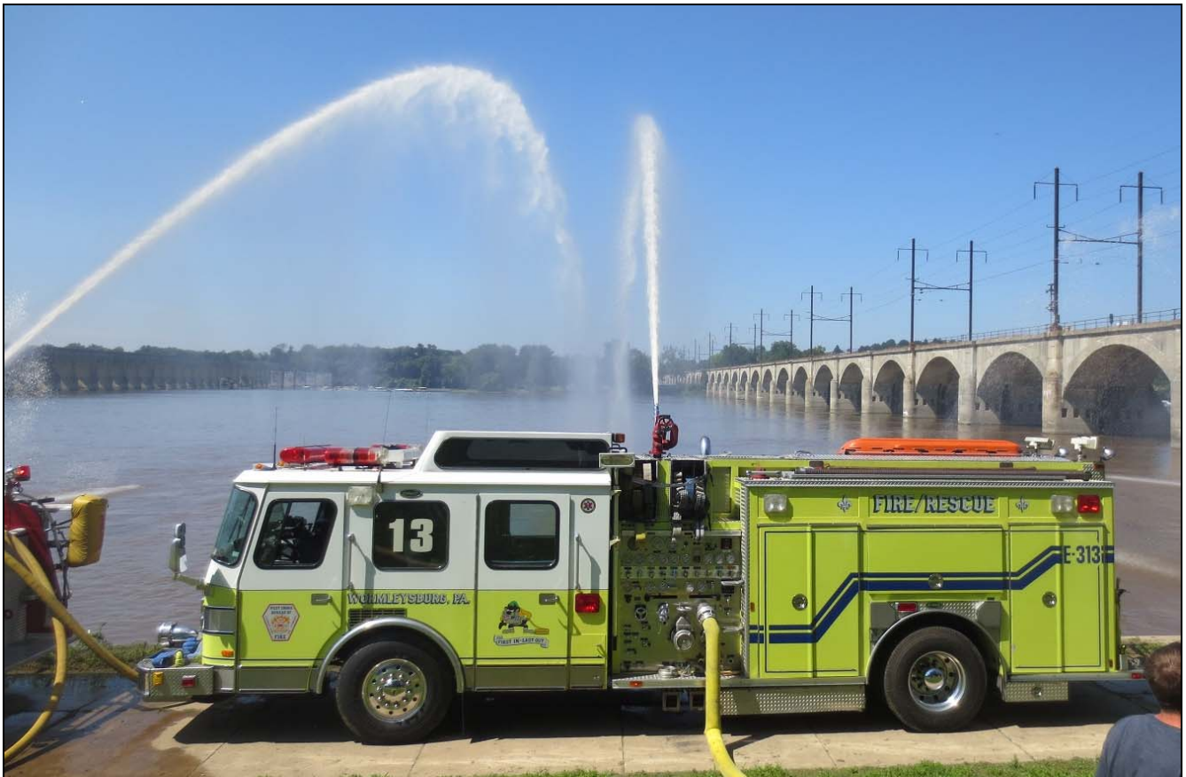
Now that we're deep into winter, here's a reminder of the very warm summer we experienced last year, taken at the Pennsylvania Pump Primers Muster in Harrisburg this past July. Above, Wormleysburg, PA Engine 3-13 lets go with a deck gun. It is a 1992 E-One Cyclone with a 1500gpm pump and 500gwt. Below, a panoply of antique and classic engines at work next to the Susquehanna River. (Greg Brown photos).
