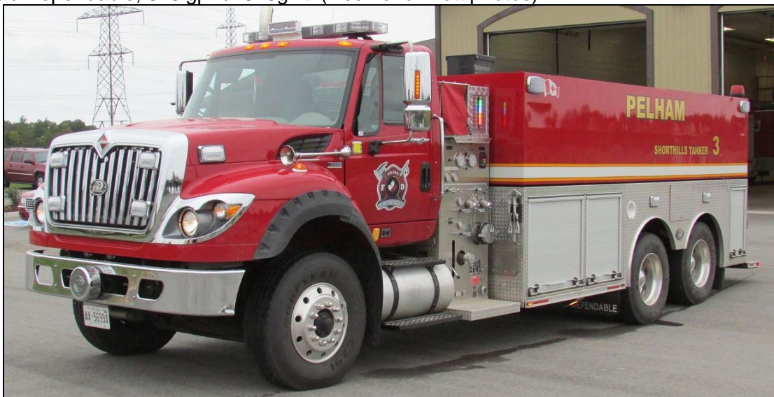
Pelham Rescue 3, a 2004 Ford F550/Fort Garry rig, and Tanker 3, a 2011 IHC Durastar/Dependable, 625igpm/2640gwt. (Desmond Brett photos)
