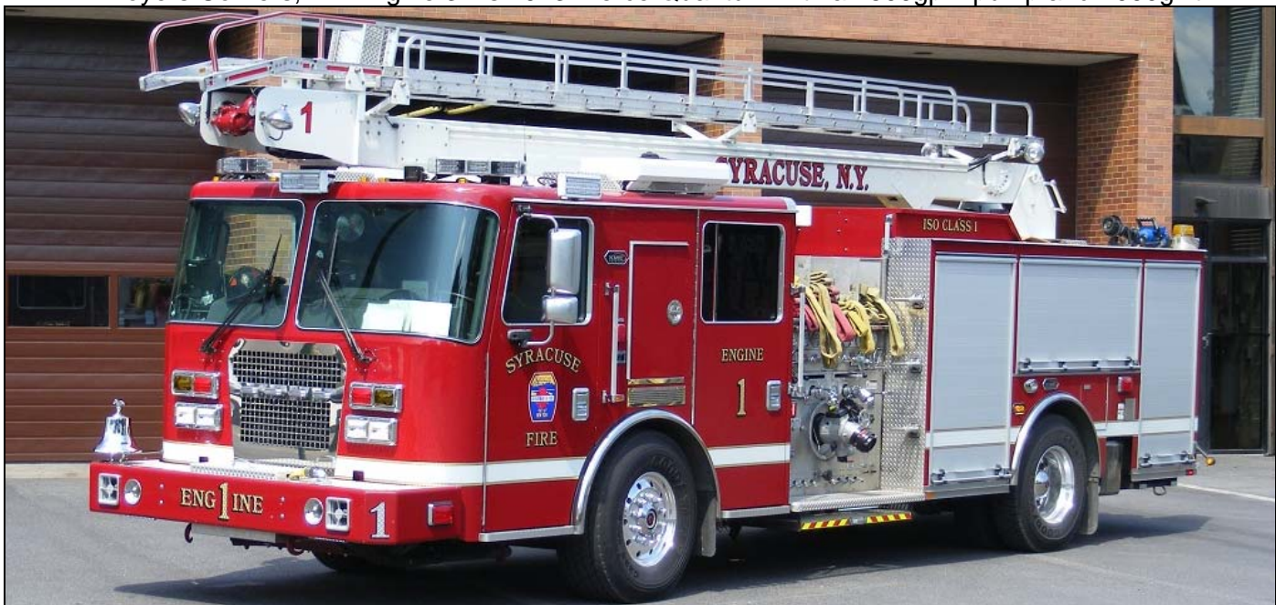
Syracuse, NY, Engine 1, a 2014 KME pumper, has 2000gpm pump, 500gwt and 55' aerial.
