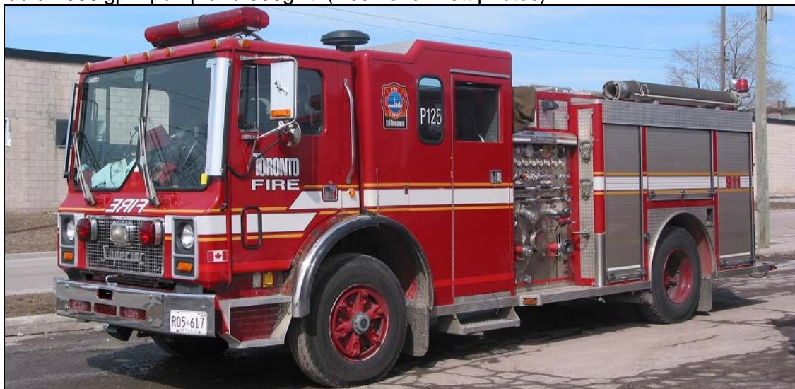
Many of the TFD Macks made it onto the roster of the new Toronto Fire Services. This 1988 MR688P/Superior pumper was later transferred out to Station 125. 1050/300 (SN#SE 935)
