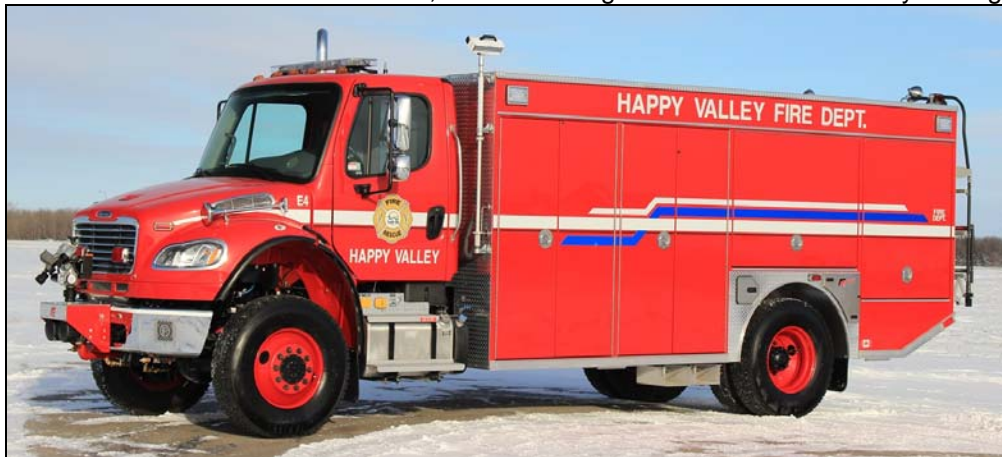
Happy Valley, AB E.4 2015 Freightliner M2-106 4x4/Fort Garry 1050igpm(D)/1000gwt /25gft s/n M648
