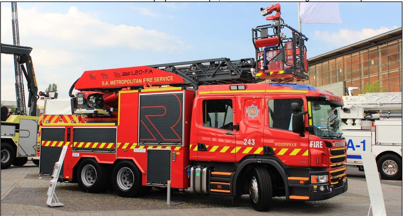
A Rosenbauer/Metz aerial-pump on a Scania P360 chassis for the South Australia Metropolitan Fire Service. It carries a Metz 20m platform, a full pump, tank and foam. It's assigned to Stn. 24 in Woodville.
