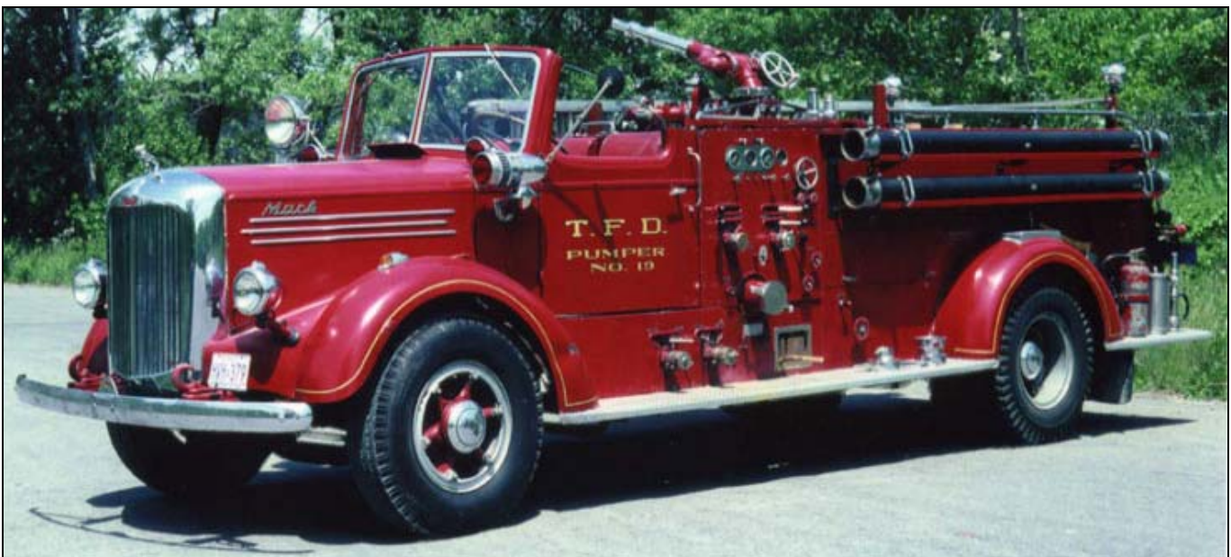
Toronto's last open cab pumper, a 1947 Mack 95LS with an 840igpm pump. (Neil McCarten photo)
