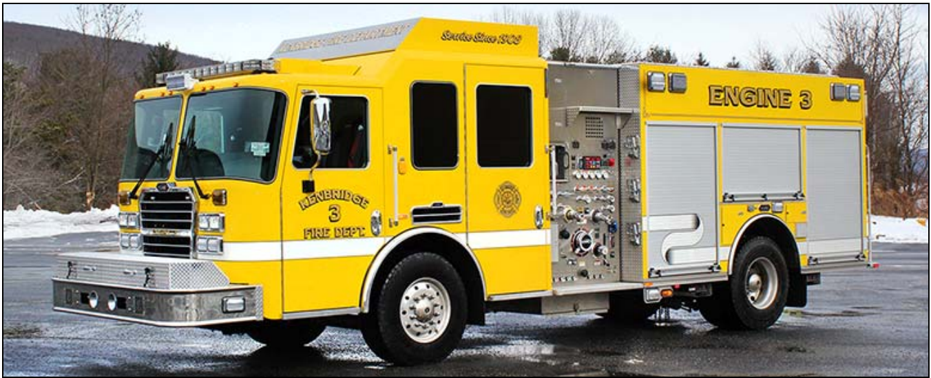
This bright yellow 2014 KME engine protects Kenbridge, VA. Engine 3 has a 1750gpm Hale pump, 1000gwt and 30gft along with FoamPro foam system (KME photo).
