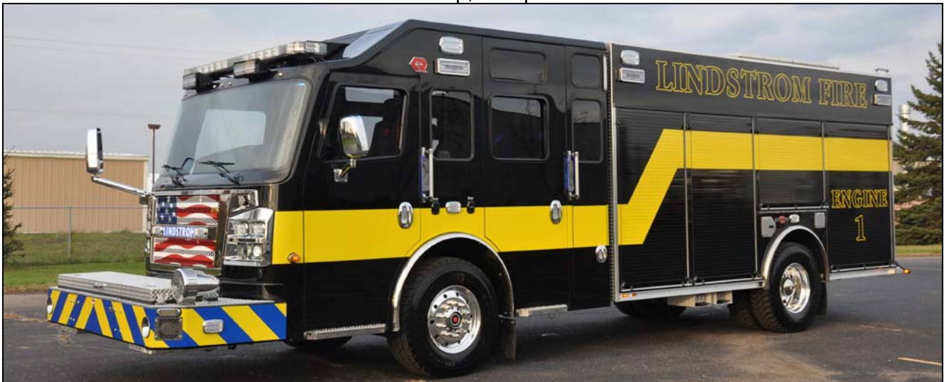
Linstrom, MN just received this 2015 Rosenbauer Commander engine. It has a Waterous rearmount 1500gpm pump, 850gwt and 20gft. S/N 14000. (Rosenbauer America photo)
