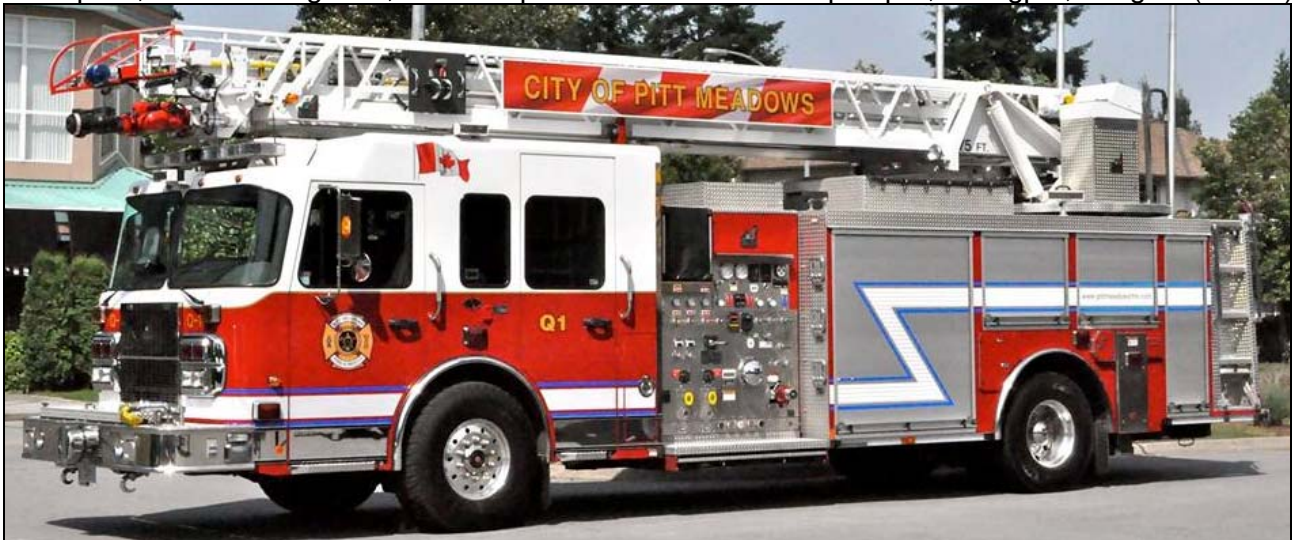
Pitt Meadows, BC bought this 2007 Spartan Gladiator Classic/Smeal aerial for Quint 1. It has a 1500gpm pump, 250gwt, 12gft(A), 20gft(B) and 75' aerial. Smeal Order # 3374. (Terry Yip photo)
