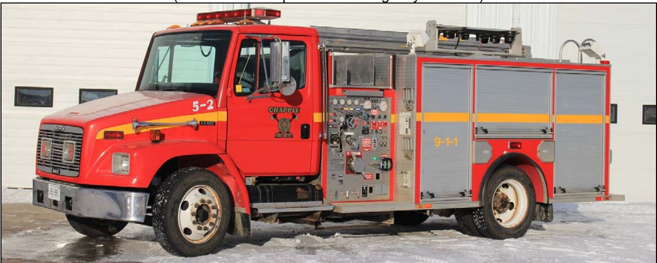
Chapple Twp., ON just bought this 2001 Freightliner FL-60/Maxi Metal 625igpm/250gwt/10gft s/n 17535-1. It's a 2015 Fort Garry rebuild, ex- Quebec City. (Dave Stewardson photo)
