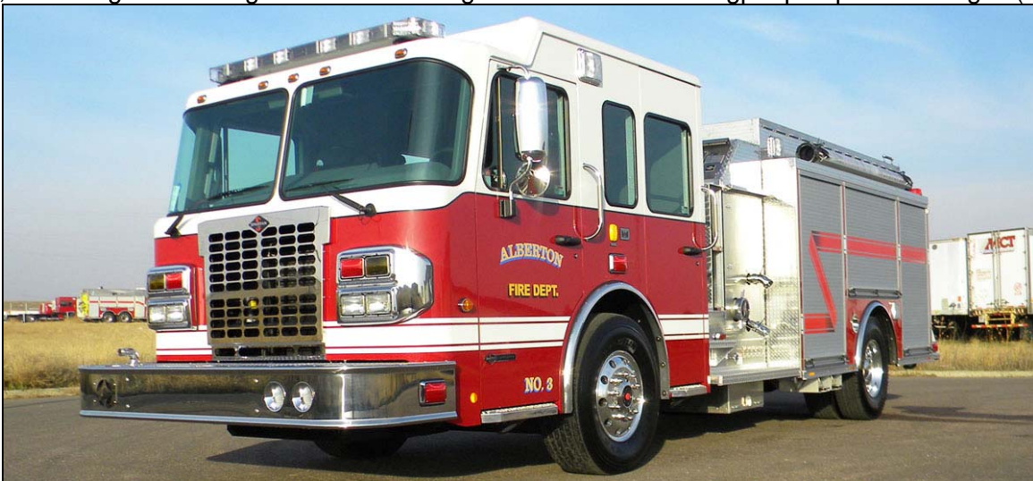
Alberton, PEI Pumper 3 is a 2012 Spartan Metrostar/Spartan ERV 1500gpm pumper with a 1000gwt and 30gft. SN 212085. (Photo credit: Dependable Emergency Vehicles)
