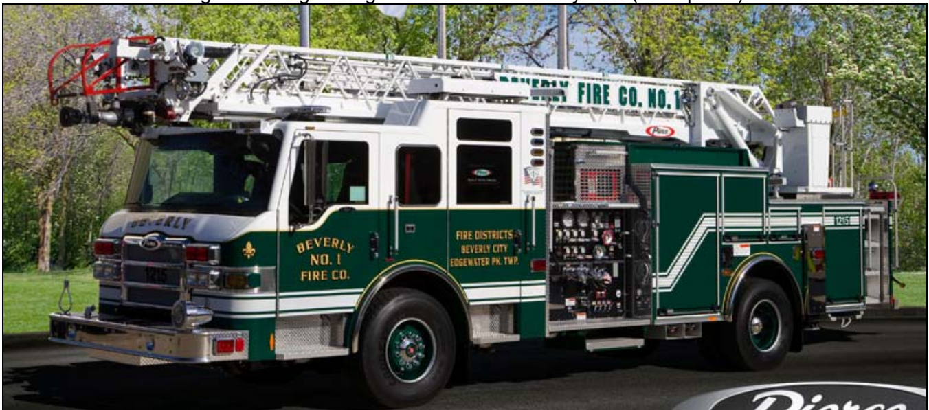
Beverly, NJ Ladder 12-15 is a 2010 Pierce Impel quint, 1500gpm, 400gwt and 75' aerial. (Pierce Fire)
