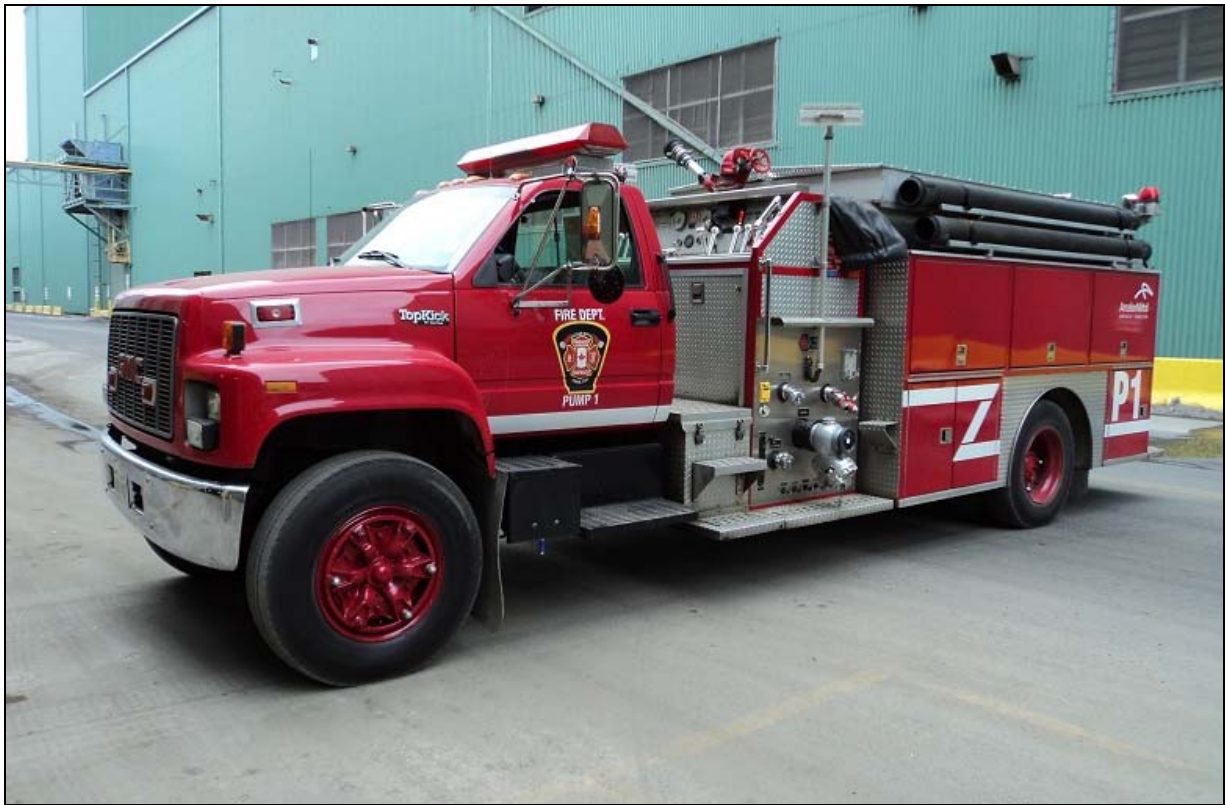
Newly repainted, this is Dofasco Pumper 1, a 1996 GMC Topkick/Fort Garry pumper, equipped with a 1050igpm pump and 500gwt. (Ken Buchanan photos)
