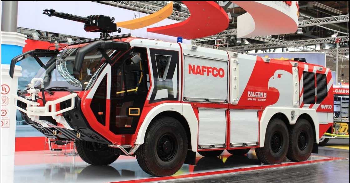
This NAFFCO Falcon 6 CRT was built in Dubai. It has an 8,000LPM pump, 12,500LWT and 1500LFT.
