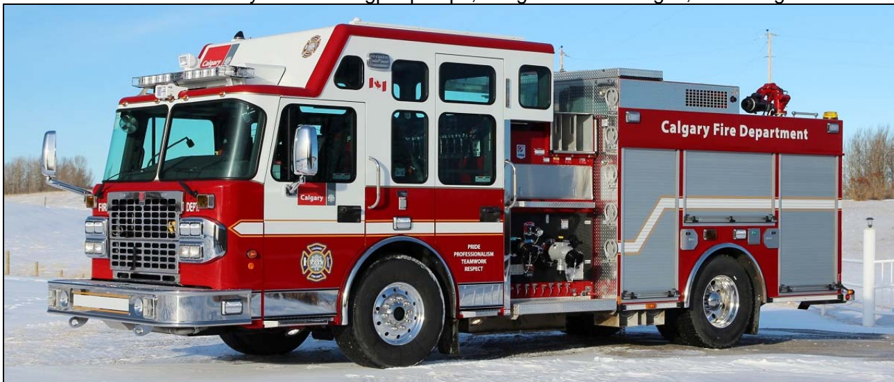
Just delivered to Calgary, the first four of an order of Sixteen 2016 Spartan Gladiator/Smeal pumpers. Each rig has a 1500igpm pump, 500gwt, 30gft and a CAFS. (John Bowerman photos)
