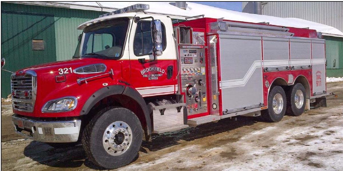
Brookfield, NS 321 got this Freightliner/Metalfab rig in 2014. It has a 625igpm pump and 2000gwt (Metalfab)
