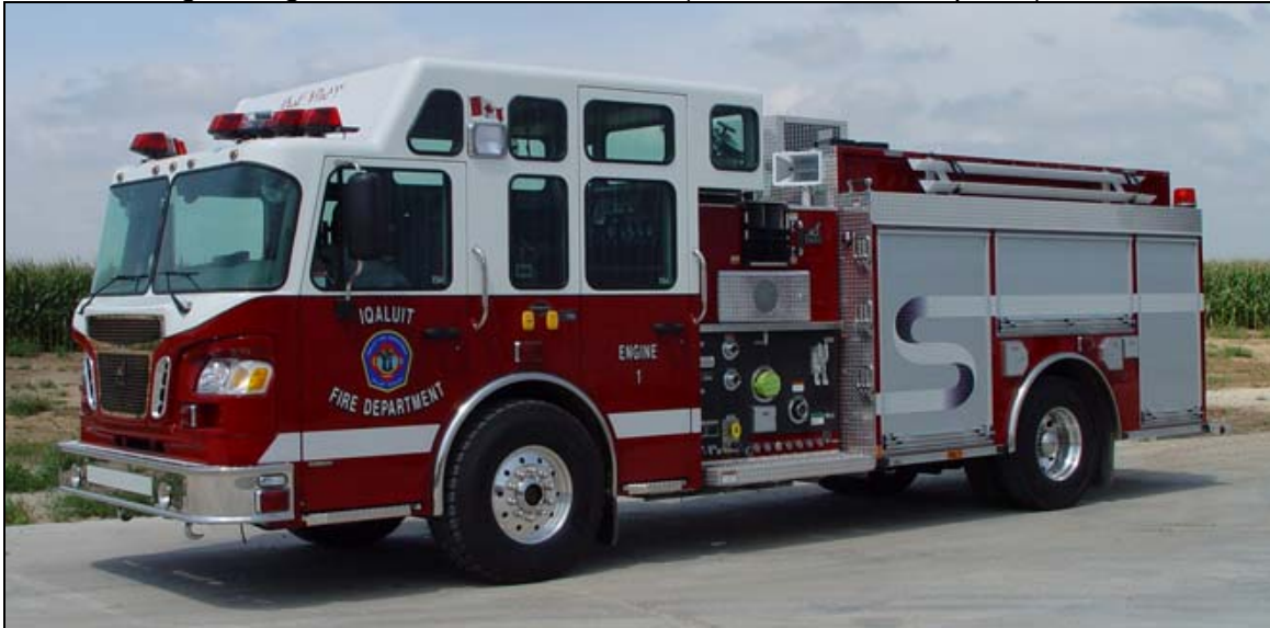
Iqaluit, Nunavut Engine 1, a 2007 Spartan Diamond/Smeal pumper, 1500igpm, 840gwt. (Smeal)
