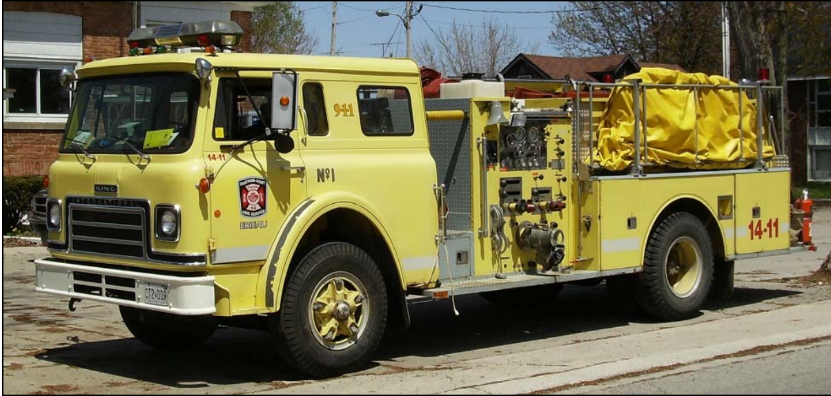
Chatham-Kent 14-11 from 2007. This 1981 IHC S1800/King pumper was formerly Erieau Pumper 1, it had a 625igpm pump and 800gwt. (Neil McCarten photo)
