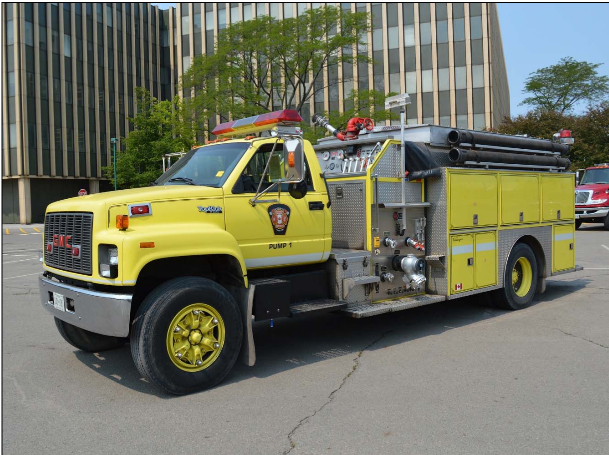
Newly repainted, this is Dofasco Pumper 1, a 1996 GMC Topkick/Fort Garry pumper, equipped with a 1050igpm pump and 500gwt. (Ken Buchanan photos)
