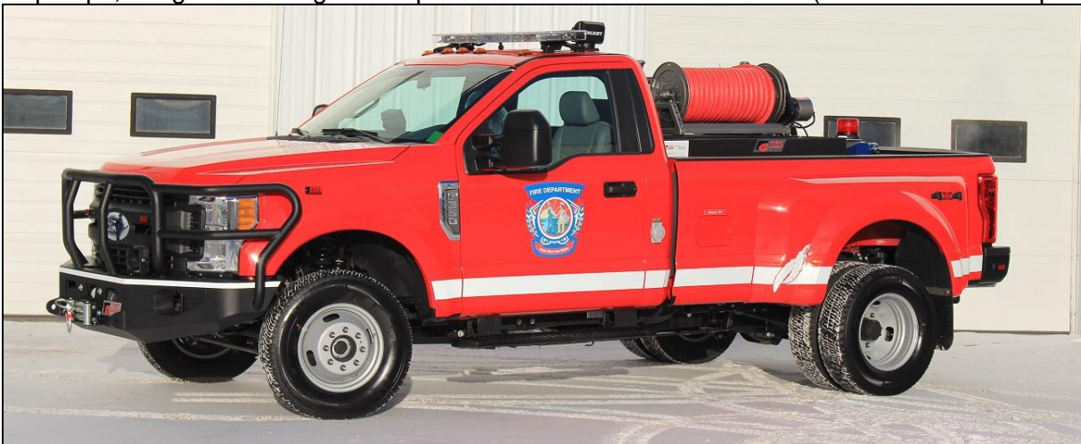
Fisher River Cree Nation, MB just took delivery of this 2017 Ford F350 4x4 /Fort Garry brush rig with a 312igpm Darley pump, 200gwt and 10gft. s/n M881 (Dave Stewardson photo)
