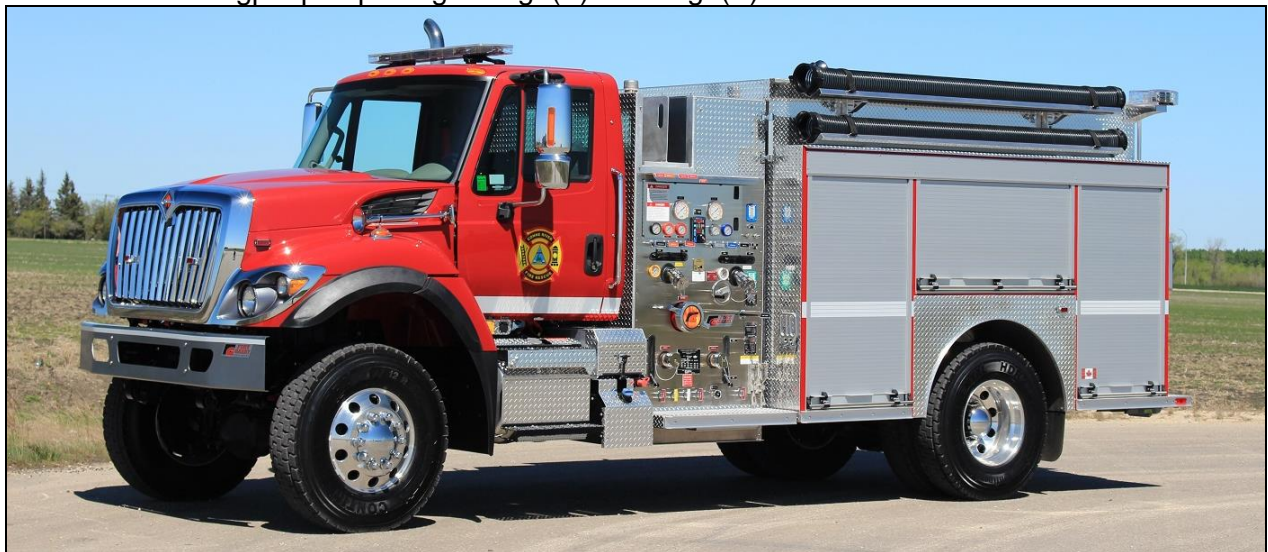
Miawpukek FN in Conne River, NL received this 2017 IHC 7400/Fort Garry rig last May. It has a 1050igpm Darley pump, 1000gwt, 25gft and a FoamPro 1600 foam system. (Dave Stewardson pics)
