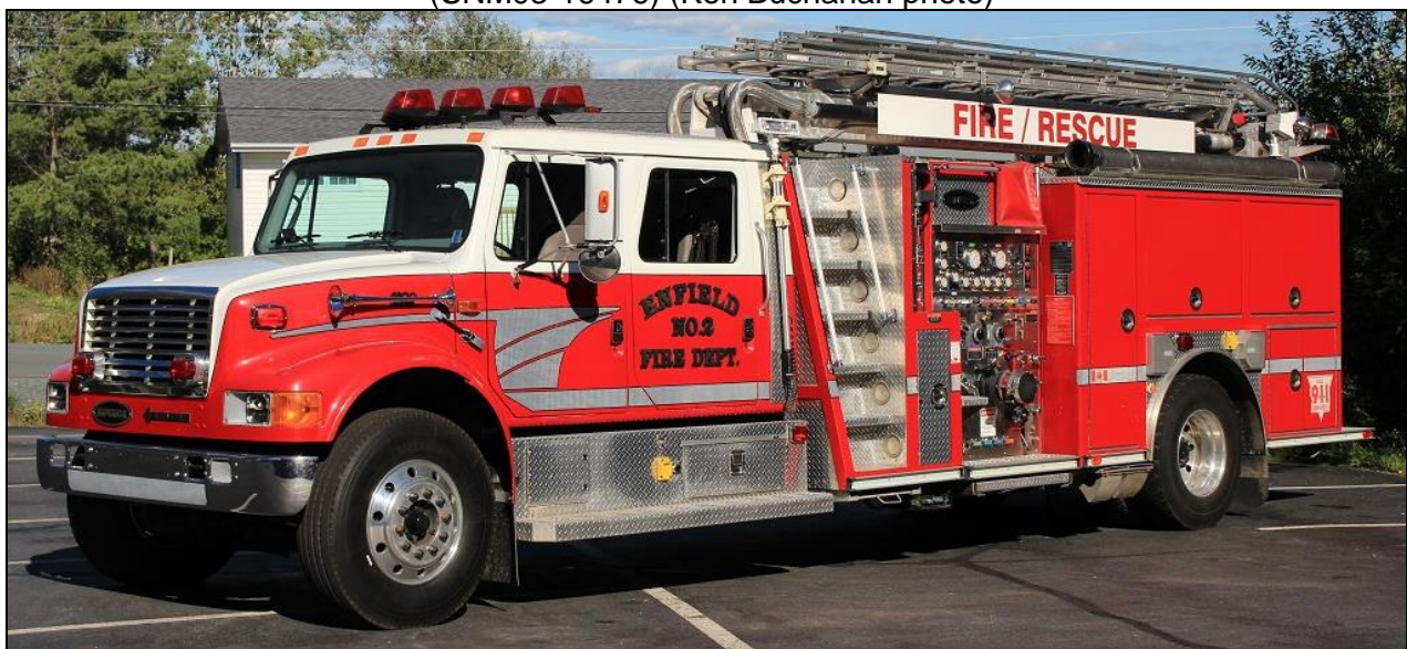
Enfield, NS No. 2 is a unique 1999 IHC 4900/Superior midmount teleboom. It's equipped with a 1250igpm pump/500gwt/10gft(A) and 20gft(B) with a 50' aerial. #SE1937
