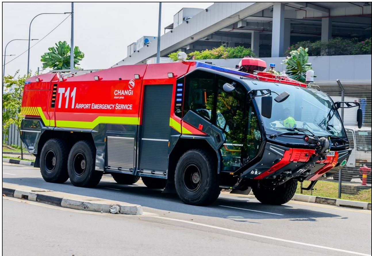
Changi Airport T.11, a 2017 Rosenbauer Panther 6x6 CRT, with an N80 9,000LPM pump, 12,000LWT, and 1500LFT. (Kenneth Lai photos)
