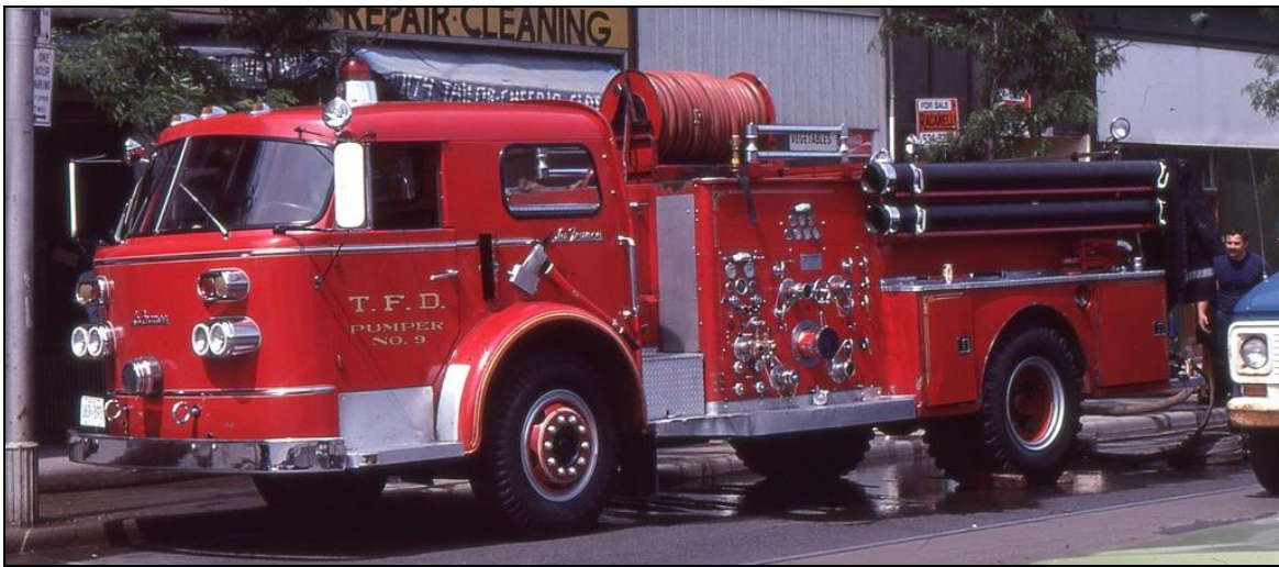
The last custom ALF rigs bought by the TFD were a pair of 1963 900 Series pumpers for Stations 9 and 19. The identical rigs had 840igpm pumps and 250gwts.
