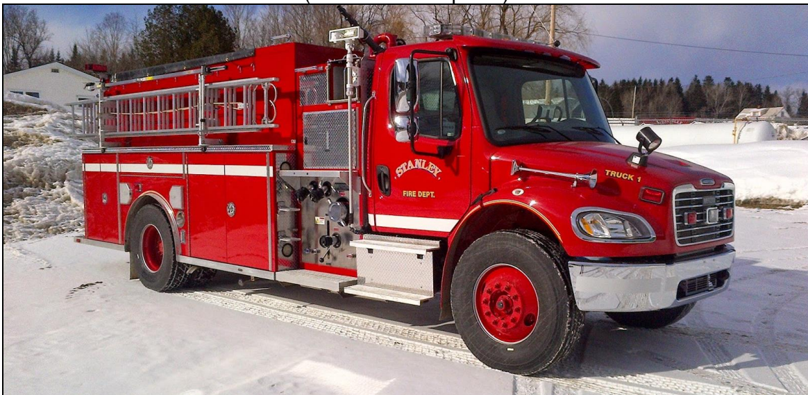
Stanley, NB Unit 1: 2014 Freightliner M2-106/Metalfab 1250igpm/1200gwt. (Metalfab)
