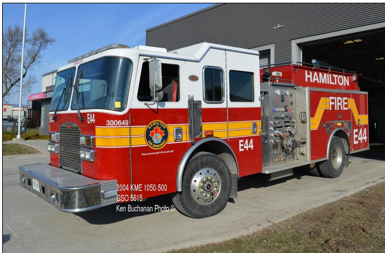
In Hamilton, a new assignment for this 2004 KME pumper, now running as reserve Engine 44. It has a 1050igpm pump and a 500gwt. (Ken Buchanan photo)
