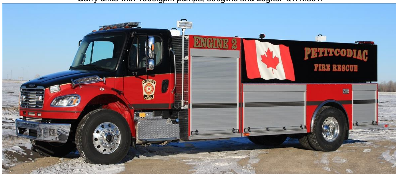
Petitcodiac, NB Engine 2, a 2017 Freightliner M2-106/Fort Garry pumper-tanker with a 1050igpm Hale pump, 1200gwt, 25gft and a FoamPro 2001 foam system. s/n M877 (Dave Stewardson photos)
