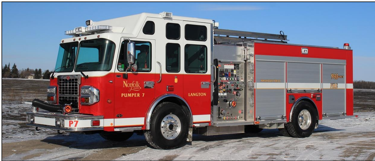
Norfolk County, ON Pump 7, a 2017 Spartan Metro Star/Fort Garry rig equipped with a 1250igpm Hale pump, a 800gwt and a 25gft. Job number M855.
