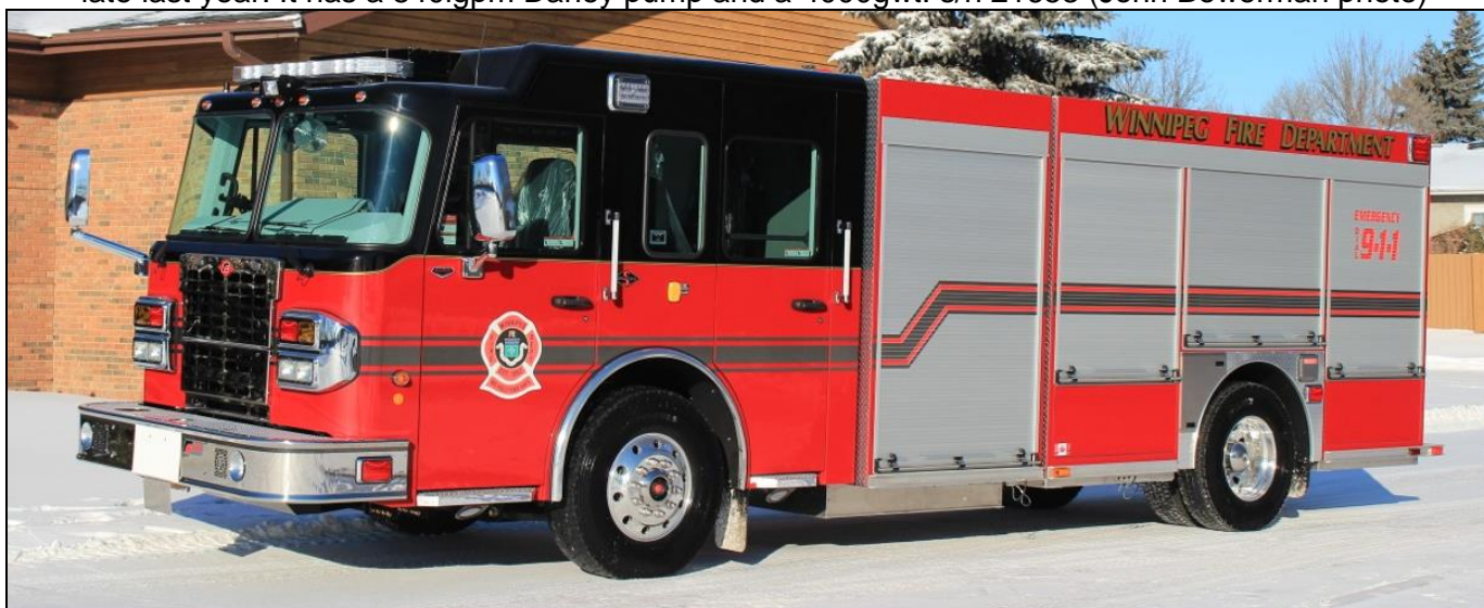
The first of four new rescue pumps for Winnipeg, MB. They are all 2018 Spartan Gladiator Classic/Fort Garry units with 1500igpm pumps, 600gwt and 25gfts. s/n M851.
