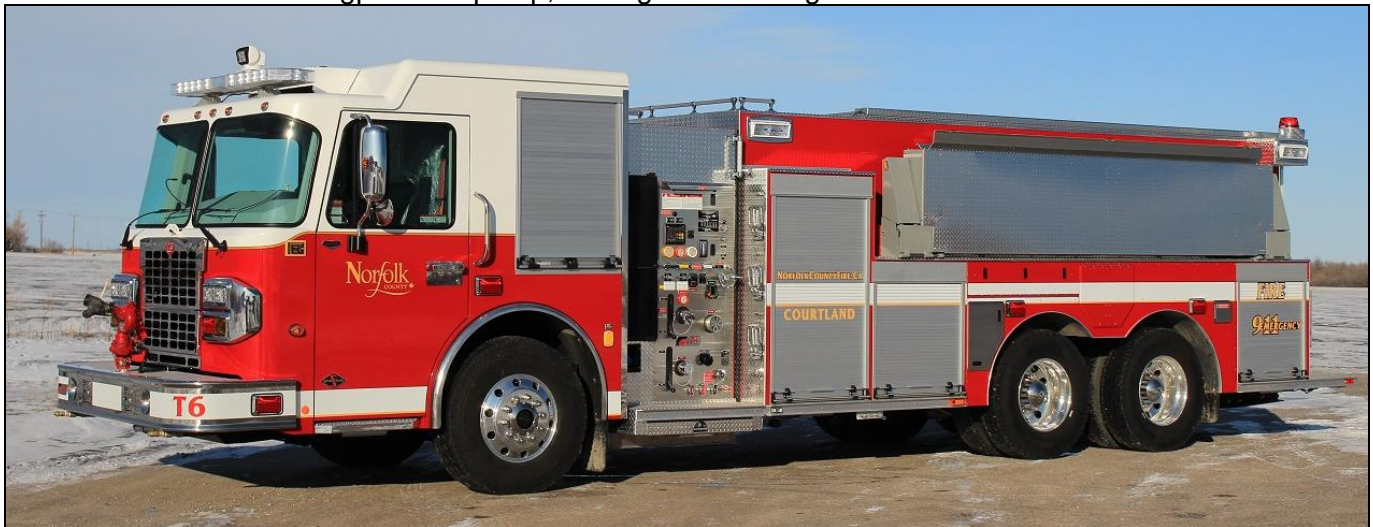
Norfolk County Tanker 6 is a 2017 Spartan Metro Star/Fort Garry collaboration with a 289igpm pump and a 2000gwt. Job Number M853. The new Tanker 1 is identical. (Dave Stewardson photos)
