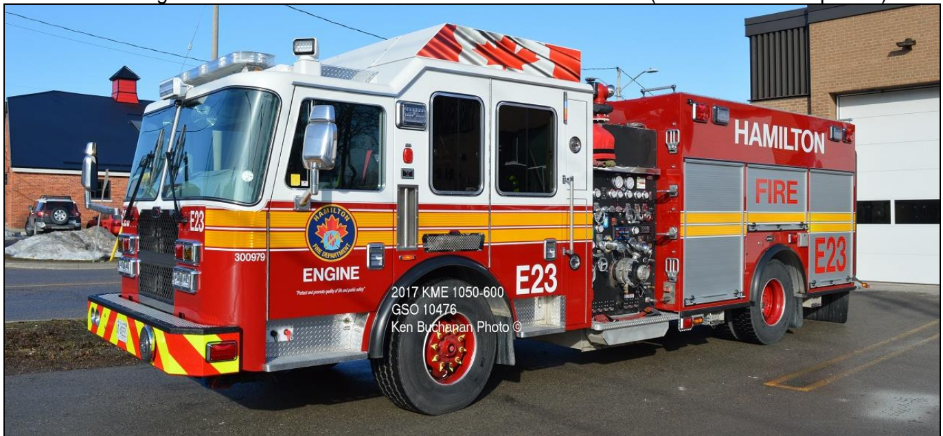
Hamilton's new Engine 23, a 2017 KME Severe Service pumper, 1050igpm pump, 600gwt. (Ken Buchanan photo)
