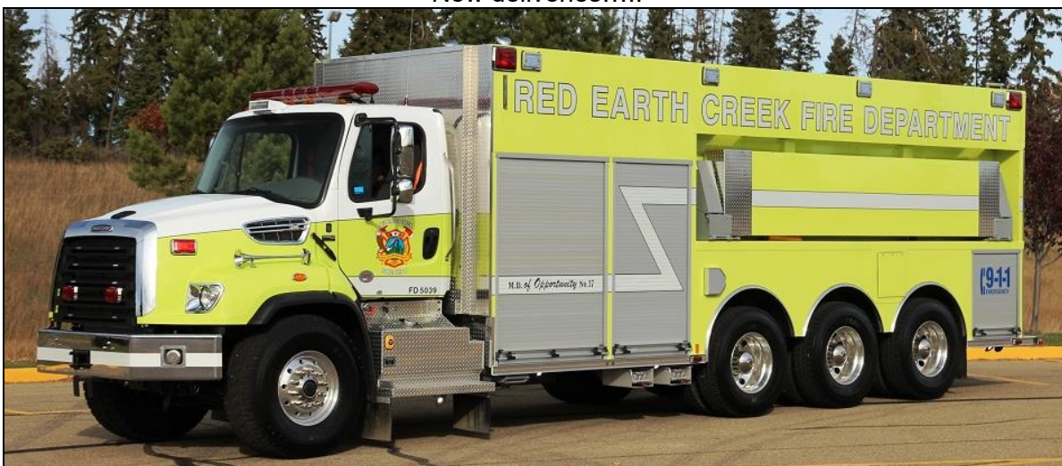
Red Earth Creek, AB, received this 2017 Freightliner M2-114SD/Rosenbauer four-axle tanker late last year. It has a 840igpm Darley pump and a 4000gwt. s/n 21653 (John Bowerman photo)
