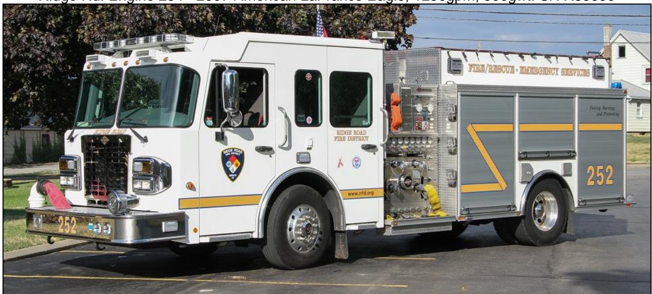
Ridge Rd., NY Engine 252, a 2013 Spartan / Spartan ERV pumper, equipped with a 1250gpm pump and 500gwt. SN 212185-01. (Ian Duke photos)
