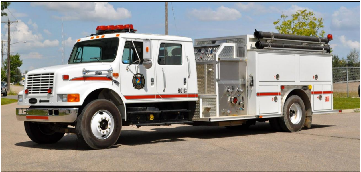
Wabasca, AB used to run this 1999 IHC 4900/Superior pumper, equipped with a x1050igpm pump, 900gwt and 30gft. It is now with the Foam Lake, AB FD.
