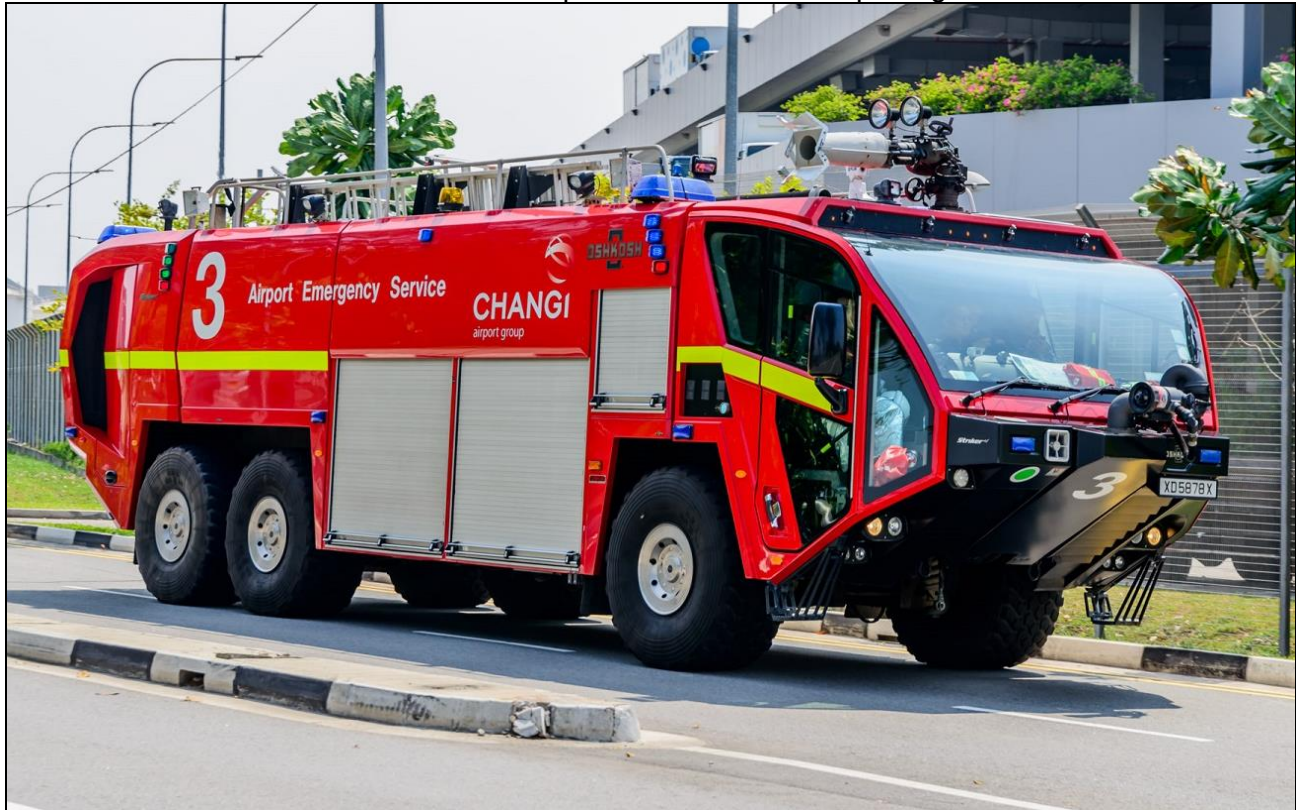
Changi Airport Red 3, a 2012 Striker 6x6, 2000gpm pump/3000gwt/420gft/550lbs DC.
