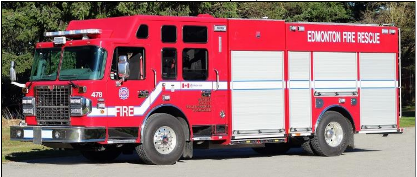
Edmonton, AB is getting no fewer than 13 of these 2017 Spartan Gladiator/Smeal pumps, all with 1500 igpm pumps, 400gwt and 60gfts. Shop Number 478 arrived in October. (Shane MacKichan photo)
