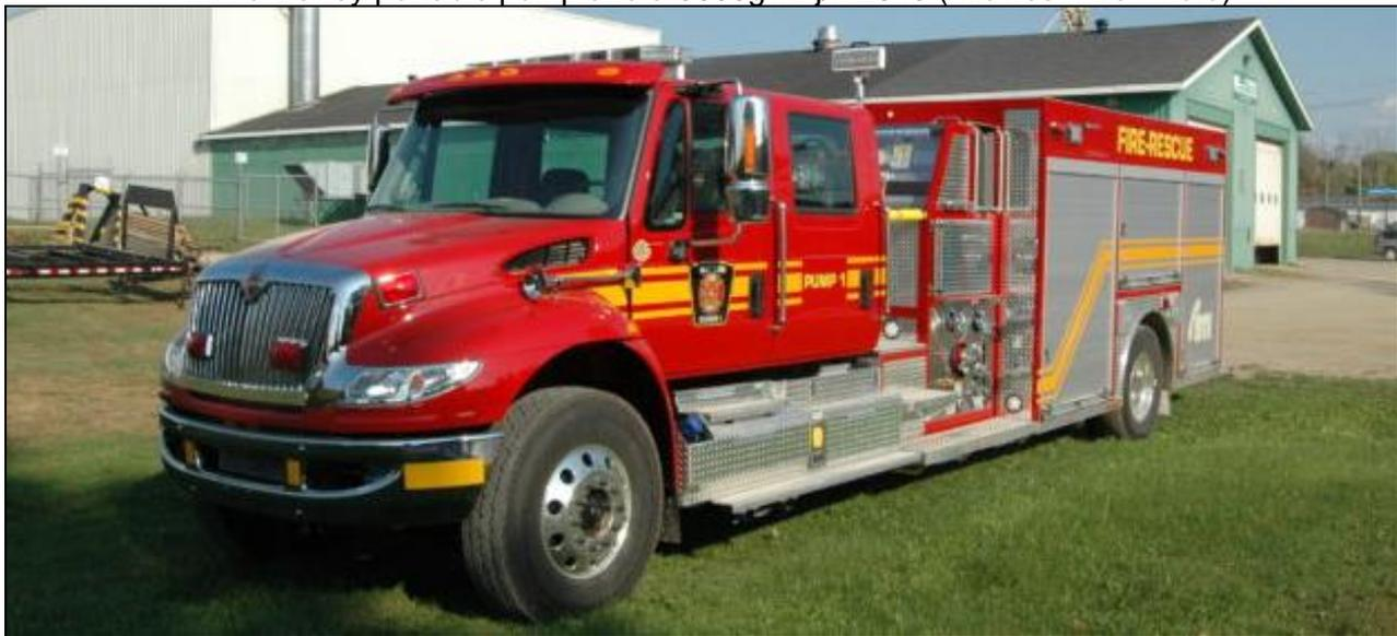
West Elgin Pump 1 is a 2017 IHC//Metalfab engine with a 1050igpm Hale pump and 1000gwt.
