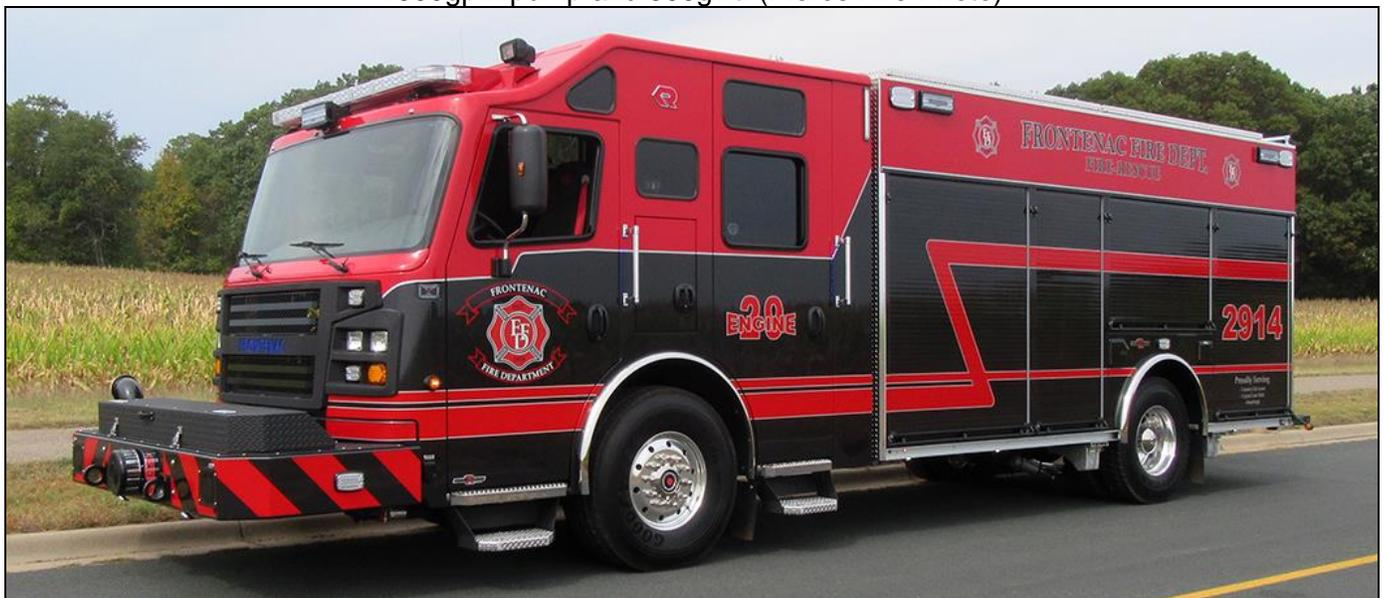
A very unusual bright red over black motif, found in Frontenac, MO. Engine 2914, a 2017 Rosenbauer Commander pumper with an S100 pump, 750gwt, and 32gft. j/n 14267. Rosenbauer U.S. photo)
