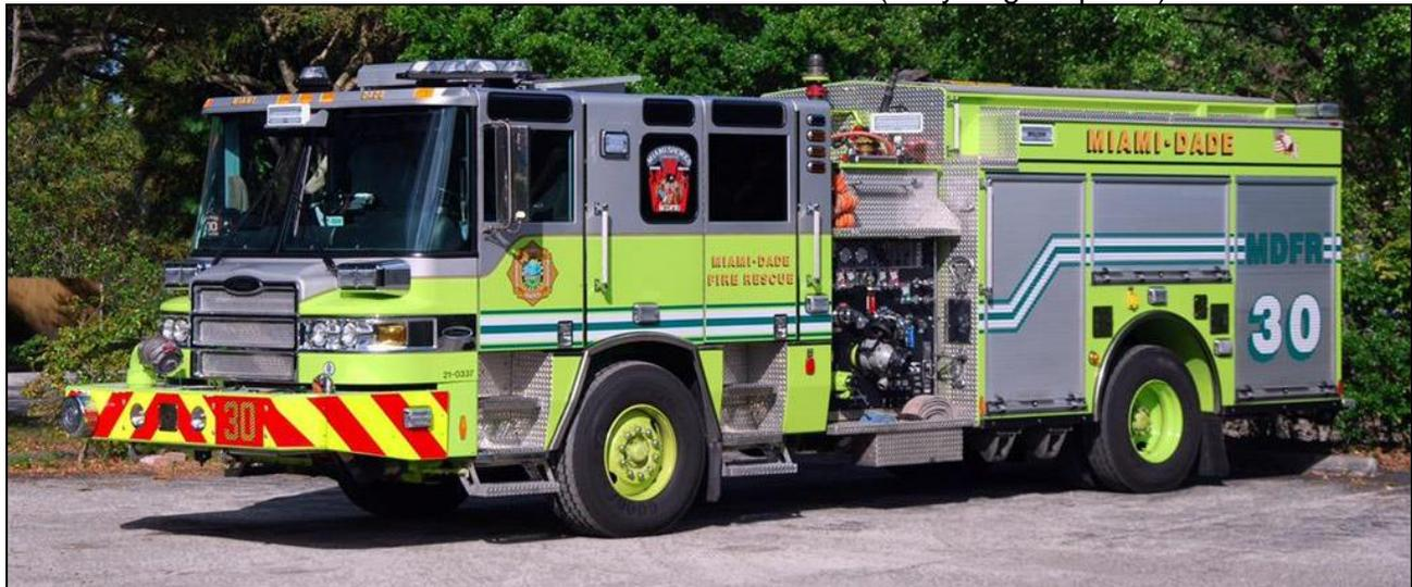
Miami-Dade, FL has a distinctive grey over lime set up. Engine 30 is a 2008 Pierce Arrow XT pumper with a 1500gpm pump and a 750gwt. (Pierce Fire Apparatus photo)
