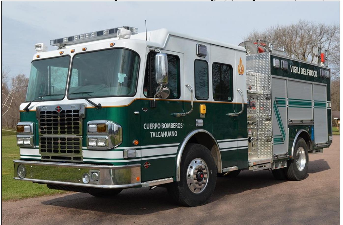
Chile is known for its colourful trucks. Talcahuano has a 2016 Spartan Metro Star/Spartan ERV rig with a 1250gpm Darley pump and a 1056gwt. s/n 215059 (Spartan ERV photo)
