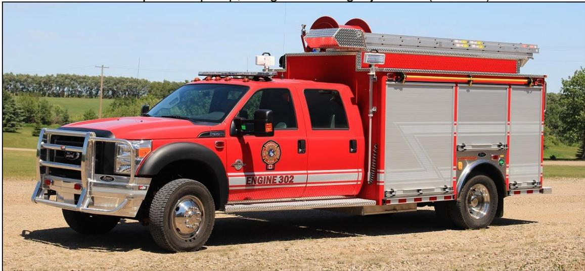
An Acres rig from 2017, this one for Transcona, MB. Unit 302 was built on a Ford F550 4x4 chassis with a 1050igpm Waterous pump, 500gwt and 20gft. s/n #170127149.
