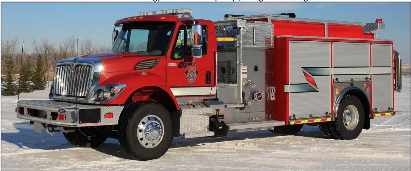
Holland, MB's newest, a 2017 IHC 7400/Acres pumper equipped with a 1050igpm Waterous pump, 1000gwt and 25gft. s/n 171117160. (Dave Stewardson photos)
