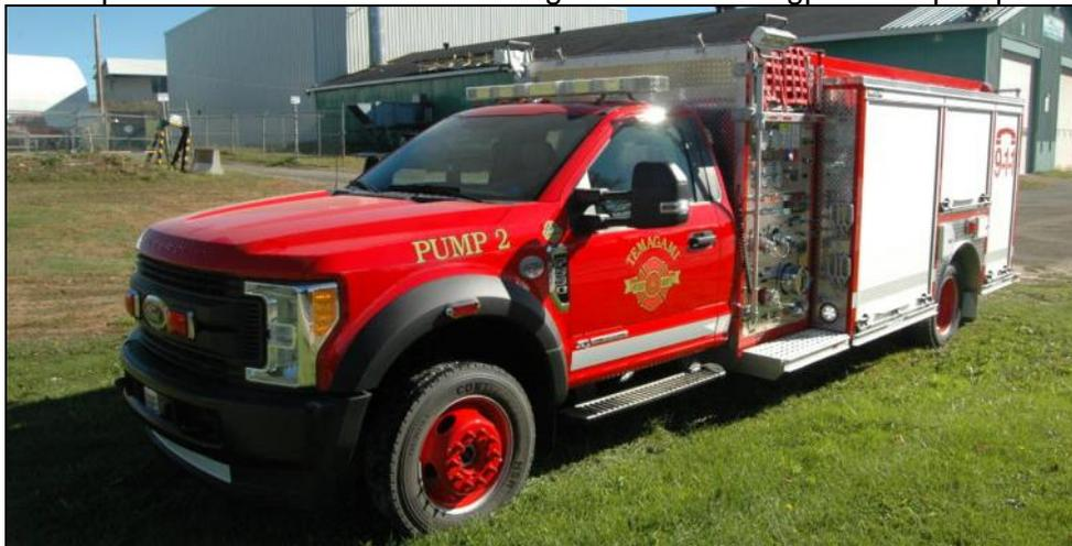
Temagami Pump 2, a 2017 Ford F550 4x4/Metalfab light pumper with 1050igpm Hale pump, 300gwt and FoamPro 1600 foam system. (Metalfab Fire photos)
