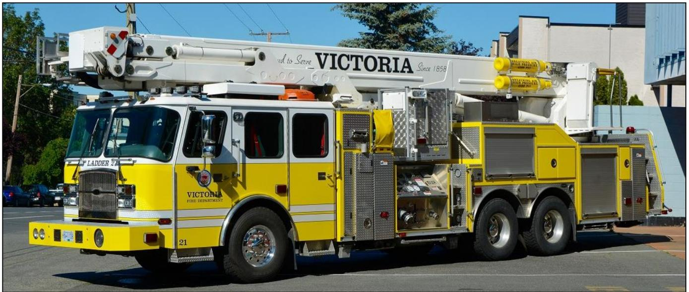
Victoria B.C. Ladder 2, sporting a new paint scheme, is a 2006 E One Cyclone II truck with a 1665igpm pump, 250gwt and a 100' Bronto tower, formerly with Brookline, Mass. (Terry Yip photo)
