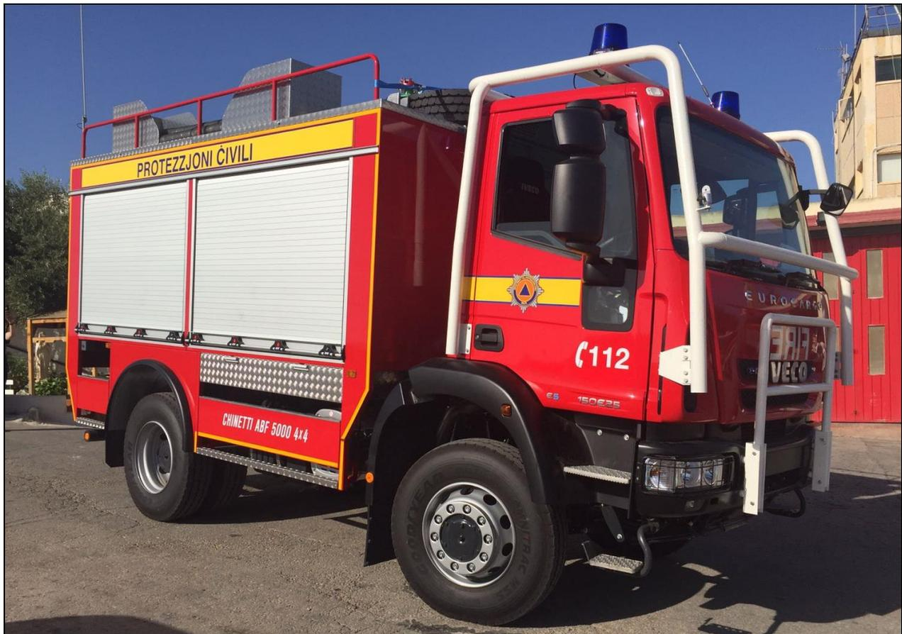
Some new appliances for Malta: a 2017 Chinetti water carrier on an Iveco 4 x 4 chassis. It carries 5000 L water with a 2000 l/min Chinetti pump.
