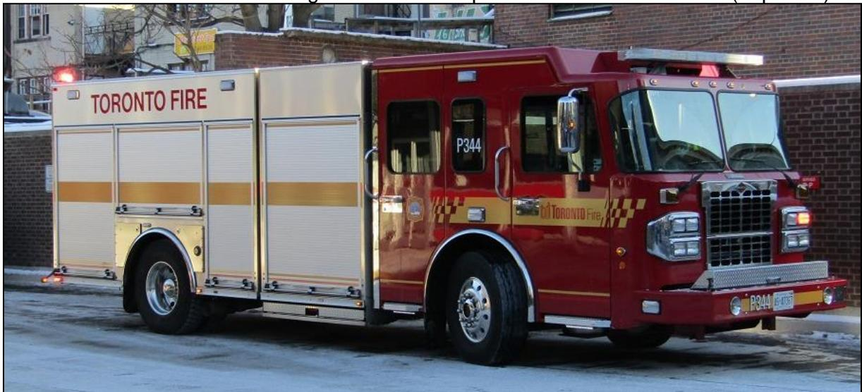
Toronto Pump 344, a 2017 Spartan Metro Star/Spartan ERV/DEV 2250gpm/600gwt/30gft(A)
