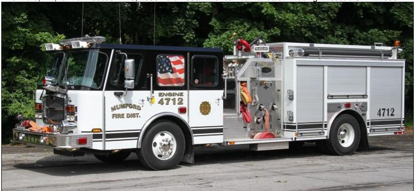
Mumford, NY Engine 4712, a 2011 E-One Typhoon with a 1500gpm pump and a 1000gwt. SN 136439.
