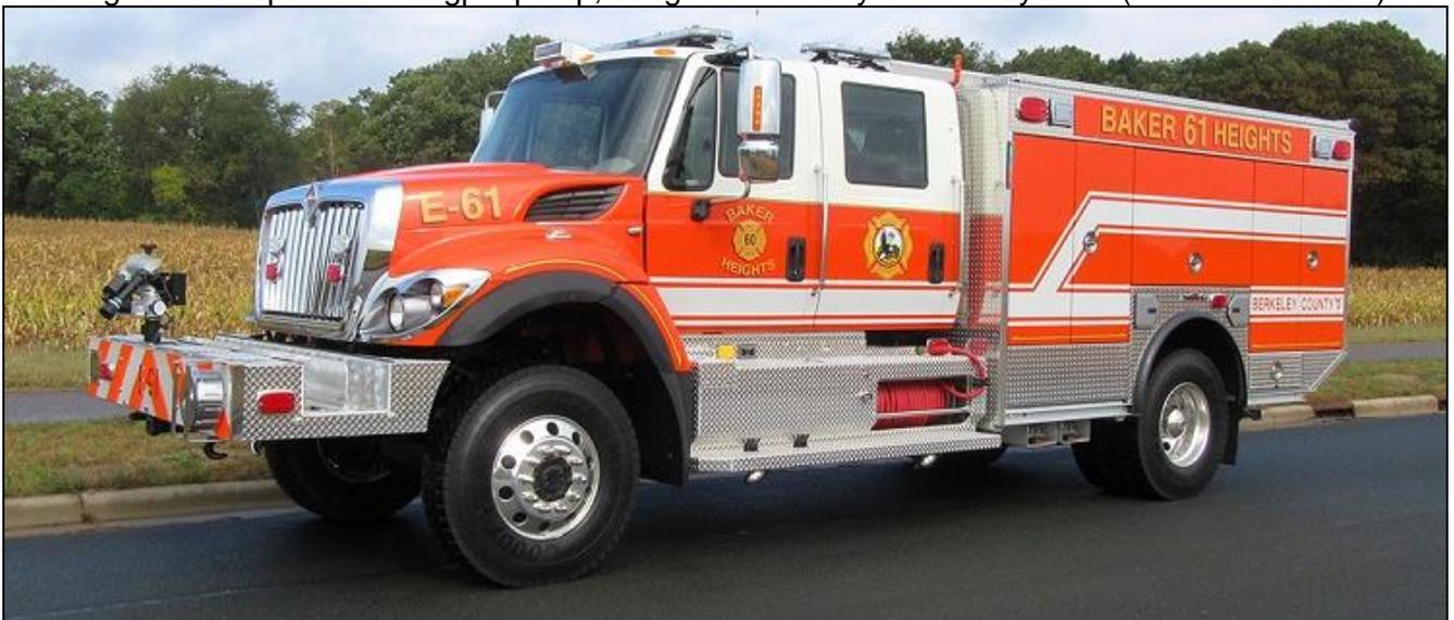
Baker Heights, Ohio Engine is a 61 2017 IHC 4x4/Rosenbauer Timberwolf built with a Rosenbauer NH45 pump, 750gwt and 30gft. (Rosenbauer U.S. Photo)
