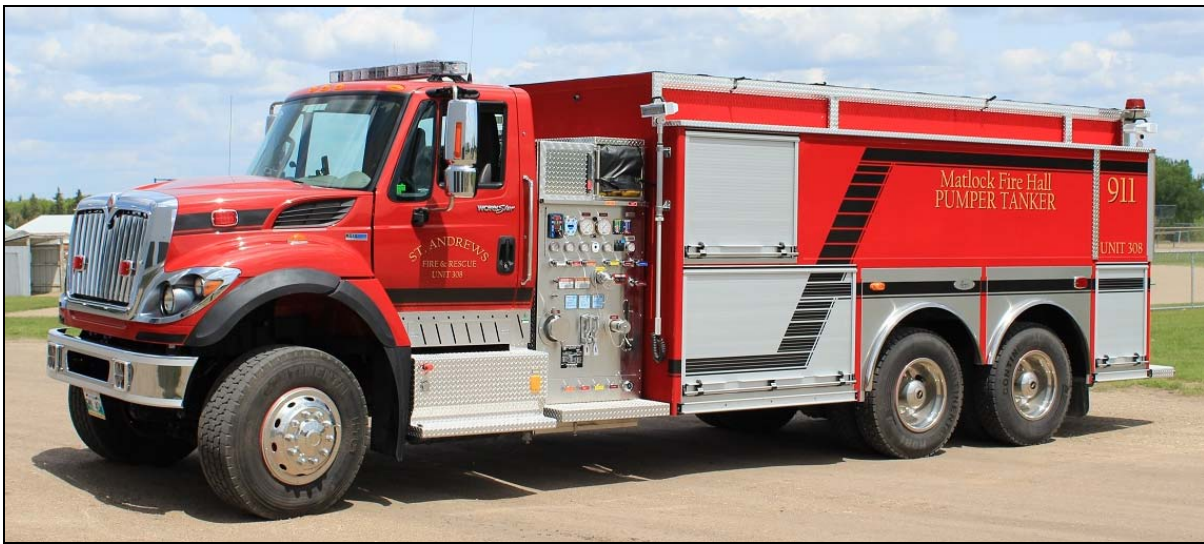
This 2013 IHC 7600/Acres rig runs from the Matlock Station in the Regional Municipality of St. Andrews, MB. It has a 625igpm pump, 2500gwt and 25gft. SN 130222102.
