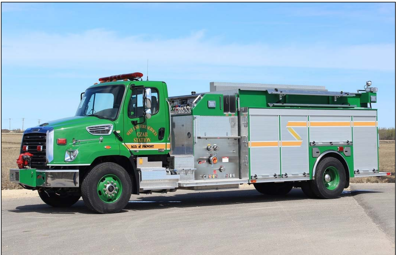
Resplendent in green, this 2013 Freightliner FL114SD/Fort Garry pumper has a 1250igpm pump, 1500gwt and twin 25g A&B foam tanks. It is operated by West End Fire Services, part of the Municipal District of Prevost, AB, from their Czar fire station. Serial Number M434.
