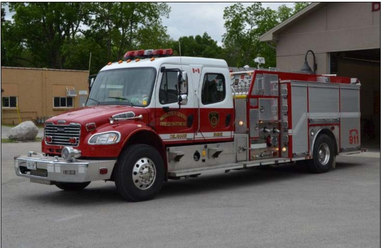
Strathroy-Caradoc Tanker 24, stationed in Mt. Brydges. It's a 2010 Spartan Metro Star /Rosenbauer pumper-tanker with a 1050igpm pump, 2000gwt and 50gft. (Bob Rupert photos).
