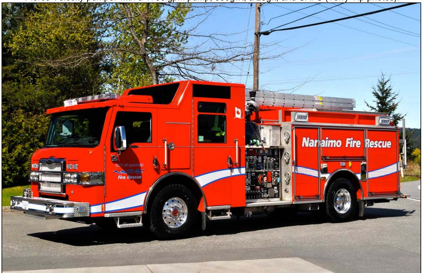
A couple from out west, this is Central Saanich's 2011 Spartan Gladiator/Smeal pumper with a 1522igpm pump, 600gwt and 60gft running as Engine 2. Also Engine 2, this Nanaimo rig is a 2012 Pierce Velocity pumper with a 1750igpm pump, 390gwt, a 25gft, and CAFS (Terry Yip photos).
