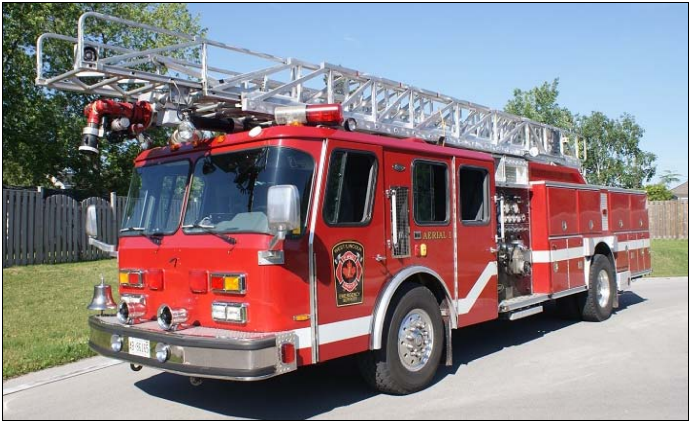
Now in service with West Lincoln as Aerial 1, is ex-Brampton A207, a 1992 E-One Cyclone II 75' quint with a 1250igpm pump and 400gwt. It is assigned to Smithville. Below: Guelph's newest rig, Pump 2 is a 2012 Rosenbauer Commander with a 1050igpm pump, 500gwt and 30gft. (Ken Buchanan photos)
