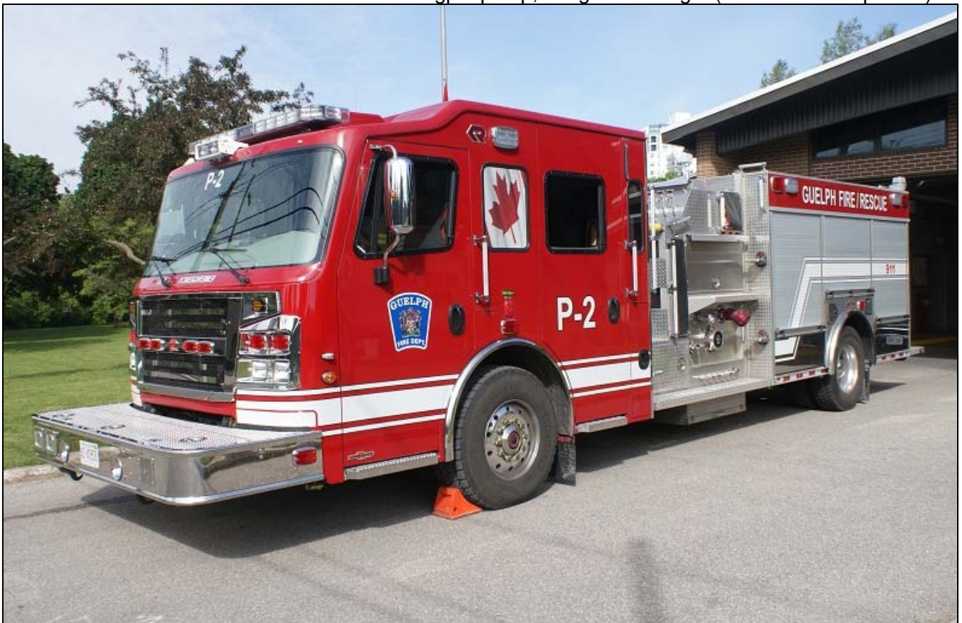
Now in service with West Lincoln as Aerial 1, is ex-Brampton A207, a 1992 E-One Cyclone II 75' quint with a 1250igpm pump and 400gwt. It is assigned to Smithville. Below: Guelph's newest rig, Pump 2 is a 2012 Rosenbauer Commander with a 1050igpm pump, 500gwt and 30gft. (Ken Buchanan photos)
