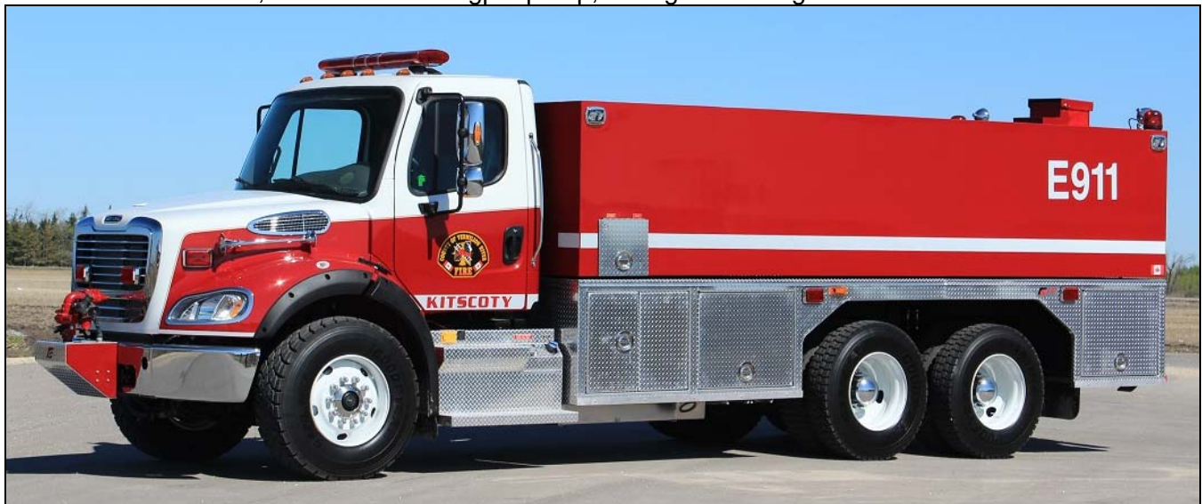
Above: Kitscoty, AB received one of three of these Fort Garry tankers bought by Vermilion County. They are all on 2013 Freightliner M2 chassis and have 420igpm pumps and 3000gwts. Below: Cold Lake, AB Ladder 2 is a 2013 Spartan Metro Star/Smeal 1750/250/20/75' quint. (D, Stewardson photos)
