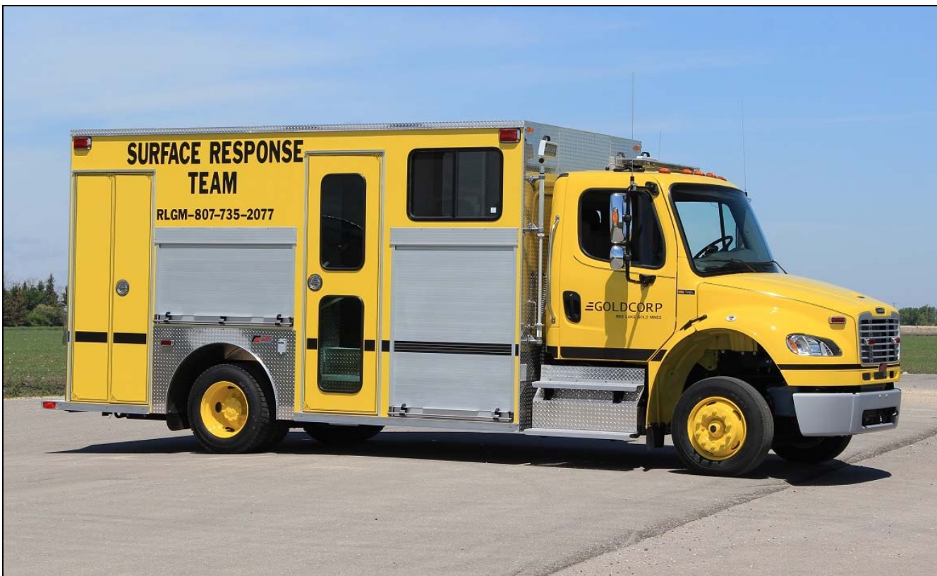
Another usually coloured rig, this belongs to GoldCorp and is used by their Surface Response Team. Also built by Fort Garry, this one is on a 2013 Freightliner M2 chassis. (Dave Stewardson photos)
