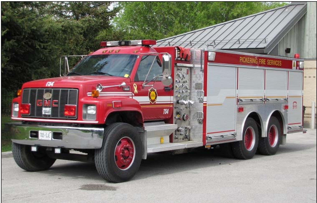
Tanker 54 is a 2000 GMC C8500/Dependable with a 420igpm pump and 2000gwt. It carries serial number TP314-500-2200-00 and is stationed in Claremont. (Desmond Brett photos).
