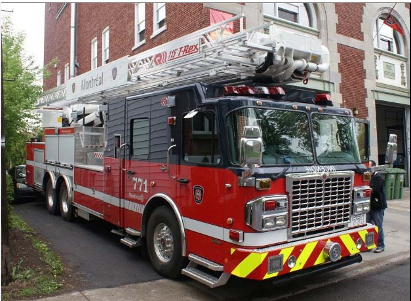
Above: one of Montreal's Rosenbauer T-Rex platforms. The four are all on 2012 Spartan Metro Star chassis, with 115' towers. Below, one of the latest deliveries of a 35 unit order of pumpers from Maxi Metal. Also on Spartan Metro Star chassis, they have 1500gpm pumps and 500gwts. (Bertrand Campo photos)
