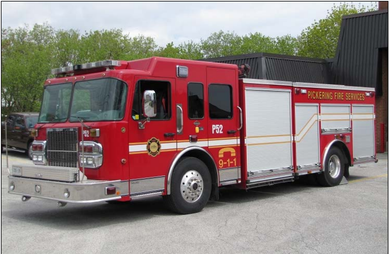
Two apparatus from the Pickering portion of the May tour: Pumper 52 is a 2005 Spartan Diamond/Smeal product with a 1050igpm pump, 500gwt and 30gft. Serial number 504111.
