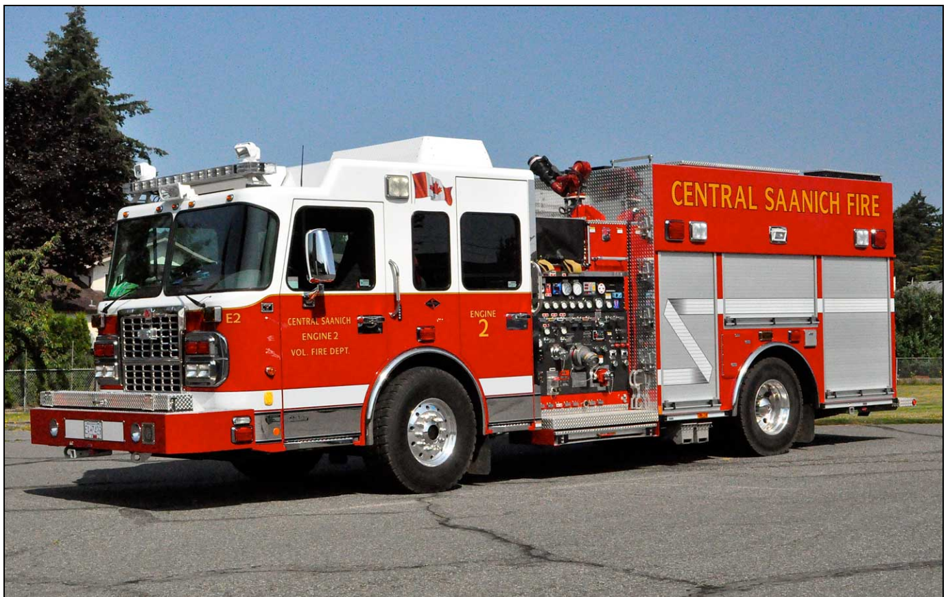
A couple from out west, this is Central Saanich's 2011 Spartan Gladiator/Smeal pumper with a 1522igpm pump, 600gwt and 60gft running as Engine 2. Also Engine 2, this Nanaimo rig is a 2012 Pierce Velocity pumper with a 1750igpm pump, 390gwt, a 25gft, and CAFS (Terry Yip photos).
