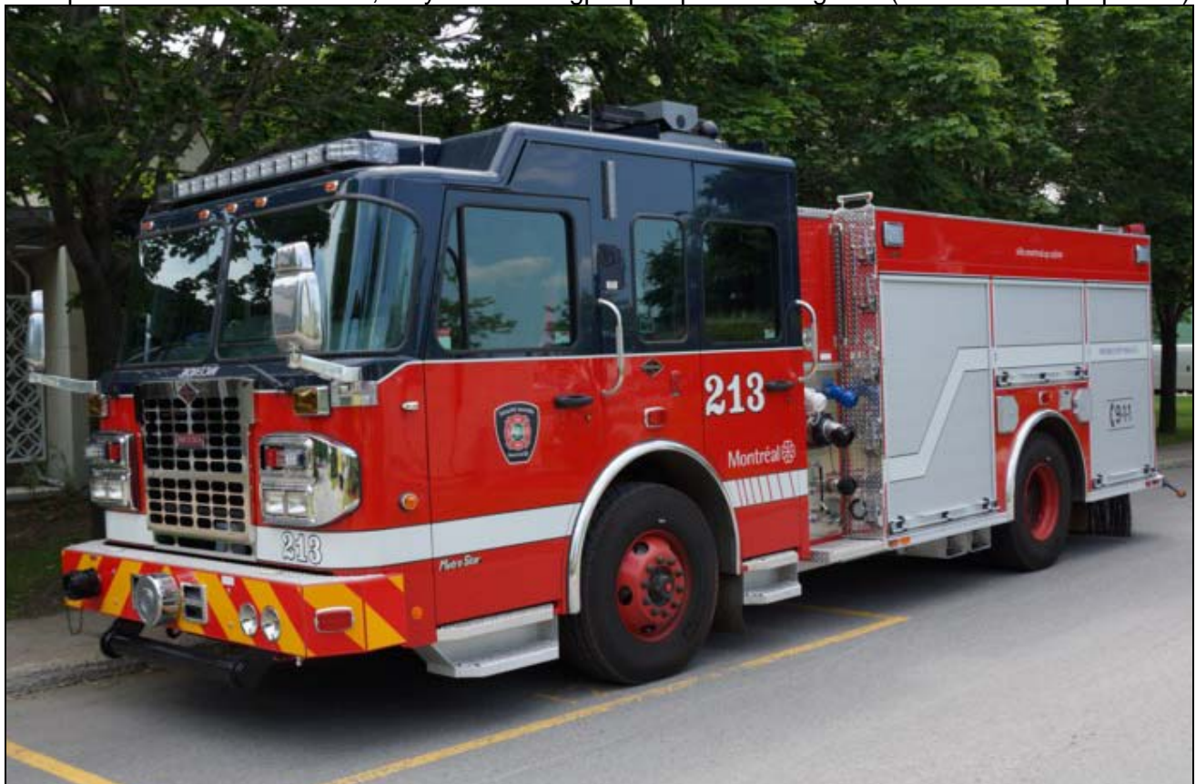
Above: one of Montreal's Rosenbauer T-Rex platforms. The four are all on 2012 Spartan Metro Star chassis, with 115' towers. Below, one of the latest deliveries of a 35 unit order of pumpers from Maxi Metal. Also on Spartan Metro Star chassis, they have 1500gpm pumps and 500gwts. (Bertrand Campo photos)
