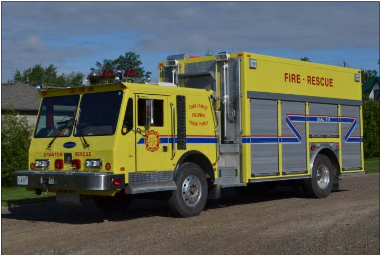
Two more from the June tour: Granton's Rescue without the buffs. This is a 1987 Amertek chassis with a body added by Superior in 1993. The truck originally belonged to Sarnia.
