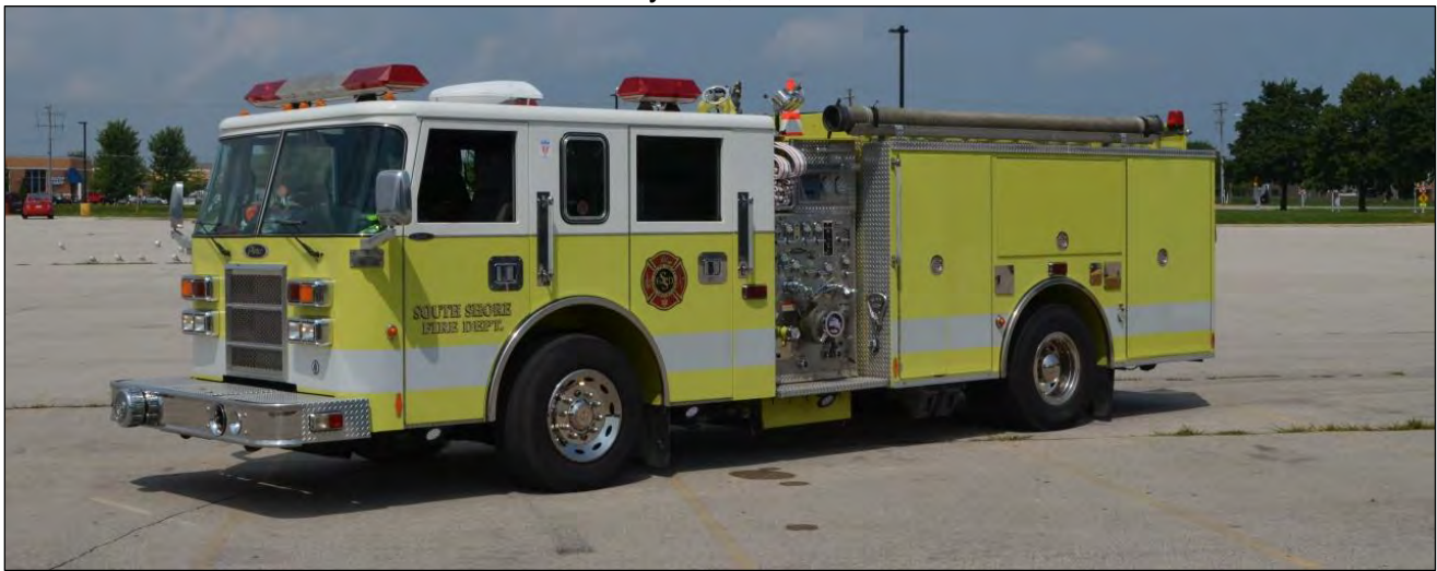
South Shore, WI Engine 8, 2000 Pierce Dash with a 1500gpm pump and 750gwt. J#11212
