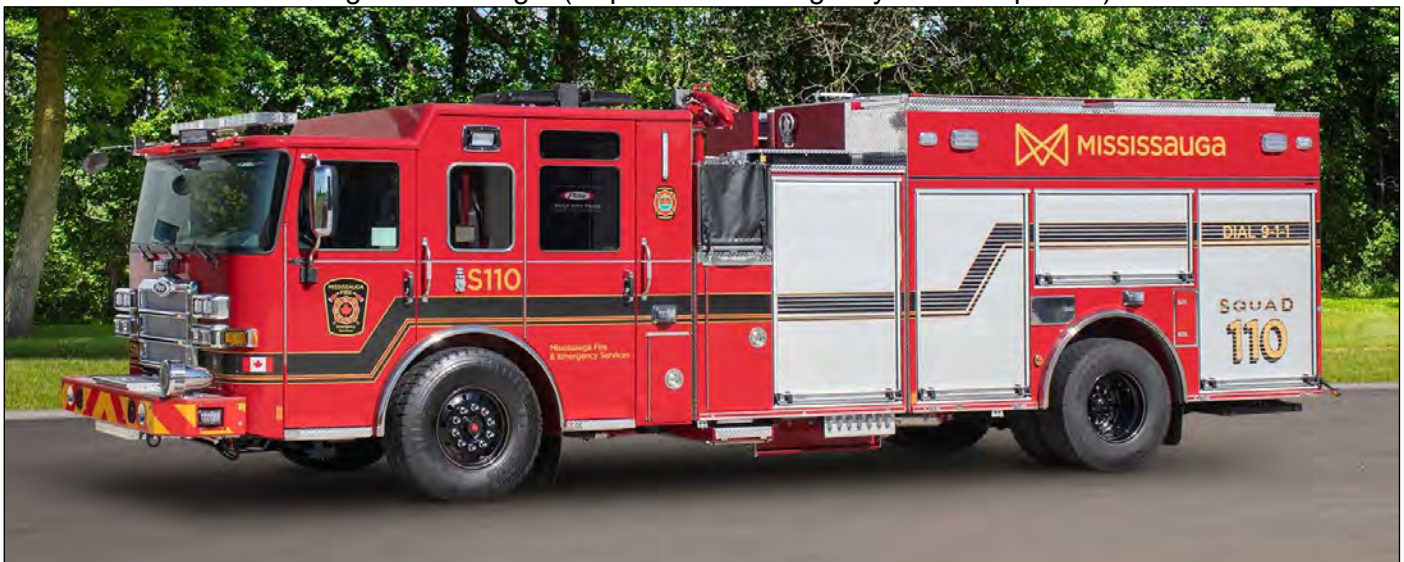
Mississauga, ON new Squad 110, a 2020 Pierce Enforcer with a 1750igpm pump, 500gwt and 50gft. (Pierce photo)
