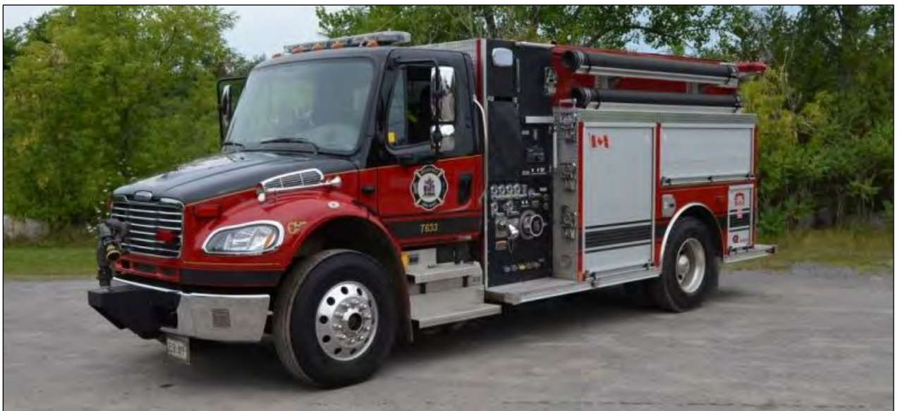
Belleville Tanker 633, a 2010 Freightliner M2 / Rosenbauer rig, with 1050igpm pump, 1250gwt and 50gft.
