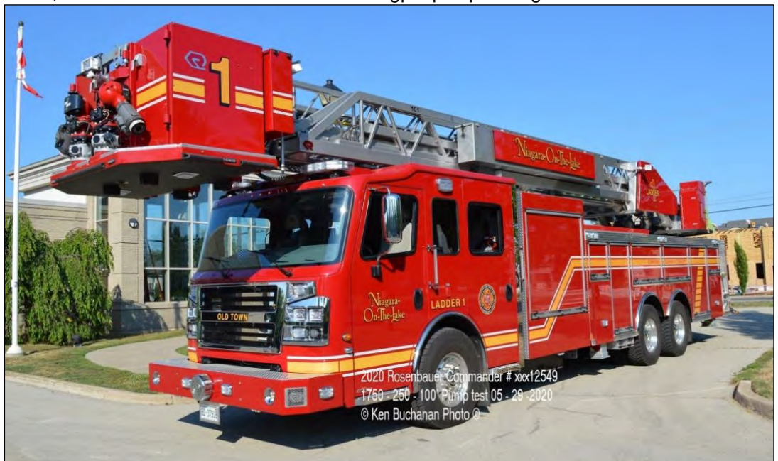
NOTL, ON Ladder 1, a 2020 Rosenbauer Commander quint with a 1750igpm pump, 250gwt and 100' tower. SN 12549 (Ken Buchanan photo)
