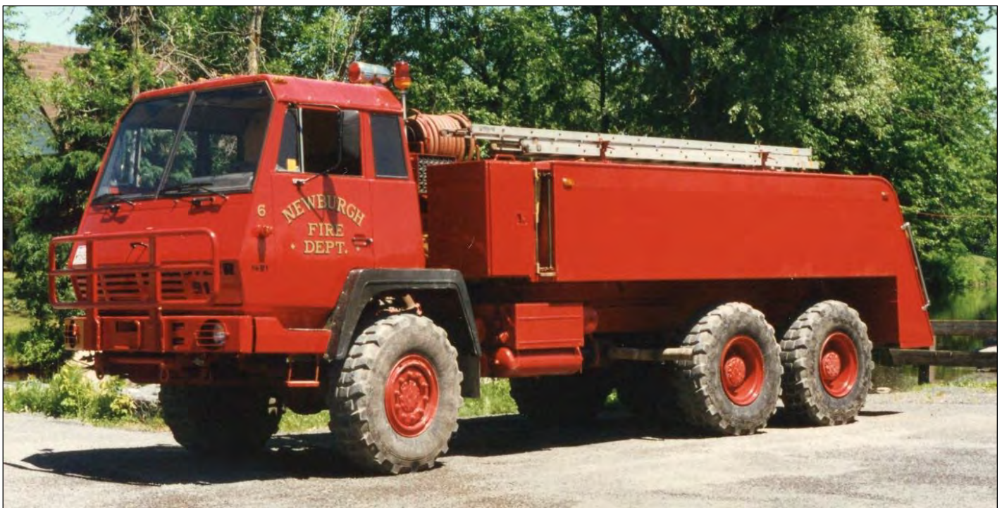
Newburgh's 1988 Steyr tanker after being refitted with a 300gpm pump and 2000gwt (Dean Nickerson photo)
