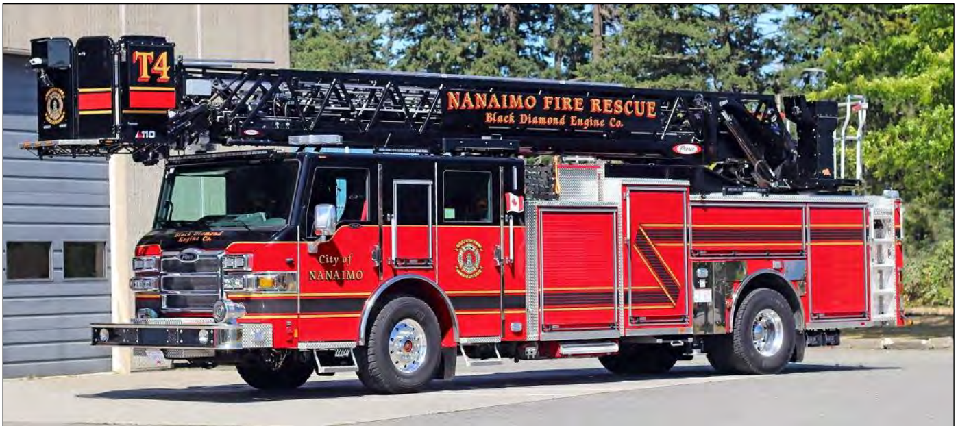
Nanaimo, Black Diamond Engine Co 2020 Pierce Velocity 1665igpm/400gwt/20gft/110' Ascendant platform 34147(Shane MacKichan photo)
