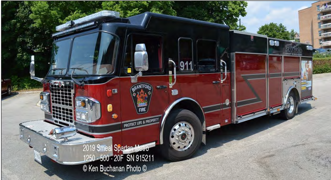
Brantford Pump 911 2019 Spartan Metro Star/ Smeal 1250igpm(W)/500gwt/20gft s/n S4969
