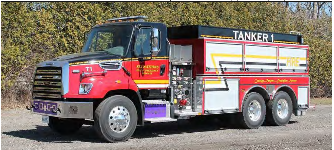
Old Tanker 1, now running from Station 4, is a 2017 Freightliner 114SD / Pierce product with an 840igpm pump, and a 2400gwt. (SN 31070) (Gary Dinkel photo)
