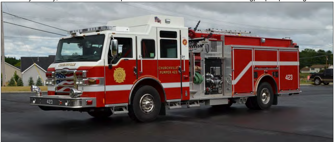
Churchville, NY Pumper 423, a 2010 Pierce Impel, 1250gpm pump, 1000gwt and 40gft. J#22934 (Bob Rupert photos)
