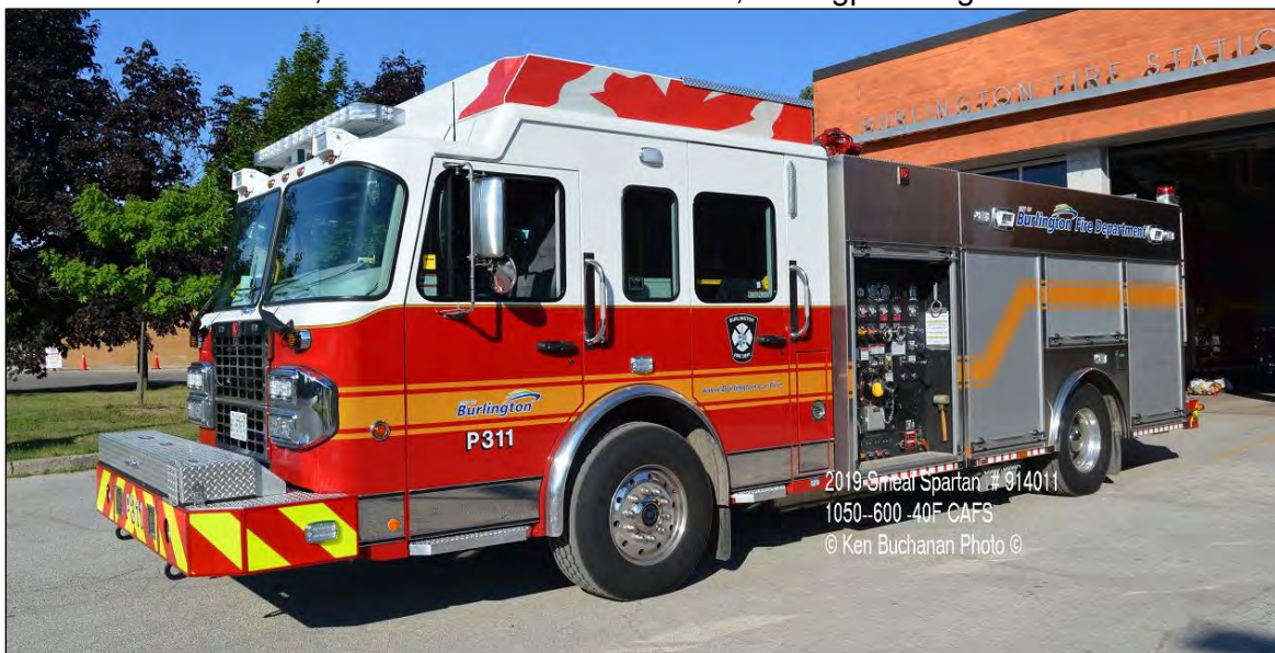
Burlington, ON Pumper 311, a 2020 Spartan Metro Star/Smeal engine with a 1050igpm pump, 500gwt, 40gft and a CAFS. (Ken Buchanan photos)
