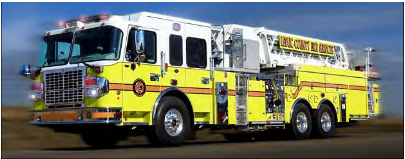
Leduc County, AB Tower 11, 2020 Spartan Gladiator Classic/Smeal 1500igpm/250gwt/17gft/100' SN S5032 (Safetek)
