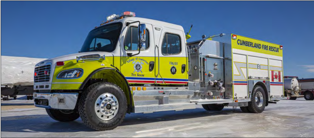
Cumberland, BC Engine 1, a 2019 Freightliner M2 106//Fort Garry 1500igpm/800gwt (Fort Garry Fire trucks)
