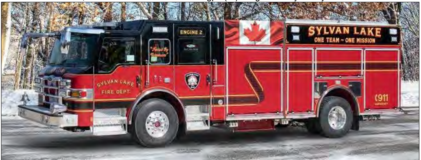
Sylvan Lake, AB Engine 2, 2020 Pierce Velocity 2000gpm(W)/750gwt Husky 12 FS j/n 33998 (Commercial Truck Equipment Co.)
