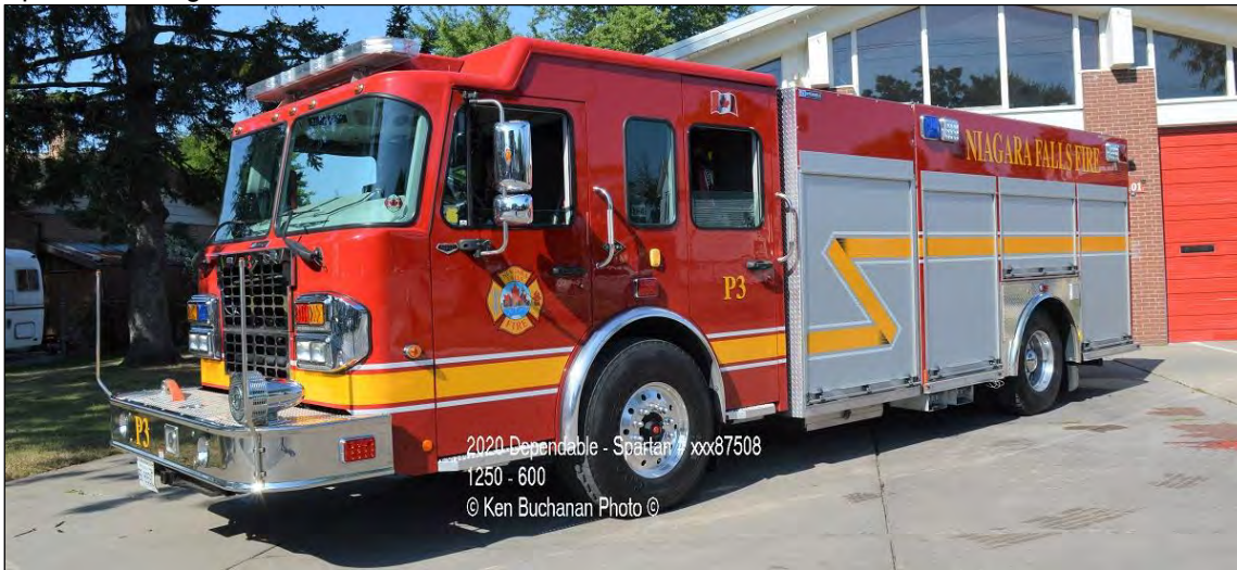
Niagara Falls, ON Pump 3, 2019 Spartan Gladiator/Dependable 1250igpm/500gwt
