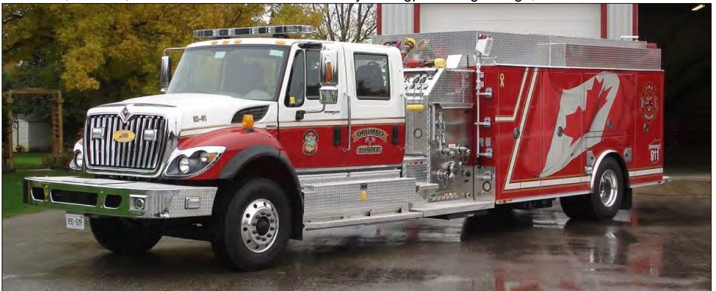
Blandford-Blenheim 82-01, a 2010 IHC/Asphodel pumper, which has a 1050igpm pump, 800gt and 30gft.
