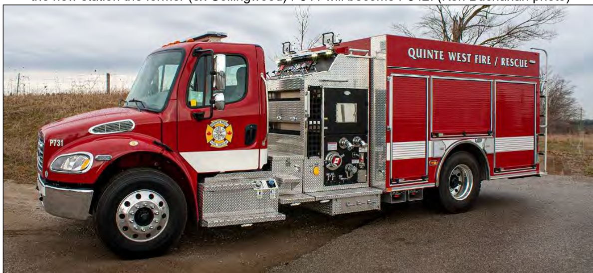
Quinte West, ON 731, a 2020 Freightliner M2-106/Pierce pumper with a 1250gpm Hale pump, 1000gwt and a Husky 3 foam system. SN 33288 (Commercial Truck Equipment Co., photo)
