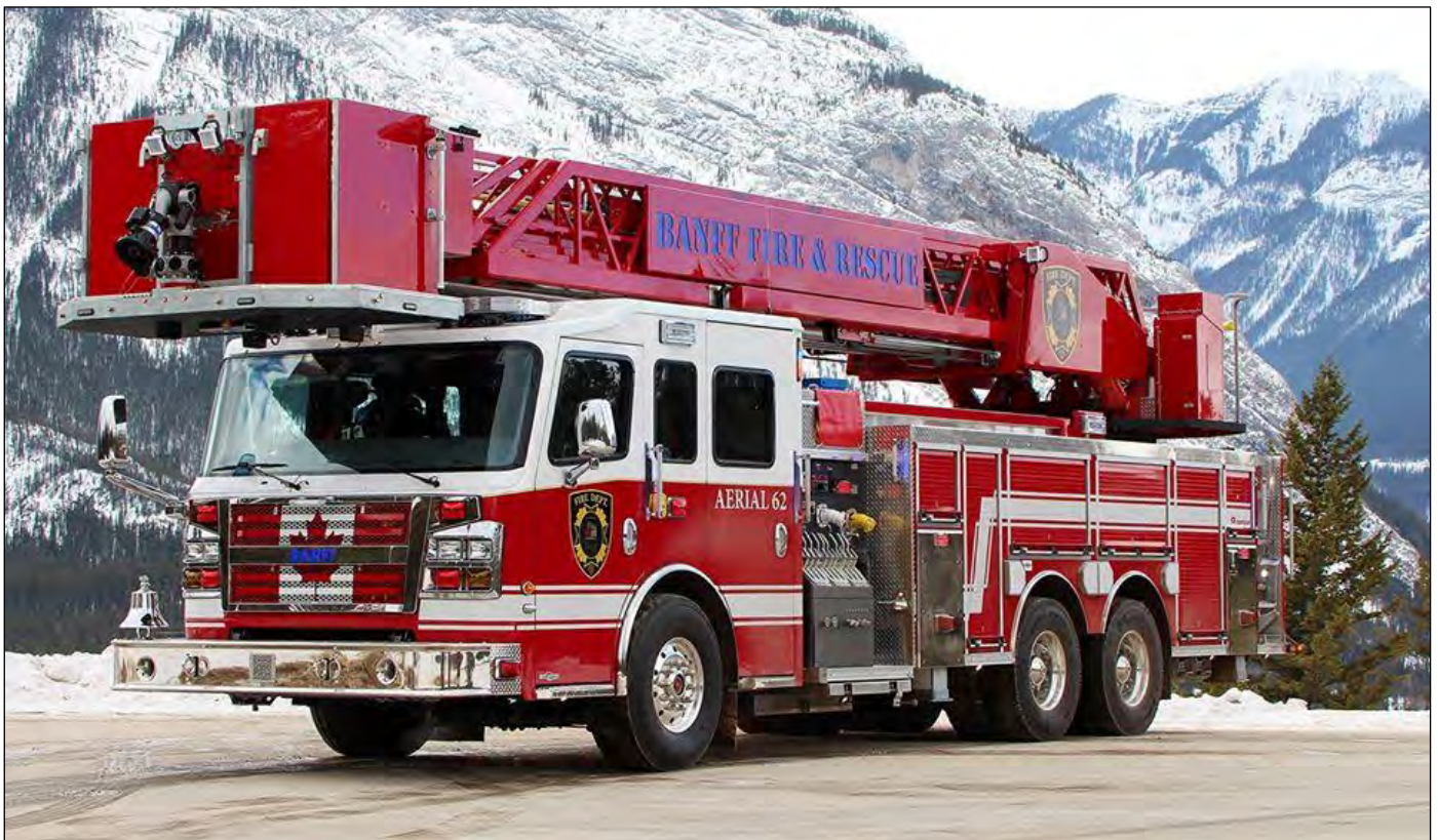
Banff, AB Aerial 62, a 2018 Rosenbauer Commander 3000 1500igpm pump, 430gwt and a 104' Cobra platform. (Rocky Mountain Phoenix photo)
