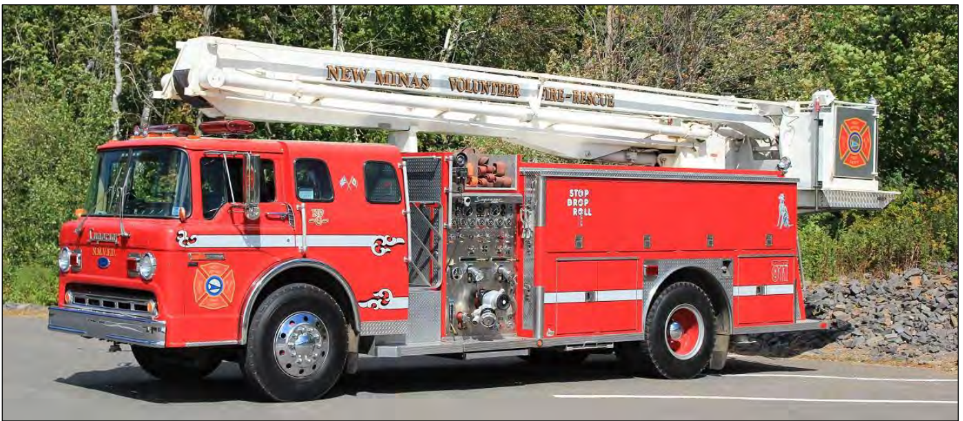
The repurposed snorkel remounted by Superior on a 1990 Ford C9000 chassis, still operated by New Minas, NS. (Dave Stewardson photo)
