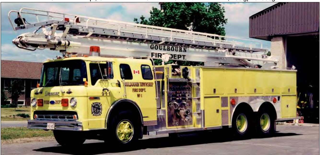
Goulbourn Aerial 1 a 1988 Ford C-8000/Superior pumper 1050igpm, 500gwt and 75' Telesqurt. (Ken Walton photos)
