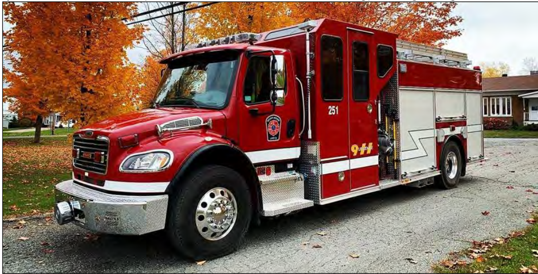
A delivery for Lambton, QC late last year, Unité 251 is a 2019 Freightliner M2/Maxi Métal, with a 1250gpm Hale pump, 1000gwt and a 25gft. (Maxi Métal Fire Trucks photo)
