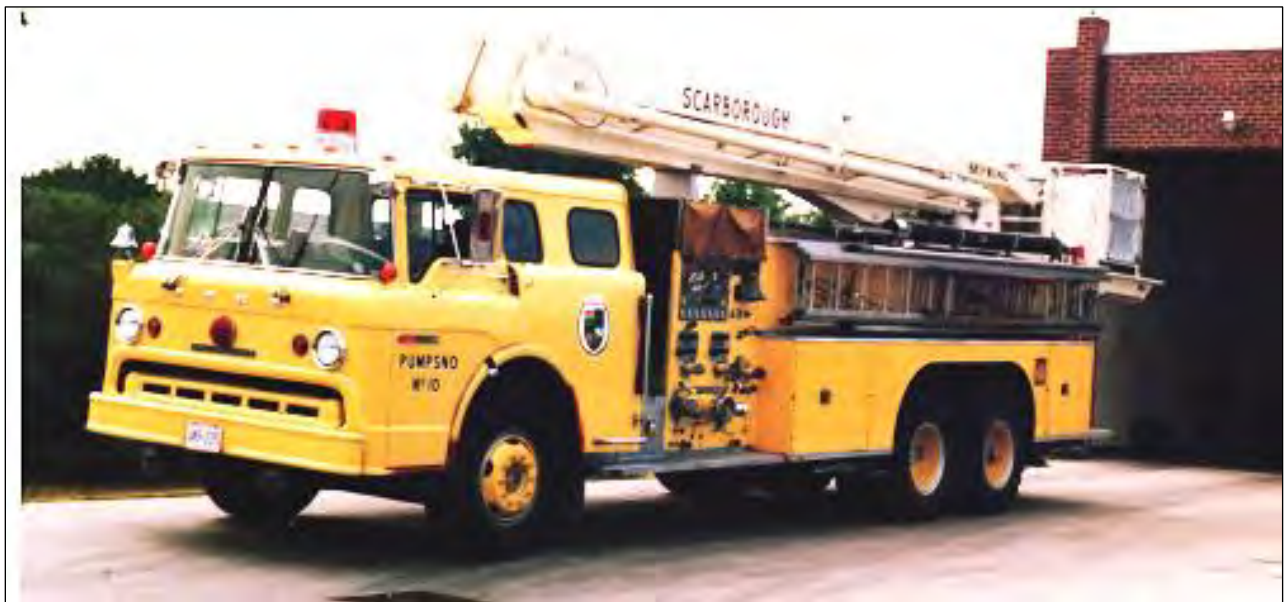
Scarborough Pumpsno 10, a 1972 Ford C/King with an 840igpm pump, 500gwt and 55' Sky King snorkel.
