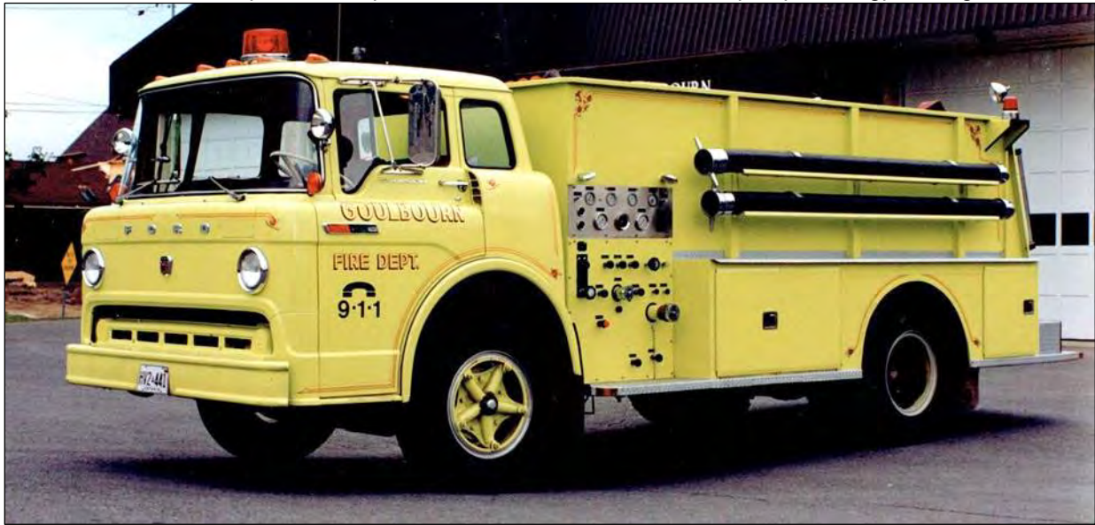
Goulbourn Twp., ON Tanker 1 a 1972 Ford C-800 / AFT tanker, 250igpm/1500gwt.
