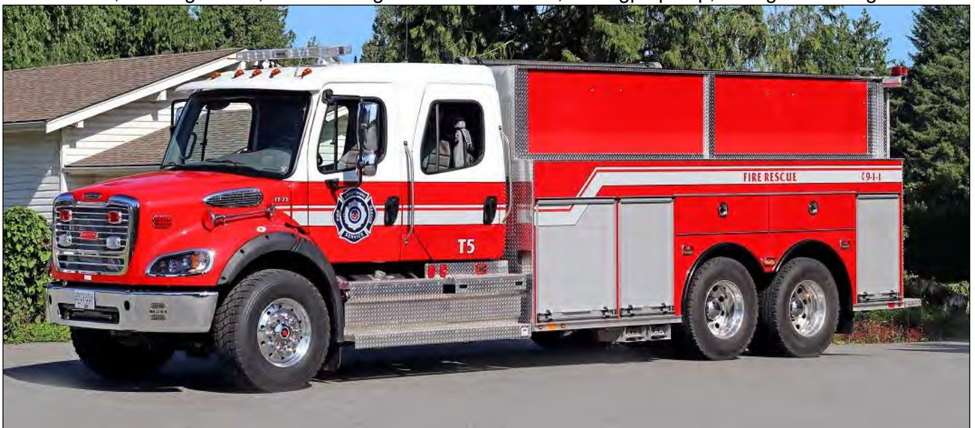
Abbotsford, BC Tender 5, a 2020 Freightliner M2-112/Maxi Métal 625igpm Hale pump, 2629gwt,
