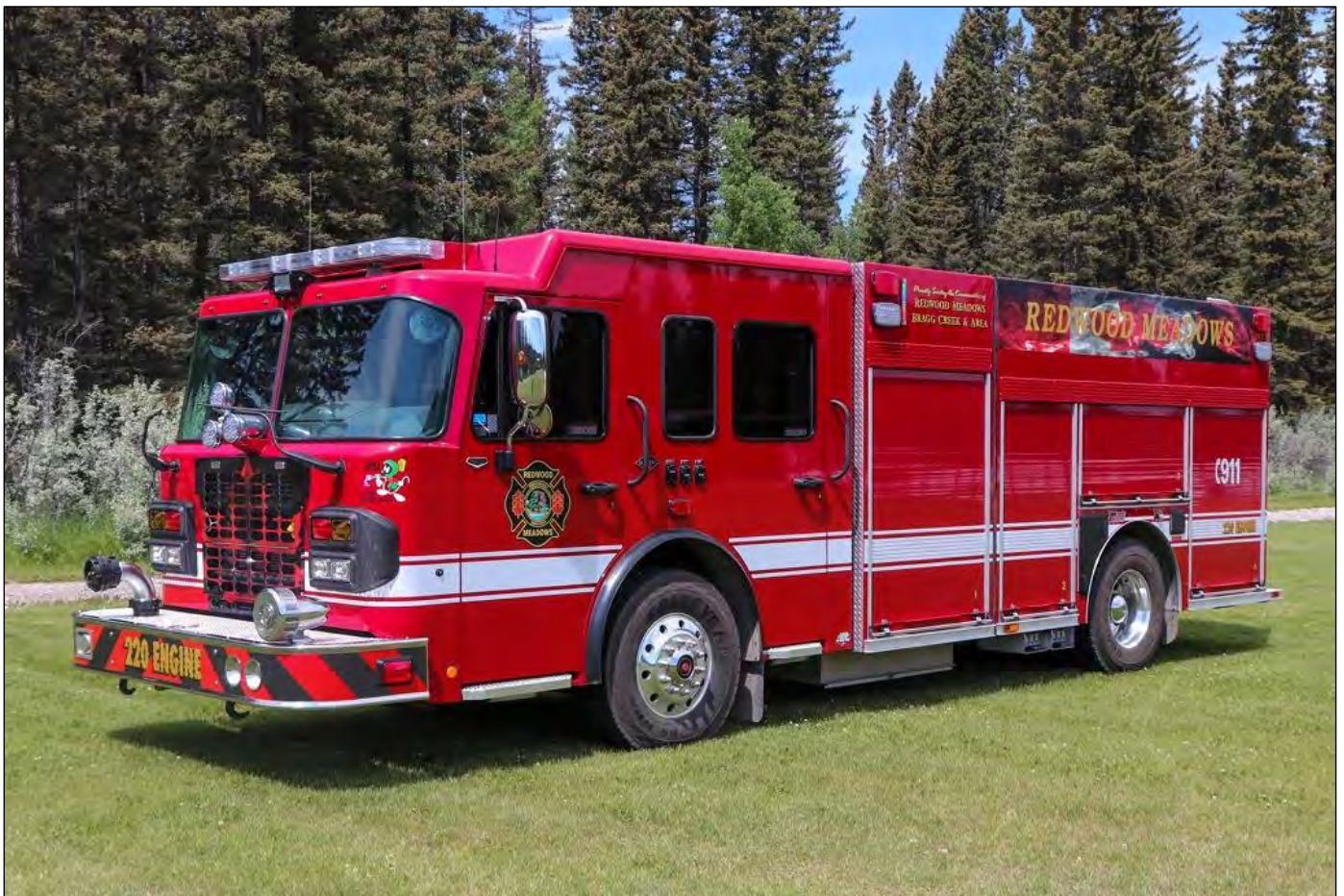
Redwood Meadows, AB Engine 220, a 2019 Spartan/Fort Garry pumper equipped with a 1333igpm pump, 800gwt and a 25gft. It also has a FoamPro foam system. JN J0022 (Redwood Meadows Fire Service photo)
