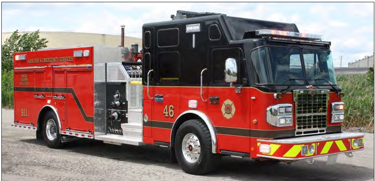
Ajax, ON Pump 46, a 2020 Spartan Metro Star/Dependable pumper with a 2000gpm Hale pump, 600gwt and 30gft, with a FoamPro 2002 foam system. It is assigned to Station 1.
