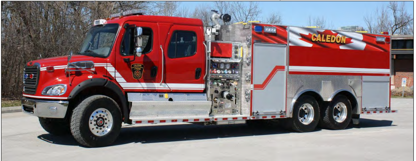
Caledon, ON Tanker 302, a 2020 Freightliner M2-112/Dependable product with a 1750 USgpm Hale pump, 2700gwt and a 20gft. (Dependable Emergency Vehicles photos)
