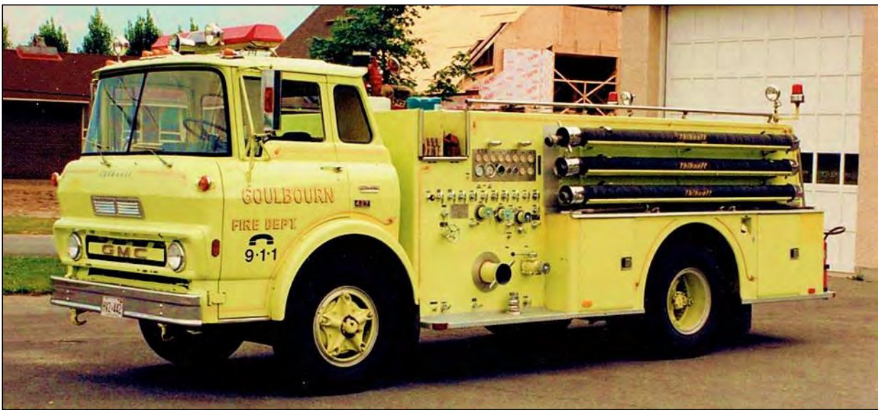
Goulbourn Twp., ON Pumper 1, 1977 GMC T6500 / Thibault pumper 840igpm/500gwt
