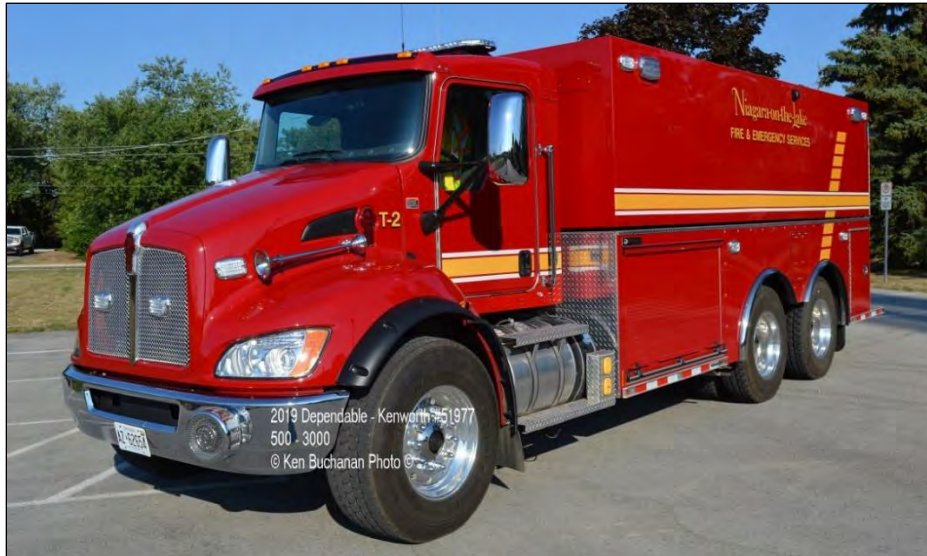
NOTL, ON T.2 2019 Kenworth T370/DEV 500igpm pump/3000igwt
