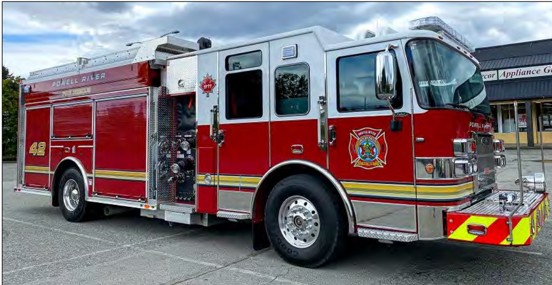
Powell River, BC E.42 Powell River Engine 42, a 2020 Pierce MaxiSaber VIO 2000gpm(W)/500gwt (CTE)
