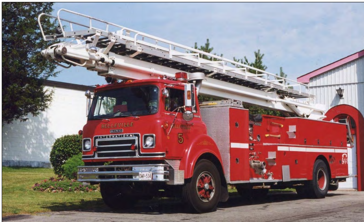
1978 International CO1950B / King pumper (840/500/75' TeleSquirt) (SN#77057)
