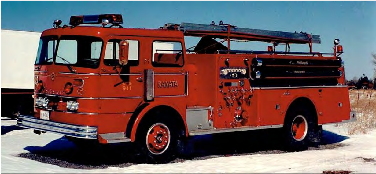
Kanata had this 1967 Thibault AWIT584 pumper with a 840igpm pump and 800gwt.
