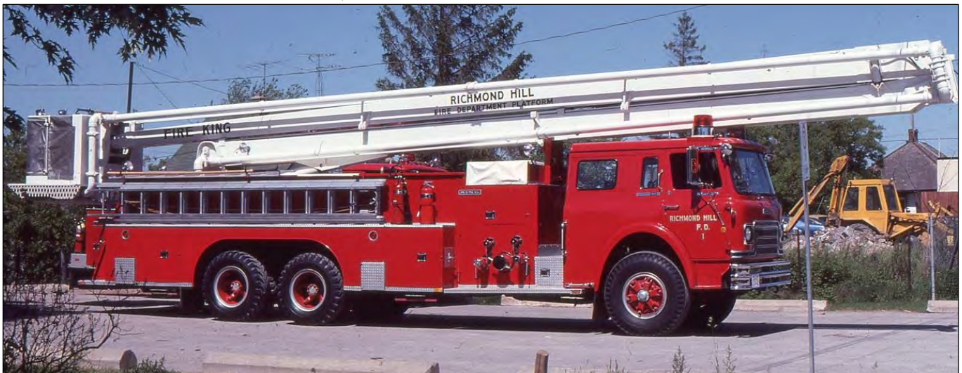
Platform 3 was a 1974 International King 85' Snorkel; with a 1050igpm pump, 200gwt. (Desmond Brett photos)
