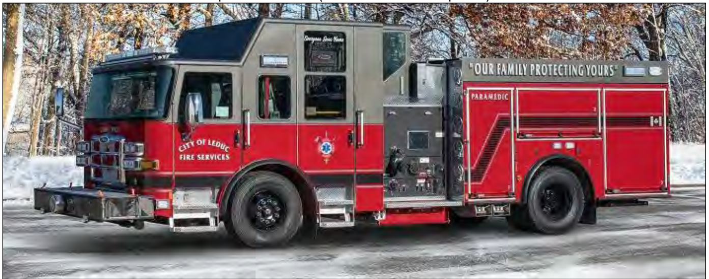
Leduc, AB 2020 Pierce Enforcer 1750gpm(W)/500gwt Husky 3 FS j/n 33928.
