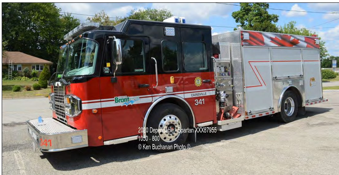
Brant County, ON P.341, 2020 Spartan Metro Star/Dependable 1500gpm/1000gwt/30gft s/n 52981 On completion of the new station the former (ex Collingwood) P341 will become P342. (Ken Buchanan photo)
