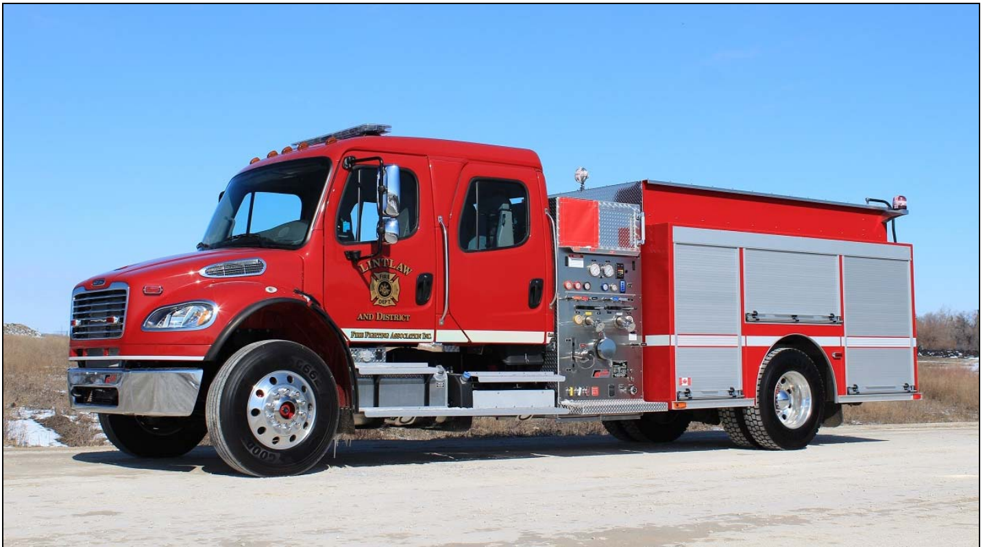
Lintlaw, SK purchased this stock unit from 2013 Fort Garry earlier this year on a Freightliner M2-106 chassis. It came with a 1050 igpm Hale pump, 800gwt. s/n M404.
