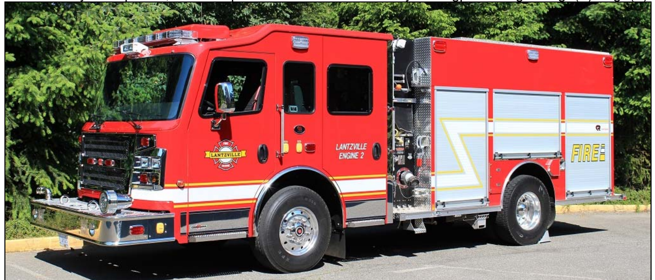
Lantzville, BC Engine 2 is a 2015 Rosenbauer pumper with 1250igpm pump, 900gwt and 25gft. (Dave Stewardson photos)
