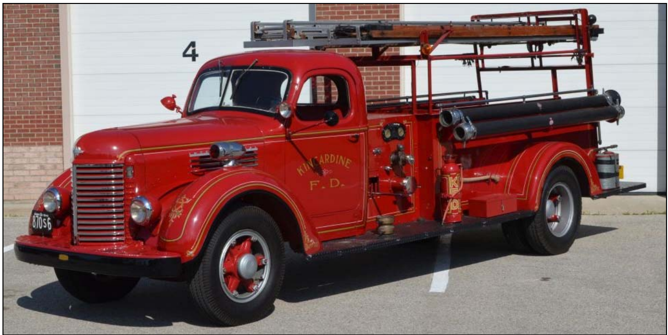
One feature of this tour was the abundance of immaculately restored apparatus. Above is Kincardine's 1946 International K chassis Bickle pumper, with a 425igpm pump and 150gwt. Below is Southampton's 1929 Chevrolet /Bickle pumper, it has a 250igpm pump and 60gwt. (Bob Rupert photos)
