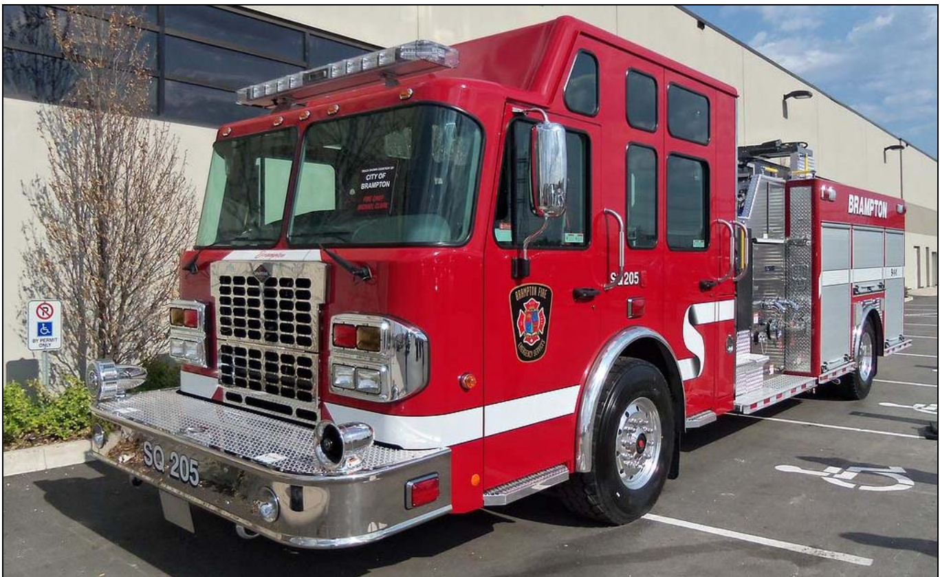
Visiting outside the venue was then new Brampton Squad 205, a 2015 Spartan Metro Star-X/DEV rescue-pump which as a 1250igpm pump, 500gwt and 25gft. (Rob Simpson photos)
