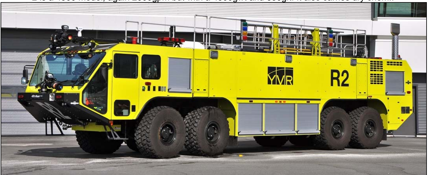
Red 4 is an Osh Kosh Striker 3000 with a 2000gpm pump, 3000gwt, 420gft and 500 lbs dry chemical. Red 2 is a 4500 model, again 2000gpm but with a 4500gwt and 630gft. It also carries dry chem..
