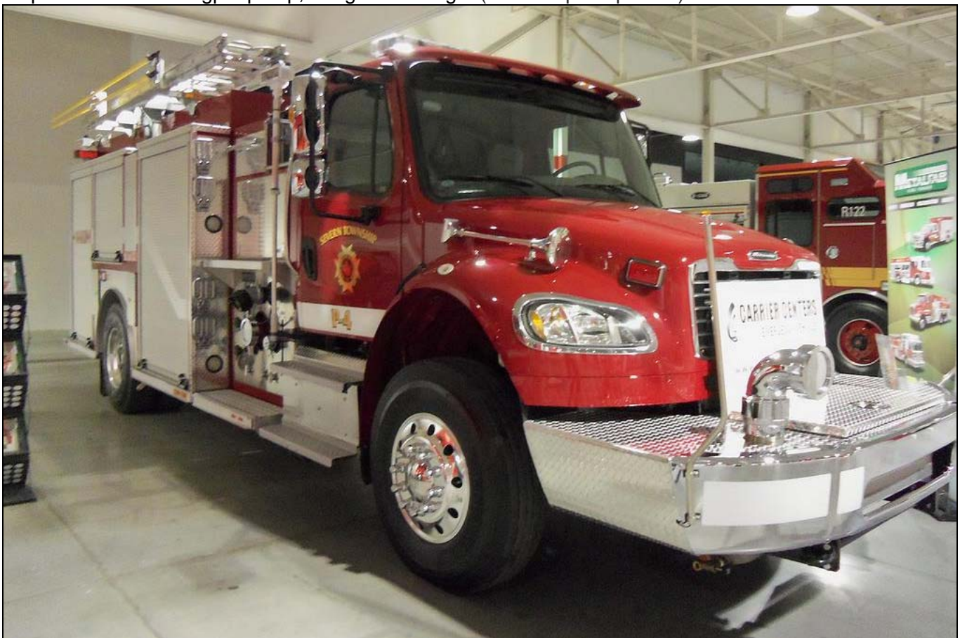
Severn Township's new Pumper 4 was also in attendance, it's a 2014 Freightliner M2-106/Metalfab rig with a 1050igpm Hale pump, 800gwt and 20gft, also has a FoamPro 2001 foam system
