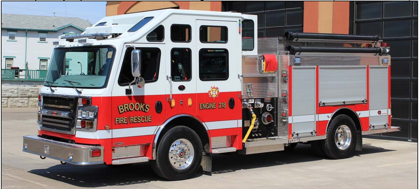
Brooks, AB recently acquired this 2015 Rosenbauer Commander engine, with a 1250igpm pump, 1030gwt and 30gft . A recent addition at CFB Borden is this 2015 IHC 7400 4x4/Fort Garry Fire brush rig with 132igpm/ pump, 1000gwt and 20gft. s/n M577. (Dave Stewardson photos)
