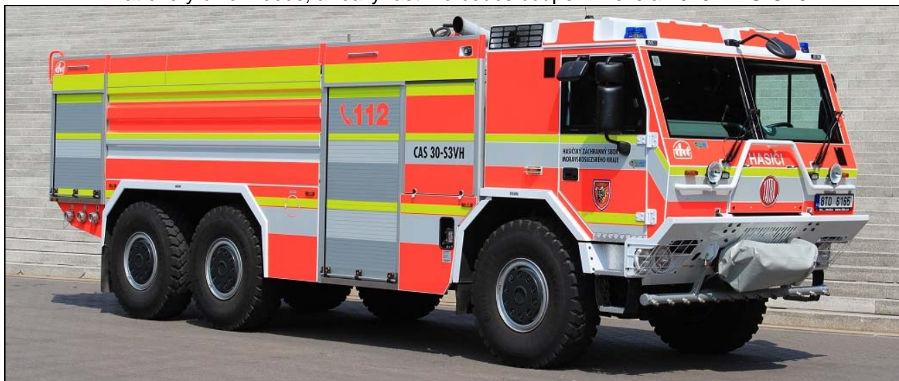
From the Czech Republic, a THT Policka 9,000L water tender on a Tatra T815 6x6 chassis. It also carries 500L foam and has a full size pump.
