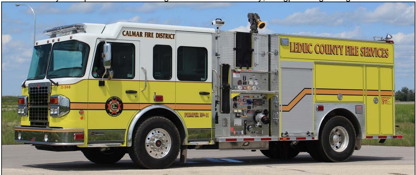
Leduc County Pumper 11, a 2015 Spartan Metro Star/Fort Garry 1050igpm/1000gwt/10gft(A)/25gft(B)
