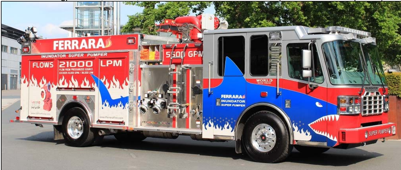
This impressive beast was on display at Intershutz. It's a 2015 Ferrara Inundator and, as indicated, flows 5500gpm or 21,000LPM, same as a decent sized fire boat. (Dave Stewardson photos)
