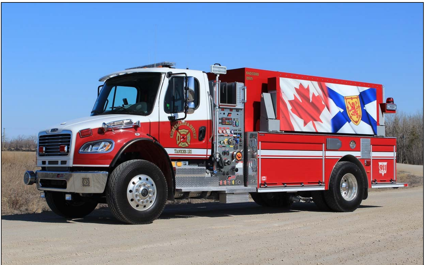
This 2015 Freightliner M2-106/Fort Garry pumper tanker went to Shubenacadie, NS. Tanker121 sports an 840igpm pump,1500gwt and a pair of 25gfts. s/n M555. (Dave Stewardson photos)
