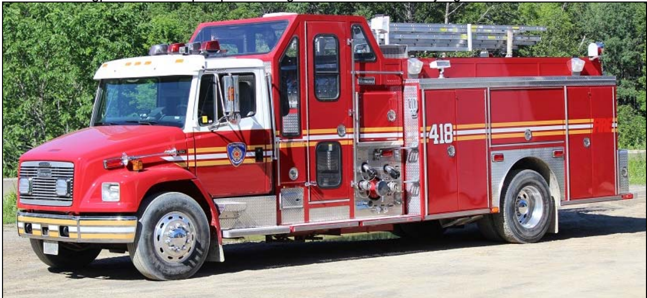
This is Wellesley Twp.'s old Pumper 1, now with Oromocto, NB. The 1998 Freightliner FL 80 /Metalfab pump, 1050igpm/800gwt, was traded in to Metalfab, who refurbished and repainted the formerly yellow truck and sold it on. (Metalfab Fire photo)
