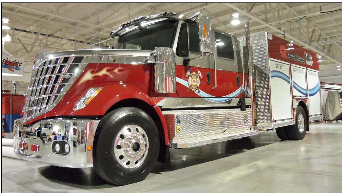
Another impressive demo, this was at the OAFCA show, this is a Rosenbauer MP3 pumper with an IHC chassis with a Lone Star hood. (Rob Simpson photo)
