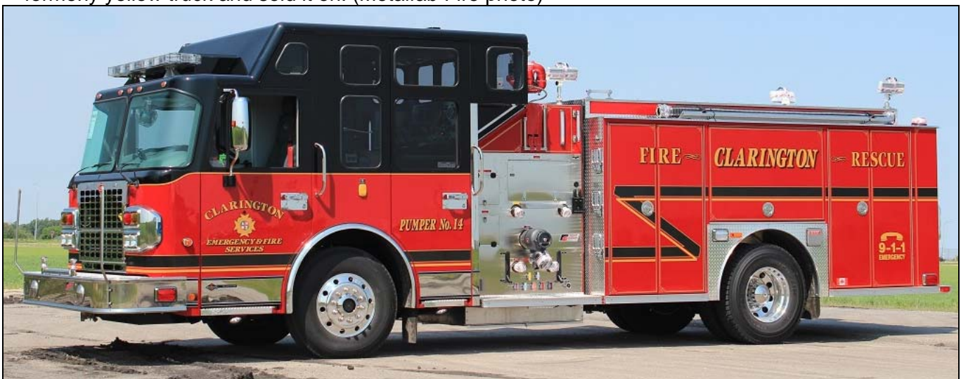
Clarington recently put this 2015 Spartan Metro Star/Fort Garry pumper in service as Pumper 14. It has a 1000igpm Hale pump, 500gwt, 25gft(A) and a FoamPro 1600 foam system, snM600. (Dave Stewardson)
