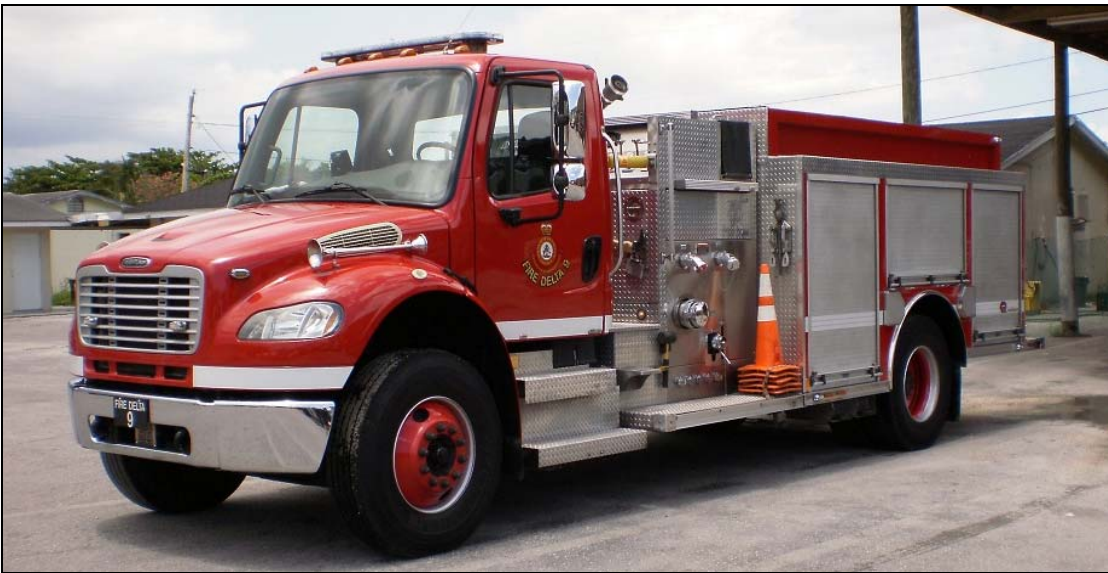
From the Bahamas, a pair of 2014 Freightliner/Rosenbauer pumpers, both with 1000gpm pumps and 1000gws. Delta 9 has a two-door cab, Delta 10 the four-door model. (Rick Loiselle photos)
