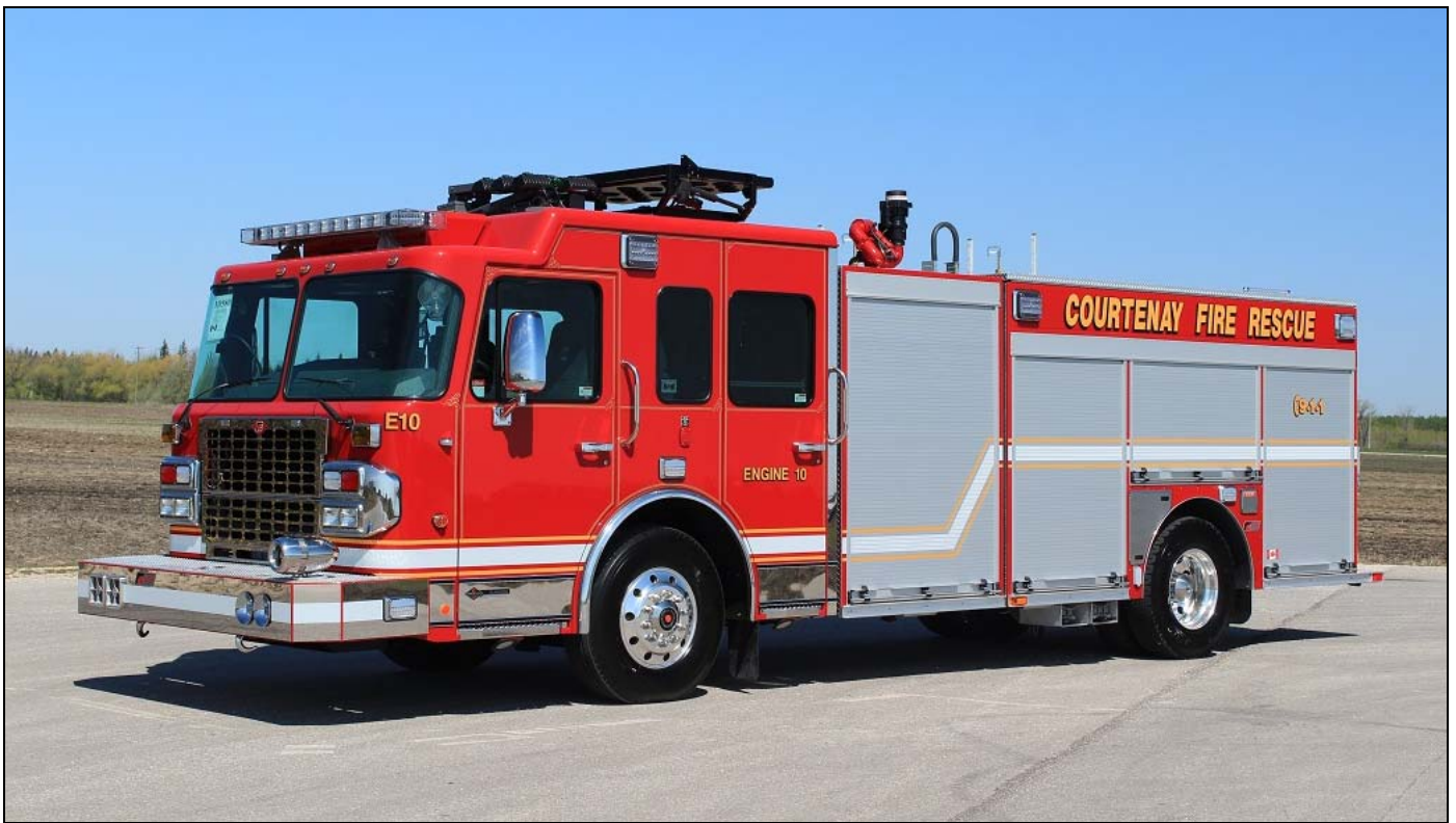
Courtenay,BC recently received this 2015 Spartan Metro Star/Fort Garry pumper. It has a 2000igpm Hale pump, 740gwt, 20gft(A) and a 30gft(B). It's assigned to Engine 10, s/n M580.
