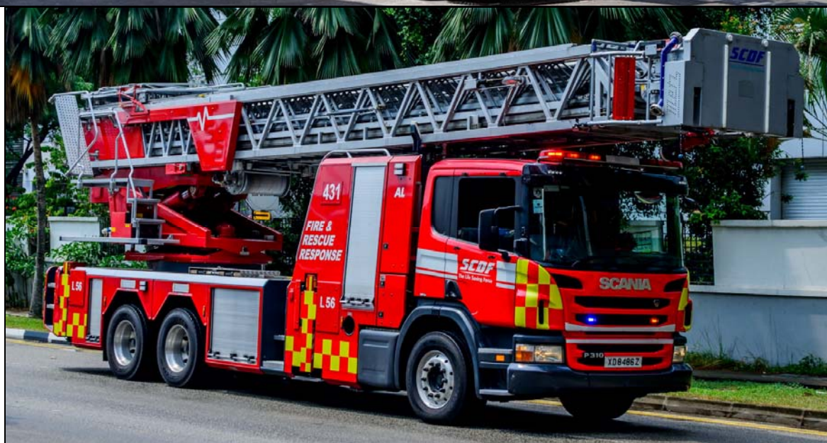
Singapore's SCDF 431, a Scania P310/Metz 56m (184') turntable ladder. (Kenneth Lai)
