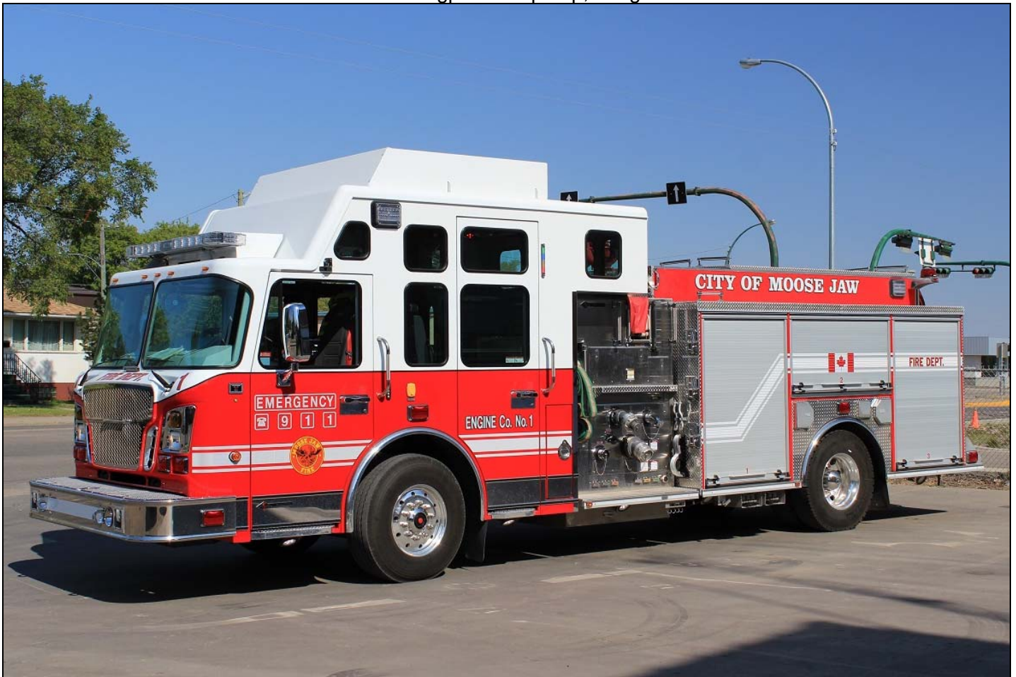
Moose Jaw, SK E.1 bought a 2014 Spartan Gladiator Evolution/Spartan ERV pumper this year, equipped with a 1500gpm Hale pump, 600gwt and 30gft. SN 213160-1 (Dave Stewardson photos)
