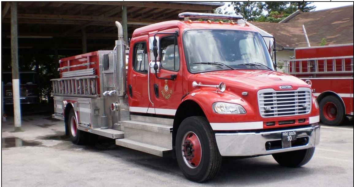
From the Bahamas, a pair of 2014 Freightliner/Rosenbauer pumpers, both with 1000gpm pumps and 1000gws. Delta 9 has a two-door cab, Delta 10 the four-door model. (Rick Loiselle photos)
