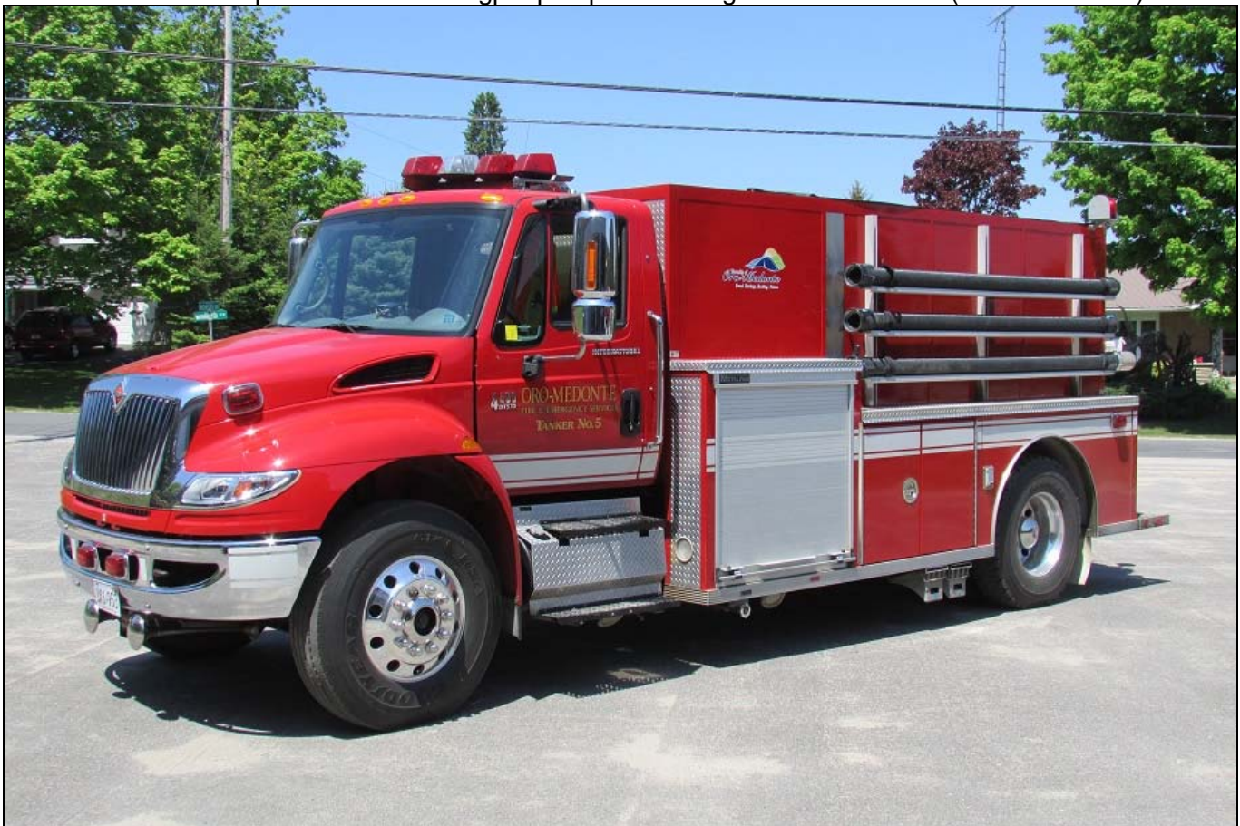
Two more from the May tour. Rama Rescue 51, a 2002 IHC 4300/Superior rig with a 625igpm pump, 300gwt and 30gft. It carries Superior number SE 2705. Oro Medonte Tanker 5 is a 2007 IHC 4400/Metalfab product with a 420igpm pump and 1600gwt. SN M07-8073 (Desmond Brett)
