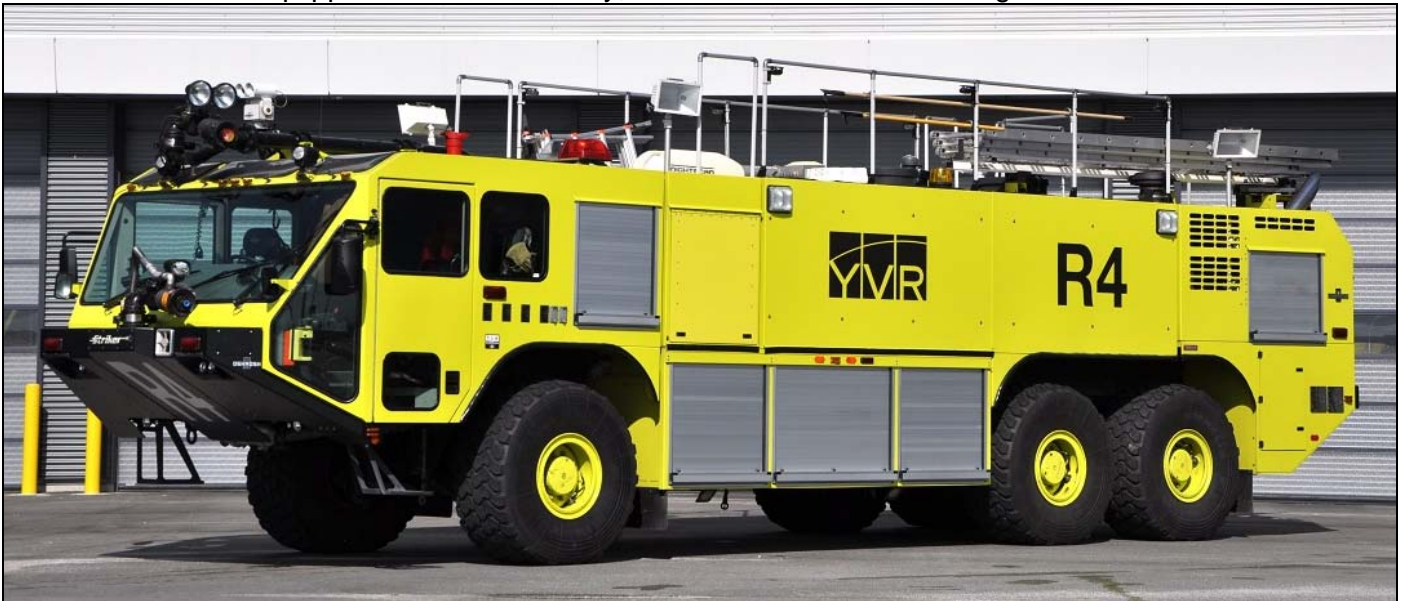
Red 4 is an Osh Kosh Striker 3000 with a 2000gpm pump, 3000gwt, 420gft and 500 lbs dry chemical. Red 2 is a 4500 model, again 2000gpm but with a 4500gwt and 630gft. It also carries dry chem..
