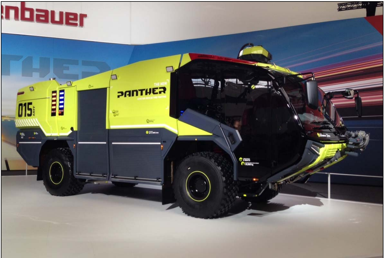
Rosenbauer unveiled the new Panther ARFF truck at Interschutz. The 4x4., above, and the 6x6, below, which has an 8000LPM pump, 12,500LWT, 1500LFT and carries 250kg of powder. This one is also equipped with a Stinger 54 HRET.
