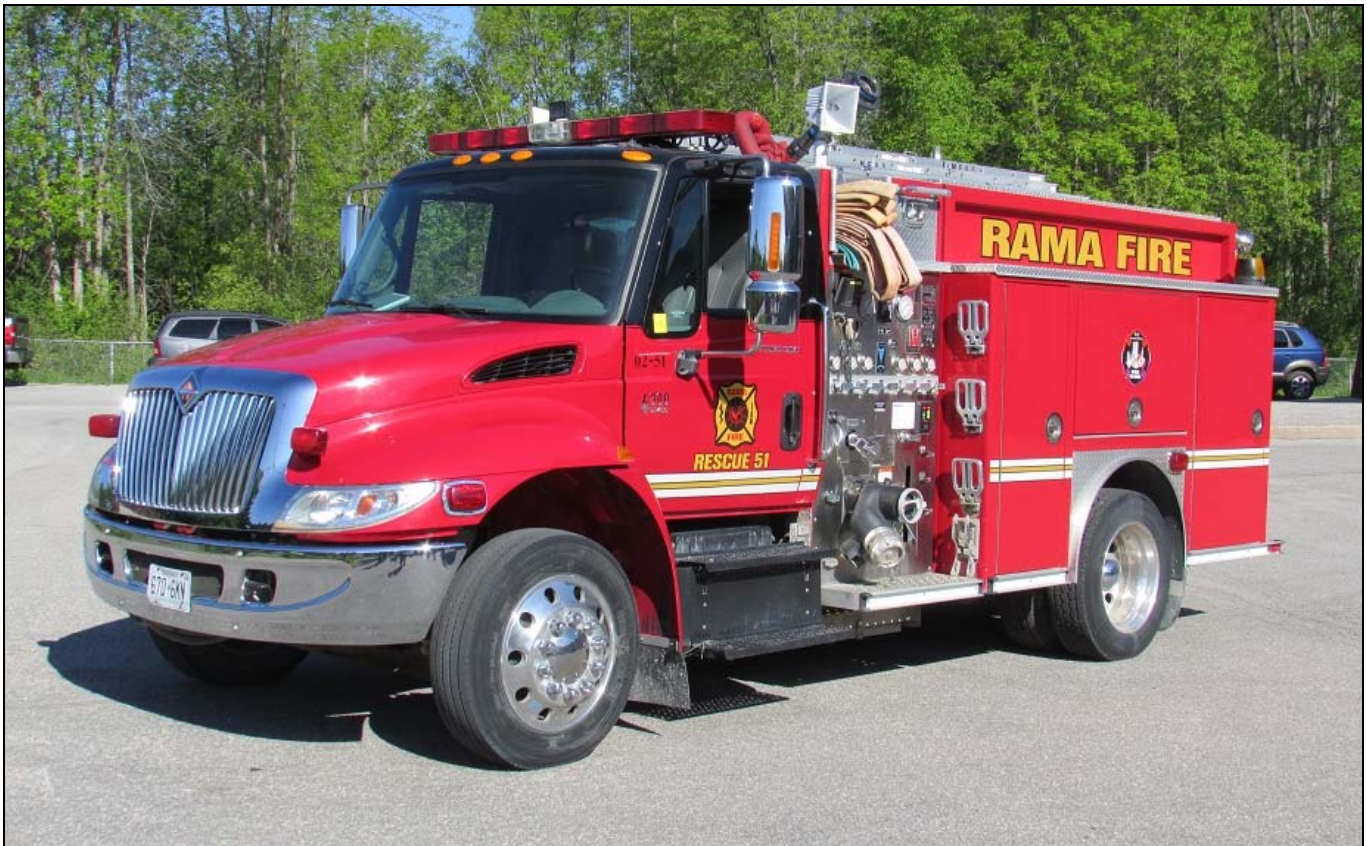
Two more from the May tour. Rama Rescue 51, a 2002 IHC 4300/Superior rig with a 625igpm pump, 300gwt and 30gft. It carries Superior number SE 2705. Oro Medonte Tanker 5 is a 2007 IHC 4400/Metalfab product with a 420igpm pump and 1600gwt. SN M07-8073 (Desmond Brett)
