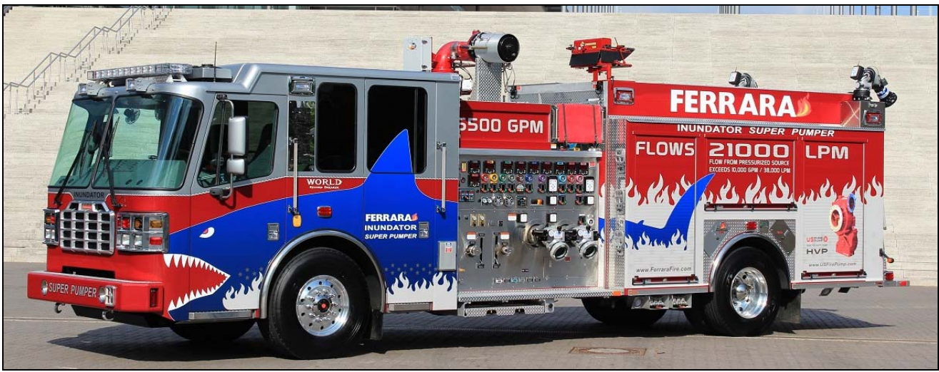
This impressive beast was on display at Intershutz. It's a 2015 Ferrara Inundator and, as indicated, flows 5500gpm or 21,000LPM, same as a decent sized fire boat. (Dave Stewardson photos)
