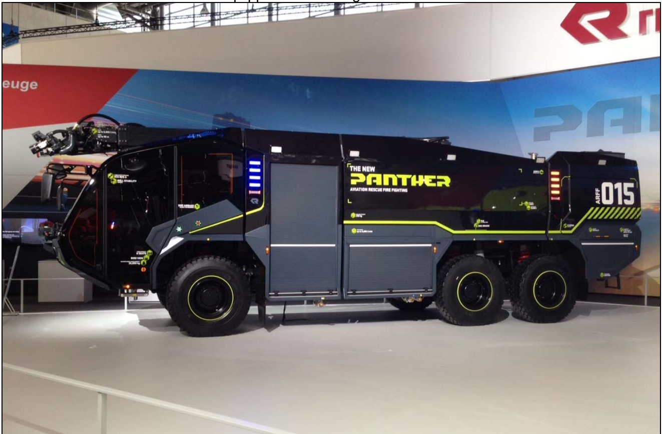
Rosenbauer unveiled the new Panther ARFF truck at Interschutz. The 4x4., above, and the 6x6, below, which has an 8000LPM pump, 12,500LWT, 1500LFT and carries 250kg of powder. This one is also equipped with a Stinger 54 HRET.
