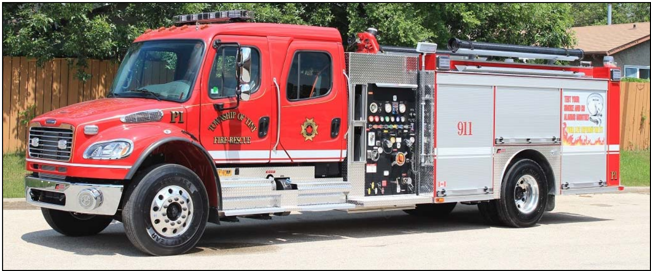
Tiny Twp., ON received this 2015 Freightliner M2-106/Fort Garry pump, along with a twin, for P.1, It has a 1250gpm Waterous pump and 800gwt. Another Fort Garry rig went to s/n M627
