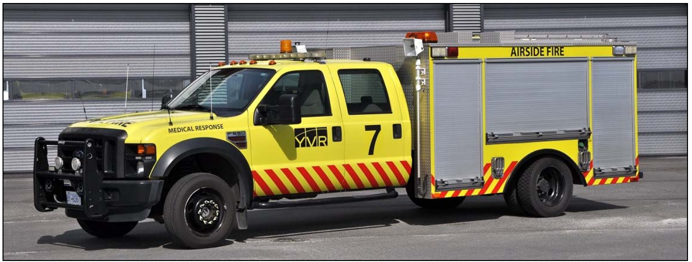
Vancouver Airport Red 7, the medical response vehicle, is a 2009 Ford F550 SD XL 4x4 chassis, equipped with an ERS body, transferred from an earlier light rescue.
