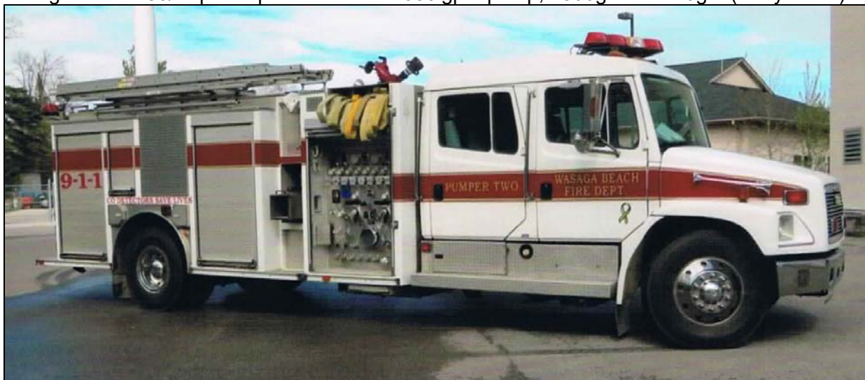
From the May tour: Wasaga Beach Car 2, a 2004 Ford F-150 pick up, and Pumper 2, a 2001 Freightliner FL80/Superior product with a 1050igpm pump, 1500gwt and 20gft. (Larry Ward)
