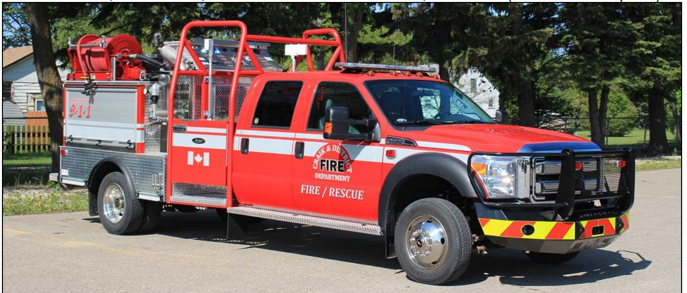
This 2016 Ford F550 4x4/Acres brush unit has a 275igpm Darley pump, 400gwt and 20gft. (D. Stewardson)
