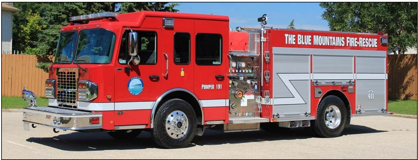
Blue Mountains new P.191 is a 2016 Spartan Metro Star/Fort Garry product with a 1250igpm Hale pump, 800gwt and 25gft. It also has a FoamPro 100 FS. S/N M731
