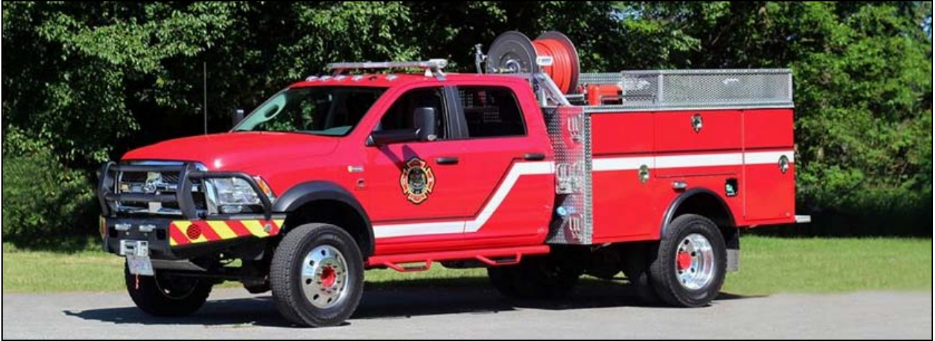
Fort St. John, BC just put this 2014 Dodge Ram 5500 4x4/SVT/2016 Profire mini in service as Brush 1. It sports a 200igpm pump, 300gwt and 10gft(A). It was purchased from Safetek, having been used by them as a demo. (Safetek Fire photo)
