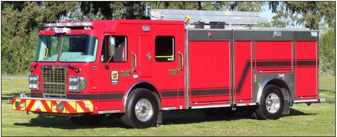
Justice Institute of BC now runs this 2016 Spartan Metrostar/Smeal pump, with a 1555igpm pump, 500gwt, and 40gft(A) with a CAFS . (Shane MacKichan photo)
