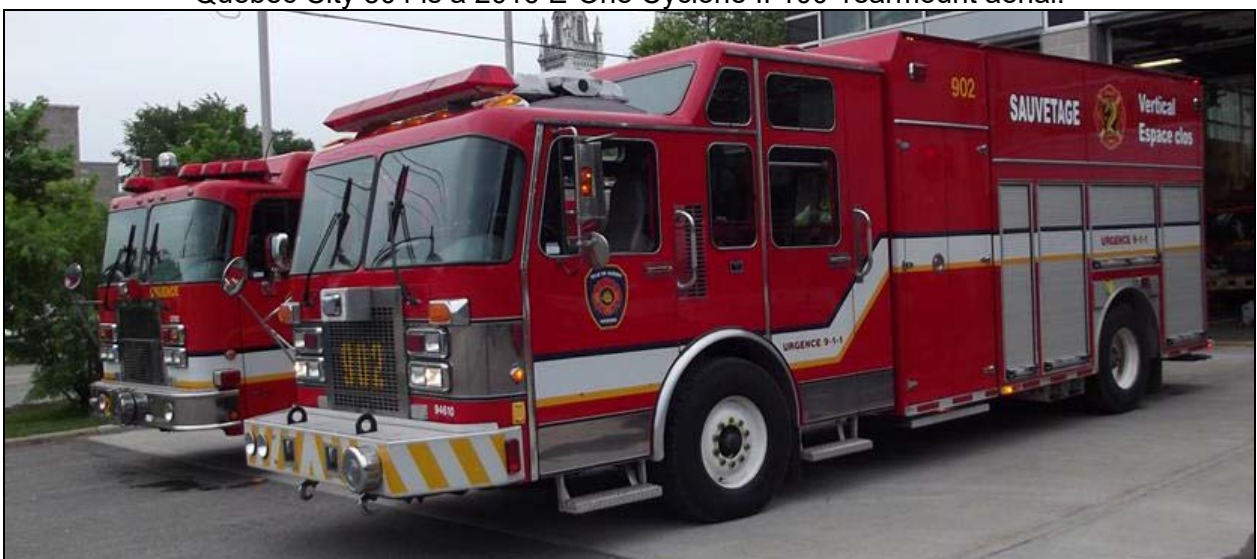
U.902 is a 1994 Spartan Gladiator/NOVAQuintech heavy rescue, rebuilt by the shops in 2008 as a tech rescue vehicle. It originally served in Ste.-Foy. (Rick Loiselle photos)
