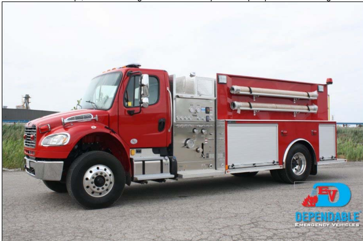
Mapleton, ON just received this 2016 Freightliner M2-106/Dependable pumper/tanker. It has a 1250igpm pump, and a 2000gwt. (Dependable Emergency Vehicles)
