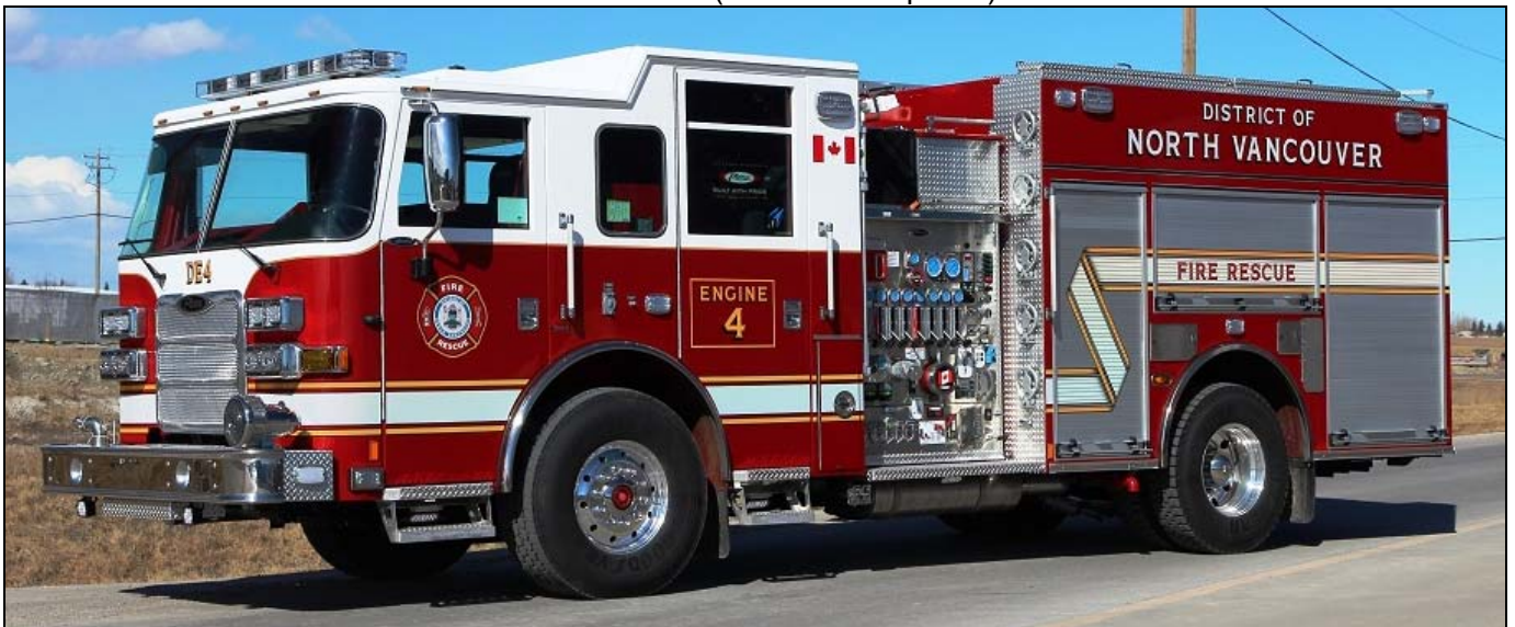
North Vancouver Dist. Engine 4, 2016 Pierce Arrow XT pumper, is one of two delivered in the spring. They have 1750igpm pumps, 330gwts and 25gfts. S/N 28956-2. (Terry Yip photo)
