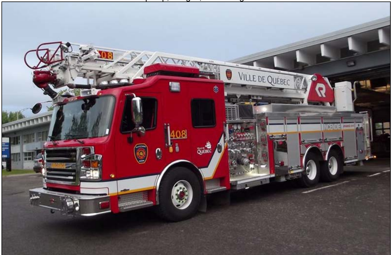
Quebec City U.408 is a 2015 Rosenbauer Viper quint. Built on a Commander chassis, it came with a 1750igpm Hale pump, 300gwt, twin foam tanks and a 100' aerial ladder. (Rick Loiselle photos)
