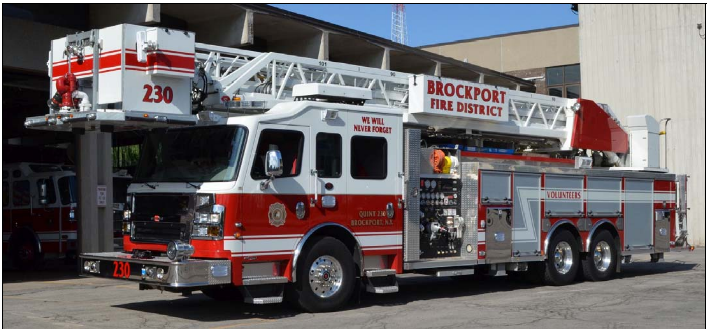
Shots from the Monroe County Tour: Brockport Fire District Quint 230, a 2014 Rosenbauer Commander Cobra 105' Platform equipped with a 2000gpm pump and 300gwt. S#737114
