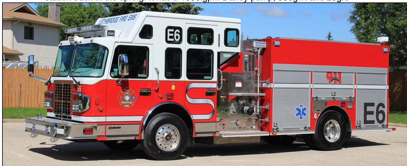
Lethbridge, AB recently acquired a 2015 Spartan Metro Star/Fort Garry pumper. Engine 6 has a 1050igpm Darley pump, 800gwt and 25gft. s/n 692. (Dave Stewardson photos)
