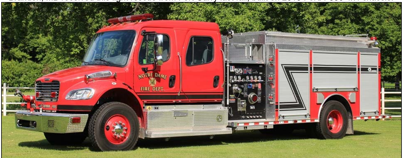
Back in May, Notre Dame de Lourdes, MB took delivery of this 2016 Freightliner M2-106/Rosenbauer pumper with a 1050igpm Rosenbauer pump, 1000igwt, and 20gft. s/n 1718416.
