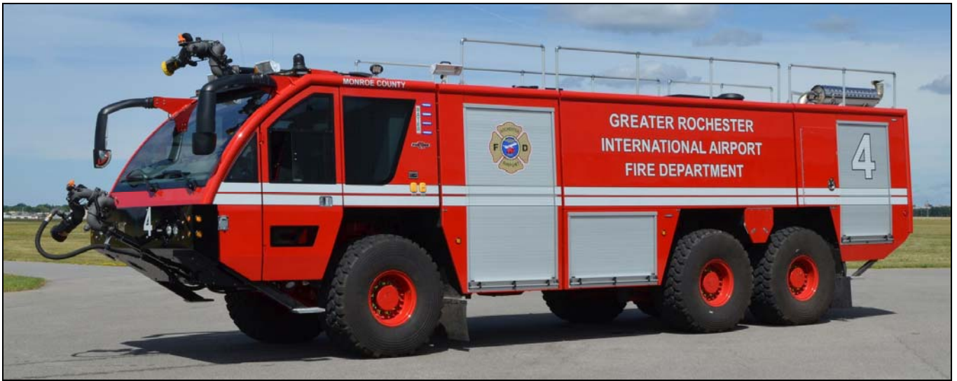
Three from Greater Rochester International Airport; Rescue 4, a 2016 Rosenbauer Panther 6x6 just delivered with an 1800gpm pump, 3000gwt, 400gft and 500# Purple K. S#104099
