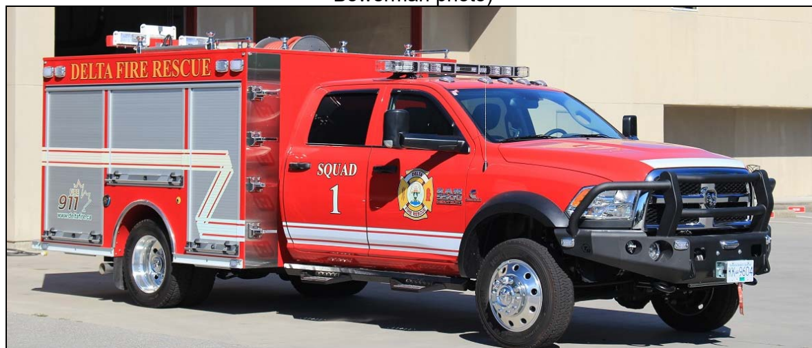
Delta, BC Squad 1, delivered in April, is a 2016 Dodge Ram 5500 HD/ITB/ProFire collaboration, with a 200igpm pump, 167gwt and 8gft(A) with a CAFS.
