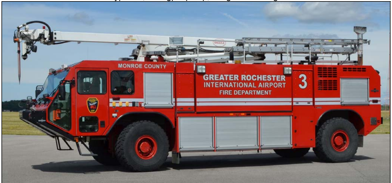
Rescue 3 is a 2006 Oshkosh Striker 4x4 with a 50' Snoodle. It's also equipped with a 1500gpm pump, 1500gwt, 200gft and 500lbs Halotron, SO87129. (Bob Rupert photos)
