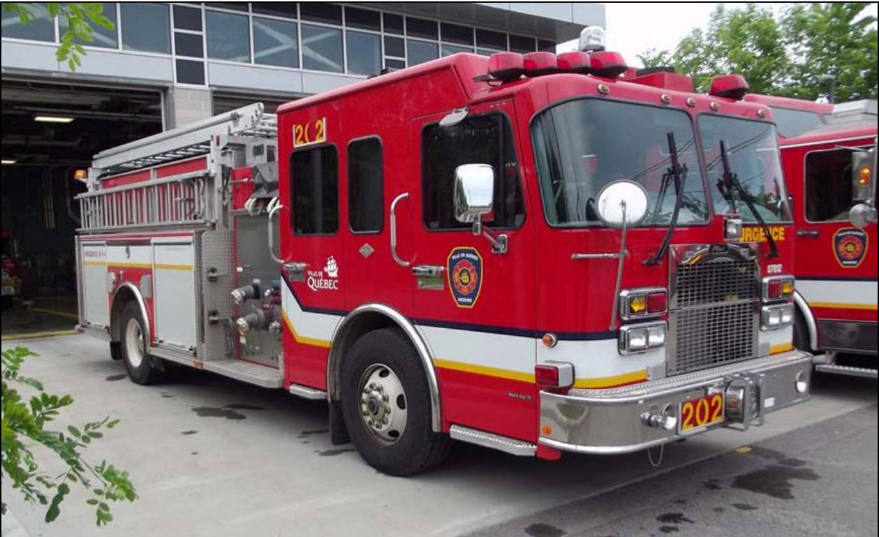
Quebec City U.202 is a 2007 Spartan Metro Star/Maxi Métal pumper, with a 1250igpm pump, 580gwt, and 2x20gft.
