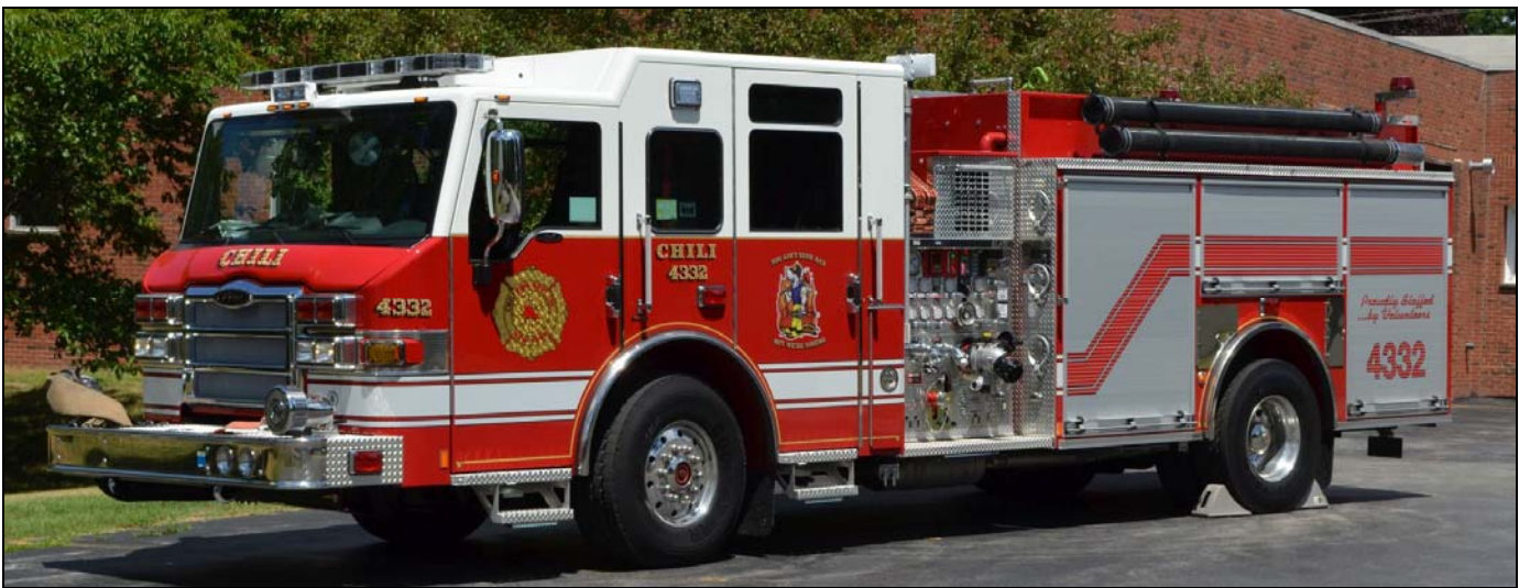
Chili Engine 4332 is a 2015 Pierce Impel with a 1250gpm pump, 1000gwt and 30gt. Job# 27949-03.
