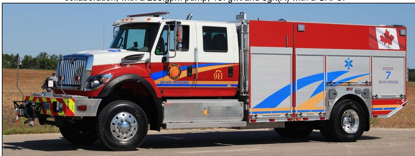
Cypress County, AB Engine 7 is assigned to the Seven Persons station. It is a 2016 IHC 7400 4x4chassied Fort Garry rig, 840igpm Waterous, 1000gwt, 25gft with pump & roll. s/n 700 (Dave Stewardson photos)
