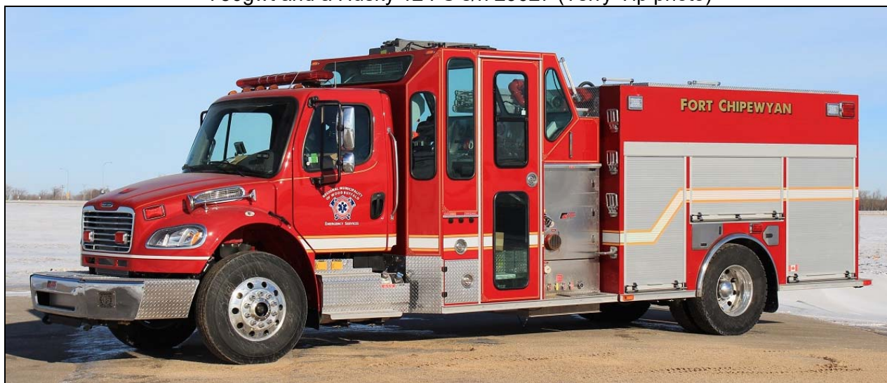
Wood Buffalo, AB placed this 2016 Freightliner M2-106/Fort Garry pump in their Fort Chipewyan station back in the spring. It has a 1050igpm Darley pump, 900gwt and 20gft.
