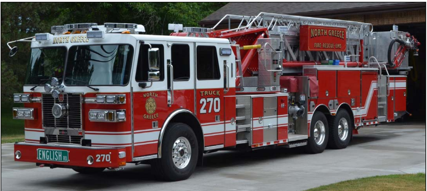
North Greece Quint 270 runs this 2015 Sutphen 100' tower, with a 2000gpm pump, 300gwt, 30gft.
