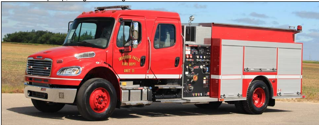
Iroquois Falls Unit 11, a 2016 Freightliner M2/Fort Garry pumper equipped with a 1050igpm Hale pump, 800gwt and 25gft. S/N M704 (Dave Stewardson photos)
