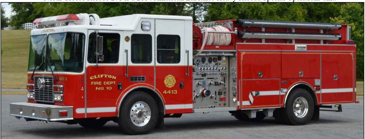
Clifton, NY Pumper 4413, a 2010 HME/4 Guys product, 1750gpm pump, 1250gwt, 100gft. S#F-2719
