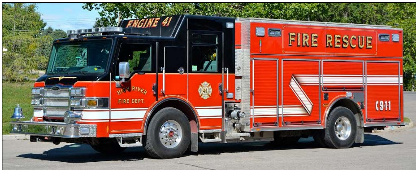
High River, AB Engine 41 is now running a 2016 Pierce Velocity PUC with a 1500gpm Hale pump, 750gwt and a Husky 12 FS s/n 29027 (Terry Yip photo)
