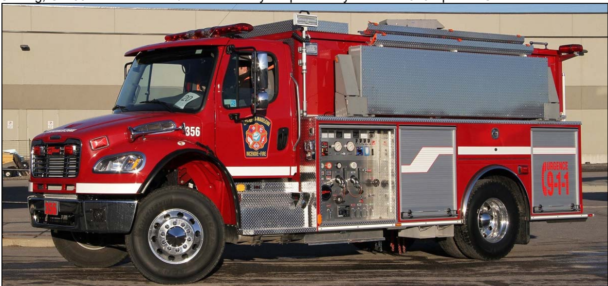
Isles-de-la-Madelaine, QC Unité 356 is a 2016 Freightliner M2-106/Carl Thibault pumper/tanker with a 1050igpm pump, 1500gwt and a 30gft. SN#2707
