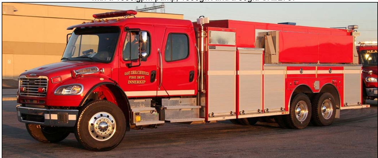
East Zorra-Tavistock, ON put this 2016 Freightliner M2-106 / Metalfab pumper/tanker into the Innerkip station. It has an 840igpm pump and 2500gwt. (Ian Duke photos)
