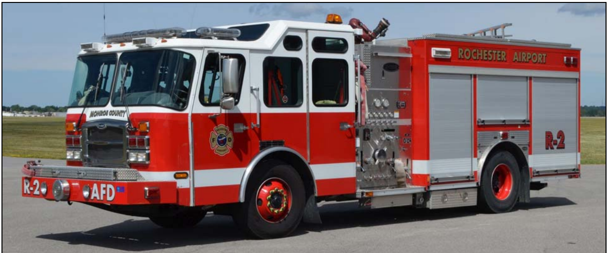
Rescue 2 is a 2009 E-One Typhoon, 1250gpm pump, 900gwt and 100g ARFFFP foam. SO#134827
