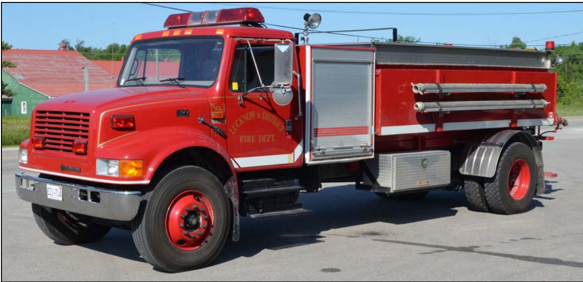
Photographed on the June Tour, this is Lucknow Tanker 3, a 2001 International 4900/Fort Garry rig equipped with a portable pump and a 1700igwt. S#856755 (Bob Rupert photo)
