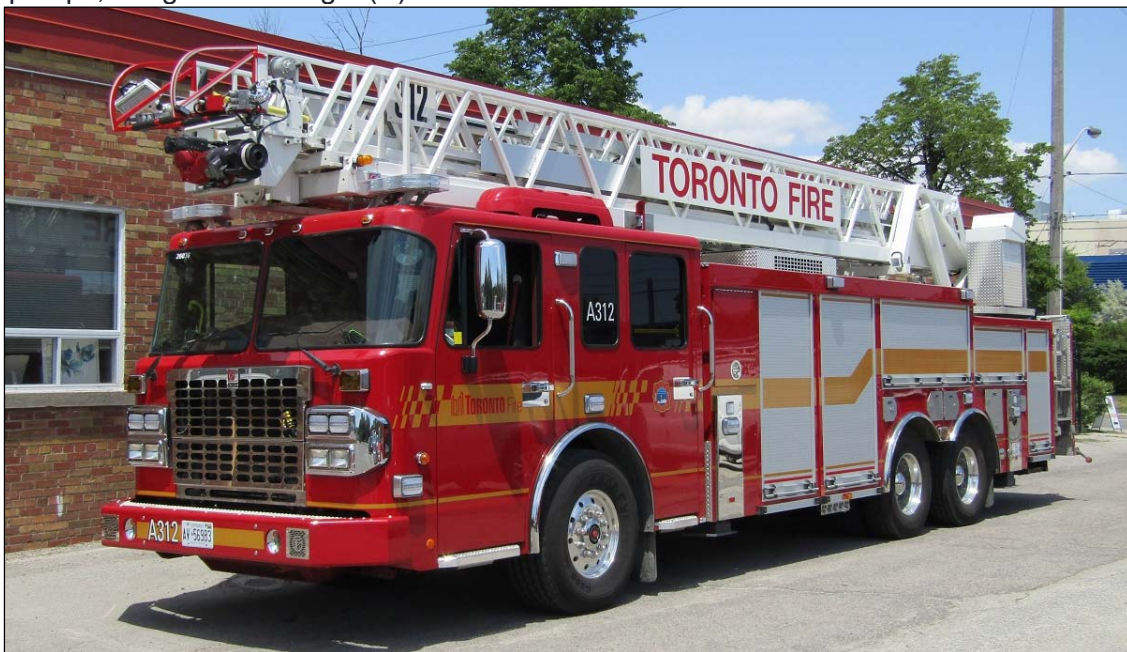
Aerial312, one of four 2017 Spartan Gladiator/Smeal105'rearmounts, no pump or water.
