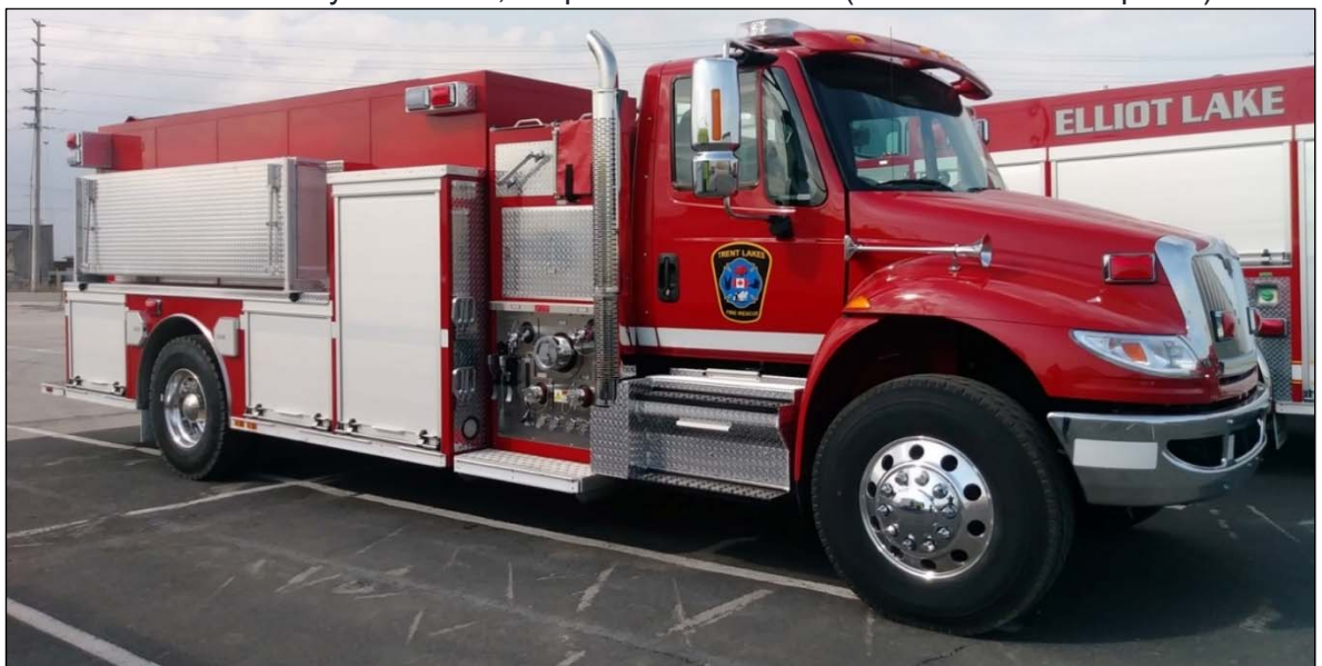
Trent Lakes, ON, 2018 IHC 4400/Metalfab rig, 1050igmpump, 1300gwt. (Larry Thorne photo)
