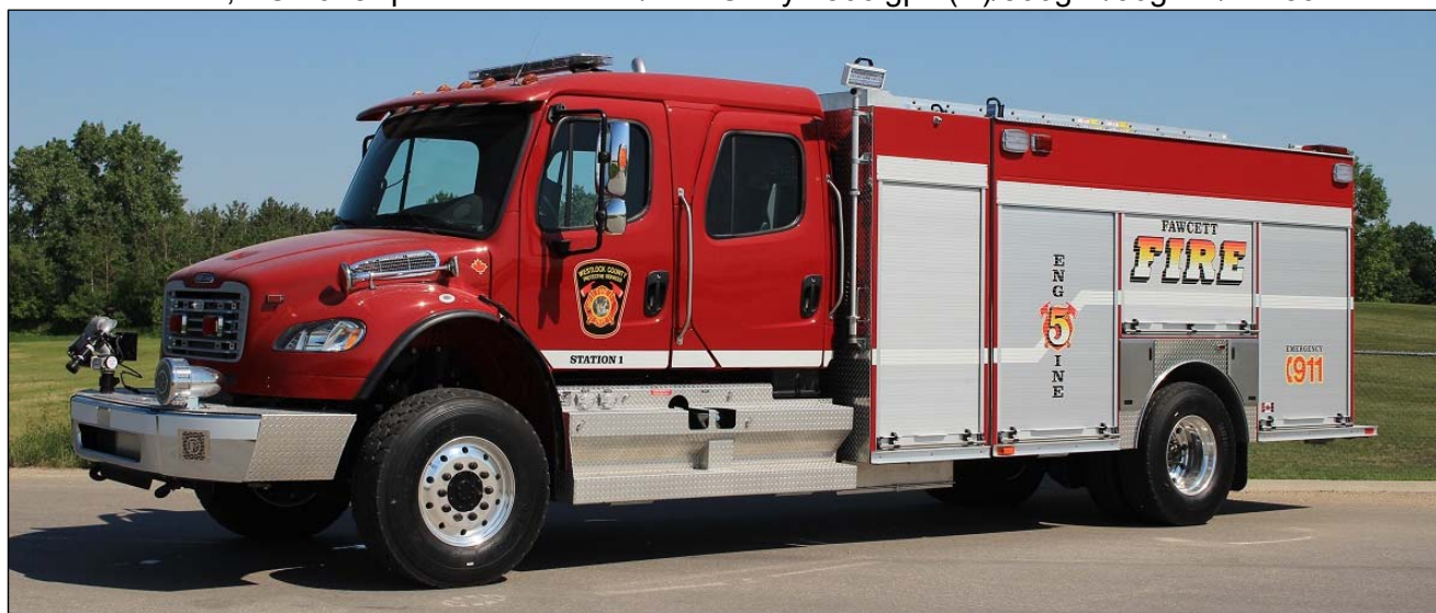
Westlock County (Fawcett), Alberta E-52018 Freightliner M2-106/Fort Garry1050igpm(D)/1000gwt/30gft s/n #M892
