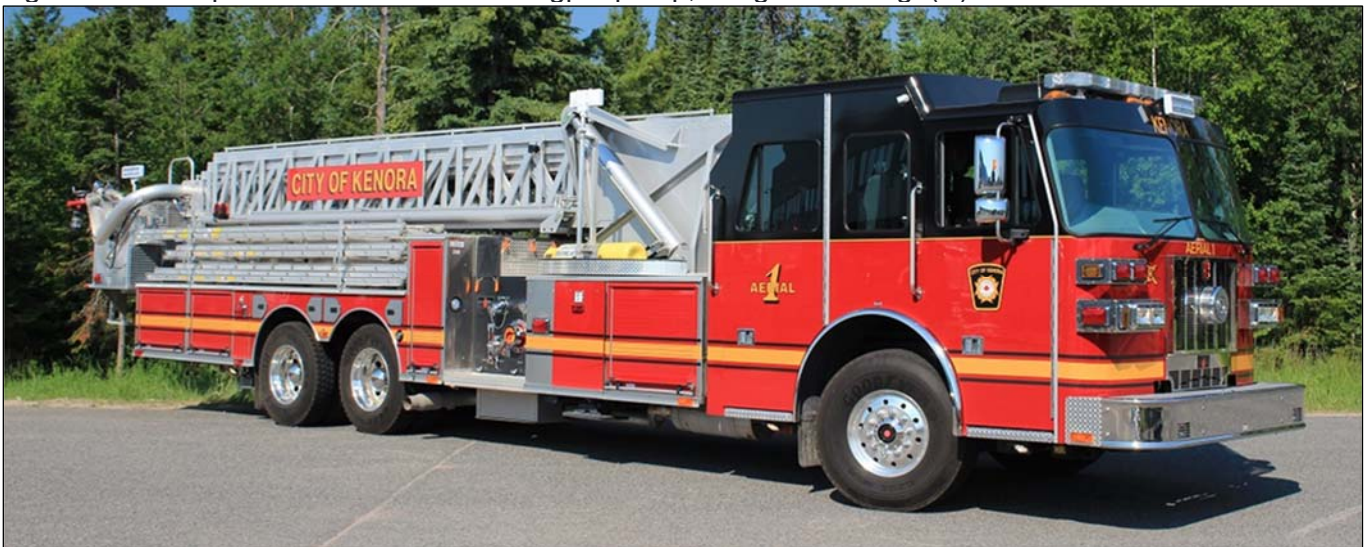
Kenora, ON Tower 1, officer's side this time, a 2018 Sutphen Fort Garry quint with a 1250igpm Hale pump, 250gwt and 95' tower. Fort Garry s/n M909, Sutphen s/n HS5829. (Dave Stewardson photo)
