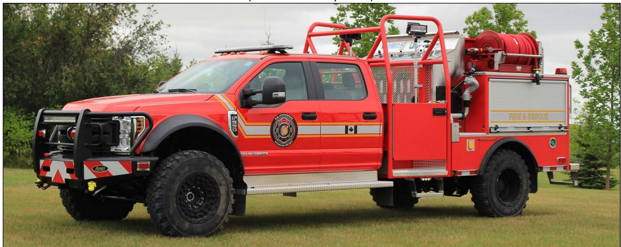
The R.M. of Enterprise, SK just got this 2018 Ford F550 4x4/Acres brush rig with a 230igpm Waterax B2X pump, 400gwt and 20gft. It runs from Richmond. sn180720167 (Dave Stewardson photo)
