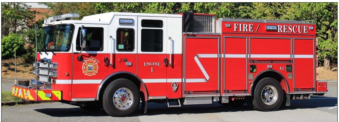
Engine 1 in New Westminster, a 2016 Pierce Enforcer pumper sporting a 1750igpm pump, 440gwt and a 40gft.s/n29792-01 (Dave Stewardson photo)
