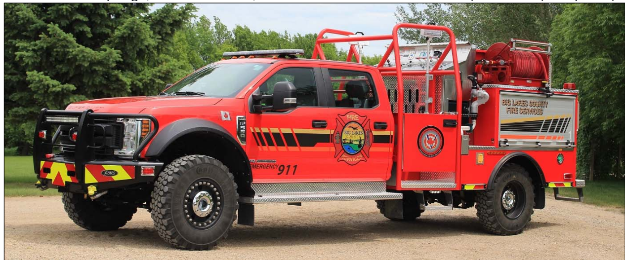
Big Lakes County, AB received this 2018 Freightliner M2-106 4x4/Acres brush unit. It has a 230igpm Waterous pump, 400gwt and 20gft. s/n #180410164 (Dave Stewardson photo)
