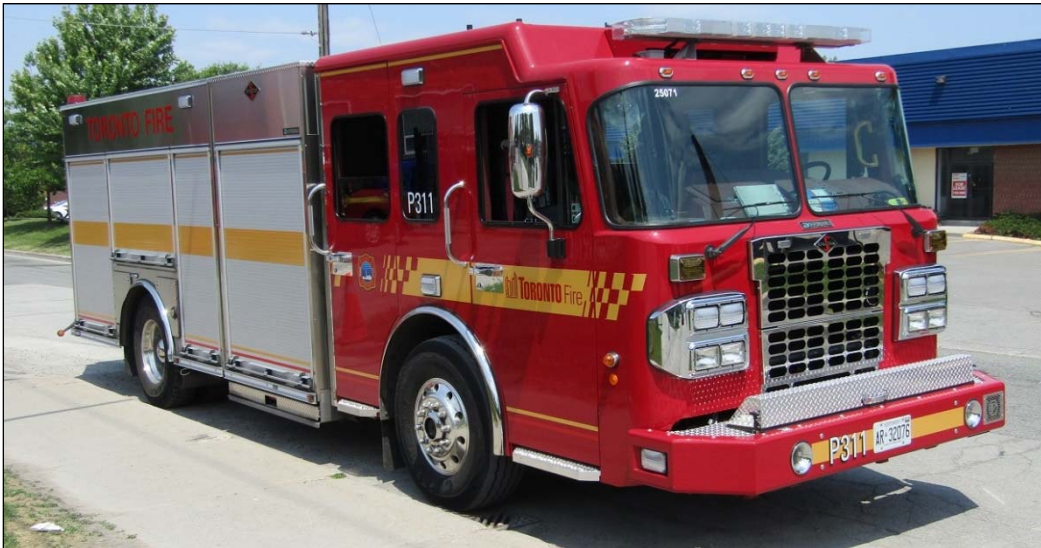
Pump 311, a 2017 Spartan Metro Star/Spartan ERV/Dependable rig from the first batch (of three) with 1750igpm pumps, 500gwts and 25gfts(A). Job # 215193
