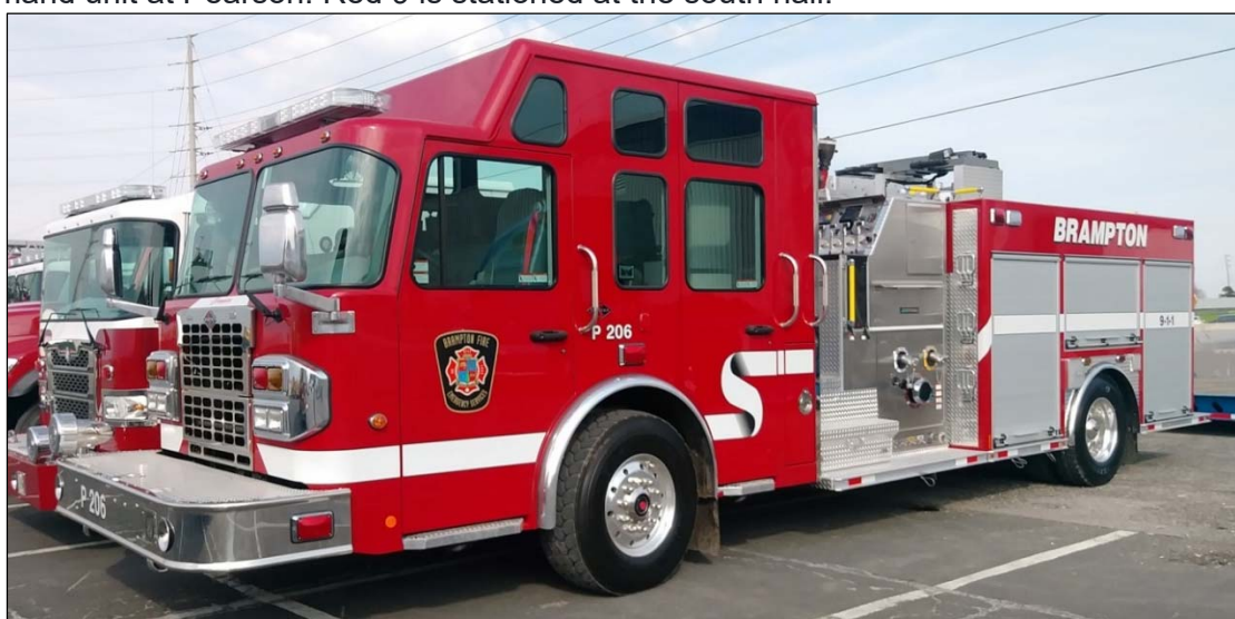
Brampton Pumper 206 - 2017 Spartan Metro Star/Dependable, 1250igpm/500gwt/25gft.
