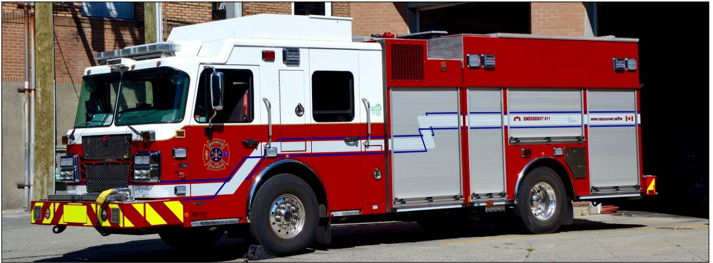
Vancouver Engine 4 using a Service Ready engine (Fully equipped spare), a 2016 Spartan Sirius/Smeal pumper with a 1780igpm pump, 440gwt, 63gft (A) and a CAFS.
