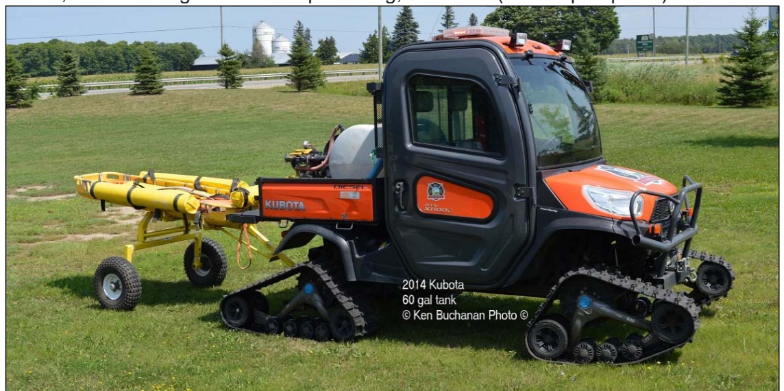
A reprise from last year's tour in Clearview Twp. Ken was lucky enough to have bright sunshine when he stopped by Station 1 in Stayner. ATV 1 is a 2014 Kubota RTV 1100, seen here with a skid mount portable pump and 60gwt,Pump 12 is a 2010 Pierce Contender, 1050igpm/1500gwt. (Ken Buchanan photos)
