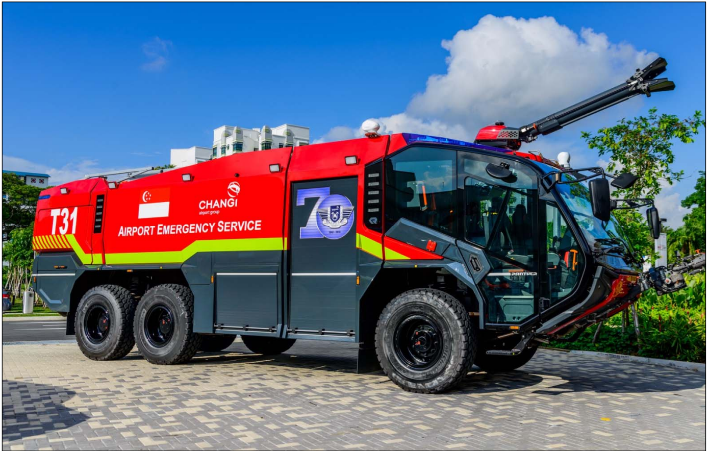
Changi Airport T.31, delivered this spring, is a 2018 Rosenbauer Panther 6x6 with a 12,500L tank and 1500L foam tank. The 70 refers to Changi Airport's 70 th anniversary.
