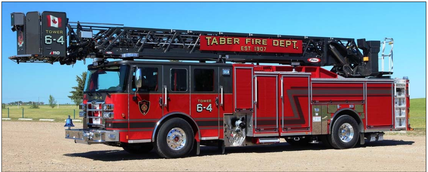
Taber, AB Tower 6-4.2018 Pierce Dash Ascendant 110' tower with a 1250igpm Hale pump, 400gwt, 30gft and Husky 3 foam system.Job # 32001. (John Bowerman Photo)
