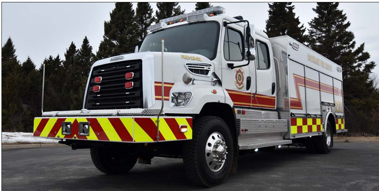
Cochrane, AB R.151 2018 Freightliner FLD-120/Rosenbauer FX 1250gpm(R/500gwt/30gft. j/n 14356 (Rosenbauer photo)
