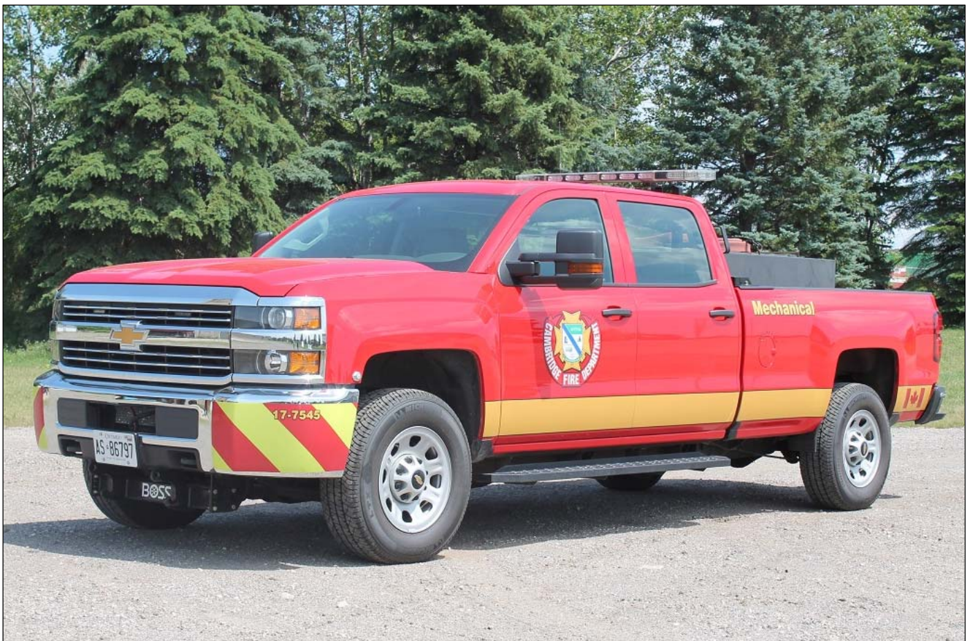
Also new is this 2017 Chev Silverado 2500 HD pick up normally used by the mechanical division but it also doubles as a wildland rig with a skid mount unit equipped with a 25igpm pump and 200gwt. (Gary Dinkel)
