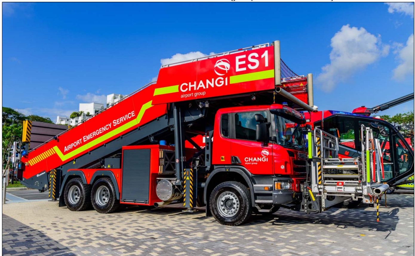
Changi Airport ES.1 is a Rosenbauer E8000 escape stair on a 2018 Scania chassis. It rises to 8.3m and is equipped with a Rosenbauer 2000LPM pump and carries 1400L of water. (Kenneth Lai photos)
