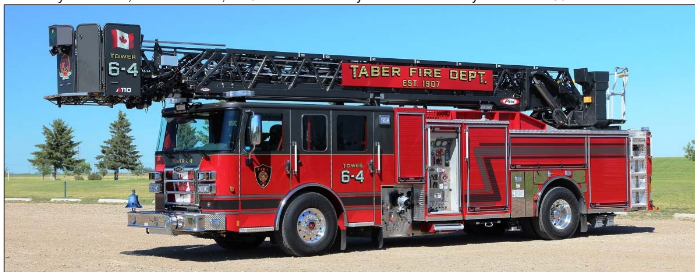
Taber's new Tower 6-4, with the pump panel this time: 2018 Pierce Ascendant 1500gpm Pierce pump, 500gwt, 110' aerial Husky 3 foam system. s/n 32001 (John Bowerman Photos)
