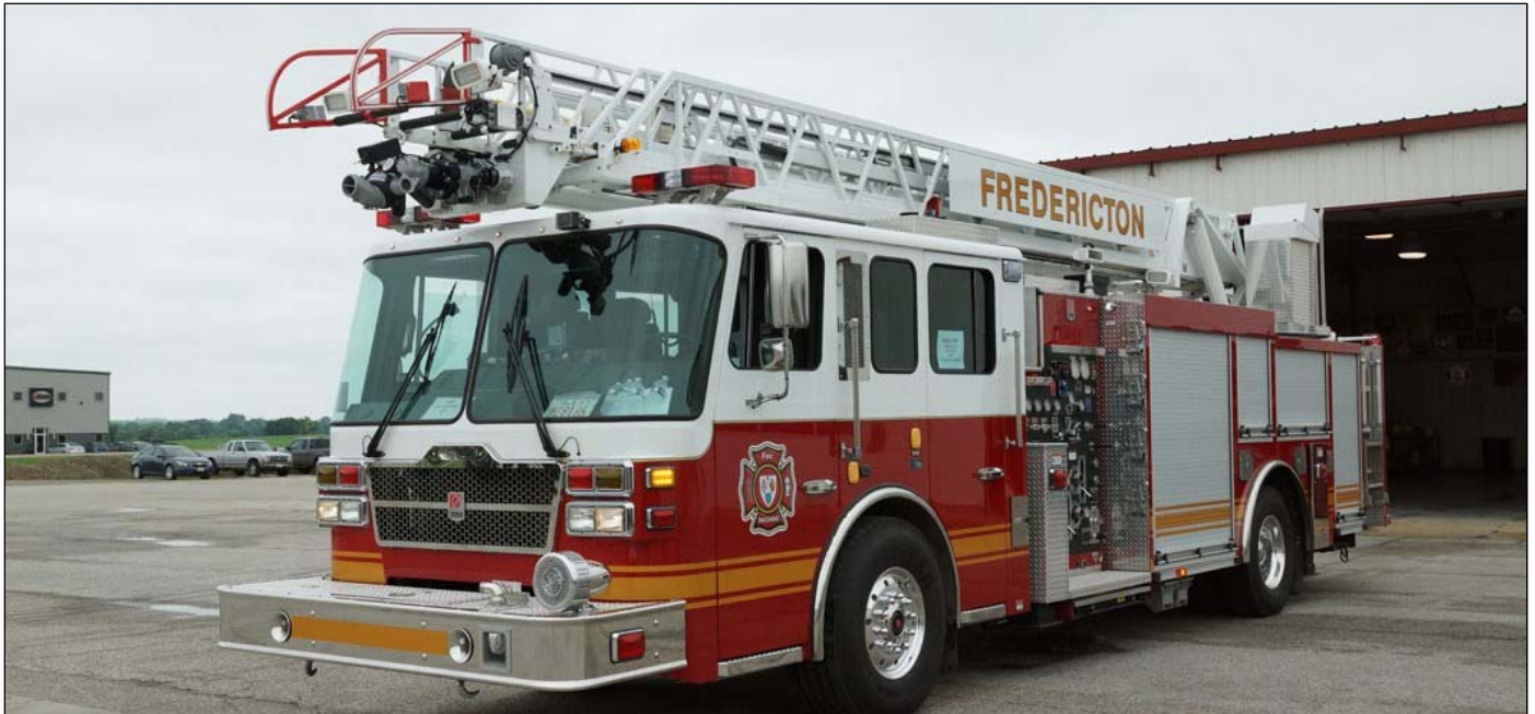
Fredericton Quint 1 - 2015 Smeal S450 aerial with a 1250igpm pump, 335gwt and 75' stick. (Smeal)
