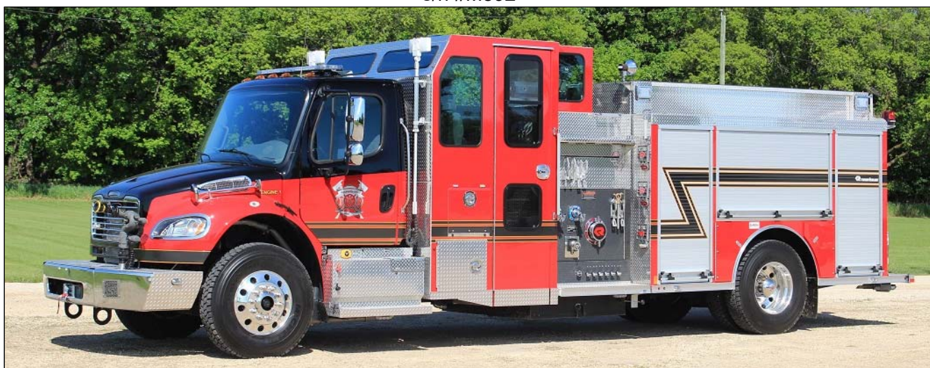
Potash Corp, SK (Rocanville)2018 Freightliner M2-106/Rosenbauer 1050igpm(R/1000gwt/25gft/CAFS s/n 17575(Dave Stewardson photos)
