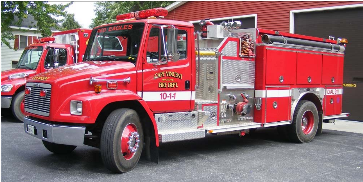
Cape Vincent, NY Engine 1011 is a 1999 Freightliner FL80/E-One, 1250gpm/1000gwt
