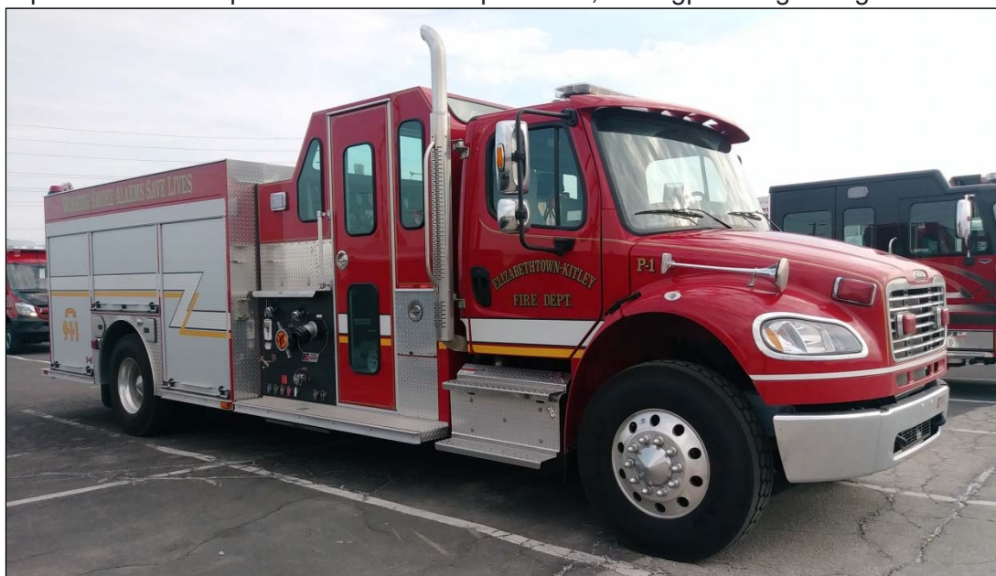
Elizabethtown-Kitley, ON Pumper 1, a 2018 Freightliner M2-106/Fort Garry 1050igpm Waterous pump, 830gwt and 25gft.s/n M879. (Larry Thorne photos)
