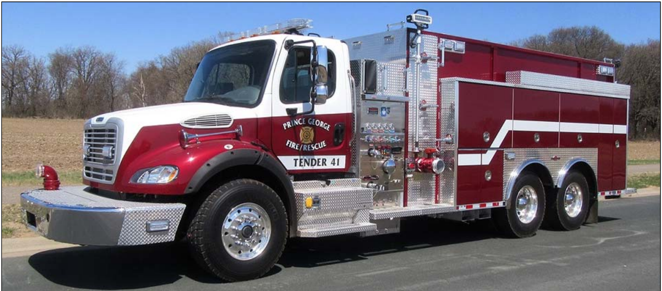
Prince George, BC T.41 2018 Freightliner M2-112/Rosenbauer 420igpm/2500gwt j/n 24362 (Rosenbauer)
