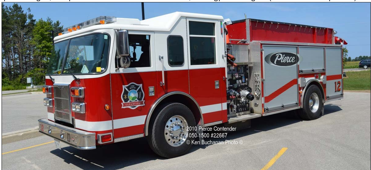
A reprise from last year's tour in Clearview Twp. Ken was lucky enough to have bright sunshine when he stopped by Station 1 in Stayner. ATV 1 is a 2014 Kubota RTV 1100, seen here with a skid mount portable pump and 60gwt,Pump 12 is a 2010 Pierce Contender, 1050igpm/1500gwt. (Ken Buchanan photos)
