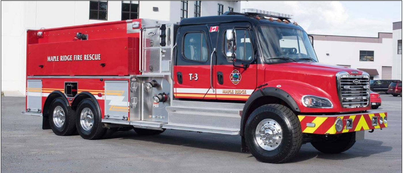
Maple Ridge, BC Tender 3, a 2018 Freightliner M2-112/Hub 840igpm/2250gwt j/n 1228 (Hub Fire Photo)
