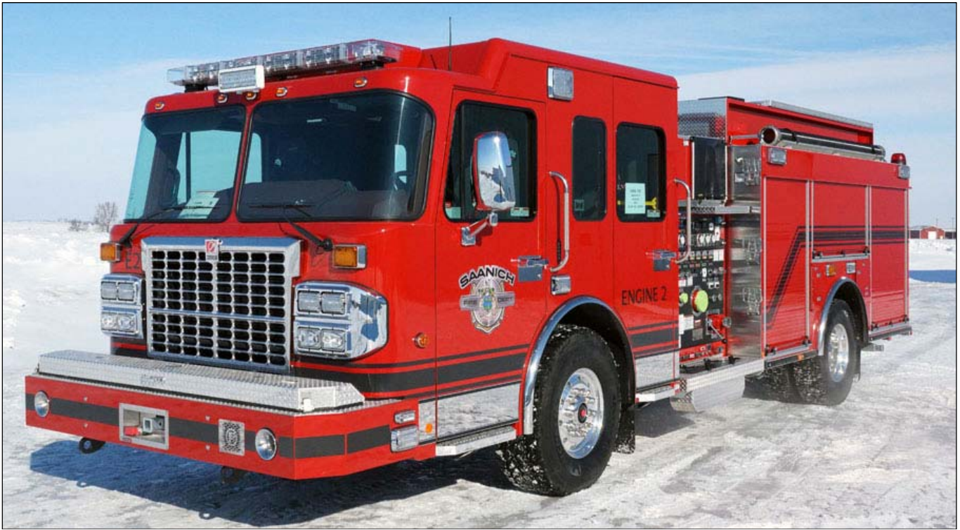
Saanich, BC Engine 2, a 2015 Spartan Gladiator/Smeal 1500igpm(W)/700gwt/50gft Advantus 6 FS s/n 514211 (Smeal Fire Apparatus Photo)
