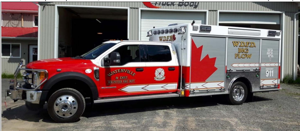
Waterville, NS new Big Flow 51 2018 Ford F550/Lantz 2500igpm pumper (Lantz Truck Photo)
