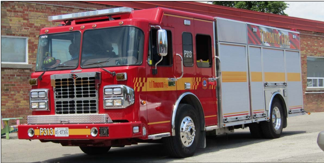
From the second batch for Toronto, this 2017 Spartan Metro Star/Spartan ERV/Dependable rig went to Pumper 313. It also has 1750igpm pump, 500gwt and 25gft(A). Job # 216007
