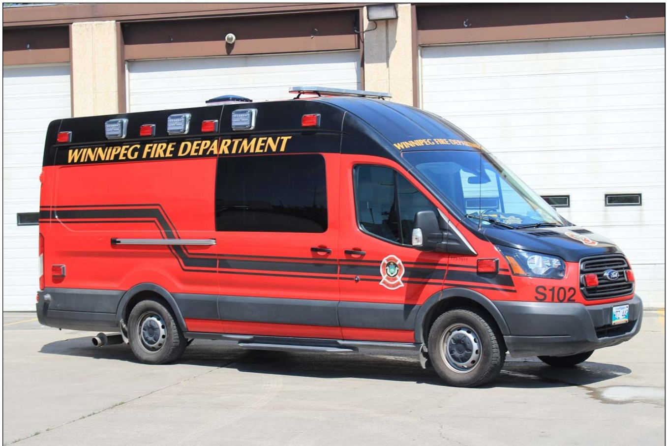
Winnipeg Squad 102, a 2017 Ford Transit with the body outfitted by a local firm; Absolute Auto Guard. There are currently two of these and they responded to medical calls and minor incidents to take the heat off the full size rigs. (Dave Stewardson photo)
