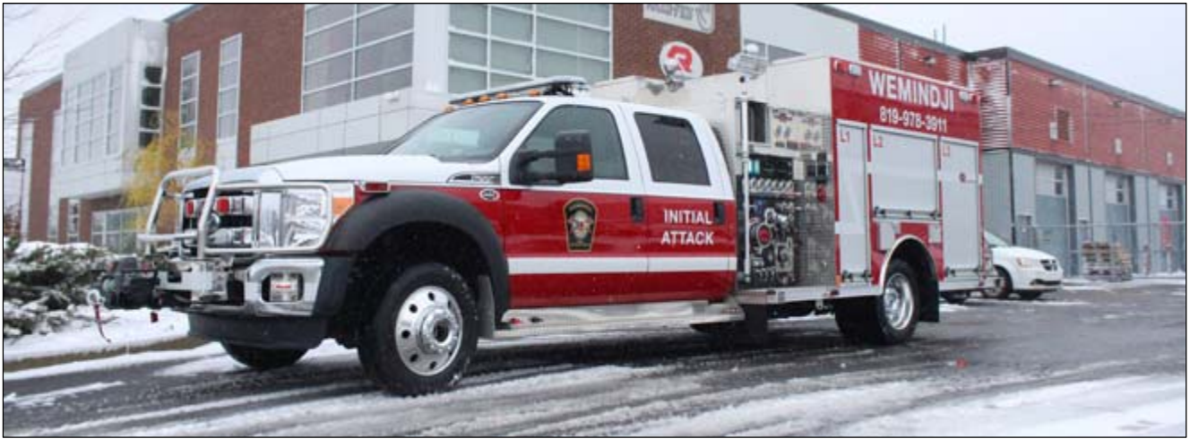
Wemindji FN, QC 2016 Ford F550/Rosenbauer 840igpm(R)/200gwt Foam Pro 2001/Rosy Fix Mix FSs
