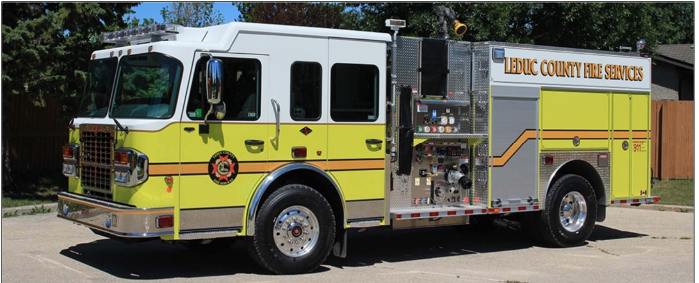
Leduc County, AB 2018 Spartan Metro Star/Fort Garry 1050igpm/1000gwt/10gft(A)/25gft(B). (D. Stewardson)
