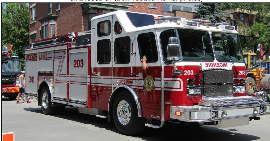
Laval, QC 203, a 2019 EpOne Cyclone pumper, 1250igpm Hale pump, 250gwt and 25gft. (Desmond Brett photo)
