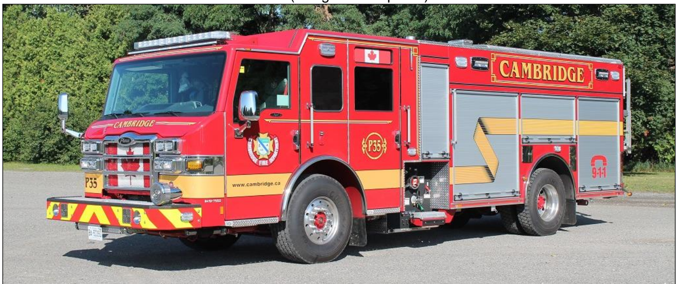
Cambridge Pumper 35 now has this 2019 Pierce Impel PUC, 1337igpm pump, 537gwt and 20ft. (Gary Dinkel photo)
