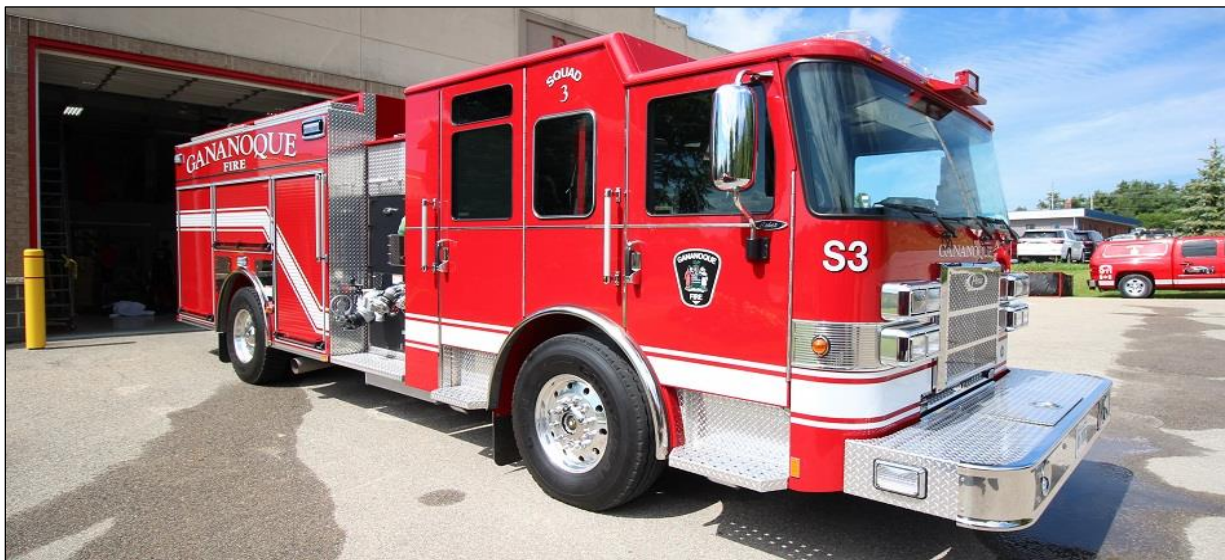
Newly in service Gananoque, ON Squad 3, a 2018 Pierce Saber pumper, with a 1250igpm pump, 640gwt and 30gft. Job no. 32324, ex-demo.
