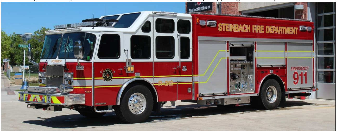
Steinbach, MB Rescue 212, a 2019 E One Typhoon 445igpm Hale pump, 333gwt.s/n 164737 (Dave Stewardson photos)
