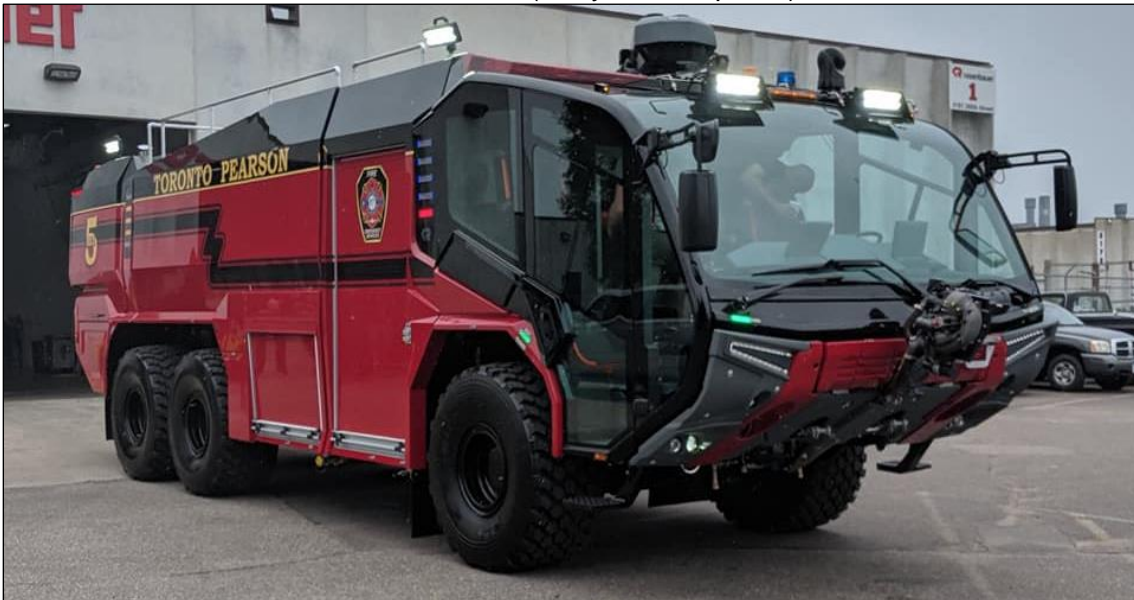
Pearson Red 5, a 2019 Rosenbauer Panther 6x6 1750igpm/2500gwt/330gft (Rosenbauer)
