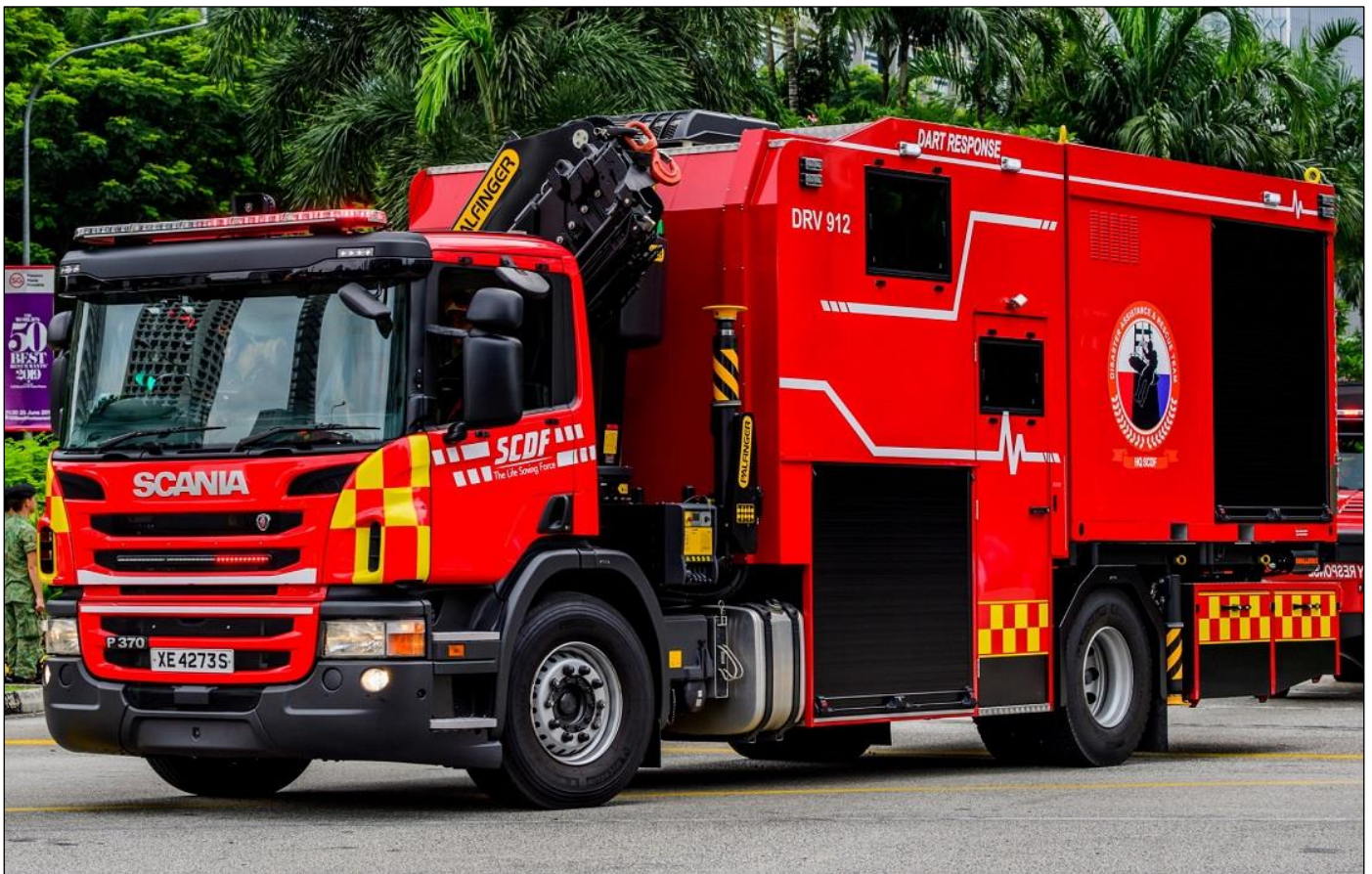
DRV912, a DART crane equipped Rescue Vehicle- on a Scania P370 chassis, Palfinger lift system.
