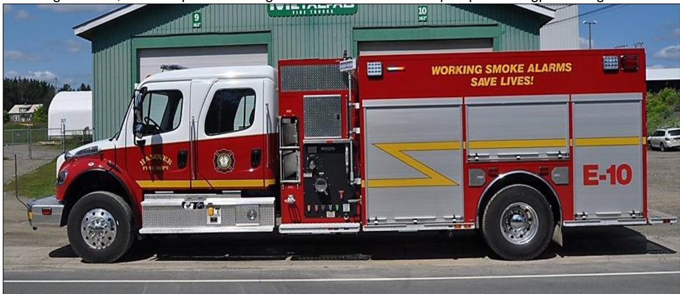
Hanover, ON Engine 10, a 2019 Freightliner M2 106/Metalfab pumper, 1250igpm/1200gwt
