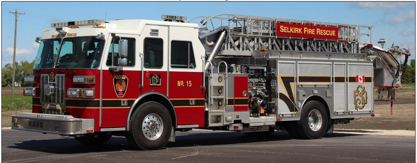
Another rig given an extended life, this 2008 Sutphen tower was completely rehabbed by Fort Garry this year. Selkirk, MB Unit 15 has a Hale Q-Max 1250igpm pump, 250gwt and 75' platform.
