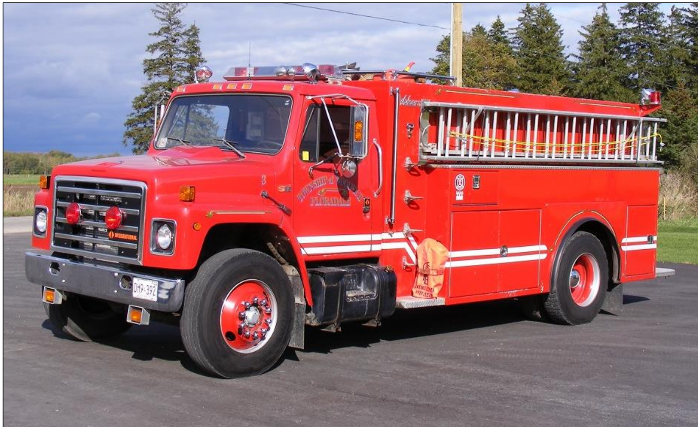
Woolwich Twp., Floradale Tanker 3, a 1989 IHC/Weber Fabricating product with a 1500 gallon tank.
