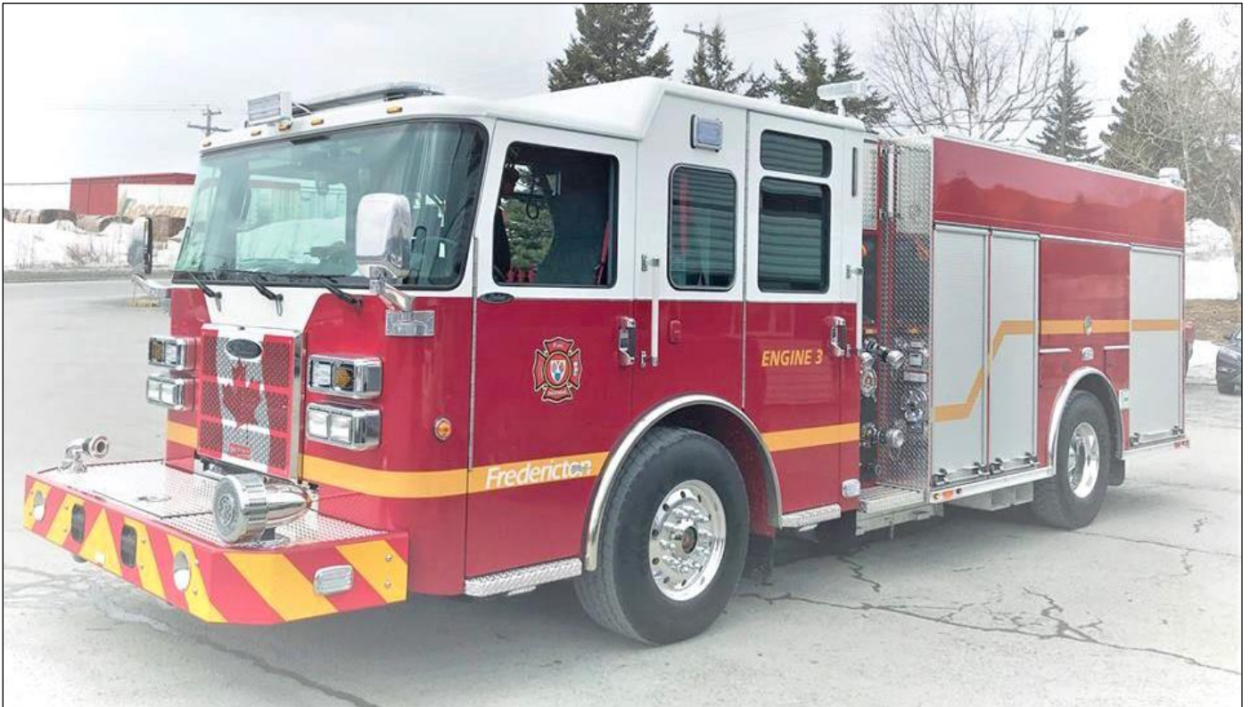
Fredericton, NB Engine 3, a 2019 Pierce Saber/Maxi Métal 1250igpm pump,1000gwt and 25gft (Maxi Métal Fire trucks photo)
