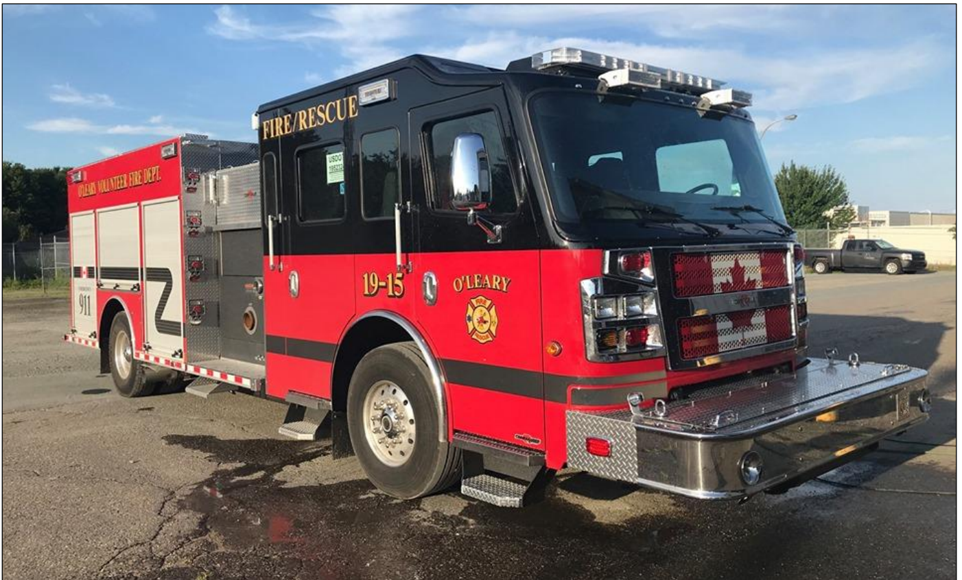
O'Leary, PEI Pumper 2 (Mutual Aid No. 19-15),a 2019 Rosenbauer Commander with a 1250igpm pump,1000gwt and 20gft(A)(Rosenbauer photo)
