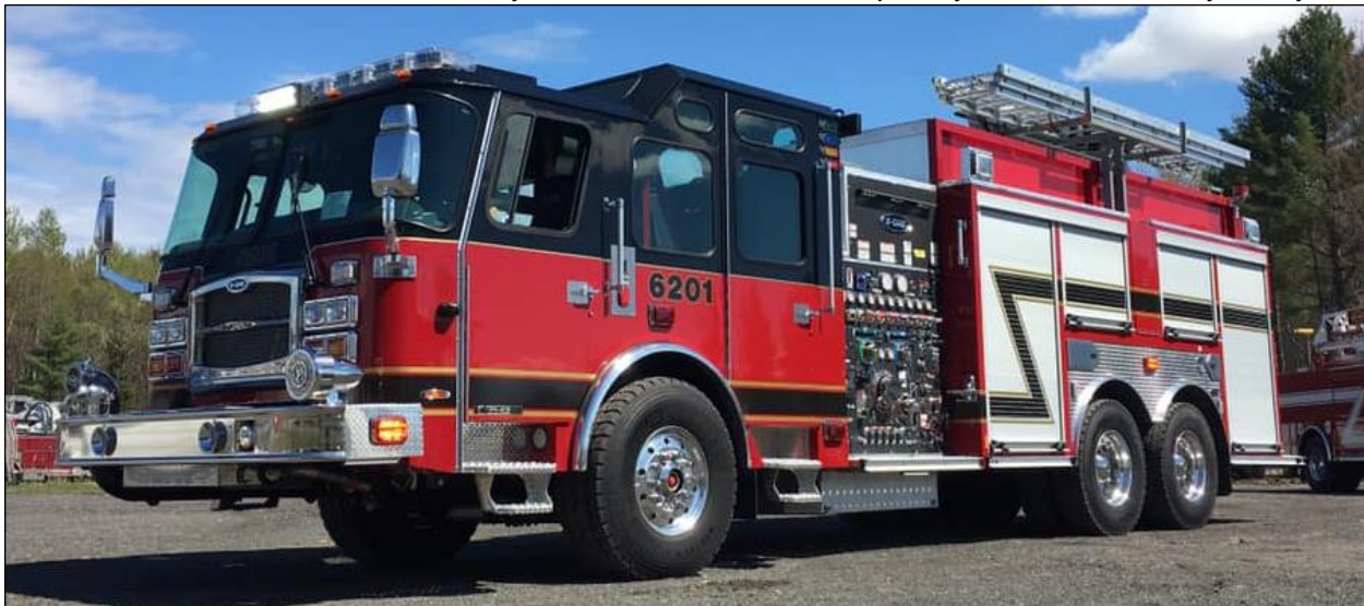
Drummondville, QC Unité 6201 - 2019 E-One Typhoon pumper/tanker 1250igpm, 2100gwt & 40ft. (SO#142298) (Photos courtesy 1200 degrees))
