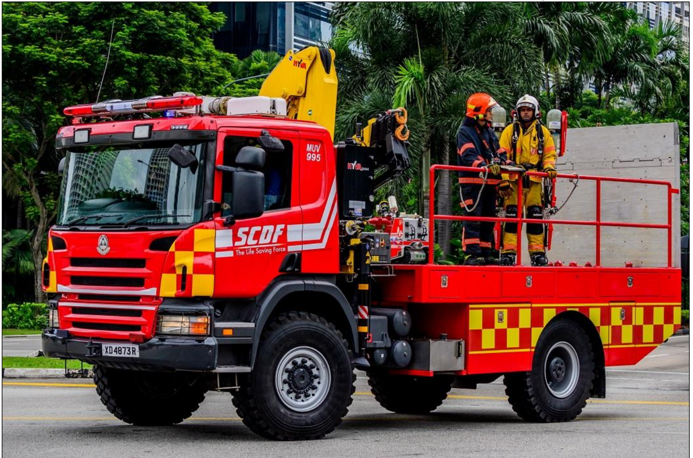
SCDF MUV995, another Scania Multi-Utility Vehicle. Equipped with a Hyva lift system. (Kenneth Lai photos)
