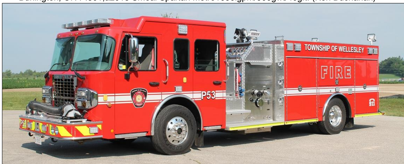
Wellesley Twp., ON Pumper 53, a 2019 Spartan Dependable 1250igpm pump, 840gwt and a 15gft.
