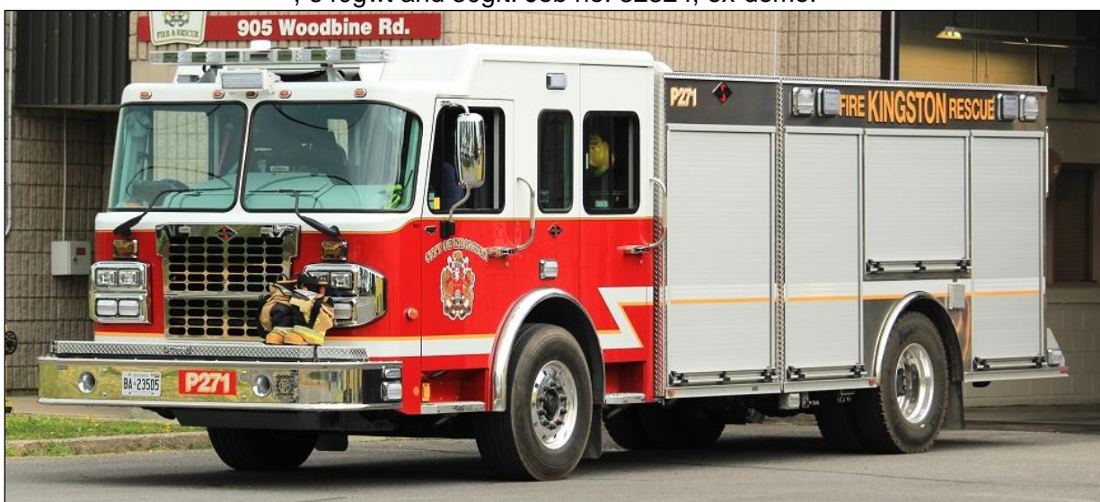
Kingston, ON P.271 2019 Spartan Metro Star/Spartan ERV 1500igpm/500gwt/40gft sn 218062-01 (Dan Tastard-Homer photos)
