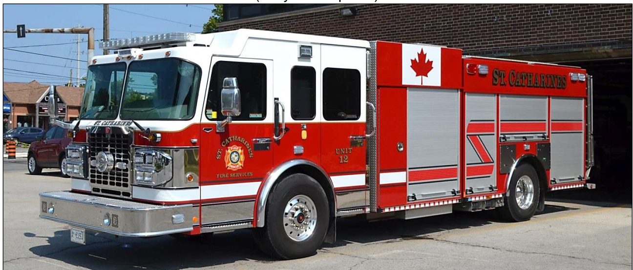
St. Catharines, ON Unit 12 running as Pump 1, a 2018 Spartan Metro Star /Smeal pumper, 1050igpm/600gwt/15ft SN 812121 (Bob Rupert photo)
