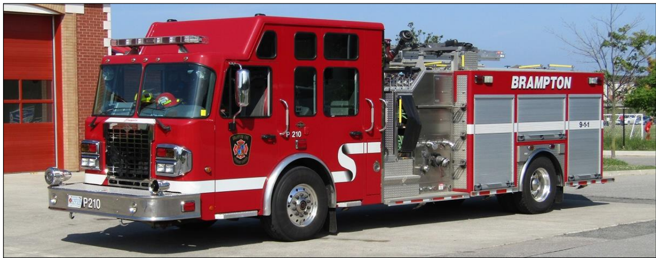
Brampton, ON Pumper 210, a 2012 Spartan Metro Star/Dependable 1050igpm/500gwt/25gft.
