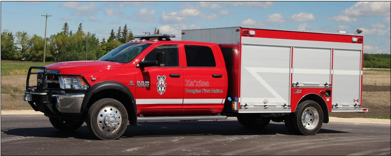
Xa'xtsa First Nations in Douglas, BC recently received this 2018 Dodge Ram 5500 4x4 brush unit equipped with an Odin CAFS, a 152igmpump, 225gwt and a 25ft.s/n M963
