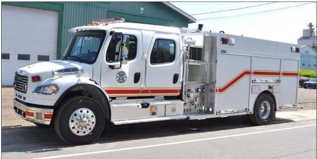
Magnetawan, ON Pumper 2019 Freightliner M2 106 / Metalfab pumper 1050igpm/1200gwt.
