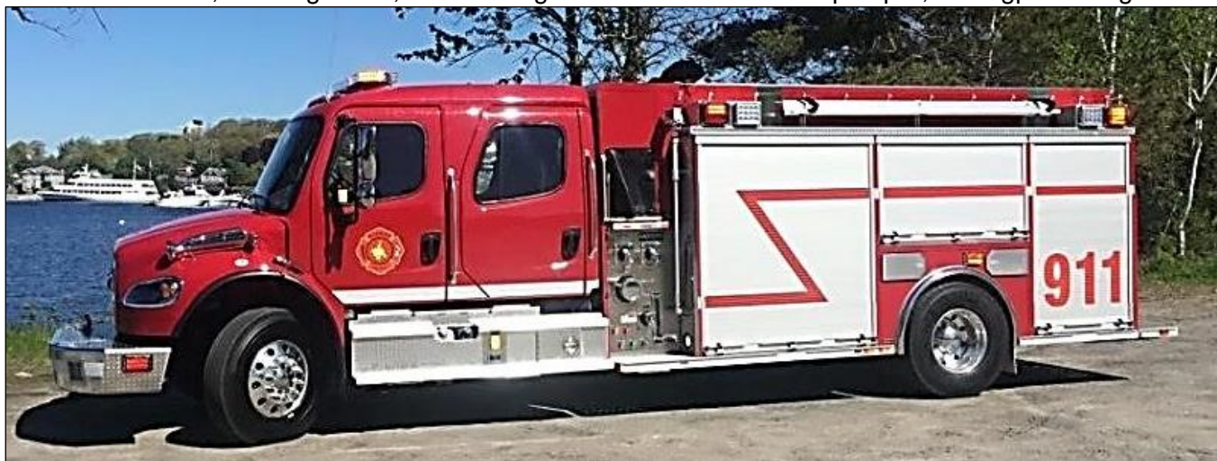
Wasauksing, ON FN 2019 Freightliner M2-106 / Metalfab HEAT pumper 1050igpm/1000gwt/30gft. (Metalfab Fire photos)
