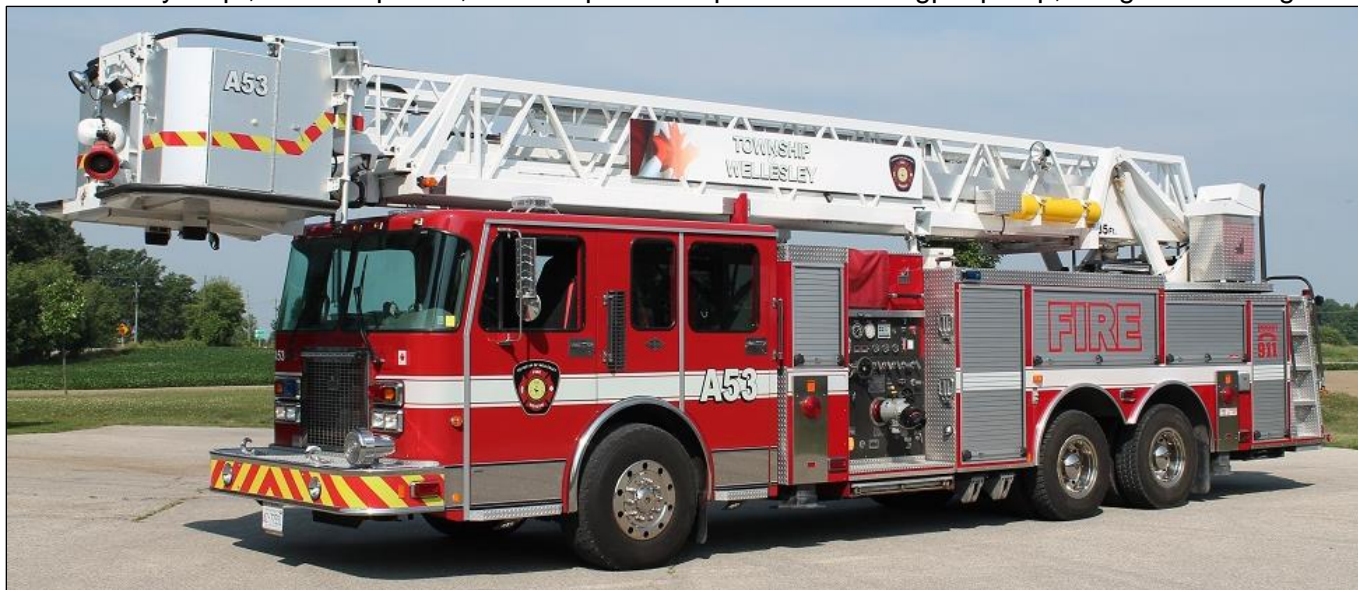
Wellesley Twp., ON Aerial 53 is now running this 1998 Spartan Gladiator/Smeal platform. Formerly with Tillsonburg, it has a 1750igpm pump, 250gwt and 85' tower. SN 894230 (Gary Dinkel photos)
