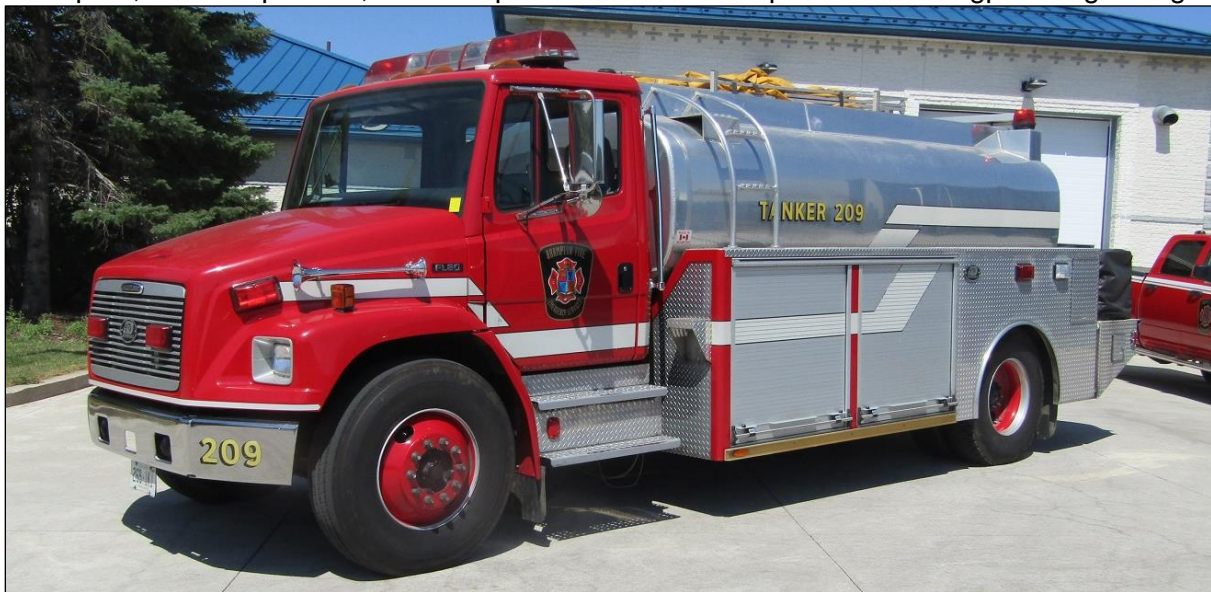
Brampton, ON Tanker 209, a 2001 Freightliner FL80/Dependable, 1050igpm and 2000gwt.
