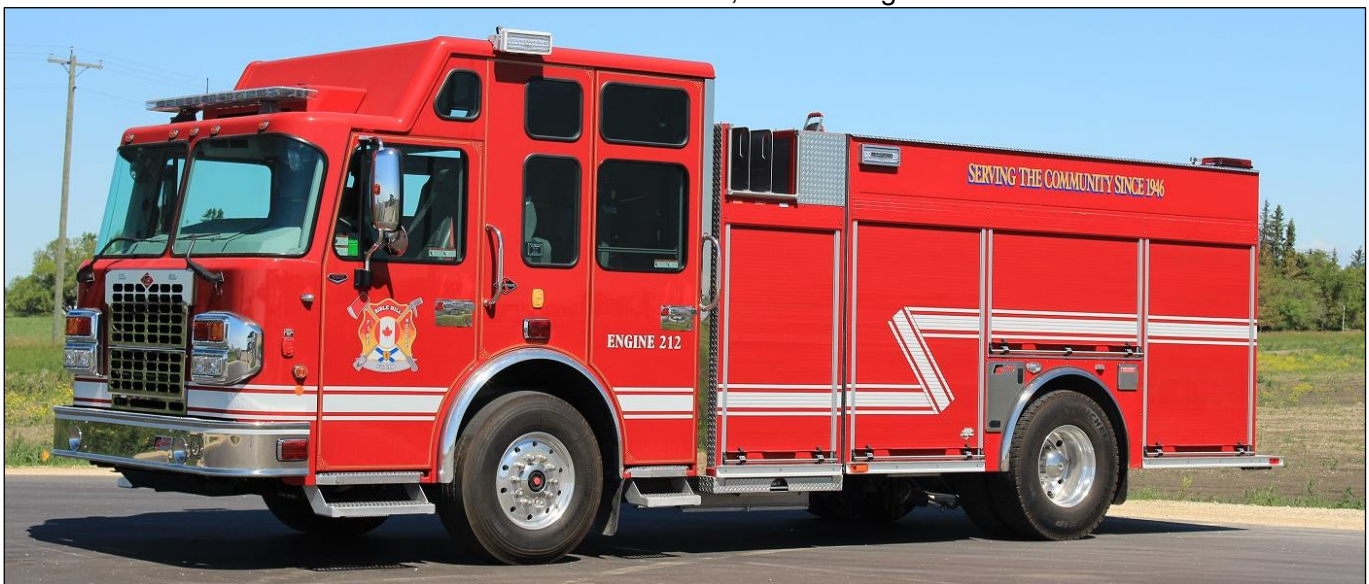
Bible Hill, NSPumper/Tanker 242, a 2019 Spartan Metro Star / Fort Garry 1050igpm/1000gwt. SN#J0003 (Dave Stewardson photos)
