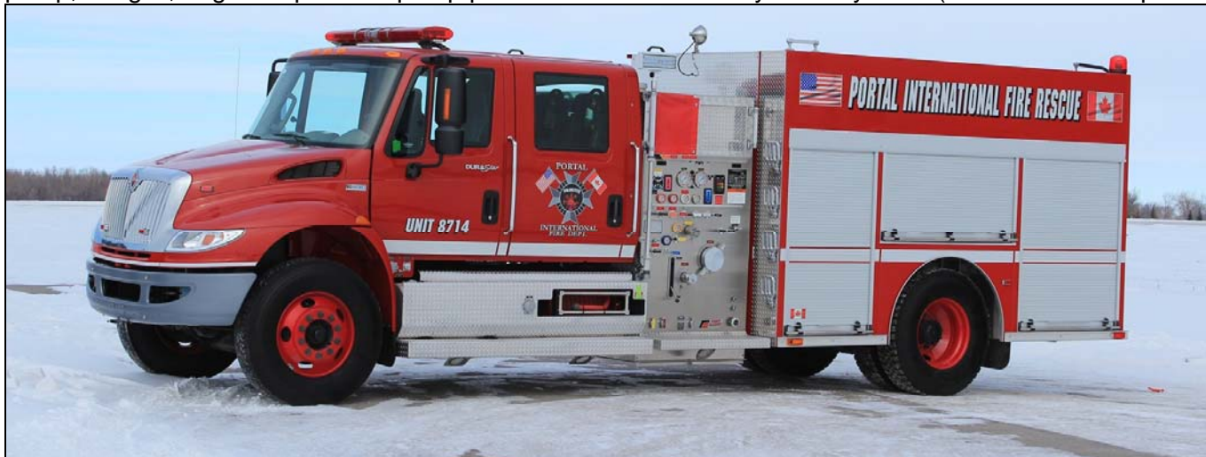
North Portal, SK received this 2012 IHC 4400/Fort Garry truck in the winter. Unit 8714 came with an 840igpm, 1000gwt and 25gft. (s/n #M377) (Dave Stewardson photo)
