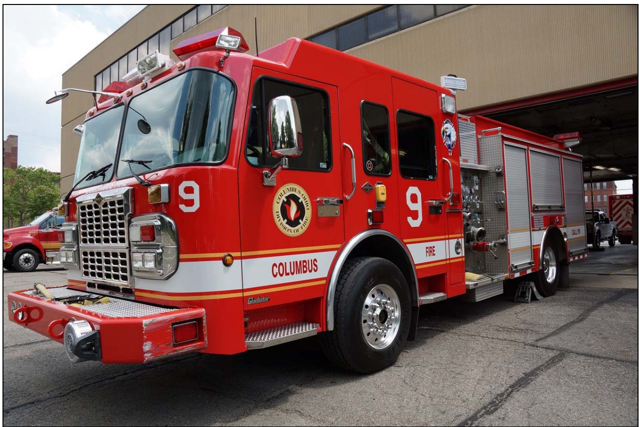
Columbus, OH Engine 9, a 2008 Spartan Gladiator/Ferrera rig, has a 1500gpm pump and 700gwt.
