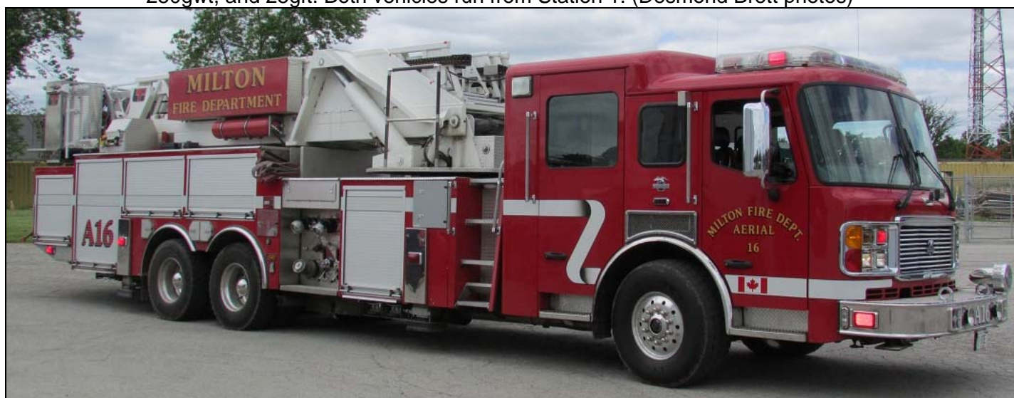
These were rolled out for shots, Support 10 is a 2013 Ford F550/DEV product equipped with a skid-mounted portable pump and 200gwt. Aerial 16 is a 2007 ALF Eagle with a 100' LTI tower, 1250igpm pump, 250gwt, and 25gft. Both vehicles run from Station 1. (Desmond Brett photos)
