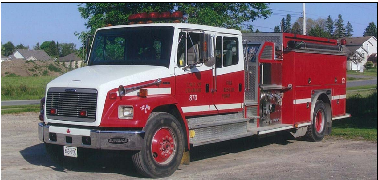
Three rigs from Northumberland County, specifically Cramahe Twp. Pumper 870 is stationed in Colborne, it's a 1999 Freightliner FL80/Superior job with a 1050igpm pump and 800gwt.
