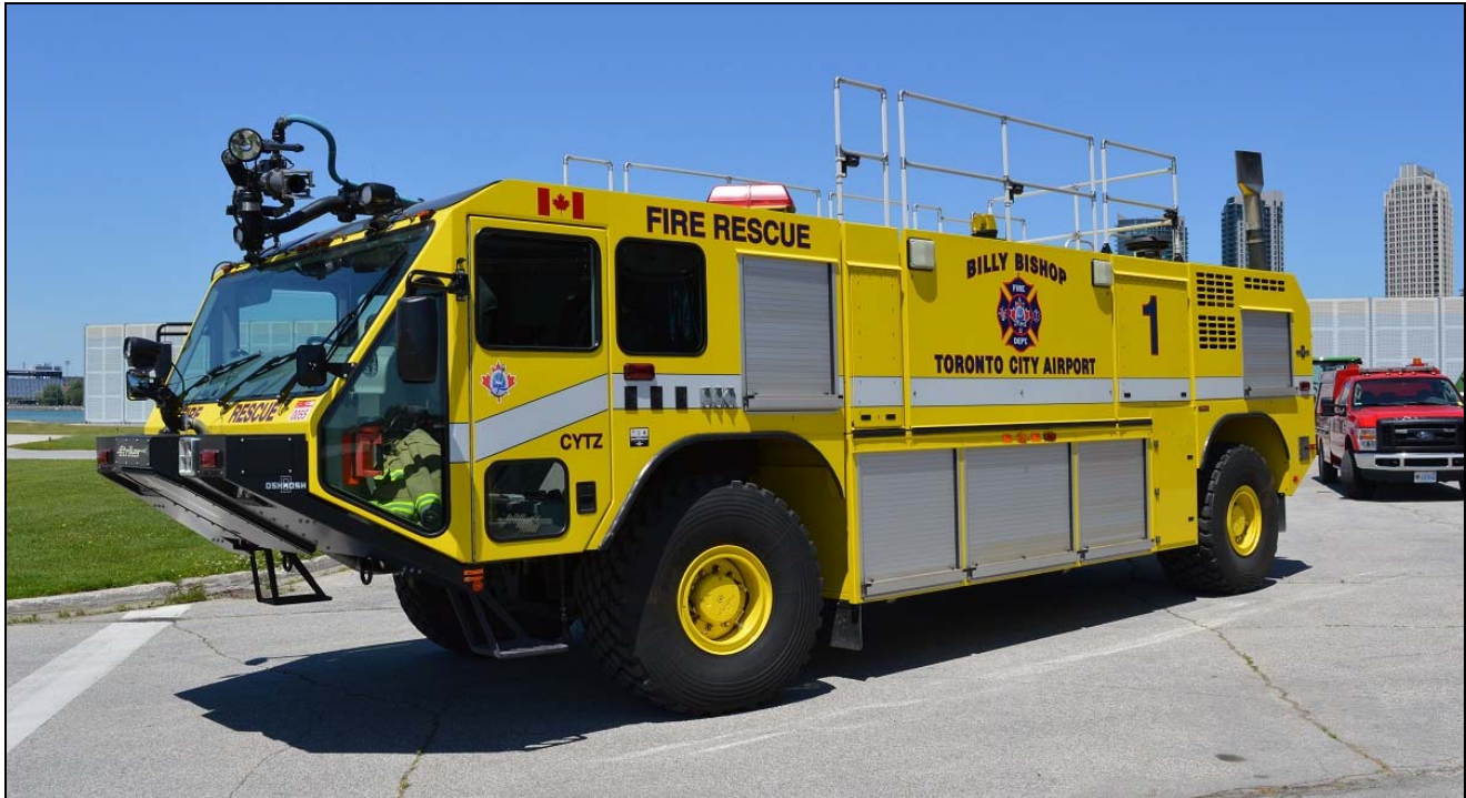
Red 1, a 2009 Oshkosh Striker with a 1950gpm pump, 1500gwt, 150gft and 500lbs dry chemical.
