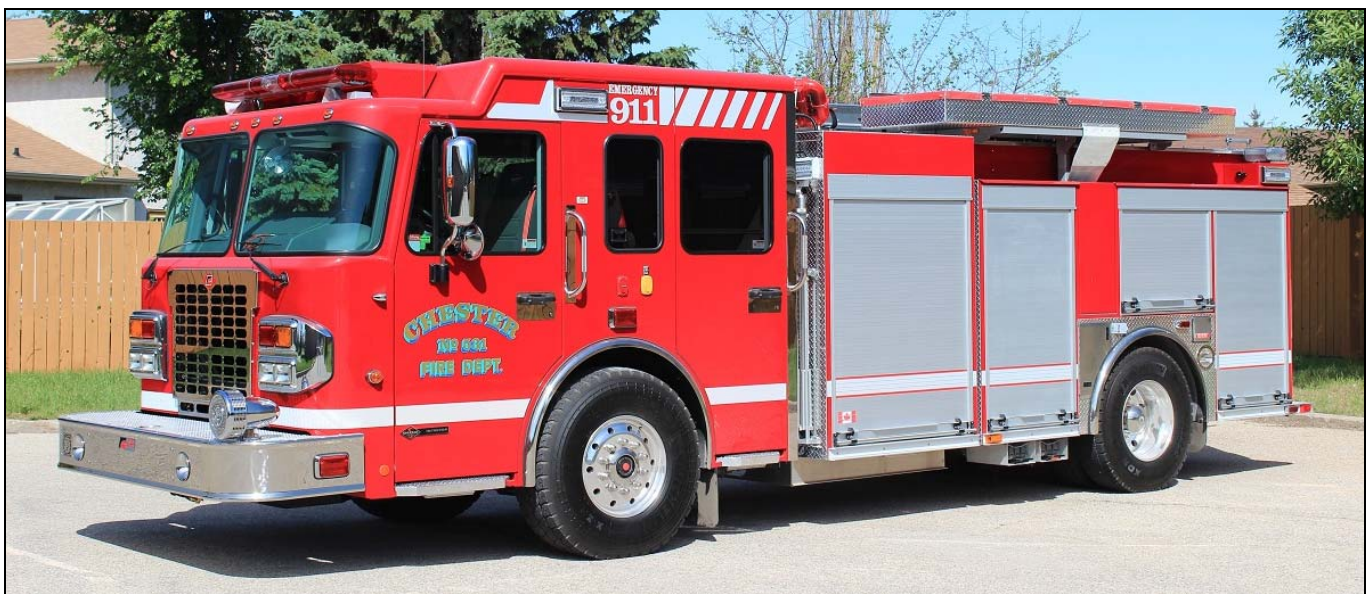
Chester, NS recently took delivery of this 2014 Fort Garry engine on a Spartan Metro Star chassis. Unit 531 has a 1050igpm pump, 800gwt and 50gft. SN M480
