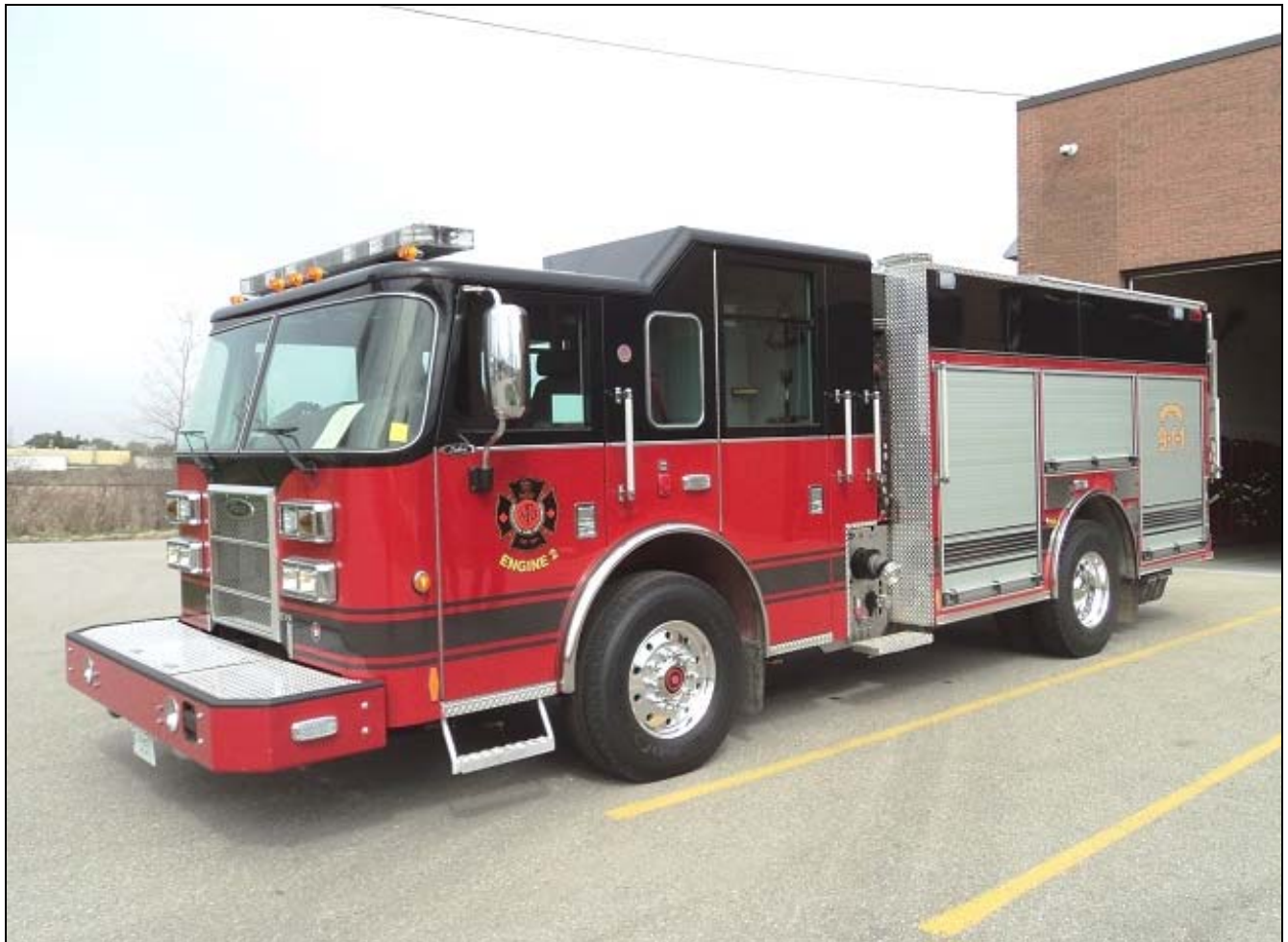
Late last year, Woodstock received this 2013 Pierce Saber pumper. Engine 2 has a 1500gpm pump and 10000wt. (Ken Buchanan photo)
