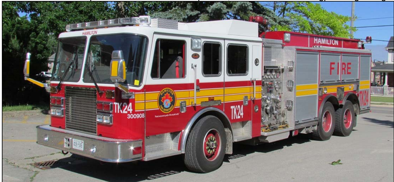
Tanker 24 is a 2008 KME Predator Severe Service rig with 1050igpm/1680gwt/25gft.
