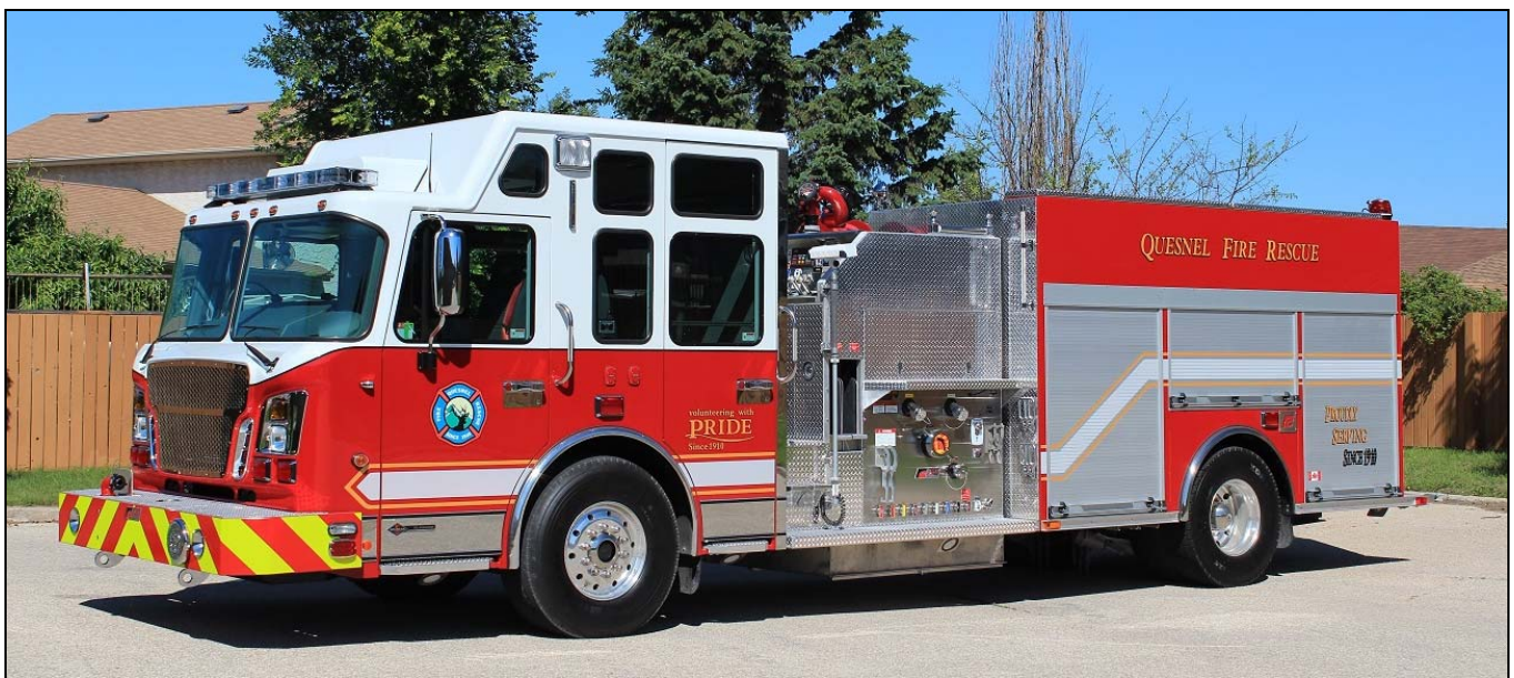
Quesnel, BC just put this 2014 Spartan Gladiator Evolution/Fort Garry pumper into service. It has a 1750 igpm Waterous pump, 1250gwt, 60gft and a CAFS. It carries Spartan No.78305 and Fort Garry s/n M527.
