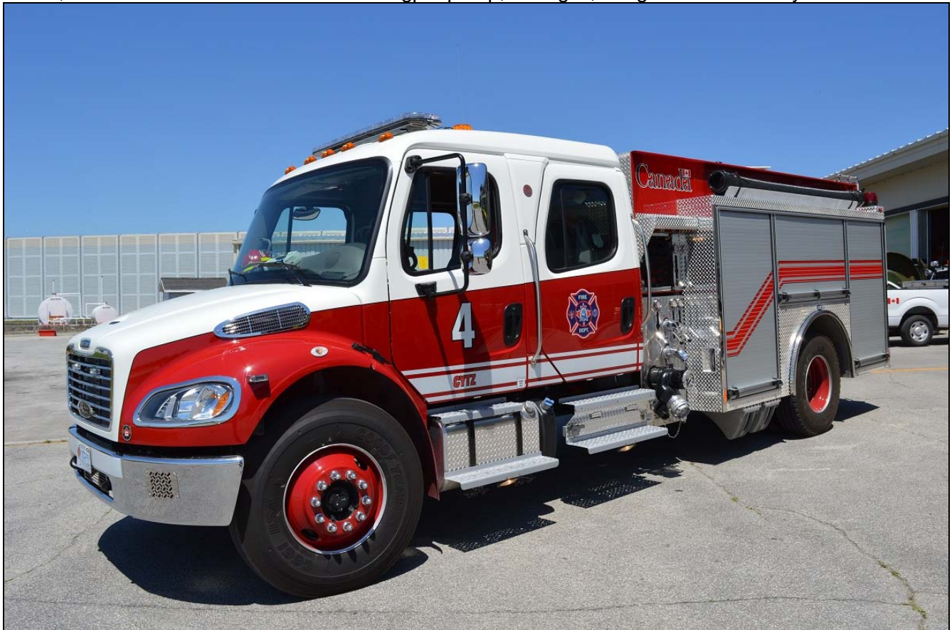
Red 4, the structural pumper, is a 2013 Freightliner M2 4x4/Pierce 1050igpm/800gwt, # FR8634
