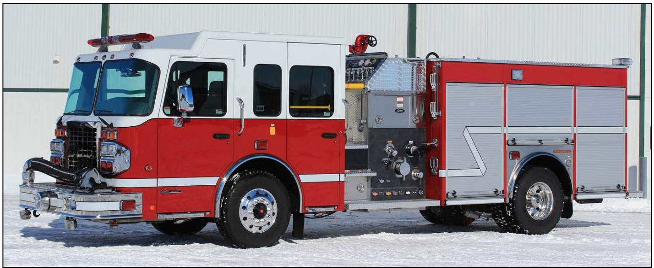
More unadorned rigs: Uniacke, NS got this 2014 Spartan Metro Star/Acres pumper in the winter. It has a 1050igpm pump, 800gwt and 20gft. s/n #140212112. Melville, SK runs this 2012 Freightliner M2/Grunthal tanker with a 625igpm pump and 2500gwt. (Dave Stewardson photos)
