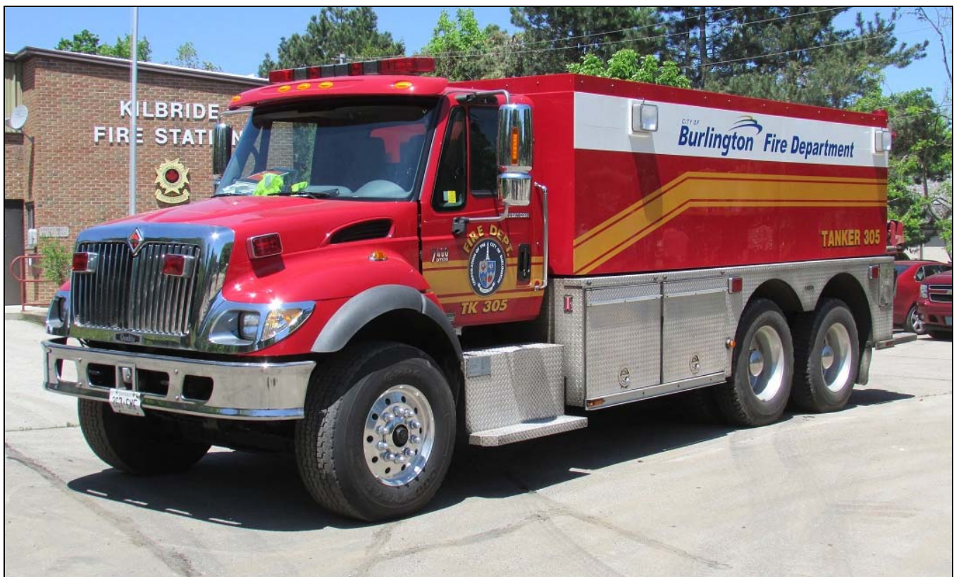
A couple from the Burlington tour, above is Tanker 305 in Kilbride. It's a 2002 IHC 7400/Crimson product with a 250gpm pump and 3000gwt. Below is Support Unit 301, a 1985 Hahn/Saulsbury heavy rescue with a 250gpm pump and 200gwt. Formerly of Packanack Lake, NJ, it runs from Station 1. (D. Brett)
