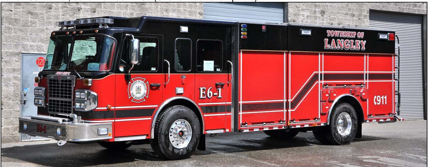
On its way to Langley Township, BC, Engine 6-1 was photographed at ProFire. It's a 2014 Spartan Metro Star/Smeal pumper with a 2250gpm pump and 1500gwt. (Terry Yip photo)
