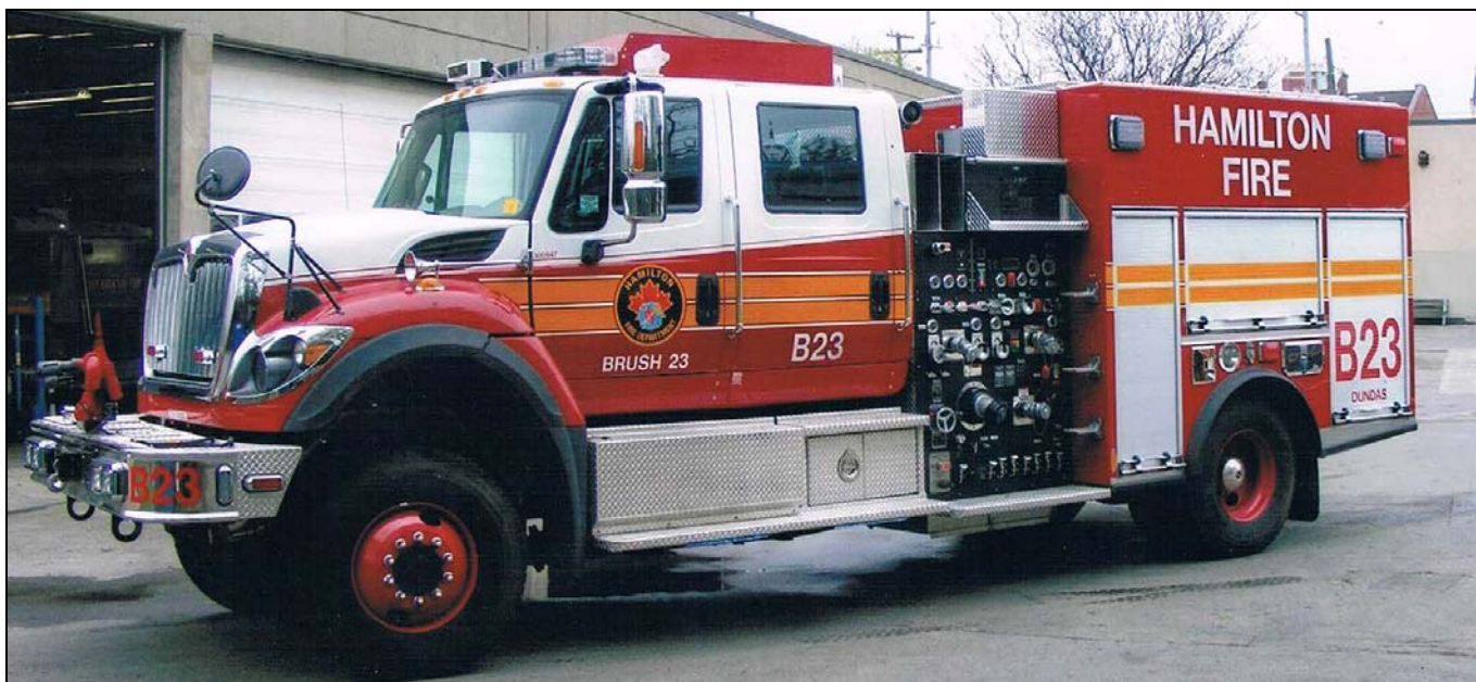
Hamilton's new KME brush unit, constructed on a 2014 IHC 4x4 chassis, is equipped with a 1050igpm pump, 750gwt and 20gft. (Doug Holmes photo)
