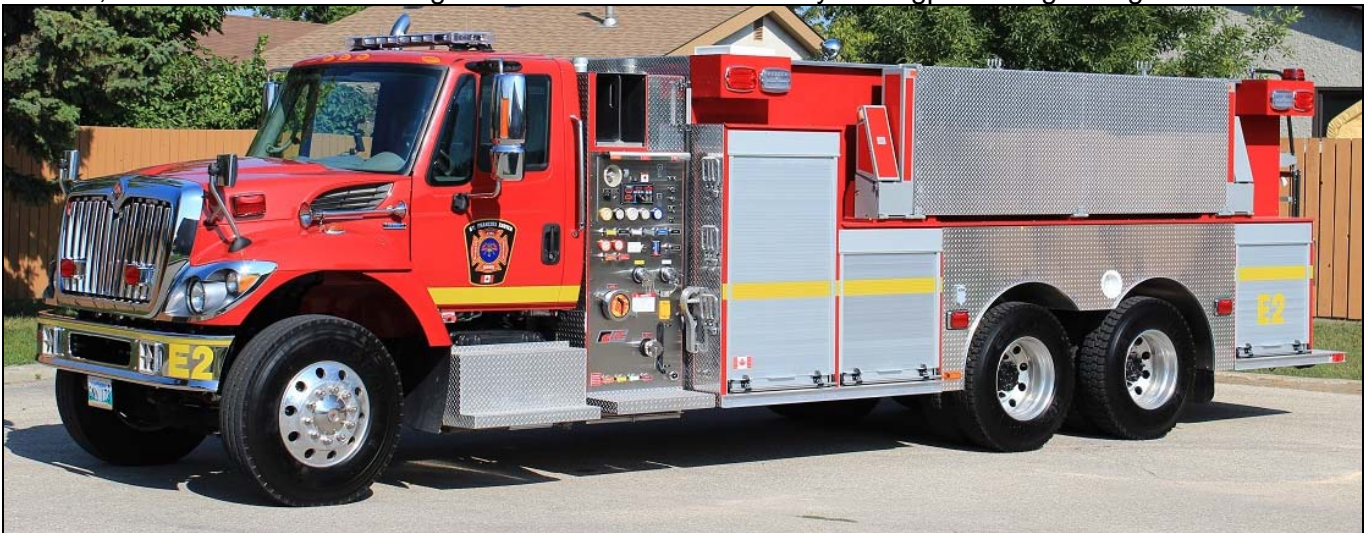
St. Francois-Xavier, MB acquired this long pumper-tanker last year. The 2013 IHC 7600/Fort Garry rig sports an 840igpm pump and 2500gwt. (M475)
