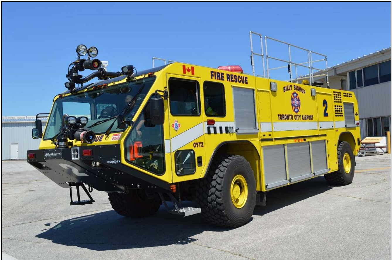
Red 2, a 2011 Oshkosh Striker with a 1950gpm pump, 1500gwt, 150gft and 500lbs dry chemical.
