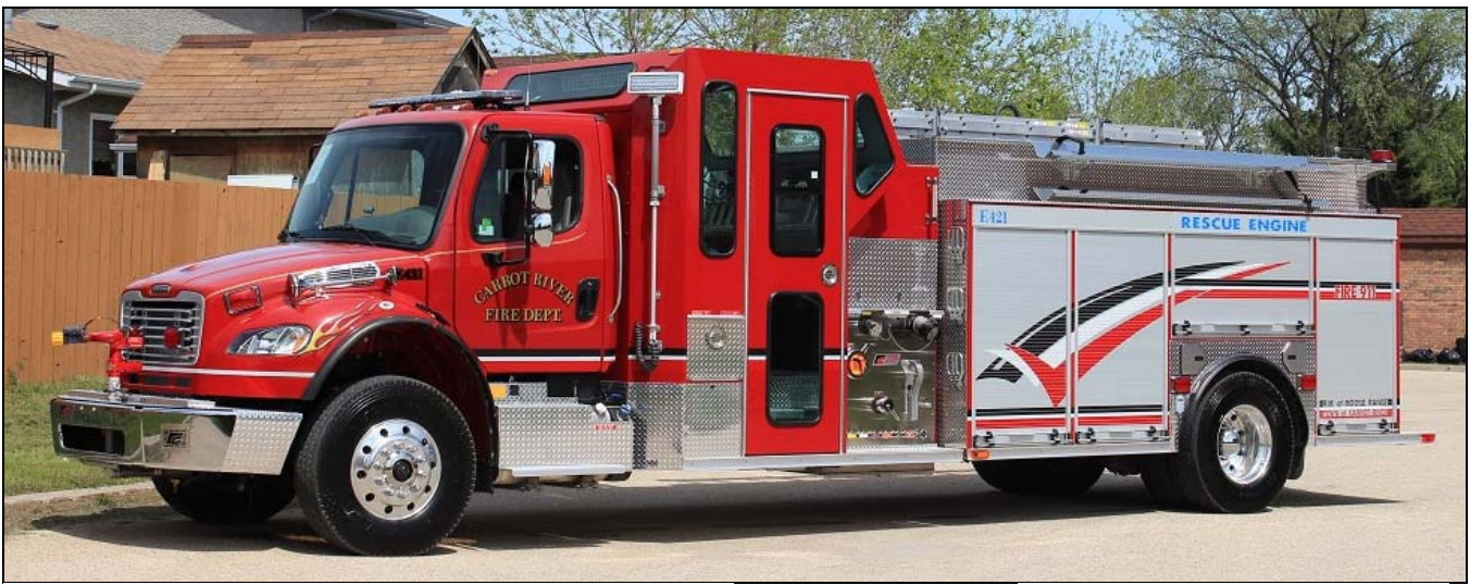
Carrot River, SK just received a new E.421, a 2014 Freightliner M2-106/Fort Garry rig with a 1050igpm pump, 1500gwt 25gft and a CAFS (s/n M530).
