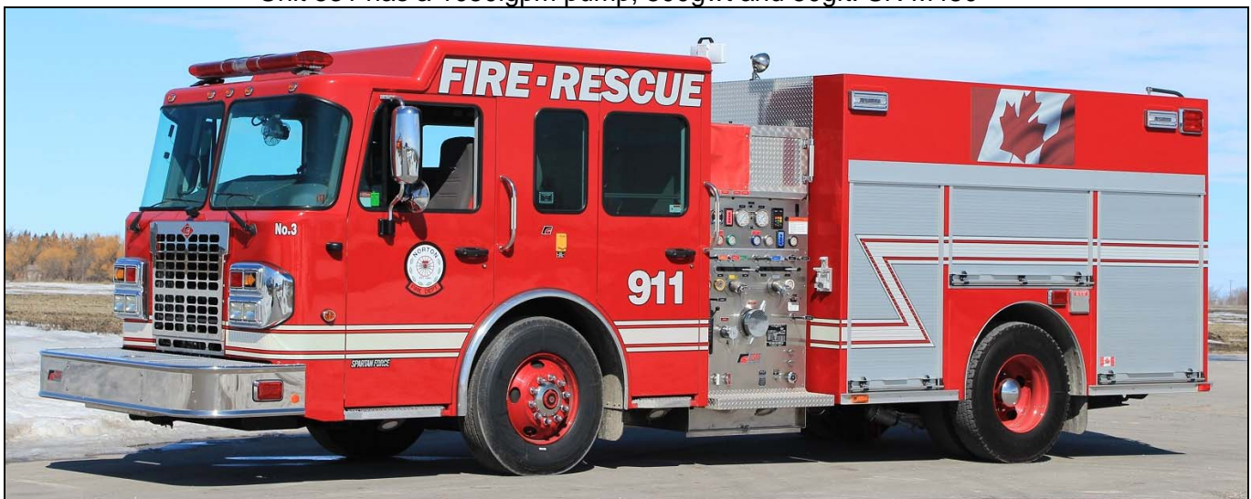
Norton, NB also bought from Fort Garry. Pumper No.3 was built as a stock unit on a 2011 Spartan Metro Star. It came with a 1050igpm Hale pump, an 800gwt and 25gft. SN M296. (Dave Stewardson photos)
