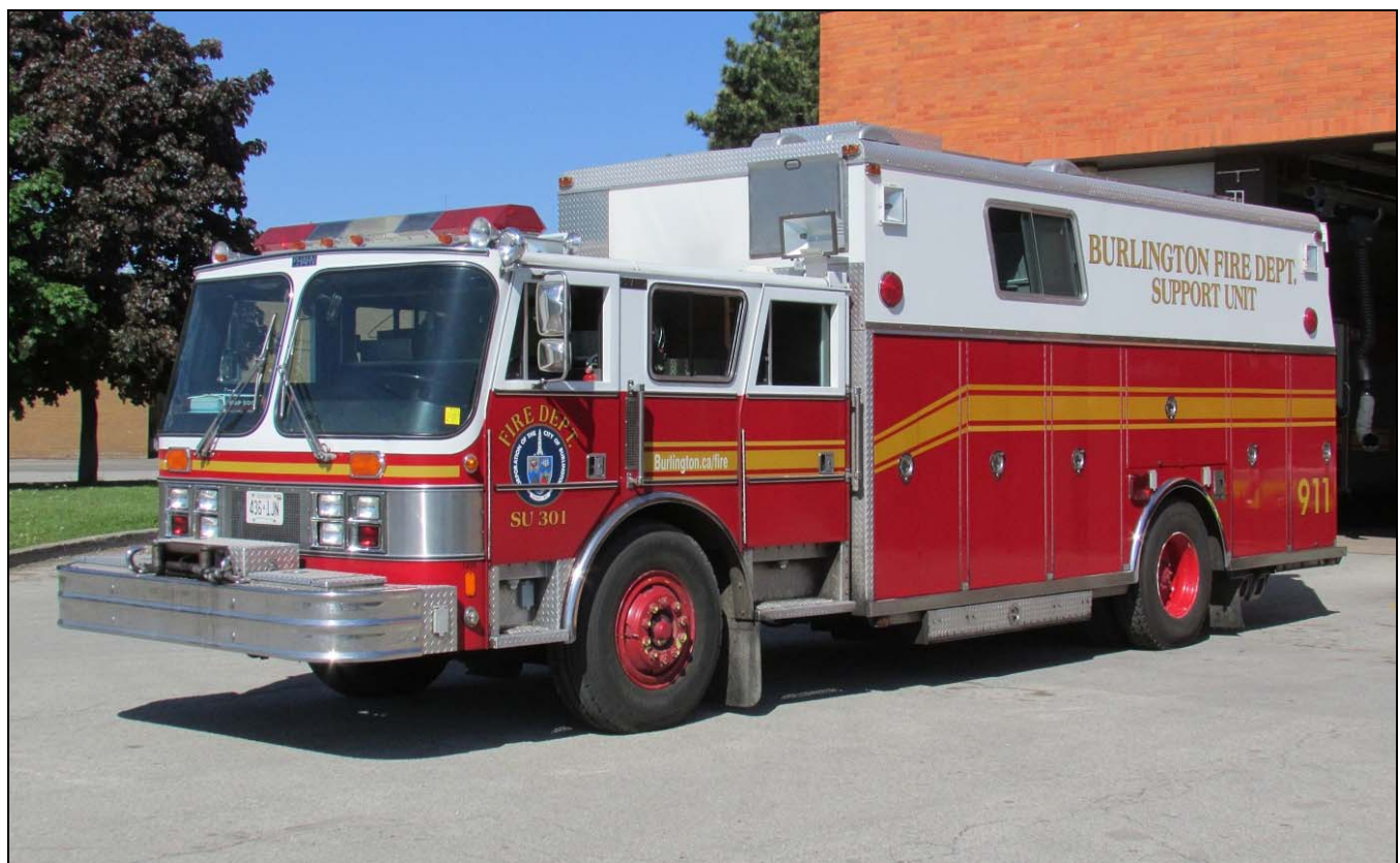
A couple from the Burlington tour, above is Tanker 305 in Kilbride. It's a 2002 IHC 7400/Crimson product with a 250gpm pump and 3000gwt. Below is Support Unit 301, a 1985 Hahn/Saulsbury heavy rescue with a 250gpm pump and 200gwt. Formerly of Packanack Lake, NJ, it runs from Station 1. (D. Brett)
