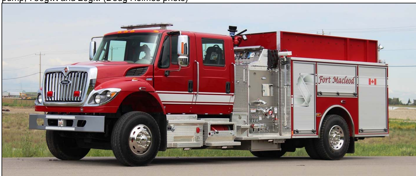
Fort Macleod, AB just received this replacement for Unit 1. It's a 2014 IHC 7400/Pierce unit with a 860igpm pump, 840gwt, 25gft & top-mount pump panel. It also has a Husky foam system. (John Bowerman photo)
