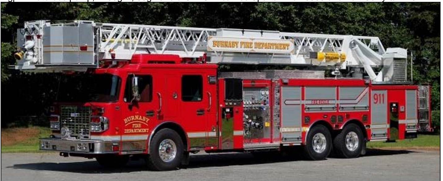
Burnaby's new tower, a 2014 Spartan Gladiator/Smeal rearmount with a 2250gpm Hale pump, 300gwt, and 100' tower, serial number 4207 (Shane Mackichan photo)
