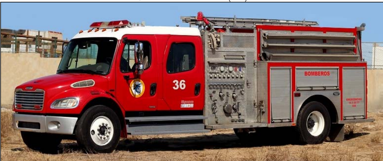
Cabo San Lucas M-36 on a 2008 Freightliner M2 chassis has a 5500L tank and 200L ft.
