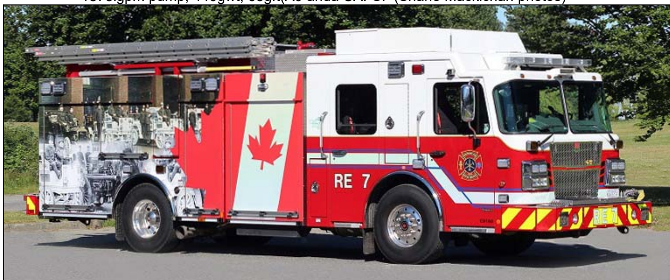
Vancouver, BC Rescue Engine 7 is a 2016 Spartan Gladiator Sirius / Smeal pumper with a 1875igpm pump, 440gwt, 63gft(A0 anda CAFS. (Shane Mackichan photos)
