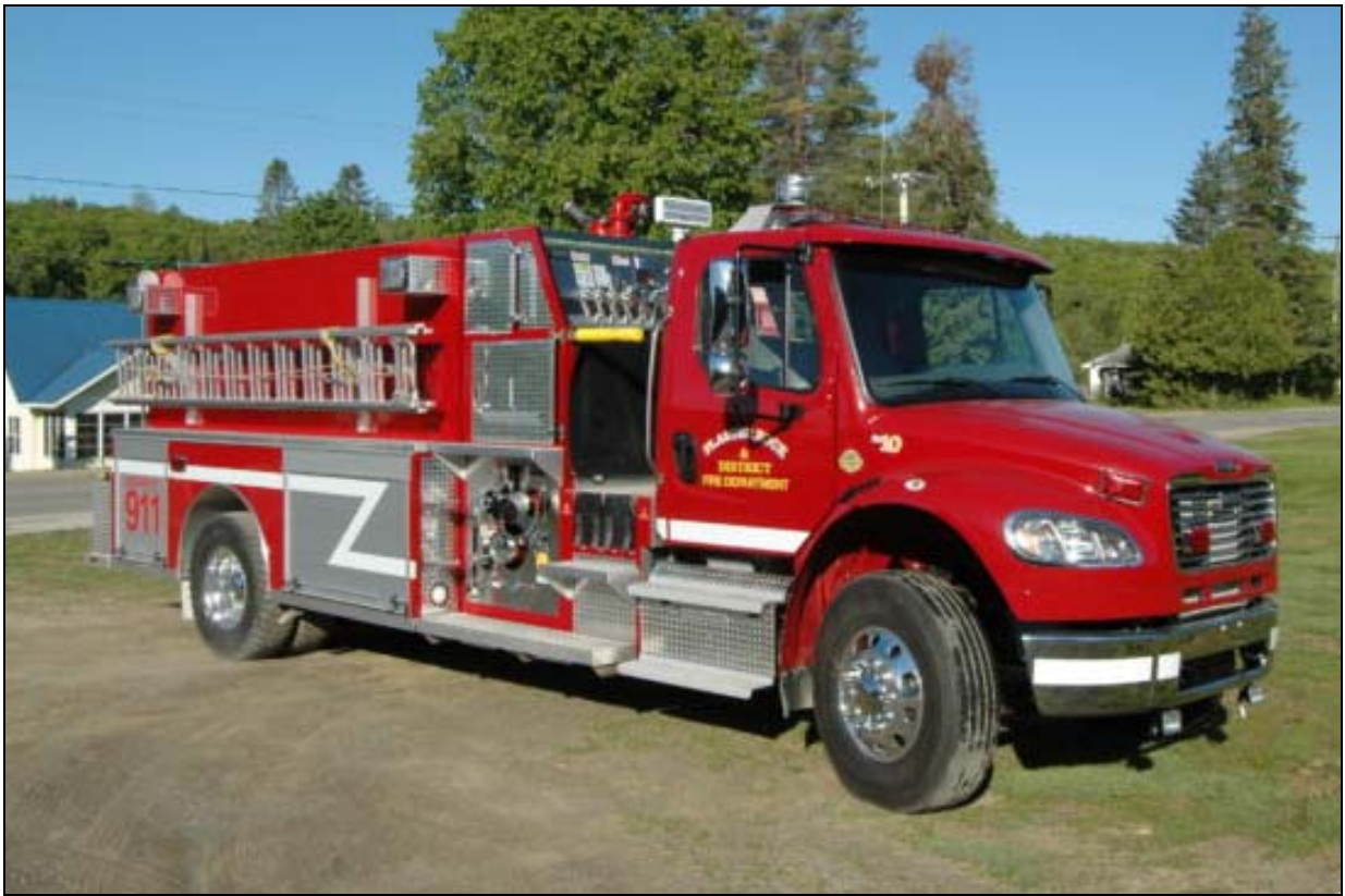
Plaster Rock, NB U.10 now runs with a 2017 Freightliner M2-106/Metalfab pumper/tanker, with a 1050igpm Hale pump, a 1200gwt and a 25gft.
