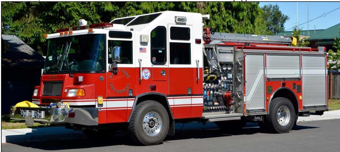
Kent Reserve Engine 2001 Pierce Quantum pumper with a 1510gpm pump, 500gwt and 30gft. (Terry Yip photos)
