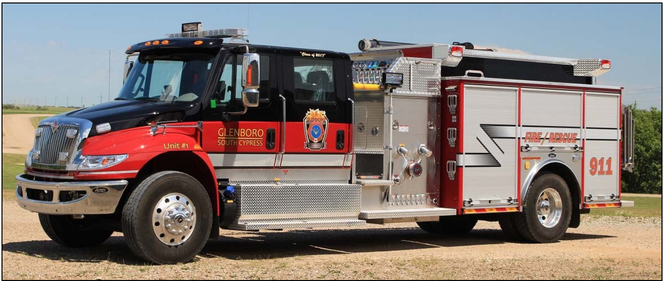
Glenboro-South Cypress, MB Unit 1 just got this 2017 IHC 7400/Acres pumper-tanker. It has a 1050igpm Waterous pump, a 1000gwt and a 25gft. (Dave Stewardson photo)
