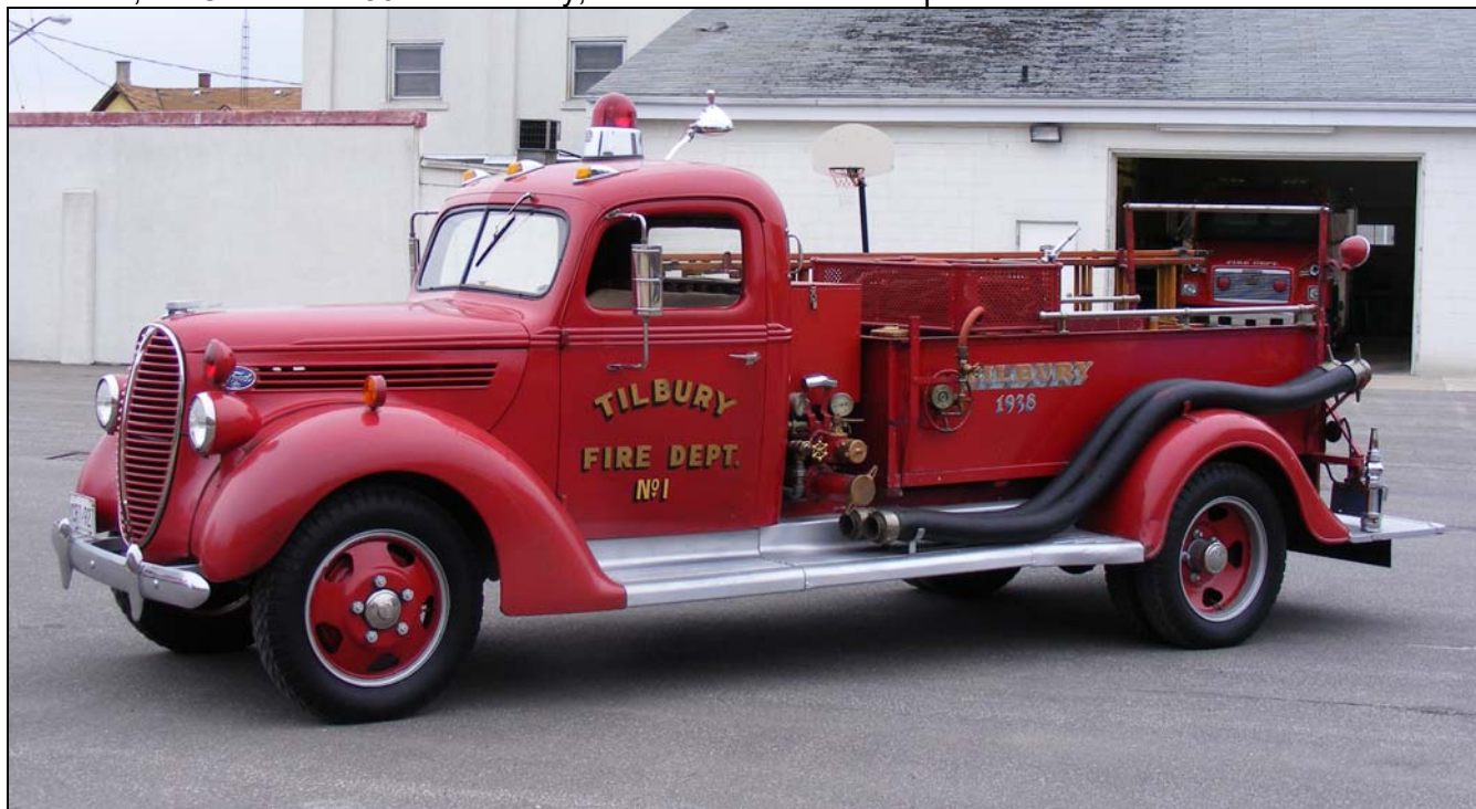
Two rigs now owned by Chatham-Kent: A 1938 Ford/Bickle Seagrave triple that served Tilbury for many years. It has a 300gpm pump and 200gwt. Wheatley's 1953 Chevrolet/Bickle Seagrave has a 500gpm pump and 200gwt. (Neil McCarten photos)
