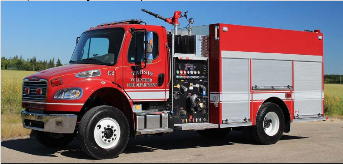
Tahsis, BC Engine 2 2017 Freightliner M2-106/Fort Garry 1050igpm(H)/300gwt/25gft s/n M806
