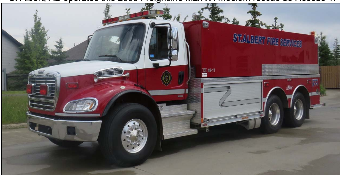
St Albert Tanker 1 is a 2007 Freightline M2/Rosenbauer rig, 625igpm/3000gwt.
