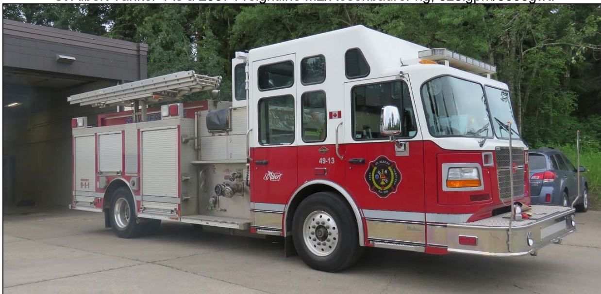
St Albert Pump 1 runs this 2008 Rosenbauer Commander pumper, it has a 1500gpm pump, with a 600gwt. (Rick Loiselle photos)
