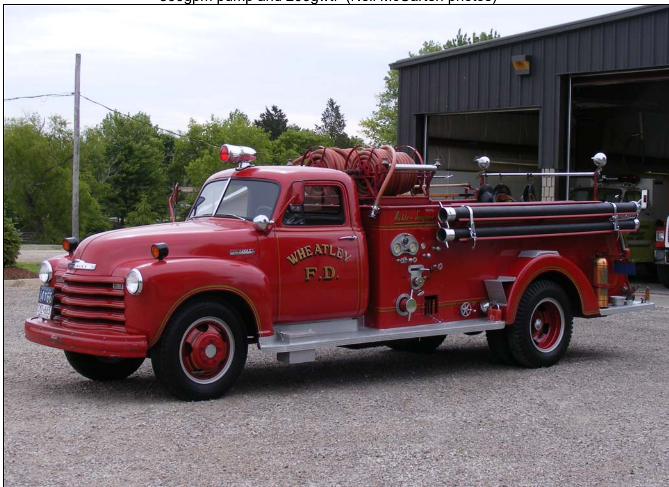
Two rigs now owned by Chatham-Kent: A 1938 Ford/Bickle Seagrave triple that served Tilbury for many years. It has a 300gpm pump and 200gwt. Wheatley's 1953 Chevrolet/Bickle Seagrave has a 500gpm pump and 200gwt. (Neil McCarten photos)
