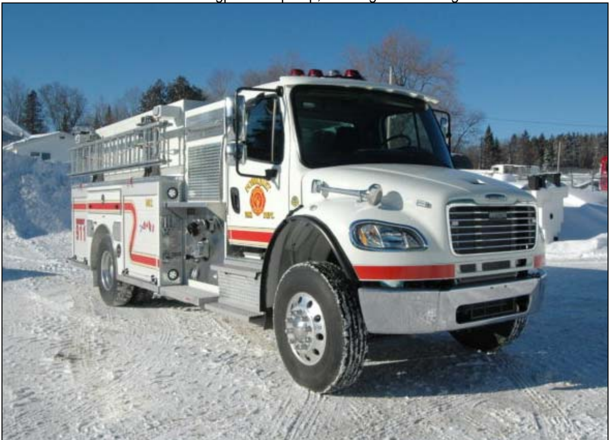
Pomquet, NS 2017 took delivery of this Freightliner M2-106/Metalfab rig last winter. It has a 1050igpm Hale pump, 1000gwt, 25gft and a FoamPro 2002 FS. (Metalfab Fire Trucks photos)
