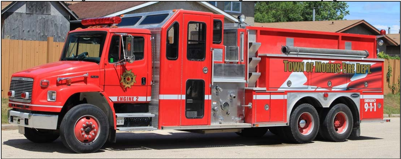
Morris, MB 2000 Freightliner/Superior 1050igpm Hale pump/2100gwt/35gft s/n #SE2051. It formerly served with the Opaskwayak Cree Nation. (Dave Sewardson photos)
