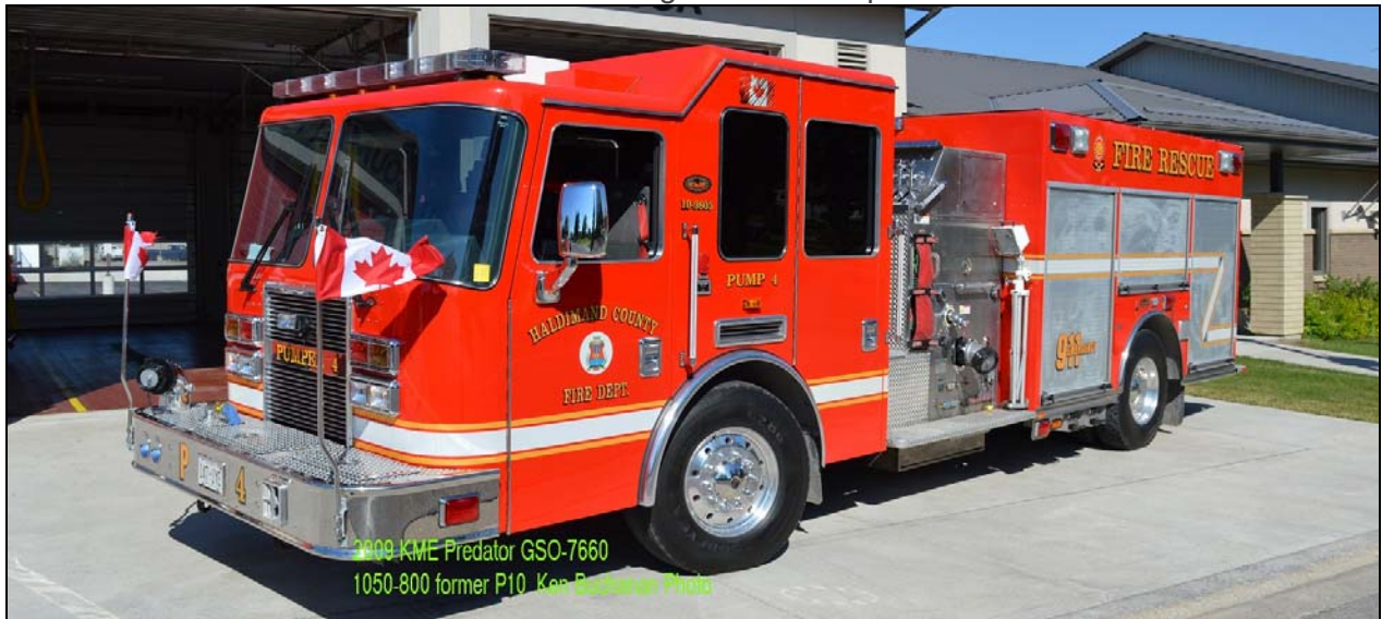
Haldimand Pump 4 is a 2009 KME Predator pump, 1050igpm, 800gwt, formerly P.10.
