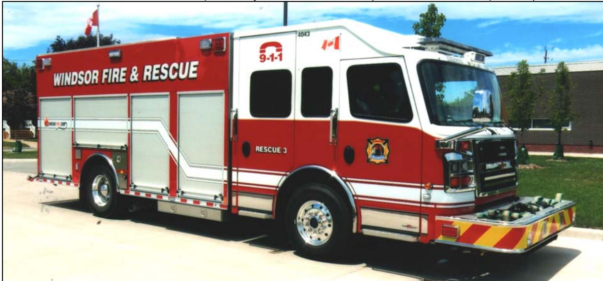
Rescue 3, Windsor's first Rescue Pumper, a 2017 Rosenbauer Commander, 1500gpm/500gwt/40gft (Walt McCall photo)
