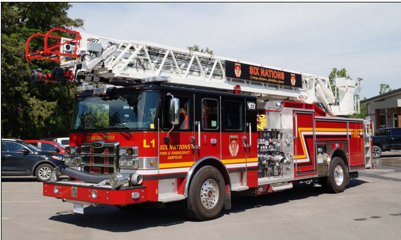
Aerial cover for Six Nations is provided by a 2016 Pierce Enforcer (1750/400) with a 107 foot Ascendant ladder.
