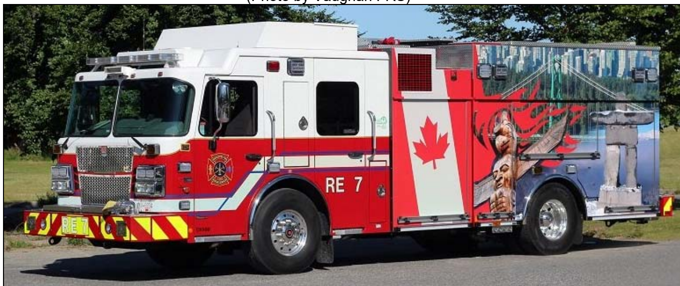
Vancouver, BC Rescue Engine 7 is a 2016 Spartan Gladiator Sirius / Smeal pumper with a 1875igpm pump, 440gwt, 63gft(A0 anda CAFS. (Shane Mackichan photos)
