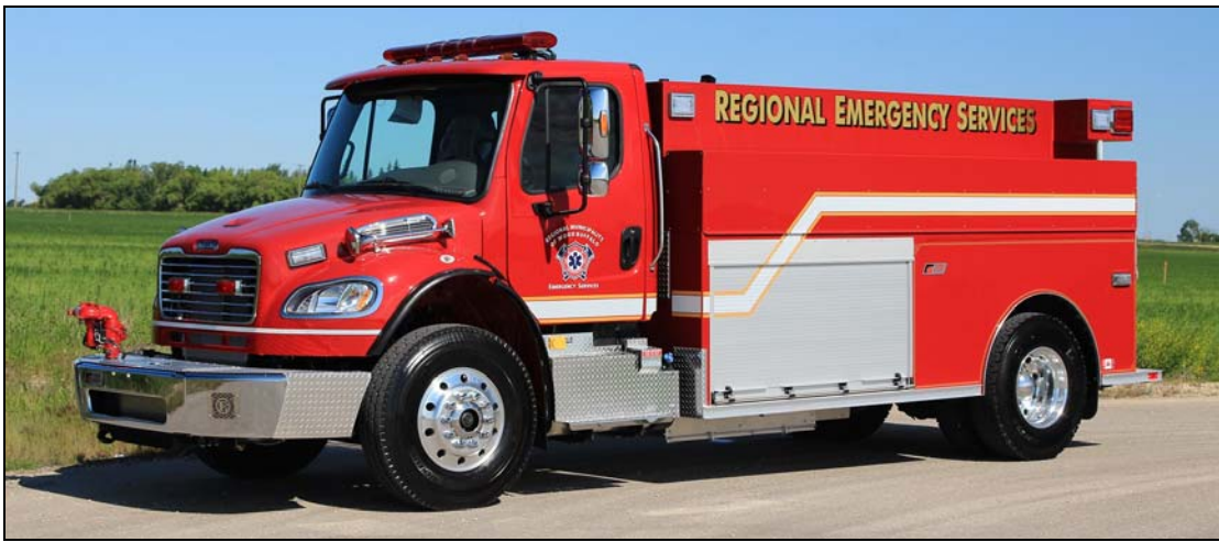
Conklin, AB 2017 recently took delivery of this Freightliner M2-106/Fort Garry tender. It has a 420igpm Darley pump and a 1700gwt. M804.
