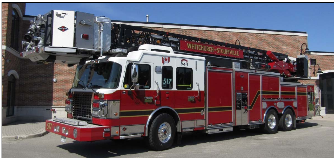
Also relatively new, Aerial 517, a 2016 Spartan Gladiator Classic/Spartan ERV/Dependable 100' platform with a 2000igpm pump and 250gwt. (All roster photos: Desmond Brett)
