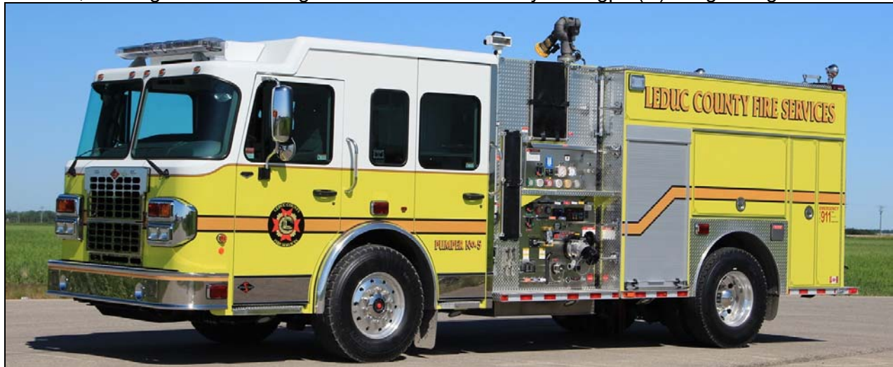
Leduc County, AB recently received a 2017 Spartan Metro Star/Fort Garry pumper with a 1050ipgm pump, 1000gwt, 10gft(A) and 25gft(B), running as Pump 5 s/n M798.
