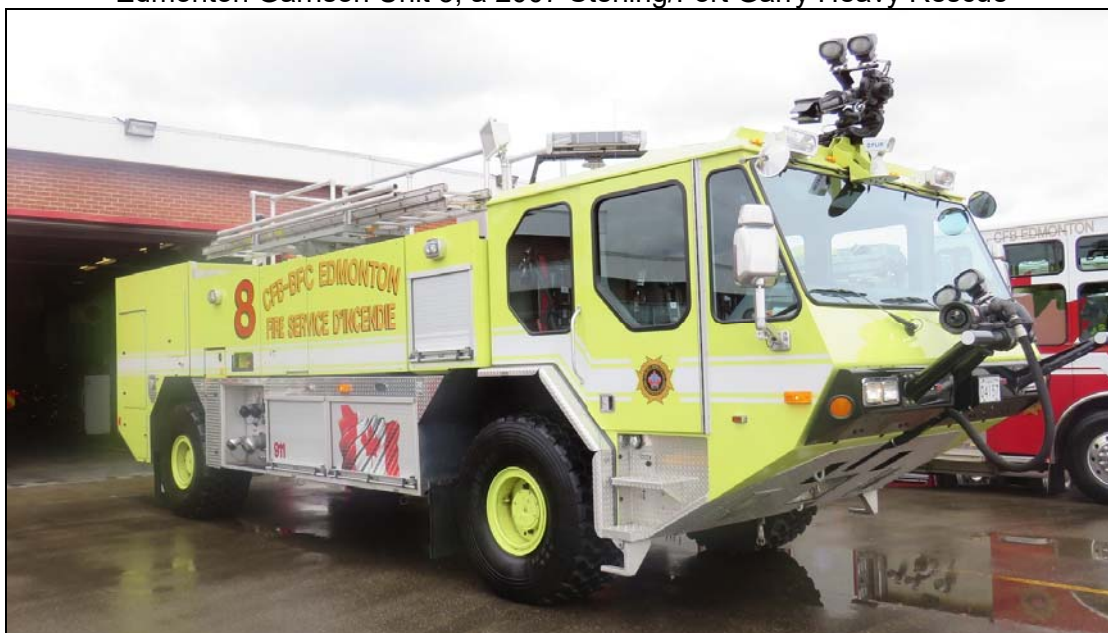
Edmonton Garrison Unit 8, a 2009 E-One Titan 4x4, 1250igpm/1250gwt/160gft.
