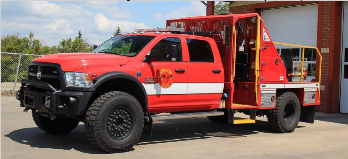
Moose Jaw, SK Unit 24 is a 2016 Dodge Ram 5500 4x4/Lite Industries/Rocky Mountain Phoenix brush unit with a 225igpm pump, 400gwt and 10gft. (Dave Stewardson photo)
