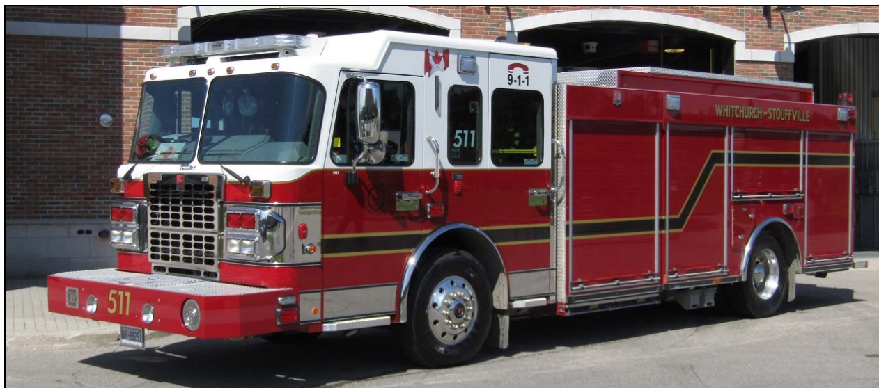
W-S Pump 511, a newly delivered 2017 Spartan/Smeal pumper, 1250igpm/750gwt/20gft V#CO81550
