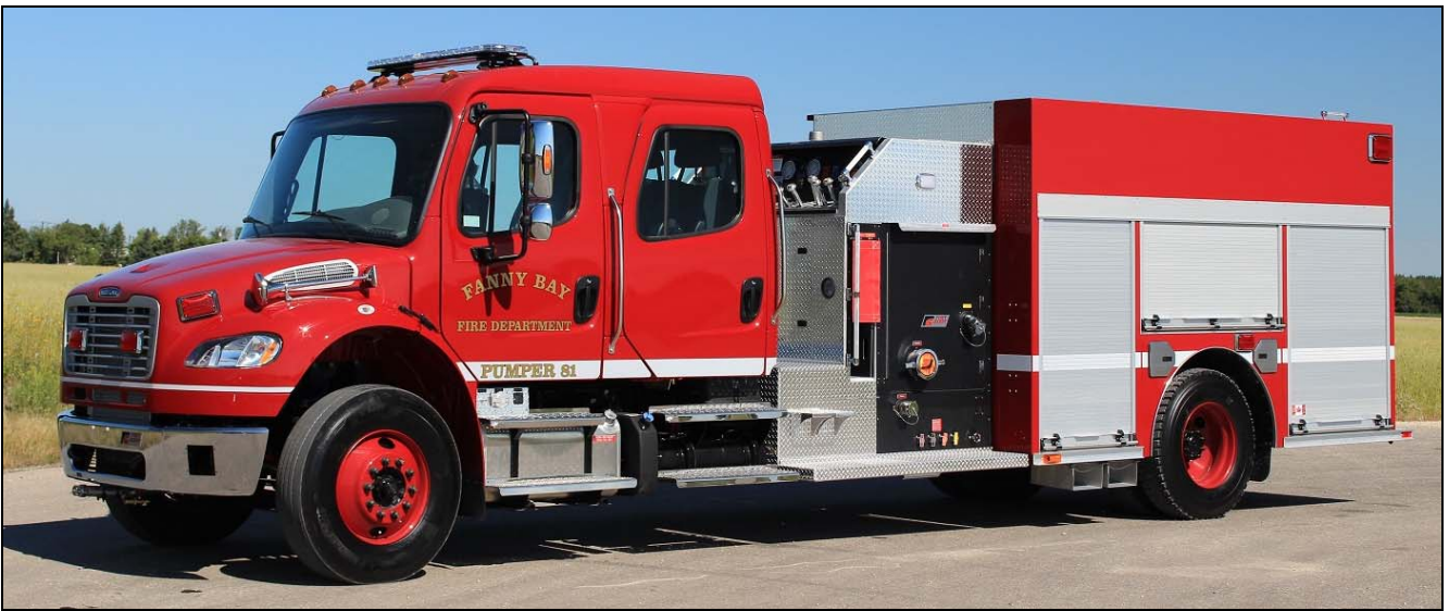
Fanny Bay, BC just received a 2017 Freightliner M2-106/Fort Garry pumper with a 1050igpm Hale pump, 1000gwt and 25gft. s/n M810. (Dave Stewardson photo)
