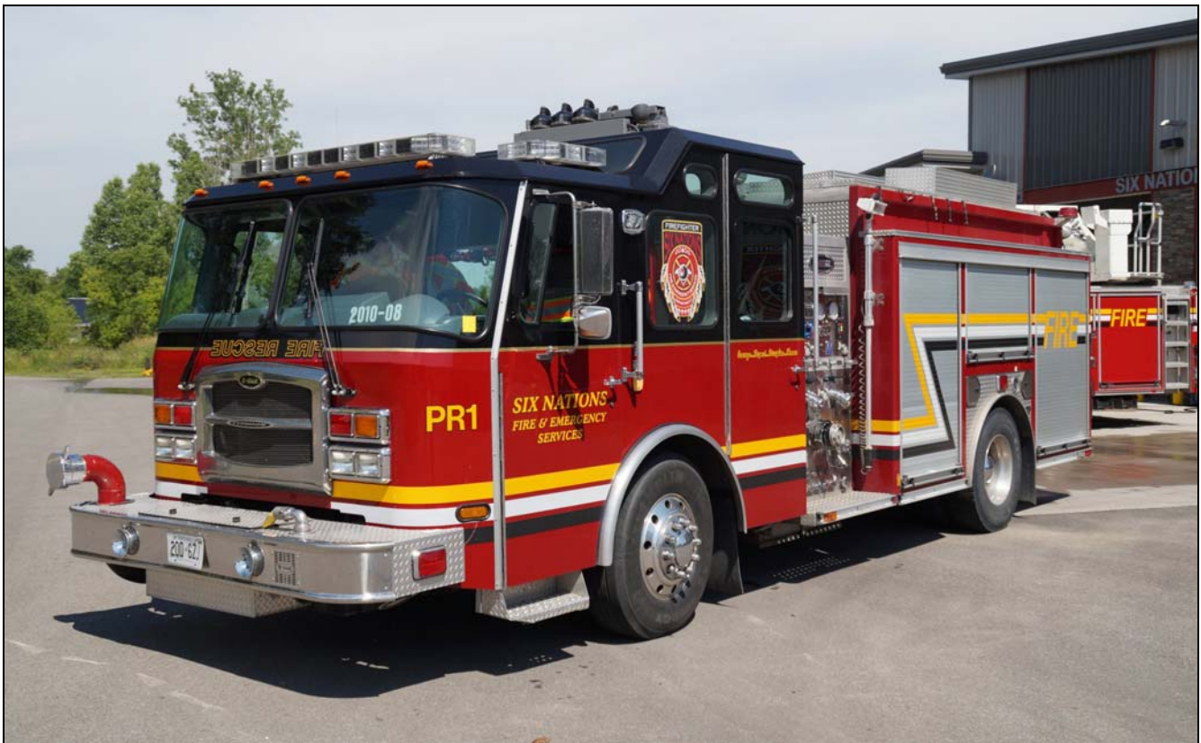
So to the closing photos, the last few taken on a trip out with Ken. 17 Veterans Lane, Oshweken is the home of the main station of the Six Nations Fire & Emergency Services. PR1 is a 2010 Emergency One Typhoon (1250/800) with a fantastic black over red livery.
