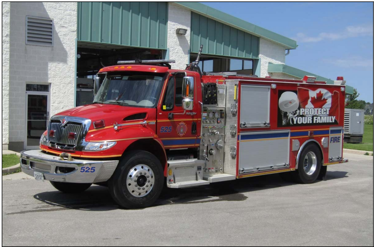
From Whitchurch-Stouffville, Tanker 525 is a 2011 Freightliner FL80/Asphodel product with an 840igpm pump and a 1500gwt runs from Ballantrae. V# CTHA0119.
