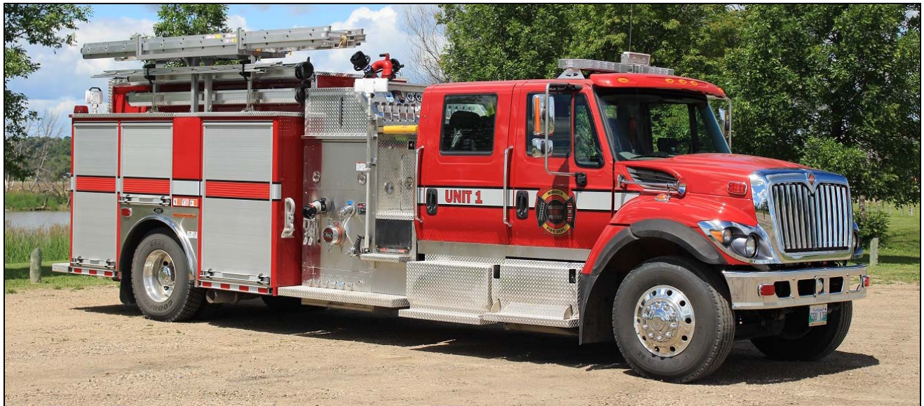
Another recent buy, Miniota, MB Unit 1 is a 2017 IHC 7400/Acres pumper-tanker, equipped with a 1050igpm Waterous pump, 1000gwt and a 25gft. s/n170324151.(Dave Stewardson photos)
