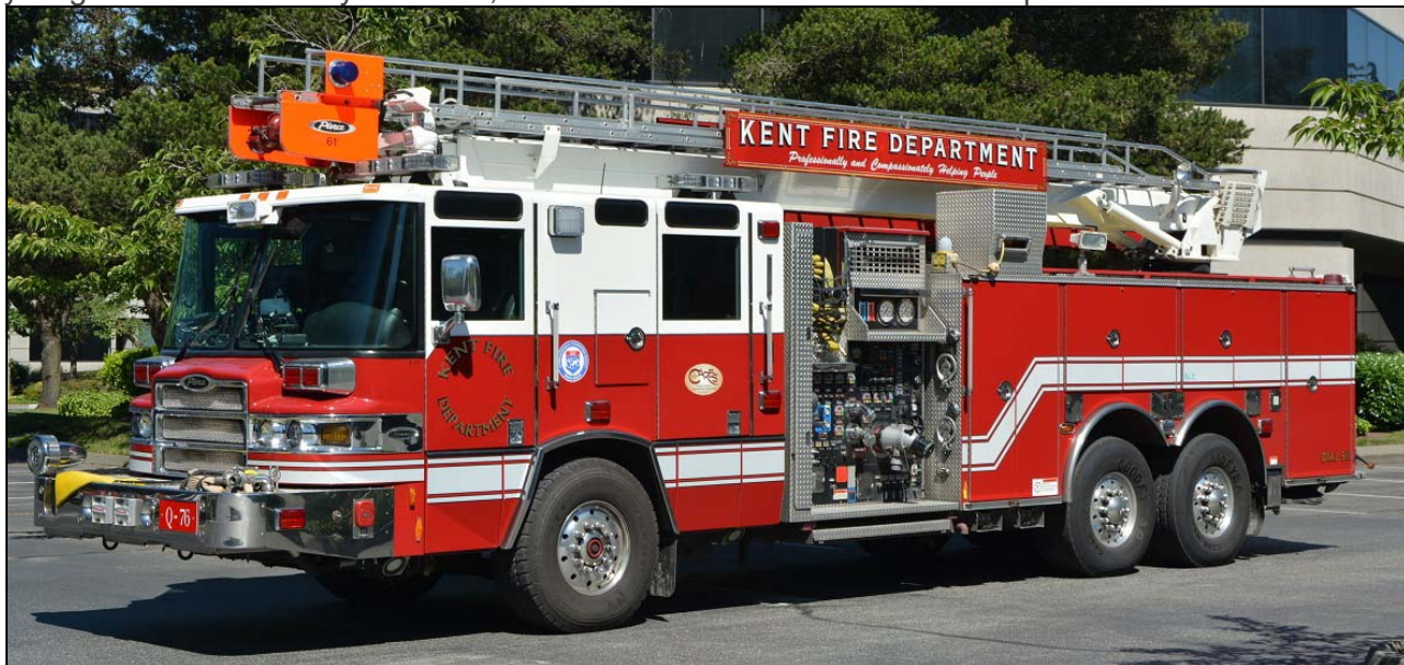
Kent, WA Q-76 2010 Pierce Quantum 1500/800/50/61' and equipped with AllSteer
