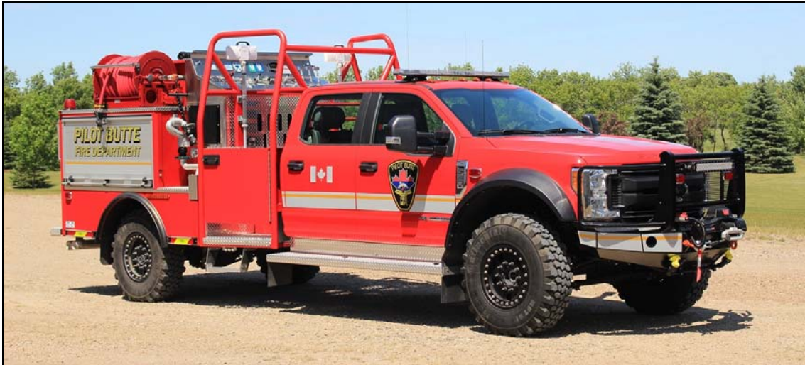
Pilot Butte, SK received this 2017 Ford F550 4x4/Acres brush truck in June. It has a 230igpm Waterax pump, a 400gwt and a 20gft.
