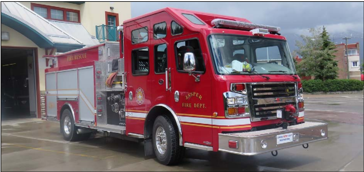
New last year to Jasper, AB is Engine 1, a 2016 Rosenbauer Commander 1500/1500.
