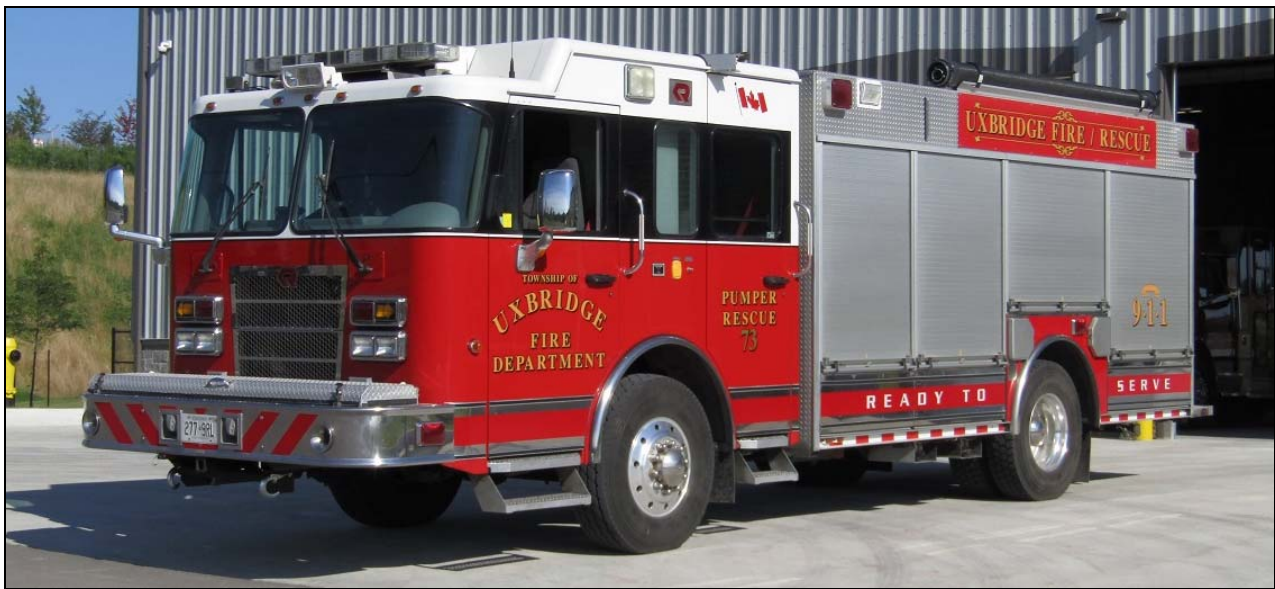
Spare 73 2005 Spartan Advantage 4x4 / Rosenbauer 1500/500/30F
