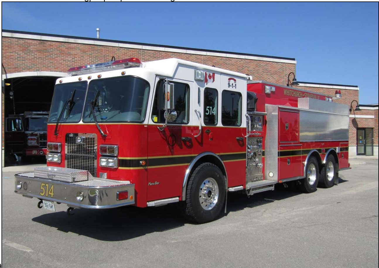
And Tanker 514, a 2008 Spartan Metro Star/Seagrave 1050igpm pump, 2200gwt and a 25gft is assigned to Stouffville. S/N 3164 (Desmond Brett photos)
