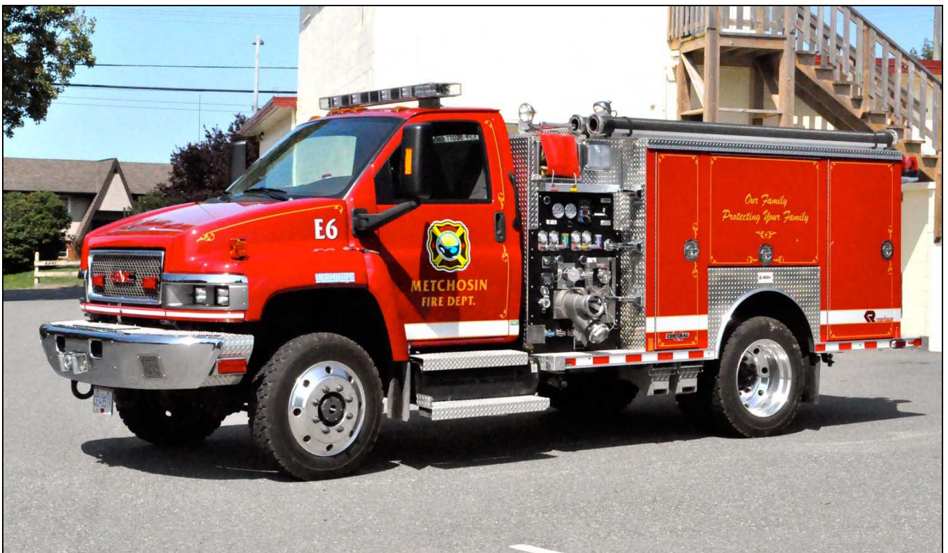
Metchosin, BC Engine 6, a 2010 GMC 4x4/Rosenbauer 420igpm/234gwt pumper. (Terry Yip photos)
