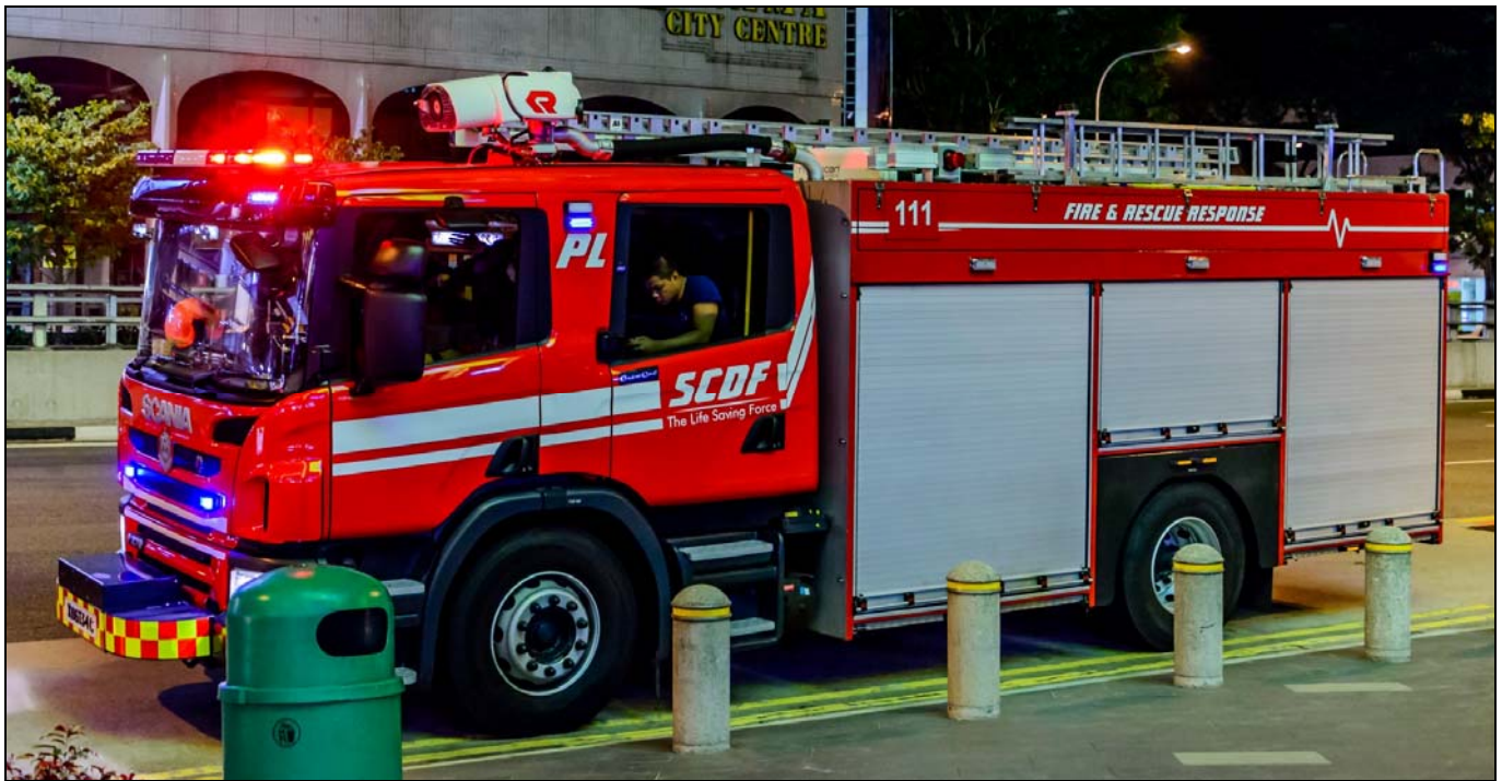
Just delivered in Singapore, one of the new rear-mounted Rosenbauer pumps, built on a 2013 Scania chassis with 500 gwt, 250gft and CAFS.
