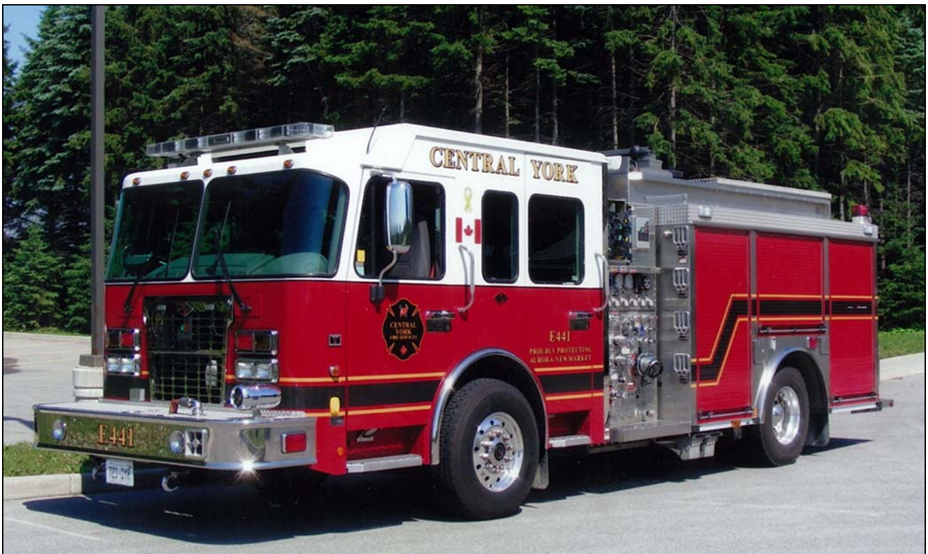
Central York Engine 441 is a 2010 Spartan Gladiator/Smeal pumper-tanker with a 1050igpm pump and 1100gwt. It runs from Station 44 in Aurora.
