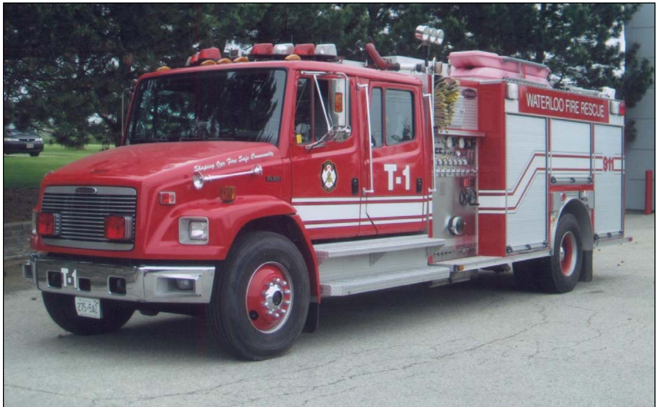
Waterloo Tanker 1, a 1996 Freightliner FL80/Superior pumper-tanker with 1050igpm pump, 1000gwt and 20gft. Additional Waterloo photos appeared in the TA, Volume 41, No.6. (Larry Ward photo)
