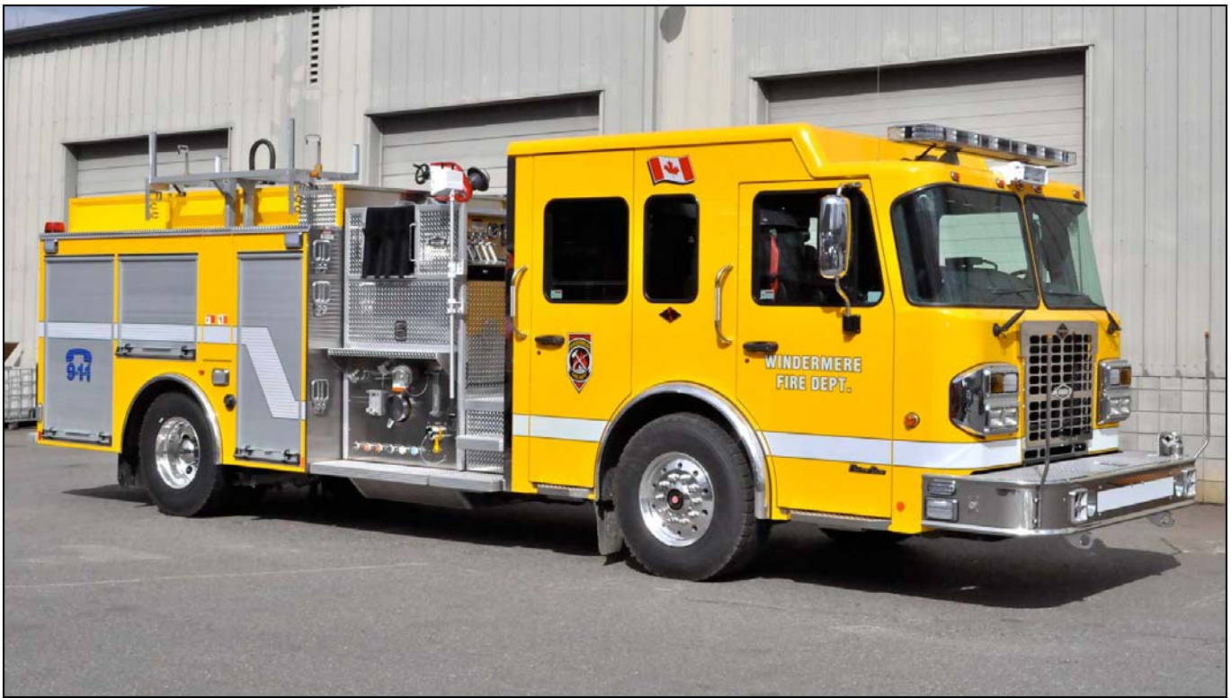
About to leave for Windermere, BC, this 2013 Spartan MetroStar/Hub pumper runs with a 1750igpm pump, 761gft and 40gft, Class A. It's painted canary yellow and has a top-mount pump panel.
