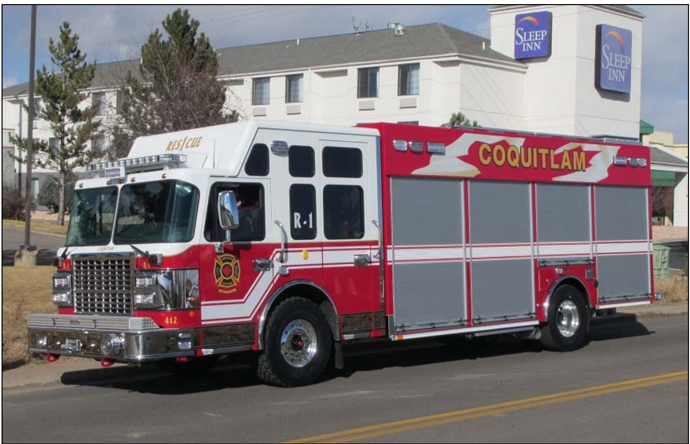
Two new rigs just delivered to Coquitlam, BC on Spartan chassis. Rescue 1 was built by SVI and Ladder 1 is a Smeal quint with a 125' aerial. The pictures were provided to us by Scott MacKenzie, Assistant Chief of the CFRS, via Terry Yip.
