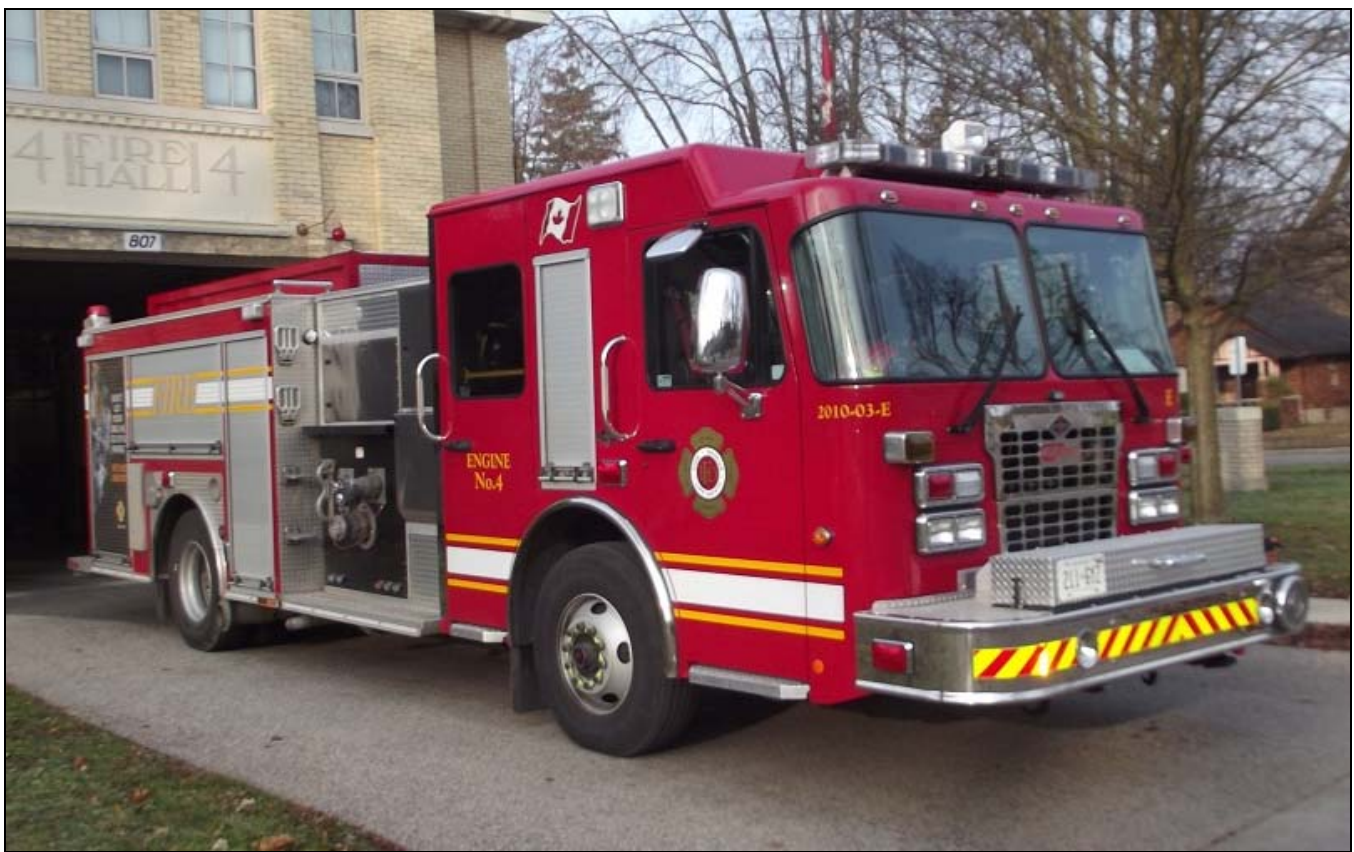
Two more of London's Spartan/Carl Thibault pumpers, from two different angles. Top is the oldest, Engine 4's 2010 model. Built on a Metro Star chassis, it has a 1250igpm pump and 500gtw. Engine 10, is on a 2012 Metro Star chassis and has a 1251igpm pump and 761gtw. (Rick Loiselle photos)
