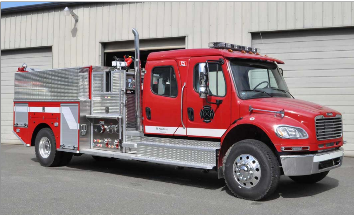
Potash Corp. in Rocanville, SK is just about to receive this Freightliner M2/Hub pumper equipped with an 840igpm pump, 1000gwt and 25gft. The four-wheel drive rig has a CAF system. (Terry Yip photos)
