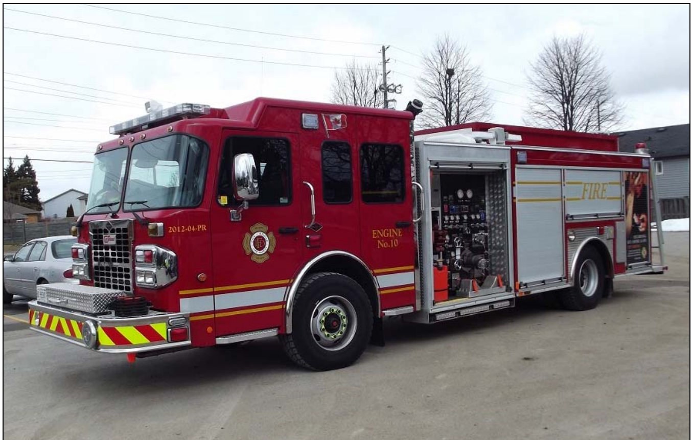
Two more of London's Spartan/Carl Thibault pumpers, from two different angles. Top is the oldest, Engine 4's 2010 model. Built on a Metro Star chassis, it has a 1250igpm pump and 500gtw. Engine 10, is on a 2012 Metro Star chassis and has a 1251igpm pump and 761gtw. (Rick Loiselle photos)
