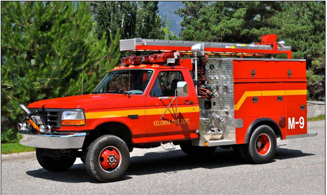
Two smaller examples of triple-combination pumpers, Kelowna, BC Mini-9 is a 1976 shop-built rig, remounted on a 1996 Ford F-350XL chassis. It has a 250igpm pump and 300gwt.
