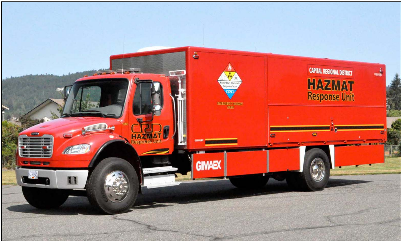
Quartered in the Central Saanich station with Engine 2, the is Capital Regional District Hazmat truck, built by Gimaex on a Freightliner M2 chassis (Terry Yip photos).
