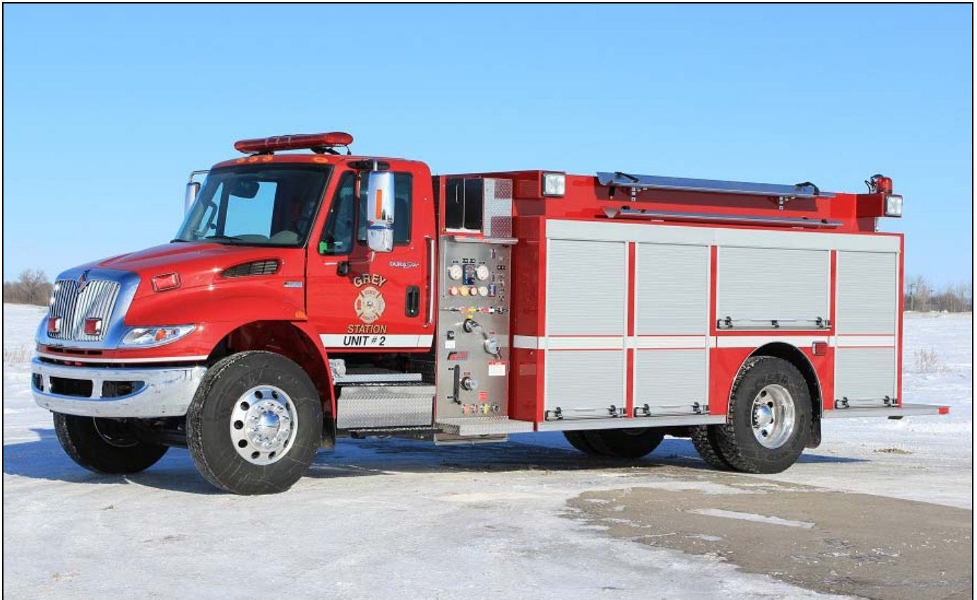
Delivered to the Huron East FD in February, this 2012 IHC Durastar/Fort Garry tanker has a 420igpm pump and 1600gwt. Unit 2 is assigned to the Grey Station. Sables-Spanish River also received a Durastar/Fort Garry rig, this one is a medium rescue. (Dave Stewardson photos)
