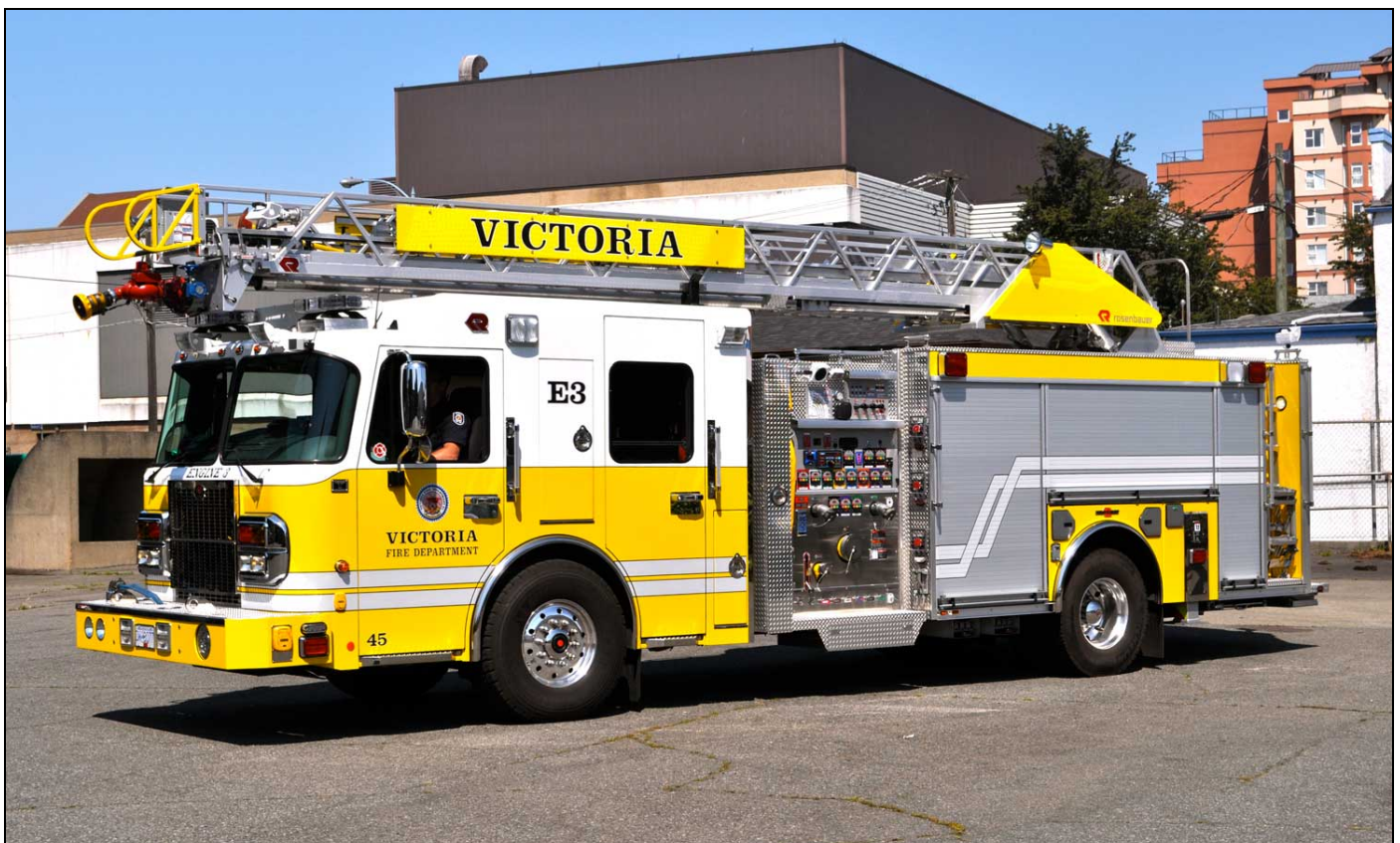
Victoria Engine 3, actually a 2011 Spartan Gladiator/Rosenbauer 1250igpm/420gft/2x20gft/60' quint.
