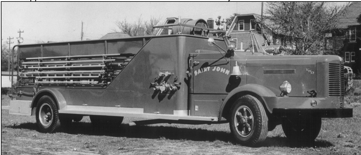
St. John, NB had this 1954 FWD quad, with an 840igpm pump and 300gwt. (Matt Lee photo)
