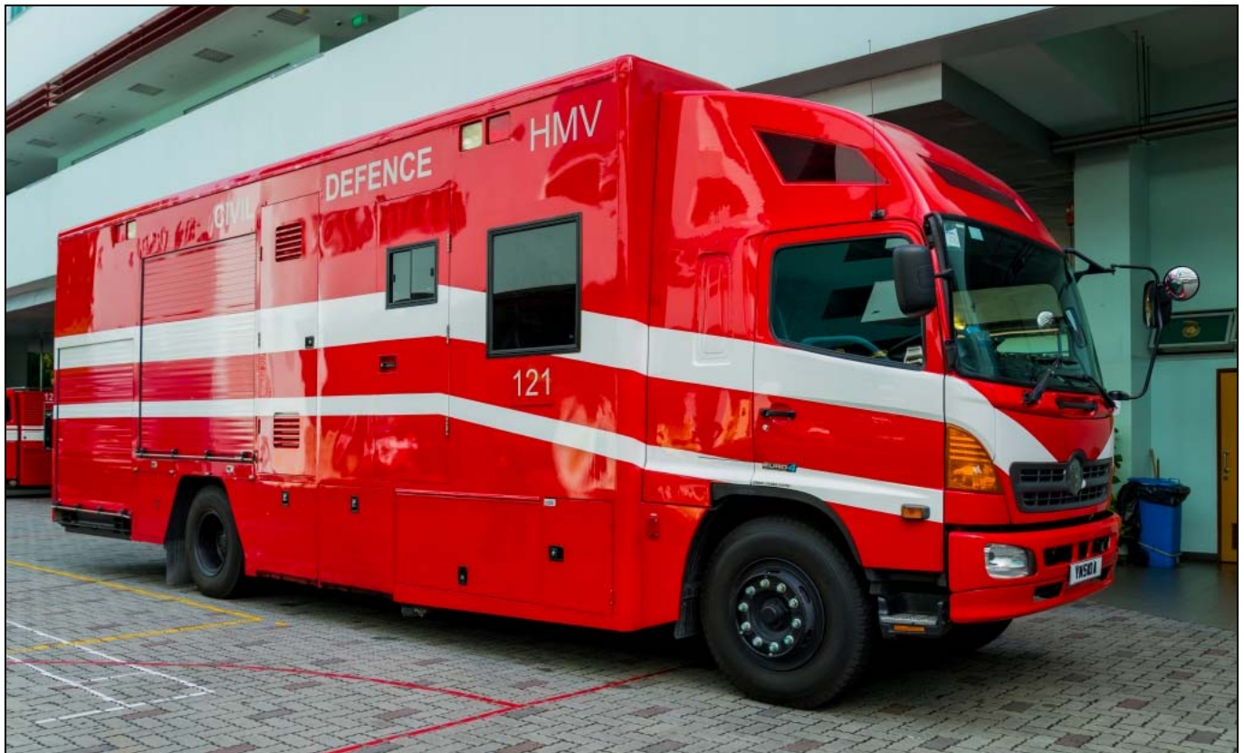
Also from Singapore, their heavy haz-mat unit. HMV 121 (Hazmat Mitigation Vehicle, station 12, no.1). Station 12 is located near the oil refineries off the south end of the island. Built on a Hino chassis, it carries a John Deere ATV for transporting equipment and crew members around large sites. (Kenneth Lai photos)
