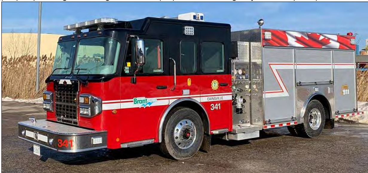
Prince Twp, ON Pump 1, a 2018 Freightliner/Maxi Contender 1050igpm/1658gwt/30gft (Stock unit) (Gary Dinkel photo) Below: Brant County, ON Pump 341, a 2020 Spartan Metro Star/Dependable product with 1500gpm pump, 1000gwt and 30gft s/n 52981 (Dependable Emergency Vehicles photo)
