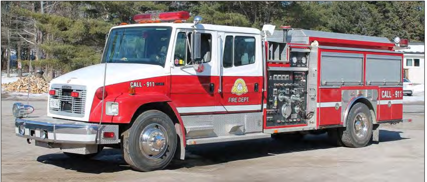
Second away: a 2004 Freightliner FL 80 / Ferrara pumper, 1050igpm pump/500gwt. Originally from Texas.
