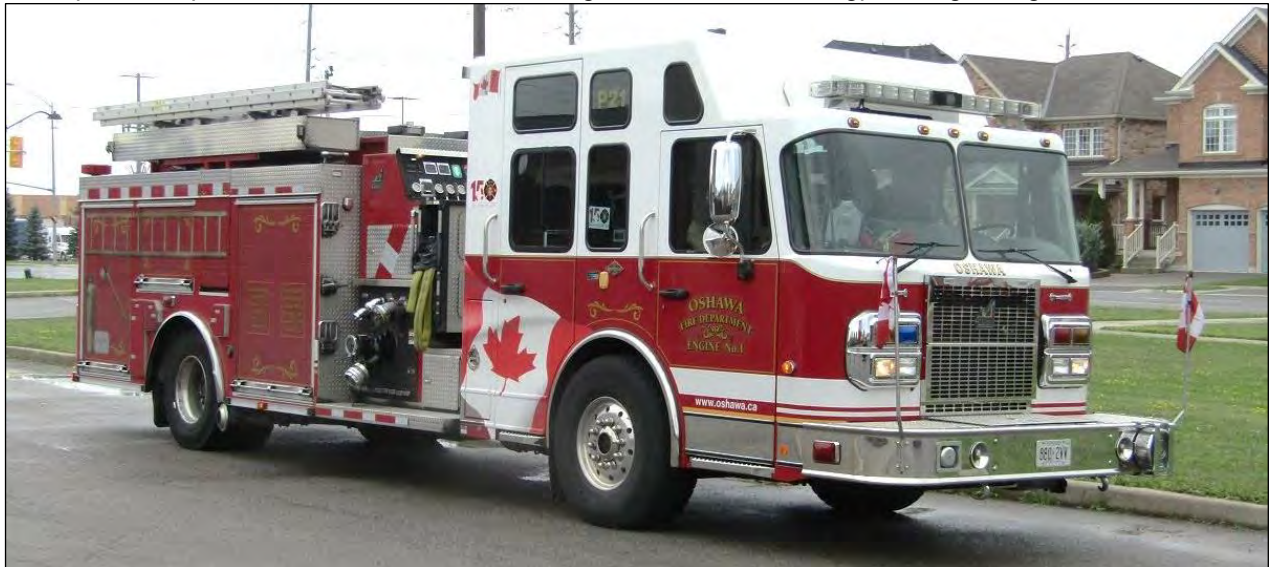
Pumper 21, a 2007 Spartan Gladiator Classic /Smeal pumper, 1250igpm/500gwt/25gft. S#709011
