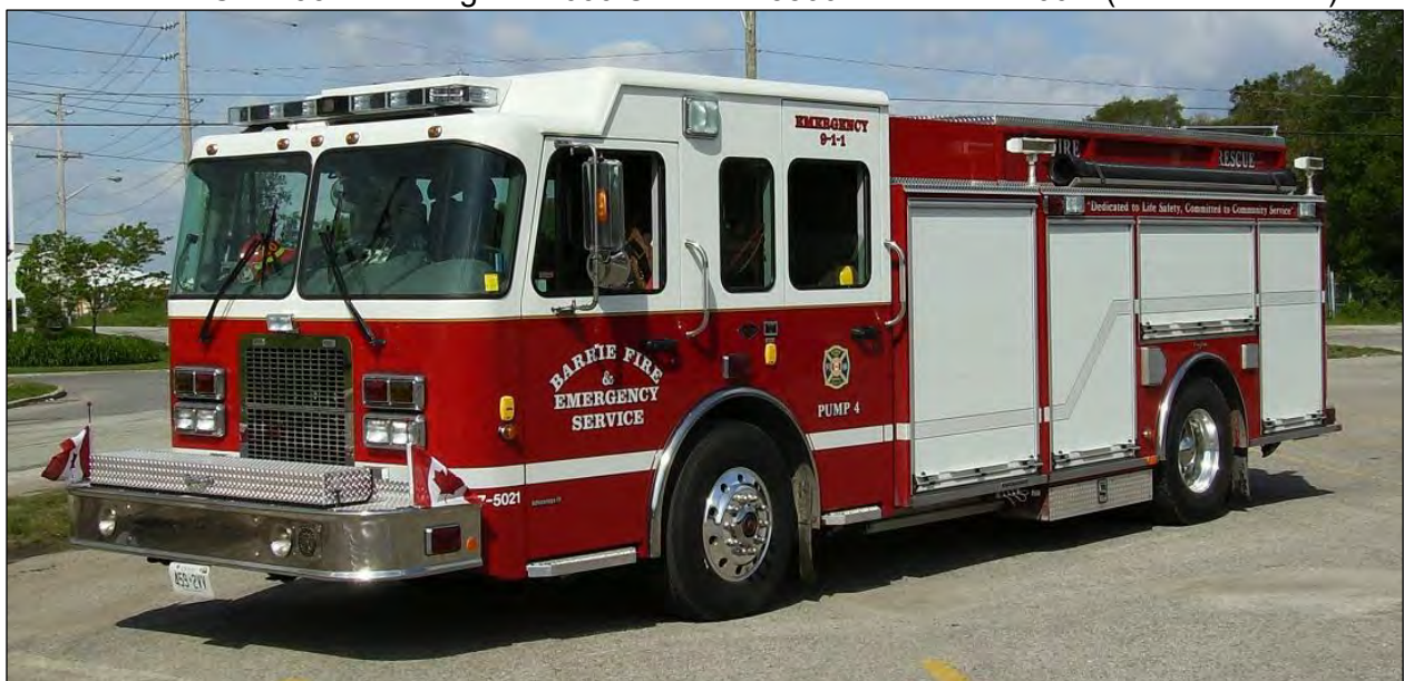
Another rig seen on the Barrie tour, this was former Pump 4, assigned as Pump 8. The 2000 Spartan/Almonte pumper was now in reserve with a 1050igpm pump, 625gwt and 40gft. (Neil McCarten)
