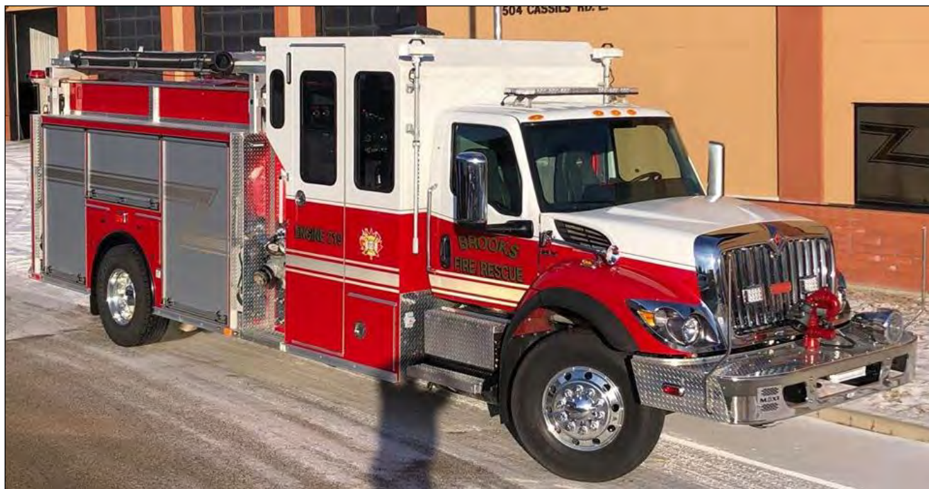
Brooks, AB Engine 219, a 2019 IHC HV607/Maxi Metal TME 1250igpm/840gwt* (MMFT)
