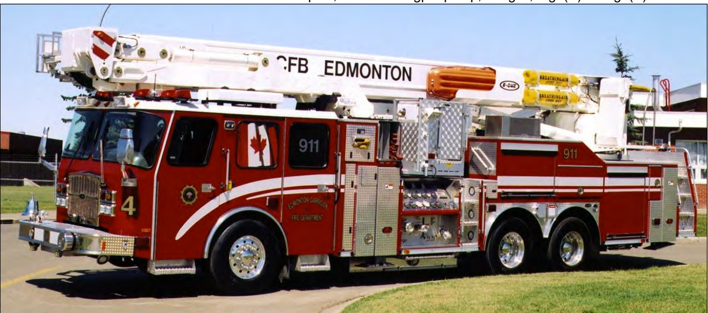
Now Red 4 is a 2006 E One Cyclone II tower with 1750igpm pump, 240gwt and a 100' Bronto. (Dave Stewardson)
