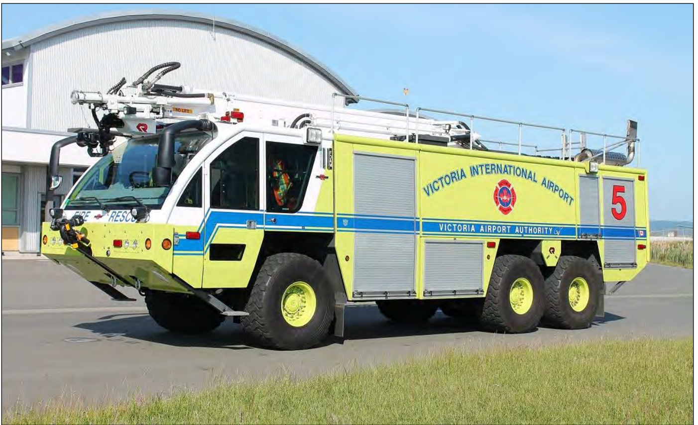
Victoria Airport Red 5 is a 2011 Rosenbauer Panther 3000 6x6 with a 1850igpm pump, 2750gwt and 330gft. It carries 500 lbs. dry chemical and 50' Stinger HRET.
