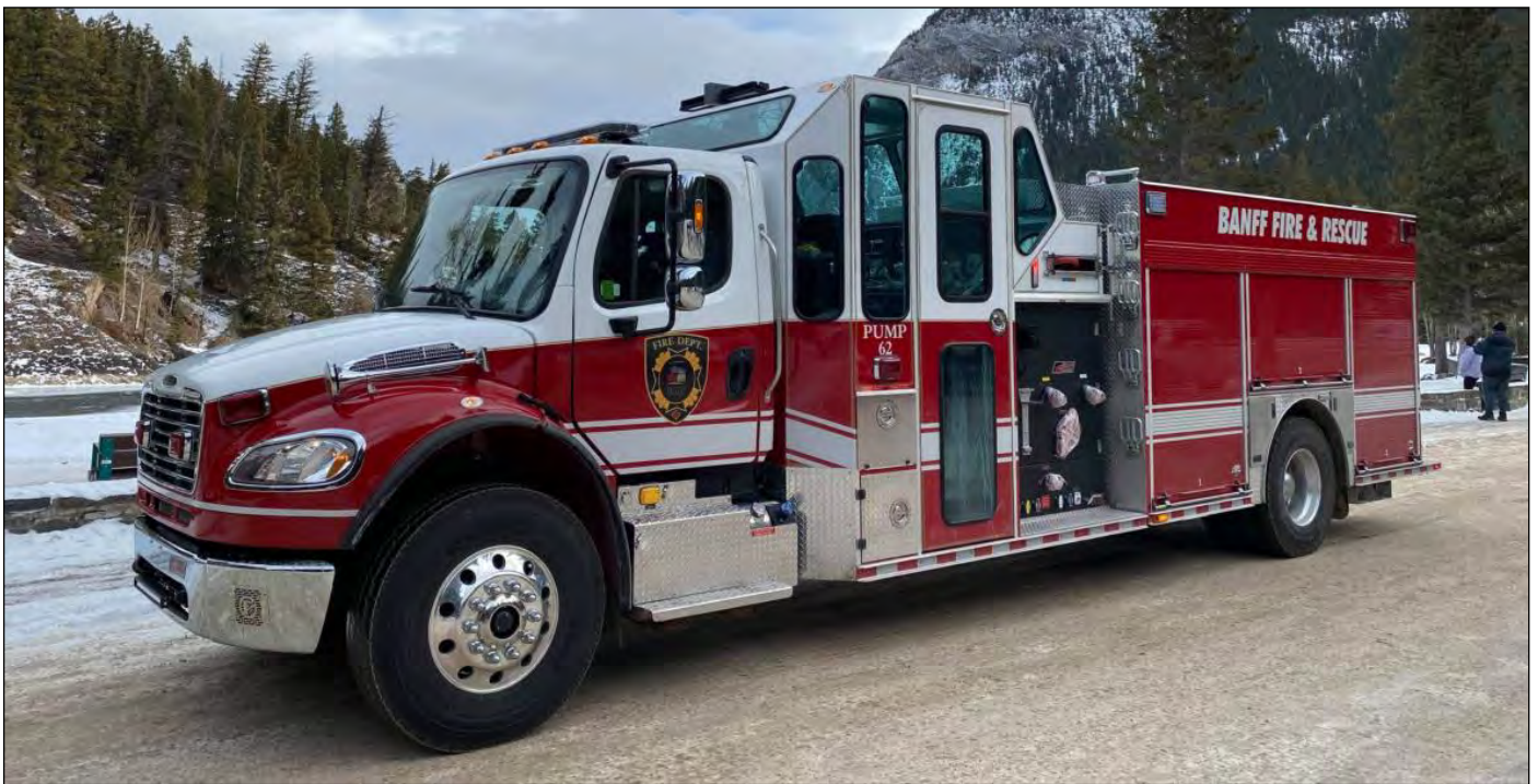
Banff, AB Pump 62, a 2020 Freightliner M2-106/Fort Garry 1250igpm Waterous pump and an 800gwt, s/n J00016 (Fort Garry Fire Trucks photo)
