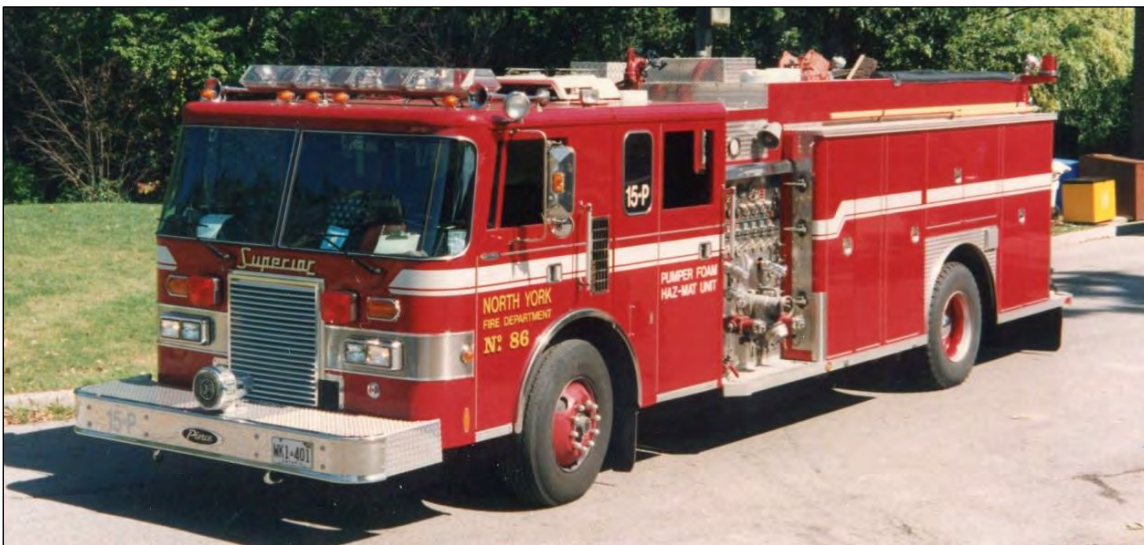
For the new haz mat and rescue pumps, the department switched to much longer Pierce chassis. 15P ran No.86, a 1991 Pierce Superior haz mat pump equipped with a 1050igpm pump, 300gwt, 100gft and dry chem. (Photos from the Larry Ward Collection)
