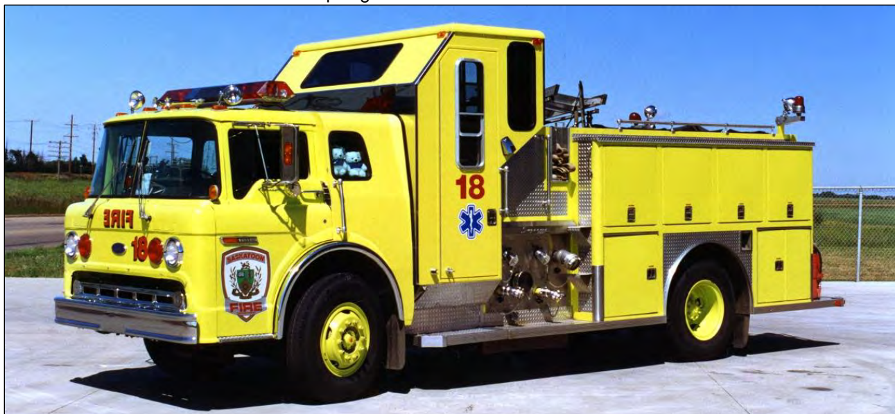
Saskatoon, SK Unit 18, a 1987 Ford C/Superior pumper, 1050igpm/500gwt, 1992 Crestline rehab. s/n SE799.
