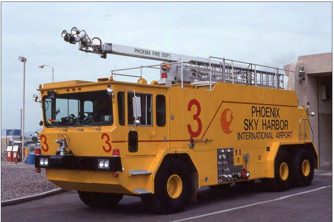
Phoenix Sky Harbor Airport Red 3 with the first Snazzle, a 50 footer, mounted on a 1987 Oshkosh TA-3000. It had a 1250 US gpm pump and a 3000gwt. Phoenix still has a Snazzle stationed at the airport, the current 65' model is on a 2006 Oshkosh Striker 4500. (Dan Goyer photo)
