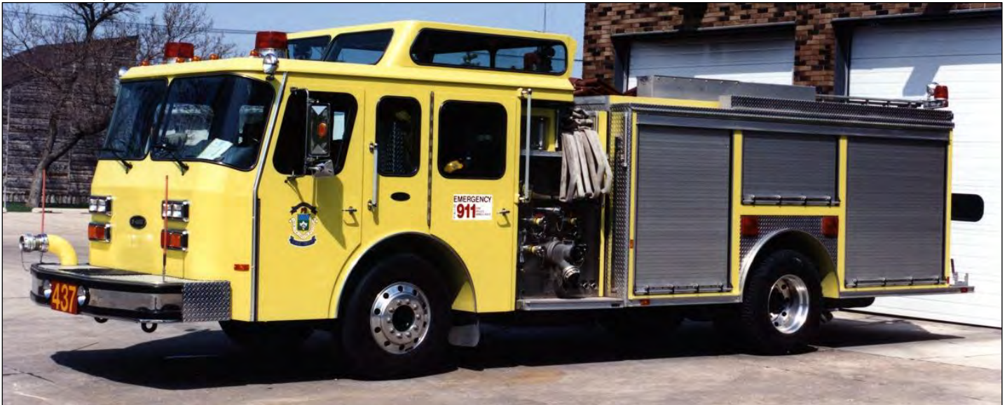
Winnipeg Shop #437, a 1990 E One Hush pumper with a 1050igpm pump and 500gwt. (Dave Stewardson)
