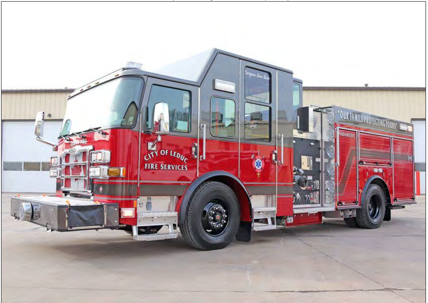
Leduc, AB P.1 2020 Pierce Enforcer, 1750gpm Waterous pump, 500gwt and a Husky 3 FS j/n 33928 (Photo courtesy Pierce Manufacturing)
