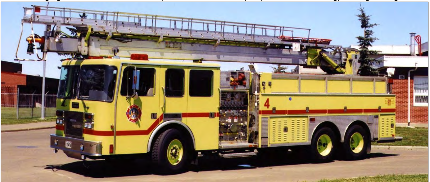
Red 4 was this 1996 Pemfab Tibotrac 75' quint, with a 1050igpm pump, 300gwt, 26gft(A) & 10gft(B).
