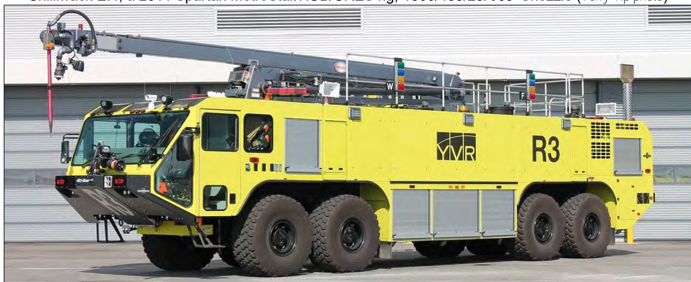
Vancouver Airport operates three HRET equipped CRTs. The largest is Red 3, a 2013 Oshkosh Striker 4500 8x8 (1665igpm/3750/525F/500lbs. DC/50' Snizzle). Red 5 & 6 are Striker 3000s. (Dan Goyer photo)
