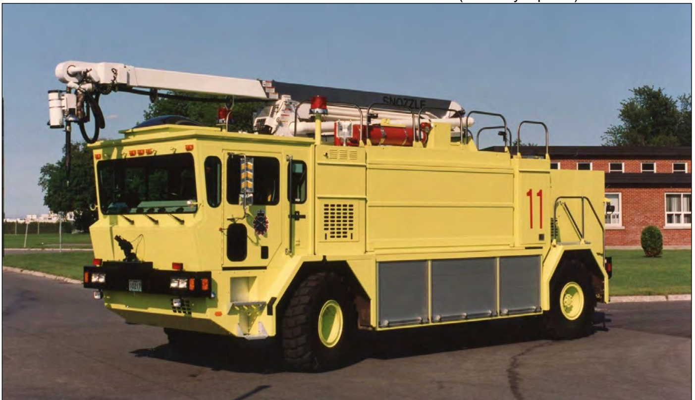
CFB Uplands, Ottawa also had a Snazzle, attached to a 1993 Oshkosh TA-1500C (MFV 6000) CRT, it had an 1100igpm pump, 1320gwt, 155gft and 500 lbs Purple K. (Dave Stewardson Photo)
