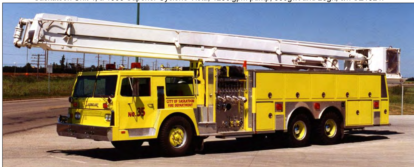
Saskatoon Unit 35, a 1974 Hendrickson originally topped with a 125' Calavar Firebird. A 1989 Superior rehab and replacement of the Calavar resulted in this 85' tower, with a 1050igpm pump and 300gwt. (Dave Stewardson photos)
