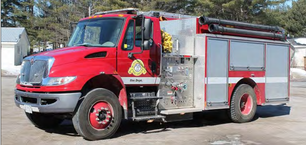
First away: a 2010 International / Pierce pumper, 1050igpm/650gwt. (SN#1HTMKAZR49H089530)
