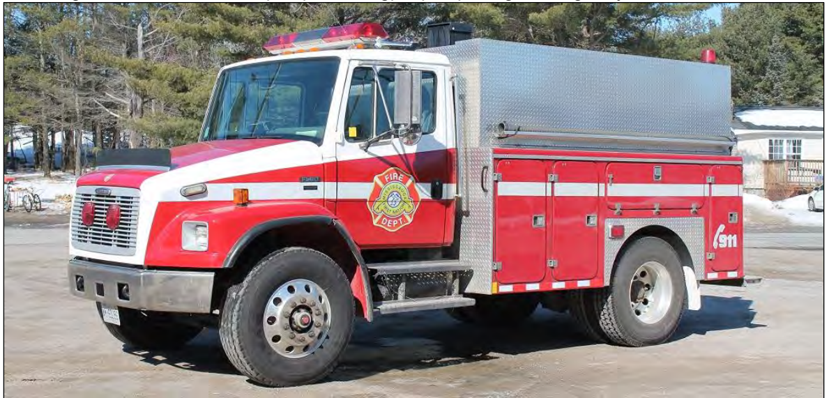
Tanker: a 2004 Freightliner FL 80 / 2018 Dependable tanker, 1500igwt, (Dan Goyer photos)
