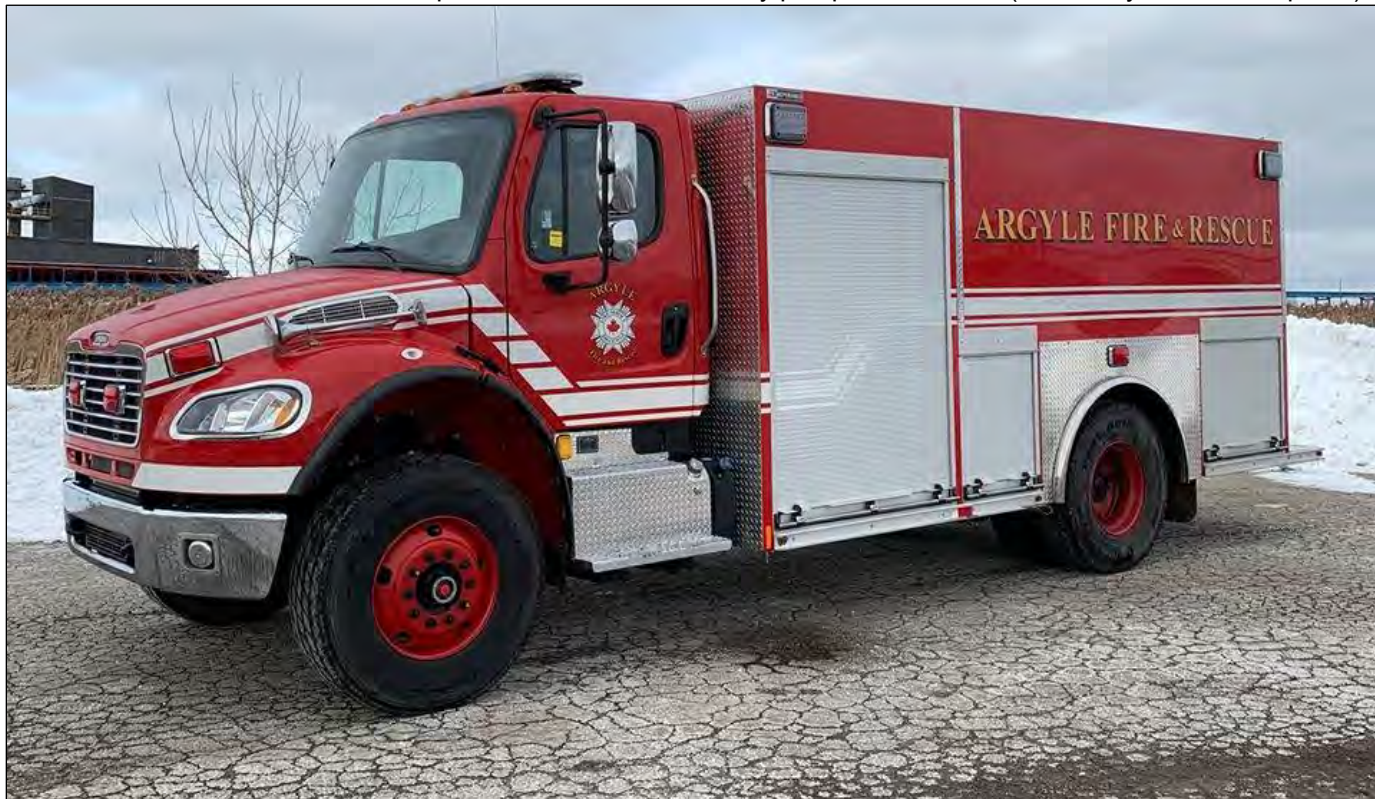
Argyle, ON's new tanker, 2019 Freightliner M2-106/Dependable equipped with a 2500igwt. (Dependable Emergency Vehicles photo)
