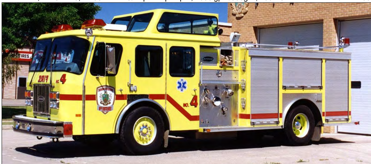
Saskatoon Unit 4, a 1993 Superior Cyclone Vista, 1250igpm pump, 500gwt and 25gft, s/n SE1324.
