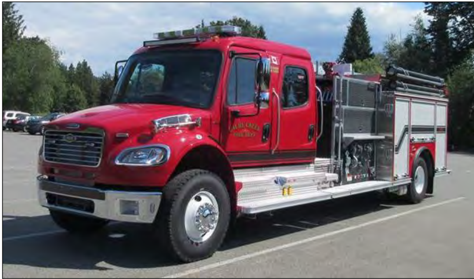
Cache Creek, BC Engine 4, a 2019 Freightliner M2-106/Hub pumper with a 1050igpm Hale pump, 950gwt and 30gft FP 2001 FS j/n 1246 (Hub Fire Apparatus photo)
