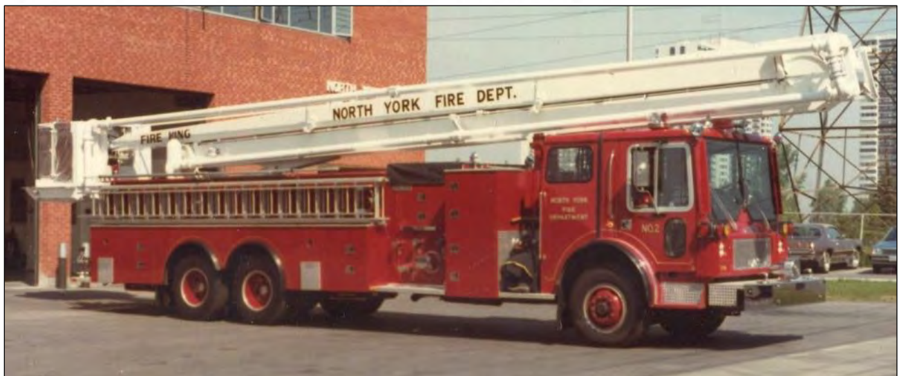
This is the 1980 Mack/King Seagrave 85' tower, seen here at Station 12. It had a 1050igpm pump.
