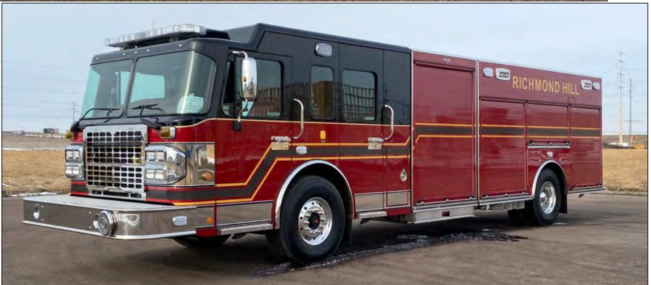
Richmond Hill, ON Engine 861 - 2019 Spartan Gladiator/ERV 1665igpm/500gft/50gft (SERV photo)
