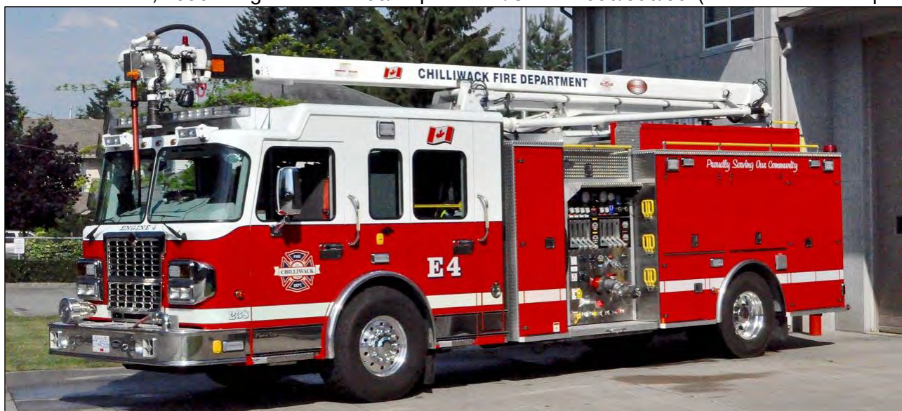
Chilliwack E.4, a 2011 Spartan MetroStar/HUB/CRES rig, 1500/485/25A/65' Snizzle (Terry Yip photo)
