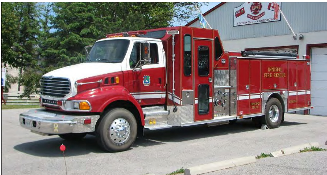
Innisfil Pumper 4, a 2007 Sterling Acterra / Fort Garry pumper 1050igpm/800gwt (SN#A342)
