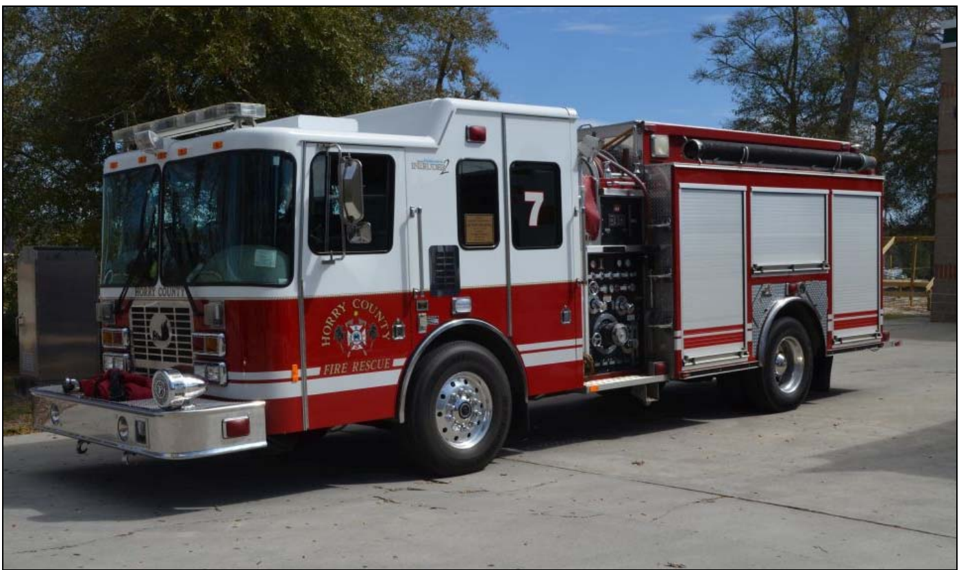
This just in: Bob Rupert, vacationing in Myrtle Beach, SC sent these from the local station in Horry County: Engine 7 is a 2008 Ferrara Intruder, 1500gpm/1000gwt (SN 97389), Tower 7 is a Spartan/Ferrera 104' rearmount quint, 1500gpm/600gwt. (SN 78676)
