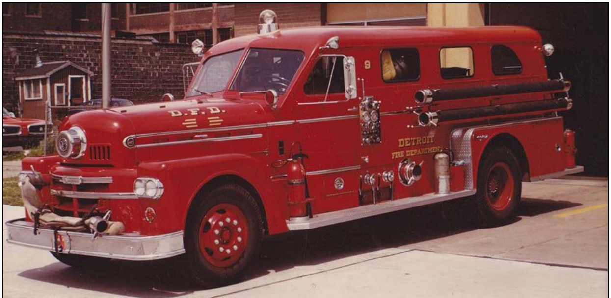
A classic 1961 Seagrave sedan cab engine from Detroit. Engine 9 had a 1000gpm pump and 300gwt. (Ken Buchanan photo)
