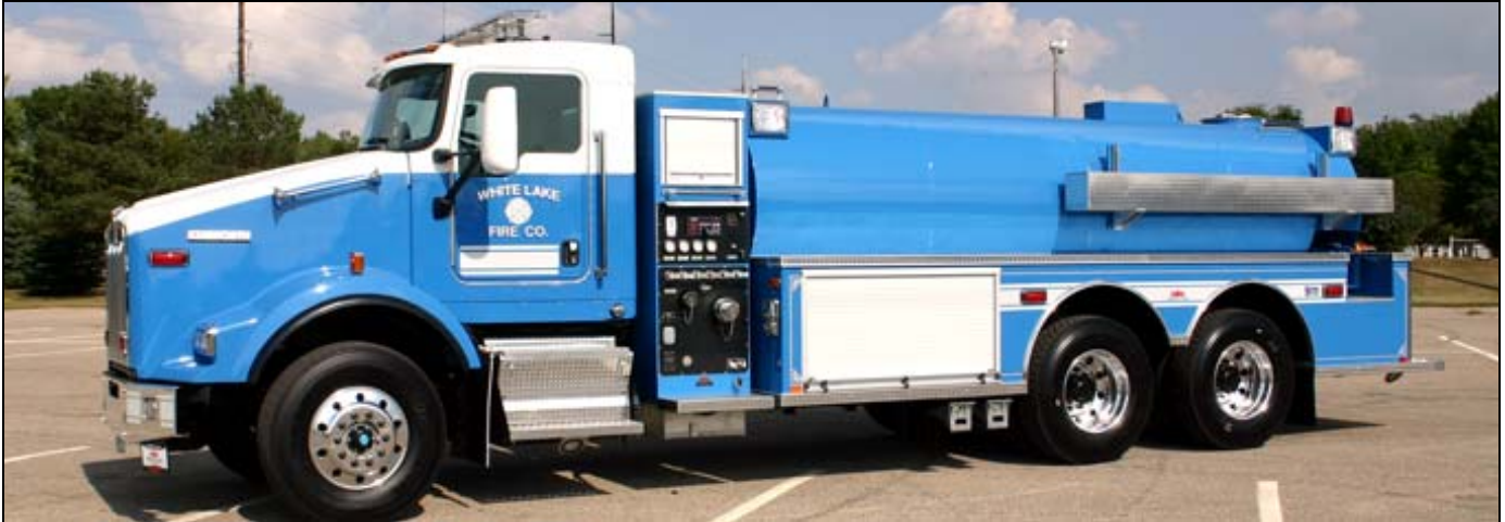
This extra long white over sky blue tanker belongs, appropriately, to White Lake, NY. It's a 2009 Kenworth T800/Midwest combination with a 500gpm pump and 3000gwt. SN 2081. (Midwest Fire photo)
