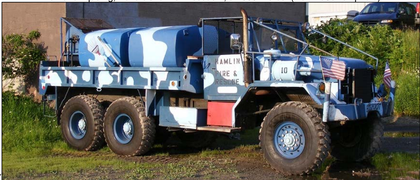
Definitely a one-off, this U.S. Army 1975 Mack 6x6 converted to a tanker for Hamlin, PA. Tanker 10 sports a unique paint scheme (Hamlin's rigs are blue but not camo) and has two 750gws. (Neil McCarten photo)
