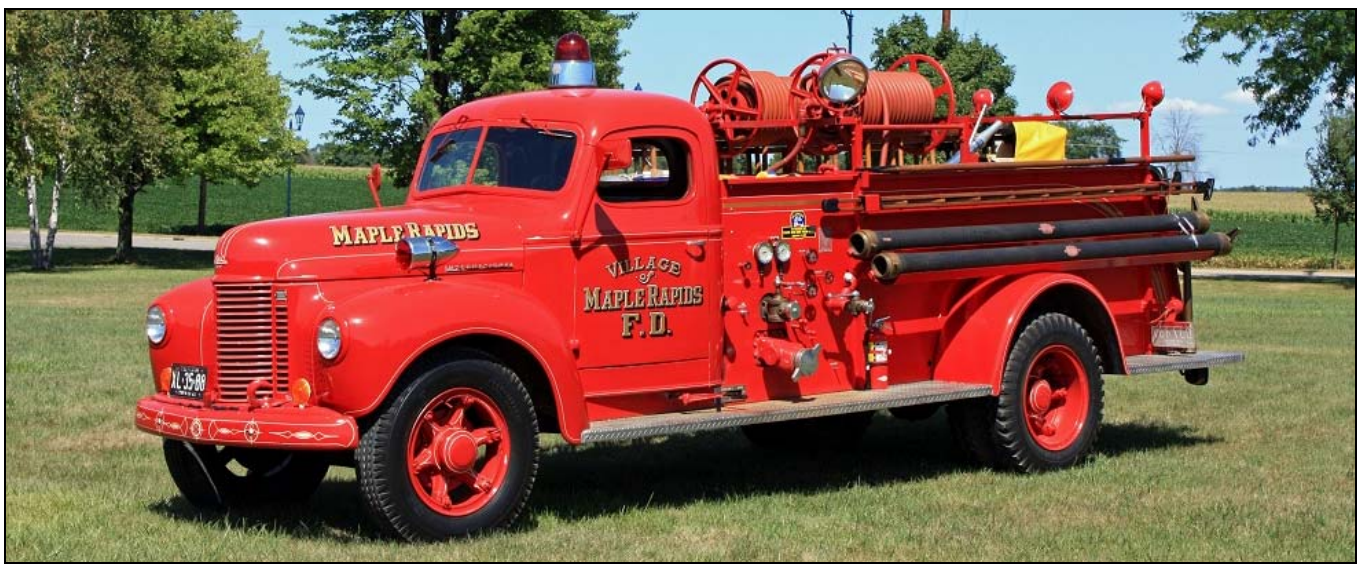
Maple Rapids, MI had this 1945 IHC KB/American pumper, it has a 500gpm pump and 300gwt, now owned by Russell Riley. (Herb Galloway photo)
