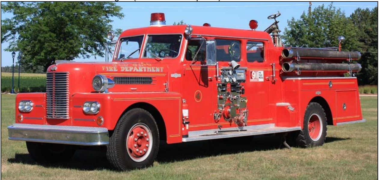
Another sedan cab, this 1967 Pirsch custom pumper served with Red Wing, MN as Engine 4. It sports a 1250gpm pump and a 300gwt. (Herb Galloway photos)
