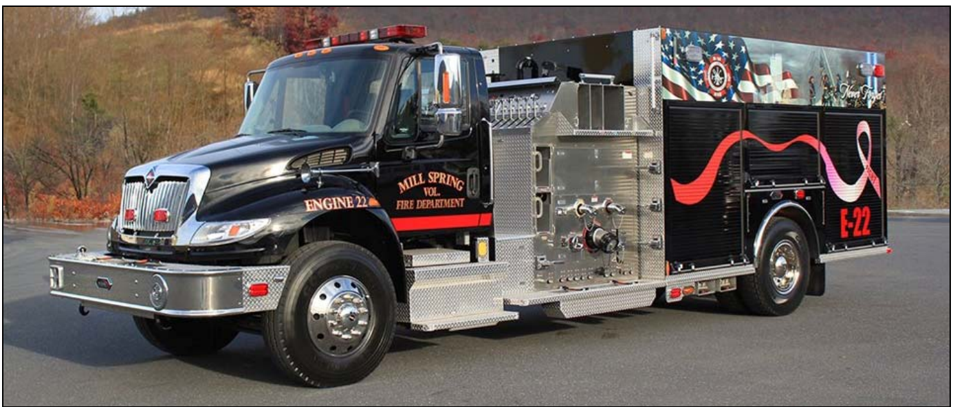
This 2013 IHC 4400/KME pumper-tanker is painted black. Mill Spring, NC Engine 22 sports a 1750gpm Hale pump and a 1500gwt. (KME photo)
