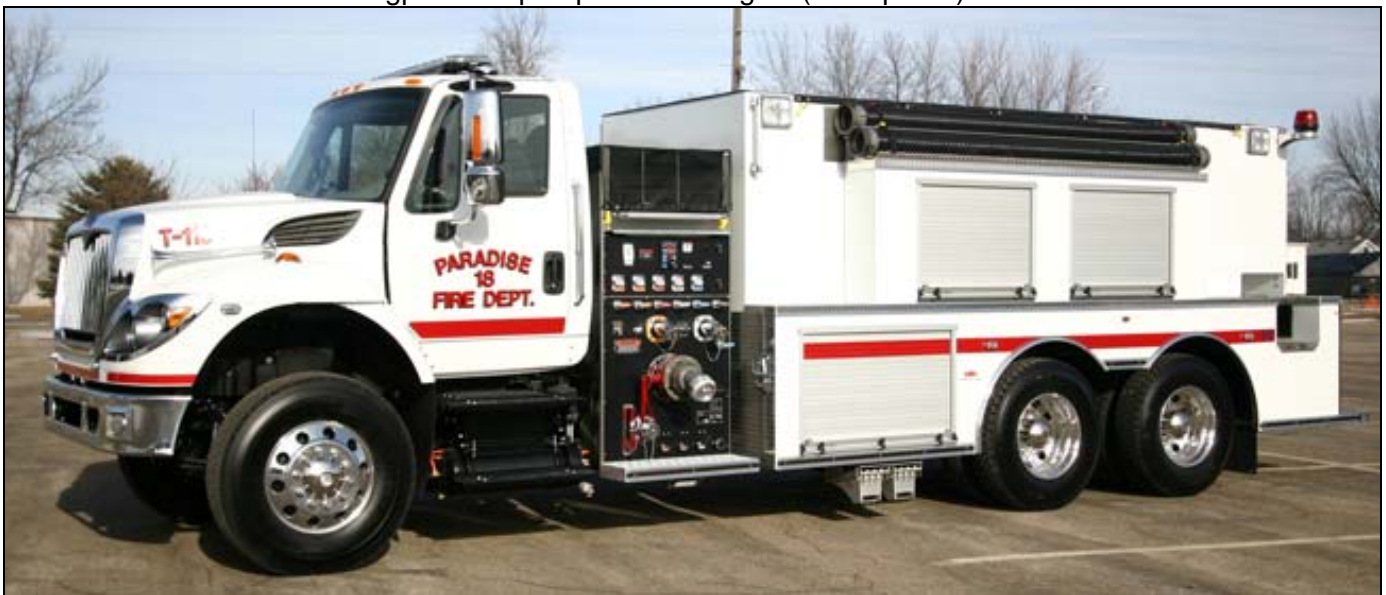
Paradise, TX owns this big all white 2012 IHC 7400/Midwest pumper-tanker. Tanker 1 has a 1250gpm Darley pump and a 3000gwt. (Midwest Fire photo)
