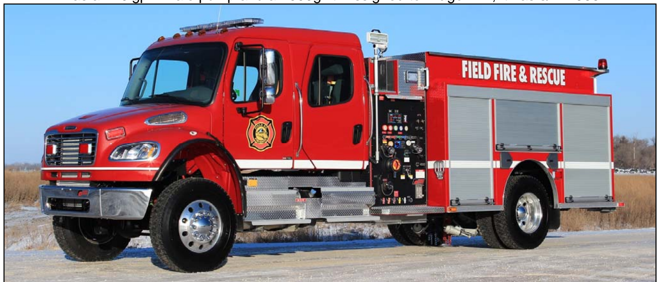
A Christmas present for Field, BC. They took delivery of this 2014 Freightliner M2-106 4x4/Fort Garry pumper early last December. It has a 1050igpm Darley pump, 800gwt and two 20gfts. S/N M592
