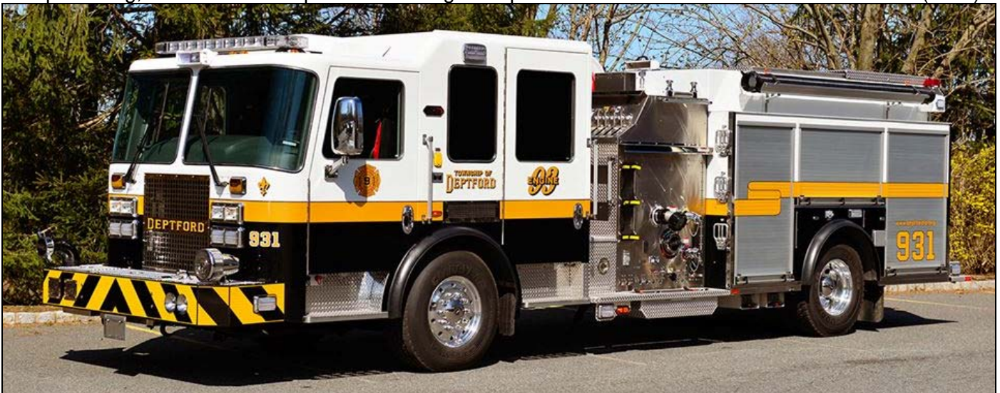
From Deptford Twp., NJ, Engine 931 in black & white. This is a 1997 KME 1750gpm pumper. (KME photo)
