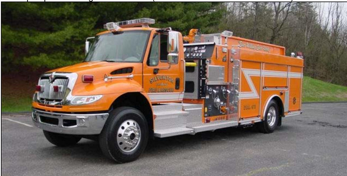
The Silvertown VFD in Ravenswood, WV just received this 2015 IHC 4400/Smeal pumper tanker resplendent in orange. It has a 1250gpm Waterous pump and a 1000gwt. (Smeal photo)
