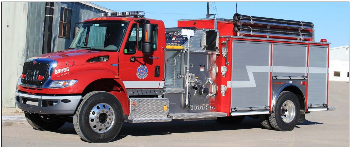
Manitoba Hydro recently took on this 2014 IHC 4400/Acres 1050/1000/25 top-mount pumper for their Keewatinohk Converter Station. SN 141031123.
