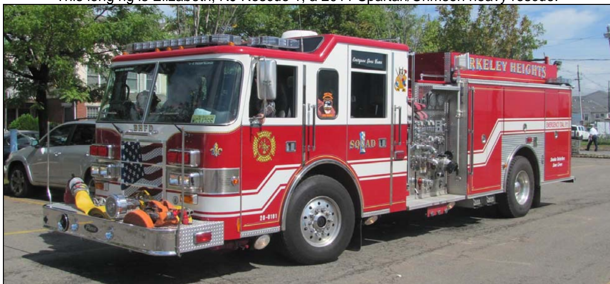
Berkeley Heights, NJ Squad 1, a 1998 Pierce Dash rescue-pumper, 2000gpm, 750gwt. (Desmond Brett photos)
