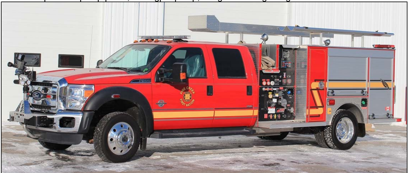
Pine Creek First Nation in Manitoba recently got this stock unit from Fort Garry on a 2013 Ford F550 4x4 chassis with a 300igpm pump, 300gwt and 10ft. SN M415. (Dave Stewardson photos)
