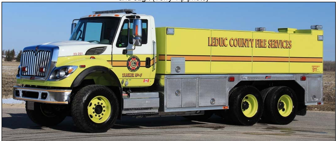
Leduc County, AB 2015 IHC 7400 4x4/Fort Garry Fire 420igpm Darley pump, 2500gwt s/n M613. (John Bowerman photo)
