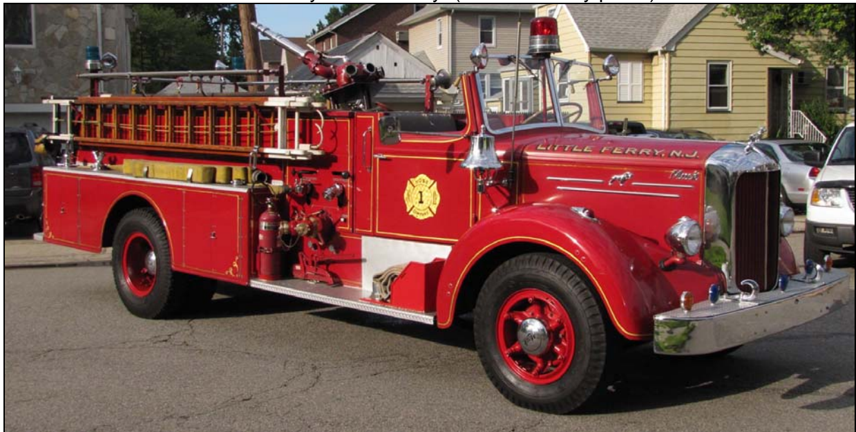
Little Ferry, NJ still has this beautifully kept 1953 Mack L95S engine, 1000gpm, 500gwt. (D. Brett)
