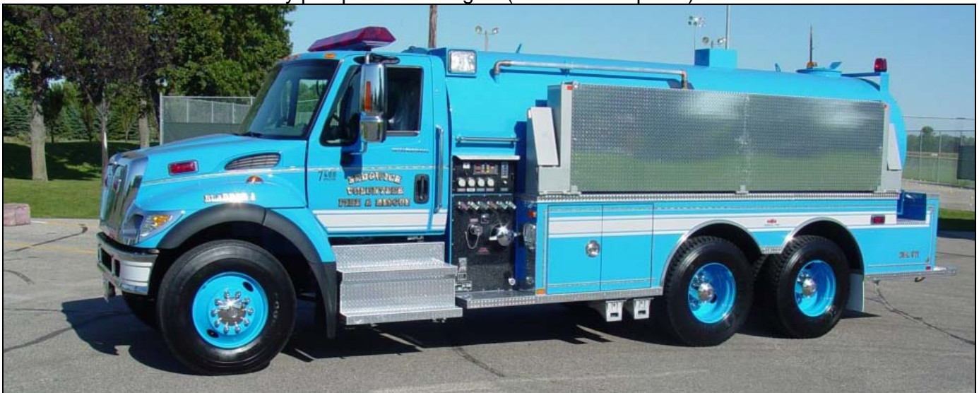
A striking sky blue, right down to the wheels, is Sedgewick, CO's 2005 IHC 7400/Midwest tanker. It's equipped with a 500gpm Hale pump and 2500gwt. (Midwest Fire photo)
