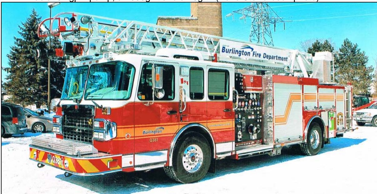
Burlington just put this 2014 Spartan Gladiator/Smeal rearmount in service as Quint 381. It features a 1500gpm pump, 345gwt/, 20ft and 75' aerial. It' also has a FoamPro 2001 FS SN 4320. Below is the BFD's Platoon Chief's vehicle, Car 30, a 2014 Ford F250 (Doug Holmes photos)
