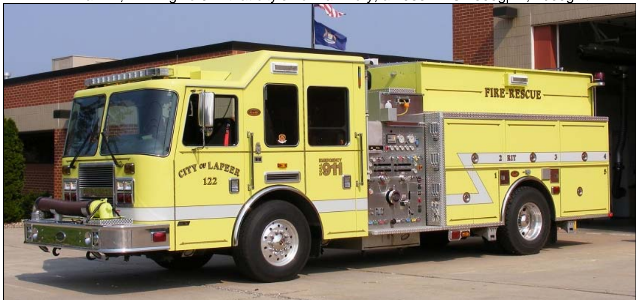
Lapeer, MI Engine 122, as were all their rigs, in pale yellow. It's a 2006 KME with a 1500gpm pump and 1000gwt. (Neil McCarten photos)
