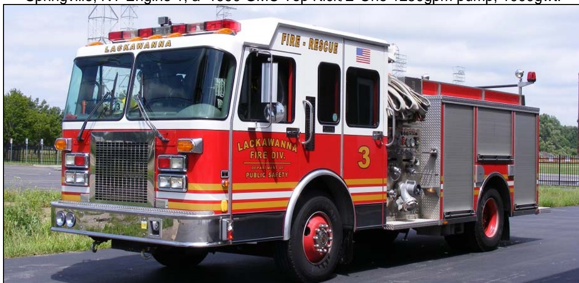
Lackawanna, NY Engine 3, a 1994 Spartan/RD Murray product with a 1500gpm pump and 750gwt. . (Neil McCarten photos)
