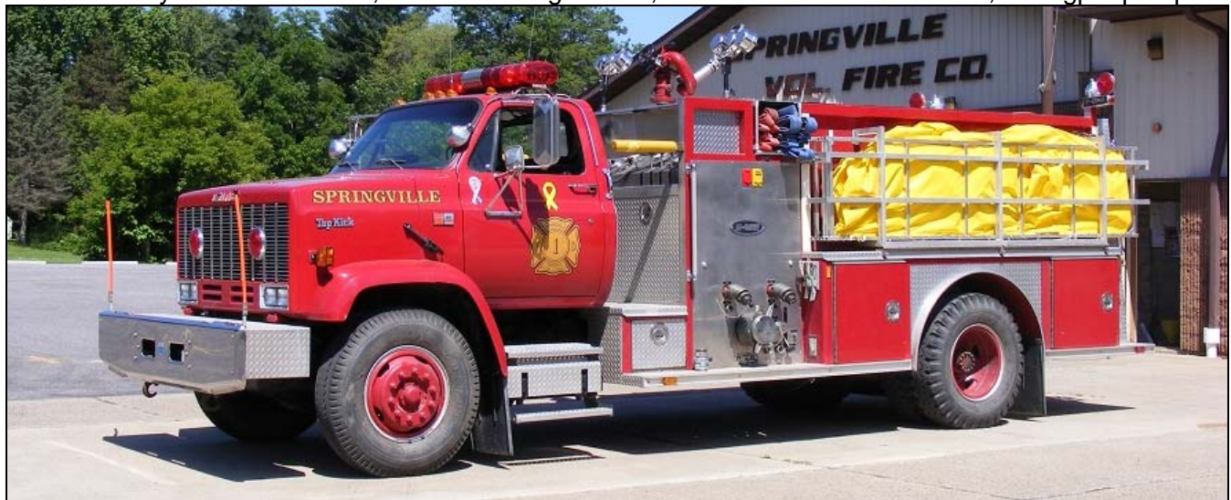
Springville, NY Engine 1, a 1990 GMC Top Kick/E-One 1250gpm pump, 1000gwt.
