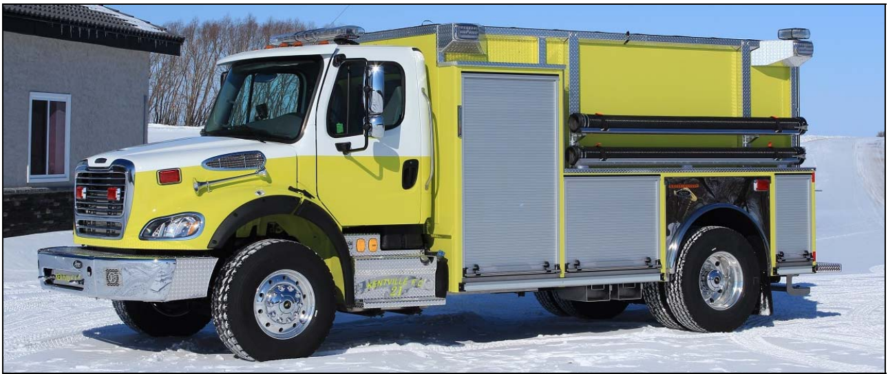
More delivery shots of rigs to be detailed by the local department: topmost is a 2015 Freightliner M2-112/Acres pumper-tanker for Kentville, NS. Tanker 21 has a 1050igpm pump and 1800gwt.
