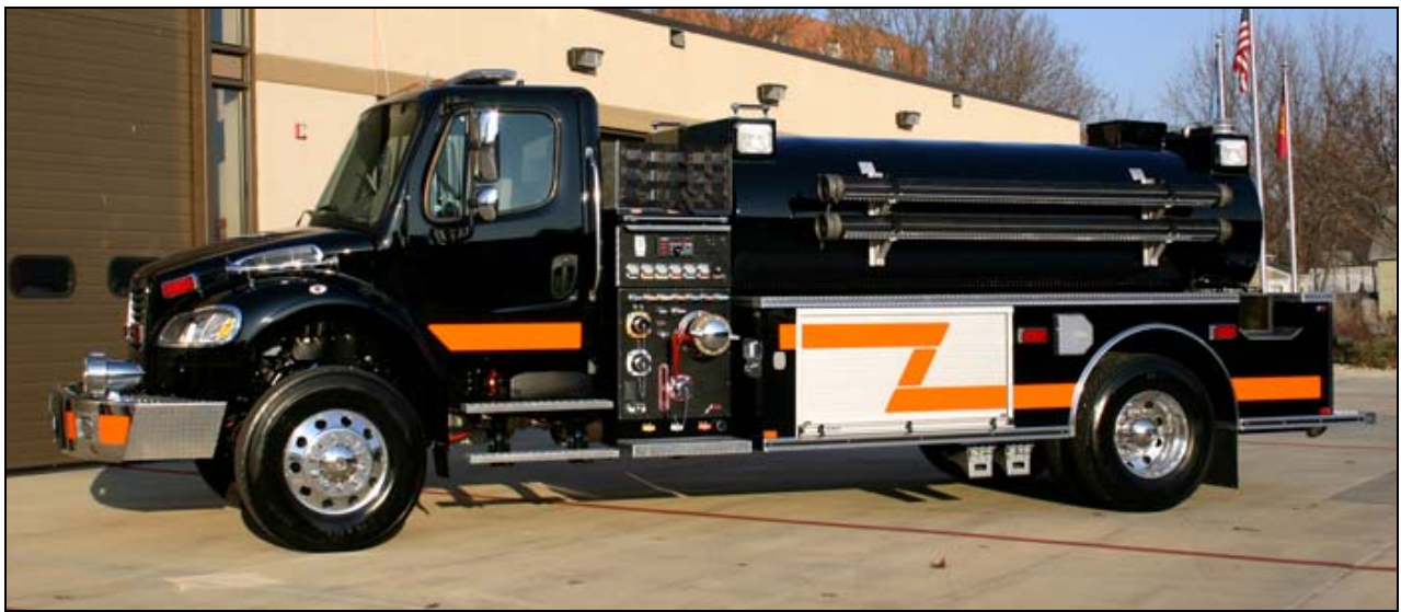
The Tri-County Fire Protection District in Richland, MO received this all-black Freightliner M2-106/Midwest pumper in 2009. It sports a 750gpm Hale pump and a 2000gwt SN 2098.
