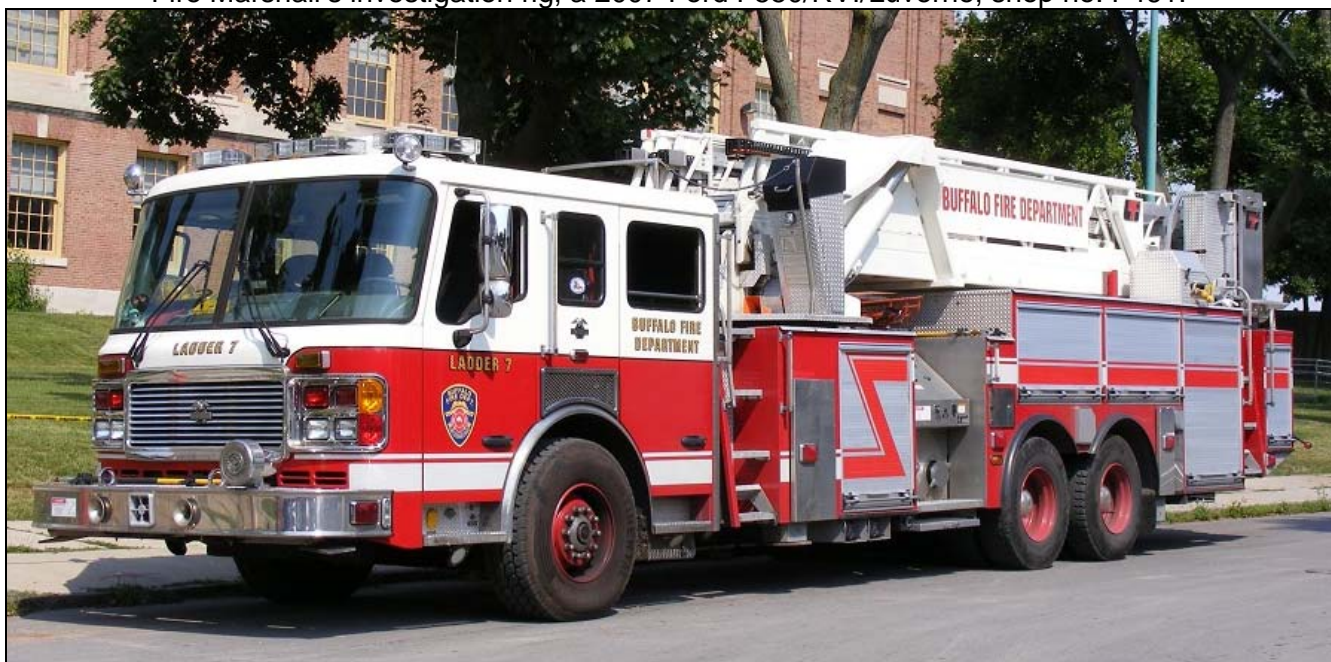
And finally, Ladder 7, a 2007 ALF/LTI 100' tower with 2000gpm pump.
