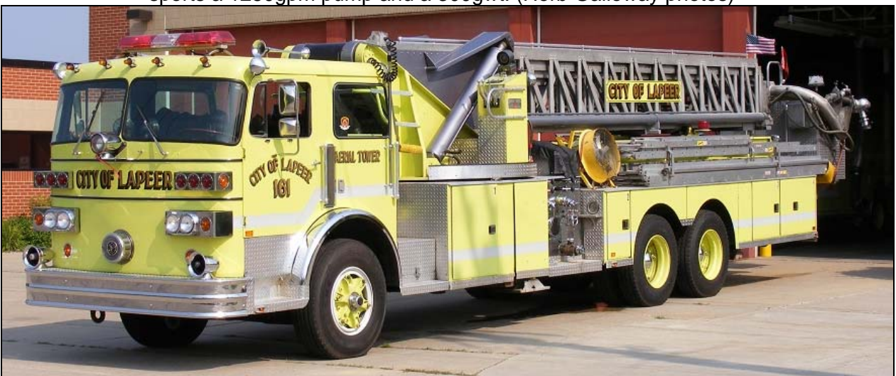
Lapeer, MI's 1976 Sutphen 95' quint. Unit 161 has a 1250gpm pump and 200 gwt. (Neil McCarten)
