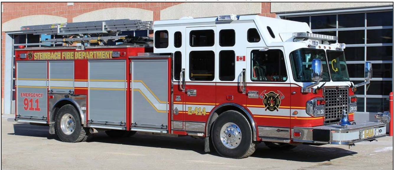
Also in Manitoba, Steinbach just got a 2014 Spartan Gladiator/Acres pumper. Equipped with an enclosed top-mount pump panel, 1250igpm pump, 700gwt and 30ft Engine 414 bears s/n 141215125.
