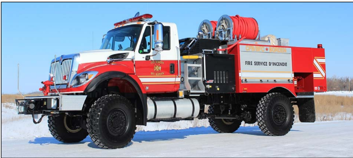
A new addition to the force at CFB Borden. This 2015 IHC 7400 4x4/Fort Garry brush unit has a 132igpm pump, a 1000gwt and a 20ft . (Dave Stewardson photo)
