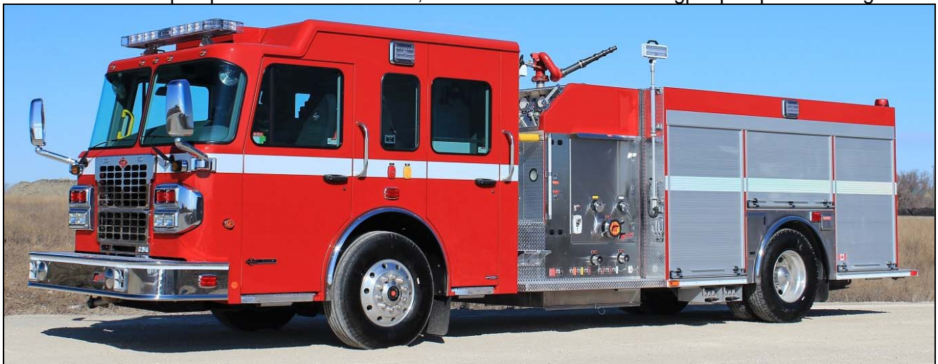
Thunder Bay's newest: a 2015 Spartan Metro Star MS/Fort Garry pump with a 1050igpm Darley pump and 600gwt. SN 597. (Dave Stewardson photos).
