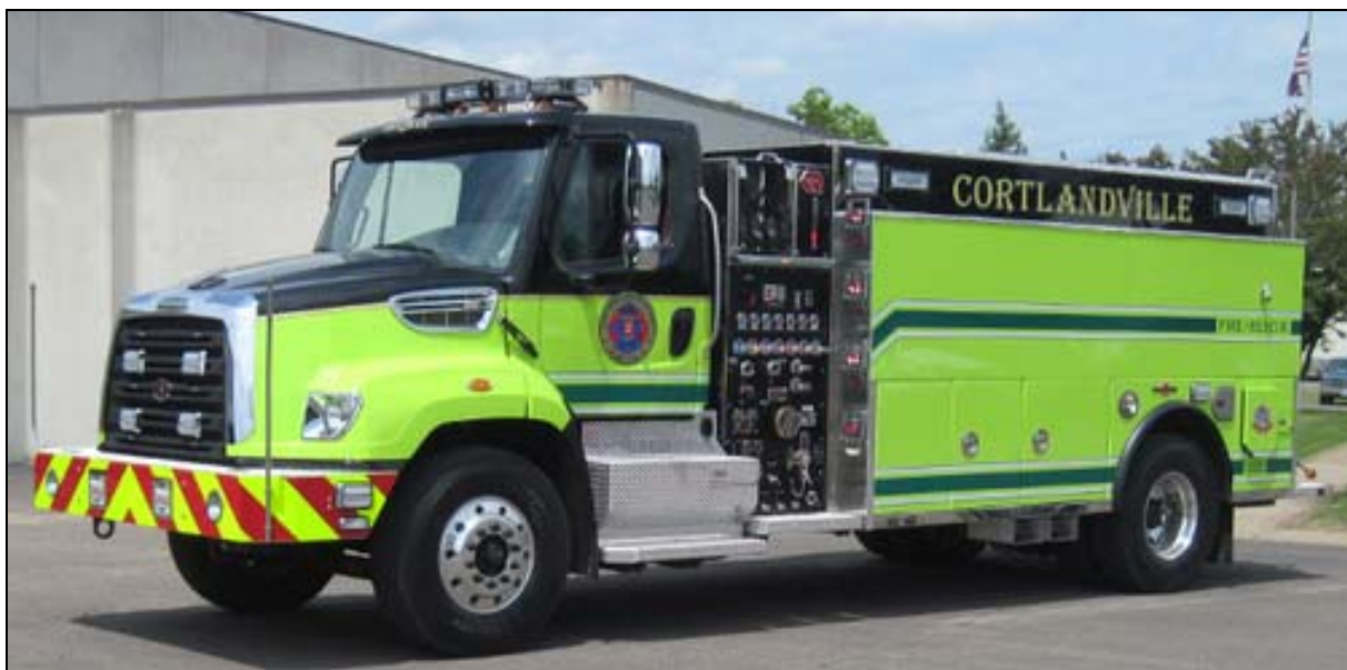
Cortlandville, NY has a unique, Freightliner Columbia/Rosenbauer rig with a 1250gpm Hale pump and 1900gwt. SN 23600. (Photo credit: Rosenbauer America)
