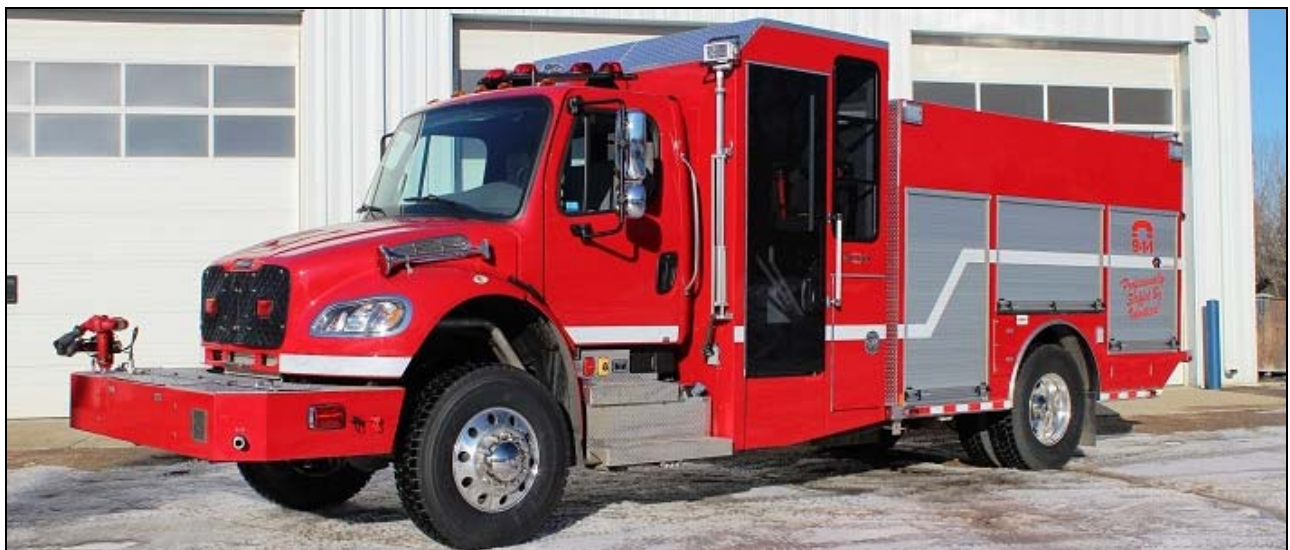
This 2015 Freightliner M2-106 4x4/Rosenbauer pumper is one of two units purchased by the Special Areas administration in Alberta. This unit went to Oyen, the other to Consort. Both rigs have a 1050 igpm Darley pump, 850gwt and a 15gft. They also have enclosed, forward facing crew seats behind the cab and inside pump controls. Also FoamPro 2001 foam systems. (Jon Bowerman photo)
