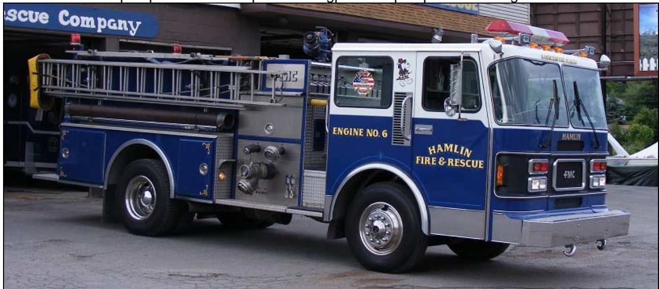
Hamlin, PA Engine 6 in that city's normal livery, a 1988 FMC 1500gpm, 1000gwt.
