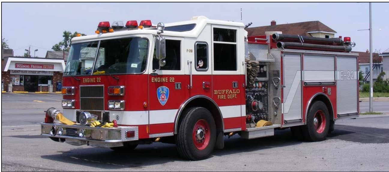
Engine 22, a 1999 Pierce with a 1250gpm pump and 500gwt, s/n 14618 and shop no. F251.
