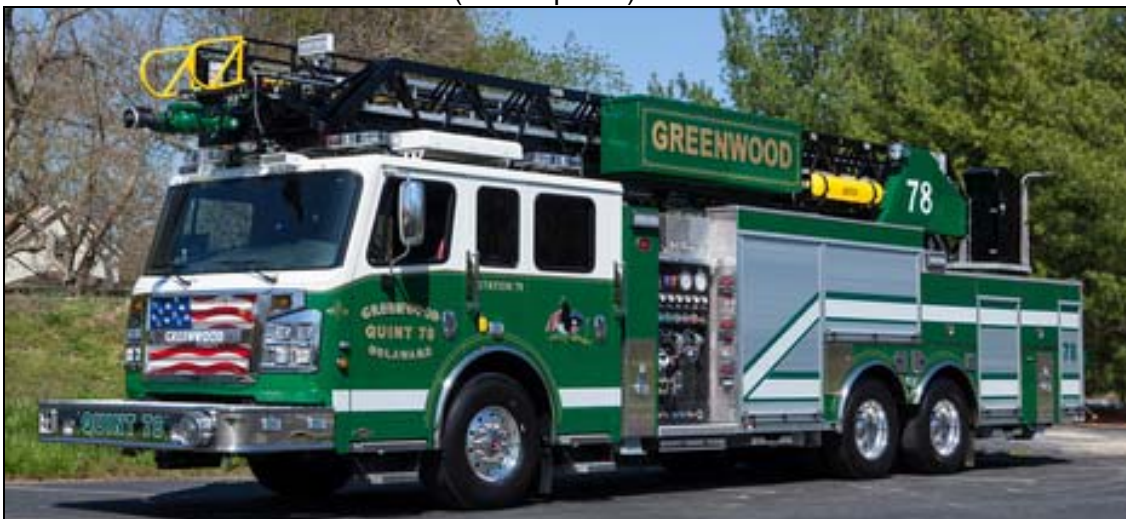
This impressive white over green Rosenbauer Viper 78' aerial belongs to Greenwood, DE. It has a 1500gpm Hale pump and 500gwt. (Photo credit: Rosenbauer America)
