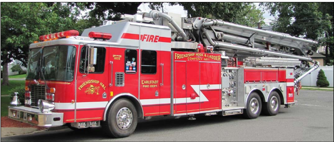
This unique apparatus is an aerial platform built by concrete pumper manufacturer Schwing for the Carlstadt, NJ FD. The 115' platform is mounted on a 1997 HME chassis. (Desmond Brett photo)
