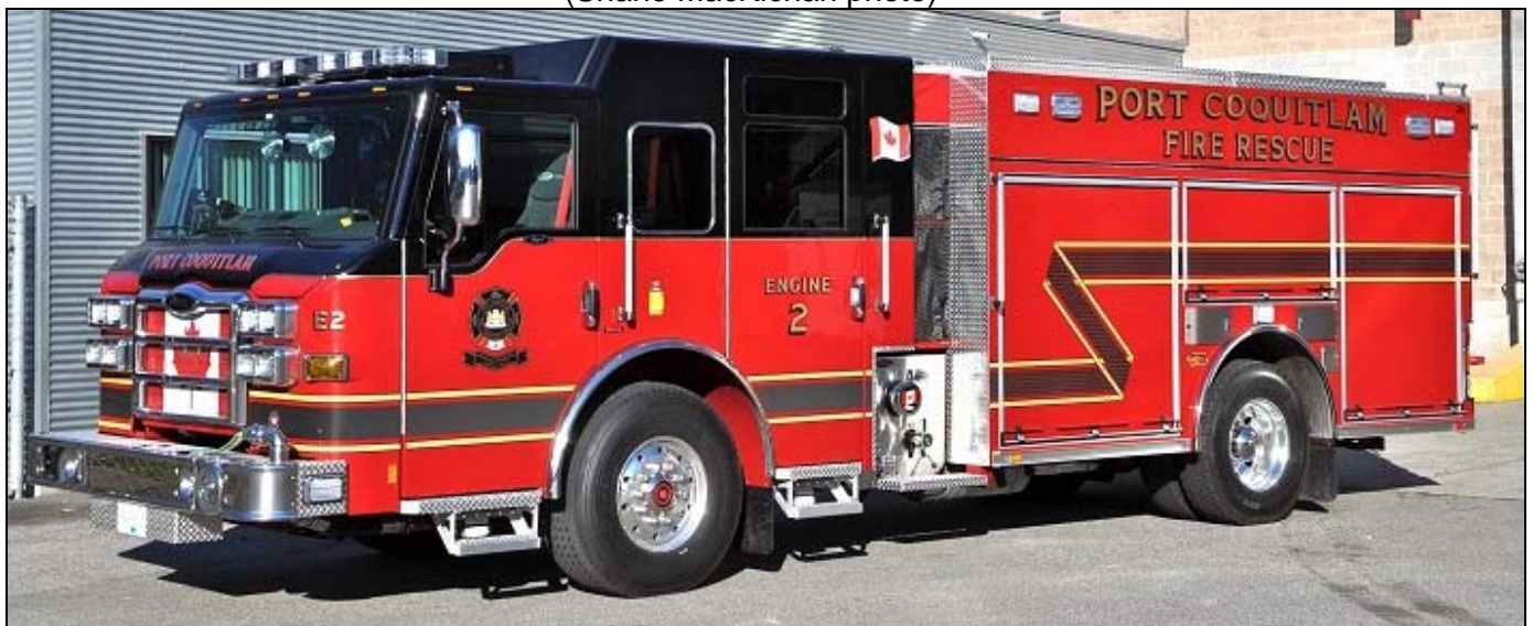
Neighbouring Port Coquitlam received a 2014 Pierce Impel PUC with 1256 gpm pump 440 gallon water and 32gft (Terry Yip photo)
