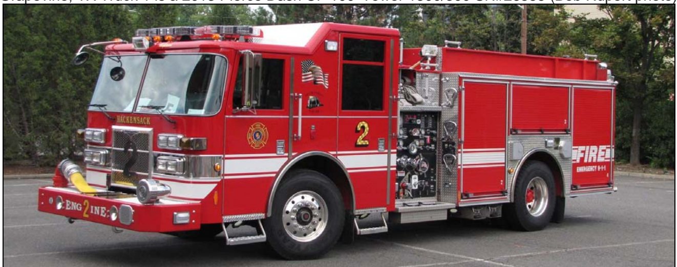
Hackensack, NJ Engine 2.is a 201 Pierce Contender, 1500gpm and 750gwt. (Desmond Brett photo)
