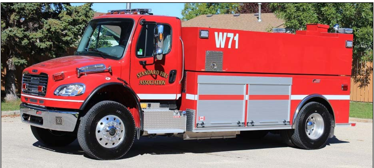
Late last year, Standard, AB accepted this 2014 Freightliner M2-106/Fort Garry Crusader tanker. It has a 420igpm Hale pump and a 2000gwt. Assigned to Wagon 71, it has s/n M566.
