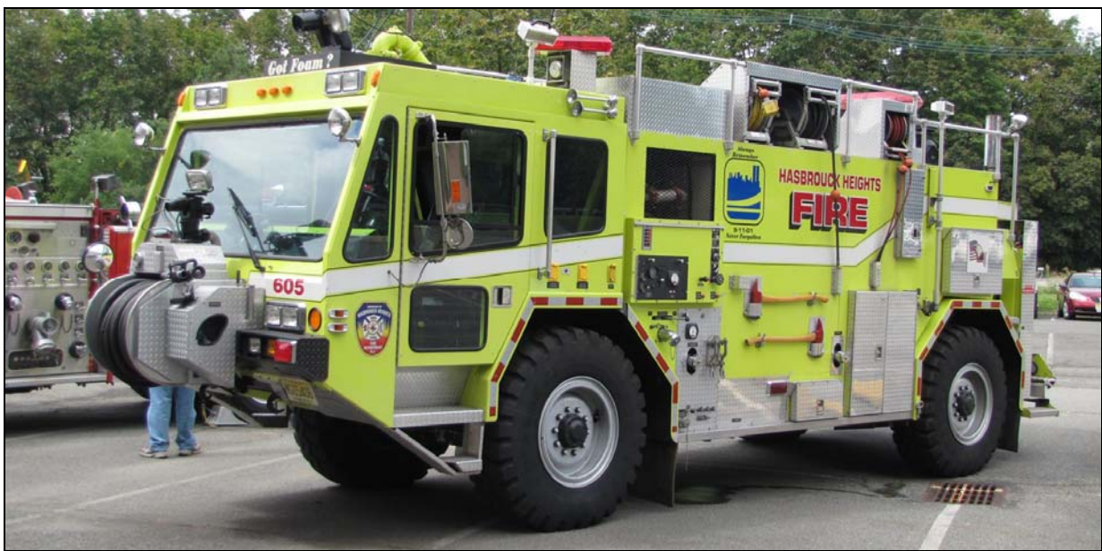
Hasbrouck Heights fire covers.. Airport, in part using this 1996 Walter CRT. Unit 605 has a 1500gpm pump, 1500gwt, 180gft and carries 450lbs of Purple K.
