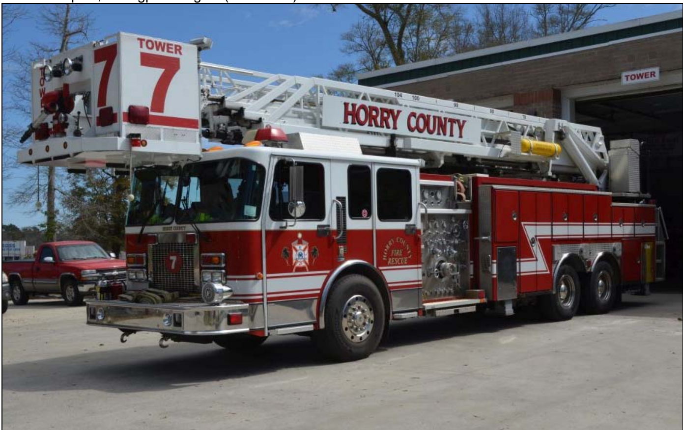
This just in: Bob Rupert, vacationing in Myrtle Beach, SC sent these from the local station in Horry County: Engine 7 is a 2008 Ferrara Intruder, 1500gpm/1000gwt (SN 97389), Tower 7 is a Spartan/Ferrera 104' rearmount quint, 1500gpm/600gwt. (SN 78676)
