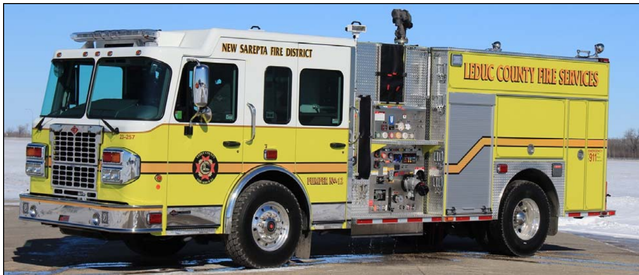
Leduc County, AB just took delivery of this 2016 Spartan Metro Star/Fort Garry pumper for New Sarepta. Pumper 12 has a 1050igpm Darley pump, 1000gwt, 10gft(A) and 25gft(B), s/n 698. An identical truck went to Thorsby, numbered Pumper 10, sn 699. (Dave Stewardson photo)
