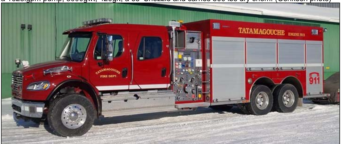
Tatamagouche, NS Tanker 3 is a 2016 Freightliner M2-106/Metalfab rig, with a 1050igpm pump and a 2500gwt. (Metalfab Fire trucks photo)
