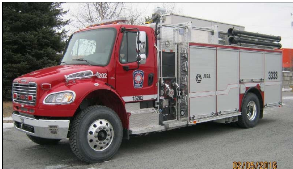
Aluminerie de Bécancour, QC just took delivery of a 2016 Freightliner M2-106/Maxi Métal VIO pumper. Unit 202 came with a 1250gpm Hale pump and a 600gwt. (Maxi Métal)
