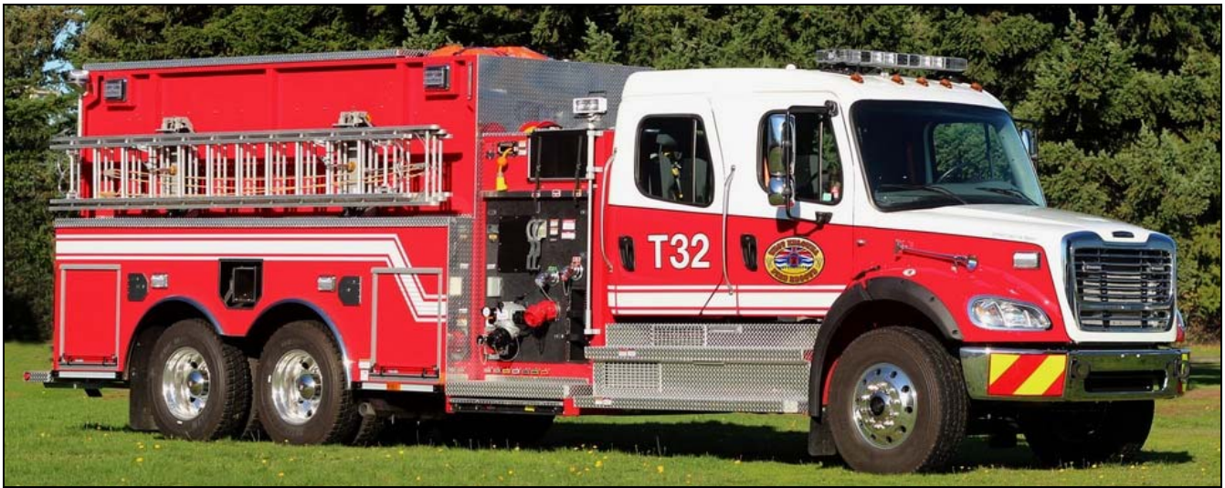
West Kelowna, BC received this 2015 Freightliner M2-112/Smeal rig last year. Tender 32 has a 1500gpm Waterous pump, 2000gwt and Advantus 6 foam system SO 4436 (Shane Mackichan photo)
