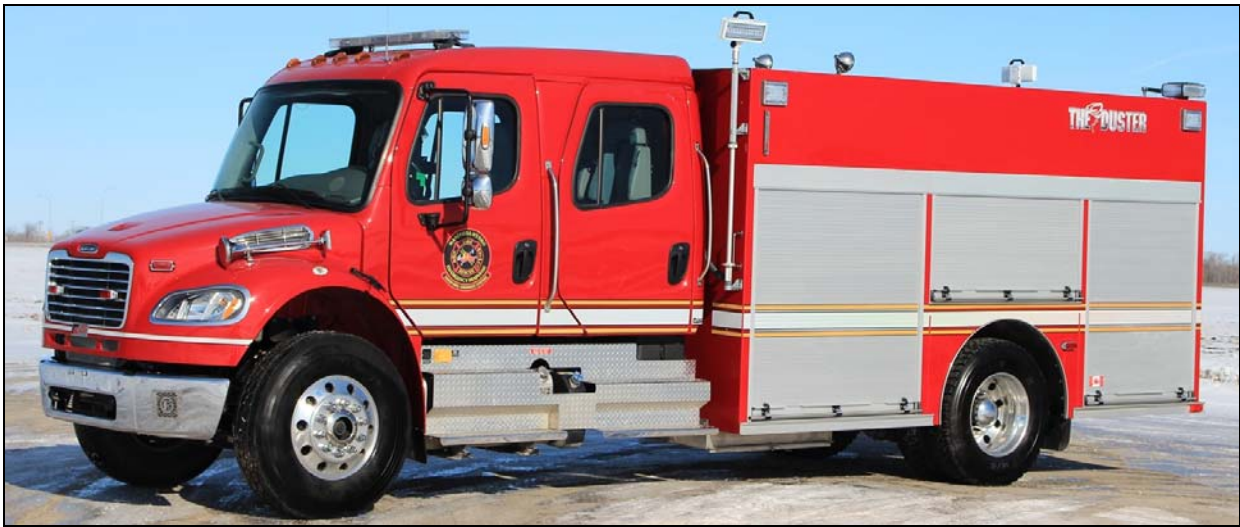
Manitoba Hydro just got this 2015 Freightliner M2-106/Fort Garry Duster pumper with a 1050igpm Darley pump, 800gwt and 25gft(B) for their Dorsey/Riel station. s/n M576. (Dave Stewardson photo)
