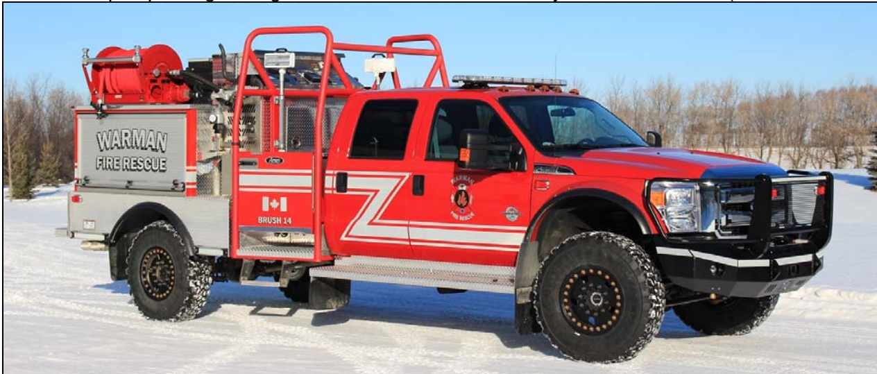
Warman, SK Brush15 is a 2016 Ford F550 4x4/Acres 229igpm Waterous pump, 400gwt and 20gft. It's equipped with an Aquis 1.5 foam system, s/n 160115135. (Dave Stewardson photo)
