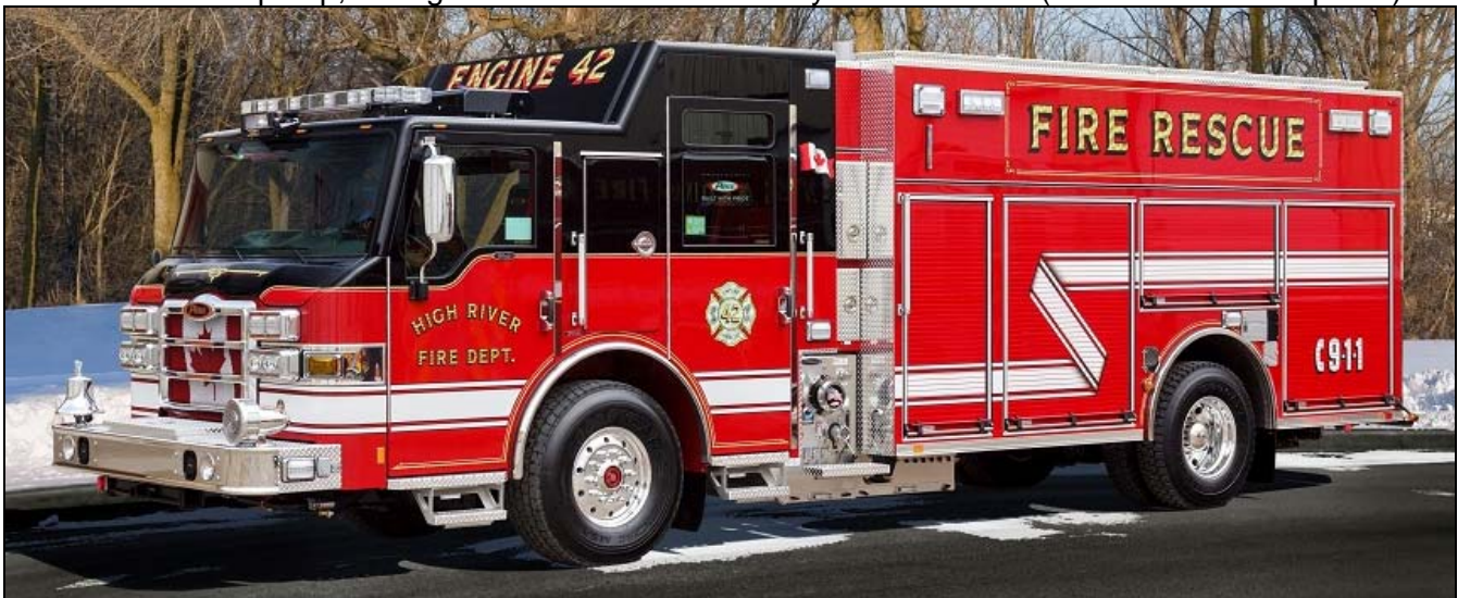
High River, AB recently purchased a 2016 Pierce Velocity PUC pumper, with a 1500gpm Hale pump, 750gwt and a Husky 12 foam system. Engine 42 has serial number 29027. (Pierce Fire Trucks photo)
