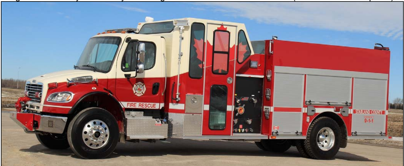
Morrin-Starland County, AB just received a 2016 Freightliner M2-106/Fort Garry pumper with a 1050igpm Darley pump, a1000gwt and a FoamPro 2001 foam system. s/n M650 (Dave Stewardson photo)
