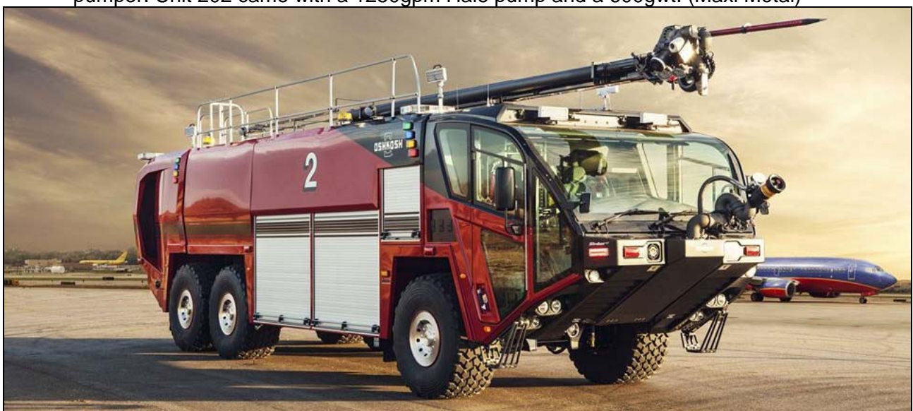
Jean Lesage Airport Red 2 is now running this 2016 Oshkosh Striker 3000 6x6 ARFF unit. It has a 1625igpm pump, 3000gwt, 420gft, a 65' Snozzle and carries 500 lbs dry chem. (Oshkosh photo)
