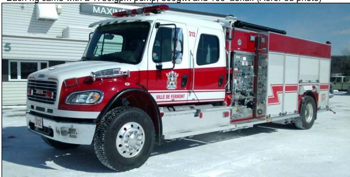
Fermont 312 is a 2016 Freightliner M2-106/Maxi Métal pumper with a 1050igpm Hale pump, 1400gwt, 40gft and CAFS. (Maxi Métal photo)
