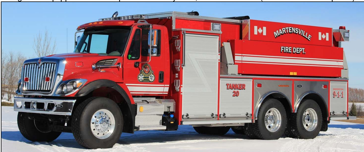
Martensville, SK just purchased a 2016 IHC 7400 6x4/Acres pumper-tanker with an 840igpm Waterous pump and a 2500gwt. Tanker 20 has serial number 160224136. (Dave Stewardson)
