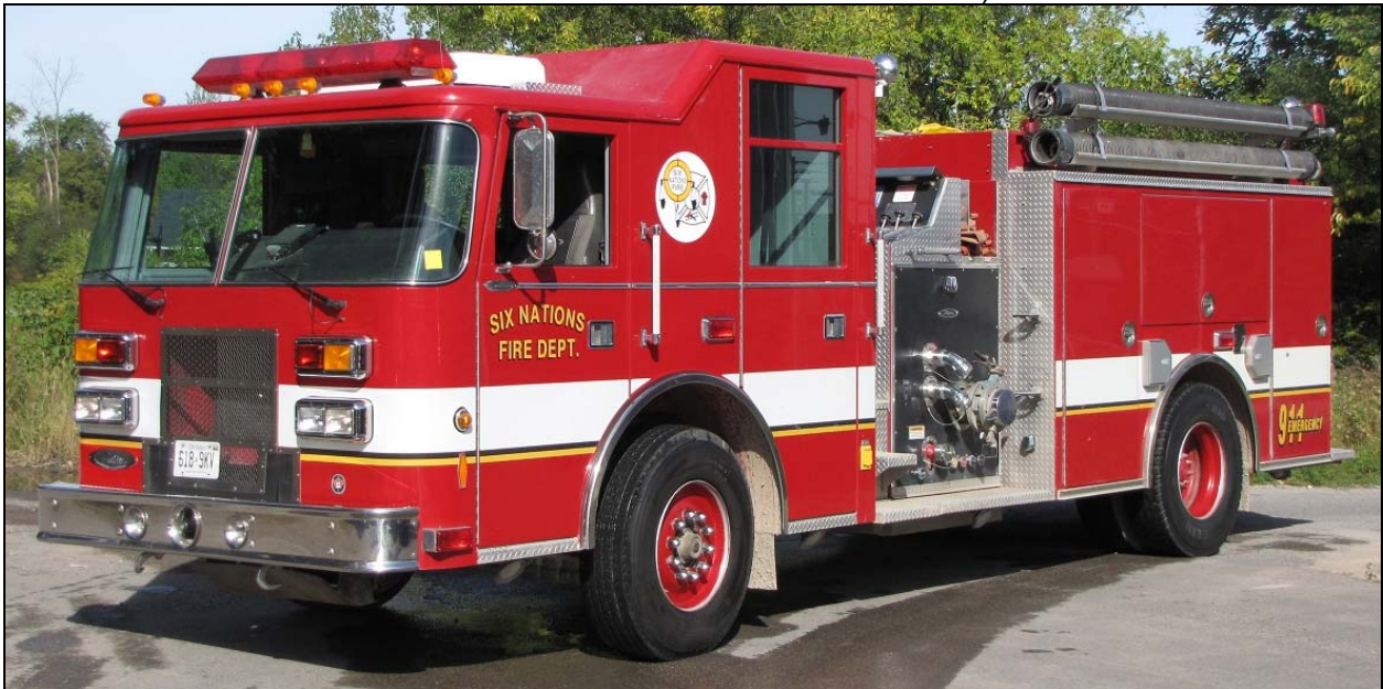
Six Nations Pumper 4 has now returned with a new paint scheme and rehab job. It's a 2002 Pierce Contender with a 1050igpm pump and 800gwt, the old scheme is seen below. (Photos from Ken Buchanan and Desmond Brett)
