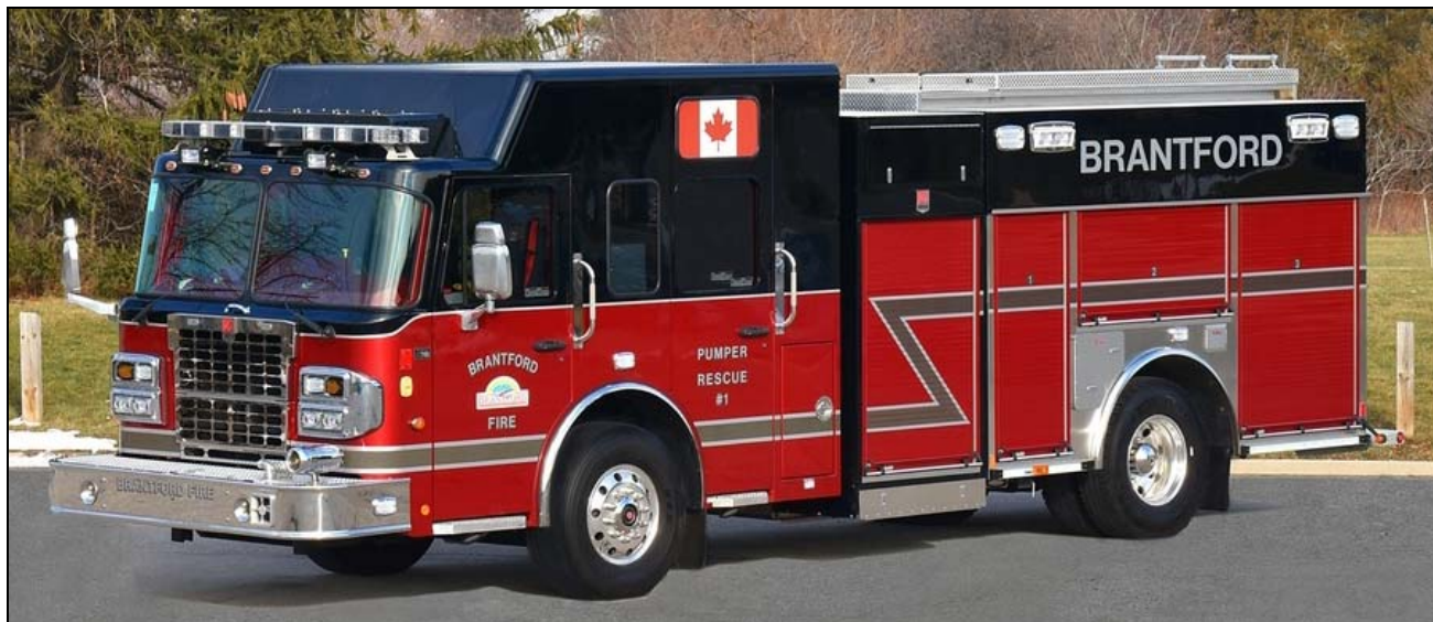
Brantford Rescue Pump 1 is a 2015 Spartan Metro Star/Smeal rig with a 1750gpm Waterous pump, 650gwt and a FoamPro 2001 foam system. s/o 4419. Photo credit: Safetek)
