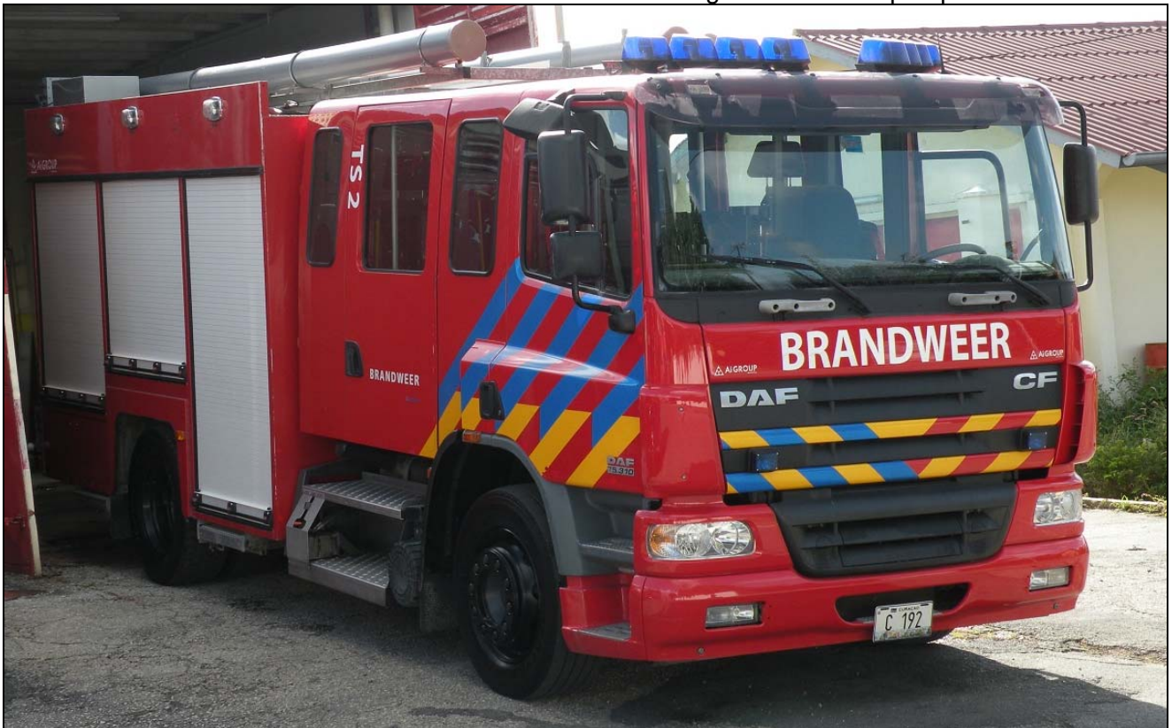
From the Netherlands Antilles, Curacao Fire Service, this an AI Group pump on a DAF CF75 chassis with a 310hp diesel. (Robert Herscovitch photos)
