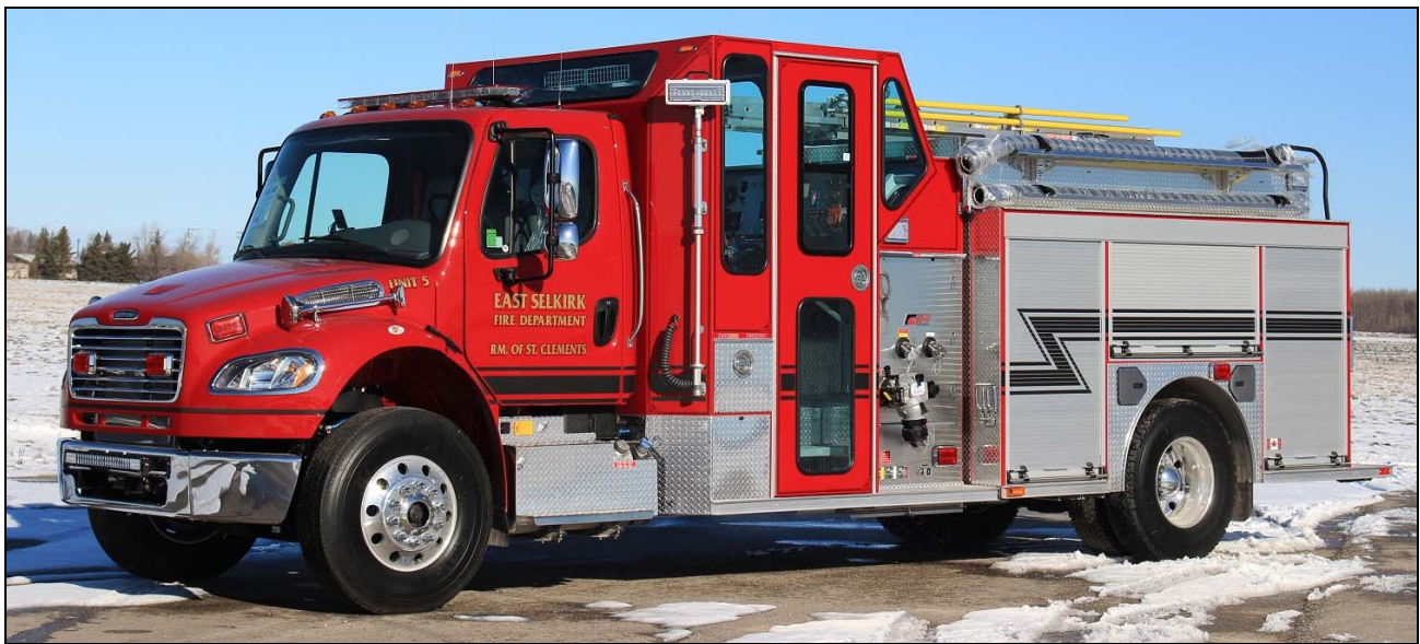
The RM of St. Clements, MB just put this 2016 Freightliner M2-106/Fort Garry rig into East Selkirk as Pumper 5. It has a 1250igpm pump, 1000gwt and 25gft. s/n M740. (Dave Stewardson photo)
