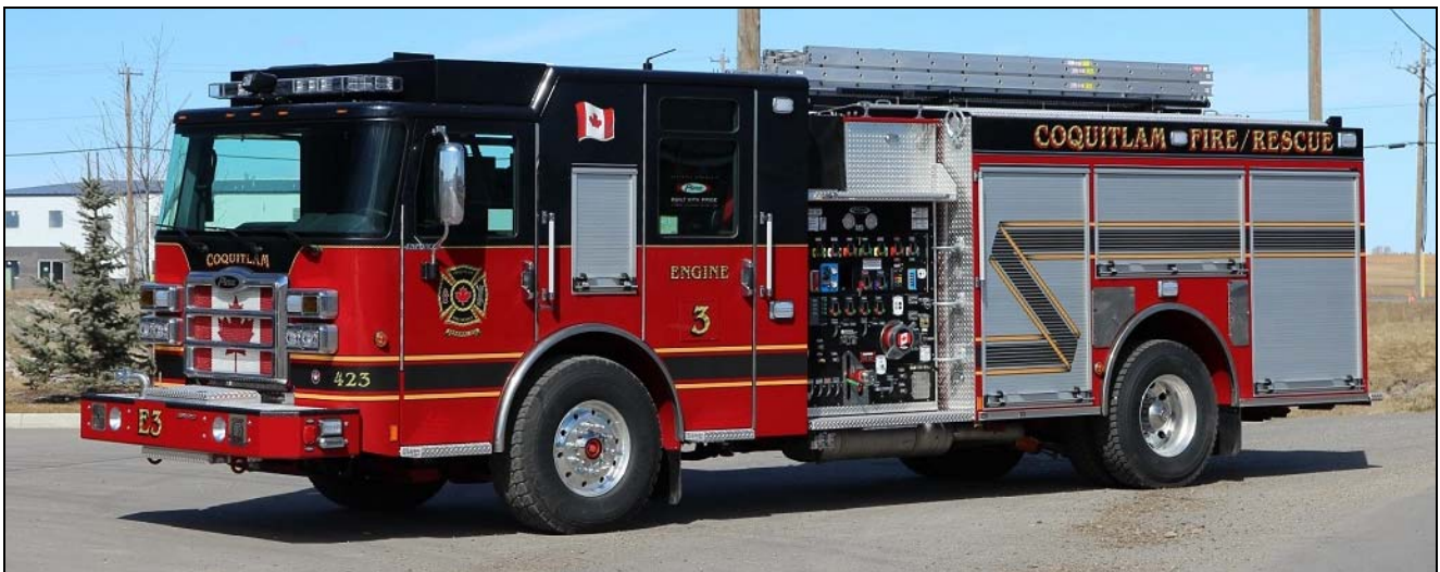
Coquitlam, BC has purchased four of these 2016 Pierce Enforcer pumpers. Each has a 1750 igpm Waterous pump, 500gwt, 50gft, Hercules CAFS and a Husky 12 FS. So 29235 (John Bowerman)
