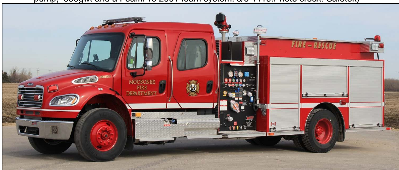
Moosonee, ON now has this 2016 Freightliner M2-106/Fort Garry pump. Pumper 2 has a 1050igpm Hale pump, 800gwt and 25gft(B). It bears job number M745. (Dave Stewardson photo)
