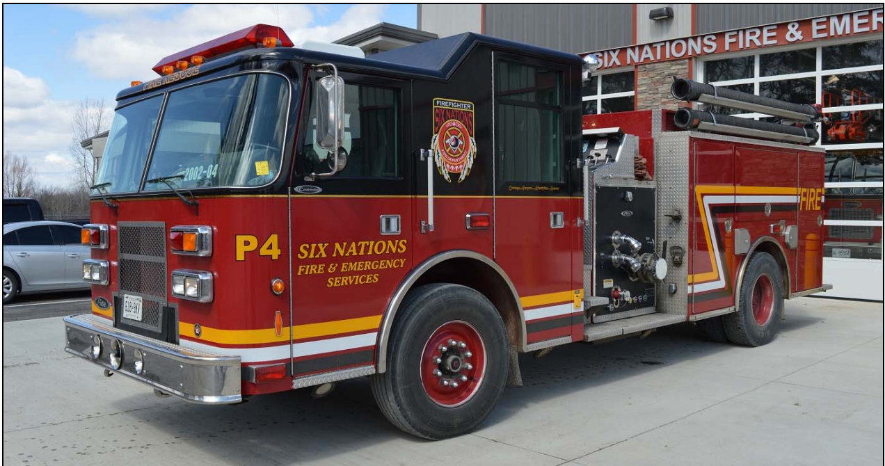
Six Nations Pumper 4 has now returned with a new paint scheme and rehab job. It's a 2002 Pierce Contender with a 1050igpm pump and 800gwt, the old scheme is seen below. (Photos from Ken Buchanan and Desmond Brett)
