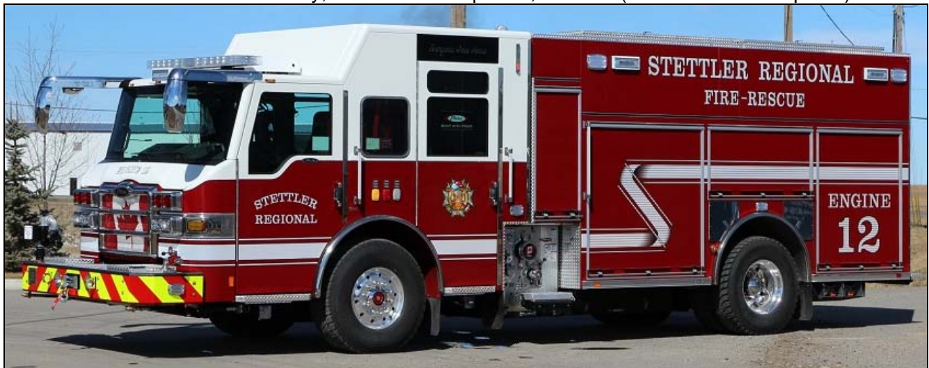
This month, Stettler, AB got a 2016 Pierce Velocity pumper with a 1250igpm Pierce pump, 625gwt, 15gft(A) and 25gft(B) with a Husky 12 foam system for E. 12. sn 29003 (John Bowerman photo)
