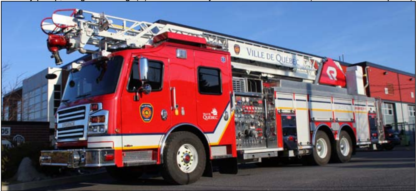
Quebec City now has three of these 2015 Rosenbauer Viper quints on Commander 4000 chassis. Each rig came with a 1750igpm pump, 300gwt and 100' aerial. (AeroFeu photo)
