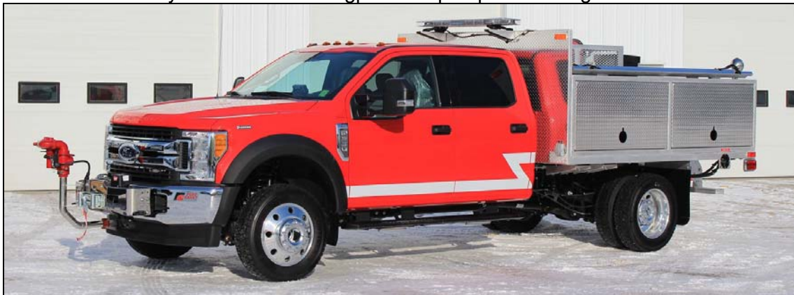
Rosebud, AB took delivery of this 2017 Ford F550 4x4/Fort Garry Cougar brush unit in the spring. It has a Darley portable pump, a 333igwt and an 8gft. s/n M788 (Dave Stewardson photos)
