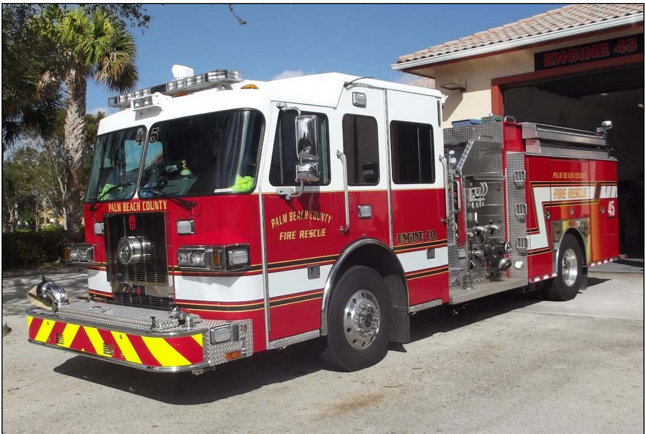
Palm Beach County, FL Engine 45, a 2013 Sutphen, 1500gpm/600gwt (Rick Loiselle photos)
