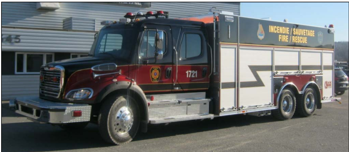
Saint-Armand 1721 2016 Freightliner M2-112/Maxi Métal 1500gpm(H)/2000gwt/30gft
