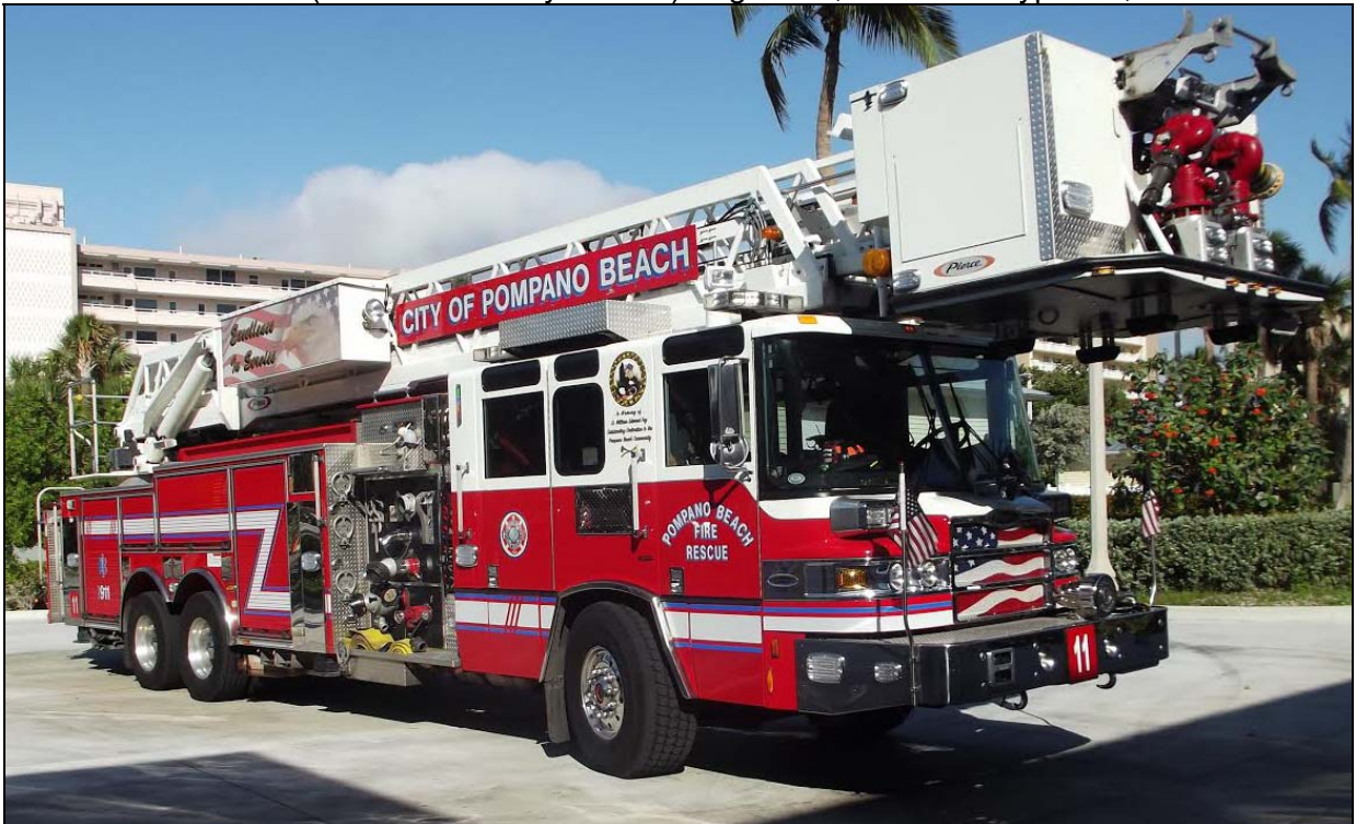
Pompano Beach Truck 11, a Pierce Quantum 100' platform, 1500gpm, 300gwt.
