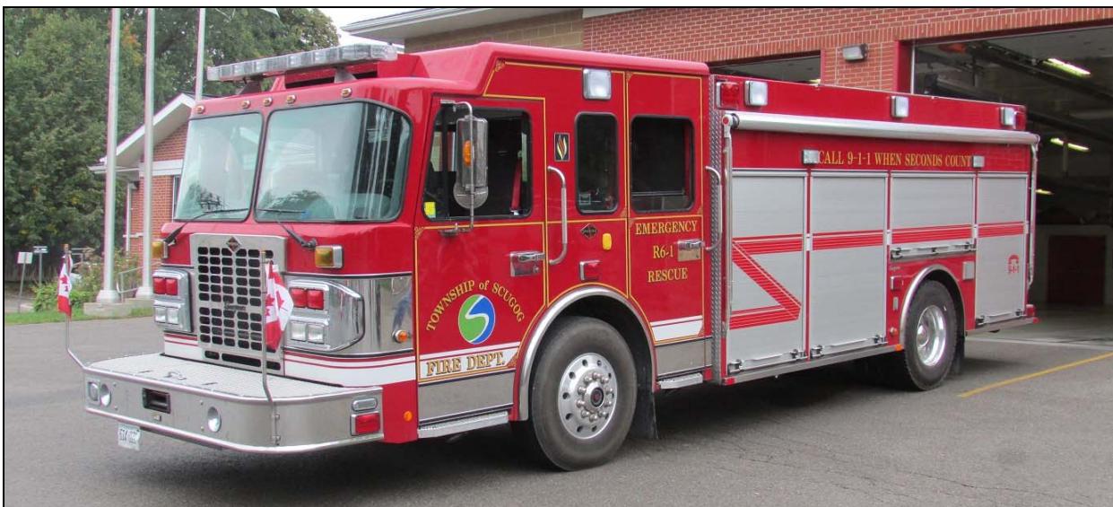
Pumper 6-1, a 2008 Spartan Metro Star / Fort Garry, 1050igpm/1000gwt/25gft. S#A622
