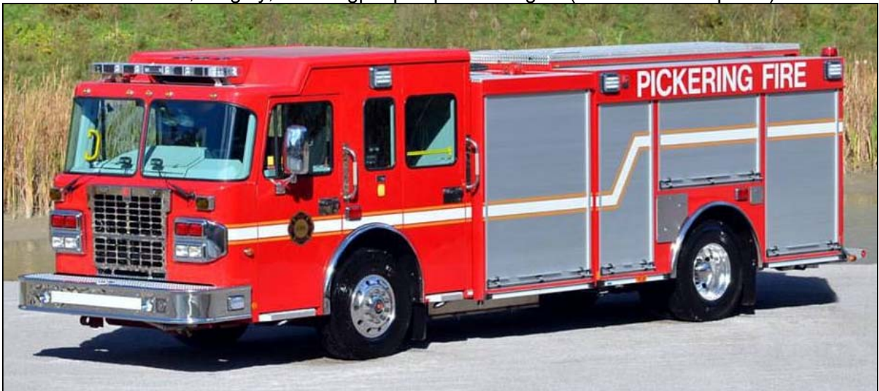
Pickering runs this 2015 Spartan Metro Star/Smeal engine as Pump 56. It was purchased through Safetek. It sports a 1500gpm pump, 500gwt and 20gft. Also a FoamPro 2002 foam system. It has s/o number4394. (Safetek photo by Jeremy Cohen)
