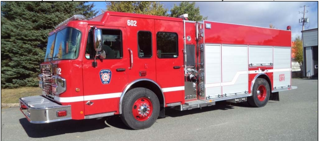
A recent addition to Oka, QC, Unité 602, a 2016 Spartan Gladiator/Maxi Métal pumper with a 1500gpm Hale pump and a 1650gwt. (Maxi Métal photo)
