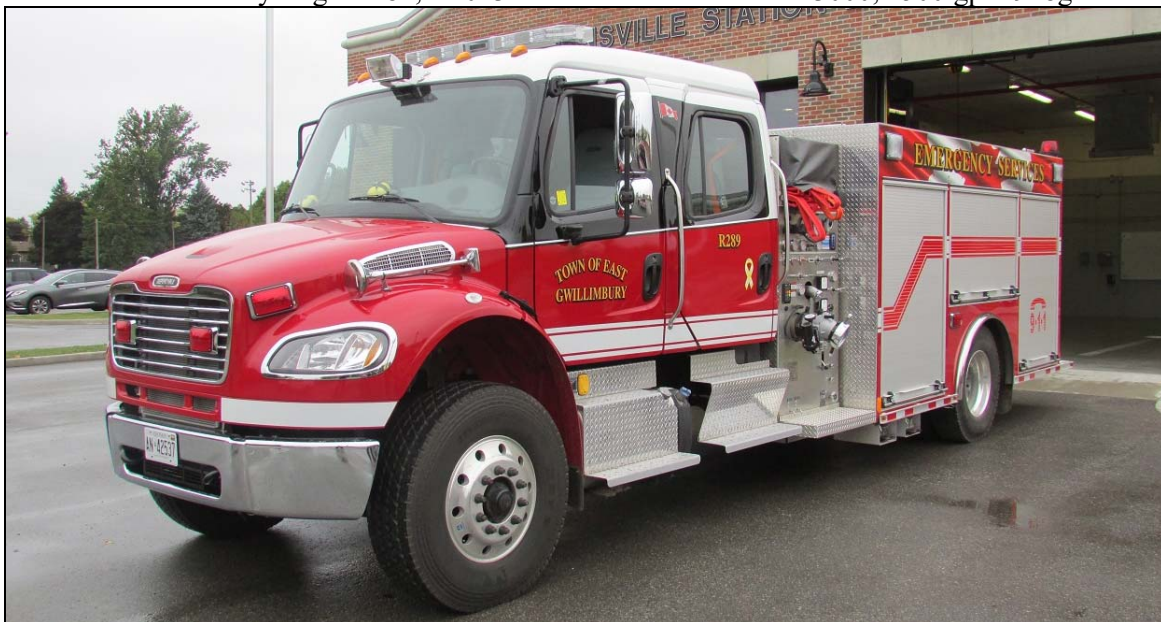
E. Gwillimbury Rescue 289, 2016 Freightliner M2/DEV Rescue Pumper, 1050igpm/790gwt. (Desmond Brett photos)
