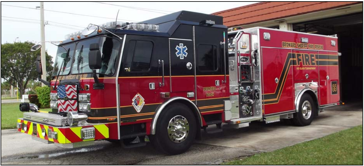
Deerfield Beach ( Broward County Sheriff ) Engine 66, an E-One Typhoon, 1500/600.
