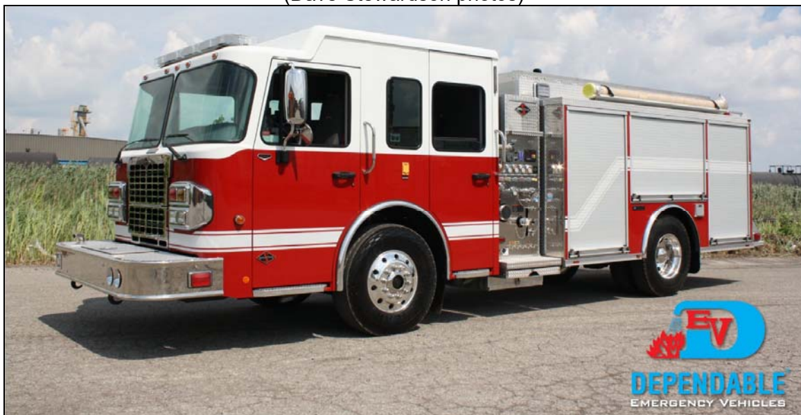
Cape Breton, NS got this 2016 Spartan Metro Star/Dependable pumper last summer, with a 1500gpm Hale pump and a 1000gwt. (Dependable Emergency Vehicles)
