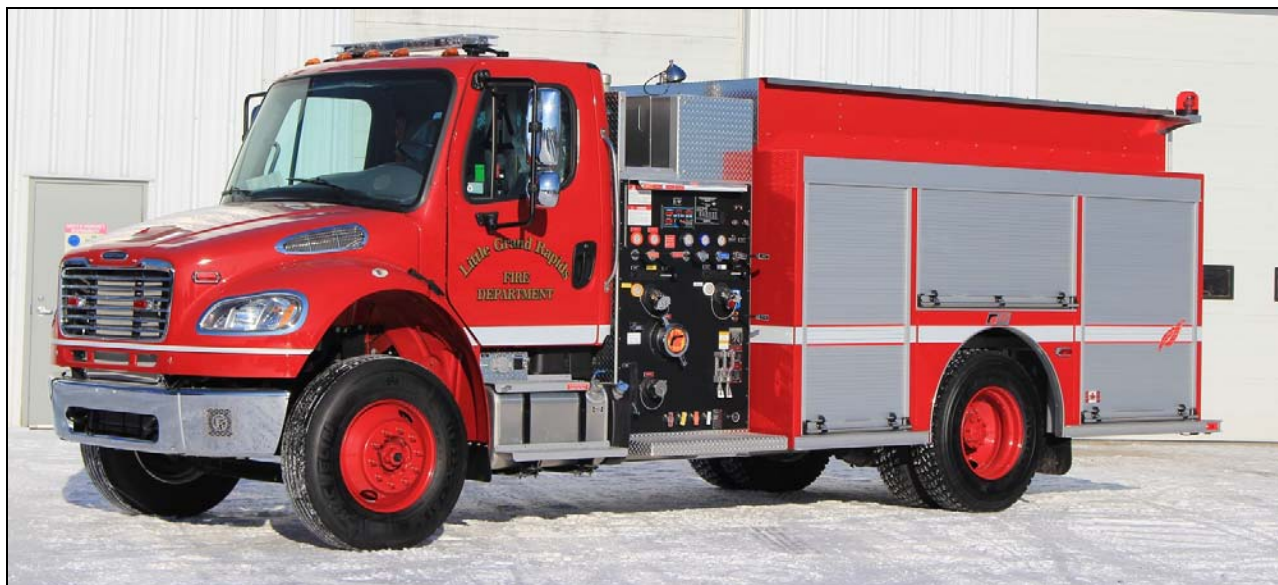
Little Grand Rapids, FN, MB recently took delivery of this 2017 Freightliner M2/Fort Garry pumper. It has a 1050igpm Hale pump, an 800gwt and a 25gft. s/n M703 (Dave Stewardson photos)
