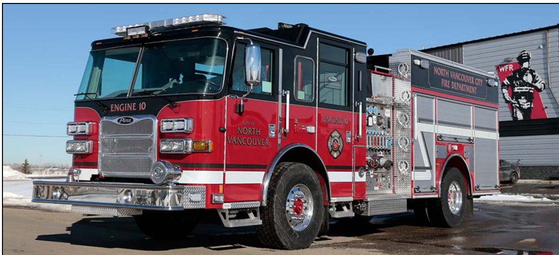
New to North Vancouver, BC. Engine 10 is a 2016 Pierce Arrow XT pumper, 2000gpm, 400gwt, 30gft and a Husky 3 foam system. (Photo: Wholesale Fire & Rescue)
