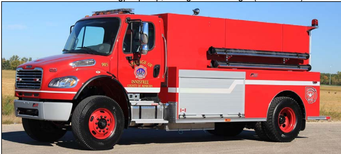
Innisfree, MB (Minburn Cnty) Tender 905, a 2016 Freightliner M2-106/Fort Garry tanker with a 420igpm Darley pump and 2000gwt. s/n M738 (Dave Stewardson photo)
