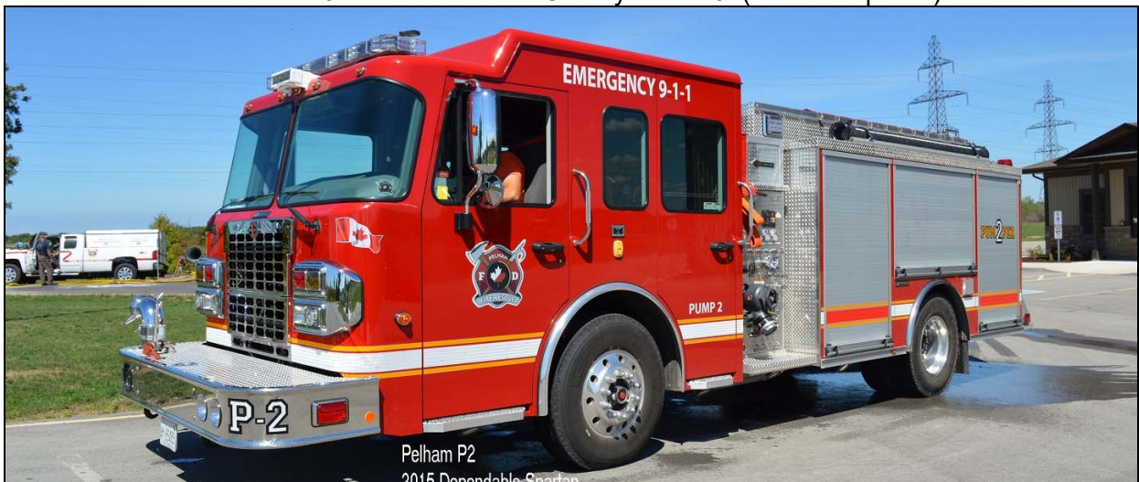
Pelham received this 2015 Spartan/Dependable rig late last summer, it was previously a demo truck. It has, roughly, a 1050igpm pump and 775gwt. (Ken Buchanan photo)
