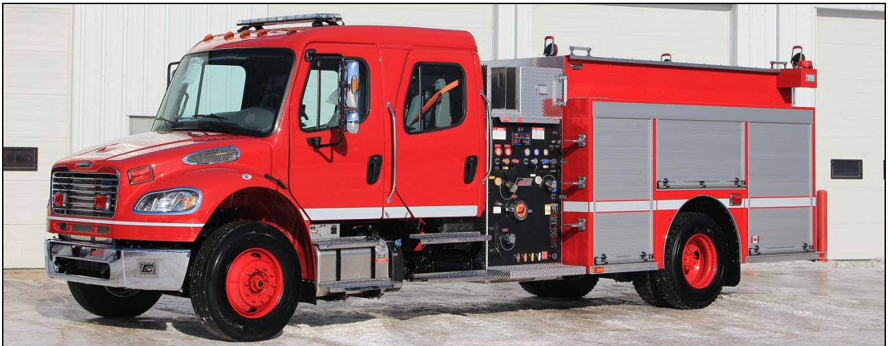
Argyle, ON recently received this 2017 Freightliner M2/Fort Garry engine, with a 1050igpm Hale pump, 800gwt and a 25gft. s/n M812
