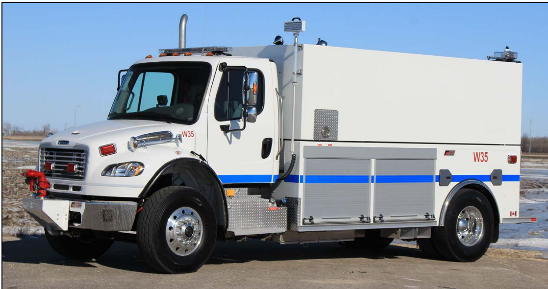
Gleichen (Wheatland County), AB just received Wagon 35, a 2017 Freightliner M2/ Fort Garry tanker with a 420igpm Hale pump and 2000gwt s/n M765
