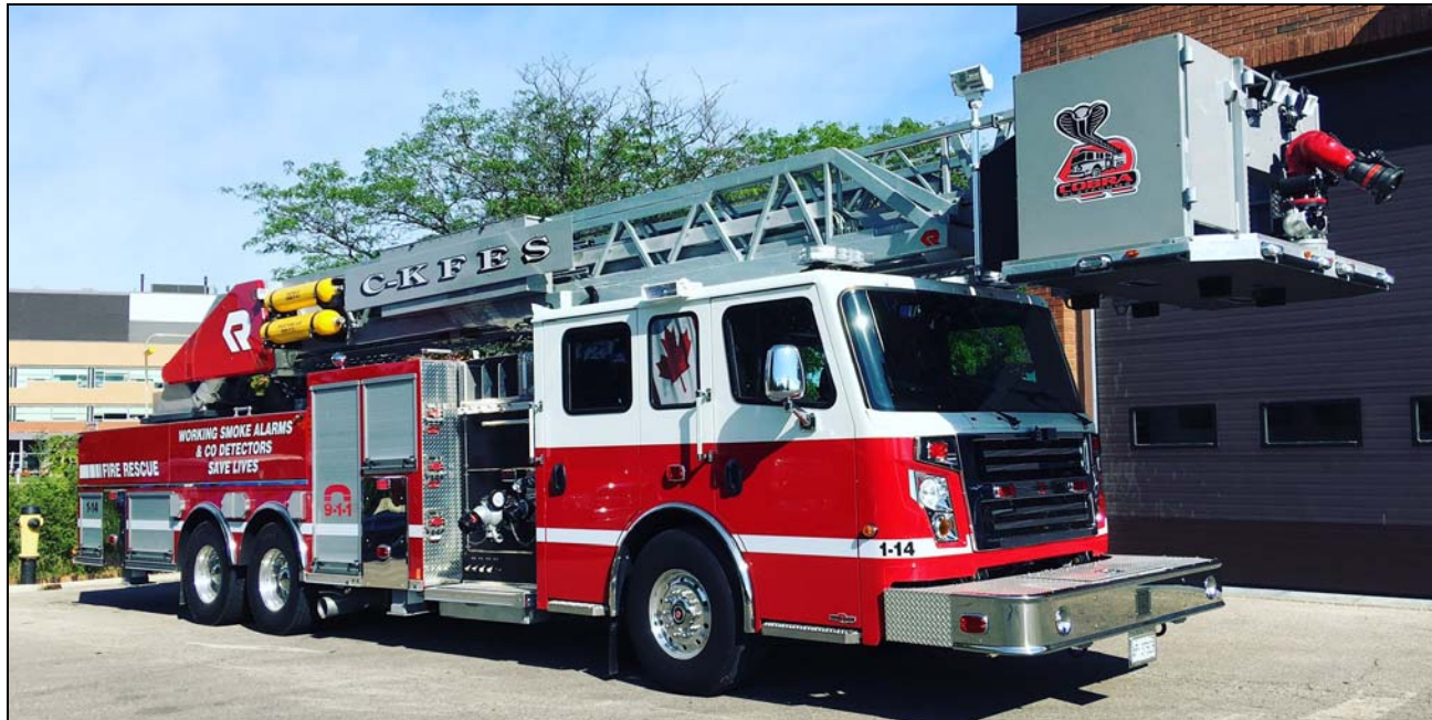
Chatham-Kent 1-14 2016 Rosenbauer Commander 1666igpm/430gwt/101' Cobra tower. This was a stock unit customized for the CKFES, it's assigned to Chatham. SN7417
