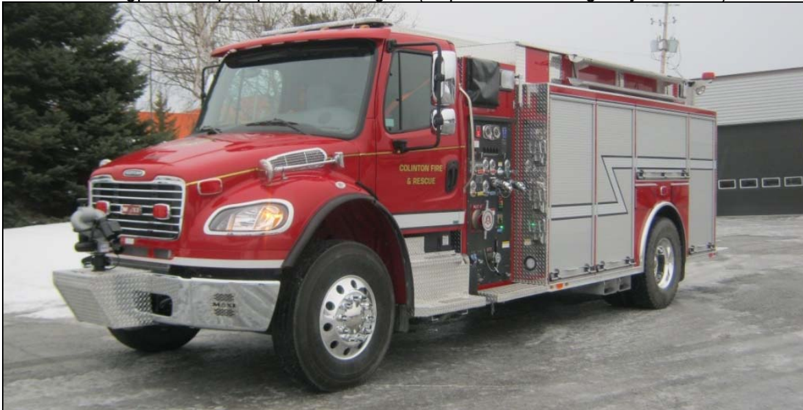
Colinton, AB recently got this 2017 Freightliner M2-106//Maxi Métal pumper-tanker. It came with a 1050igpm pump, 1670gwt and a 20gft. (Maxi Métal)
