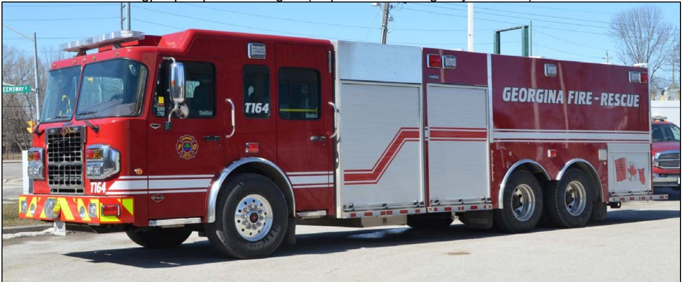
Just delivered to Georgina is a 2017 Spartan Metro Star/Spartan ERV/Dependable pumper-tanker equipped with a 1250igpm pump and 2517gwt. (Bob Rupert photo)
