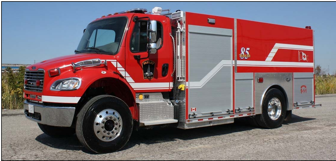
Paisley, ON bought this 2015 Freightliner M2-106/DEV for Tanker 85. It has a 1000gpm Hale pump and a 2500gwt. (Dependable Emergency Vehicles)
