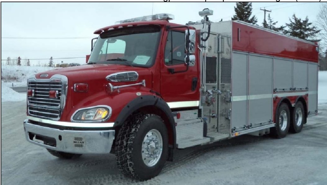
Whitcourt, AB 2017 Freightliner M2-112/Maxi Métal 1250igpm(H)/2500gwt/30gft (MMFT)
