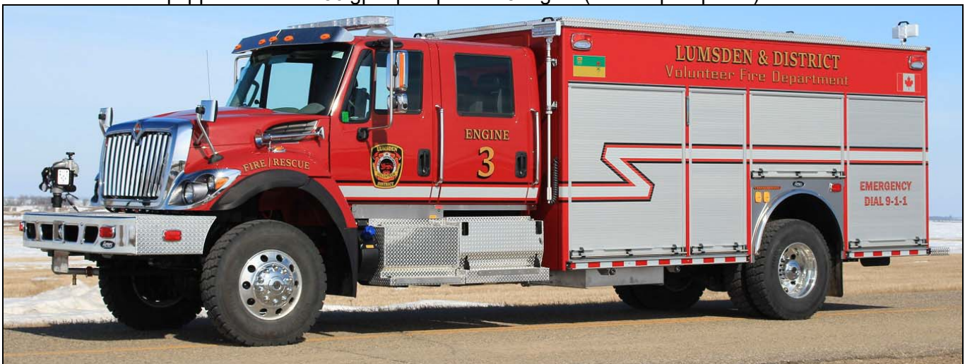
Lumsden, SK Engine 3 now has a 2017 IHC 7500/Acres, 1050igpm(W)/800gwt/25gft. s/n170224150 (Dave Stewardson photo)
