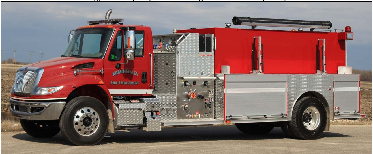
Miminigash, PEI just took delivery of this 2017 IHC 7500/Fort Garry engine. It has a 1050igpm pump, 1500gwt and 25gft. s/n #M784 (Top & bottom photos: Dave Stewardson)
