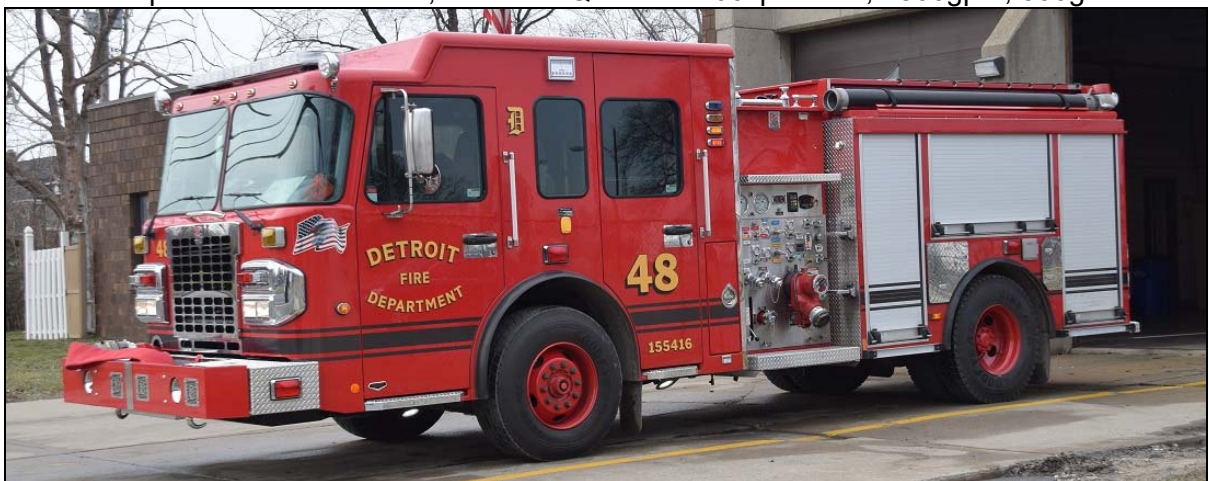
Detroit's newest engines, 2016 Spartan/Smeal rigs, have 1500 gpm pumps and 500gwts. They are assigned to Engines 9, 17, 32, 39, 40, and 48. (Dan Jasina photo)
