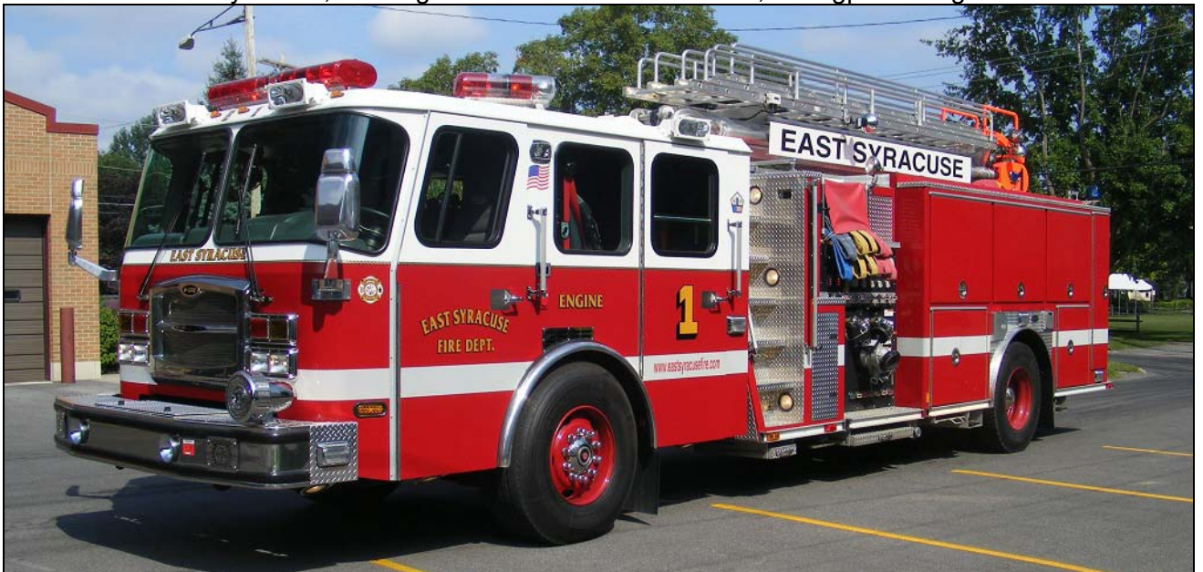
East Syracuse Engine 1 is a 2009 E-One, 2000gpm/1000gwt/65 foot.
