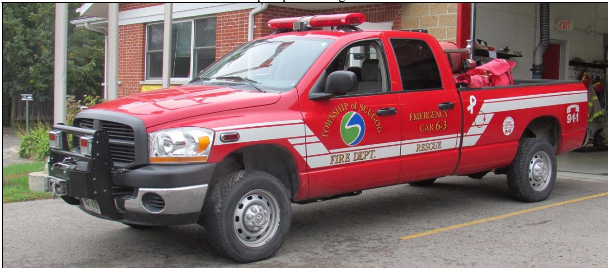
Scugog Twp., Car 6-3, 2006 Dodge Ram brush truck, portable pump and 200gwt.
