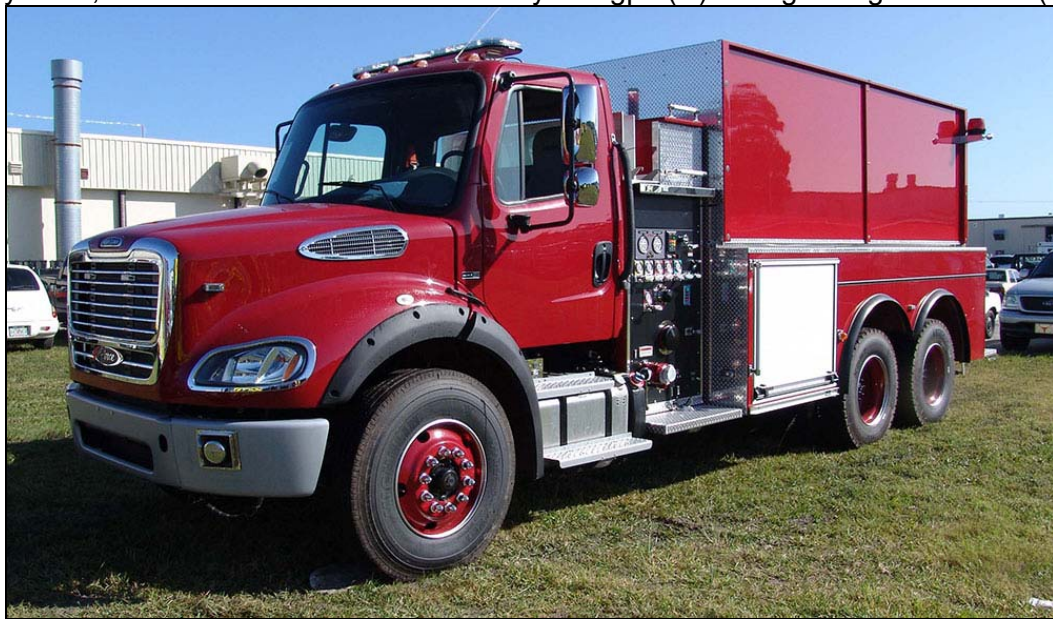
Lesser Slave Lake, AB put this 2015 Freightliner M2-106/Pierce tanker in service in Flatbush. Tender 151 has an 840igpm Hale pump and a 2500gwt. (WFR)
