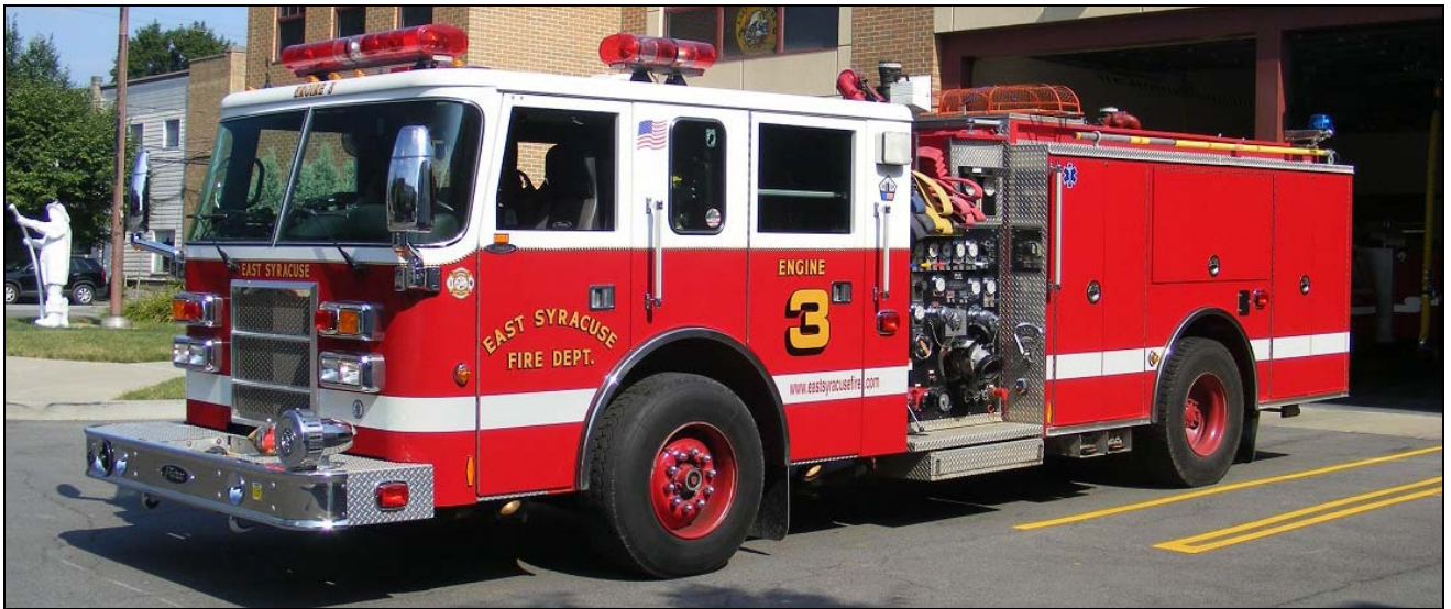
East Syracuse, NY Engine 3 is a 2000 Pierce Dash, 1750gpm/1000gwt.
