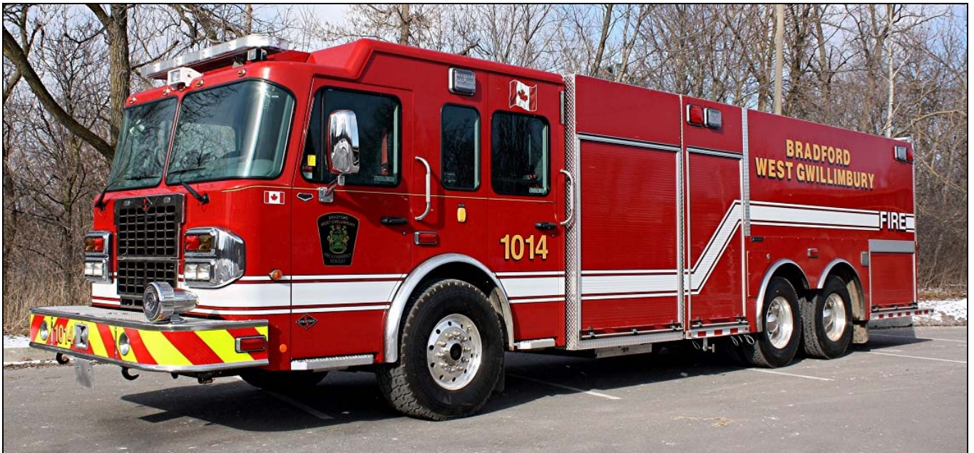
Bradford-W. Gwillimbury 1014 is now running this 2017 Spartan/ERV/DEV pumper tanker, 1500gpm pump and 3000gwt. (Dependable Emergency Vehicles)
