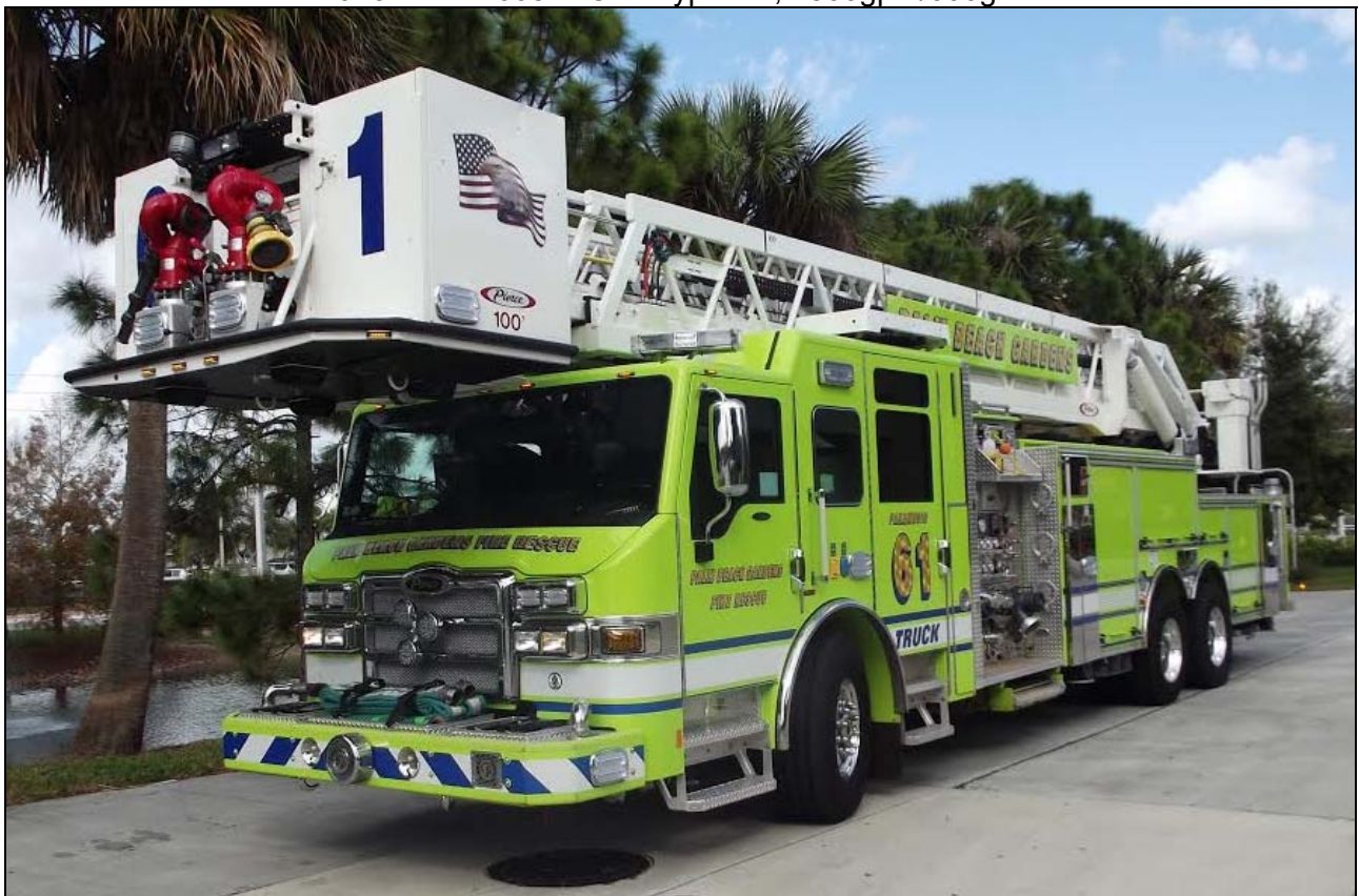
Palm Beach Gardens Truck 61, a Pierce Velocity tower, with a 2000gpm pump, 300gwt and a 100' platform. (Rick Loiselle photos)
