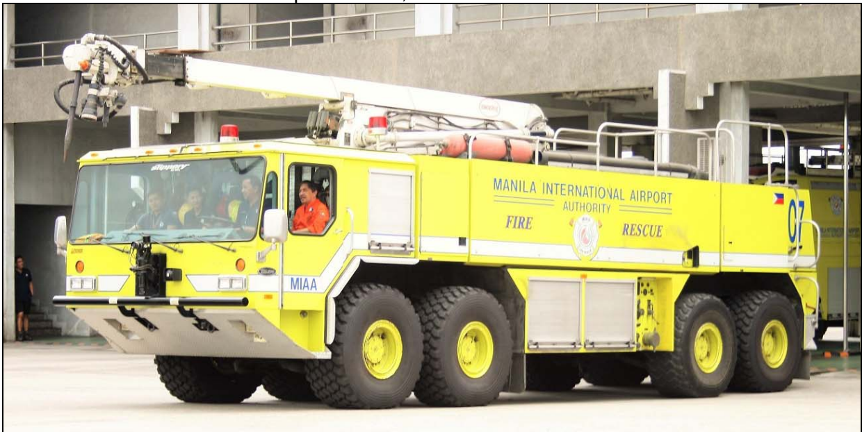
07 is a circa 2007 E-One Titan 8x8 HPR with 50' Snozzle S/N 19575.
