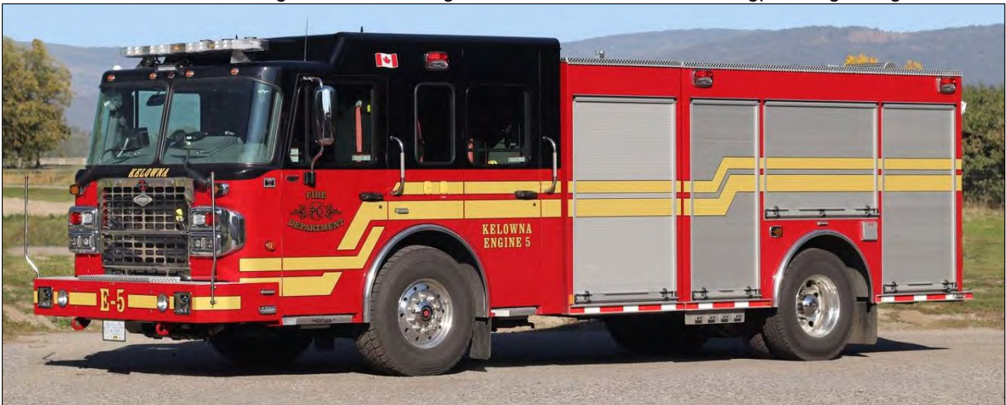
Kelowna, BC Engine 5 is a 2019 Spartan Gladiator/Hub product with a 1250igpm pump, 500gwt and 40gft. SO#1257 (Shane MacKichan photos)
