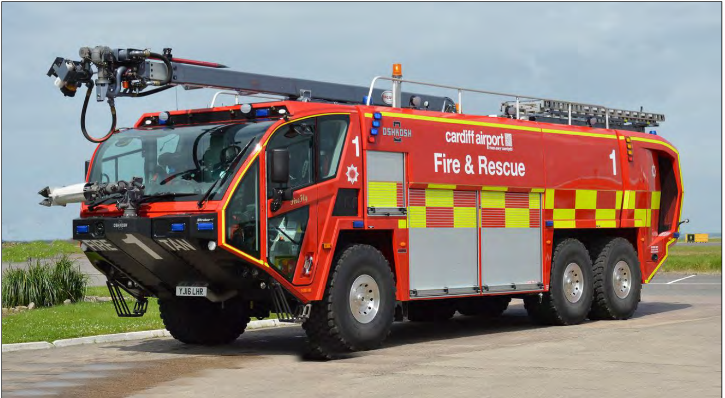
One of three Oshkosh Strikers from Cardiff Airport in Wales, delivered in 2016. Red 1 is a model 3000, with an 11,340L water tank and a 1,600L foam tank. They were purchased through Terberg DTS UK.
