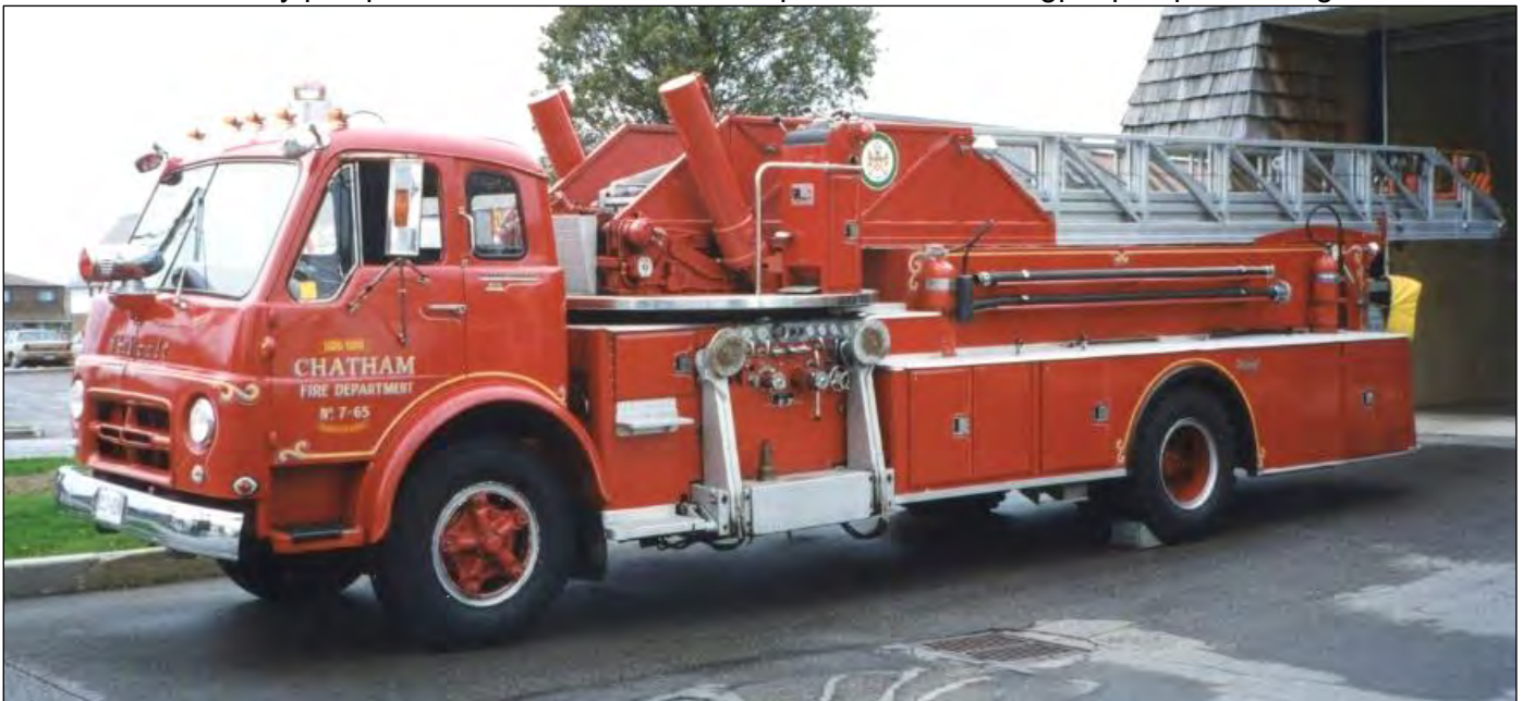
Aerial duties were split between Unit 7, a 1965 International/Thibault 100' aerial with a 250igpm pump, and Unit 9 (Next page)
