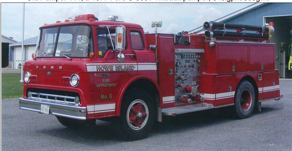
Old Pumper 6, a 1976 Ford C-900 / Pierreville pumper, 840igpm/600gwt
