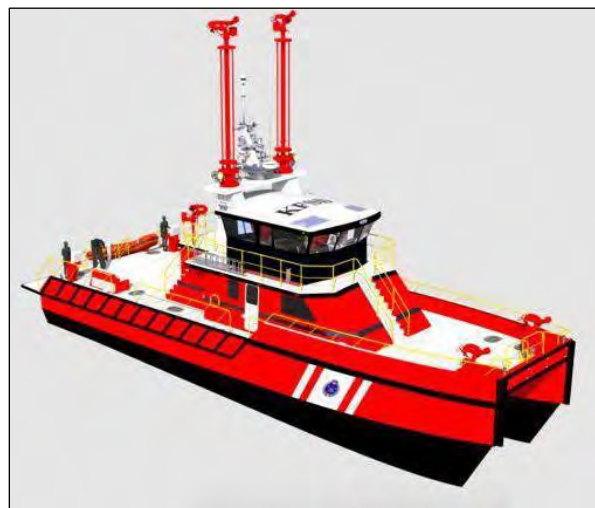
Drawings of the proposed craft, with extendable turrets down and up. The 82' FireCat should be in service next year. (Workboat.com)
