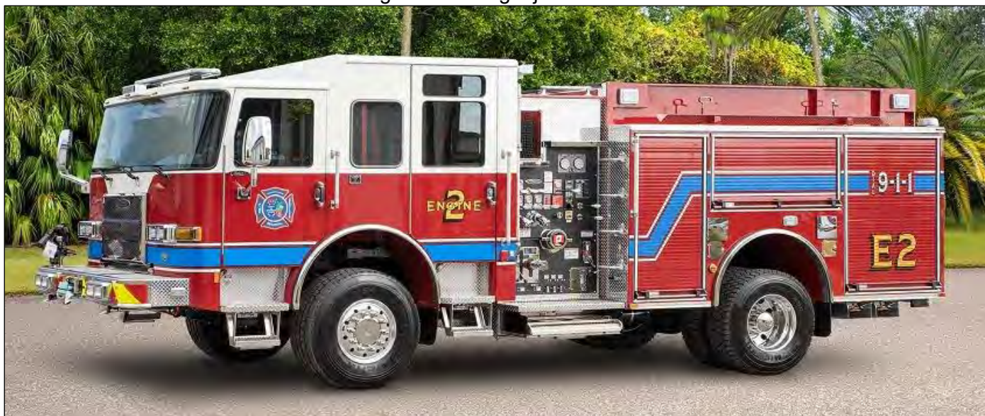
Northern Lights, AB Engine 2, a 2020 Pierce Saber 4x4 with a 1500igpm Waterous pump, a 750gwt and a Husky 3 foam system, j/n 33997. (pierce Fire Photos)
