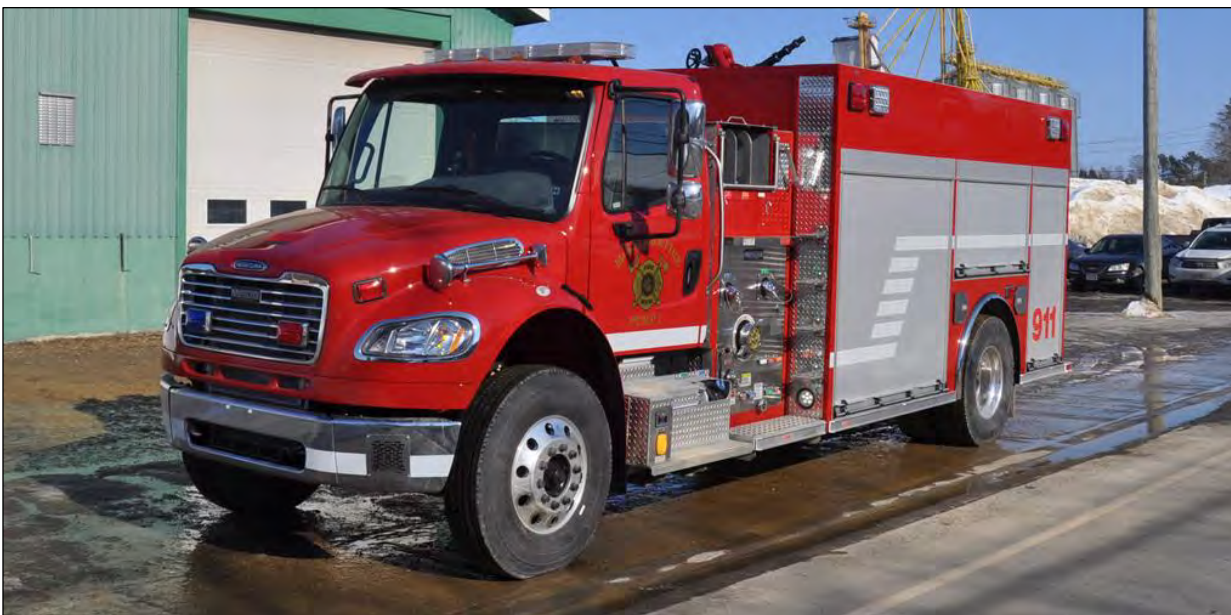
McKellar, ON P. 1, a 2020 Freightliner M2-106/Metalfab pumper-tanker has a 1050igpm Waterous pump, 1500gwt and a FoamPro 1600 foam system. (MetalFab Fire Trucks Photo)
