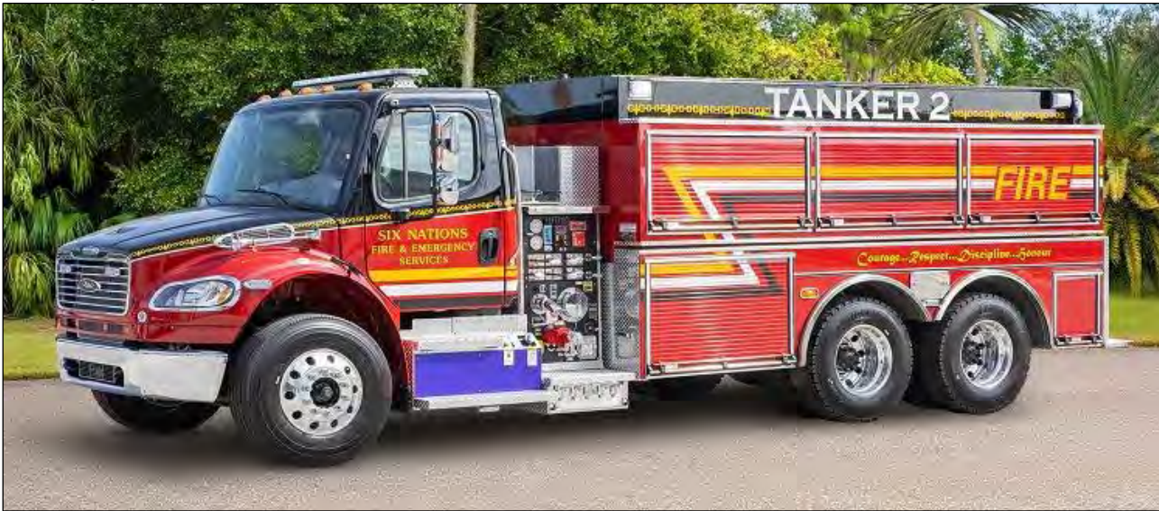
Six Nations, ON Tanker 2, one of two new 2020 Freightliner M2-106/Pierce pumper-tankers. They have 1000gpm Hale pumps, 3000 gwt and Husky 3 foam systems, SN 34200 (Pierce Fire photo)
