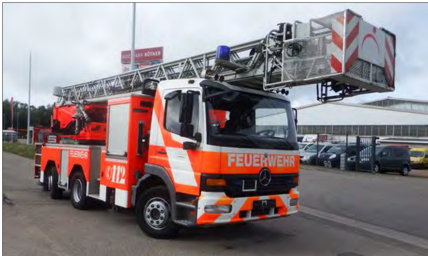
A slightly later model of the DLK23-12 aerial ladder mounted on a 2001 Mercedes Atego 1228 6x2 chassis with front and rear steering axles. (Truck1.NL photo)
