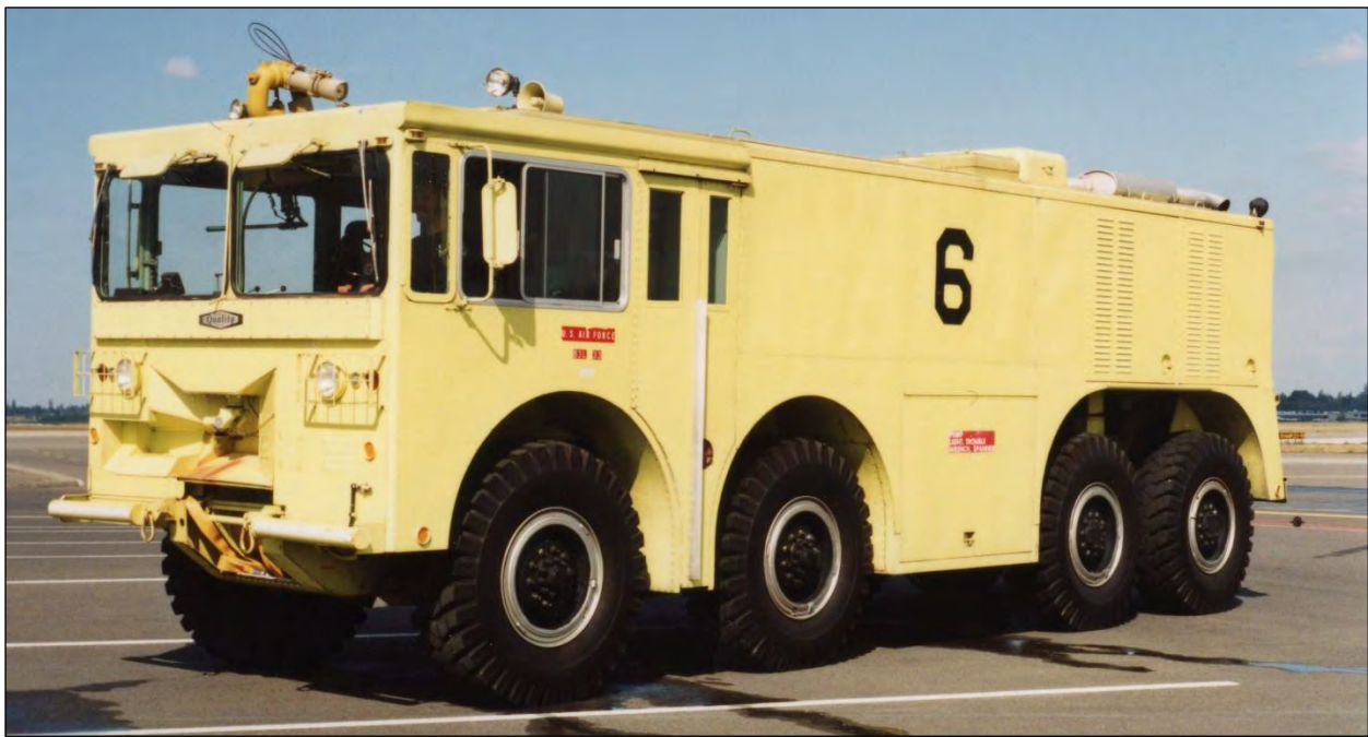
One of the 1962 FWD P-2 CFR rigs, this went to McChord Air Force Base. Red 6 was a 1962 FWD P-2 that underwent a 1983 Quality rebuild, equipped with a 1400gpm pump, 2300gwt and 200gft.
