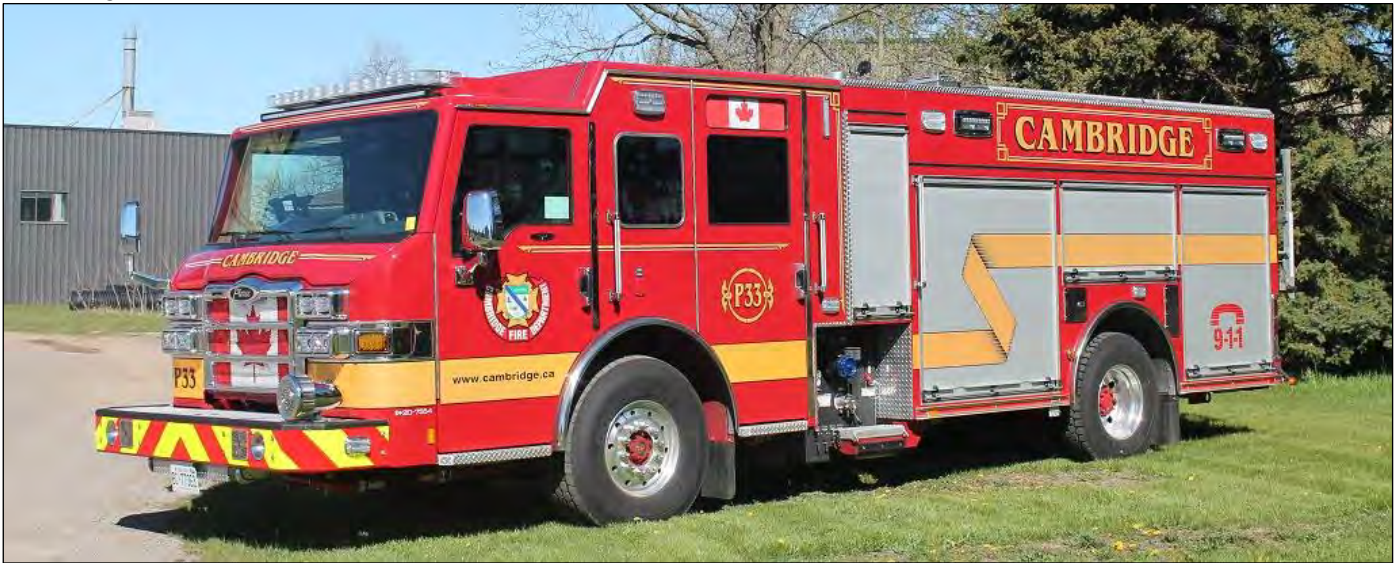
Recently in service in Cambridge is this 2020 Pierce Impel rig, Pumper 33 has a 1250igpm pump, 542gwt and 20 gft, serial no. 34256 (Gary Dinkel photo)
