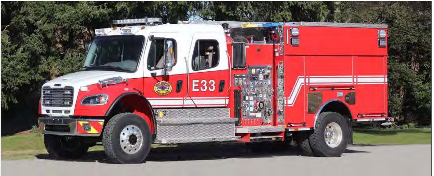
West Kelowna, BC Engine 33, 2019 Freightliner M2-106 4x4/Smeal 1050igpm/800gwt/40gft
