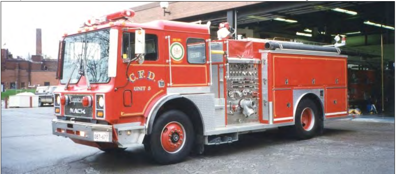
Station 1's first-away pump was this 1988 Mack MC/Superior with a 1050igpm pump and 500gwt.
