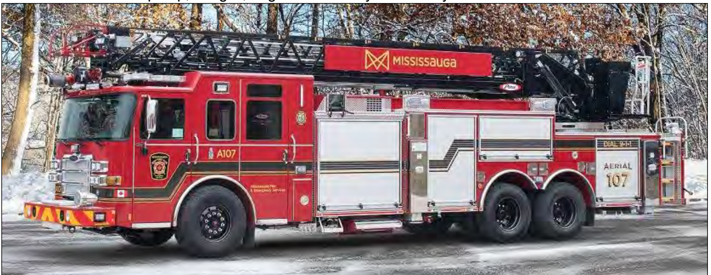
New for Mississauga Aerial 107 is a 2020 Pierce Enforcer Ascendant 2000igpm Hale pump, 400gwt and 107' stick. It also has a Husky 3 foam system. SN 33850 (Pierce Fire Apparatus photos)
