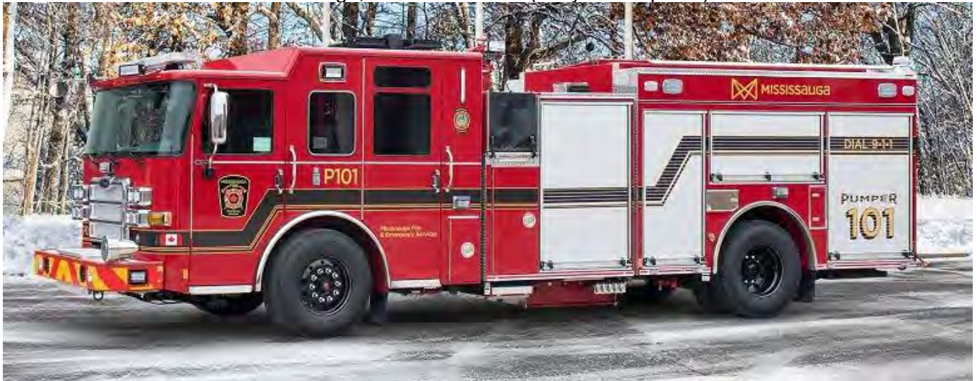
Mississauga, ON Pump101 now has this 2020 Pierce Enforcer pumper equipped with a 2000gpm Hale pump, 600gwt, 50gft and a Husky 3 Foam System. SN 32848.
