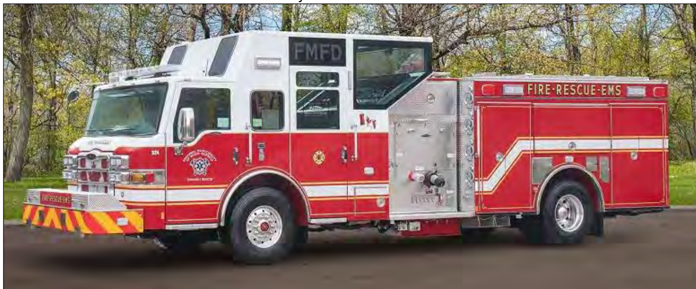
RM of Wood Buffalo, AB Engine 324 is a 2020 Pierce Velocity FR 8426 with a 1500igpm Waterous pump, 540gwt and a 42gft. j/n 34207-01.
