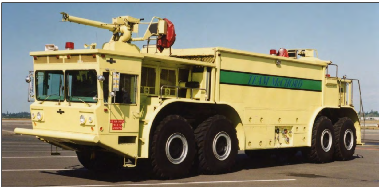
McChord AFB also had this 1988 Oshkosh P-15 CRT, it had twin 1250gpm pumps, a 6100gwt and a 515gft, all stats in U.S. gallons. (Photos by Dan Goyer)
