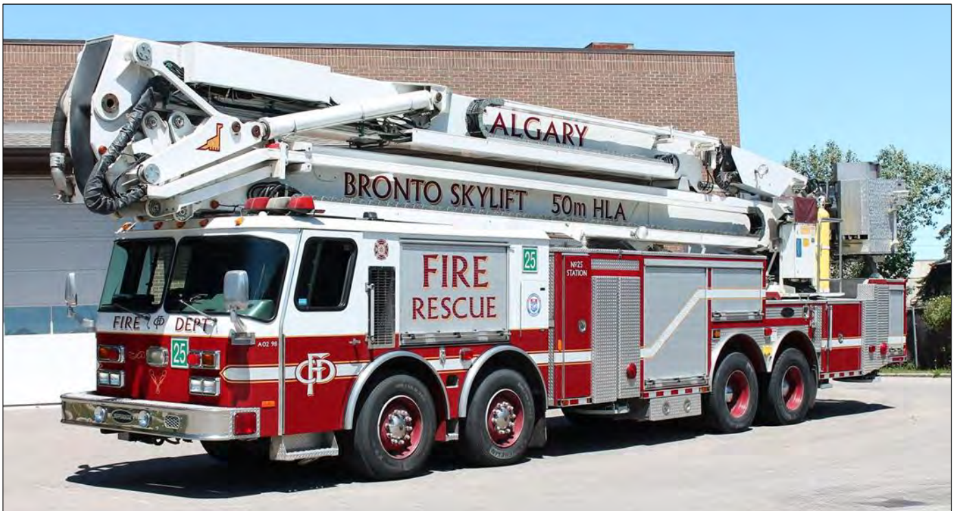
Calgary's 1998 E-One Hurricane/Superior/Bronto 50m HLA model with dual steer front axles. (Dan Goyer)
