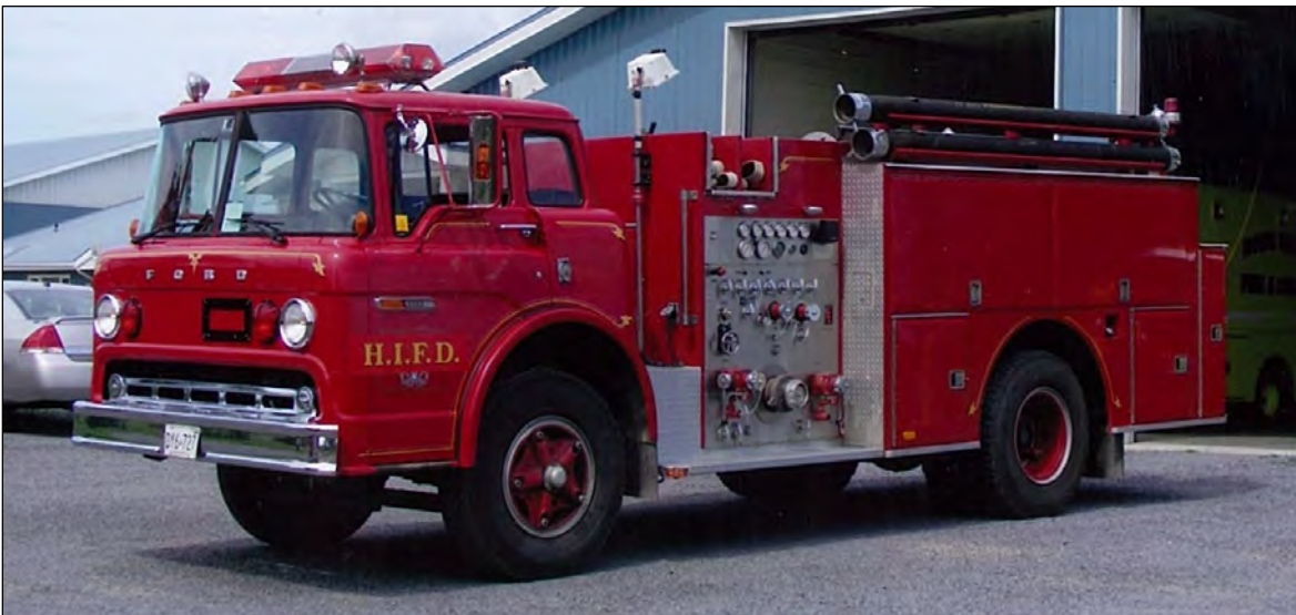
Old Pumper 111, a 1977 Ford C-900 / Thibault pumper, 840igpm/800gwt.
