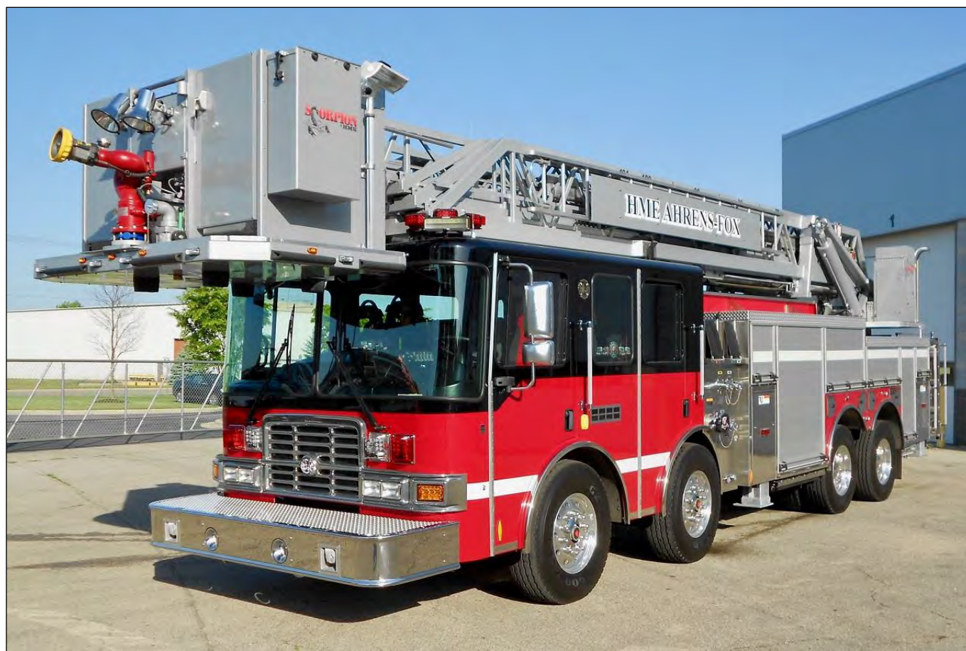
THE HME demonstrator purchased by West Nipissing in 2016 is a 2012 HME 1871 Spectre equipped with a 1500gpm pump, 500gwt and a 104' tower. (HME photo)
