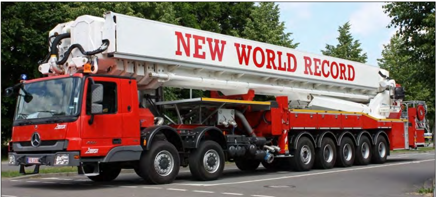
The Bronto F112HLA, at 112m or 335', on a 2010 Mercedes Benz Actros chassis. (Rosenbauer photo)
