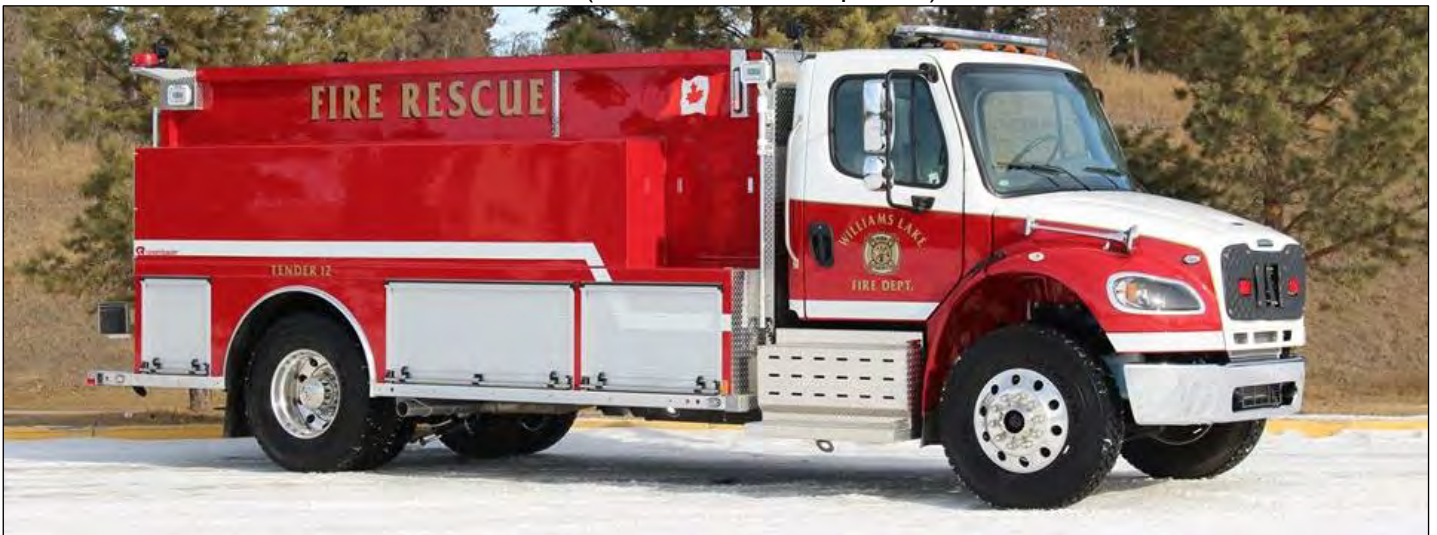
Williams Lake, BC Tender 12 now has a 2020 Freightliner M2 106/Rosenbauer rig, 840igpm/1500gwt.
