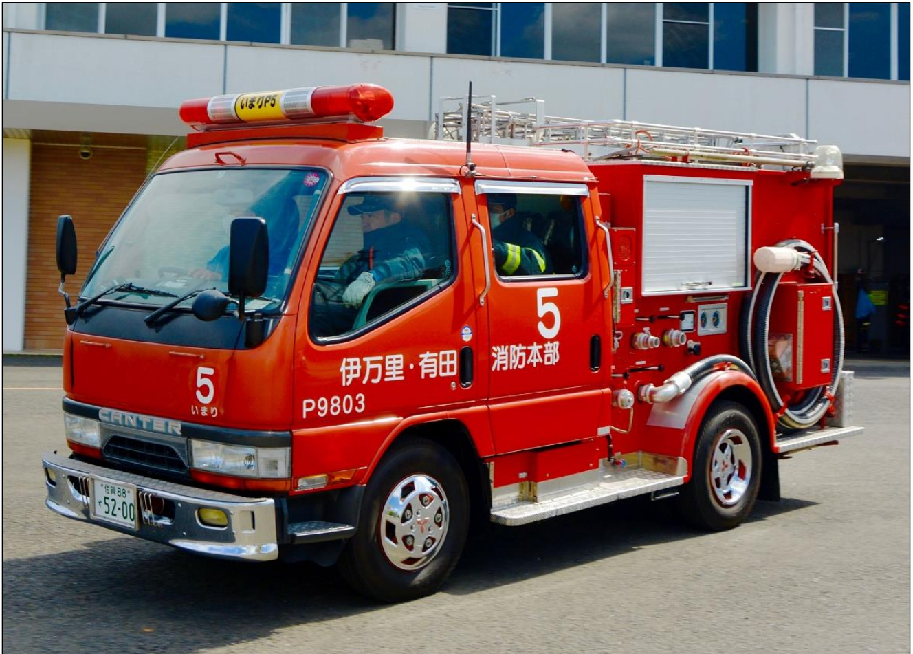
Imari-Arita's Pump 5, a Mitsubishi Canter equipped with a small tank. This is the smallest pumper, generally first away as it can respond quickly to almost any area.
