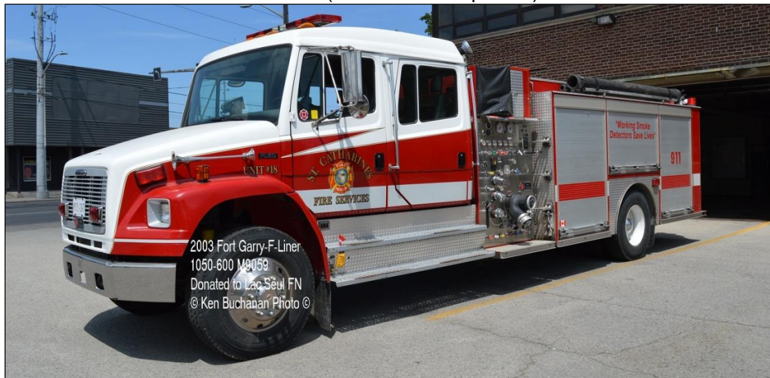
Turns out it was this rig that was donated to Lac Seul. Unit 18 is a 2003 Freightliner FL80/Fort Garry 1050igpm/600gwt/15gft.SN M6559. Unit 19 is still in the spare pool
