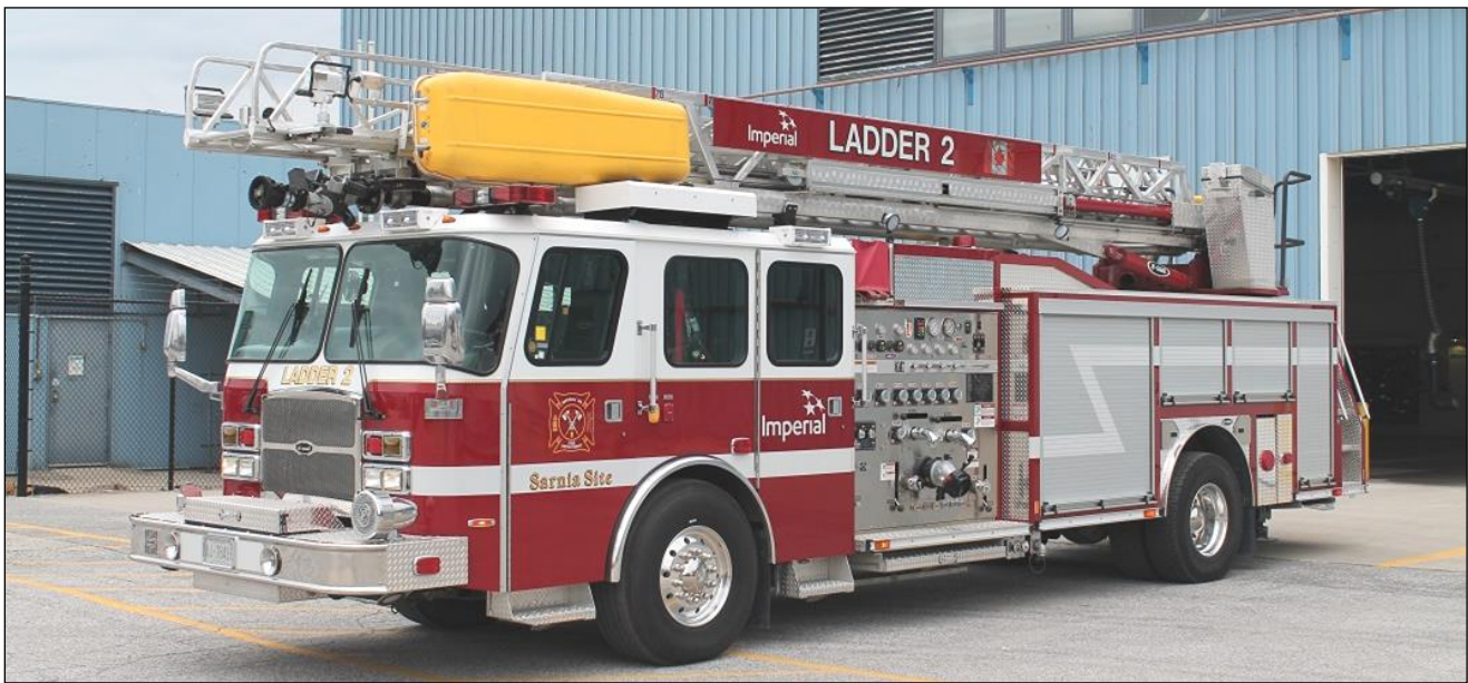
Imperial Oil, Sarnia Ladder 2 is a 2014 E-One Cyclone II, 1763igpm/500gft/78'
