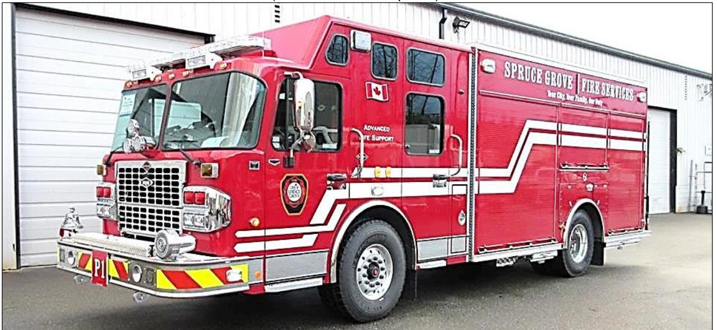
Spruce Grove, AB Pump 1 (919) - 2019 Spartan Gladiator Classic LFD / Hub (1750/500/40F) (SO#1239) (Hub Fire Apparatus)
