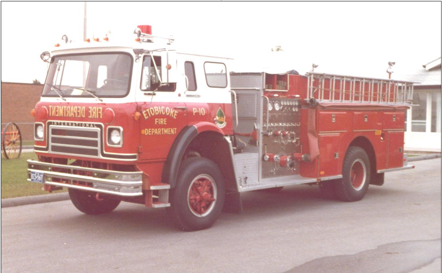
From the former Etobicoke FD, Pumper 10, a 1979 IHC CO1950B/Thibault, 1050igpm and 500gwt.
