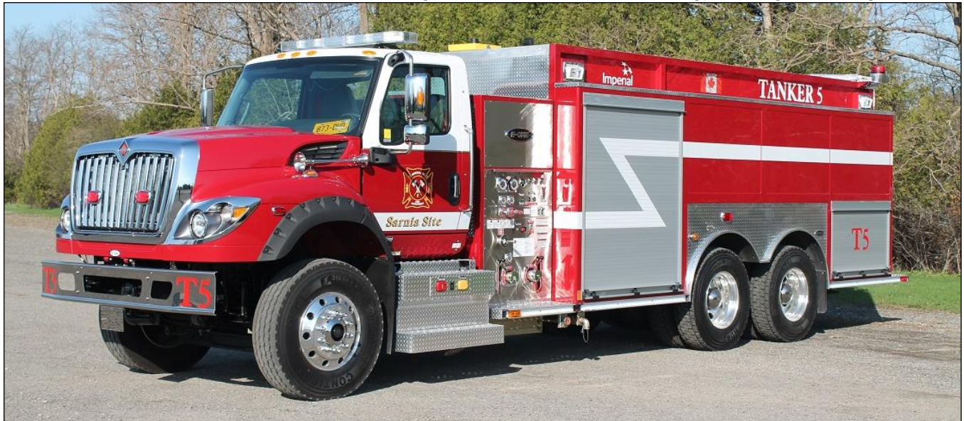
Another new rig, Imperial Oil Sarnia Tanker 5 is a 2019 IHC MV/E-One, 1000gpm pump/3030gft.
