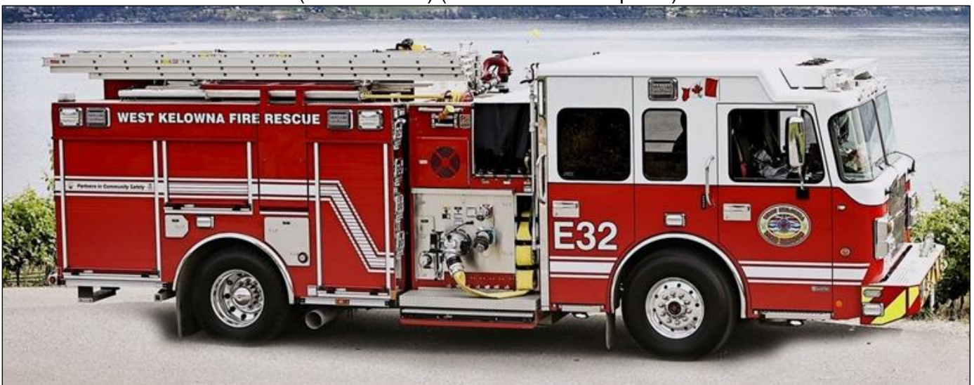
West Kelowna, BC Engine 32 - 2018 Spartan Gladiator Sirius MFD / Smeal (1750/500/20A) (SO#4685) (Photo above courtesy Safetek, below Associated Fire Safety Group)
