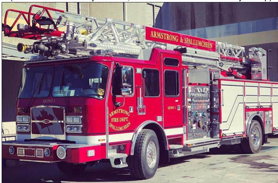
Armstrong & Spallumcheen, BC Quint 1 2019 E-One Typhoon 1500gpm(H)/500gwt/78' sn 142134
