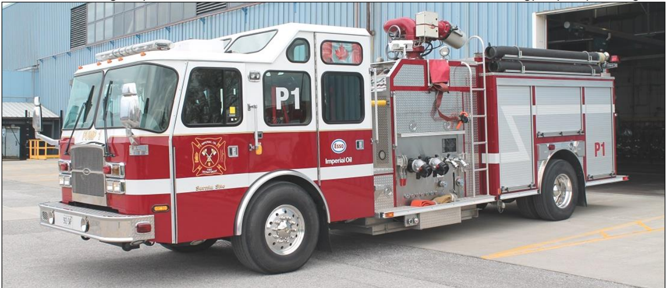
Imperial Oil, Sarnia Pump 1 is a 2008 E-One Cyclone II industrial pumper, 2922igpm pump, 858gft and Trident 250igpm foam pump. (SN#99047) (Gary Dinkel photos)
