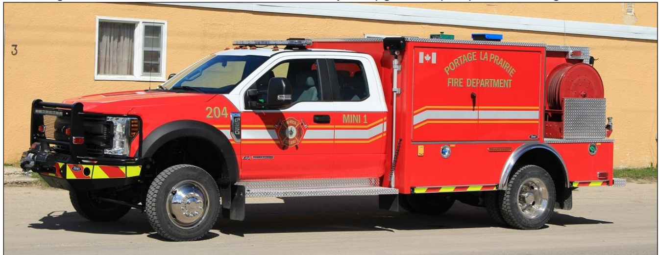
Portage-la-Prairie, MB 204, a 2019 Ford F-550 4x4/Acres brush unit equipped with a 230igpm pump, a 300gwt and a 20gft. SN 190426180 (Dave Stewardson photo)
