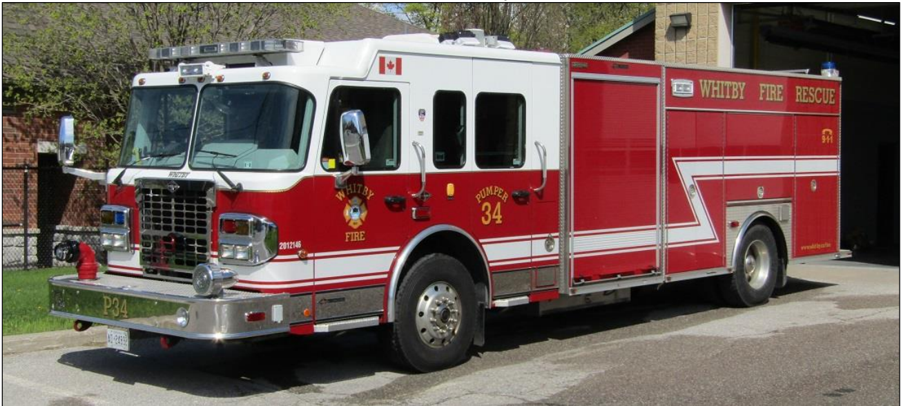
Pumper 34 is a 2012 Spartan Metro Star/Spartan ERV/Dependable rig, 1750igpm pump, 500gwt and twin 25gfts.
