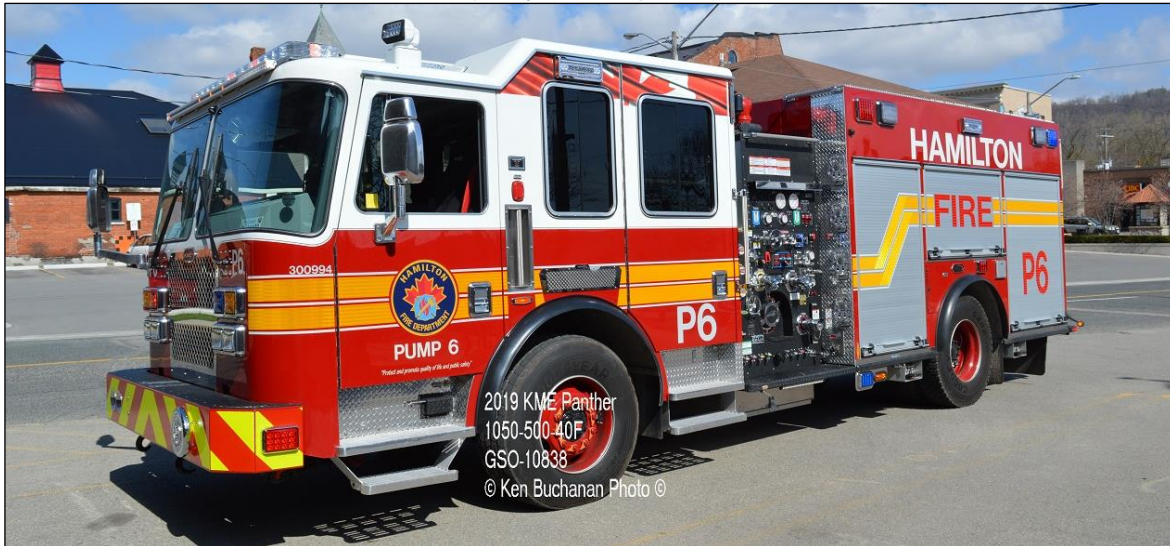
Hamilton Pump 6 is a 2019 KME Panther, 1050igpm, 500gwt & 40gft. GSO-10838. One of 3 Urban Pumps, lower overall height, length and wheelbase. Pump 1 and Pump 9 are the others.
