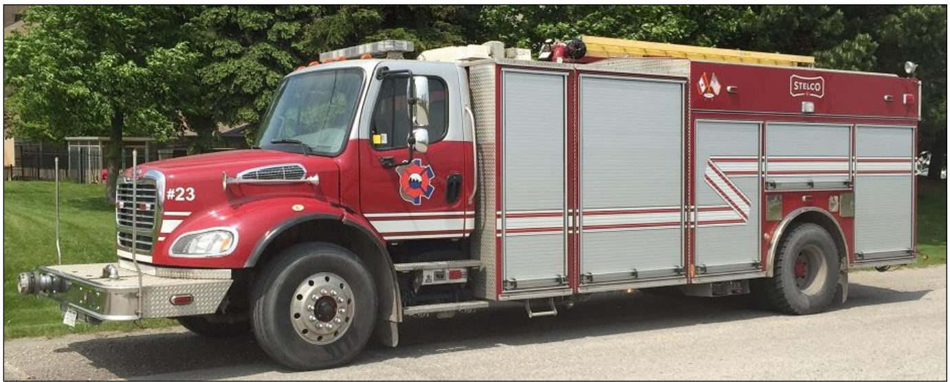
Stelco Nanticoke Unit 23, a 2011 Freightliner M2 112/Pierce, 1556igpm, 628gwt & 200gft
