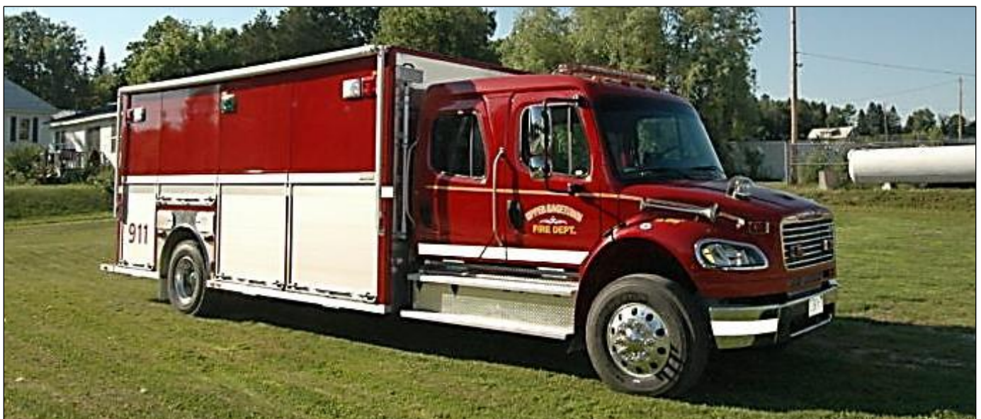
2018 Freightliner M2-106 / Metalfab walk-in heavy rescue (Metalfab Fire Trucks photos)
