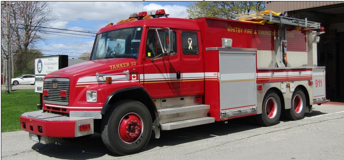
Tanker 33 is a 1999 Freightliner FL80 / Dependable, 420igpm pump and 2500gwt.
