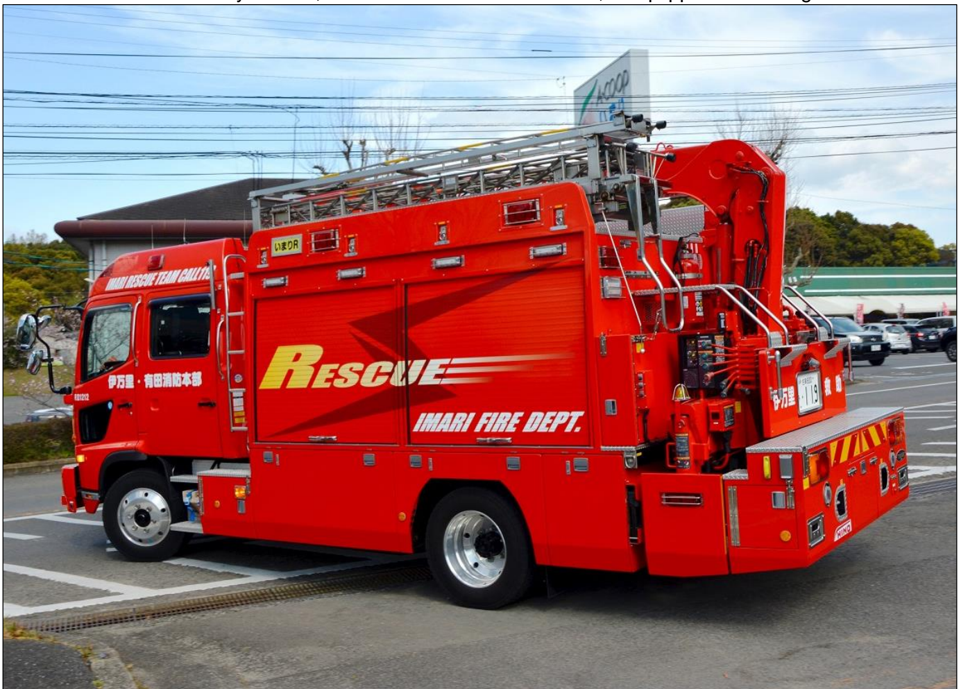
Imari-Arita's Heavy Rescue, constructed on a Hino chassis, is equipped with a large crane.
