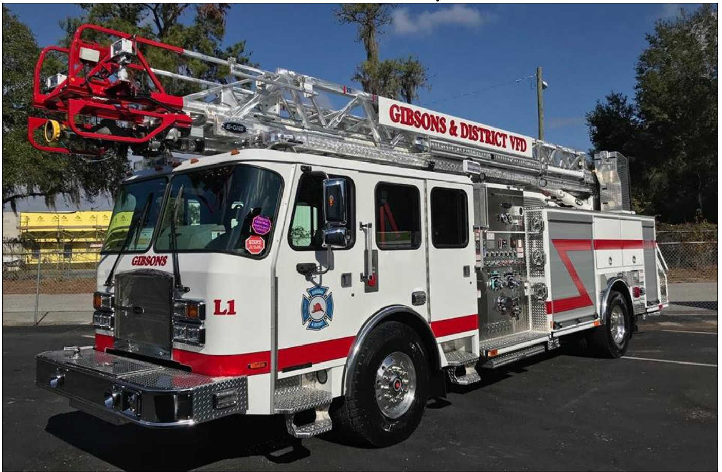
Gibsons, BC Ladder 1, 2018 E-One E78 quint 1250igpm(H)/400gwt/25gft/78' rearmount Foam Logix FS sn 141325 (Associated Fire Safety)
