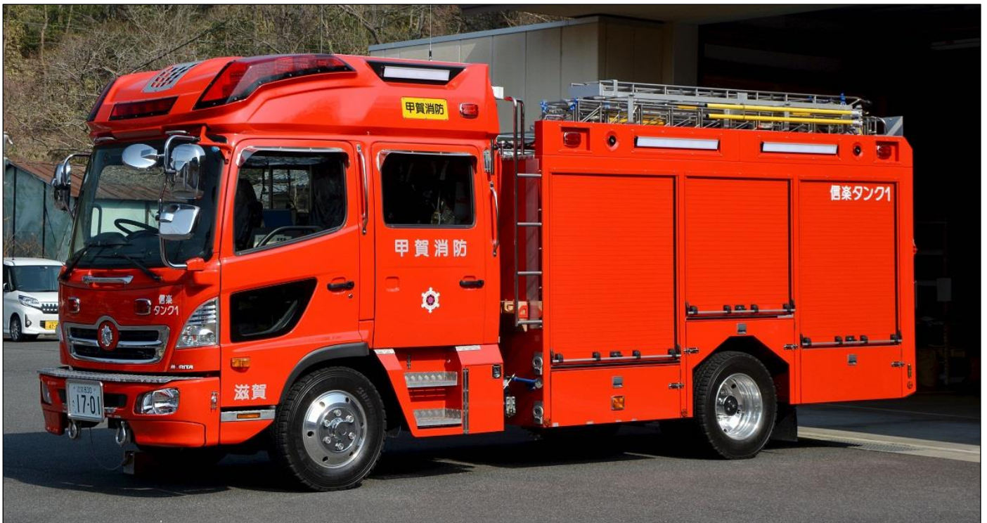
Imari-Arita's Large Pump, built by Morita. This is a rescue-pump, it carries 1500 litres of water and also has a CAFS. (All pictures in this feature by Terry Yip)
