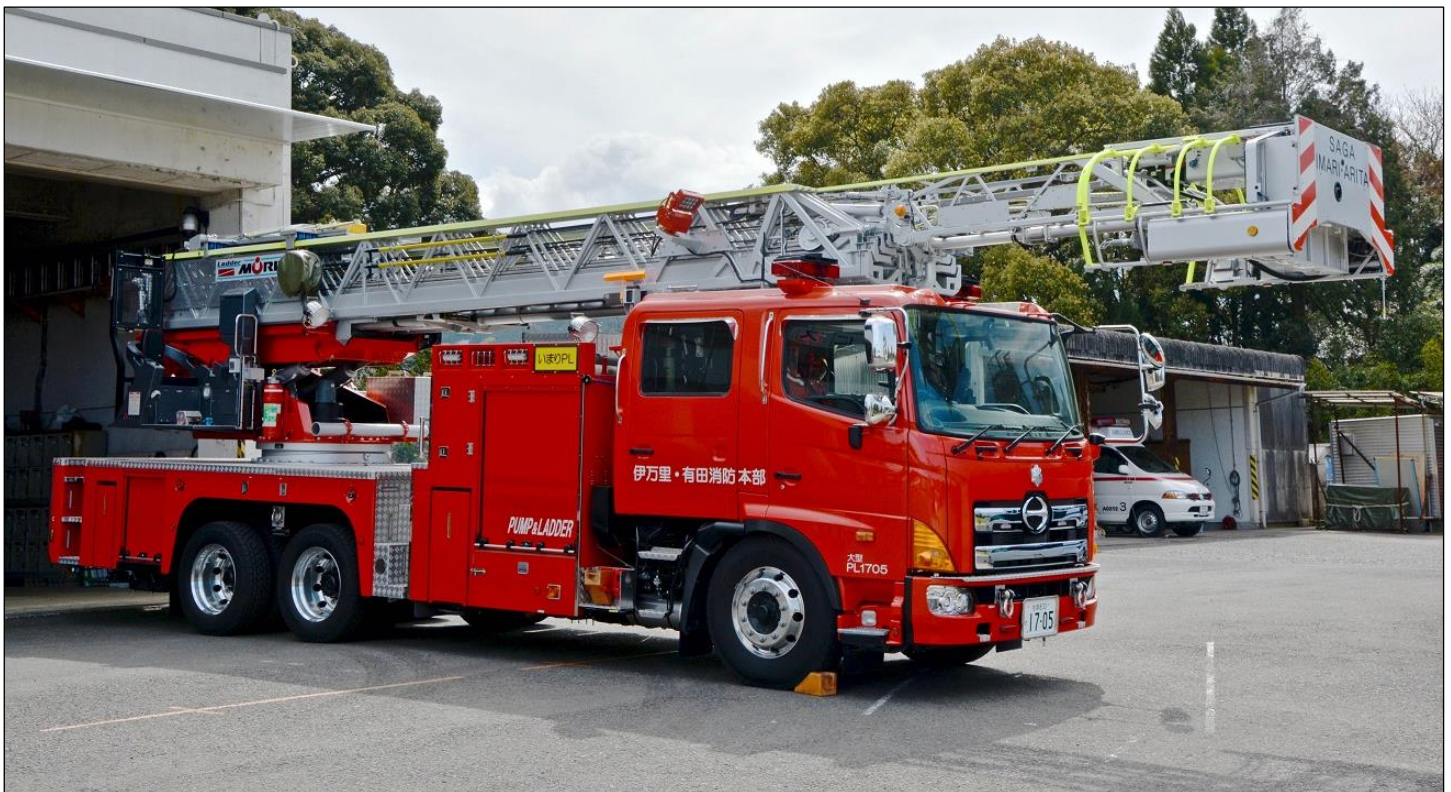
Imari-Arita's Pump Ladder, built by Morita in 2017, it has a 35m turntable ladder and a 4500LPM pump.
