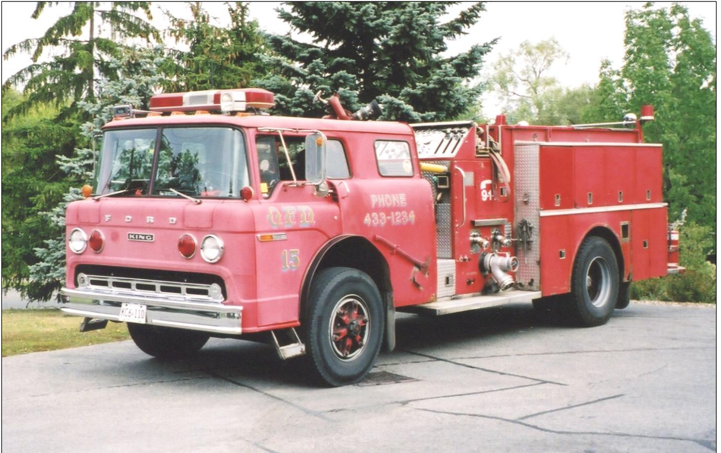
And from Oshawa, Unit 15, a 1969 Ford C/King pumper, 840igpm and 500gwt. (Photos courtesy Larry Ward)
