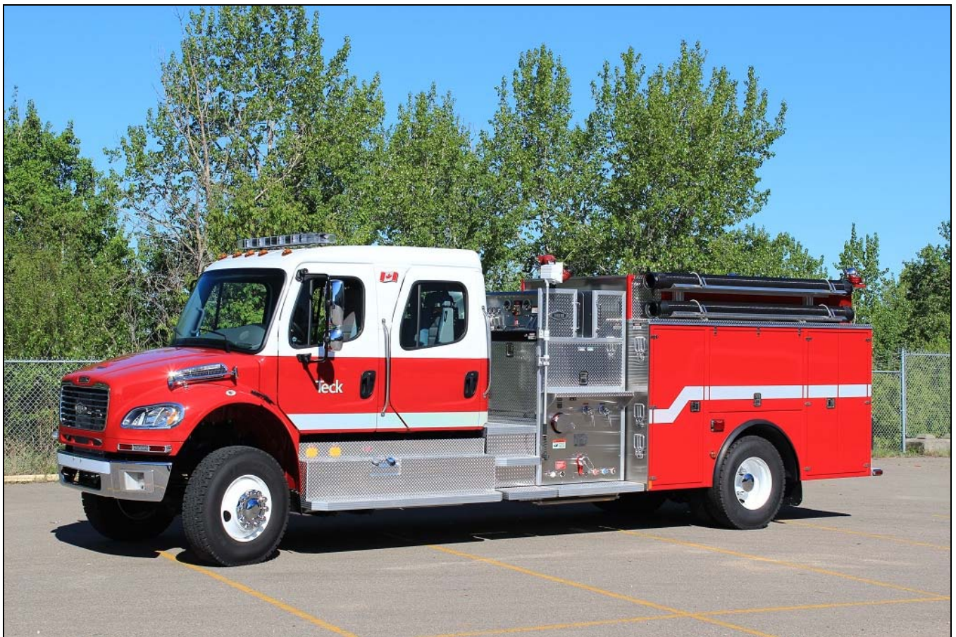
Teck Coal, B.C. got this 2013 Freightliner M2/Hub pumper last year. It has a 1500gpm pump, 1000 gwt, 15gft(A) and 30gft (B) with a FoamPro 2001 system. S.N. 5350-1128 was sent to the Cardinal River site.
