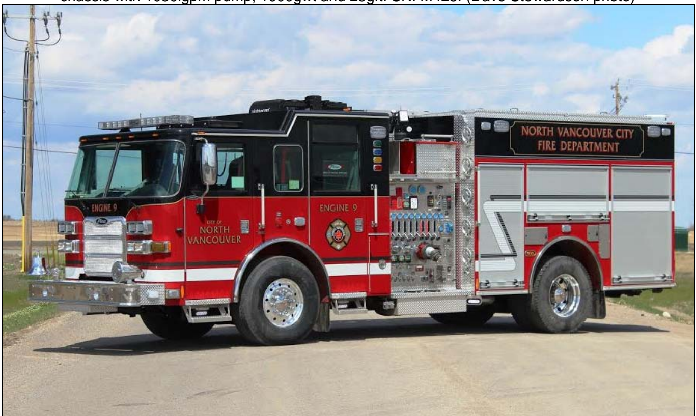
Just delivered to North Vancouver, this is Engine 9 a 2014 Pierce Arrow XT pumper with a 1770 igpm Waterous pump, 328gwt, 25gft a Husky Foam System and a Night Scan light tower, job # 27188. This and two very similar rigs were received by north shore communities (see the round-up), apparently another five to nine are expected. (Info and photo from John Bowerman)
