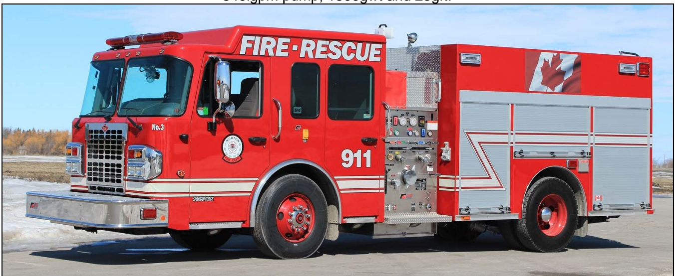
Norton, NB just purchased this stock unit from Fort Garry Fire Trucks. Mounted on a 2011 Spartan Metro Star chassis, it has a 1050igpm pump, 800gwt and 25gft. SN M296 (Dave Stewardson photos)
