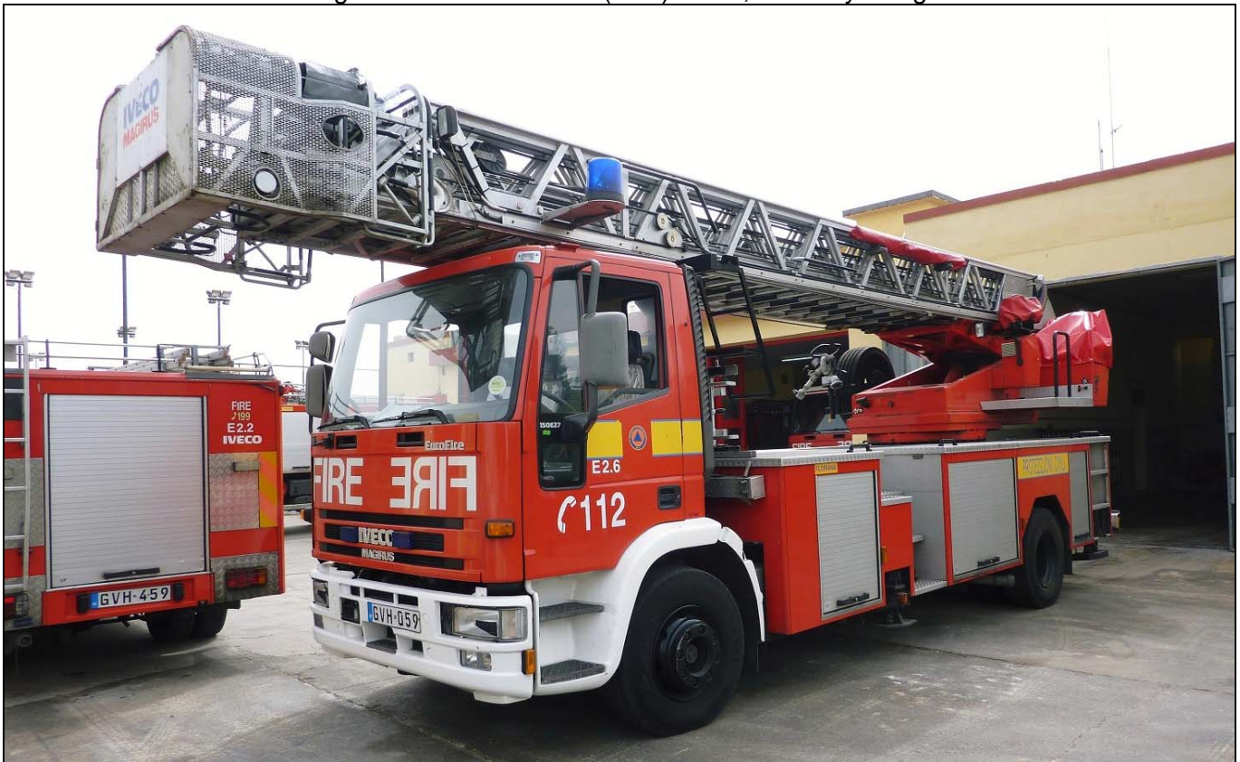
E1.6, above, is a heavy rescue, and runs from the Hal Far station. E2.6 is a Magirus/EuroFire turntable ladder on an Iveco Cargo chassis with a 37m (120') aerial, normally assigned to Floriana station.
