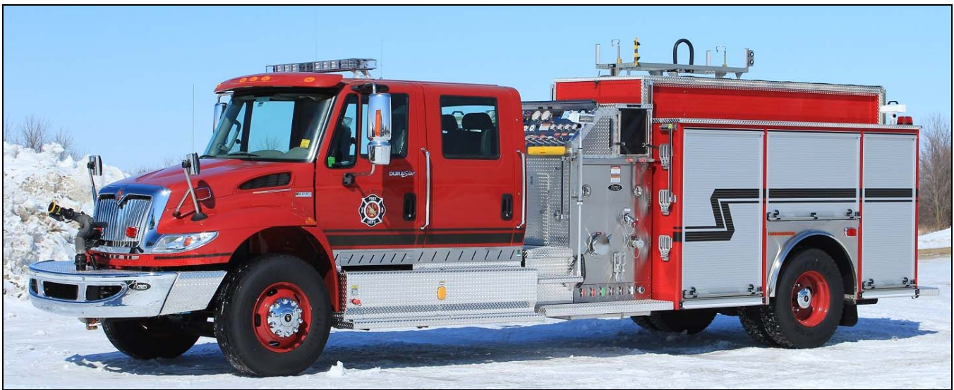
Oak River, MB received this long rig in the spring, it's a 2014 IHC 4400/Acres pumper equipped with a 1050igpm pump, 1000gwt and 25gft. SN 140228113
