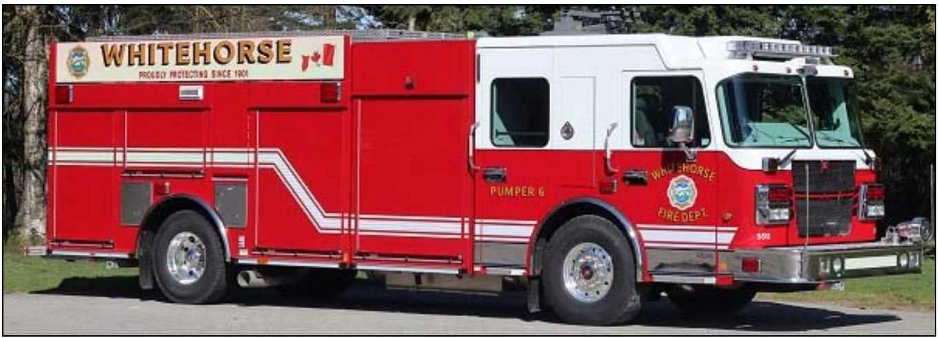
On it's way to Whitehorse, YT, Pumper 6 is a 2014 Spartan Sirius/Smeal 1500gpm/900gwt. SN 4260. (Shane MacKichan photo)
