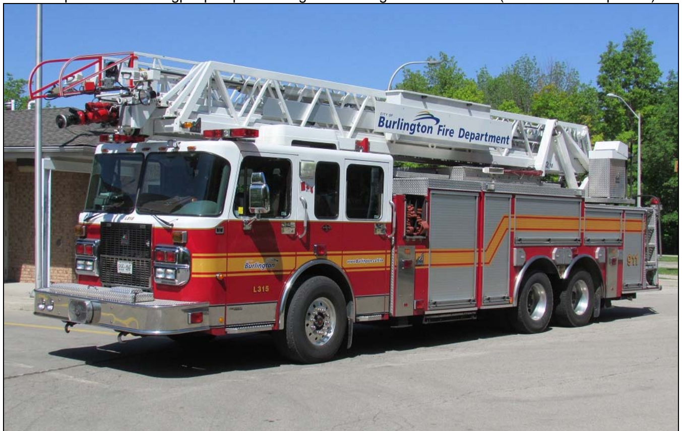
Two vehicles presented on the tour of Burlington on May 31. Pump 301 is a 1996 Spartan Gladiator/Saulsbury pumper with a 1050igpm pump and 800gwt. Ladder 315 is a 2004 Spartan Gladiator/Smeal 105' quint with a 1500gpm pump and 300gwt. It's assigned to Station 8. (Desmond Brett photos)
