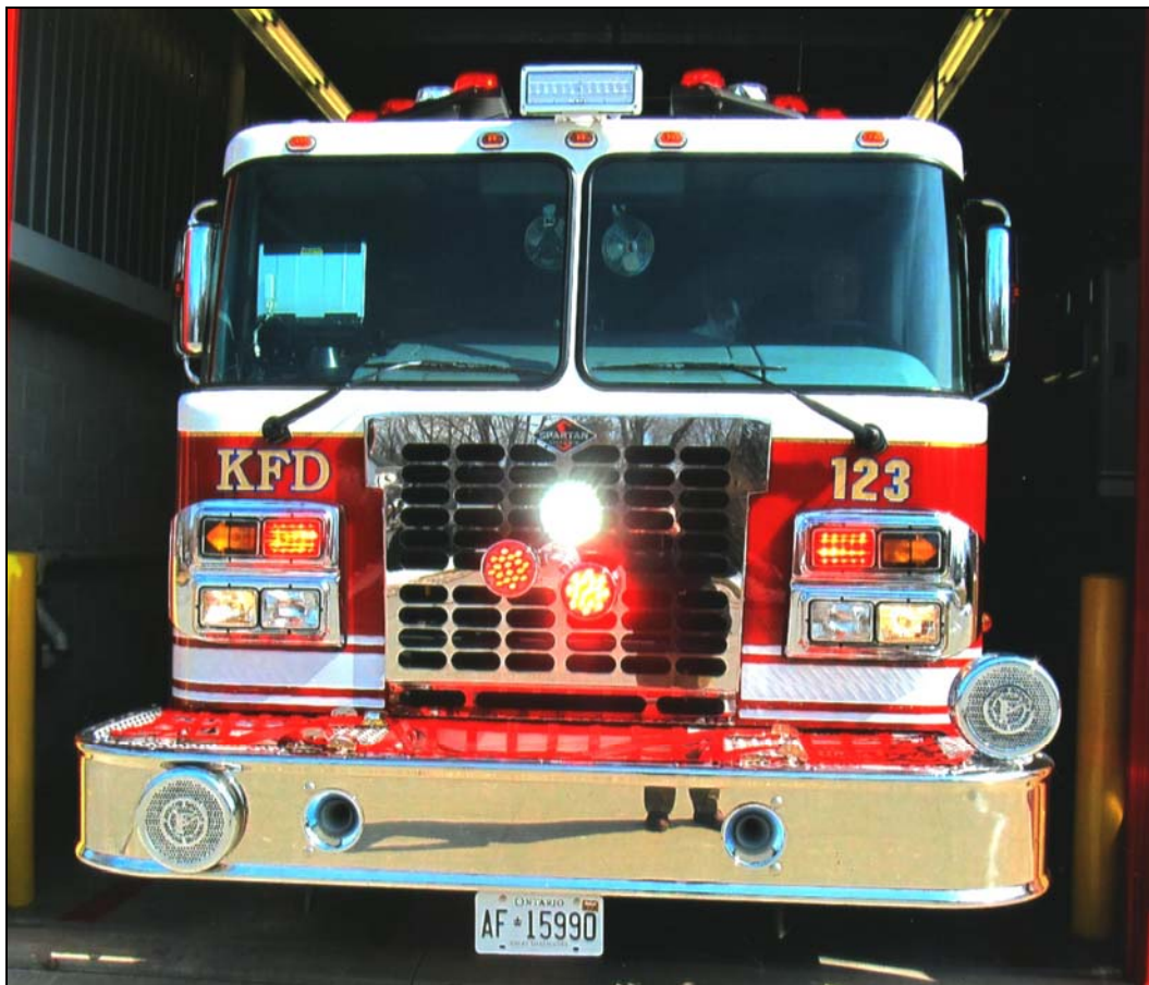
Kingsville pumper 123, a 2013 Spartan Metro Star/Metalfab product, with 1050igpm/1000gwt, seen below sporting its Roto-Ray. (Walt McCall photos)
