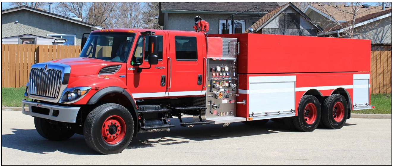
This unusual looking rig is bound for China, where it will be lettered. It's a 2014 IHC 7400/Fort Garry industrial pumper with an 840igpm pump, 2200gwt and 800gft. s/n #M501. (Dave Stewardson)
