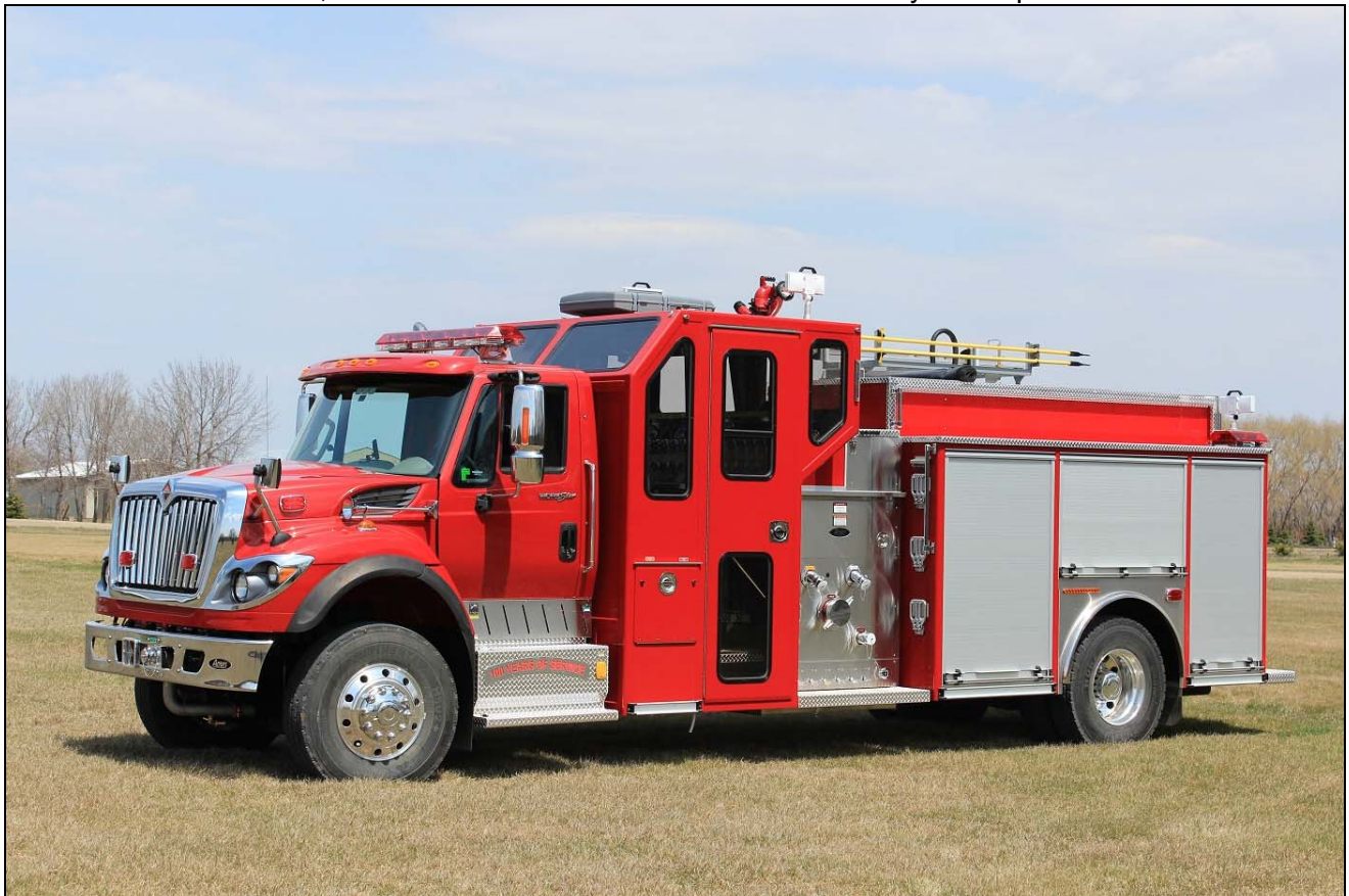
Another yet-to-be lettered rig, this went to Holden, AB in May. It's a 2014 IHC 7400/Acres product with a 1050igpm pump, 1000gwt and 25gft. s/n #140513116 (Dave Stewardson photos)
