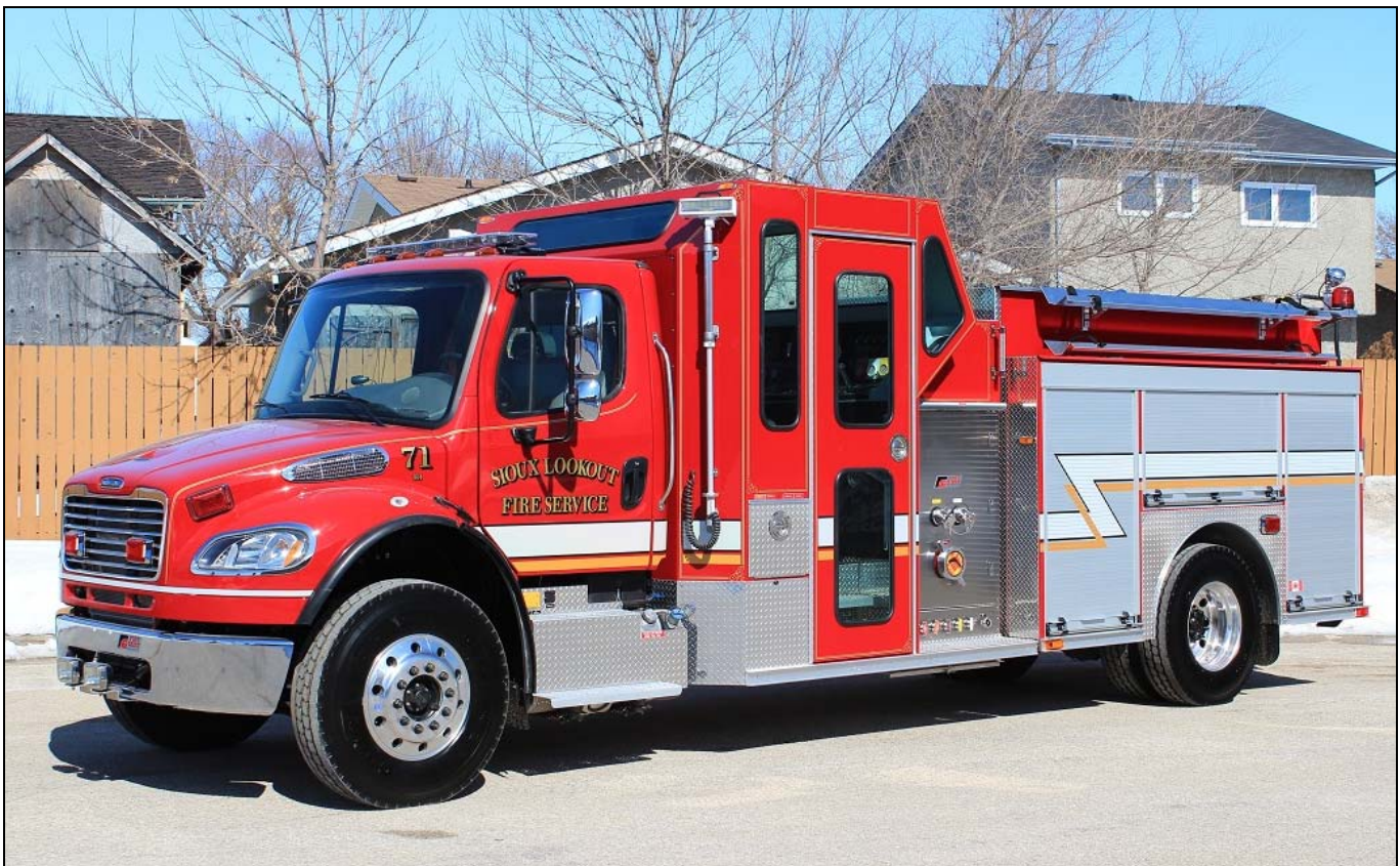
Delivered in April to Sioux Lookout, this is Pump 71, a Fort Garry product on a 2014 Freightliner M2 4x4 chassis with 1050igpm pump, 1000gwt and 25gft. SN: M428. (Dave Stewardson photo)
