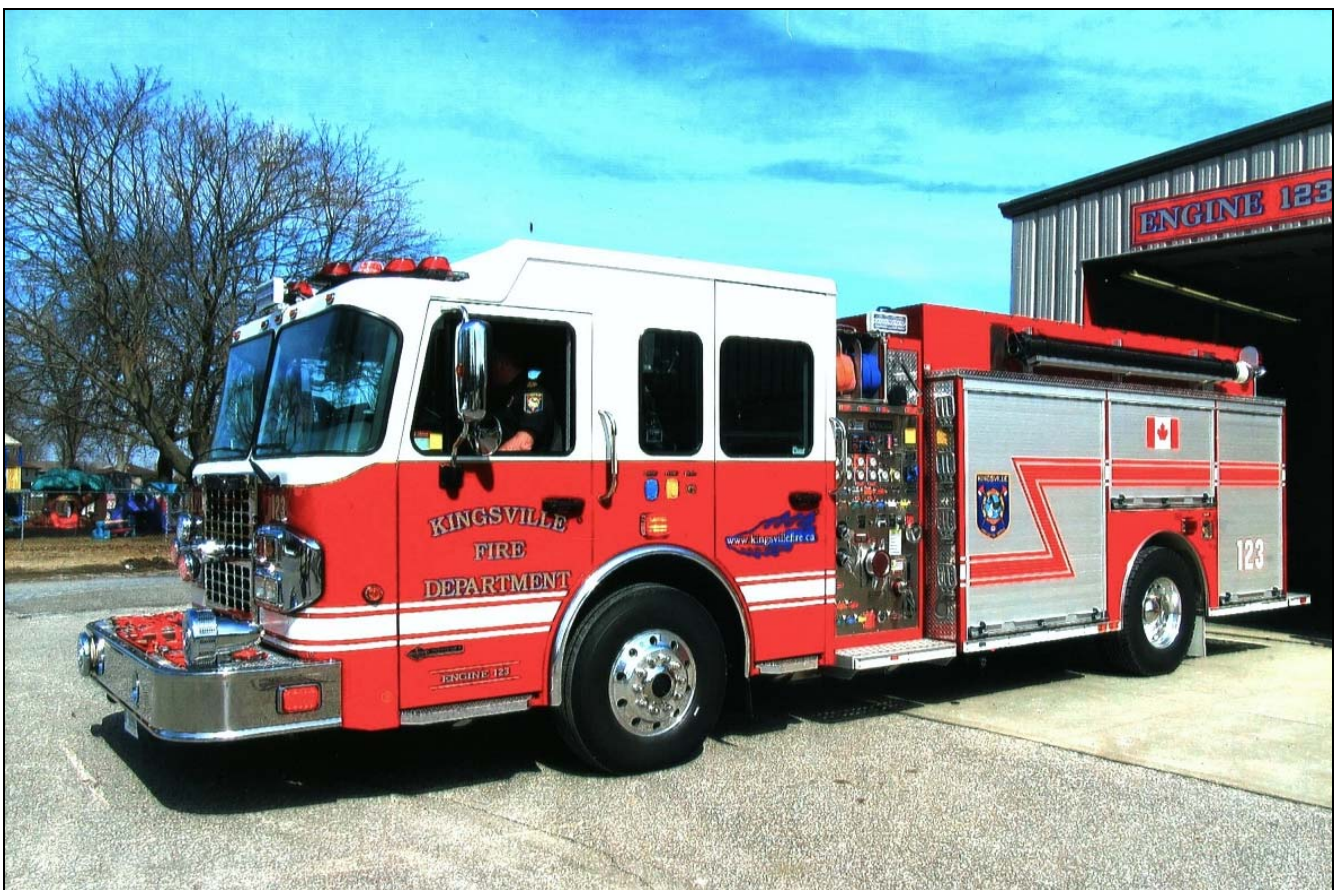
Kingsville pumper 123, a 2013 Spartan Metro Star/Metalfab product, with 1050igpm/1000gwt, seen below sporting its Roto-Ray. (Walt McCall photos)
