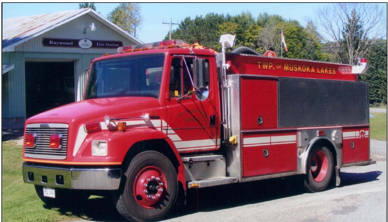
The TA continues to honour Neil McCarten, this is his shot of Muskoka Lakes Pump 77, a 2007 Sterling/Fort Garry pumper with a 1050igpm pump, 500gwt and 25gft. It carries serial number A534.
