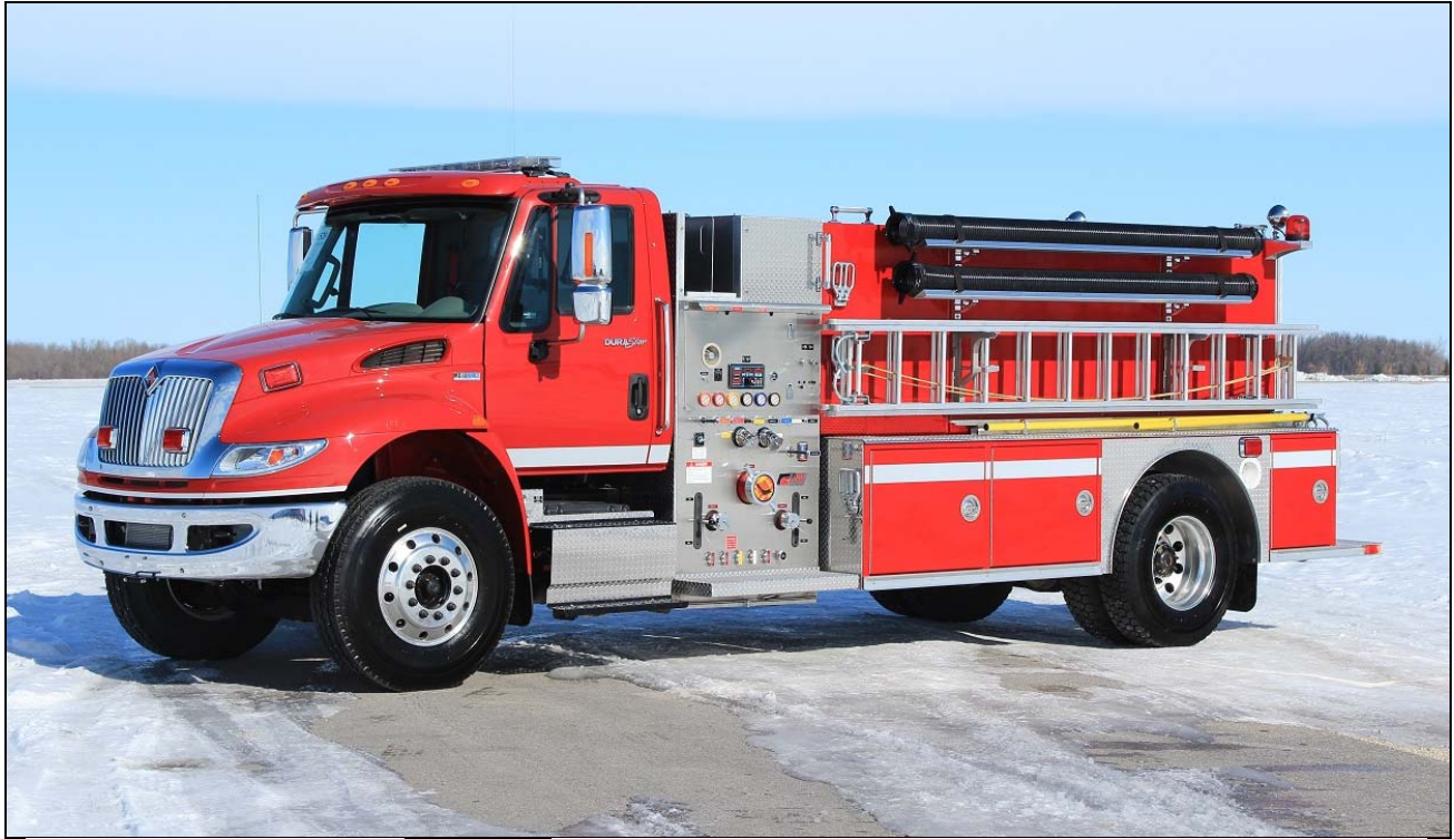
Trent Lakes got this 2014 IHC 4400/Fort Garry pumper 840igpm Darley pump and 900gwt during the winter, serial number M520. It was to be detailed by the department.
