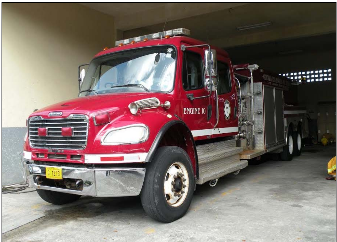
Antigua Engine 10 is a 2006 Freightliner M2/Seagrave tanker with a 1000gpm pump and 3000gwt. (Robert Herscovitch photo)
