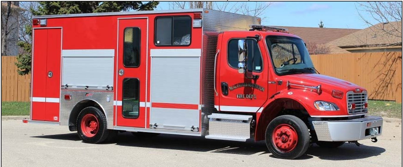
Above: Newly in service with Black River/Matheson, ON is this 2014 Freightliner M2/Fort Garry medium rescue with a 16' box. The truck has smaller wheels so it will fit in the hall, the photographer assures me that it still delivers a nice ride. It is assigned as Unit 10. Below: Ramara Township, ON. P-3 2014 IHC 4400/Fort Garry 1050igpm/1000gwt #M523 PTD 26 Feb 2014 (Dave Stewardson photos)
