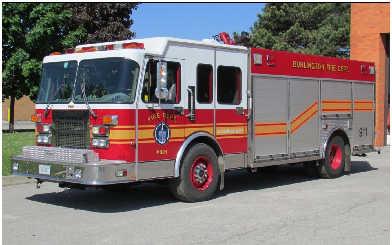
Two vehicles presented on the tour of Burlington on May 31. Pump 301 is a 1996 Spartan Gladiator/Saulsbury pumper with a 1050igpm pump and 800gwt. Ladder 315 is a 2004 Spartan Gladiator/Smeal 105' quint with a 1500gpm pump and 300gwt. It's assigned to Station 8. (Desmond Brett photos)
