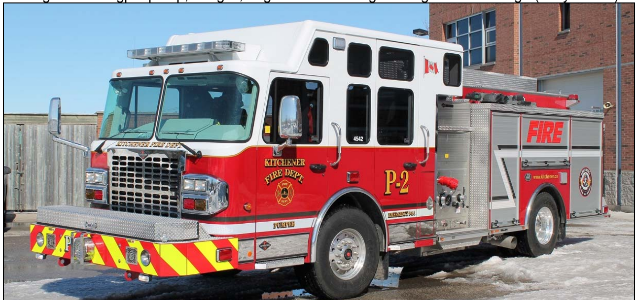
Kitchener has refurbished Car 23, remounting the box on a 2014 Ford F450 chassis. One of a pair of pumpers just delivered to Kitchener by Dependable, this is P.2, a 2013 Spartan Gladiator/ERV/DEV rig with 1250gpm pump, 600gwt, 40gft and Foam Logix. P.1 got the other rig. (Gary Dinkel)
