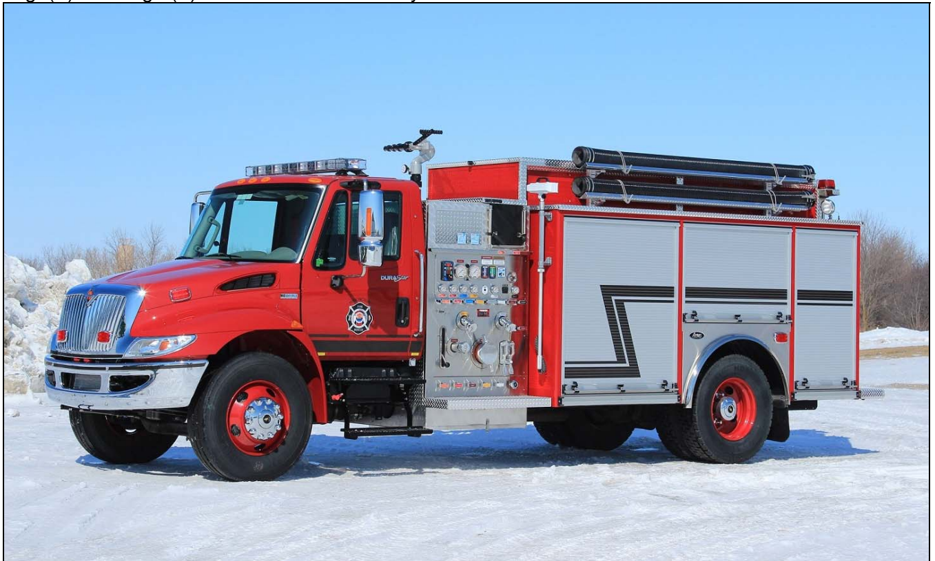
York Factory FN received this 2014 IHC 4300/Acres rig back in the winter. It features an 840igpm pump, 1000gwt and 25gft. Serial number 140318114. (Dave Stewardson photos)
