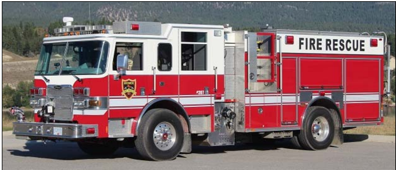
Two fine examples of western scenery from Invermere, BC. Engine 207, above, is a 2008 Pierce Arrow XT pumper with a 1500gpm pump, 650gwt and 25gft. SN#19999. Engine 202, below, is a 2007 Freightliner M2 4x4/Rosenbauer product with a 1050igpm pump and 1000gwt, serial 1388806. (Shane MacKichan photos)
