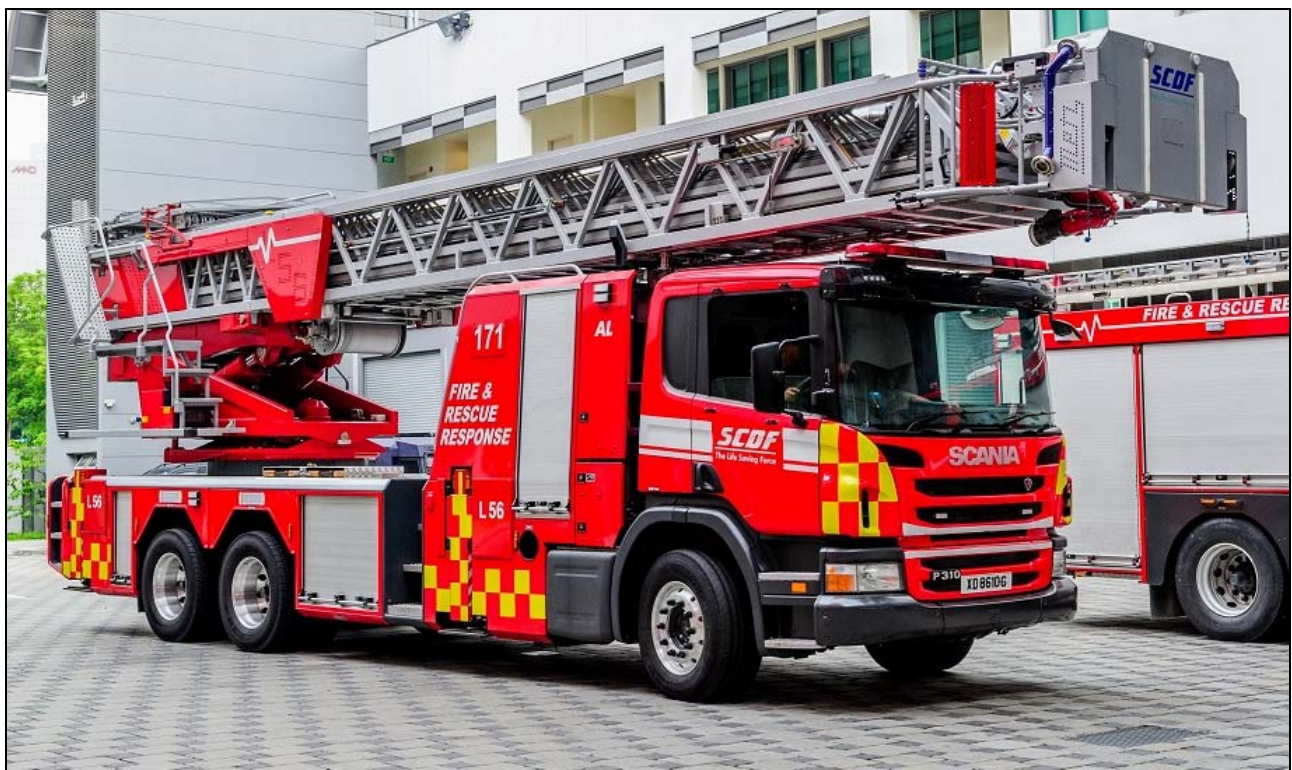
Recently delivered to the SCDF, Singapore, this is Aerial Ladder 171, a 2014 Scania 310/Metz L56 turntable ladder, which tops out at 184' {56m}. (Kenneth Lai photo)
