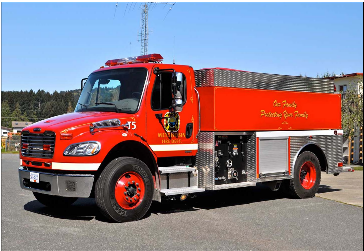
Metchosin, BC Tender 5, a 2010 Freightliner M2/Hub tanker with a 420igpm pump and 1700gwt.
