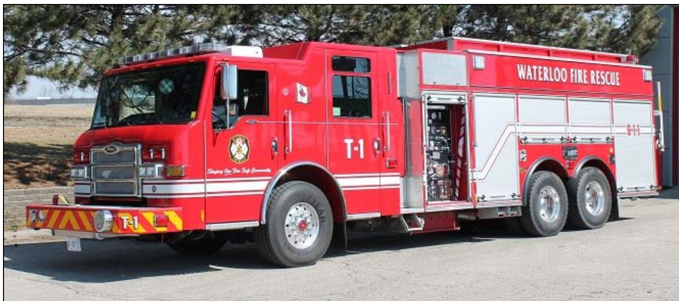
Waterloo's new Tanker 1, a 2013 Pierce Impel 1050igpm/2455gwt/33gft (Gary Dinkel photo)
