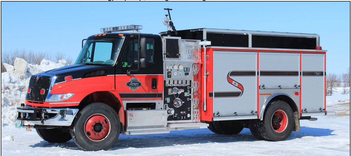
Green Acres, MB recently bought this 2008 IHC 4400/Pierce pumper rebuilt in 2013 by Acres. It has a 840igpm pump, 1500gwt and 25gft.
