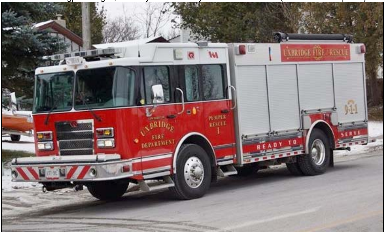
Uxbridge Pumper Rescue 1 is a 2005 Spartan Advantage 4x4/Rosenbauer rig with a 1500gpm pump, 500gwt and 30gft. (Mark Appleman photo)
