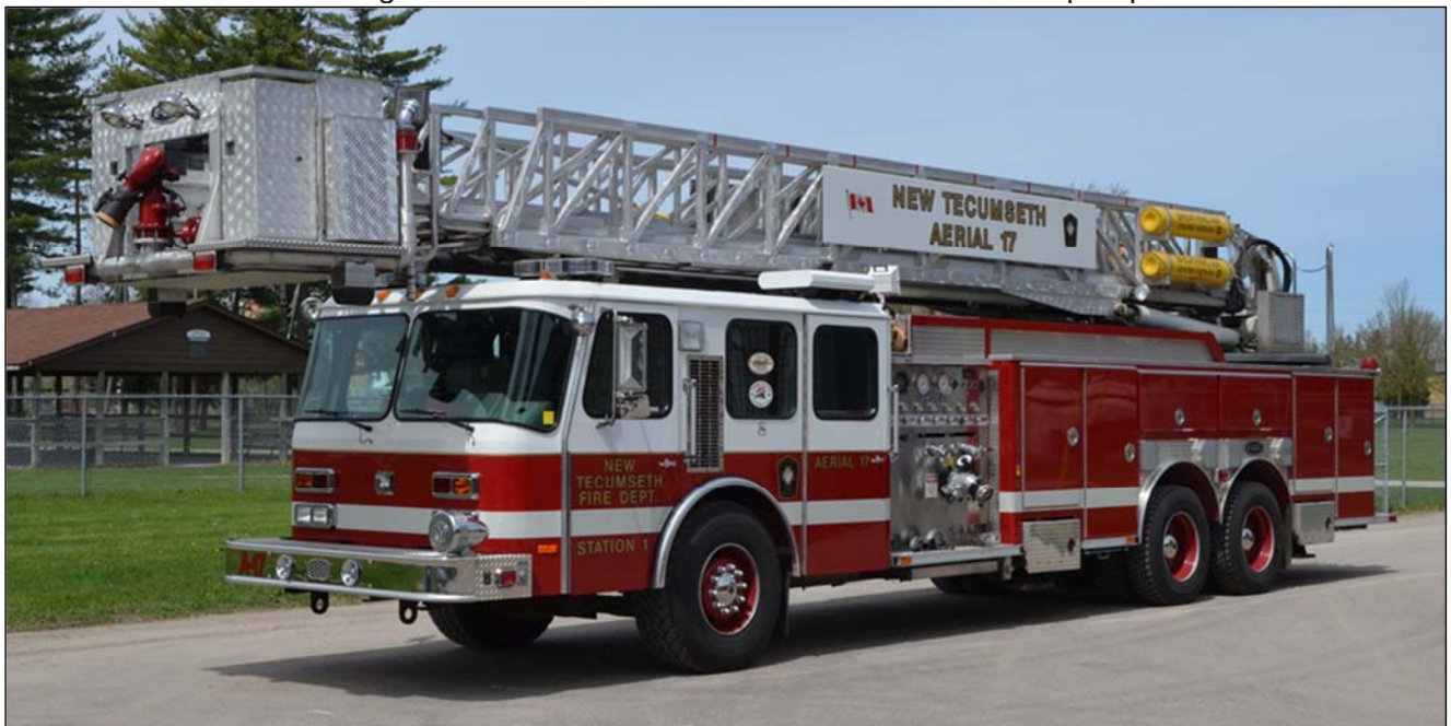
New Tecumseth Aerial 17, a 1997 E-One Hurricane 95' tower, 1500igpm/250gwt. S#16481
