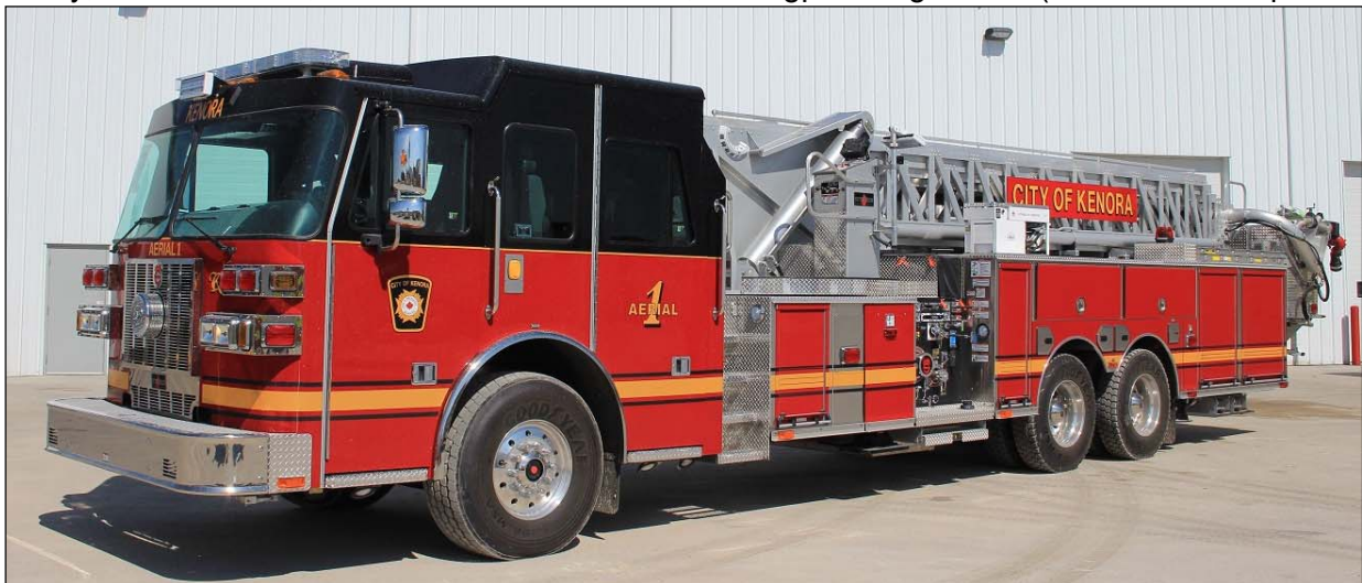
Kenora, ON Tower1, a 2018 Sutphen tower via Fort Garry, 1250 Hale Q-Max pump, 250gwt and a 95' platform. s/n #M909 and #HS5829 (Dave Stewardson photo)
