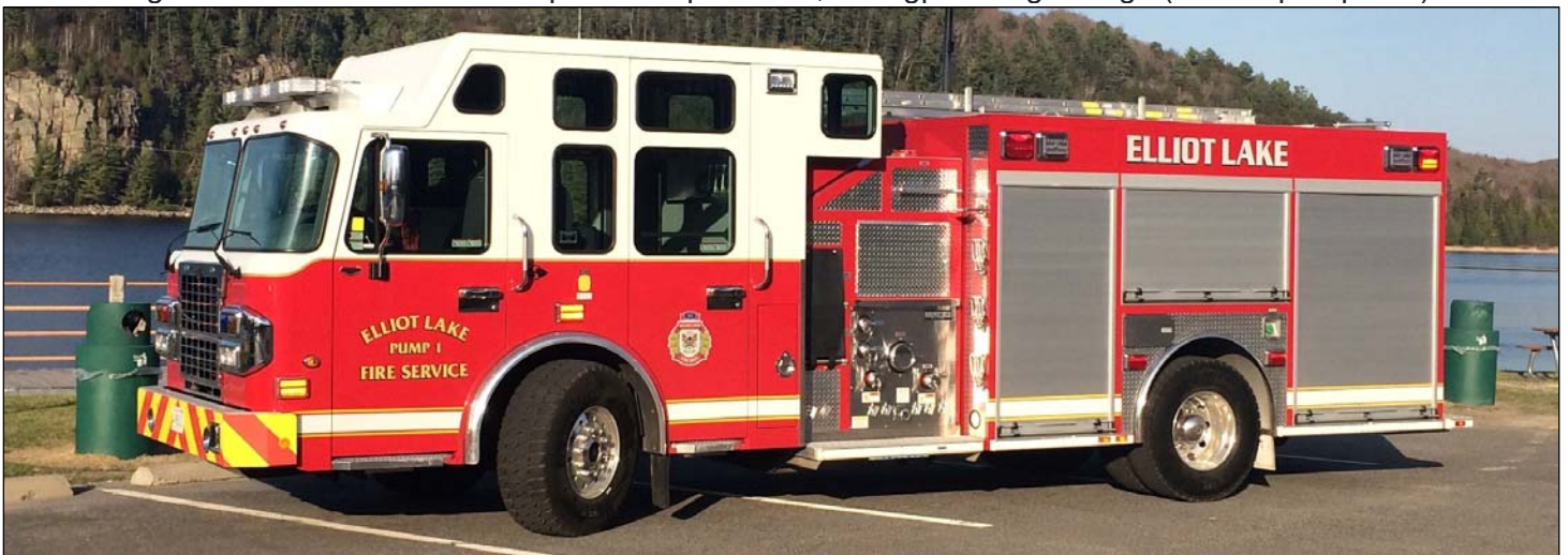
Elliott Lake, ON Pumper 1, a 2018 Spartan Metro Star/Metalfab, 1050igpm/750gwt/20gft (Metalfab photo)
