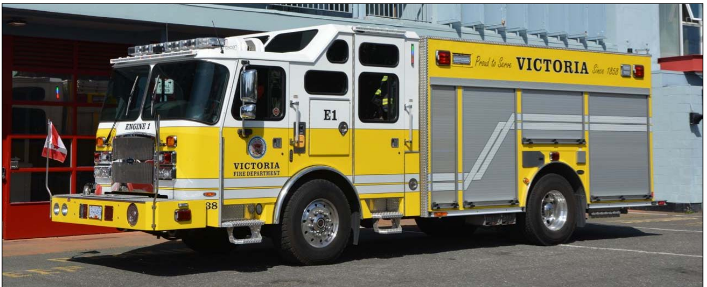
Victoria Engine 1 is a 2017 E One Typhoon with 1331igpm pump, 416gwt and 2x20gfts.
