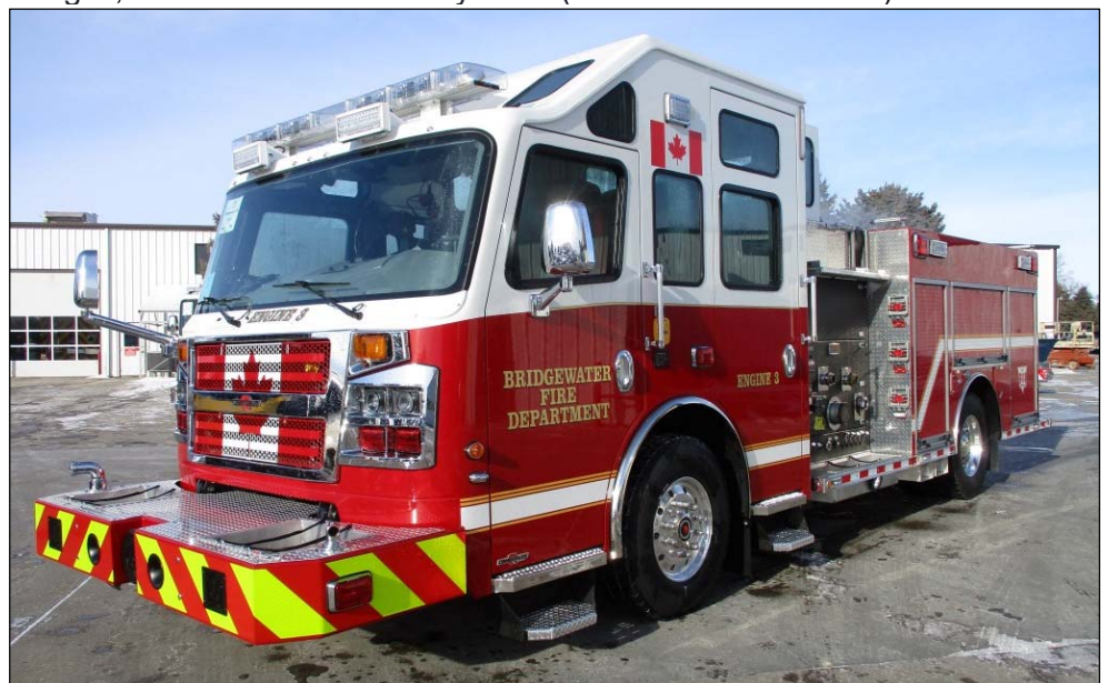
Bridgewater Engine 3, a 2018 Rosenbauer Commander 1250igpm/800gwt. (Rosenbauer)
