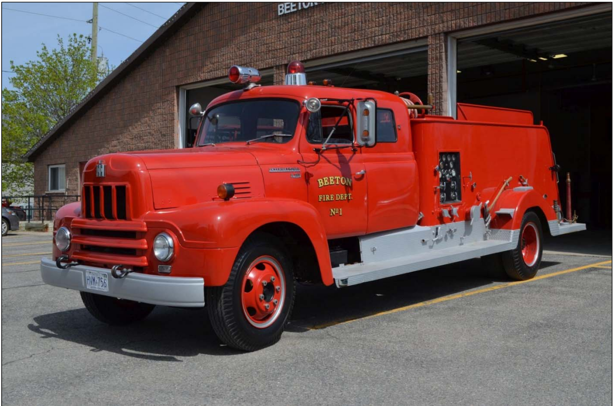
Beeton firefighters preserved 1951 International R185/American Marsh rig, it has a 625igpm pump and a 500 gwt. It originally served with Civil Defence, S#440. (Bob Rupert photos)
