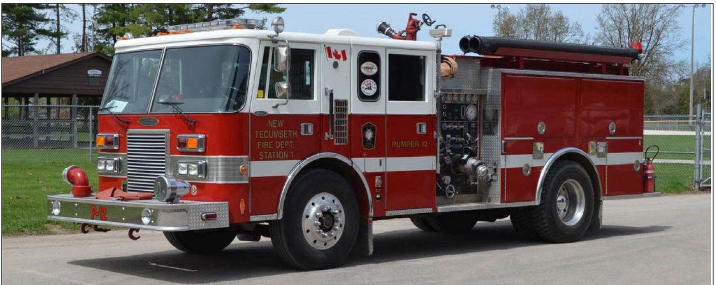
New Tecumseth Pumper 12, a 1989 Pierce Lance/Superior, 1250igpm/500gwt. SN E4830 / SES060.
