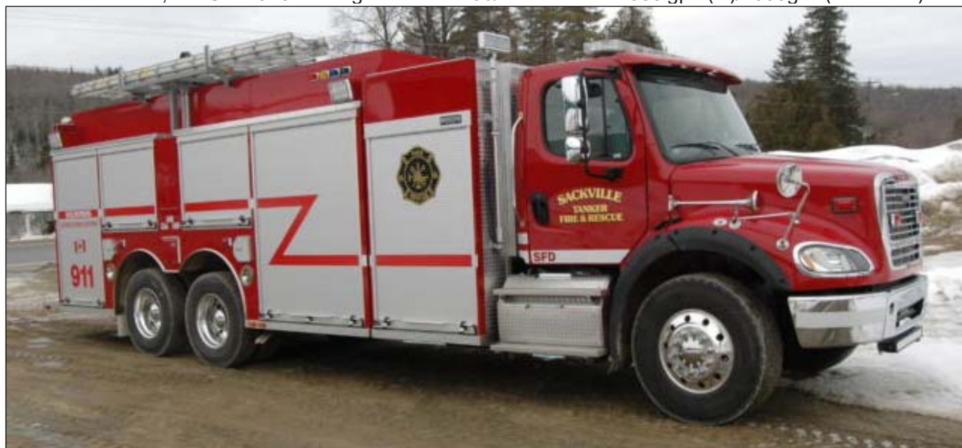
Sackville, NB Tanker 1, a 2018 Freightliner M2-112/Metalfab 1250igpm/2500gwt (Metalfab photo)
