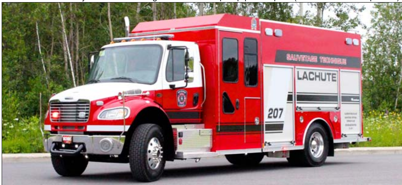
Lachute U.207 2017 Freightliner M2-106/Rosenbauer walk-in heavy rescue (Aero-Feu)
