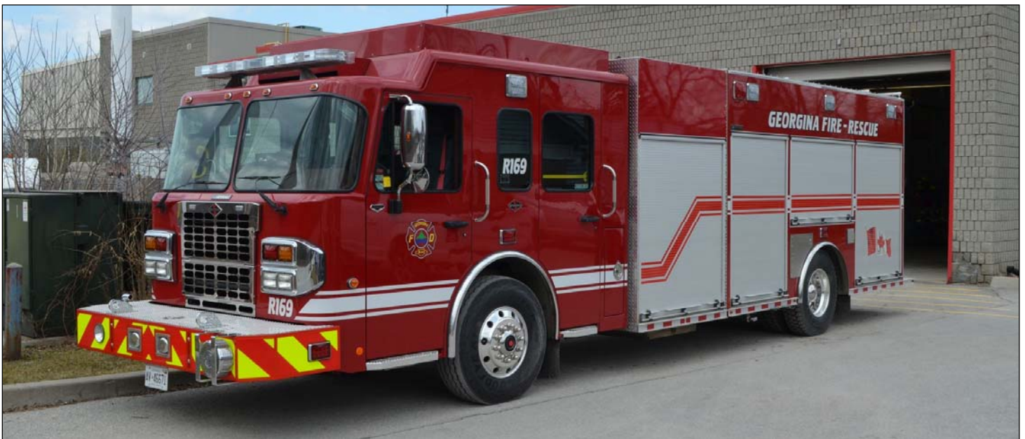
Georgina Rescue 169 is a 2018 Spartan/Dependable, 1585gpm/820gwt/30gft (Bob Rupert photo)
