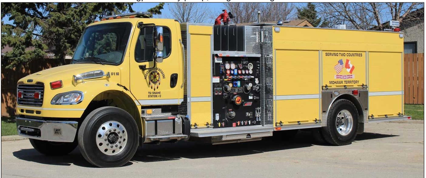
Hogansburg-Akwesasne, QC purchased a 2018 Freightliner M2-106/Fort Garry pumper, 1050igpm(W)/775gwt/ 25gft and s/n M878. Engine 17-E-93 is assigned to station No. 3 at Tsi Snaihe. (Dave Stewardson photos)
