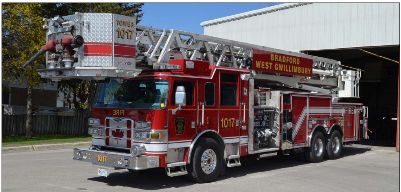
BWG Tower 1017 is a 2011 Pierce Arrow XT 100' Platform, 1750igpm/250gwt/30gft. J#23686. (Bob Rupert photos)
