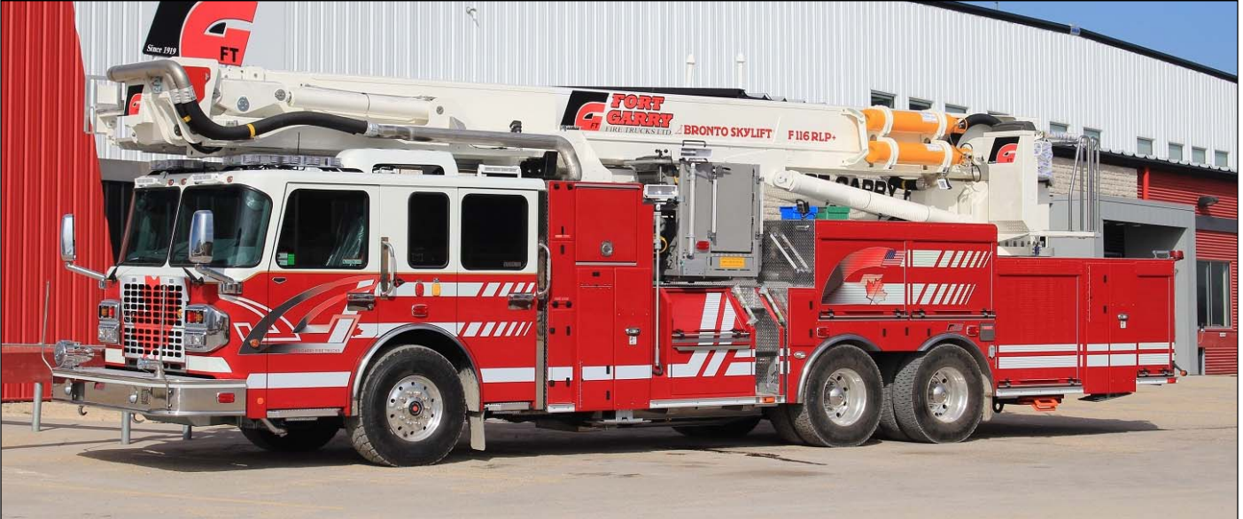
Ft. Garry Bronto Demo, 2018 Spartan Gladiator/Fort Garry/Bronto 1750igpm Hale pump/270gwt/30gft s/n #M857 (Dave Stewardson photos)
