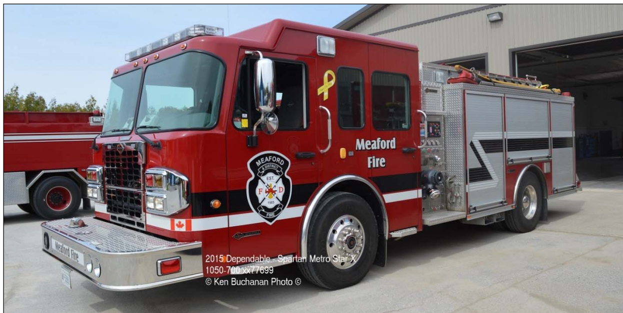
Unit 311, a 2015 Dependable Spartan Metro Star-X 1050 igpm & 700gwt.
