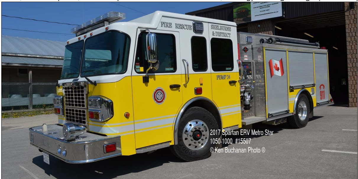
Shelburne, ON Pumper 24, a 2017 Spartan/Spartan ERV/DEV10500gpm/1000gwt/30gft. (Ken Buchanan photo)
