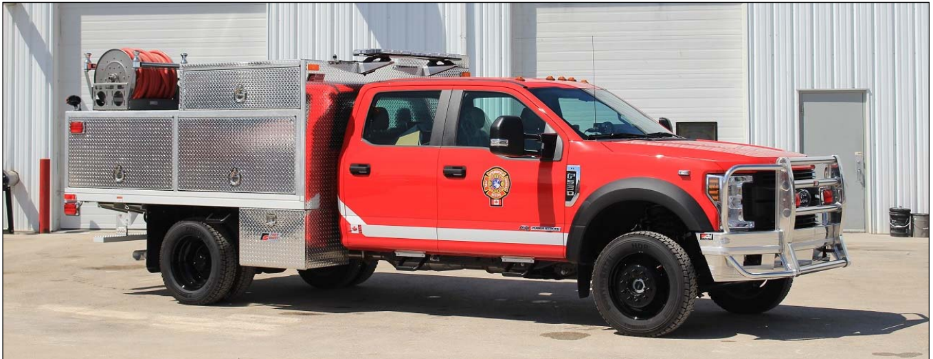
Springfield, MB just got this 2018 Ford F550 4x4/Fort Garry brush truck with a Darley Fast Attack skid unit. It has a 310igpm Darley pump, 350gwt and 10gft. s/n #M900
