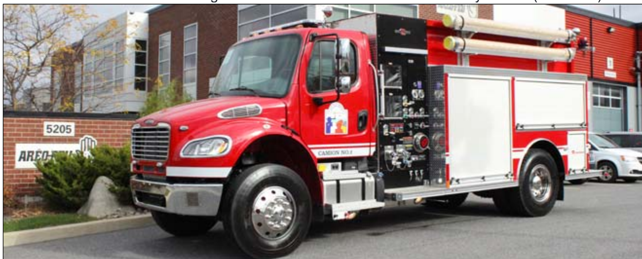
Petit-Rocher, NB U. 22016 Freightliner M2-106/Rosenbauer 1050igpm(D)/1000gwt (Aero-Feu)
