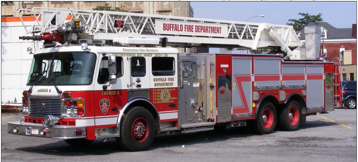
Ex- Ladder 5, 2007 American LaFrance quint with an LTI 110' aerial, and a 1500gpm pump.
