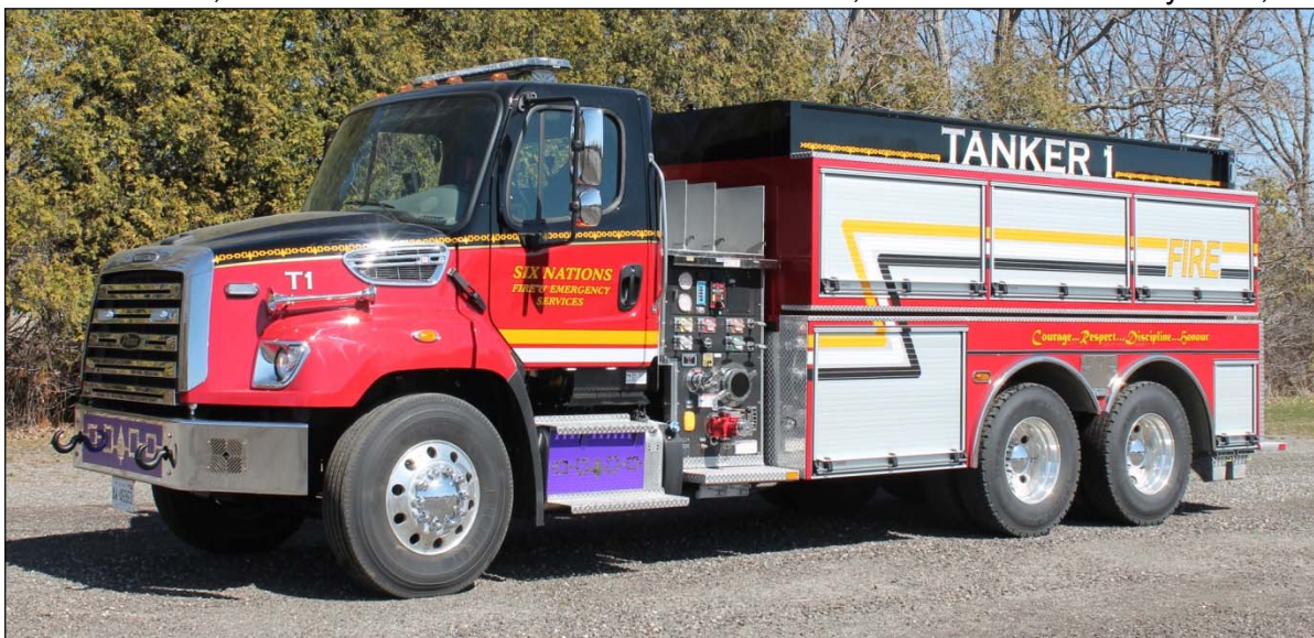
Six Nations, ON Tanker 1, a 2017 Freightliner M2 106/Pierce model with an 840igpm pump and a 3000gwt. (Gary Dinkel photos)
