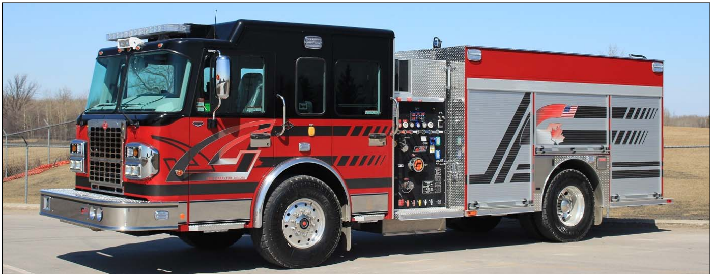
Ft. Garry FDIC Demo, a 2018 Spartan Metro Star/Fort Garry pumper, 1250igpm/774gwt/25gft s/n #M888
