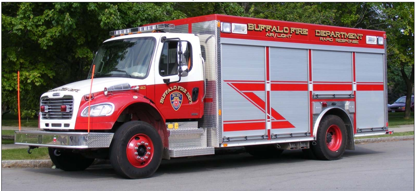
The airlight is a 2007 LaFrance build on a Freightliner M2-106 chassis.
