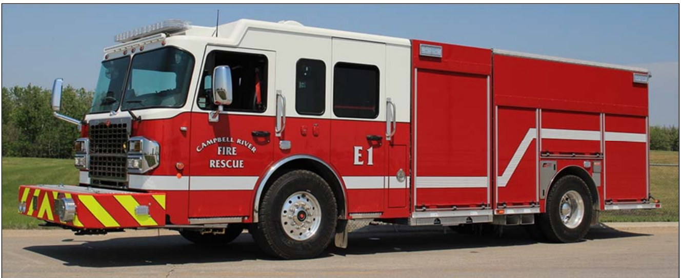
Campbell River, BC Engine 1, a 2018 Spartan Gladiator/Fort Garry pumper, with a 1750igpm Waterous pump, 500gwt and 42gft. s/n M867.
