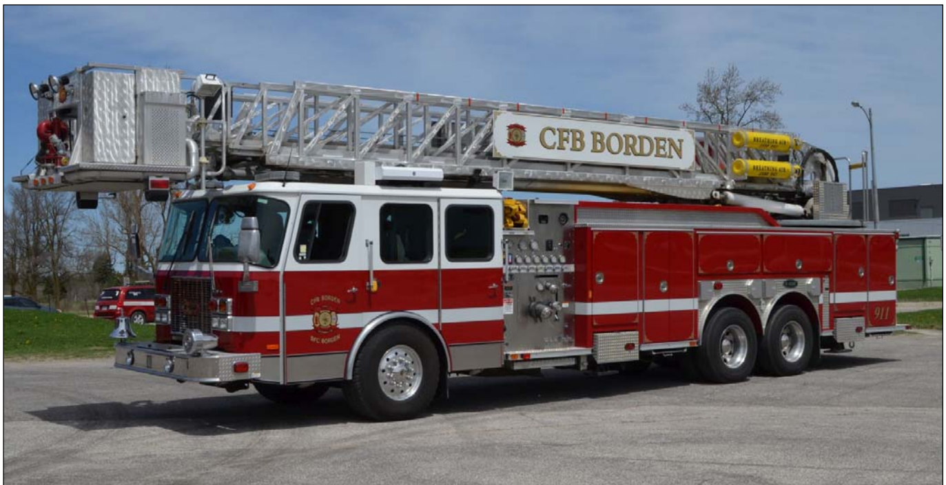
CFB Borden Red 2, a 2000 E-One Cyclone II quint, 1250igpm, 300gwt and 95' tower. S#20726
