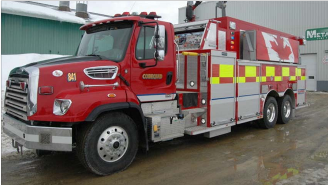
Cobequid Tanker 841, a 2018 Freightliner 114SD/Metalfab collaboration, 1500igpm Waterous pump, 2250gwt, FoamPro 2001 foam system. (MetalFab Fire Photos)
