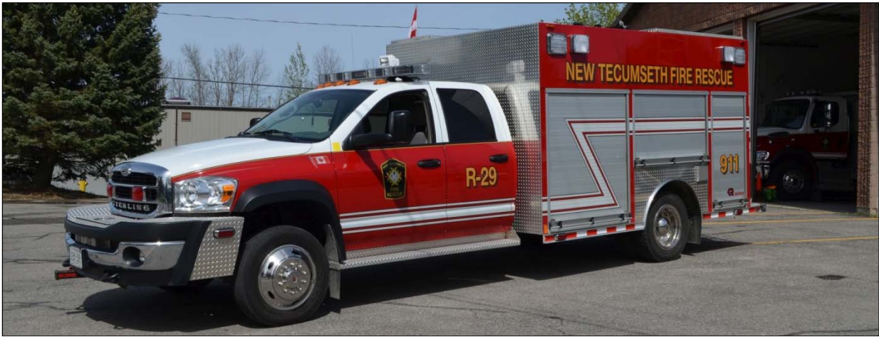
Rescue 29, a 2008 Sterling Bullet/Rosenbauer, Skid mount with a 250gwt
