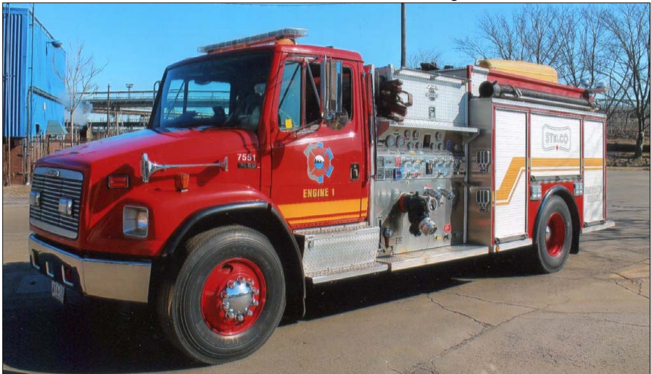
Engine 1, a 2002 Freightliner FL-70/LaFrance pumper, 1050igpm/500gwt/500gft. (Doug Holmes photos)
