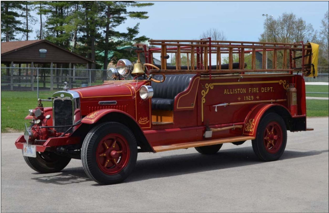
Alliston Parade Unit is this 1929 International/Lorne/Marsh with a front mount 250 gpm pump.
