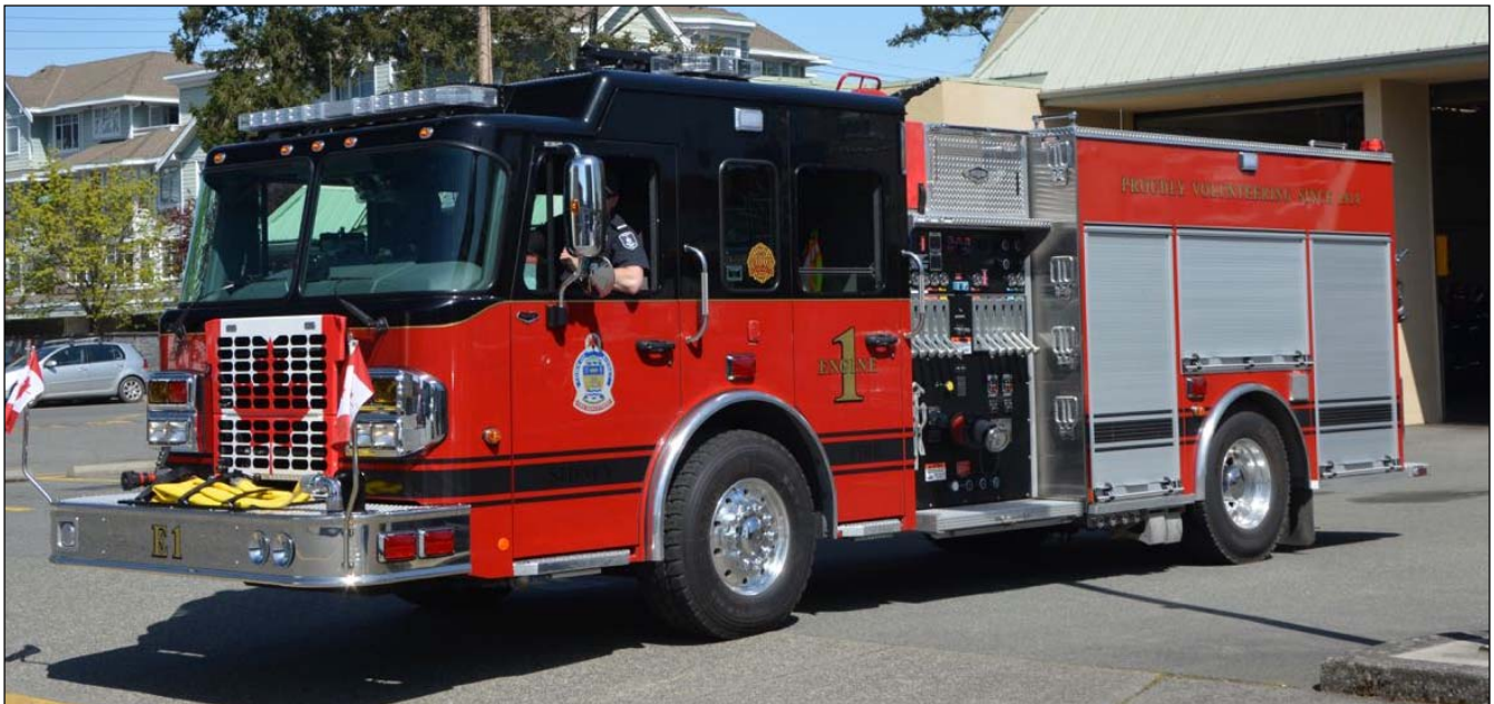
Sidney Engine 1 is a 2016 Hub Spartan MetroStarX with 1750/500/30 spec.s
