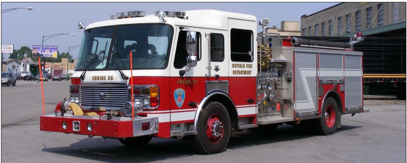
Engine 35, a 2005 American LaFrance Eagle/RD Murray job, 1500gpm/750gwt/30gft
