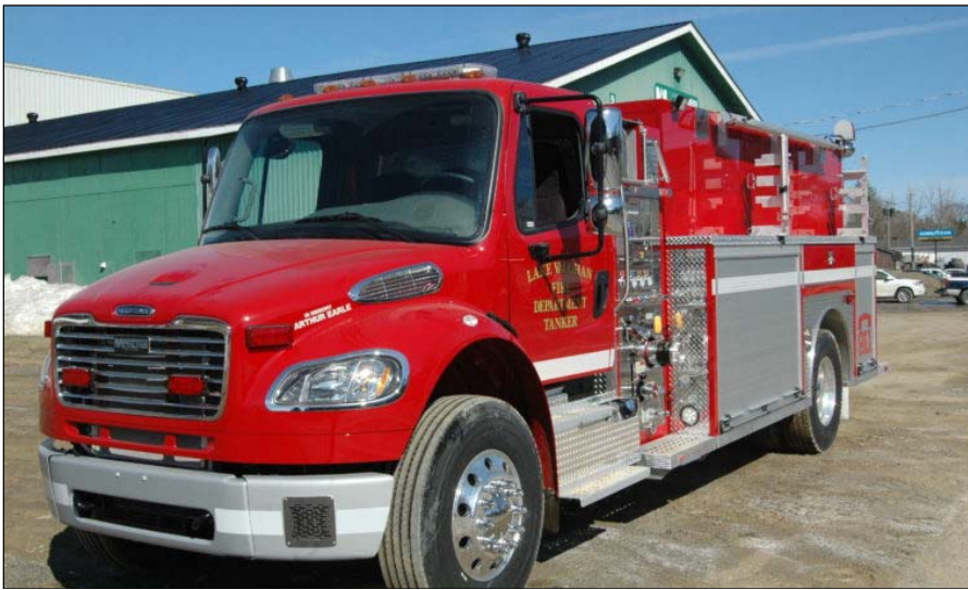
Lake Vaughn, NS, a 2018 Freightliner M2-106/Metalfab, 420igpm/1500gwt
