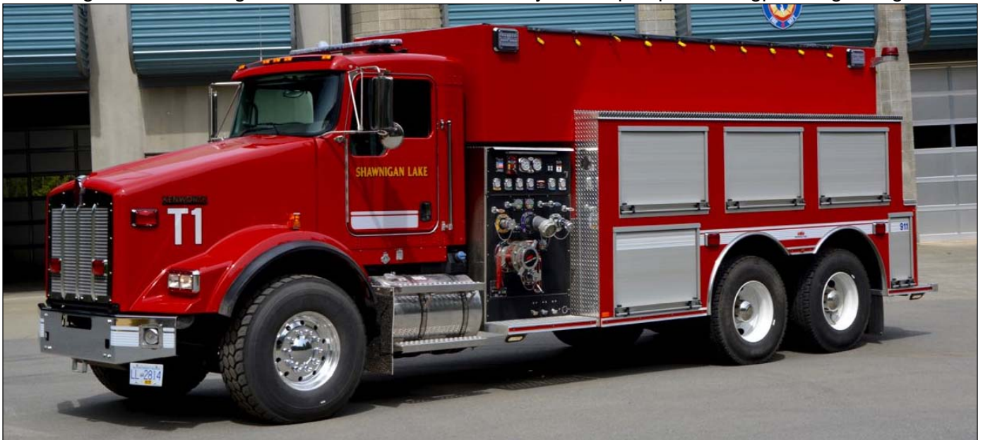
Tanker 1 in Shawnigan Lake is a 2017 Kenworth T800/Midwest product, 1250igpm pump, 3000gwt. (All photos by Terry Yip)
