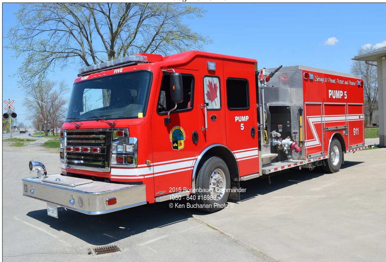
Fort Erie Pumper 5 is a 2015 Rosenbauer Commander rescue pumper with a 1050igpm pump and an 840gwt. S/N #16989 used to run as Heavy Rescue 5. (Ken Buchanan photos)
