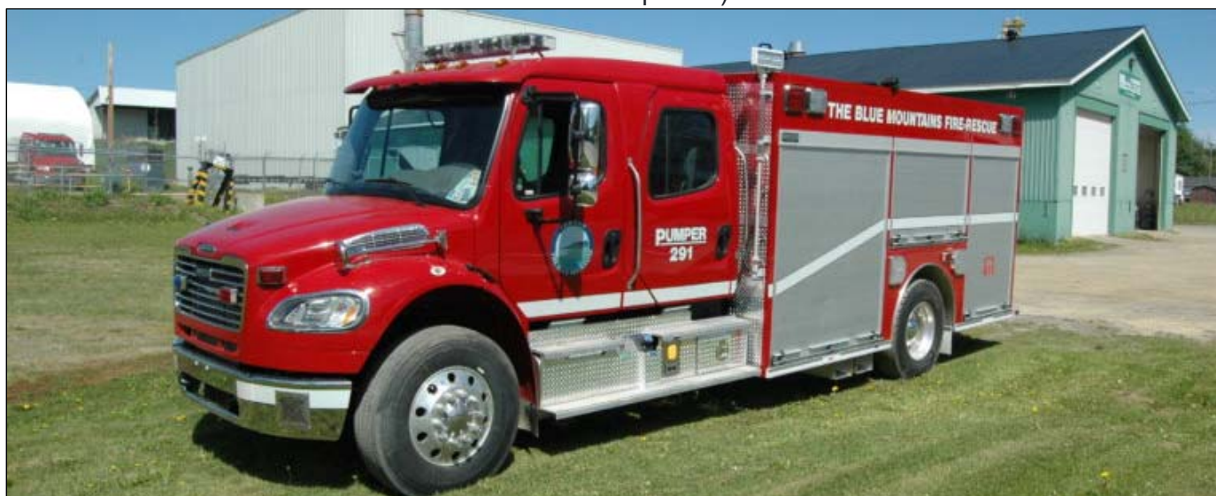
Blue Mountains Pump 291, a 2018 Freightliner M2-106Metalfab, 1250igpm/600gwt/25gft (Metalfab photo)
