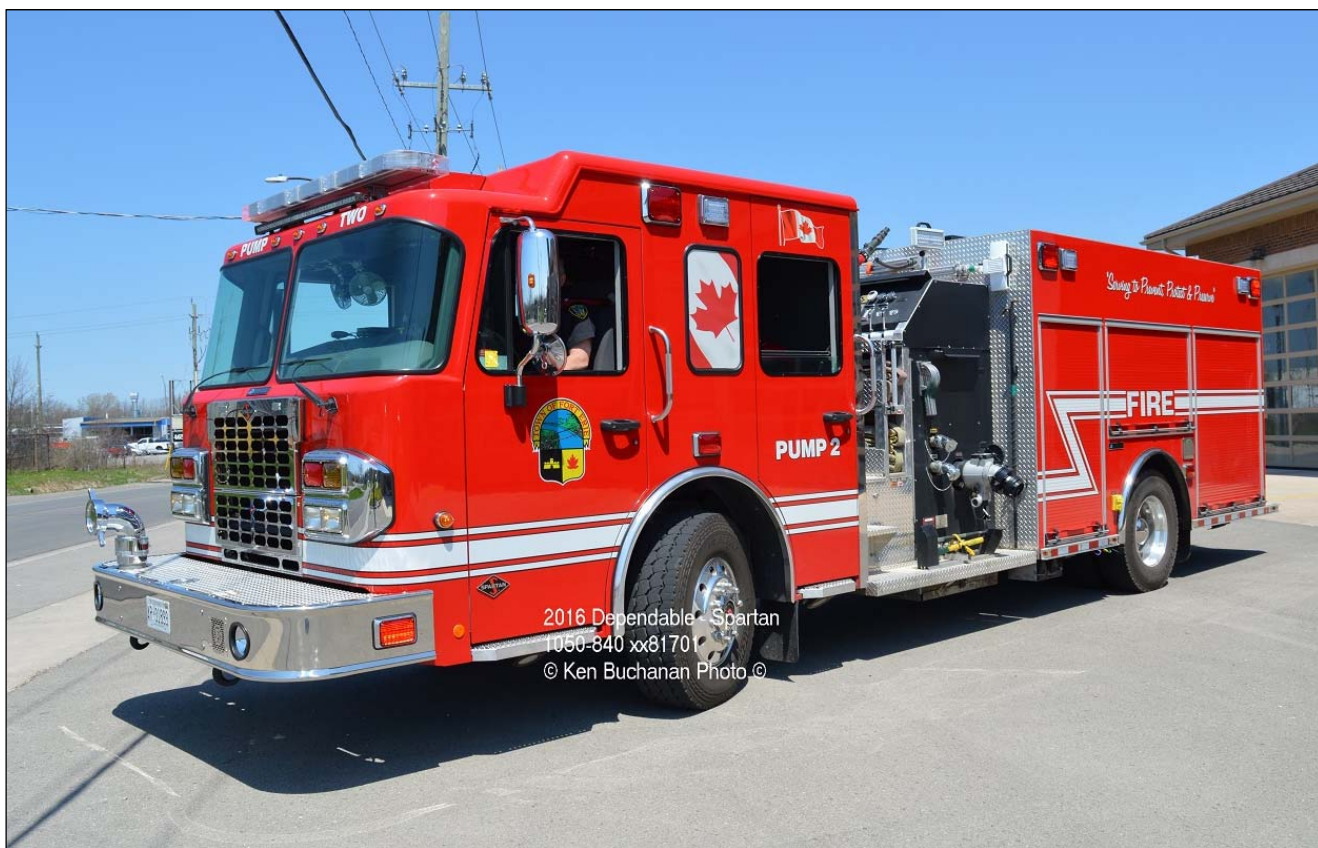
Fort Erie Pumper 2 is a 2016 Spartan Metro Star/Dependable, with a 1050igpm pump, 840gwt and 30gft s/n 81701
