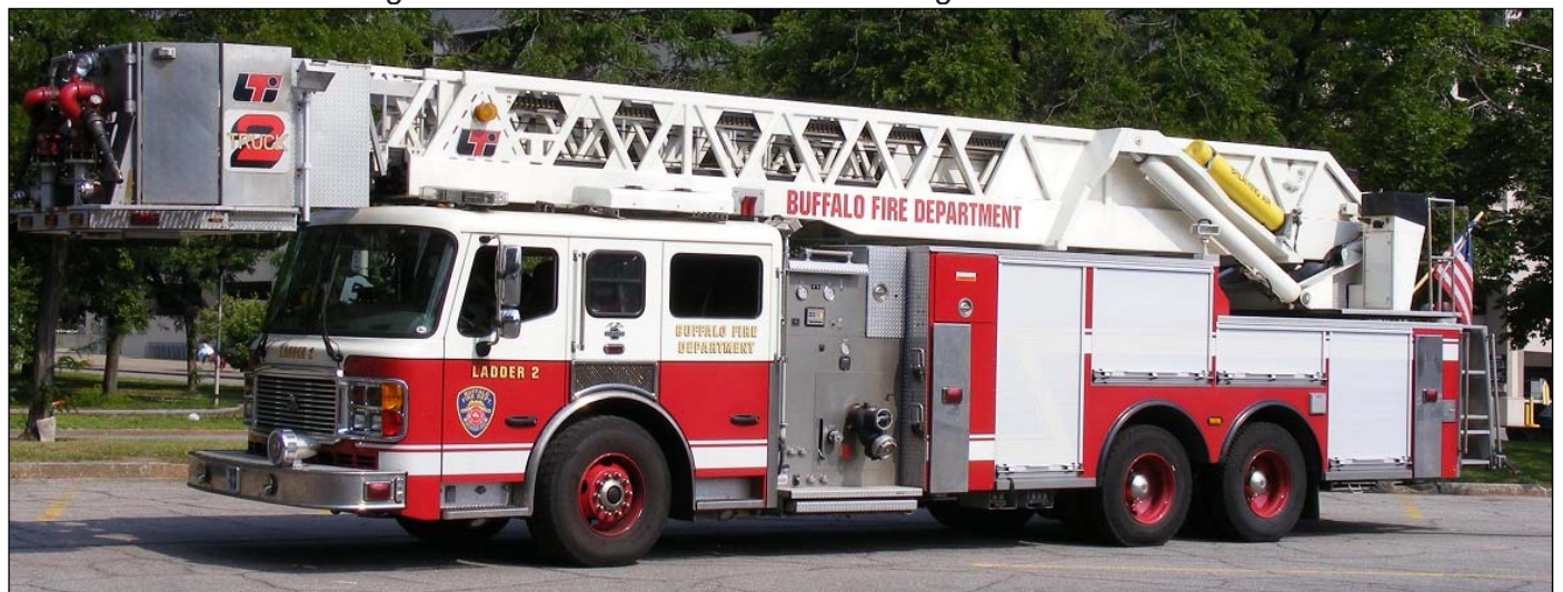
Former Truck 2, a 2005 ALF/LTI 2000gpm, 100' HPS rear-mount tower. (Neil McCarten photos)
