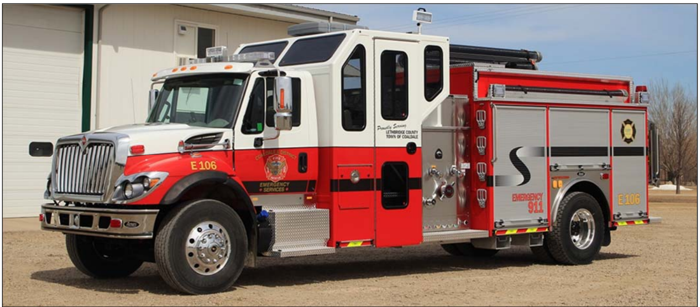
Coaldale, AB recently received this 2018 IHC 7400/Acres pumper, it's equipped with a 1050igpm pump, 1000gwt and 25gft. s/n 1803233163.
