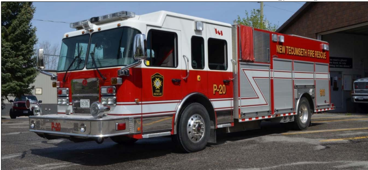
Pumper 20, a 2009 Spartan Metro Star/Rosenbauer 1500igpm/625gwt/40gft J#1459209
