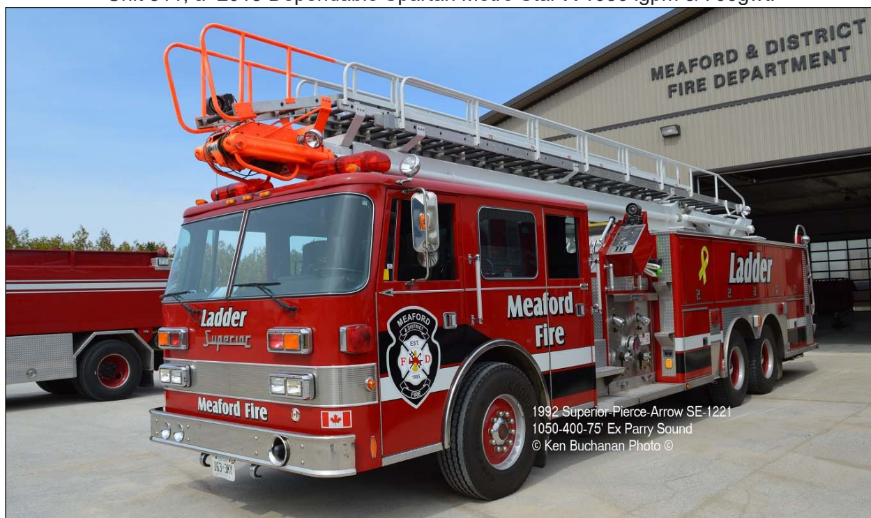
Unit 317, a 1992 Pierce Arrow/Superior quint with a 1050igpm pump, 400gwt and 75' Telesqurt SE-1221 (Ken Buchanan photos)
