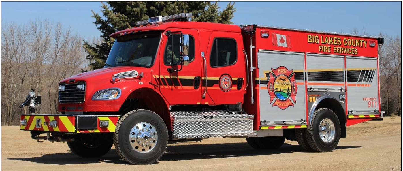
Recently delivered to Big Lakes County, AB, this 2018 Freightliner M2-106 4x4/Acres off-road rig has a 230igpm Waterous pump, 400gwt and a 20gft. s/n 180410164
