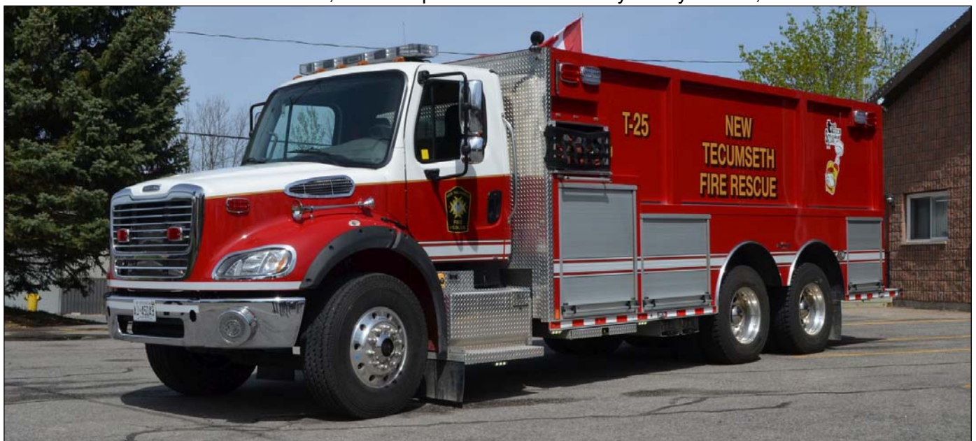
New Tecumseth Tanker 25, a 2014 Freightliner / Rosenbauer product, 840igpm/2500gwt V/N FHFZ7951 (Bob Rupert photos)
