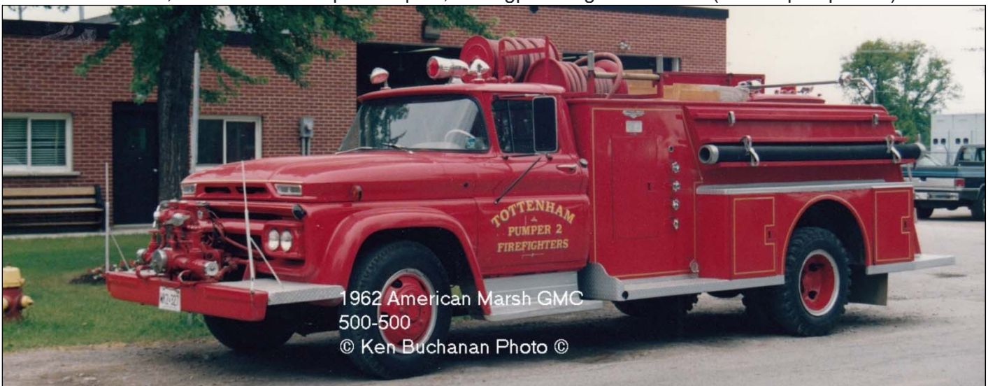
Finally, Tottenham station's parade rig, which could not be taken out on this trip, seen in 1992. It's a GMC/American Marsh with a 500igpm front-mount pump and 500gwt. (Ken Buchanan photo),
