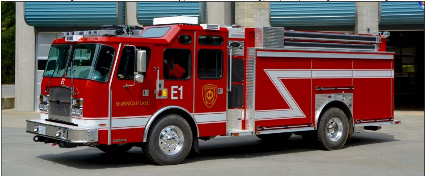
Engine 1 in Shawnigan Lake, BC is a 2017 E One Cyclone II pumper, 1555igpm/832gwt/25gft.
