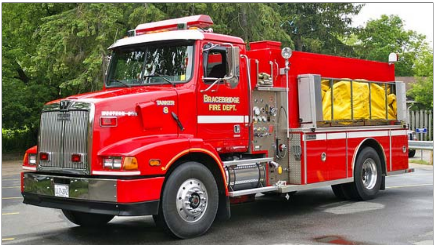
Taken on the tour, this is a shot of Bracebridge Tanker 8, a 1999 Western Star/Metalfab product with a 625igpm pump and 1500gwt. (SN#M99-8728)
