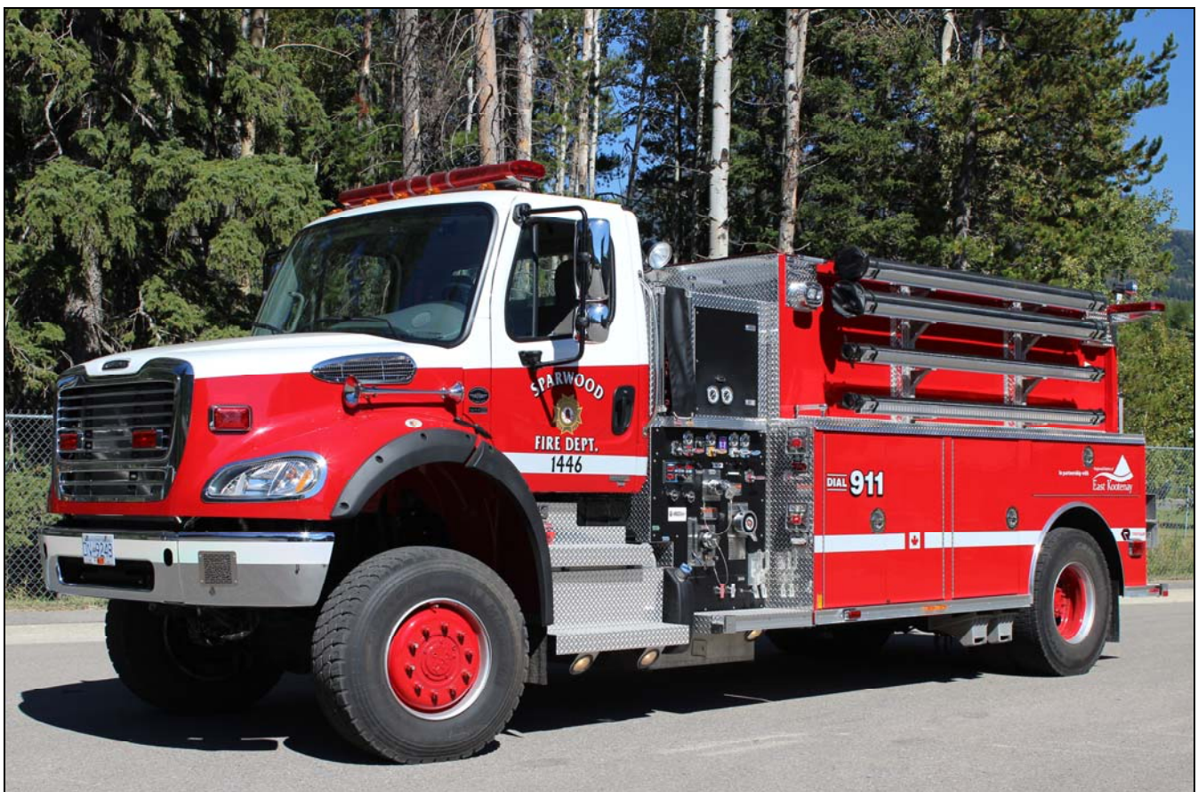
Sparwood Tender 1446, a 2011 Freightliner M2/Rosenbauer Central tanker with a 425igpm pump and 1800gwt.
