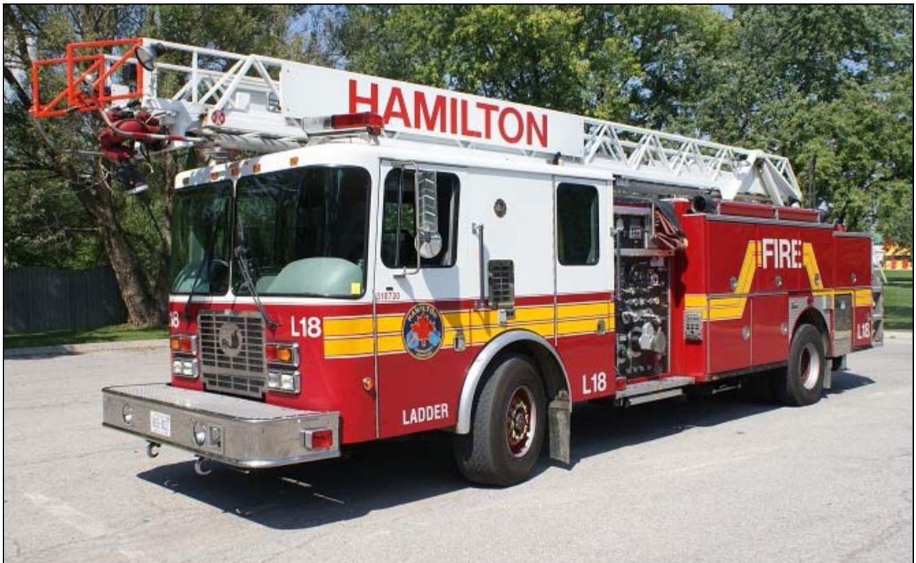
New to Station 18, this is a 1998 HME/Ferrara quint. Ladder 18 sports a 1050igpm pump, 500gwt and 65' aerial. (Ken Buchanan photo).
