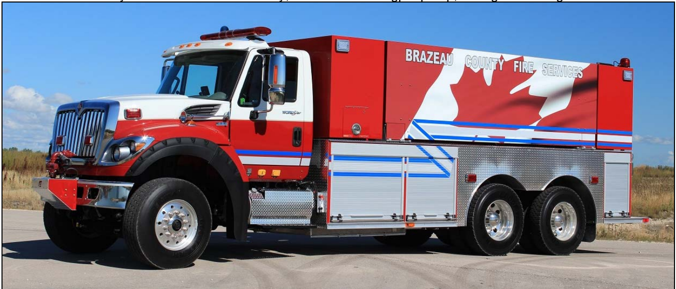
Above, Medicine Hat's new 2012 IHC 7600 4x4/Fort Garry 1050igpm, 1500gwt pumper. Below, a 2012 IHC 7600/ Fort Garry tanker for Brazeau County, AB. It has a 625igpm pump, 3000gwt and 25gft. s/n #M369.
