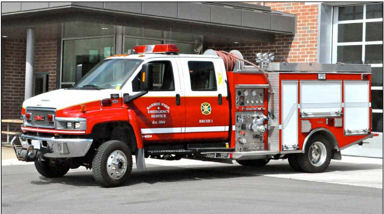
Barrie Brush 1, a 2006 GMC 5500 4x4/Seagrave pumper with a 420igpm pump and 300gwt. The rig runs from Station 1, downtown, and also tows the BFD airboat on a trailer.
