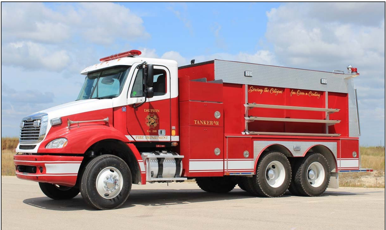
This is Dauphin, MB's new water carrier. Tanker 1 is a Heloc product on a 2012 Freightliner Columbia chassis. It carries 2500 gallons.
