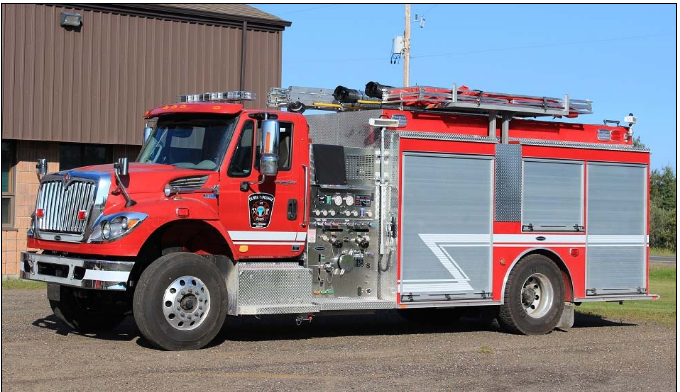
Oliver Paipoonge, a First Nations community in Northern Ontario, received this 2012 IHC 7400/Fort Garry Fire Trucks pumper-tanker during the summer. It has a 1050igpm pump, a 1200gwt and 25gft. s/n #15037
