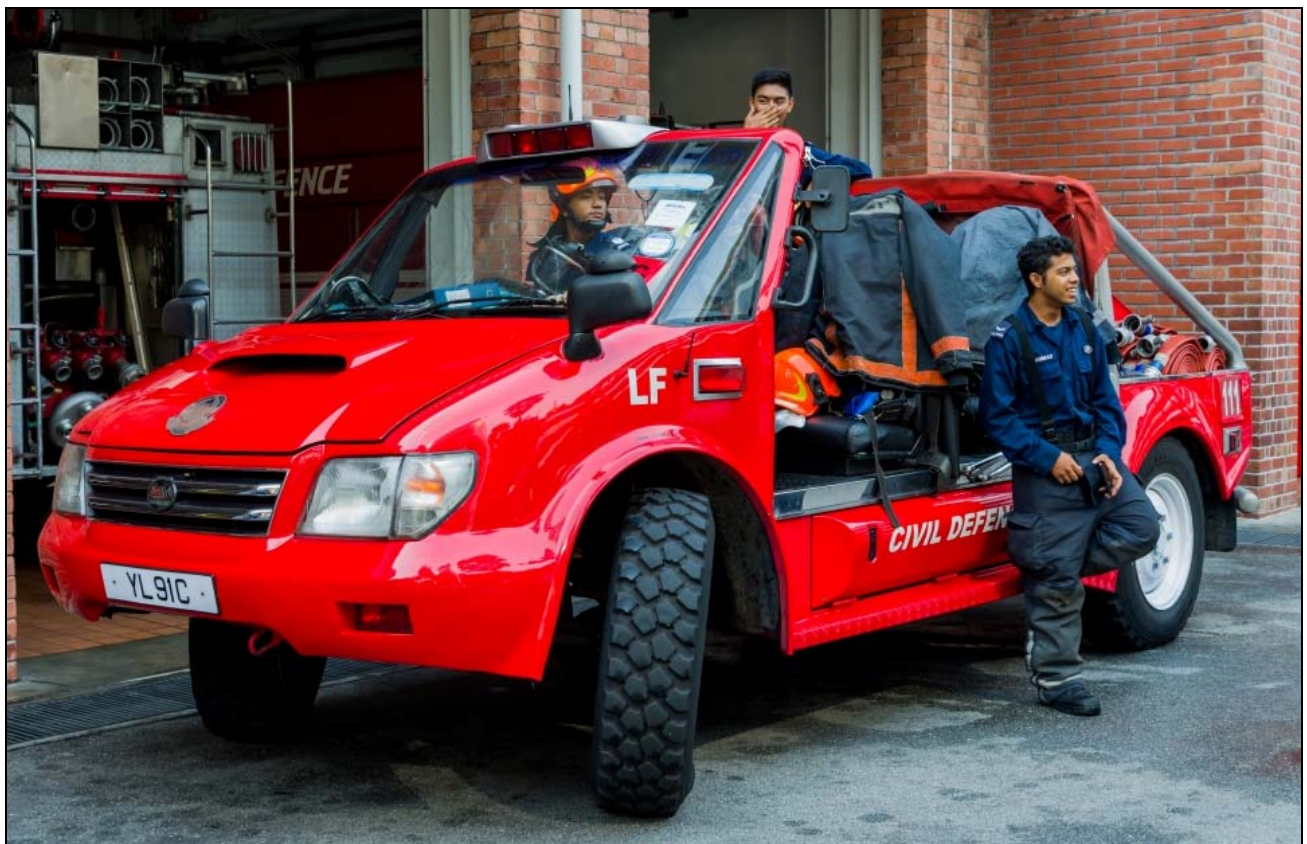
Also from Singapore is this Light Fire Attack Vehicle, also known as a Red Rhino. It is a 2002 Bucher Duro/Delgo light pump. They have 500gpm pumps, 150gfts and four-wheel drive. (photos by Kenneth Lai)
