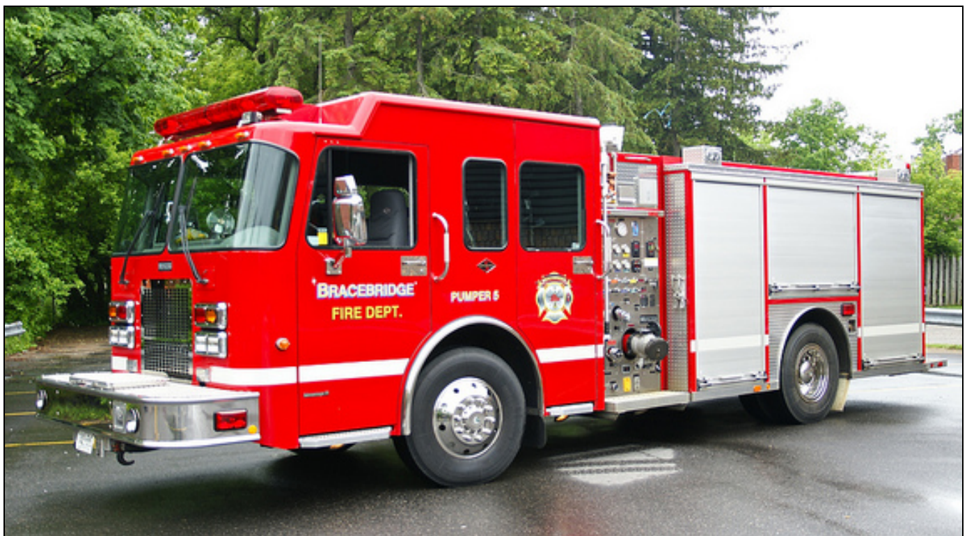
Also on the tour, Pumper 5, a 2003 Spartan Advantage/Metalfab with 1050igpm and 800gwt. Both rigs run from Station 1. (SN#M03-15413) (Jon Lasiuk photos).
