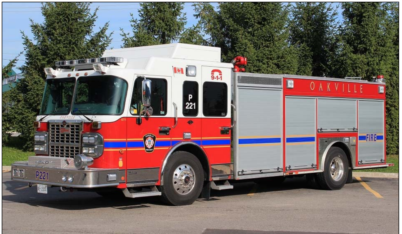
Oakville put into service this 2012 Carl Thibault pumper on a Spartan Gladiator chassis in Station 2. It's equipped with a 1250igpm pump, 725gwt and a 20gft. (Dave Stewardson photos)
