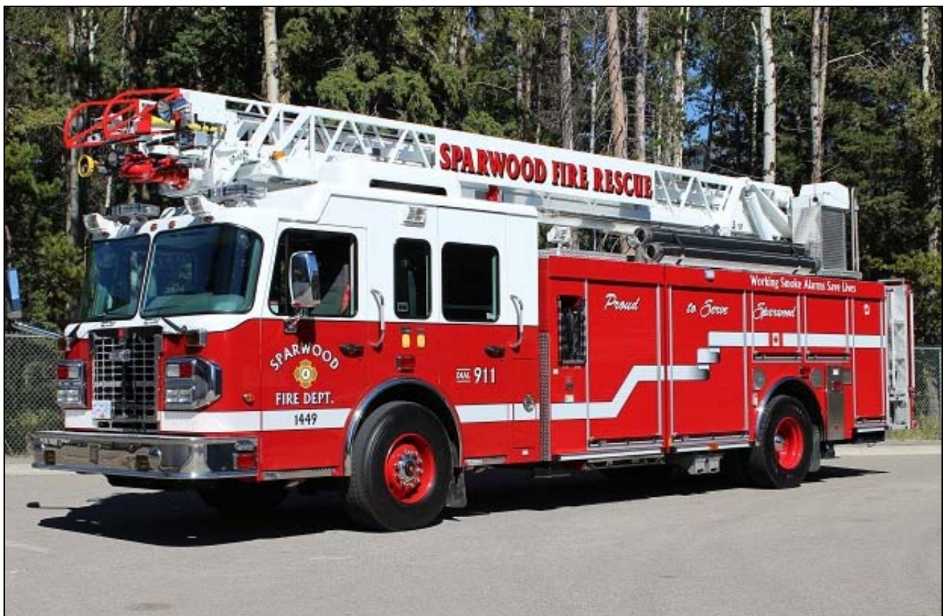
Sparwood Aerial 1449, a 2012 Spartan Metrostar/Smeal quint with a 1750igpm pump, 300gwt and 75' rear mount aerial. It carries serial numbers from Spartan, 75165 and Smeal, 214150. (John Bowerman photos).
