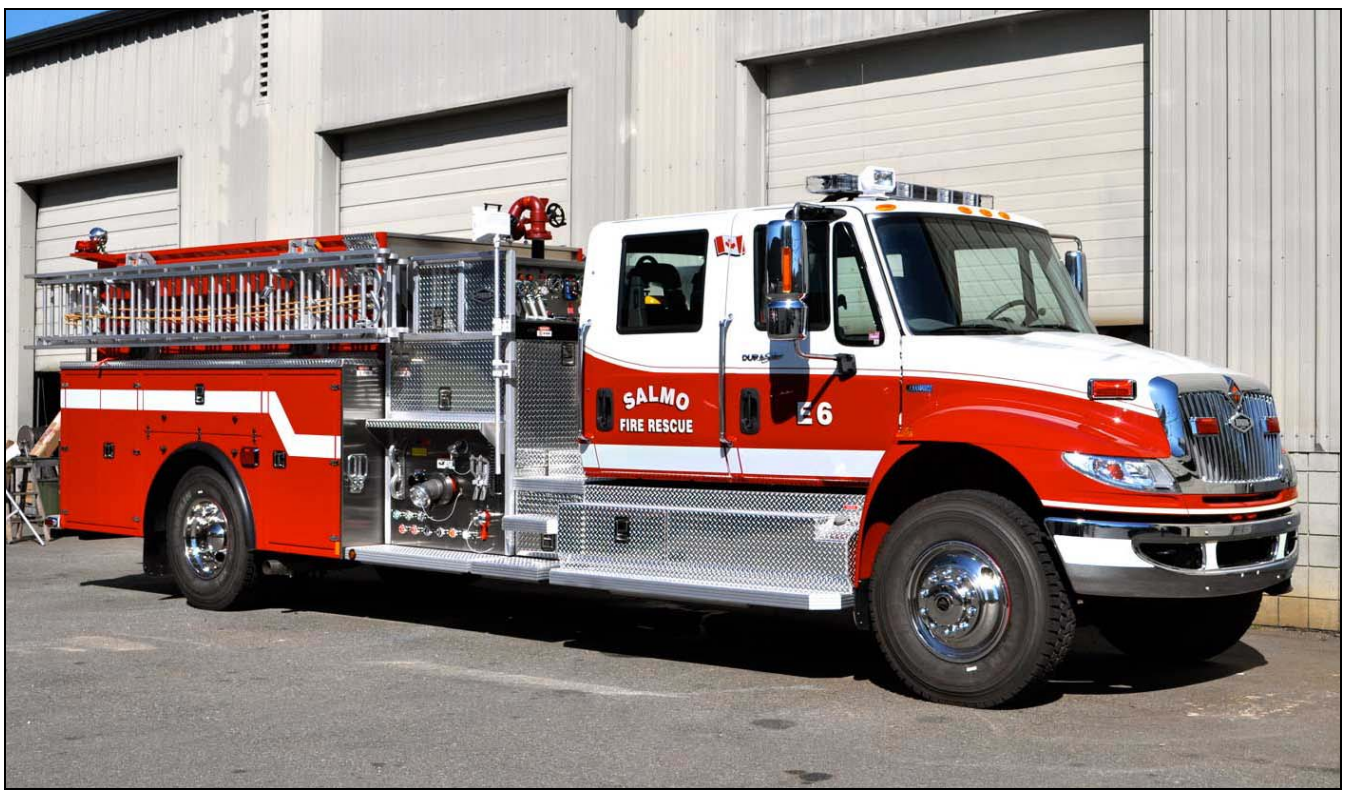
Salmo, BC Engine 6, a 2012 IHC 4400/Hub pumper-tanker with a 1050igpm pump, 1000gwt and 20gft.
