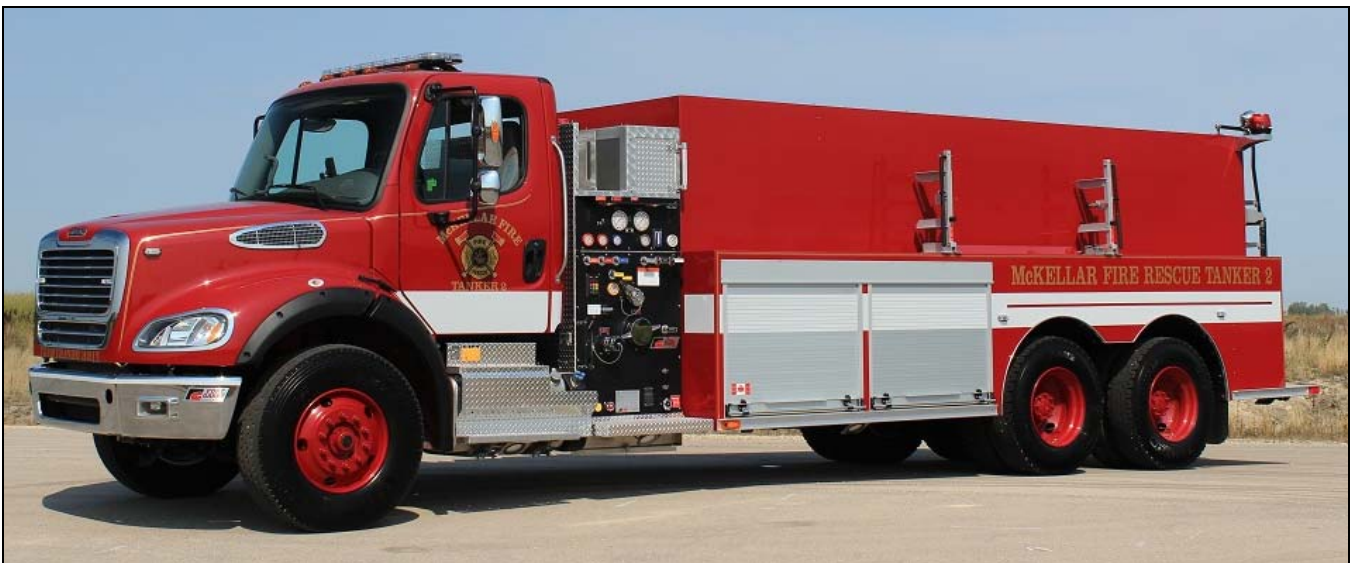
This 2012 Freightliner M2/Fort Garry product belongs to McKellar, ON. The long rig has an 840igpm pump and 2500gwt, running as Tanker 2. (s/n #M334) (Dave Stewardson photos)
