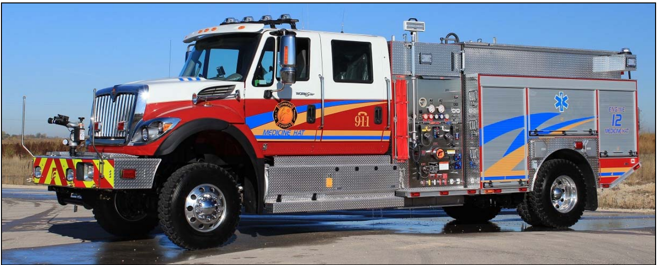
Above, Medicine Hat's new 2012 IHC 7600 4x4/Fort Garry 1050igpm, 1500gwt pumper. Below, a 2012 IHC 7600/ Fort Garry tanker for Brazeau County, AB. It has a 625igpm pump, 3000gwt and 25gft. s/n #M369.
