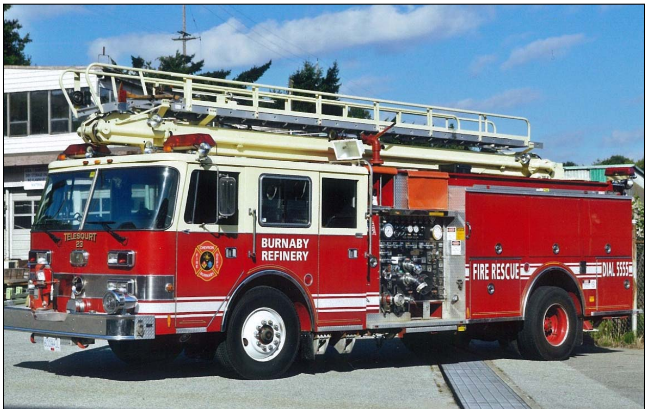
Telesqurt 23 of the Burnaby Chevron Refinery, a 1989 Pierce Arrow XT quint with a 1750igpm pump, 700igft and 50' telesqurt. (Terry Yip photos)
