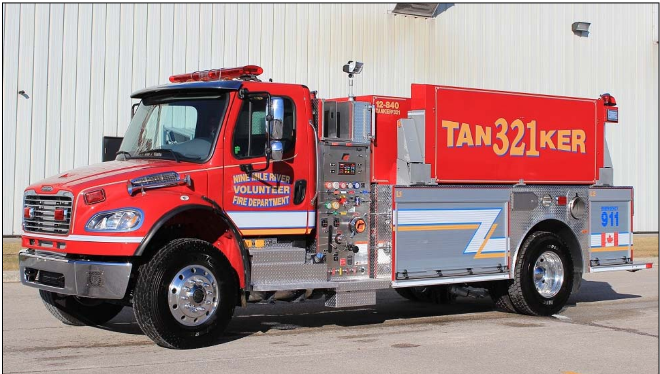
Nine Mile River, NS Tanker 321 is a Fort Garry product on a 2012 Freightliner M2 chassis with an 840igpm pump and a 1500gwt. (Dave Stewardson photos)
