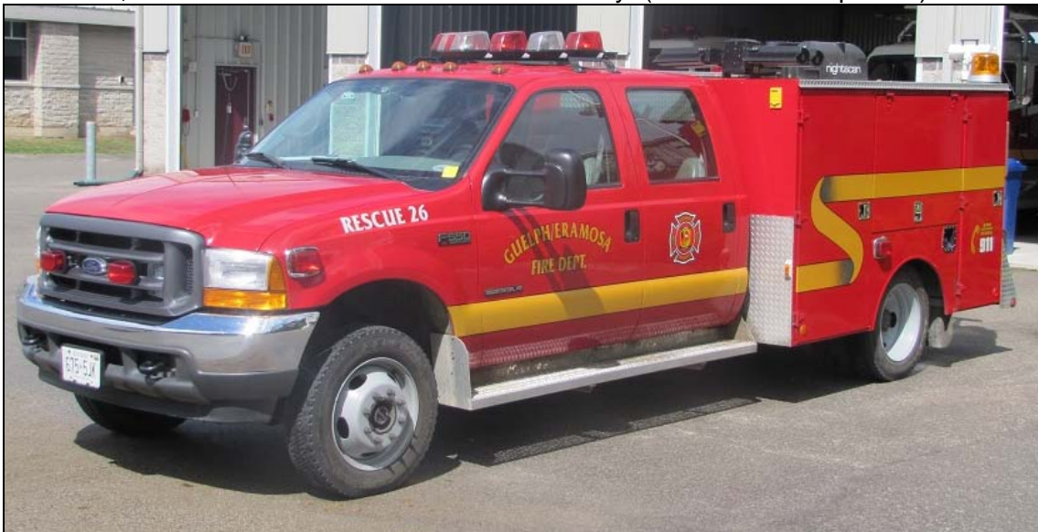
From the recent tour, these are two of Guelph/Eramosa Twps. FD's rigs. Above is Pumper 21, a 1999 Freightliner/Superior 1050igpm/600gwt/20gft (SN SE2030), below, Rescue 26, a 2001 Ford F550 4x4 with a Wilcox body. (Desmond Brett photos)
