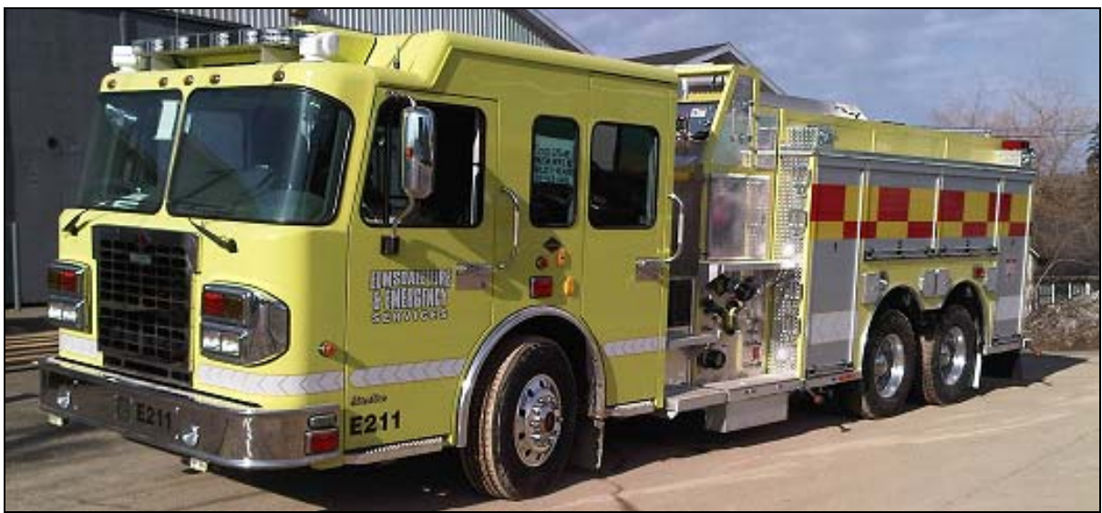
Elmsdale, NS E.211 runs this 2012 Spartan Metro Star/Metalfab pumper tanker. It has a 1050 igpm pump, 1200gwt and 2x20gft, also a FoamPro 2002 foam system. (Photo credit: Elmsdale FES)
