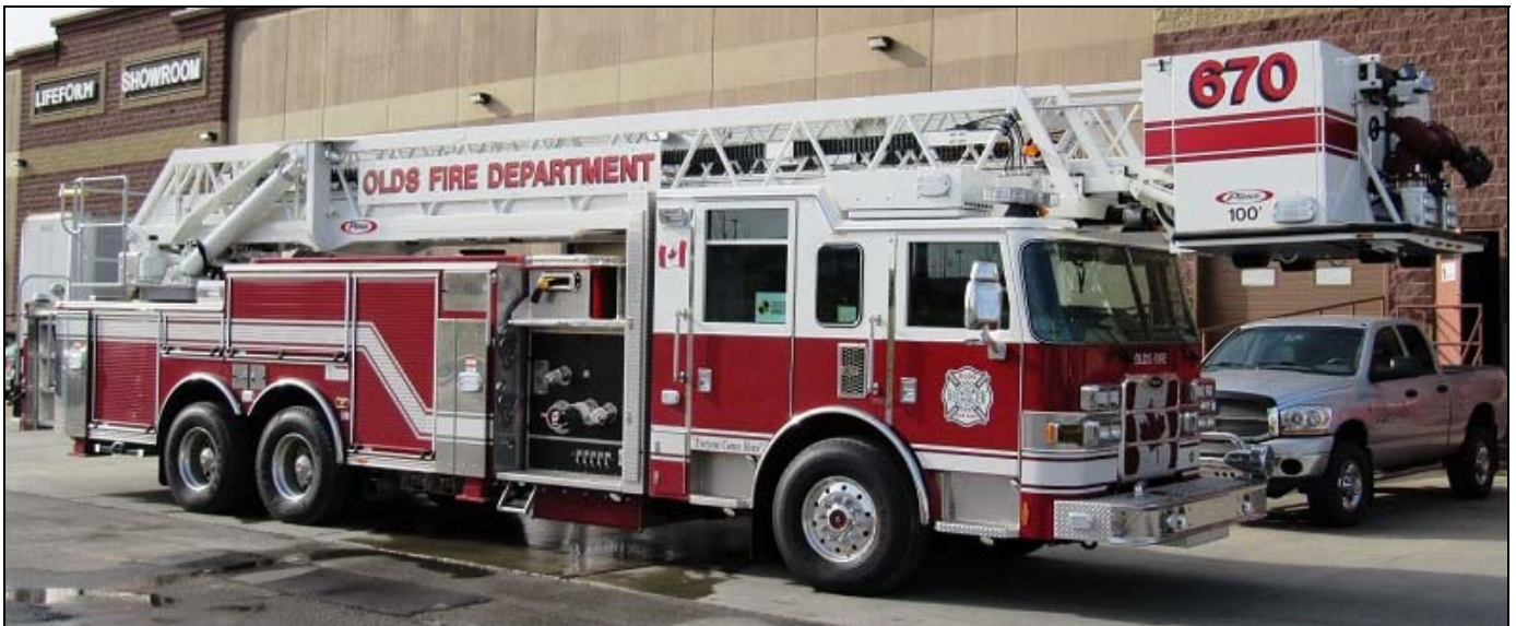
Slightly older vintage is this 2010 Pierce Arrow XT tower in Olds, AB. Unit 670 has a 1750igpm pump, 270gwt and a 100' ladder tower. (John Bowerman photo)
