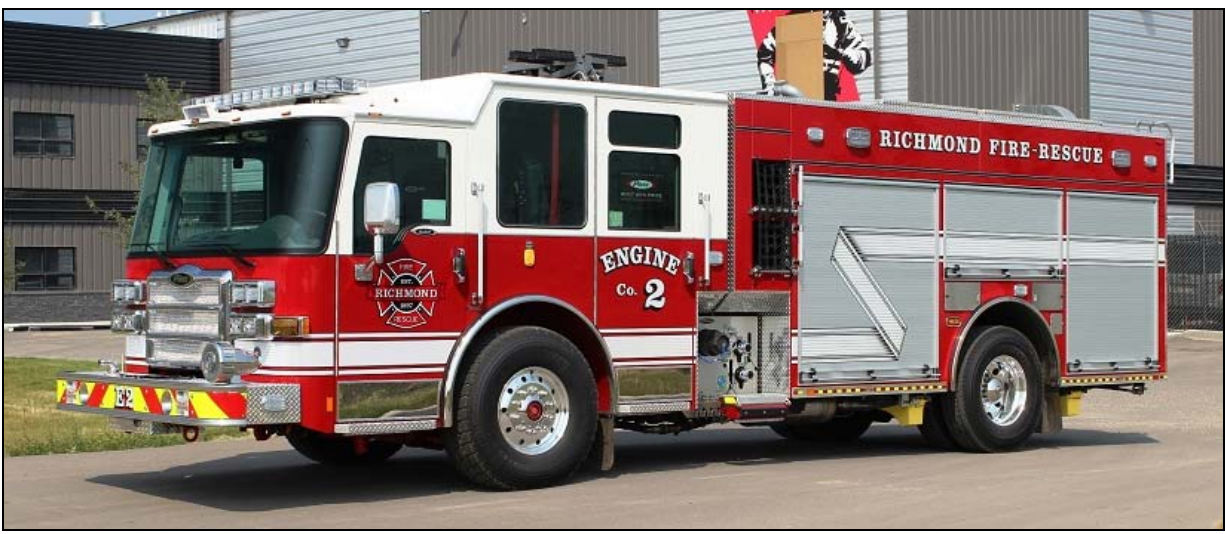
New to Richmond, B.C. is this 2014 Pierce Dash CF PUC pumper equipped with a 1250igpm Waterous pump, 350gwt, and 40gft (SN 27210). Also new from Pierce is Ladder 7, a 2014 Dash CF PUC quint with 1250igpm pump, 350gwt, 40gft and 105' stick. (SN 27211) (Terry Yip photos)
