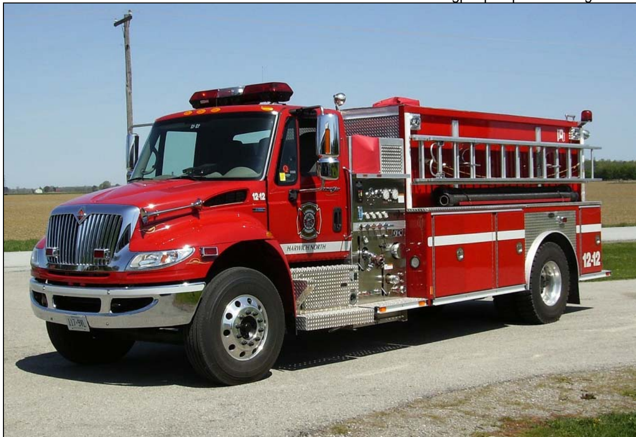
Another pair from Chatham-Kent, above is a 1984 Ford/Childs command unit, formerly with North Harwich. Unit 12-12 below is a 2007 IHC/E-One tanker with a 400igpm pump and 1250gwt.
