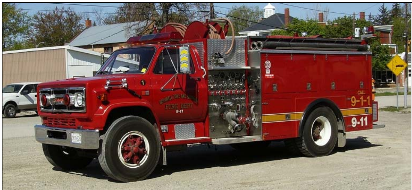
Three items from Chatham-Kent, Station 9 in Bothwell. All three served with the Bothwell-Zone-Euphemia prior to the 1998 amalgamation. Top-most is CKFS 9-11, a 1987 GMC/Hub pumper with 625igpm pump and 500gwt. 912 below is a 1995 GMC/Robina tanker with a 400igpm pump and 1800gwt. Last is a 1991 Ford/Champion command unit. (Neil McCarten photos)
