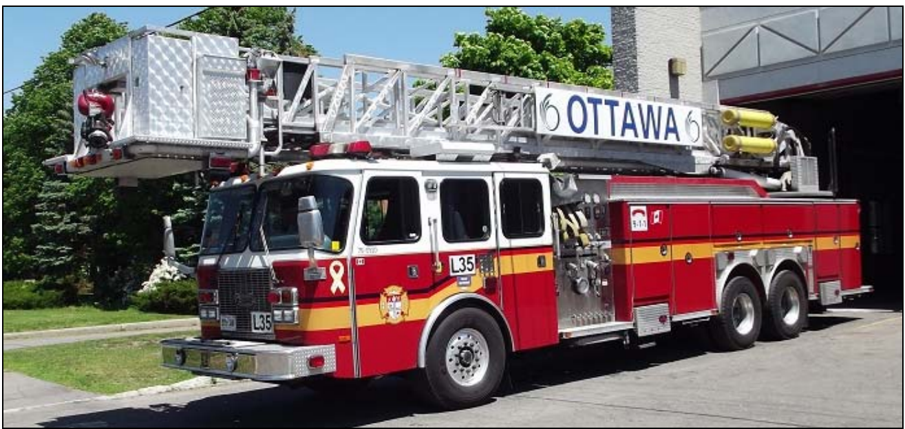
A pair from Ottawa. Ladder 35 is a 2002 E-One Cyclone II tower with a 1750gpm pump, 300gwt and 95' tower. Pump 35 is a 2006 Spartan/CarlThibault with a 1250gpm pump and 500gwt. (Rick Loiselle photo)
