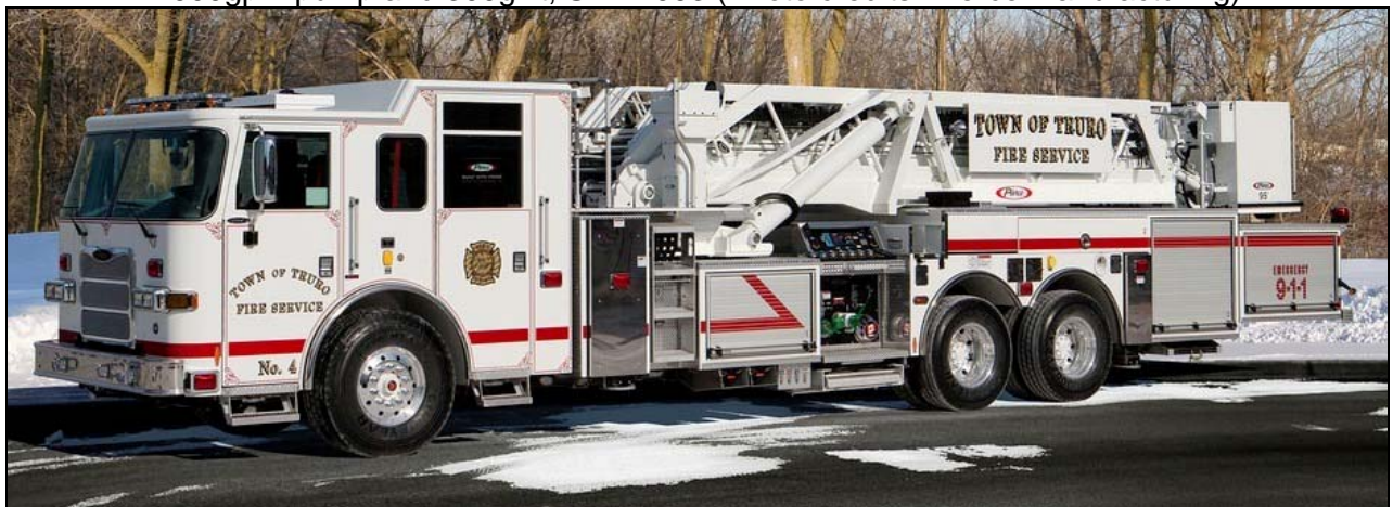
Moncton, NB Truck 4 is a 2013 Pierce Impel rearmount with a 1750gpm pump, 500gwt and 75' aerial. Truro, NS received this 2014 Pierce Arrow XT 95' tower earlier this year. It has a 2000gpm pump and 300gwt, SN 27093 (Photo credits: Pierce Manufacturing)
