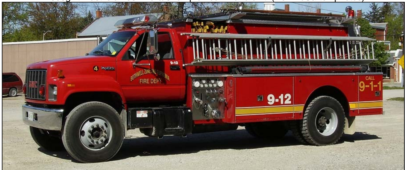
Three items from Chatham-Kent, Station 9 in Bothwell. All three served with the Bothwell-Zone-Euphemia prior to the 1998 amalgamation. Top-most is CKFS 9-11, a 1987 GMC/Hub pumper with 625igpm pump and 500gwt. 912 below is a 1995 GMC/Robina tanker with a 400igpm pump and 1800gwt. Last is a 1991 Ford/Champion command unit. (Neil McCarten photos)
