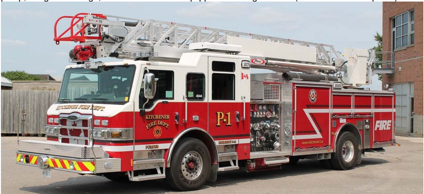
And Kitchener's new Pump 1, a 2014 Pierce Impel 1666igpm/416gwt/18gft/75' aerial. (Gary Dinkel photo)
