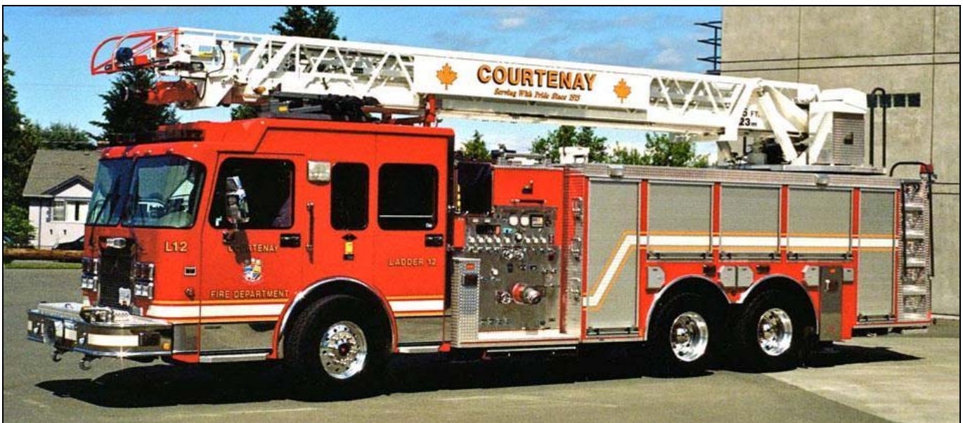
Courtenay Ladder 12 is a 2002 Spartan Galdiator Smeal quint with a 1750igpm pump, 500gwt, 30gft and 75' aerial. SN 202040. (Terry Yip photos)
