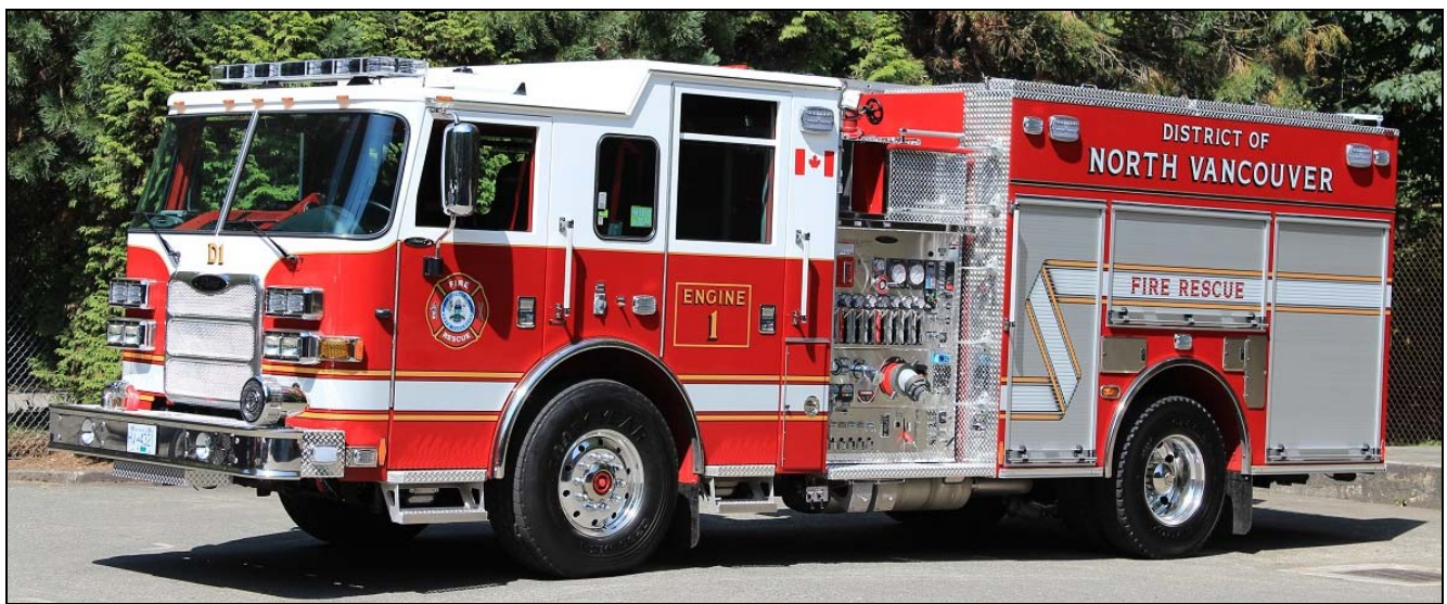
North Vancouver District just put this 2014 Pierce Arrow XT pumper into service at Engine 1. It features a 1750igpm Waterous pump, 330gwt, 25gft, and a Husky Foam System, Serial # 27192.
