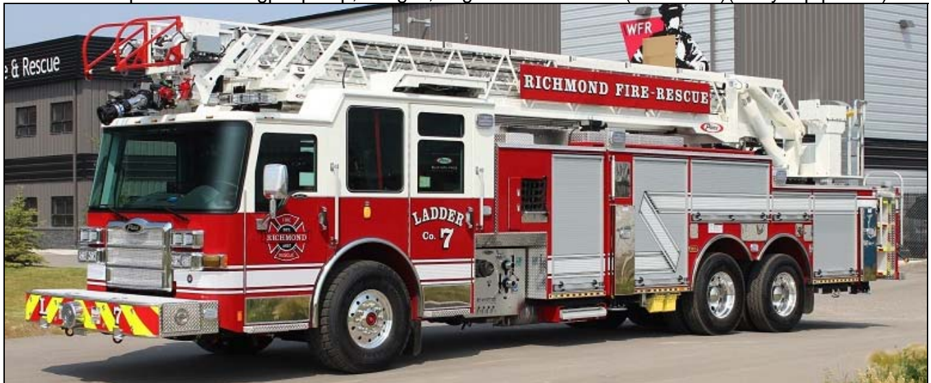
New to Richmond, B.C. is this 2014 Pierce Dash CF PUC pumper equipped with a 1250igpm Waterous pump, 350gwt, and 40gft (SN 27210). Also new from Pierce is Ladder 7, a 2014 Dash CF PUC quint with 1250igpm pump, 350gwt, 40gft and 105' stick. (SN 27211) (Terry Yip photos)
