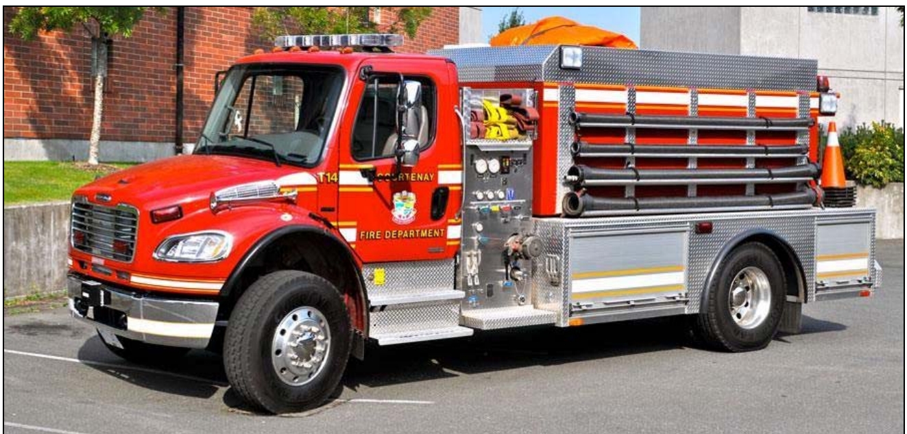
Courtenay, BC Tanker 14, a 2007 Freightliner M2-106/H Commercial Body 420igpm(H)/1700gwt, Rescue 71 is a 1992 American Fire & Rescue body on a 2013 Spartan chassis, conversion done by Fort Garry.
