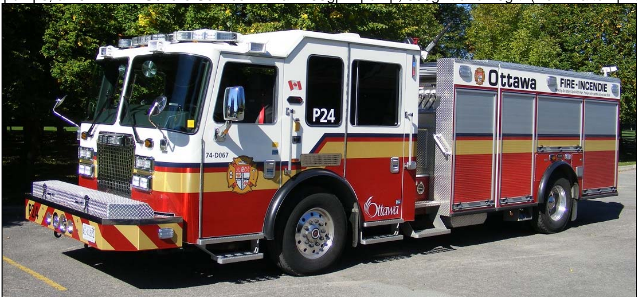
New to Ottawa, above: Car 20, the Western District Chief. It's a 2013 Chevrolet Tahoe, below: one of the new pumps, a 2014 KME Severe Service with a 1250gpm pump, 600gwt and 20gft. (Ken Walton photos)
