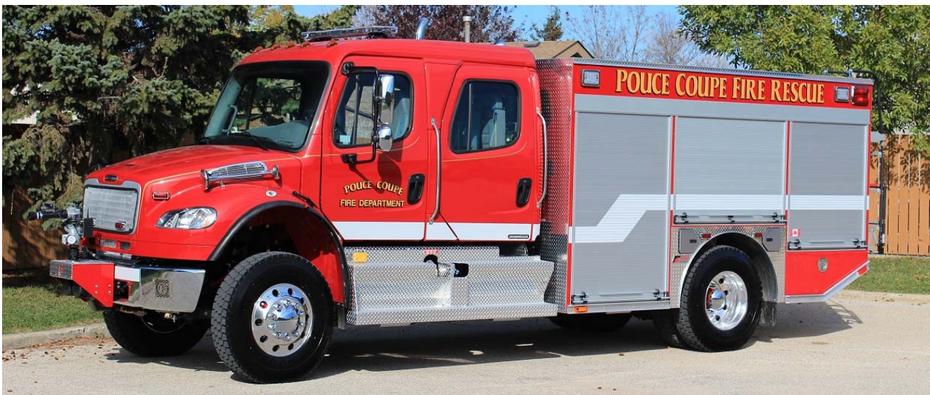
This is Pouce Coupe, BC's new 2014 Freightliner M2-106/Fort Garry pumper. It has a 1050igpm, 1000gwt, 25gft and CAFS, It bears s/n M567. (Dave Stewardson photo)
