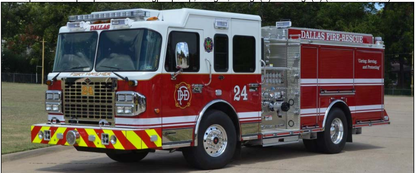
More from the Dallas IFBA Convention, Brush 54, above, is a new Type 3 brush truck, a 2014 International Maxx 4x4/SVI with a 500gpm pump, 500gwt, 20gft(A). (SN#150141). Engine 24 is a 2014 Spartan /SVI pumper with a 1500gpm pump, 500gwt, a 15gft(A) and 30gft(B) (SN#213103-05)
