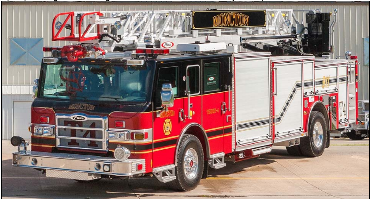
Moncton, NB Truck 4 is a 2013 Pierce Impel rearmount with a 1750gpm pump, 500gwt and 75' aerial. Truro, NS received this 2014 Pierce Arrow XT 95' tower earlier this year. It has a 2000gpm pump and 300gwt, SN 27093 (Photo credits: Pierce Manufacturing)
