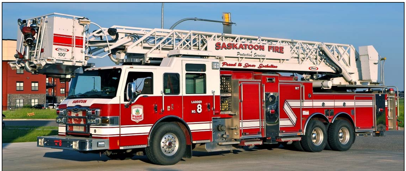
Ladder 8 is a 2010 Pierce Velocity PUC quint with a 1750igpm pump, 300gwt and 100' ladder tower. It is located at 8 Station. (All Saskatoon photos courtesy Terry Yip)
