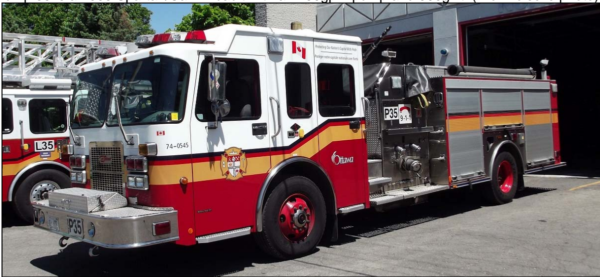
A pair from Ottawa. Ladder 35 is a 2002 E-One Cyclone II tower with a 1750gpm pump, 300gwt and 95' tower. Pump 35 is a 2006 Spartan/CarlThibault with a 1250gpm pump and 500gwt. (Rick Loiselle photo)
