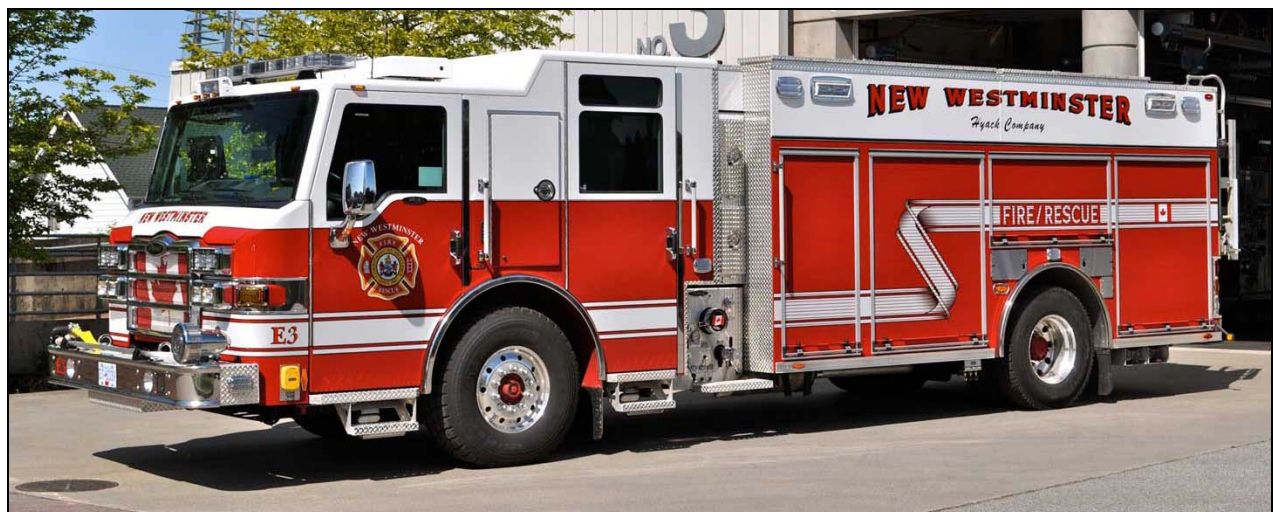
New Westminster Engine 3 is a 2012 Pierce Velocity PUC pump with 1250gpm, 420gwt and 40gft. (Dave Stewardson photos)
