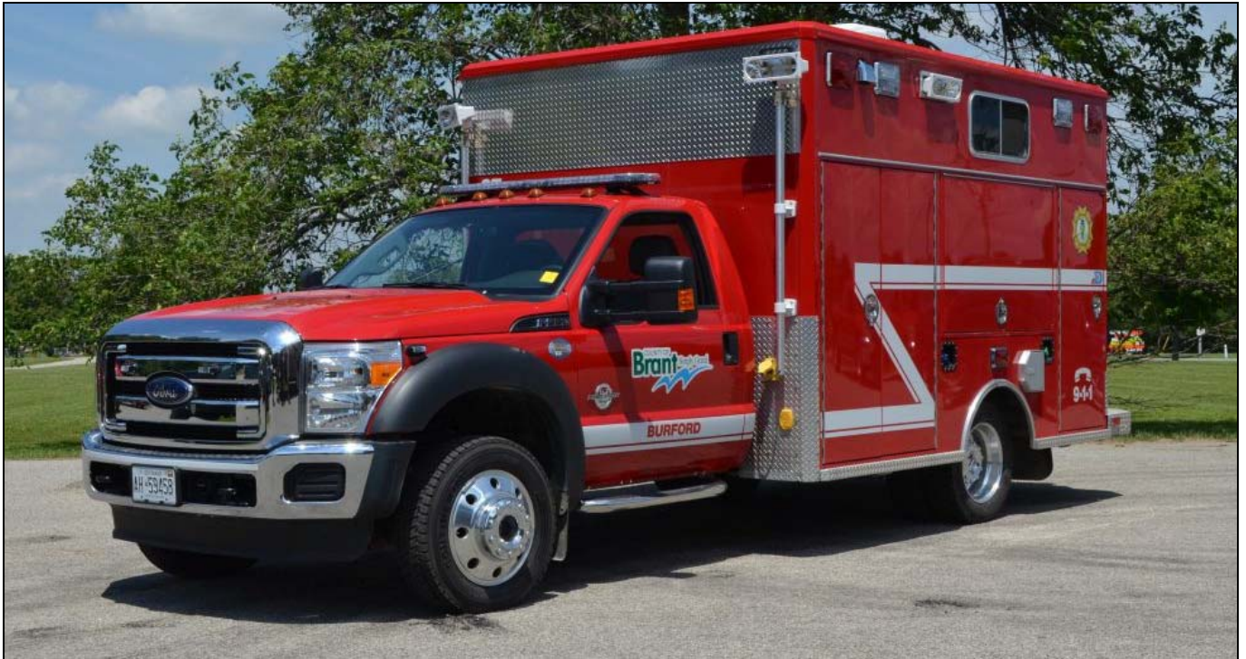
Brant County Rescue 37 which features a remounted 1992 Sentinel body (ex Richmond Hill, ON) on a 2014 Ford F550 chassis, the work was done by Dependable.
