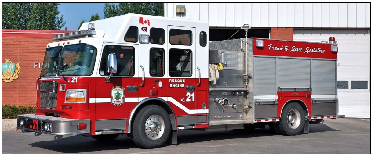
Terry Yip enjoyed a successful tour of Saskatchewan's second city last month with great results. First up; Saskatoon Rescue Engine 21, a 2009 Spartan Rosenbauer pumper has a 1500gpm pump, a 500gwt and two 25gfts. It runs from Station 2.
