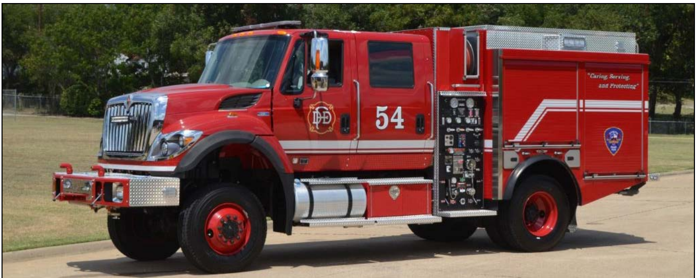
More from the Dallas IFBA Convention, Brush 54, above, is a new Type 3 brush truck, a 2014 International Maxx 4x4/SVI with a 500gpm pump, 500gwt, 20gft(A). (SN#150141). Engine 24 is a 2014 Spartan /SVI pumper with a 1500gpm pump, 500gwt, a 15gft(A) and 30gft(B) (SN#213103-05)
