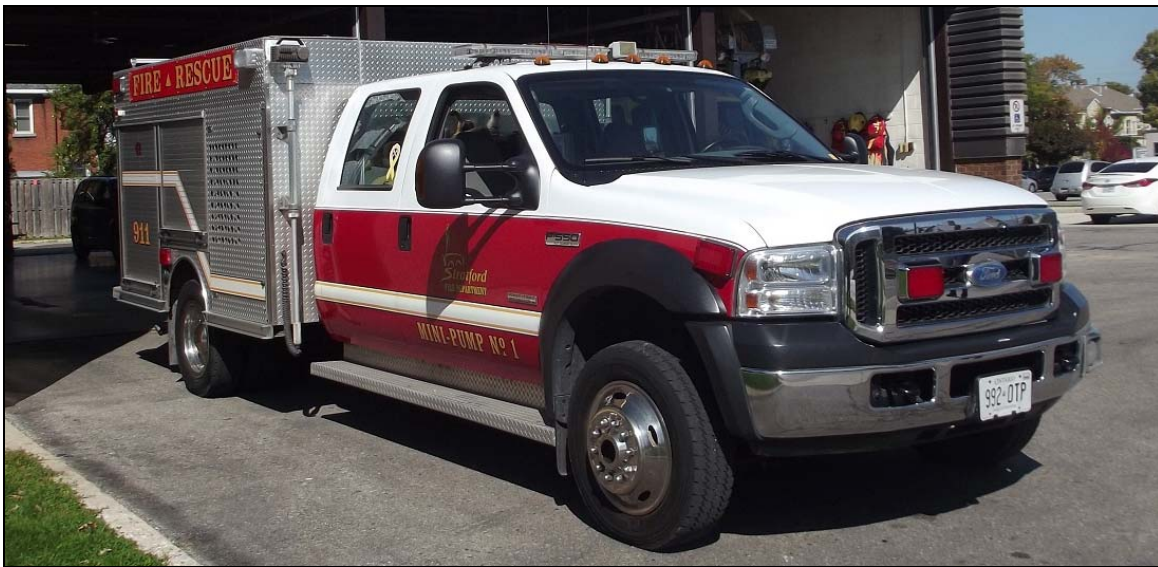
A pair from Stratford: Mini-pump 1 is a 2007 Ford F550/Rosenbauer 420/250/20, Pumper 2 is a 2008 Spartan/Rosenbauer 1050/625/2x20F, with rear mount pump. (Rick Loiselle photos)
