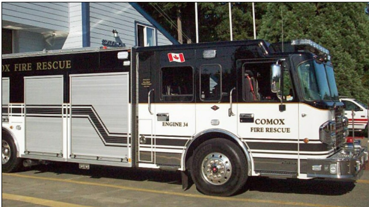
Photo courtesy Comox Fire Rescue twitter feed. E.34 is a 2011 Spartan Metro Star/Hub 1750/700/30.
