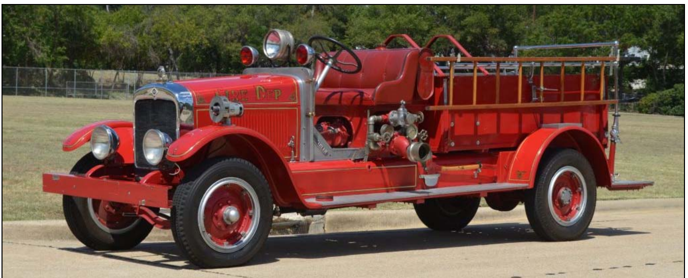
This 1923 Southern pumper was built in Dallas, and features a 500 gpm rotary gear pump. It was restored as a parade rig. (All photos courtesy Bob Rupert).
