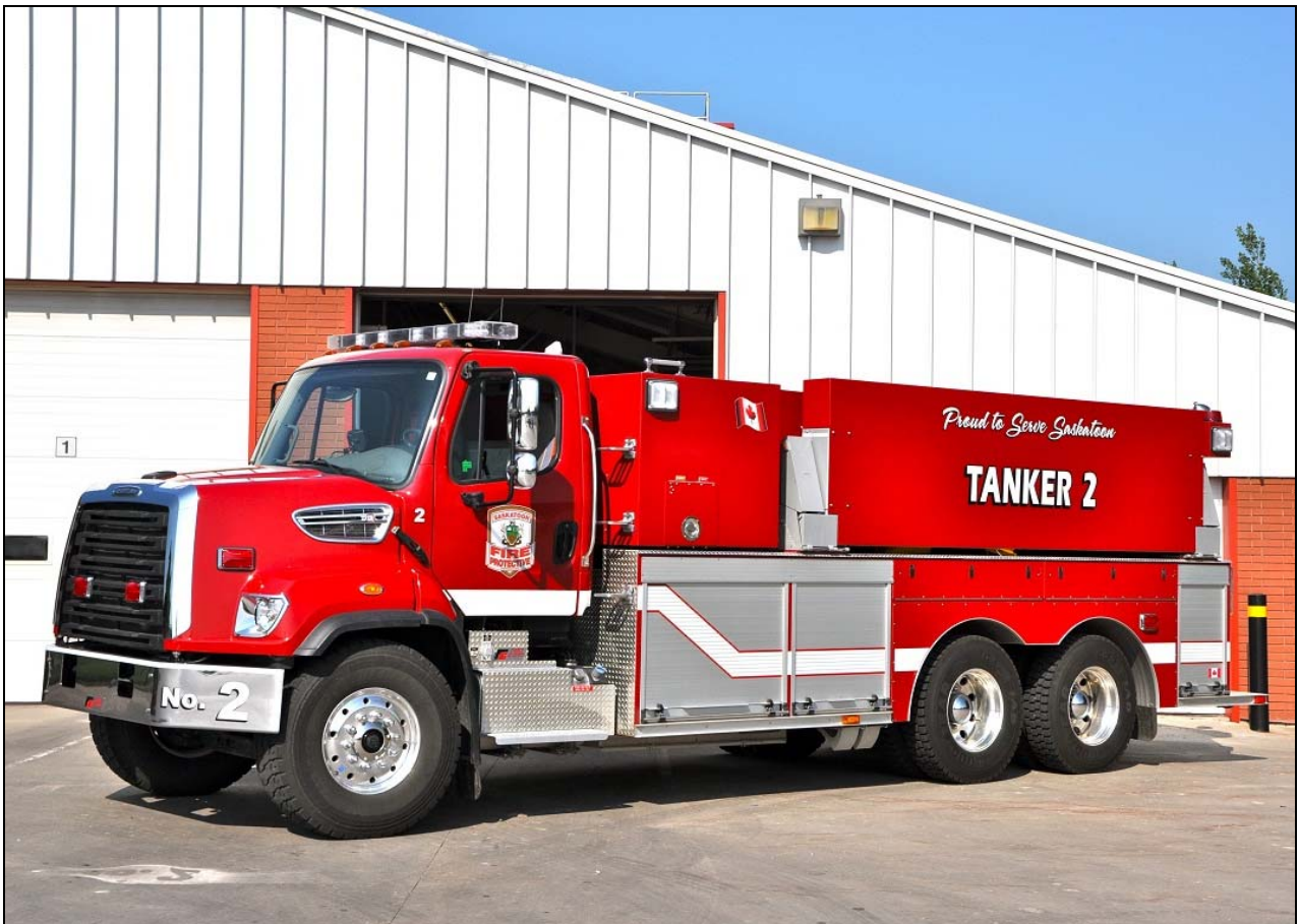
Tanker 2 is a 2013 Freightliner FL108SD Fort Garry rig with a 425igpm pump and 2500gwt.
