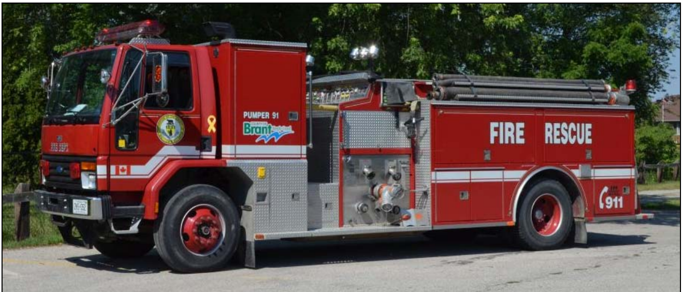
Another photo from the August tour: Brant County Pumper 91, a 1994 Ford CR8000/Almonte is now a spare, it has a 840igpm pump and 800gwt. SN#8717 (Bob Rupert photo)
