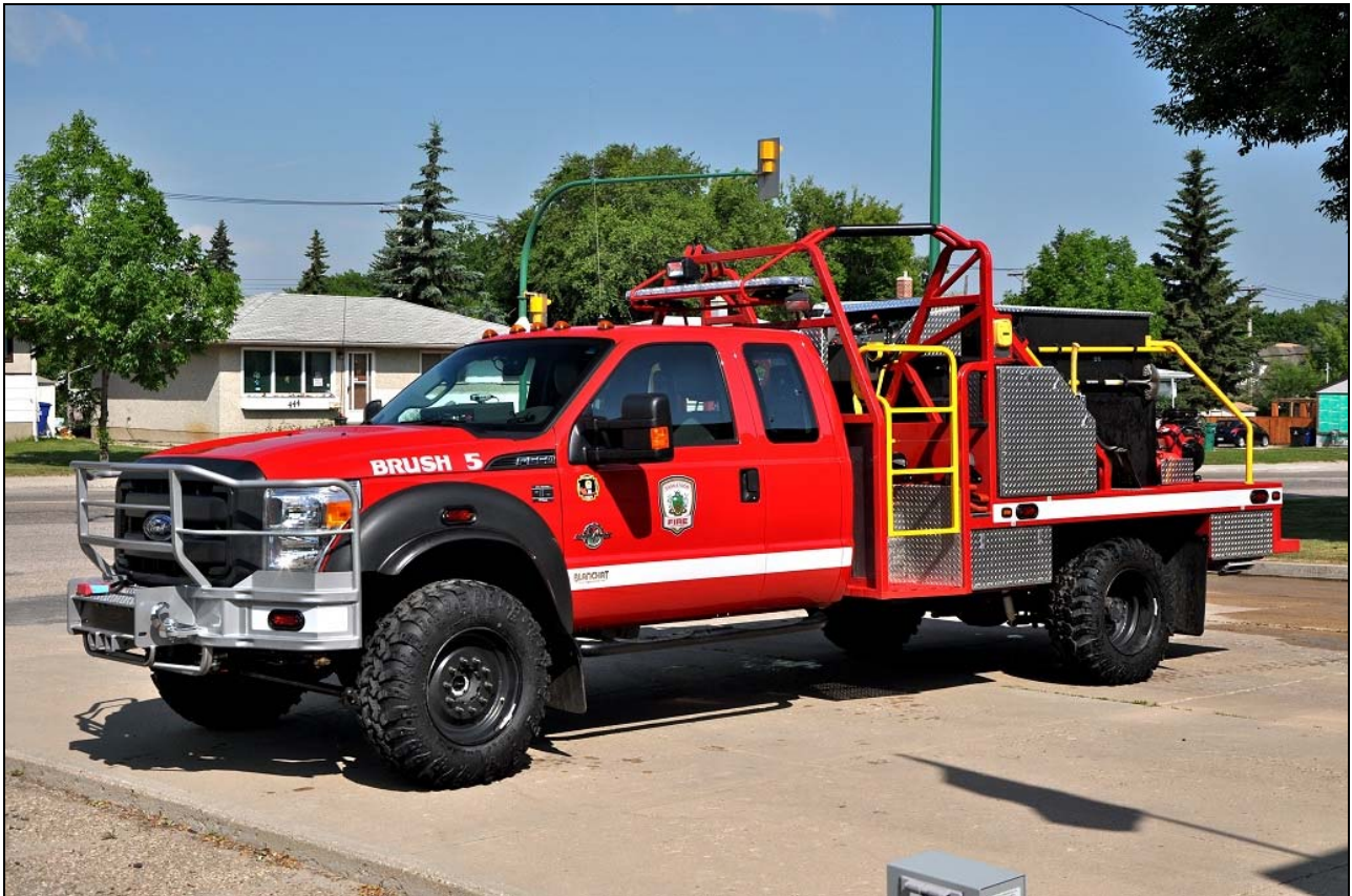
Saskatoon Brush 5, a 2013 Ford F 550 4x4 Blanchat unit has 150gpm, 500gwt and 10gft.
