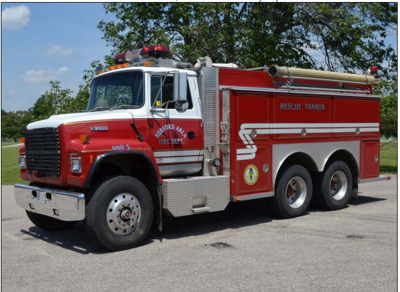
Another rig with a second home, Brant County Tanker 35, a 1993 Ford L8000 with a 1986 Superior body bought from Calgary, AB. It has a portable pump and a 2000 gwt. (Bob Rupert photos)
