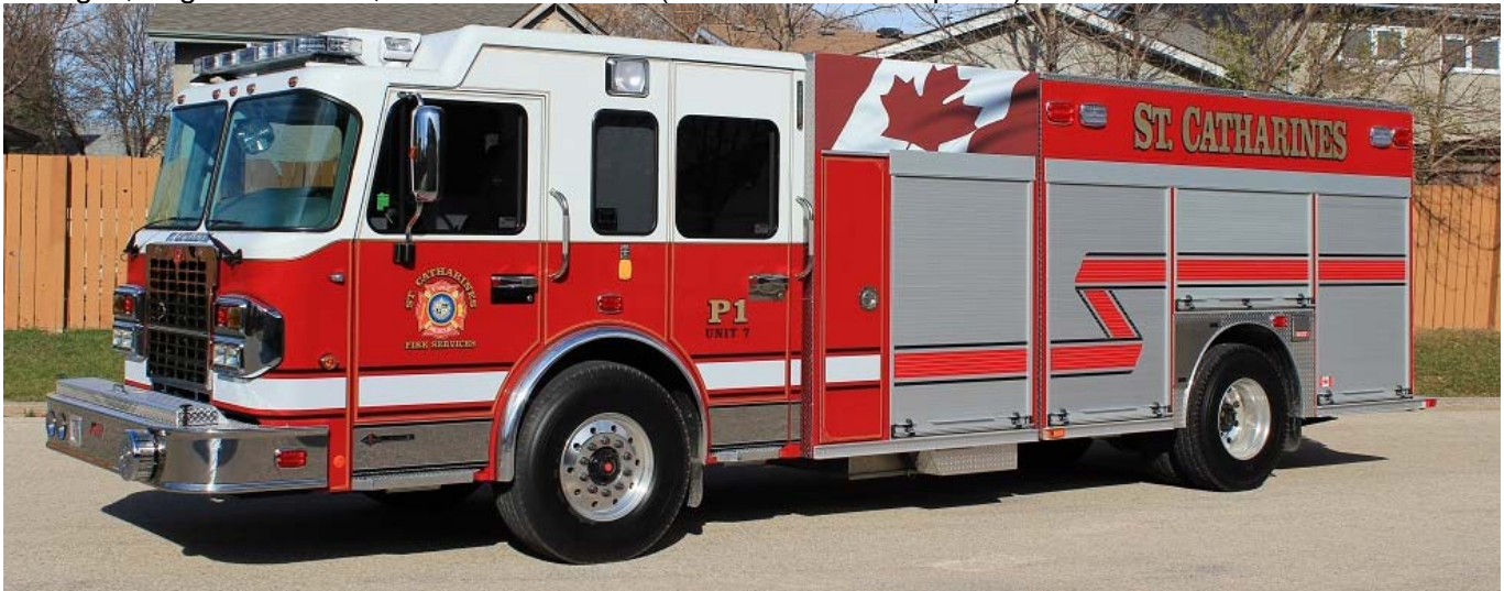
St. Catharines latest delivery, a 2014 Spartan Metro Star/Fort Garry pumper with a 1050igpm Waterous pump, 600gwt and 20gft, s/n M529. It is also equipped with a light tower. (Dave Stewardson photo)
