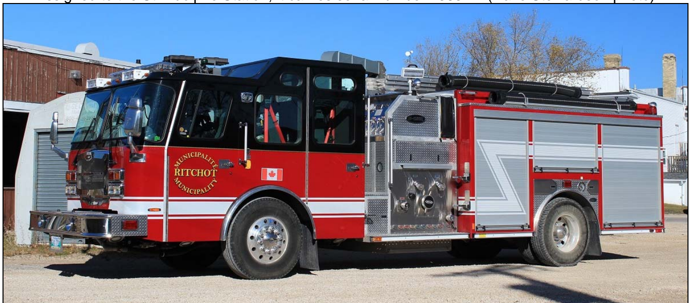
A couple of fairly recent examples, above is Minto, ON P.140, a 2011 Spartan Metro Star/Metalfab rig assigned to Clifford station. It has a 11250gpm pump and 600gwt. (Ian Duke photo). Richot, MB put this 2013 E-One Typhoon pump in service last December. It features a 1250gpm pump, 800gwt and 30gft. Assigned to the St. Adolphe Station, it carries serial number 138312. (Dave Stewardson photo)
