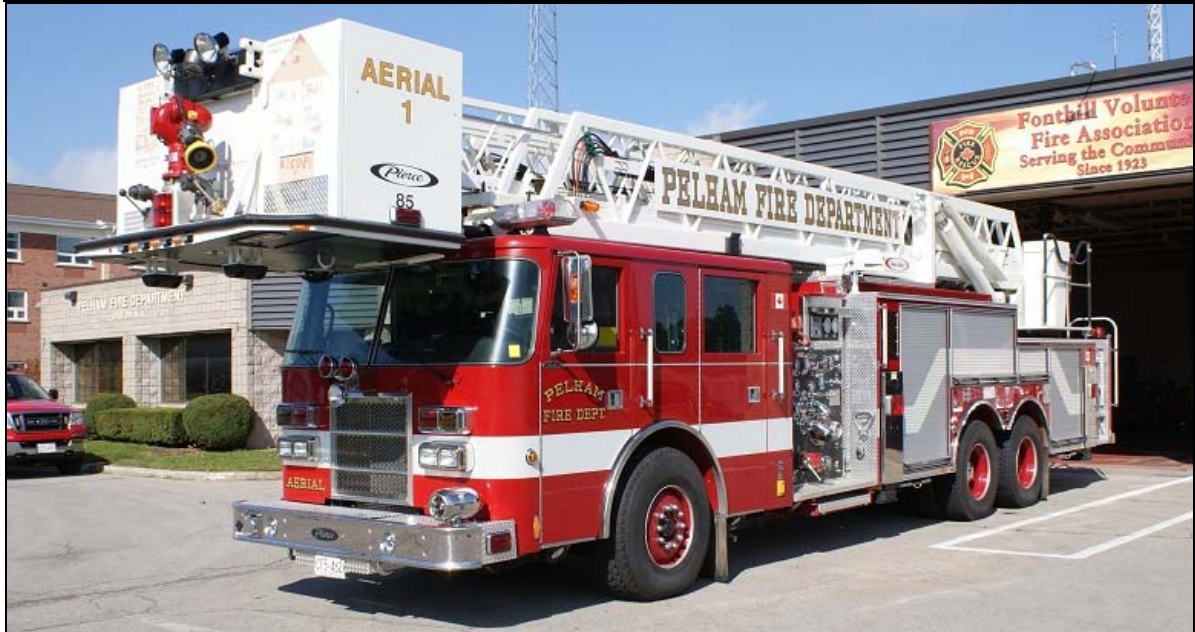
Another find with a Roto-Ray, Ken Buchanan passed on this shot of Pelham's Aerial 1, a 2001 Pierce Dash 85' tower with 1250gpm pump and 500gwt. It runs from Station 1, Fonthill. SN 12189.
