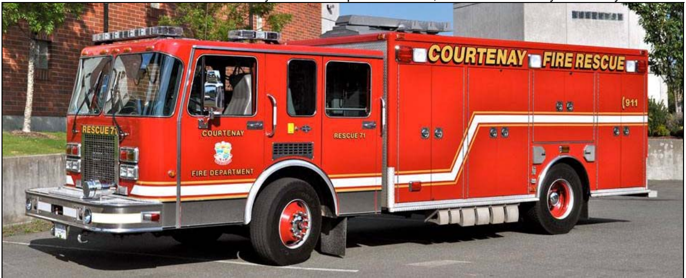
Courtenay, BC Tanker 14, a 2007 Freightliner M2-106/H Commercial Body 420igpm(H)/1700gwt, Rescue 71 is a 1992 American Fire & Rescue body on a 2013 Spartan chassis, conversion done by Fort Garry.
