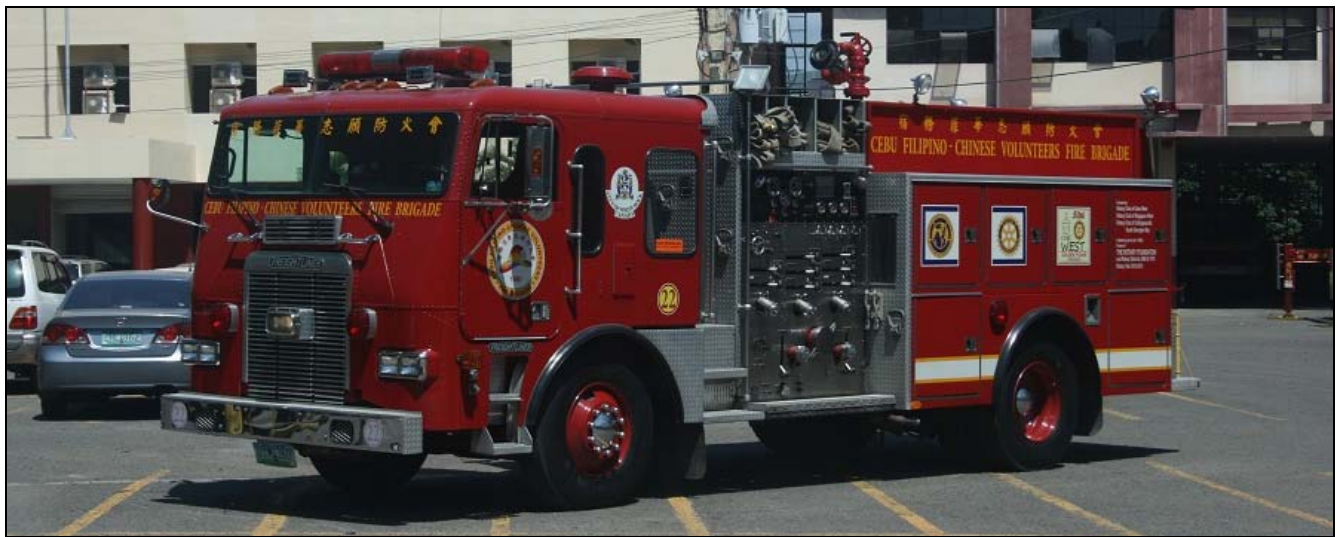
Three rigs from the Filipino-Chinese fire services in Cebu, Philippines. Engine 22 is a 1990 Freightliner FLL6302Anderson, 1500gpm/600gwt, S/N MS1250-171. (Photos and info from Bob Dubbert)
