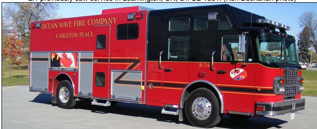
The first of two Eastway rigs bought by the Ocean Wave Fire Company in Carleton Place, ON was delivered in October. Rescue 240 is a walk-in squad recently built on a 2010 Spartan Gladiator chassis Eastway had on hand. It was originally a tri-axle but was shortened. (Ken Walton photo)
