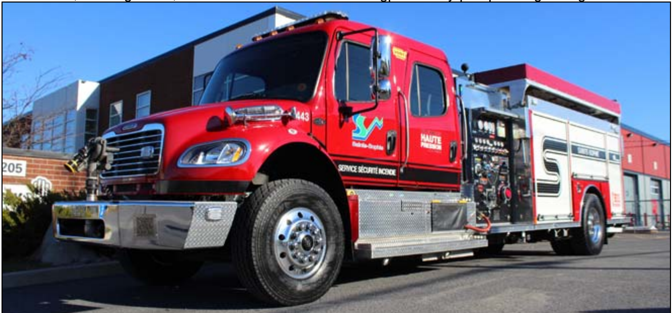
Sainte Sophie, QC just took delivery of this 2015 Freightliner M2-106/Rosenbauer pumper. Unité 443 has a 1050igpm Rosenbauer pump and a 1000gwt. (AeroFeu photo)
