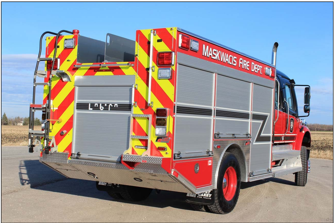
Additional views of Maskwacis Pump 51, a 2015 Freightliner M2-106 4x4/Fort Garry 1050/1000 rural pumper-tanker . The writing on the rear is Cree. The rig features pump & roll capability, and has a remote-controlled bumper turret. (Dave Stewardson photos)
