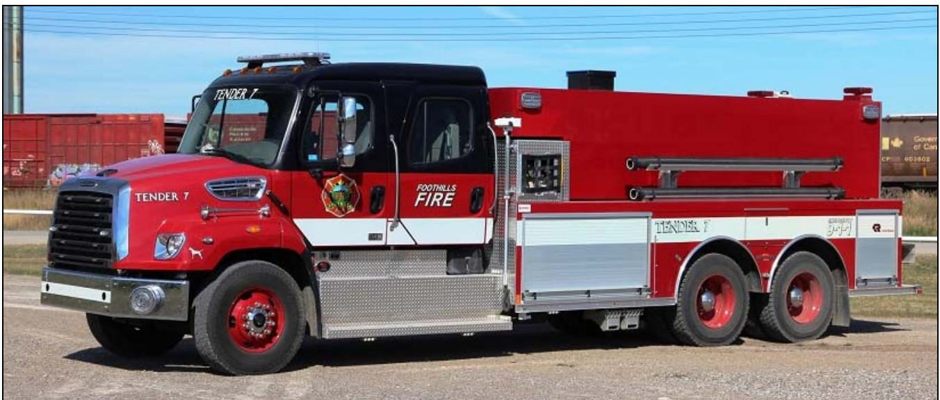
The MD of Foothills, AB recently placed this 2014 Freightliner 114SD/Rosenbauer tanker in service in Blackie as Tender 7. The long rig has a 633igpm pump and 2910gwt, with pump and roll. (#21450)
