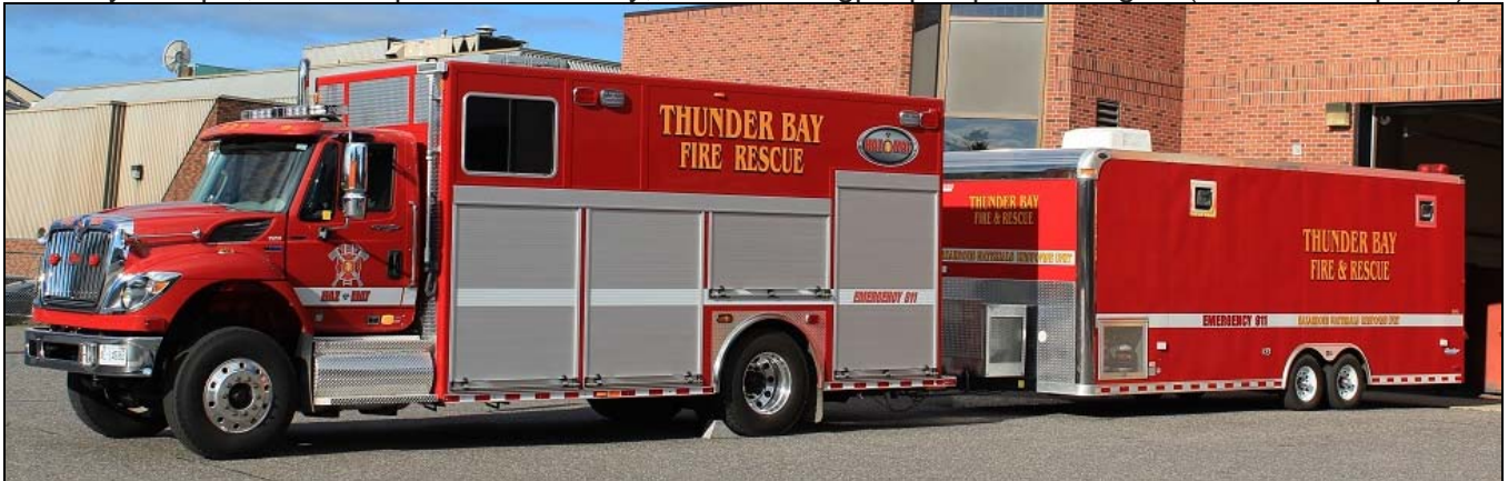
Thunder Bay Haz Mat 1, with trailer, is a 2013 International 7500/Carl Thibault rescue with a portable pump and 250gwt. (Dave Stewardson photos)
