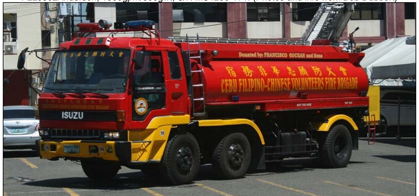
Engine 19 is a 2004 Isuzu L280 chassis 14,000L tanker from Japan, it uses a portable pump;
