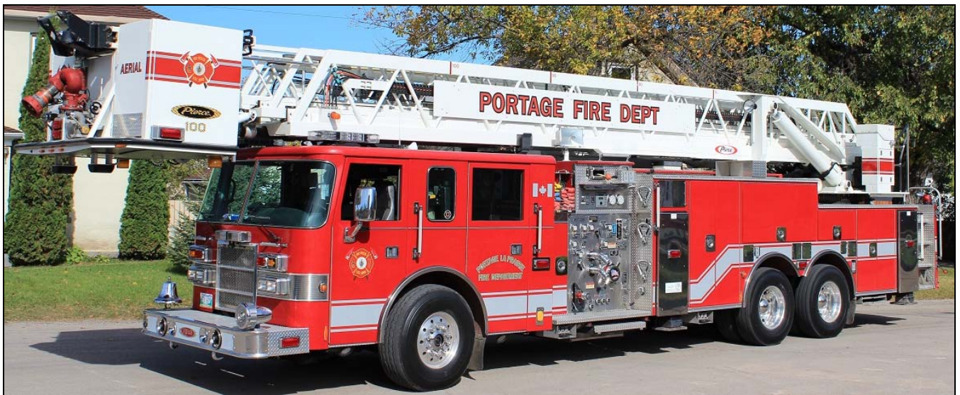
This 2000 Pierce Dash 100' tower formerly served with Bedford Park, IL. And was purchased by Portage la Prairie, MB. It's equipped with a 1750gpm pump and 2500gwt, and carries serial number 11749. It was rehabbed by Carriere Fire & Safety earlier in the summer with graphics applied by Acres. (Dave Stewardson photos)
