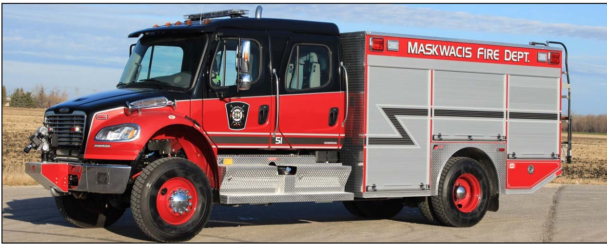
The Maskwacis F.D. protects the Samson Cree Nation in Alberta. They just took delivery of this 2015 Freightliner M2-106 4x4/Fort Garry rural pumper-tanker equipped with a 1050igpm Hale pump and 1000gwt. Unit 51 bears s/n M637. (Dave Stewardson photo)
