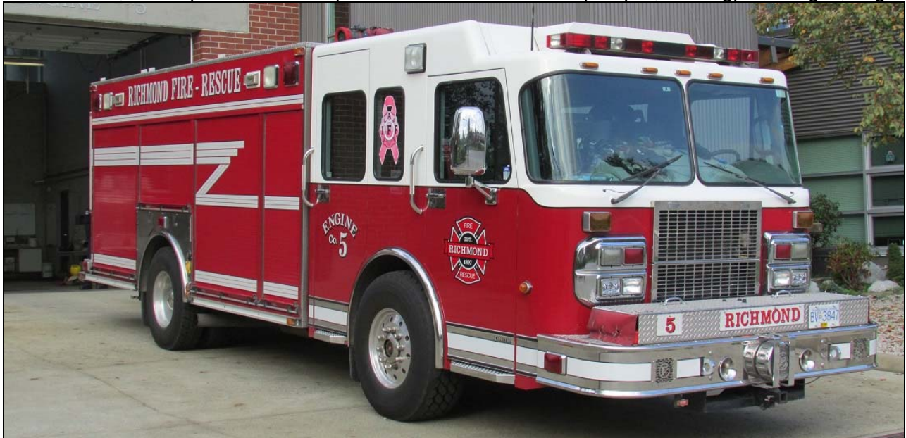
Richmond Engine 5 is a 2003 Spartan Gladiator/E-One 2100gpm, 500gwt, 30gft(A), 50gft(B).
