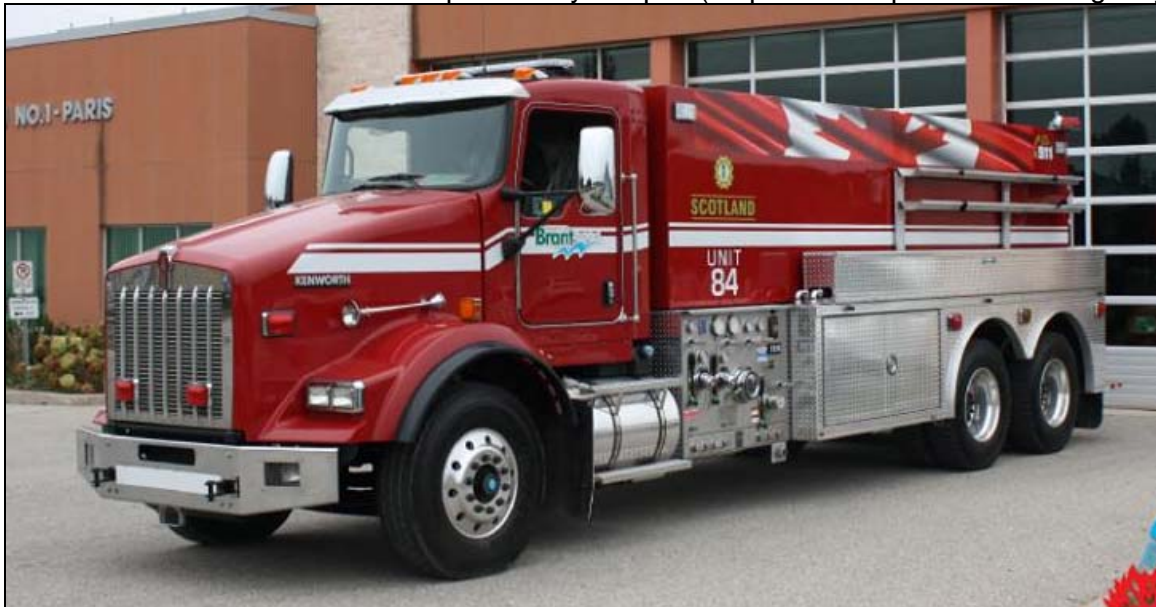
Brant County recently took delivery of this 2015 Kenworth/Dependable tanker. Unit 84 is stationed in Scotland and is equipped with a 750gpm pump and 3000gwt.
