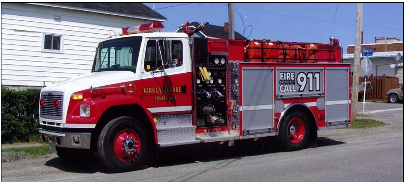
Kirkland Lake Pumper 3 is a 2003 Freightliner FL70/American LaFrance product, it is equipped with a 1050igpm pump and 800gwt, and carries SN#3604. (Gary Dinkel photos)
