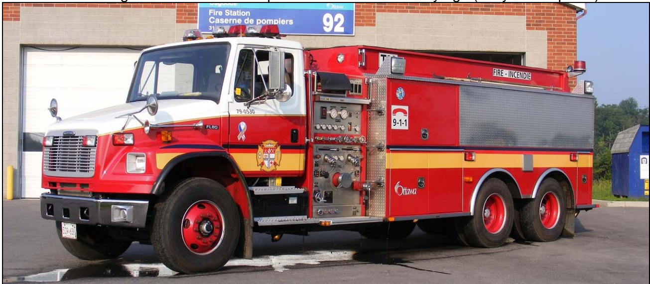
Ottawa Tanker 92, a 2004 Freightliner/Almonte pumper-tanker with a 1050igpm pump and 2500gtw.
