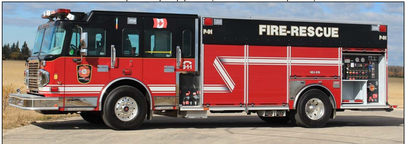
A look at the business end of OPG Pump 91, one of three Spartan/Fort Garry high capacity pumpers delivered to the plant. Each is equipped with a massive 2650igpm Darley pump so that the trio can be used to supplement the reactor cooling system in case of failure. Below is Pump 91 with its rear-position pump panel. (Dave Stewardson photos)
