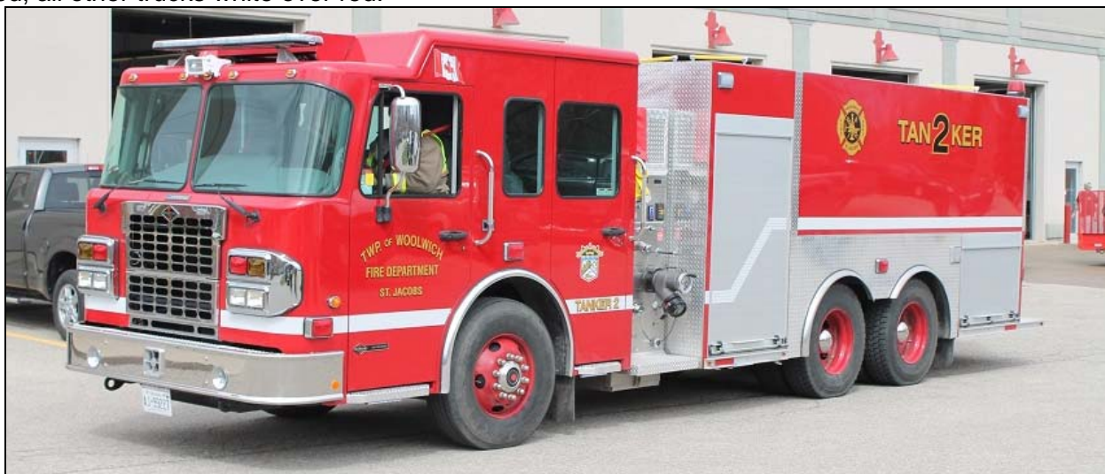
St. Jacob's Tanker 2, a 2015 Spartan Dependable, has a 500igpm pump and 2500gwt.
