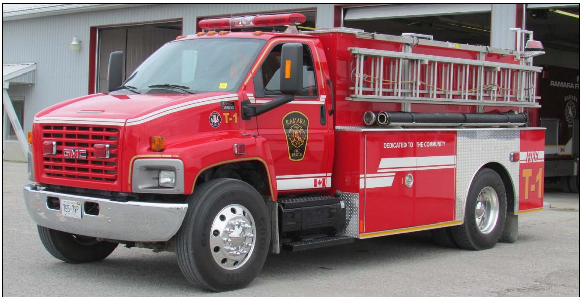
Ramara Tank 2, a 2007 GMC Top Kick/Asphodel 1500 gallon tanker with a portable pump.
