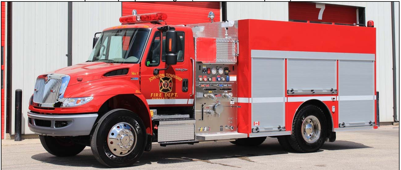
This IHC 4400/Fort Garry pumper was delivered to Johnson Township, ON in Algoma in 2012. It sports a 1050igpm pump, 1000gwt and 25gft. Assigned to the Desbarats station, it carries s/n M350
