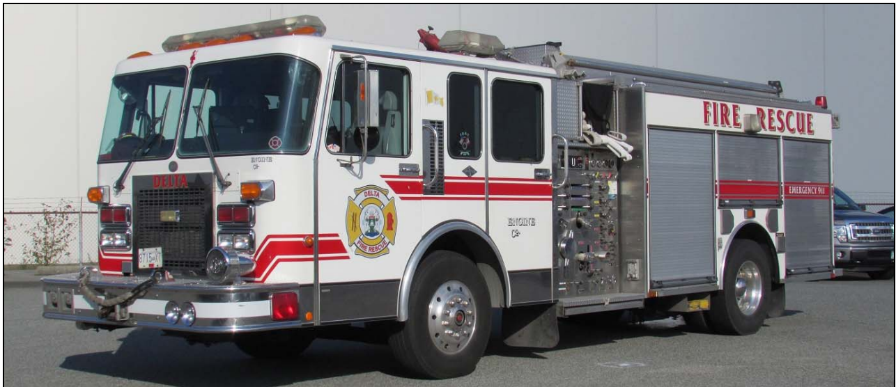
One of Delta, BC's spares, a 1994 Spartan Gladiator/Anderson pumper, 1750 igpm, 500gwt, 50gft.
