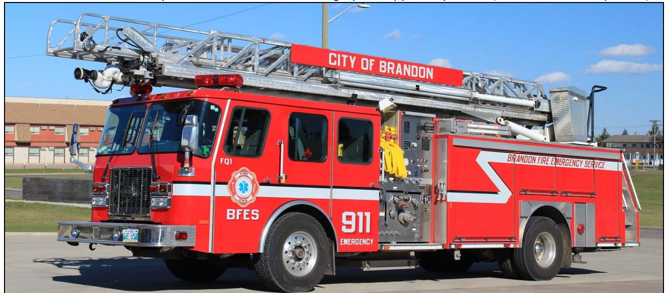
Brandon, MB acquired this 2001 E-One Cyclone II/Superior 75' quint, 1050igpm, 400gwt, 10gft(A), 25gft (B) back in 2012 from Fort Garry, who did the repaint. Serial Numbers SE2431 & 132831. Dauphin, MB T.12 is running a 2001 E-One Hurricane 2000gpm/250gwt/85' tower ex-Chicago Ridge, IL Serial Number 123706.
