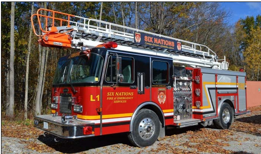
Six Nations F.D. recently purchased this 1994 Spartan/Superior quint from Darch Fire after a complete rehab and paint job. It has a 1050igpm Waterous pump, 400gwt and 50' Telesqurt. L.1 previously saw service in Leamington, ON, s/n SE 1381. (Ken Buchanan photo)
