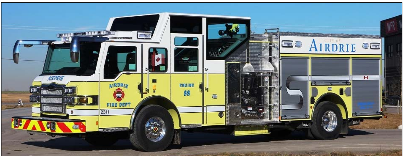
Airdrie, AB recently replaced Engine 88 with this 2016 Pierce Velocity pumper. It has a 1500gpm pump, 500gwt and 30gft. Serial number 28730. (John Bowerman photos)
