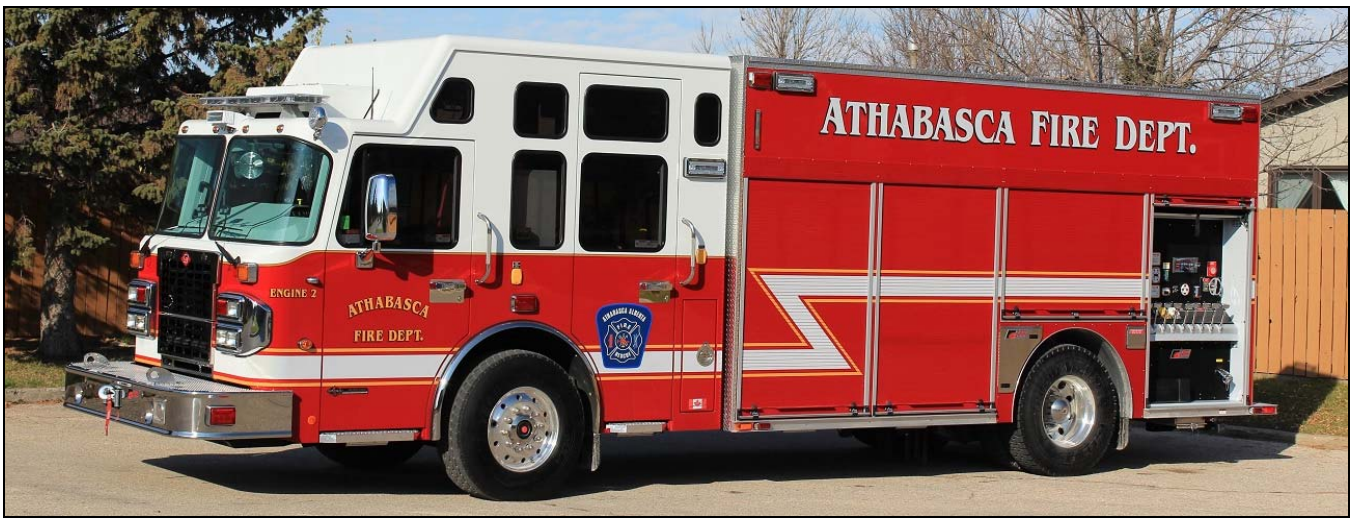
Athabasca, AB now has a 2015 Spartan Metro Star/Fort Garry rearmount pumper at Engine 2. It has a 1050igpm Hale pump, 500gwt and 25gft, and serial number M621. (Dave Stewardson photo)
