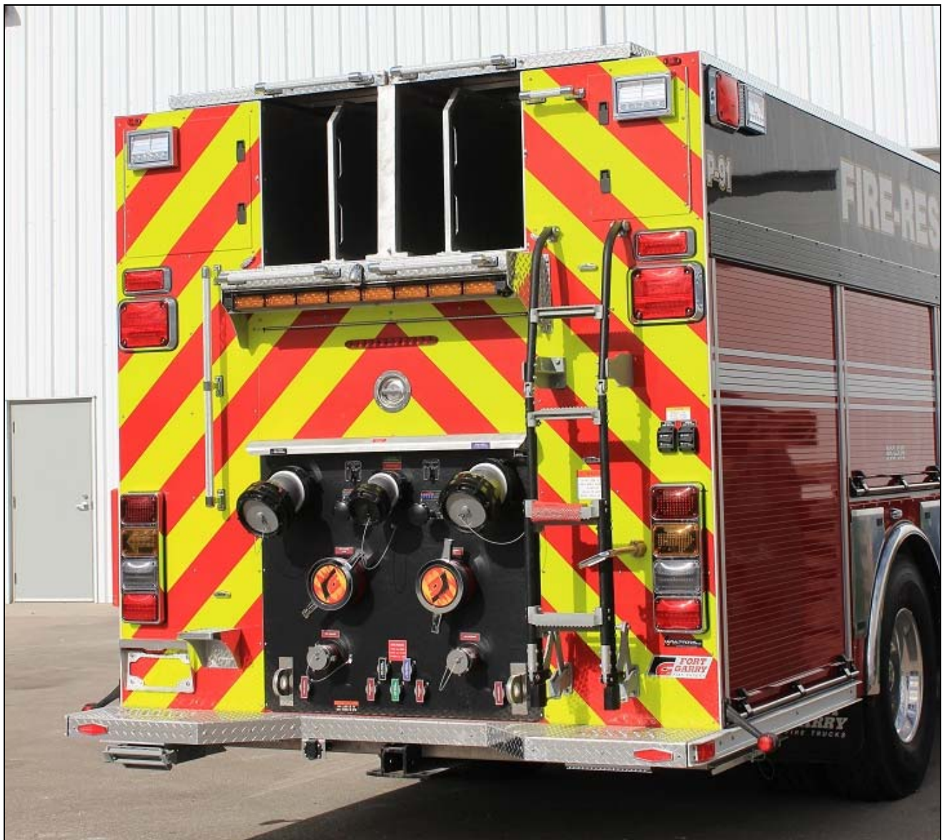
A look at the business end of OPG Pump 91, one of three Spartan/Fort Garry high capacity pumpers delivered to the plant. Each is equipped with a massive 2650igpm Darley pump so that the trio can be used to supplement the reactor cooling system in case of failure. Below is Pump 91 with its rear-position pump panel. (Dave Stewardson photos)
