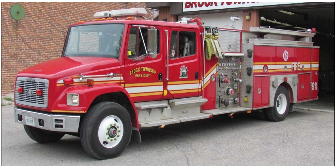
Pumper 82, a 2000 Freightliner FL80/Advance Engineering pumper, 840igpm/830gwt.
