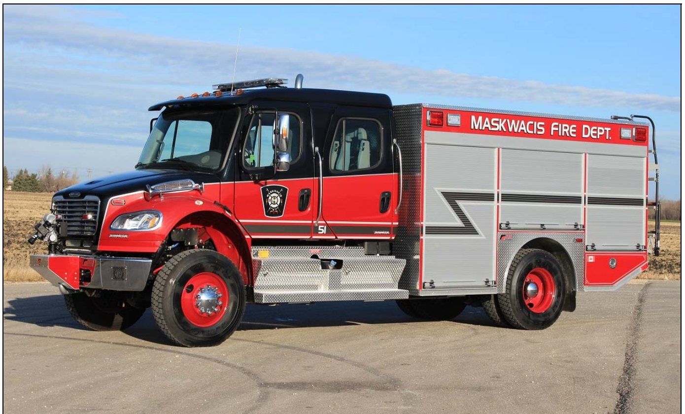
Additional views of Maskwacis Pump 51, a 2015 Freightliner M2-106 4x4/Fort Garry 1050/1000 rural pumper-tanker . The writing on the rear is Cree. The rig features pump & roll capability, and has a remote-controlled bumper turret. (Dave Stewardson photos)
