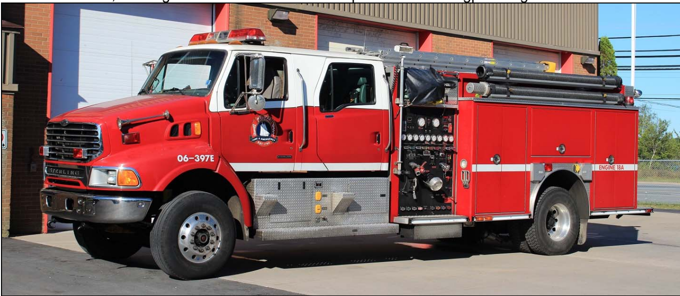
Halifax, NS E.18A: 2006 Sterling L9500/Superior 1750igpm/750gwt/30gft #SE3653
