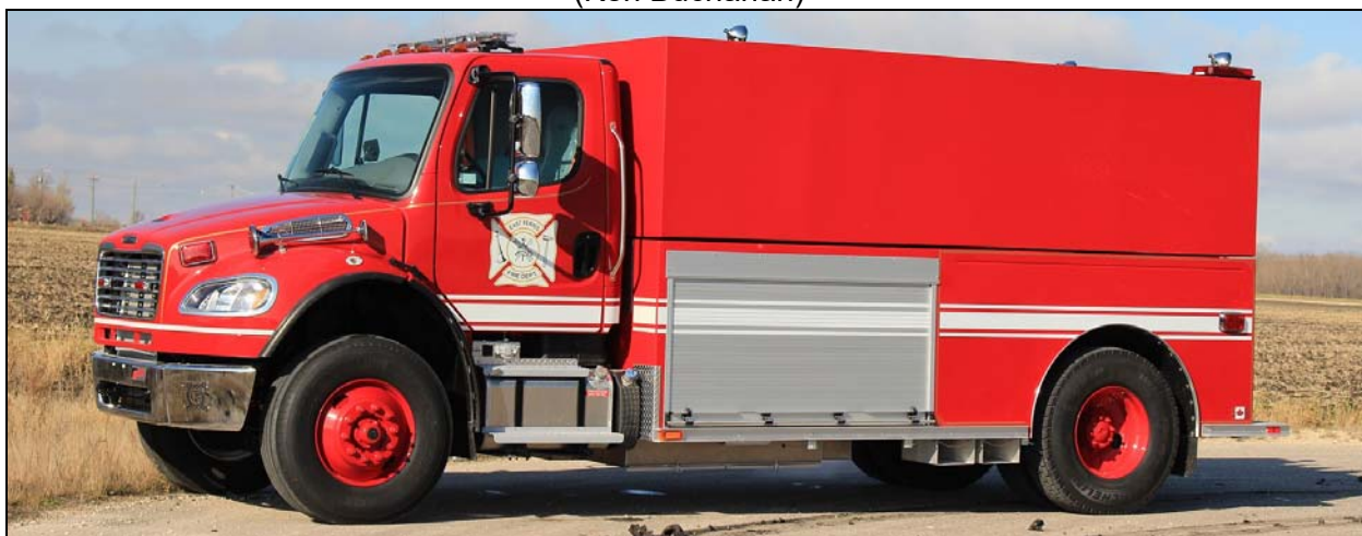
East Ferris, ON 2016 Freightliner M2-106/Fort Garry 420igpm(D)/1700gwt s/n M712 (Dave Stewardson photo)
