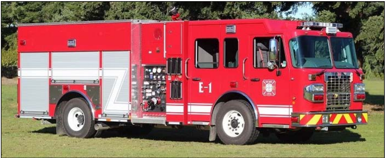
East Sooke, BC Engine 1 received this 2016 Spartan Metro Star/Smeal pumper earlier this year, it has a 2250igpm pump, /900gwt, 50gft and a FoamPro 2001foam system, sn 4468 (Shane MacKichan photo).
