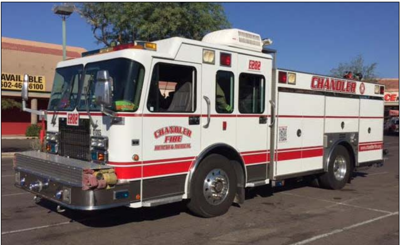
Chandler, AZ Engine 282 has a 2001 Salisbury pump on a Spartan Metro Star chassis with a 1250gpm pump and 500gwt. (Tom Sheppard photos)
