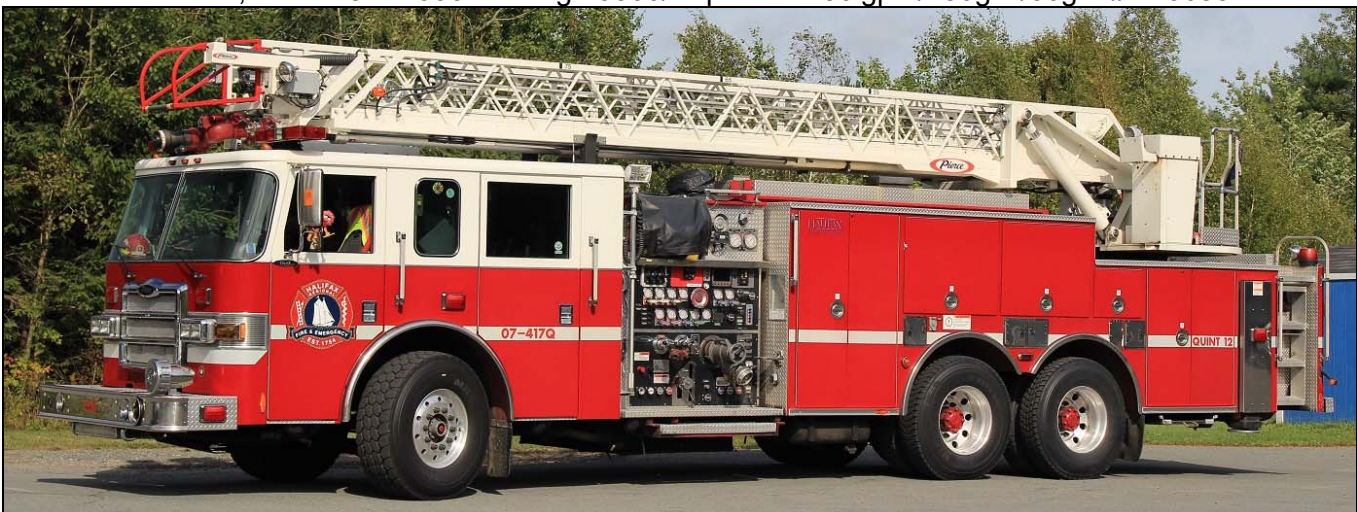
Halifax, NS Q. 9: 2007 Pierce Dash, 1750igpm/500gwt/75' aerial. s/n19430. (Dave Stewardson photos)
