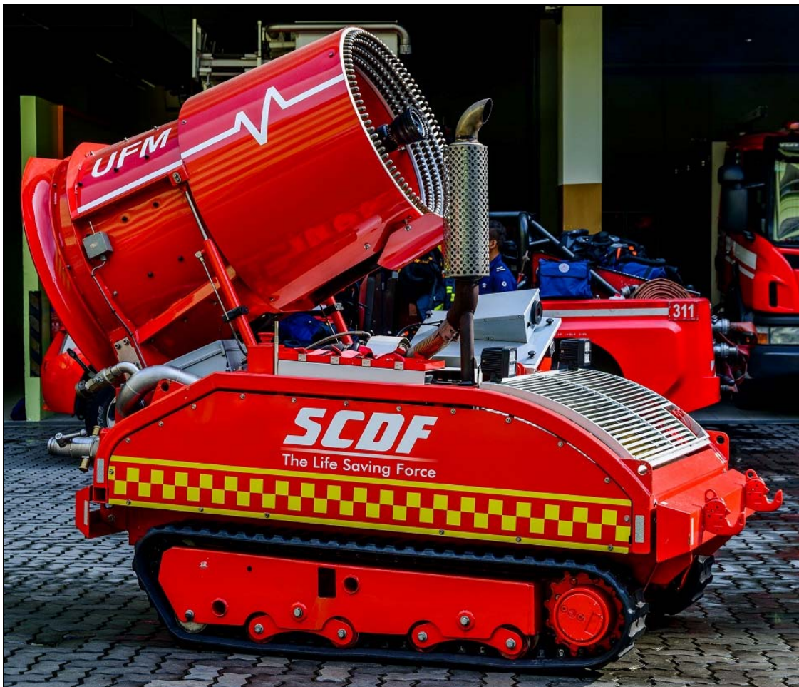
Part of the fleet in Singapore; one of four remote fire-fighting vehicles (unmanned fire-fighting machine or UFM) built in Austria by Rechner. Delivered in 2014, the LUF-Mobiles are equipped with a large fan and nozzle, they can dispense water or foam and are camera equipped. They are carried on the Hino 300 trucks, below or on custom designed rail cars for use in tunnels. (Kenneth Lai photos)
