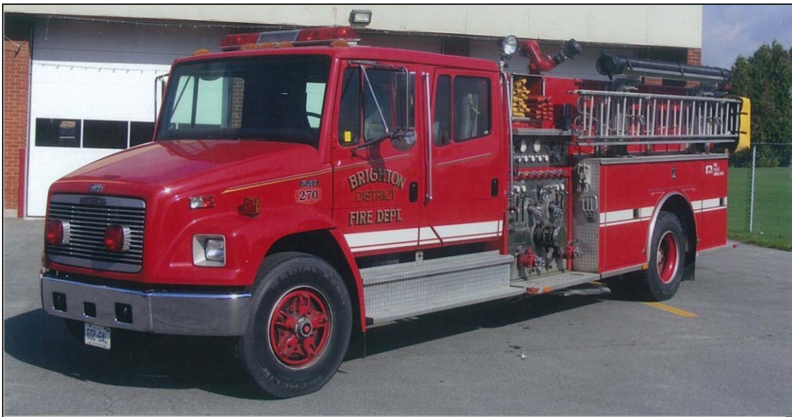
Unit 270, a 1995 Freightliner FL80/Almonte 1050igpm/500gwt, S#9944
