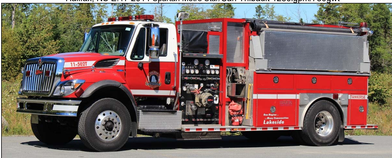
Halifax, NS Tanker 58: 2010 IHC 7500/Carl Thibault 1050igpm/1400gwt.
