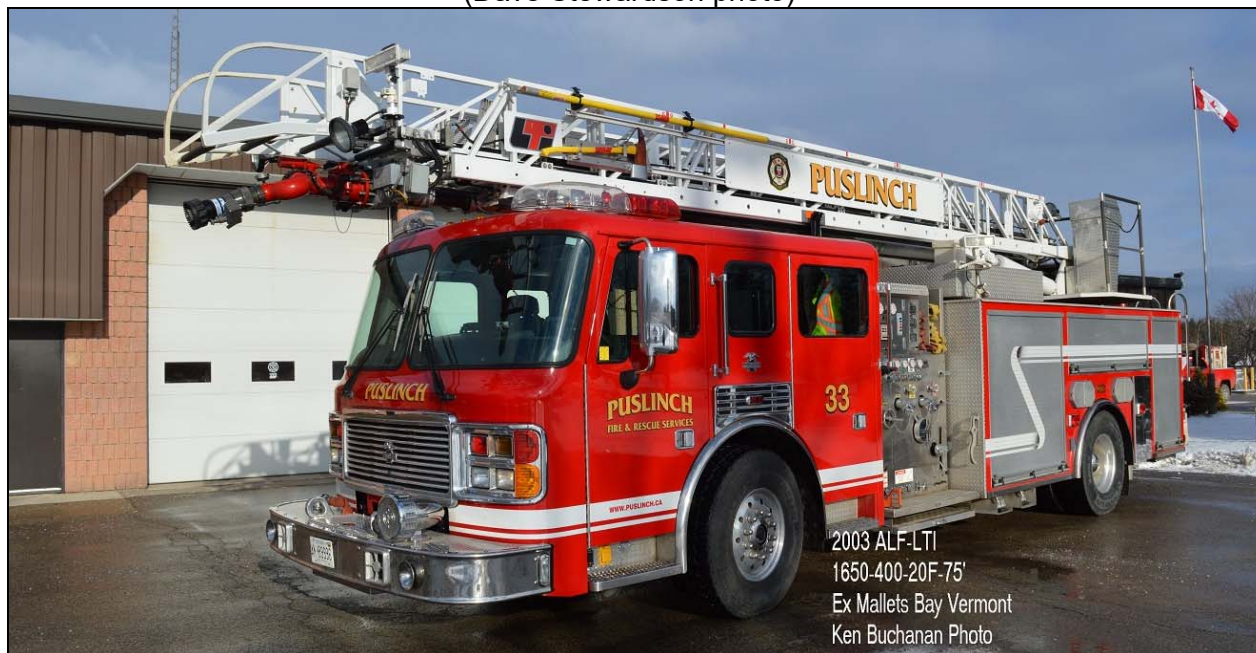
Formerly with Mallets Bay, VT, this 2003 ALF/LTI quint just went in service in Puslinch. U.33 has a 1650igpm pump, 400gwt, 20gft and 75' aerial. (Ken Buchanan photos)
