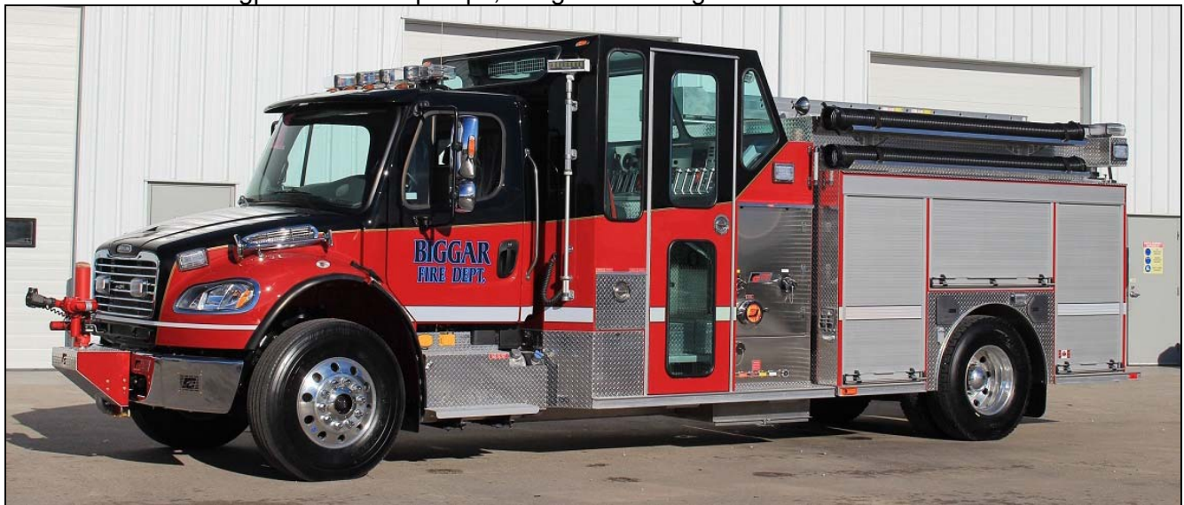
Biggar, SK now has this 2016 Freightliner M2-106/Fort Garry rig, with a 1050igpm Darley pump, 1000gwt and a 25gft. s/n M752 (Dave Stewardson photos)
