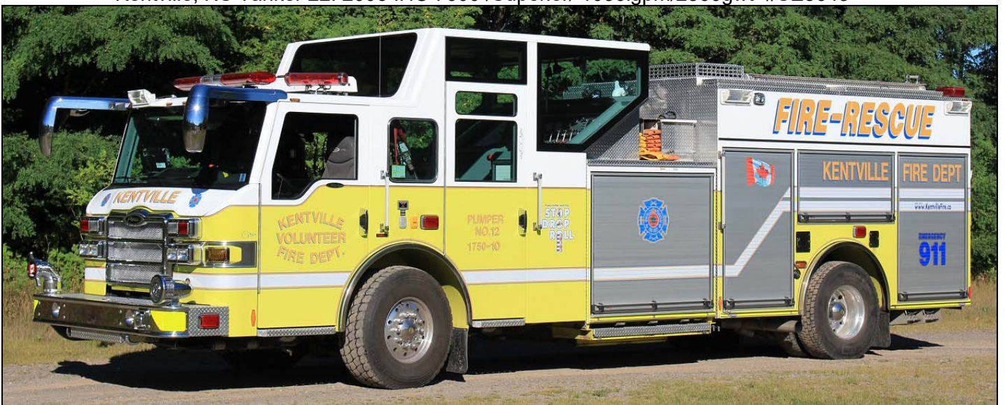
Kentville, NS Engine 12 is a 2010 Pierce Velocity 1750igpm/1000gwt. (Dave Stewardson photos)
