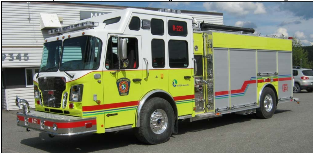
Last year, Rouyn-Noranda, QC 2015 Spartan Metro Star/ Maxi Métal rescue pump. Unité 221 has a 1500gpm pump, 1830gwt, 20gft(A) and 50gft(B) with a CAFS (Maxi Métal photos)
