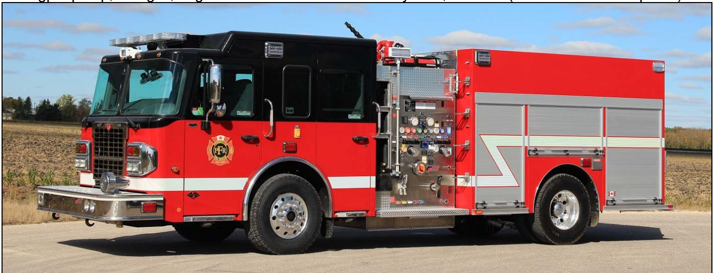
Pemberton, BC recently got this 2016 Spartan Gladiator/Fort Garry pumper. It has a 1250igpm Hale pump, 900gwt and 25gft. sn M734 (Dave Stewardson photos).
