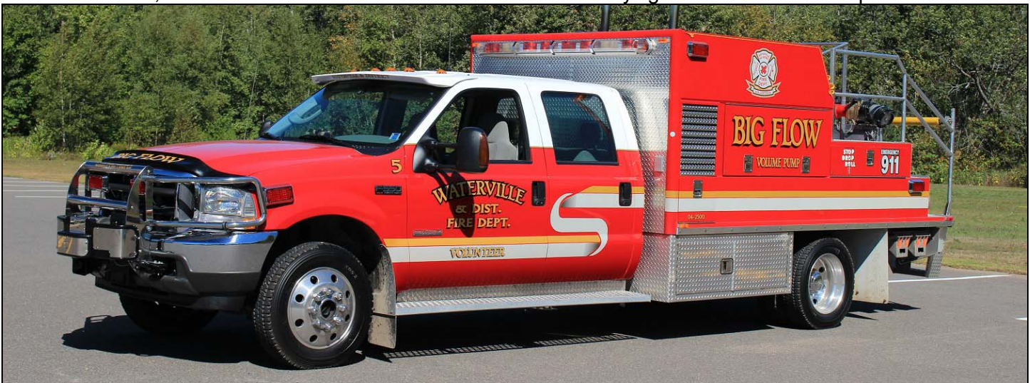
Waterville, NS Unit 51 is a 2004 Ford F550/Lantz Truck Body with a 2500 igpm pump.
