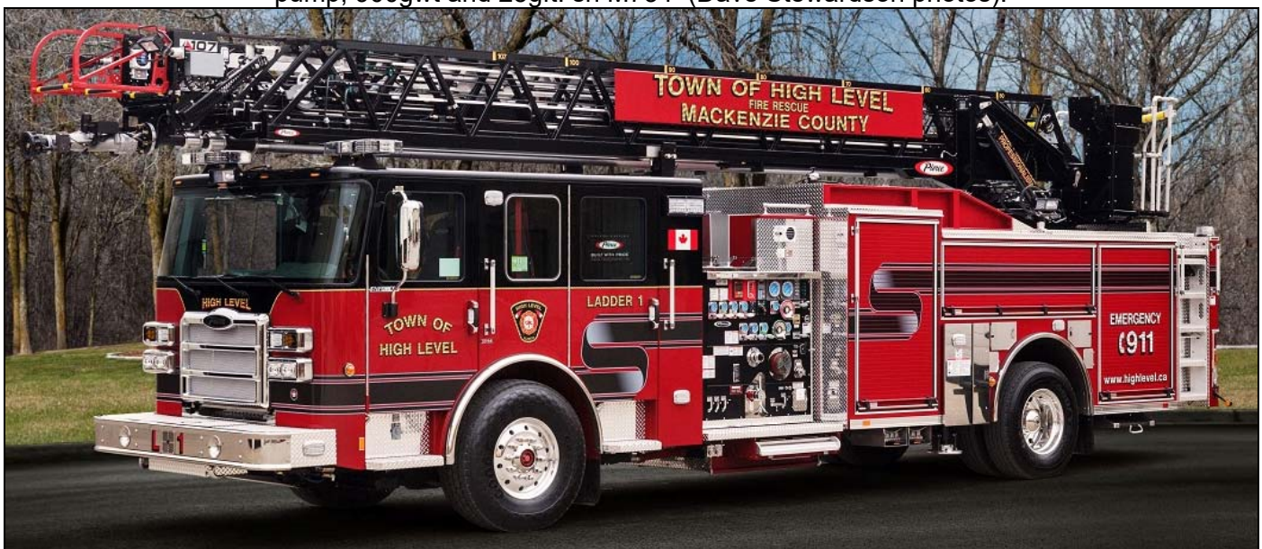
Another delivery from earlier this year, High Level, AB Ladder 1 is a 2016 Pierce Ascendant quint with a 1500gpm pump, 500gwt and 107' aerial. (Pierce Fire photo).
