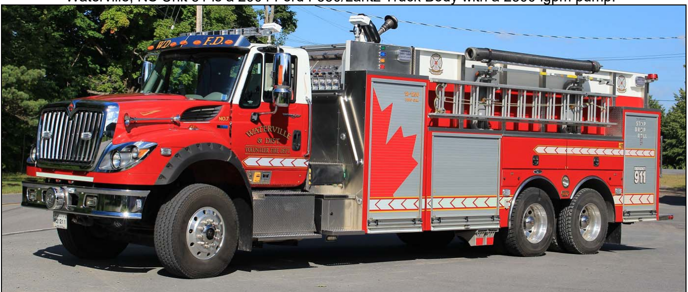
Tanker 21 of the Woodville station of Waterville, NS. An unusual builder for Canada, a 4 Guys tanker on a 2012 IHC 7600 chassis. It has a 1050igpm pump and 2500gwt. (Dave Stewardson photos)
