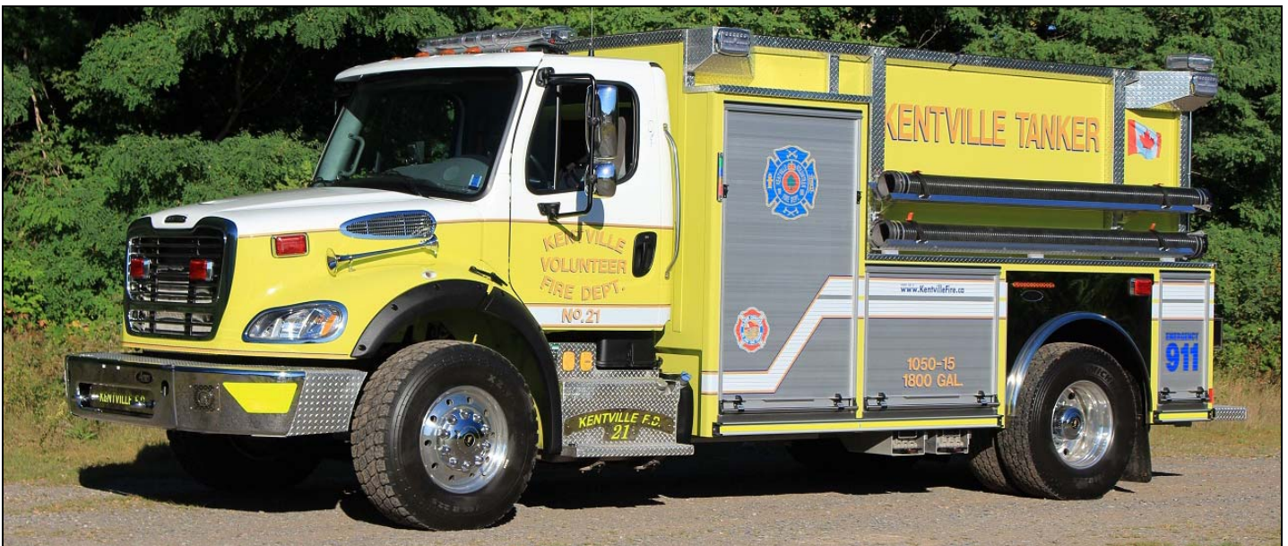
Kentville, NS Tanker 21: 2015 Freightliner M2-112/Acres, 1050igpm/1800gwt.
