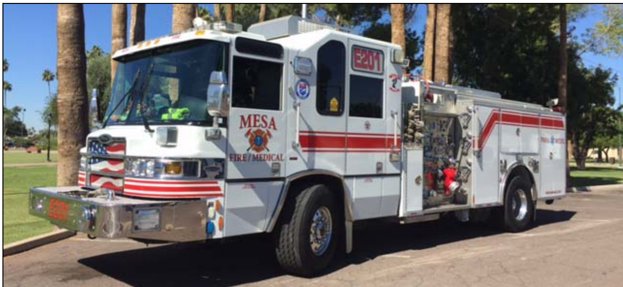
Mesa, AZ Engine 201, a 2009 Pierce Quantum 1250gpm/500gwt.
