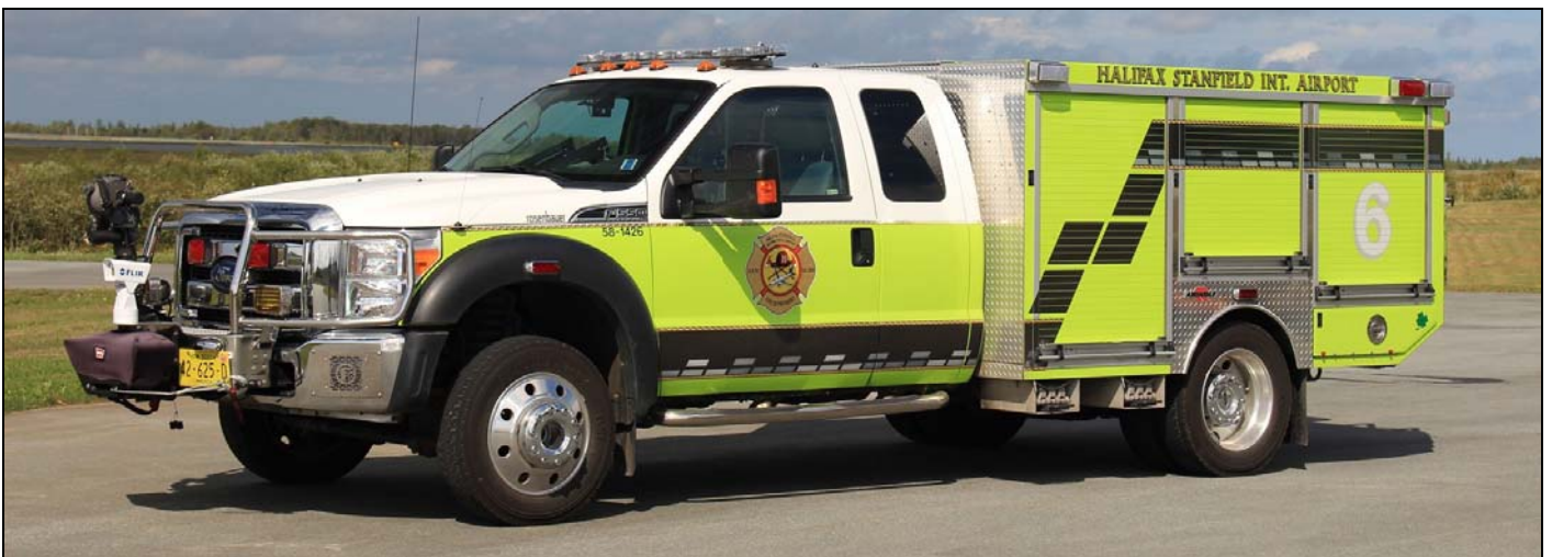
Halifax (YHZ) Red 6 2014: Ford F550/Rosenbauer 210igpm/250gwt/33gft/500# PK (Dave Stewardson photos)
