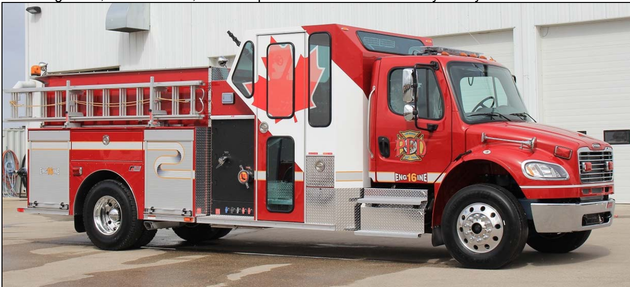
Ponoka, AB Engine 16 is a 2016 Freightliner M2/Fort Garry pump. Equipped with a 1050igpm Hale pump, 1000gwt and 25gft. It also has a FoamPro 100 foam system. s/n M707
