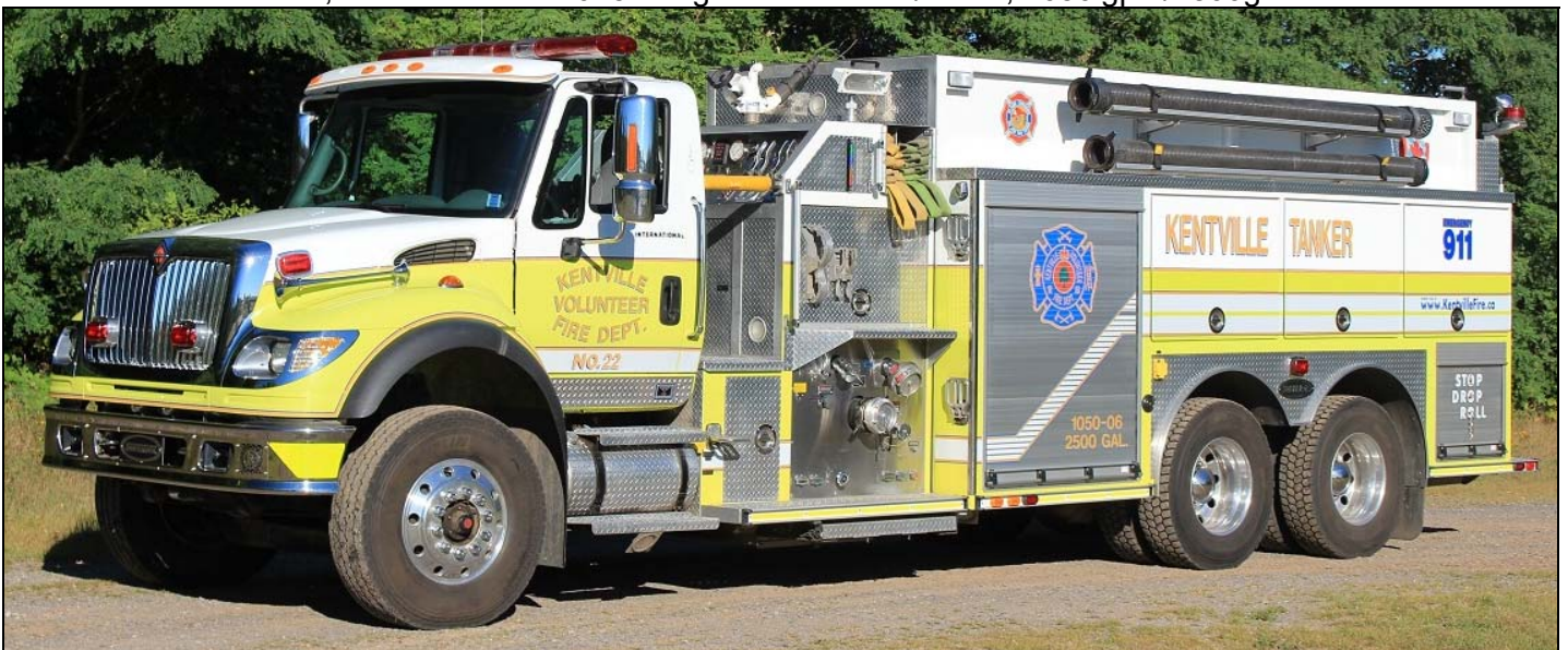
Kentville, NS Tanker 22: 2006 IHC 7600 /Superior/ 1050igpm/2500gwt #SE3648
