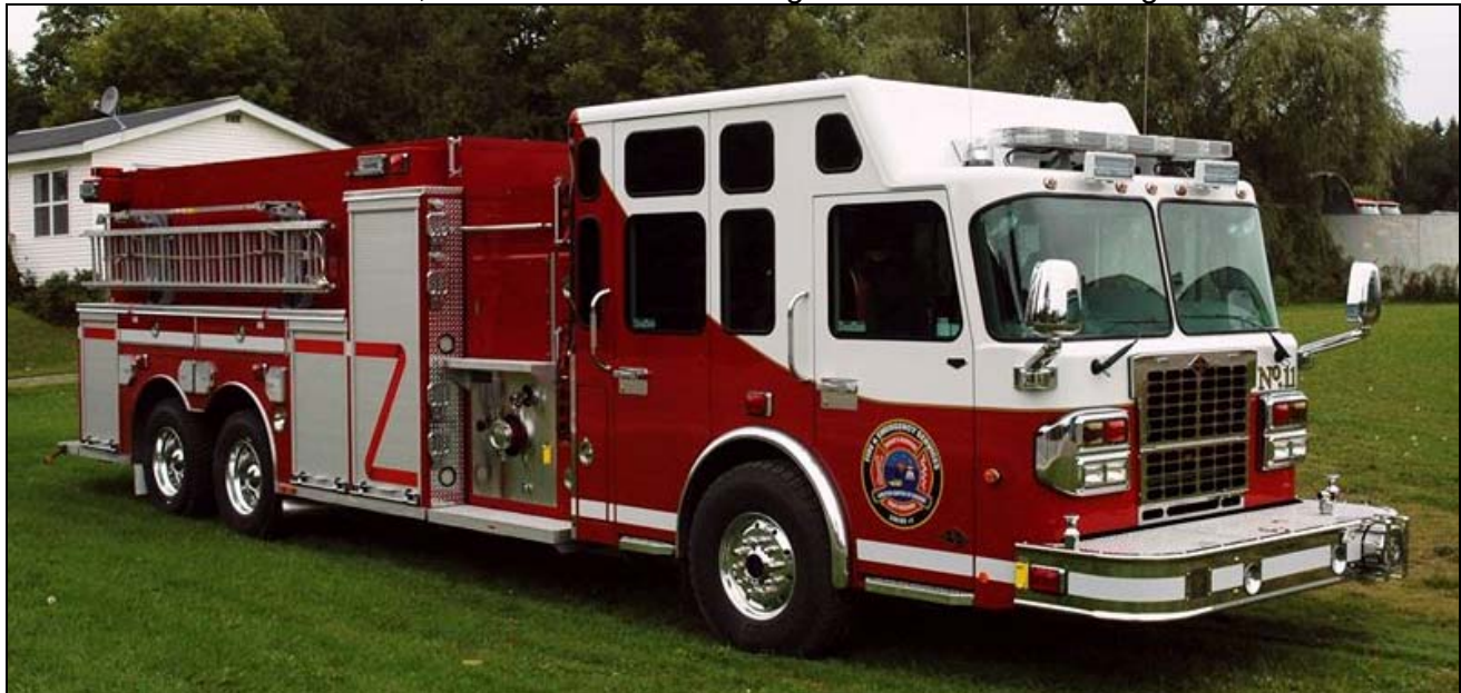
Woods Harbour, Shag Harbour, NS Unit 11, a Spartan Metro Star/Metalfab 1250igpm/2500gwt (MFT)
