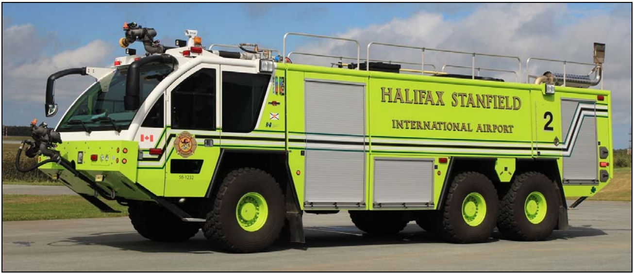
Halifax (YHZ) Red 2: 2012 Rosenbauer Panther 1540igpm/2500gwt/333gft/500# PK
