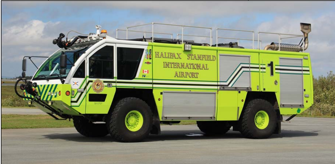
Halifax (YHZ) Red 1: 2007 Rosenbauer Panther 1540igpm/1250gwt/167gft/500# PK.
