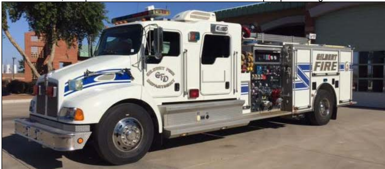
A Reserve Engine for Gilbert, a 2001 Pierce/Kenworth unit, 1500gpm/500gwt.
