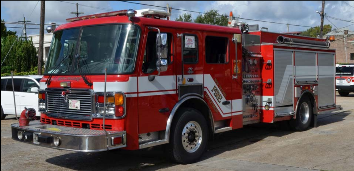
Engine 29 is a 2006 American Lafrance Eagle/Becker, 1250gpm pump/500gwt, S#1827.
