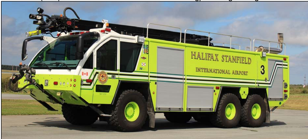
Halifax (YHZ) Red 3: 2012 Rosenbauer Panther 1540igpm/2500gwt/333gft/500# PK/54' HRET.
