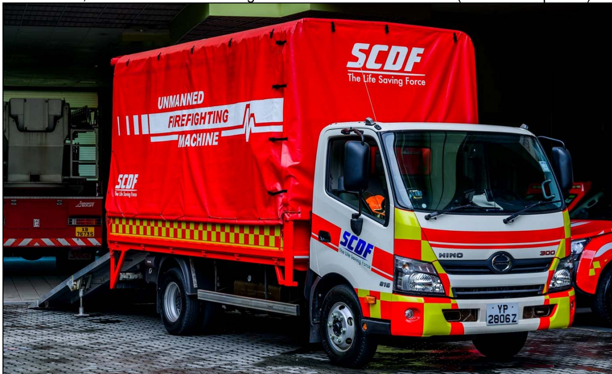
Part of the fleet in Singapore; one of four remote fire-fighting vehicles (unmanned fire-fighting machine or UFM) built in Austria by Rechner. Delivered in 2014, the LUF-Mobiles are equipped with a large fan and nozzle, they can dispense water or foam and are camera equipped. They are carried on the Hino 300 trucks, below or on custom designed rail cars for use in tunnels. (Kenneth Lai photos)
