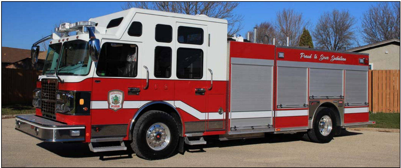
Saskatoon, SK just bought two of these 2016 Spartan Metro Star/Fort Garry engines. They have 1500igpm Waterous pumps, 600gwts and 25gfts. This one has s/n M757
