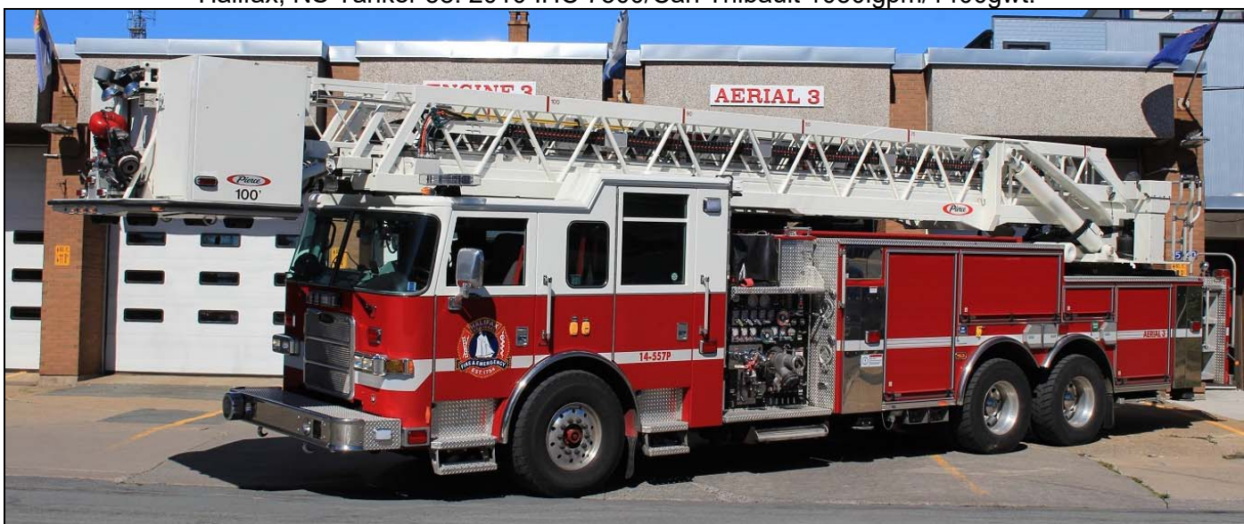
Halifax, NS Ladder 3: 2014 Pierce Arrow XT 1750igpm/300gwt/100' s/n 26852 (Dave Stewardson photos)
