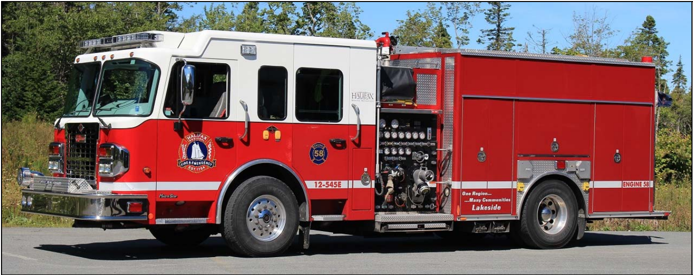
Halifax, NS Engine.58: 2012 Carl Thibault/Spartan MS 1250igpm/750gwt S#605070.
