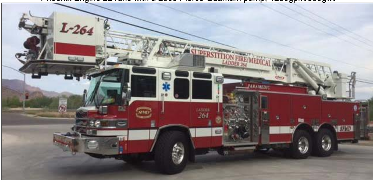
Superstition Medical/Fire Department Ladder 264, a 2013 Pierce Quantum 1250/350/85'
