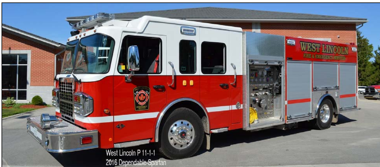
West Lincoln P.1 2016 Spartan Metro Star/Spartan ERV/Dependable 1500gpm/1000gwt (Ken Buchanan)
