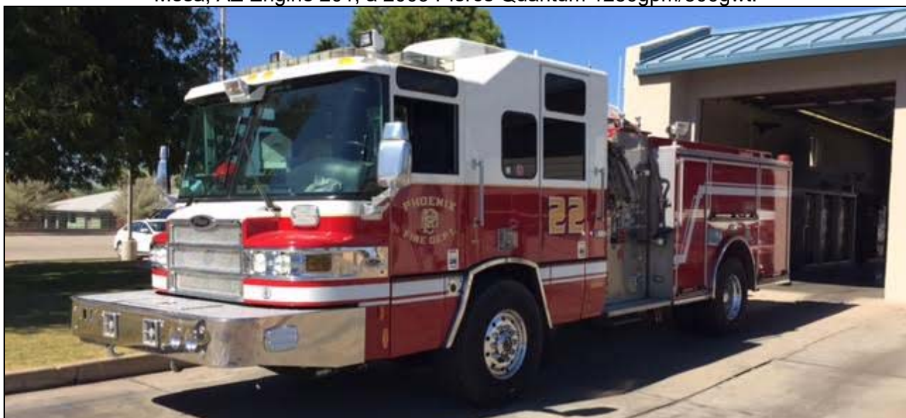
Phoenix Engine 22 runs with a 2009 Pierce Quantum pump, 1250gpm/500gwt
