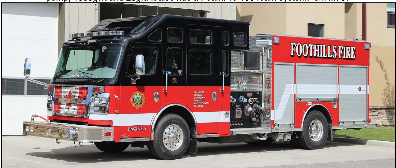
Foothills, AB recently got this 2016 Rosenbauer Commander product for Engine 9 in De Winton with a 1250gpm pump, 750gwt, 20gft and FoamPro 2001 foam system. s/n 25501 (Dave Stewardson photos)
