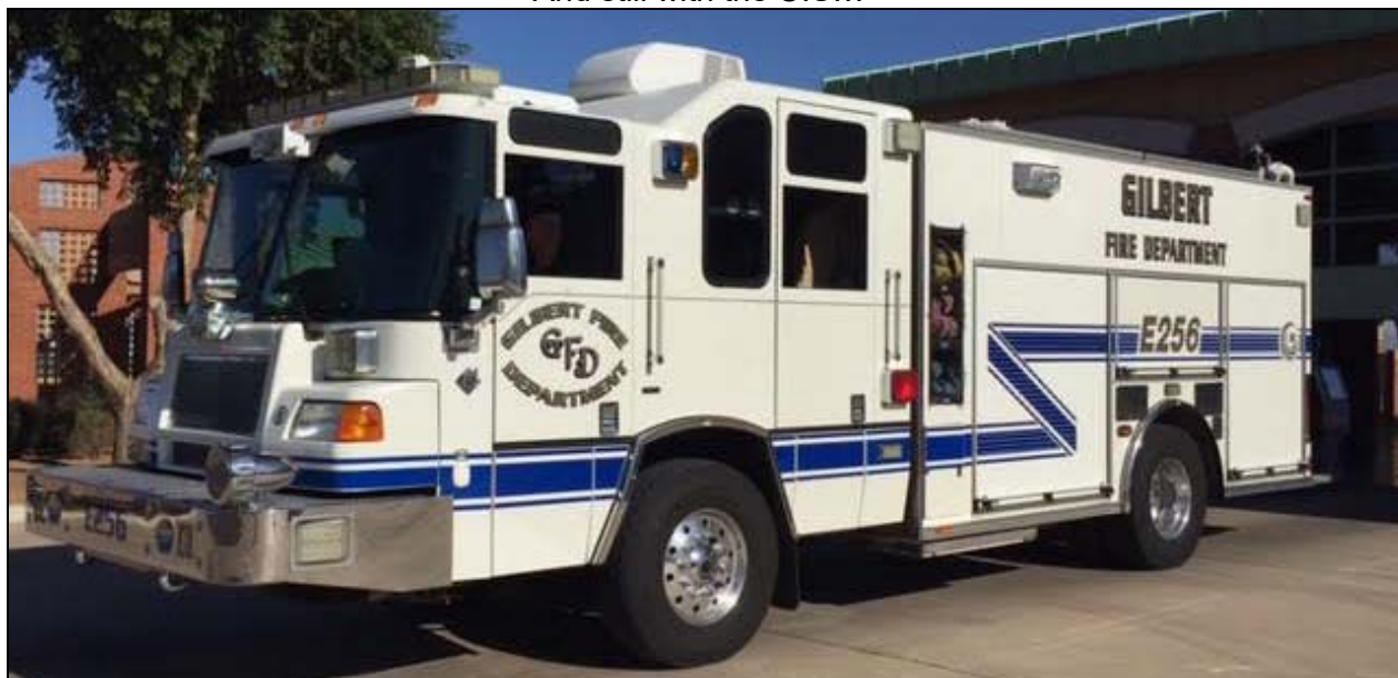
Gilbert, AZ operates this 2005 Pierce Quantum 1500/500 pumper as Engine 256.
