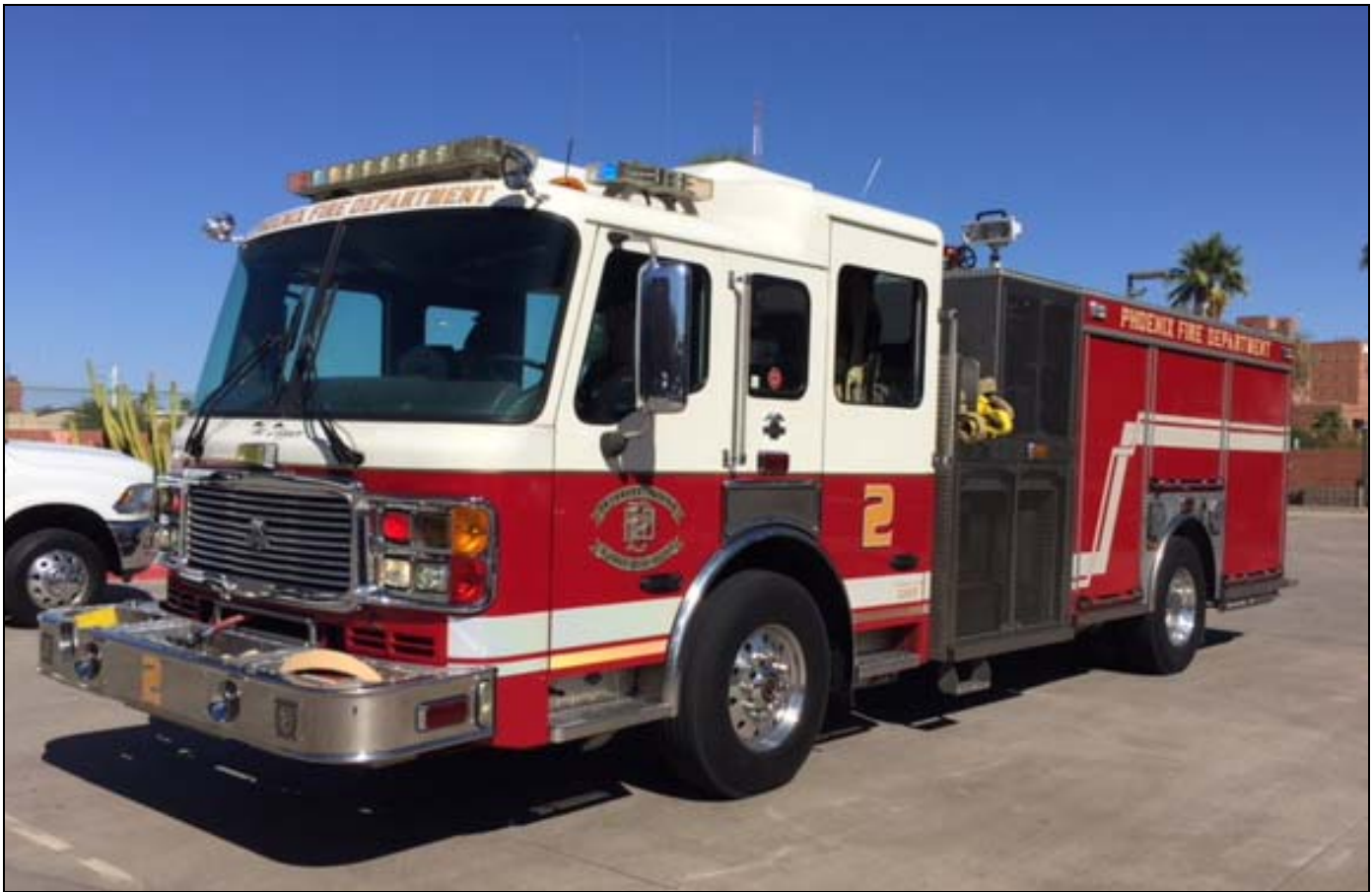
Phoenix Engine 2 is equipped with this 2003 ALF pumper, 1250gpm pump and 500gwt
