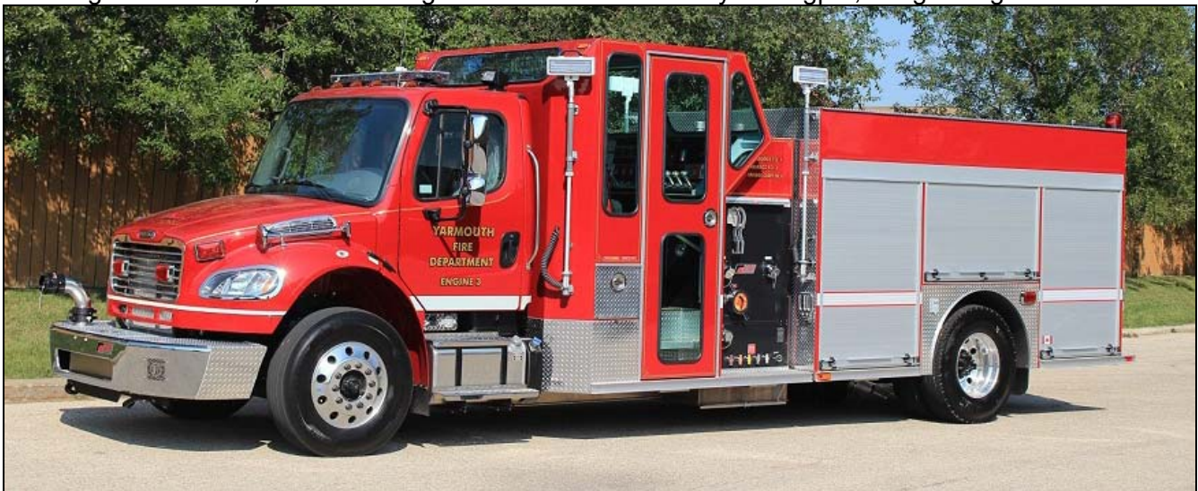
Yarmouth No. 3, NS 2016 Freightliner M2-106/Fort Garry 1050igpm(H)/800gwt/2x25gft s/n M753.
