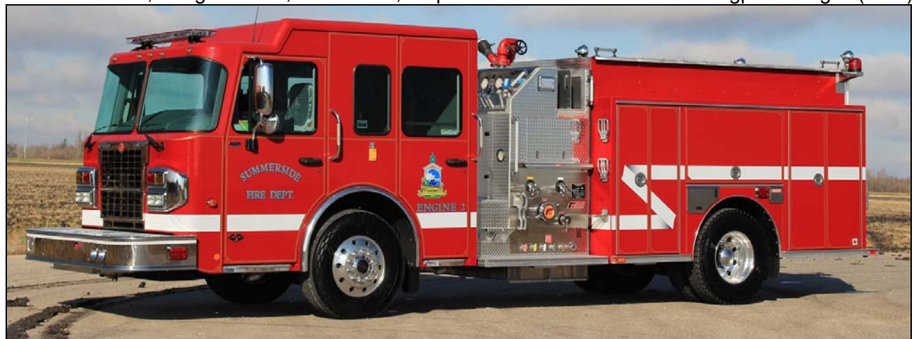
Twin to Engine 1, Summerside, PEI Engine 2, also a 2016 Spartan Metro Star/Fort Garry pumper, with a 1050igpm Darley pump, 800gwt & 10gft s/n M756 (Dave Stewardson photo).
