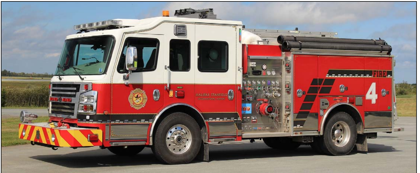
Halifax (YHZ) Red 4 2013: Rosenbauer Commander 1250igpm/630gwt/33gft
