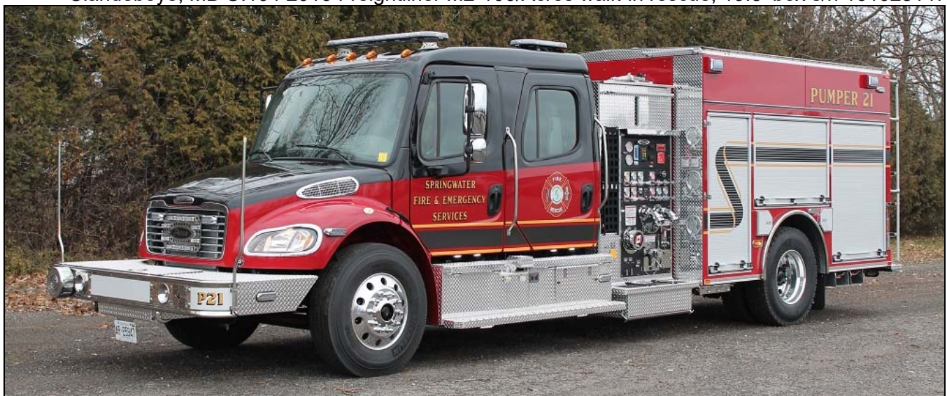
Springwater, ON P.21 (GD) 2016 Freightliner M2-106/Pierce 1061igpm(W)/840gwt/25gft Husky FS
