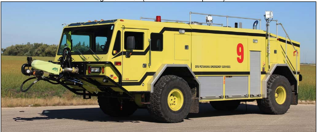
Black River FN, MB recently purchased this 2000 Waltek P4-6000 crash tender, formerly with CFB Petawawa as Red 9 (seen in it's former markings). It sports a 1050igpm pump, 1250gwt and a 95gft.
