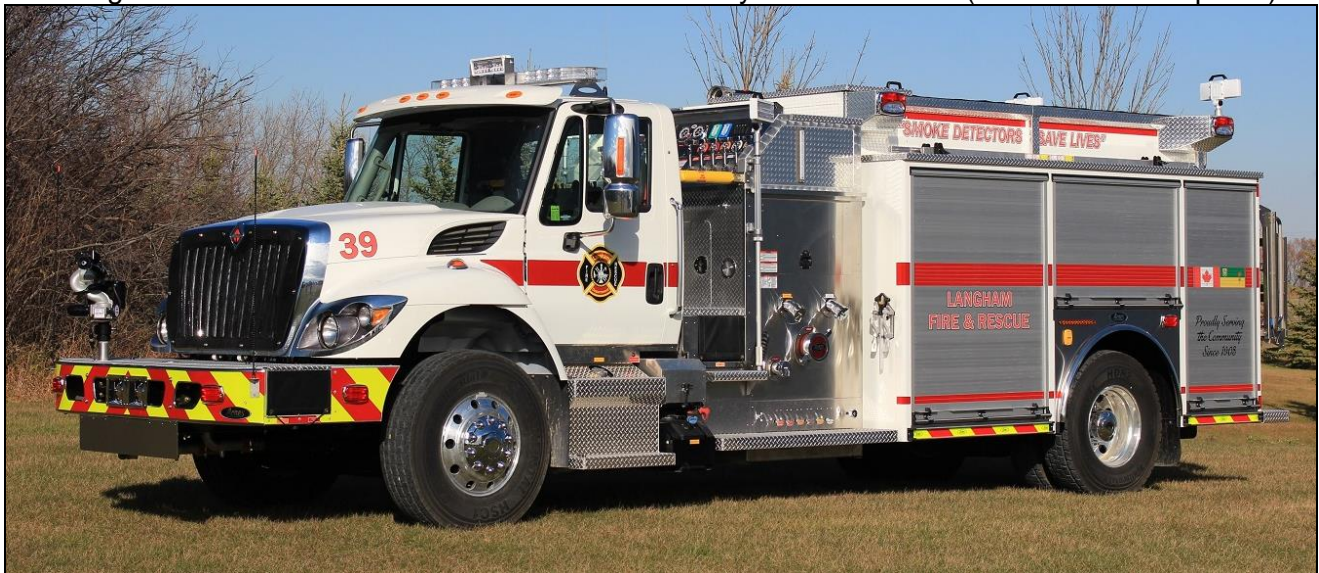
Langham, SK's new 2017 IHC 7400/Acres pump. P.39 has a 1050igpm Waterous pump, 800gwt and 25gft. s/n 171006159. Below: Carman, MB just got this 2017 Freightliner Columbia/Acres tanker, it carries 2500 imperial gallons. (Dave Stewardson photos)
