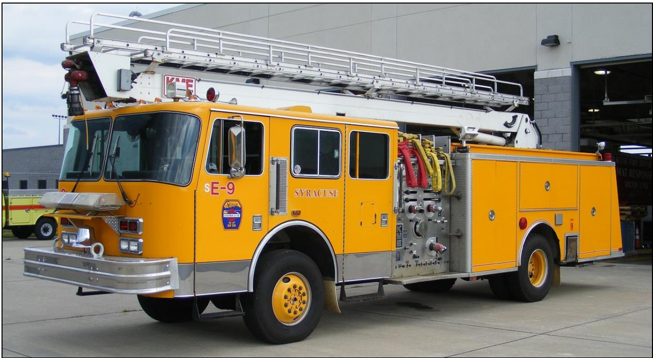
Also stationed at the airport is Spare Engine 9, a 1991 KME, 2000gpm/500gwt/50gft.
