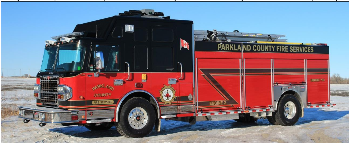
Parkland County, AB E.2 just got this 2017 Spartan Gladiator/Fort Garry pumper, it has a 1250igpm Wterous pump, 1000gwt and 2x25gft. s/n M820
