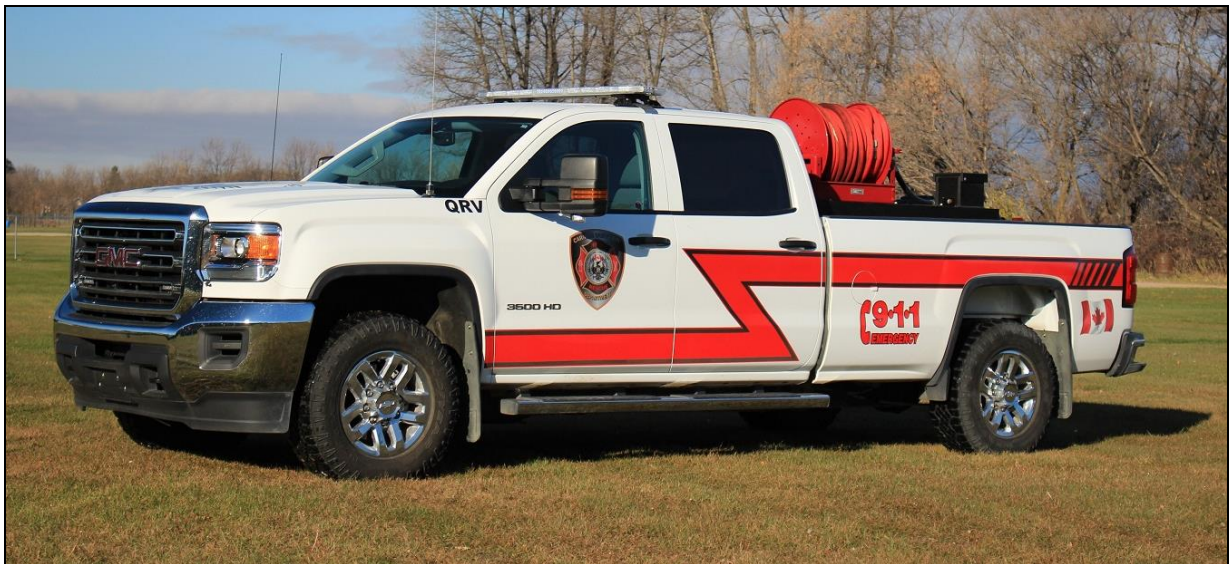
Carman, MB QRV - quick response vehicle. A 2015 Seahawk/ GMC Sierra 3500 HD 4x4 with a Waterax portable pump; 250gwt, 10gft. (Dave Stewardson photos)
