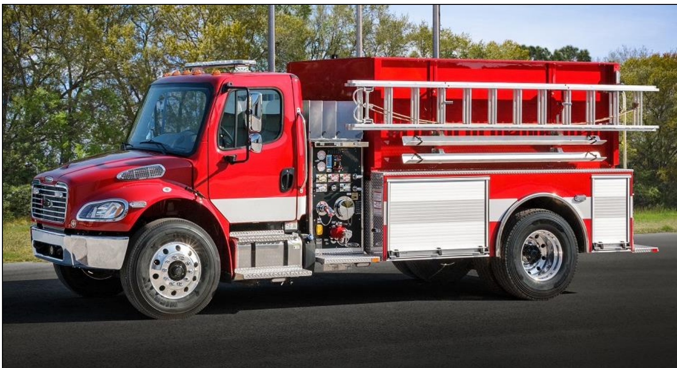
Bluewater, ON recently received this 2017 Freightliner M2 106/Pierce FXP pumper-tanker for their Brigden station. It has a 1000gpm Hale pump and a 2100gwt. s/n 30855 (Pierce photo)
