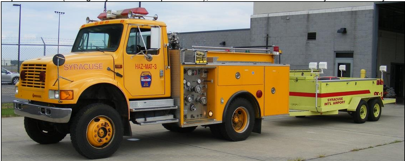
Hazmat 3 is a 1992 IHC 4900/Sutphen rig with 250gpm pump and 300gwt, also a 1000 gallon foam trailer.
