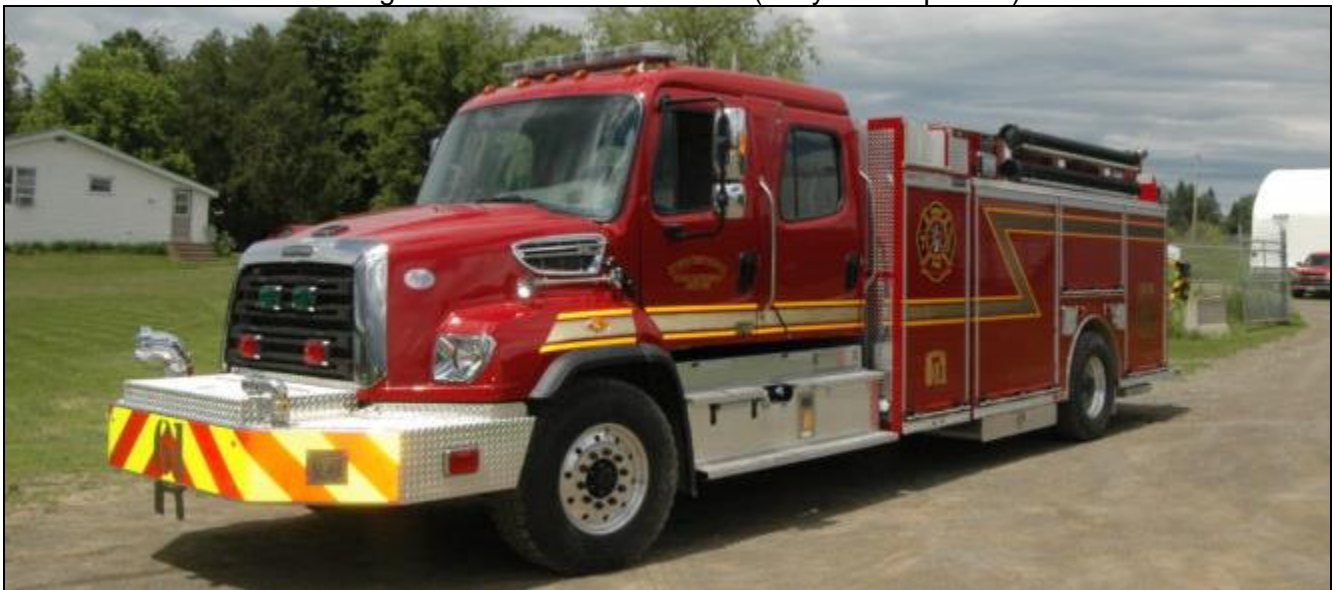
Back in the summer, Metalfab delivered this pumper to S. W. Oxford on 2017 Freightliner 114SD chassis . P.61 has a 1050igpm pump, 1000gwt, 25gft and a FoamPro 2001 foam system. (Metalfab photo)
