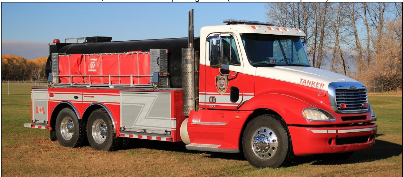
Langham, SK's new 2017 IHC 7400/Acres pump. P.39 has a 1050igpm Waterous pump, 800gwt and 25gft. s/n 171006159. Below: Carman, MB just got this 2017 Freightliner Columbia/Acres tanker, it carries 2500 imperial gallons. (Dave Stewardson photos)
