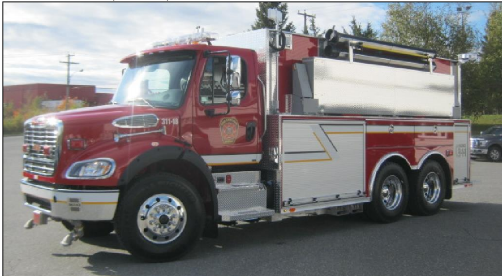
Baie St.-Paul, QC 211, a 2017 Freightliner M2-112/Maxi Métal pumper with a 1050igpm pump, 840gwt, and a 25gft, with a FoamPro 2002 foam system.
