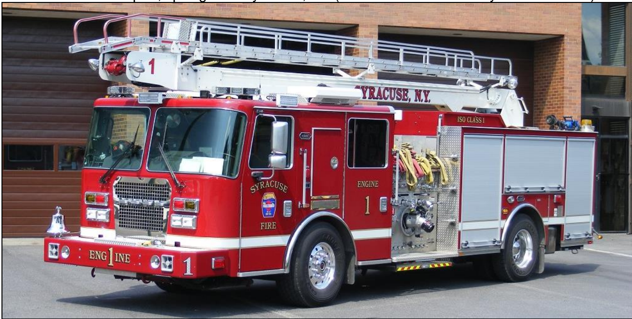
Syracuse Engine 1 is a 2014 KME pumper with a 2000gpm pump, 500gwt and 55' aerial.
