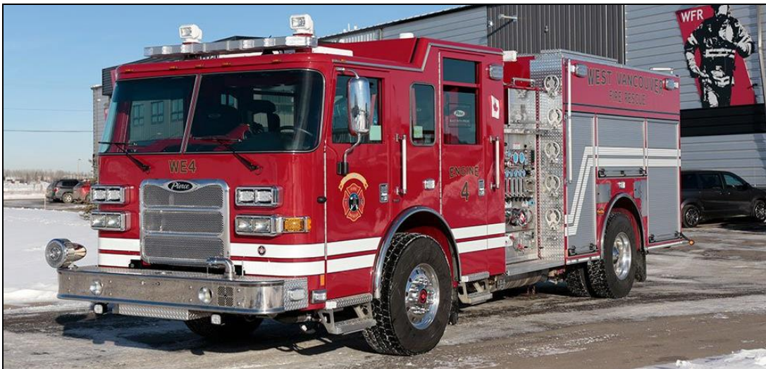
Received last year, W. Vancouver, BC Engine 4, a 2016 Pierce Arrow XT, with a 1750igpm Waterous pump, 330gwt, 25gft, and Husky Foam System, JN 30100. (WFR photo)
