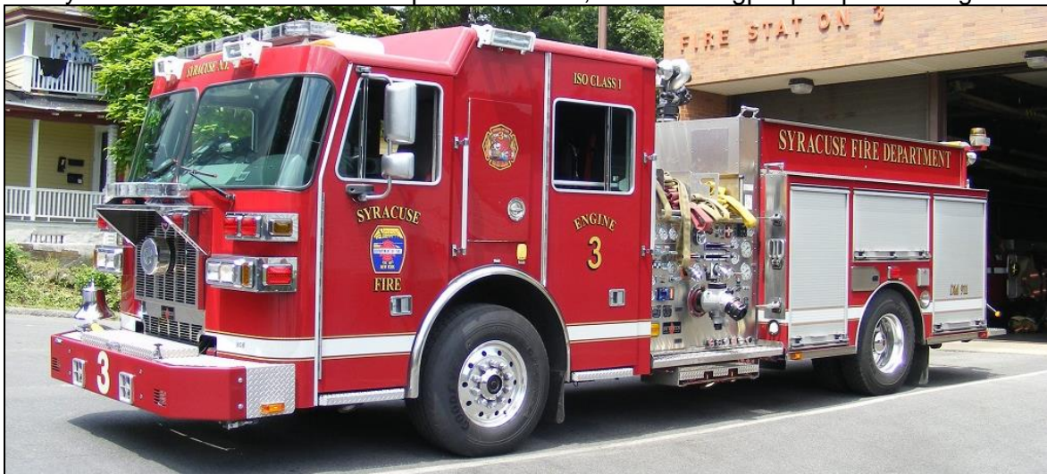
Engine 3 is a 2010 Sutphen pumper, with a 2000gpm pump and 500gwt.
