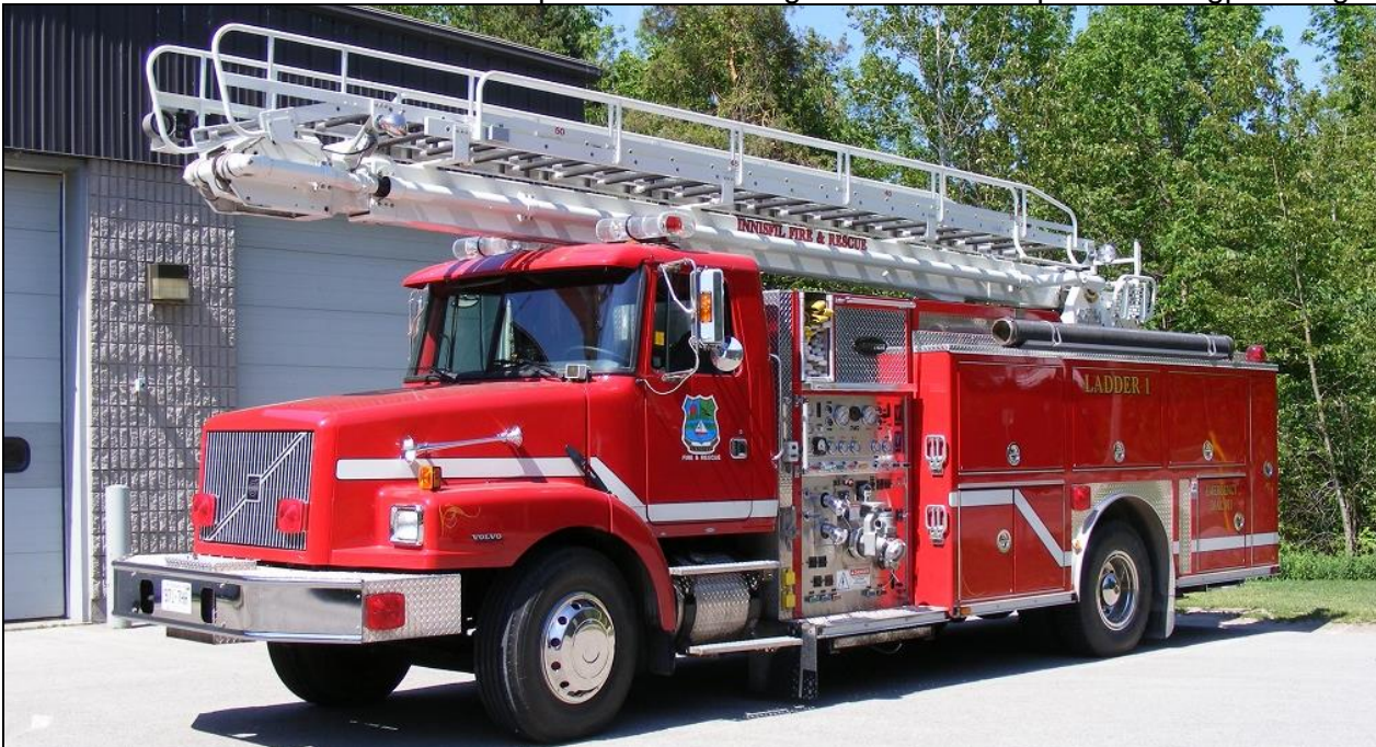
Ladder 3 - 2000 Volvo WG42 / Superior 50' TS 1050igpm/500gwt/40gft(B). S#SE 2144
