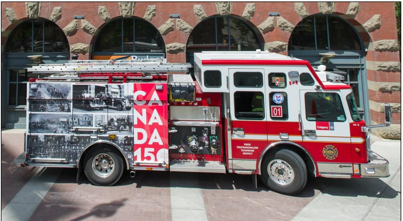
Calgary FD's wrap for Canada 150. CFD Engine 1 in front of the fire museum at former CFD Station 1. It is a 2016 Spartan Gladiator Classic/Smeal pumper with a 1500igpm pump, 500gwt, 30gft(A) and a CAFS.
