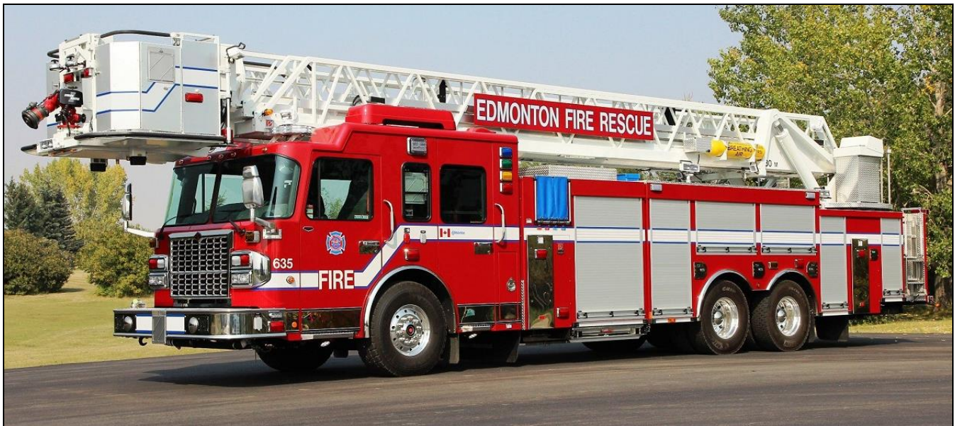
One of Edmonton's new 2017 Spartan/Smeal platforms, each one has a 1500igmpump, 250gwt and 2x25gfts with a 100' tower and FoamPro 2002 foam system. S/O 4678 (John Bowerman photo)
