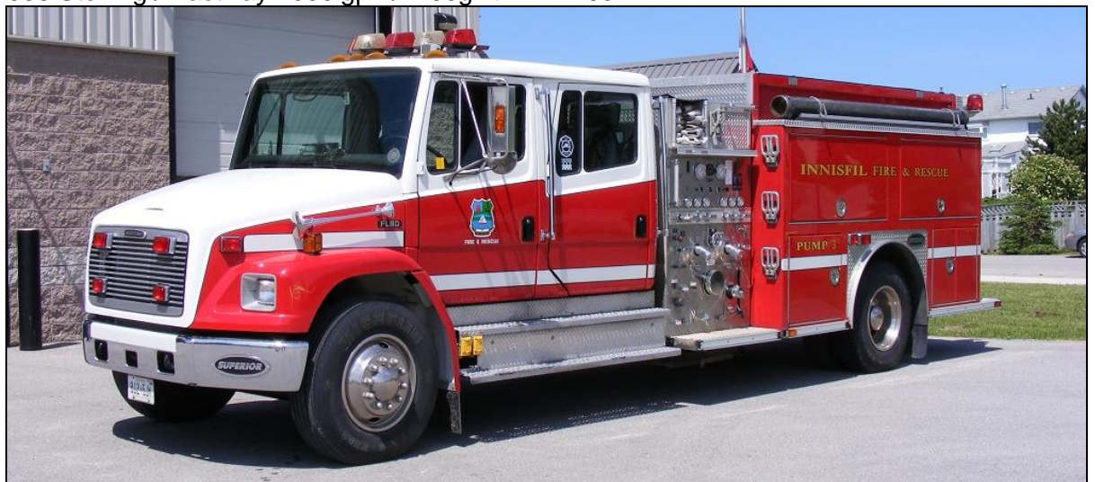
Pumper 3 - 2000 Freightliner FL80 / Superior 1050igpm/900gwt/30gft S#SE 2038
