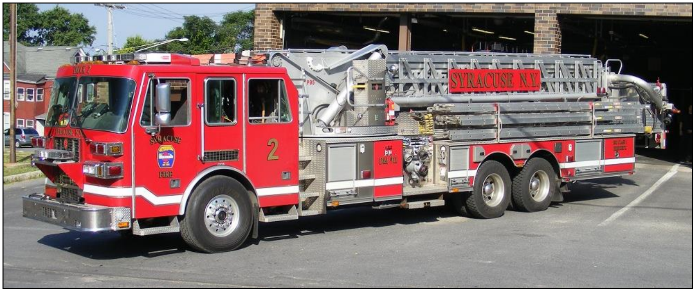
Syracuse Truck 2 is a 2007 Sutphen 95' tower, with a 1500gpm pump and 300gwt.
