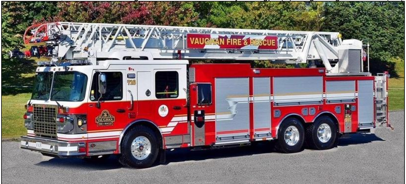
Vaughan's new Aerial 716, a 2017 Spartan/Smeal quint with a 1750igpm Waterous pump, 400gwt and a 105' stick. s/n S4675. (Smeal)
