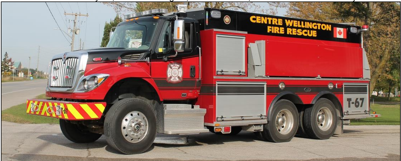
Center Wellington, ON Tanker 67 is a 2015 International 7500/KME rig, it has a 500gpm pump and a 2500gwt. It is stationed in Elmira. (Gary Dinkel photos)
