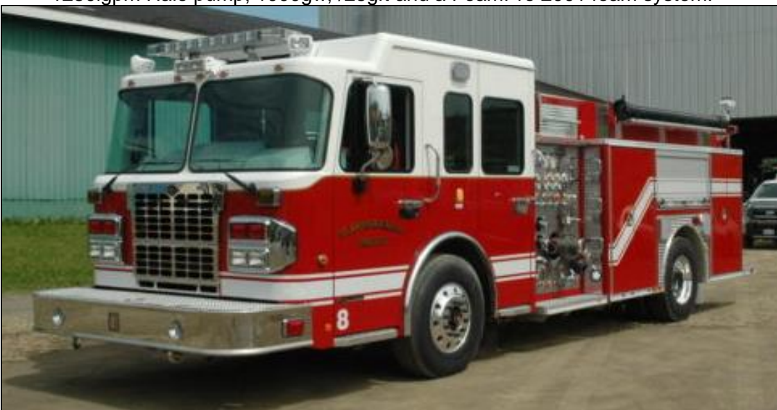
St. Johns, NL Unit 8, a 2016 Spartan Advantage/Metalfab rig, 1500igpm/500gwt. (SN M06-6193) (Photos this page from Metalfab Fire trucks)
