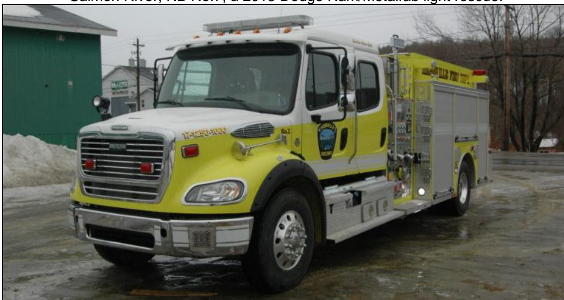
Hebbville, NS is a Engine 15 2017 Freightliner M2-112/Metalfab product, with a 1250igpm Hale pump, 1000gw, /25gft and a FoamPro 2001 foam system.
