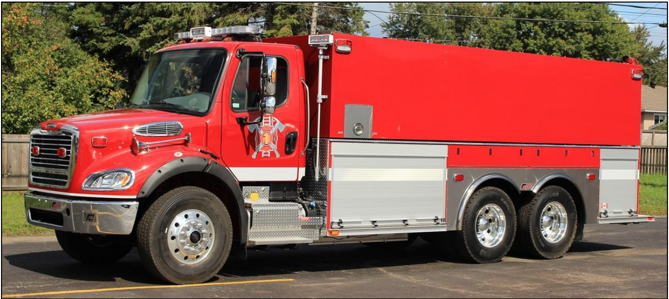
Thunder Bay Tanker 1, a 2017 Freightliner M2 112/Fort Garry rig, 420igpm Hale, 3000gwt (SN M851)
