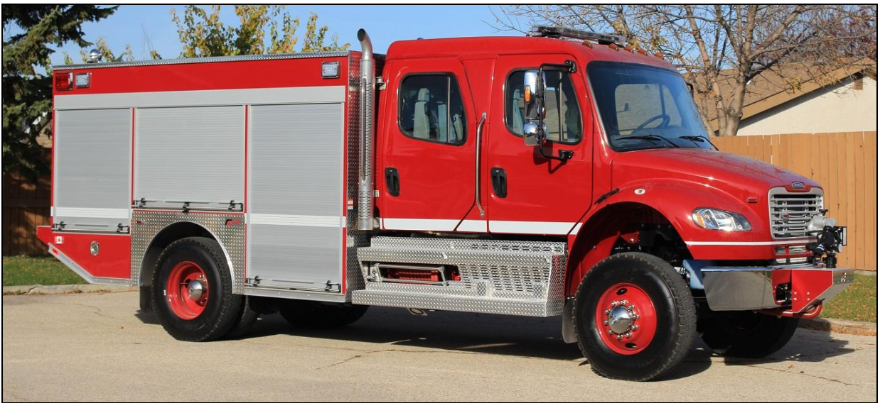
Sturgeon Lake Cree Nation, Alberta. 19 Sept 2017 Fort Garry Fire Trucks/FL-M2-106 4x4 Farley PSR 1250 pump 1050/1000. s/n #M819
