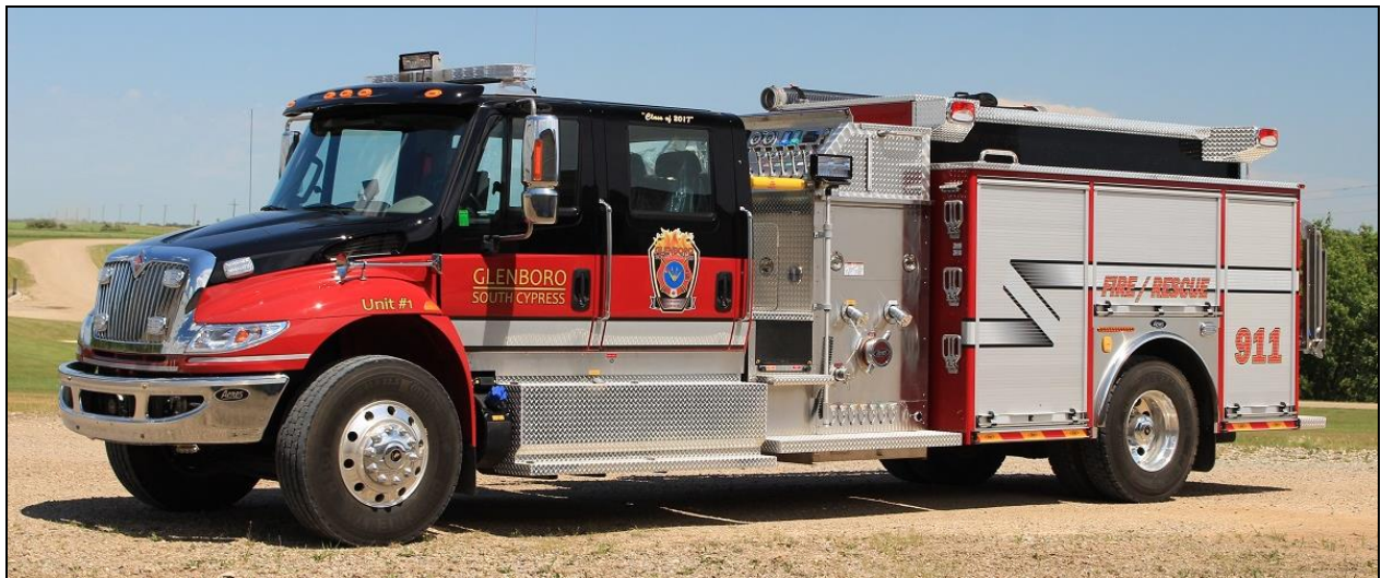
A recent acquisition by Glenboro-South Cypress, MB, is this 2017 IHC 7400/Acrs truck, equipped with a 1050igpm Waterous pump, 1000gwt and 25gft.
