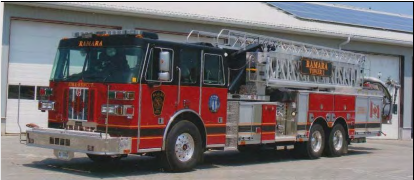
Three new rigs from Simcoe County, first up is Ramara's new 2011 Sutphen Monarch Tower 1, received last fall in Brechin. The 100' midship mount has a 1250igpm pump, 250gwt & 20gft. SNs M271 & HS4960.
