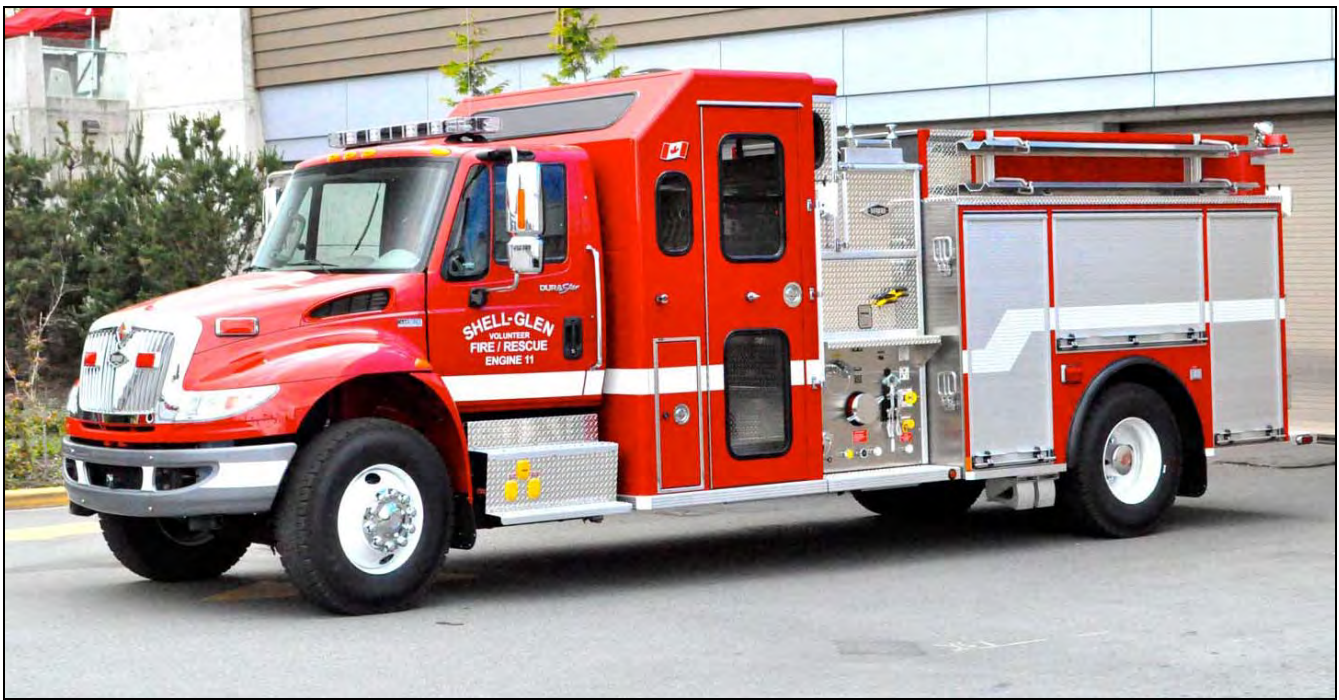
This IHC 4400/Hub 1050igpm/800gwt/25gft is new to Shell-Glen, BC. Running as Engine 11, is it equipped with a Foam Pro 2001 foam system and fully enclosed top-mount pump panel. (Terry Yip photo)
