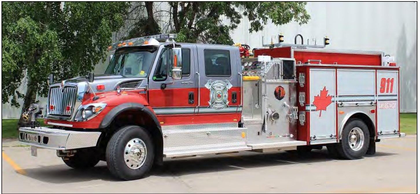
This grey over red pumper belongs to Erickson, MB. Delivered in the summer, it is the first rig produced under the Acres badge (formerly Green Acres). Built on a 2012 IHC 7500 chassis, it has a 1050igpm pump, 840gwt and a 25gft along with a CAFS. (Both photos and info from Dave Stewardson)
