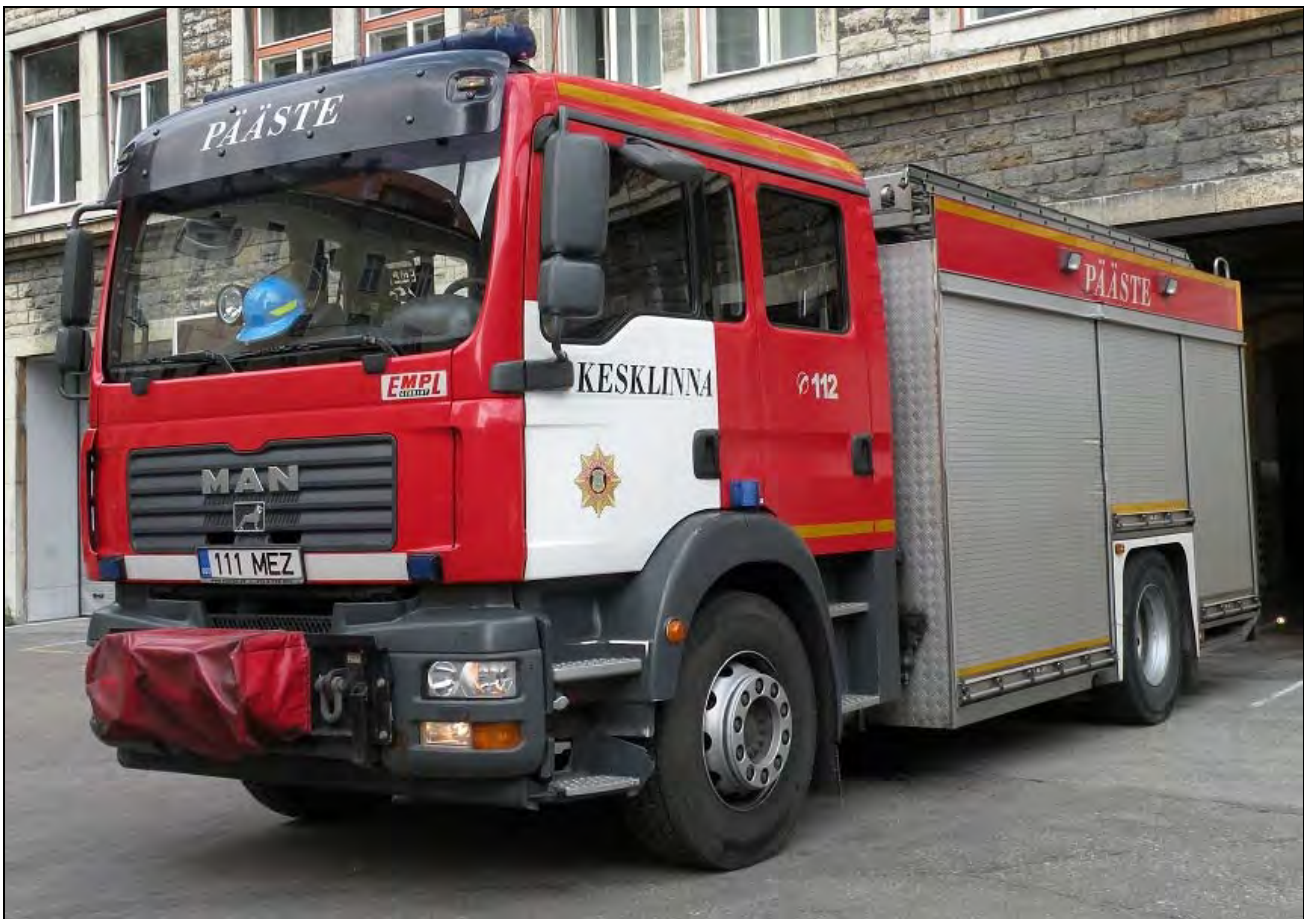
This MAN chassis heavy rescue belongs to Tallinn, Estonia. The 2007 vehicle with body by EMPL, has a 3000L water tank, 200L foam tank and carries 50L of firefighting chemicals. EMPL is an Austrian custom apparatus builder known for all-terrain vehicles and specialty rigs. Below is a rescue pumper from Gdynia, Poland. This was built on a 2009 Scania P340 chassis by ISS (another major manufacturer), and has a 3200LPM pump, 5000LWT and carries 500L of foam. (Robert Herscovitch photos)
