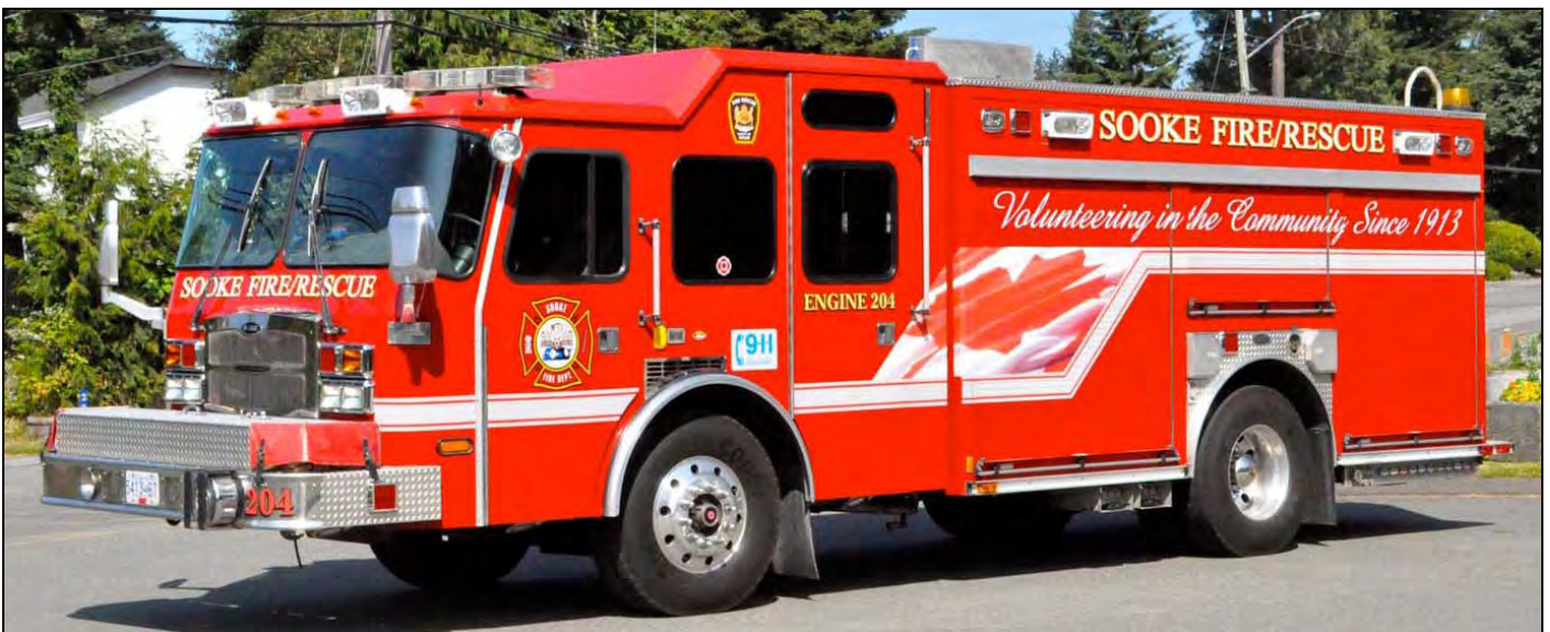
A couple from the left coast: Pitt Meadows BC Engine 1-1 is a 2011 Pierce Arrow XT 1250/650/30. Now in service as Sooke FRS Engine 204 is a 2006 E-One Typhoon 1250/500 with CAFS, formerly with Maricopa FD.
