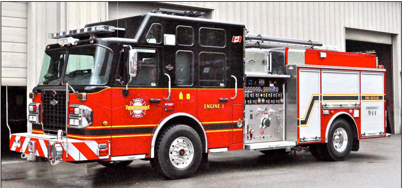
Mission, BC E1, a 2012 Spartan Metro Star/Hub pumper equipped with a 1500igpm pump, 500gwt and Foam Pro 2001 foam system. The black over red rig was delivered this summer. (Terry Yip photo)
