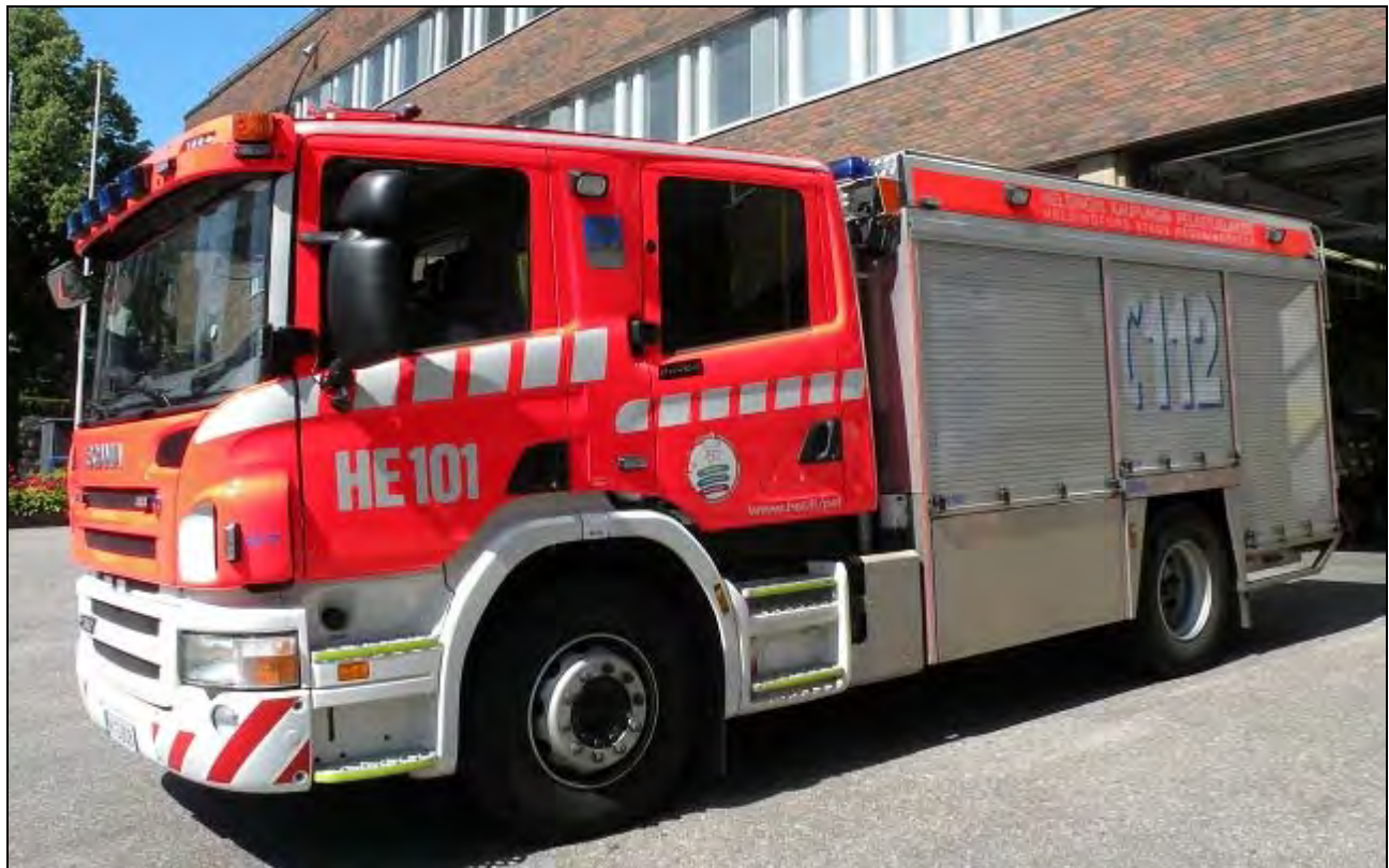
Also running from HQ is this 2012 Scania chassied Rescue Pump. HE 101 has a 2400L pump and carries 3000L of water. (Robert Herscovitch photos).
