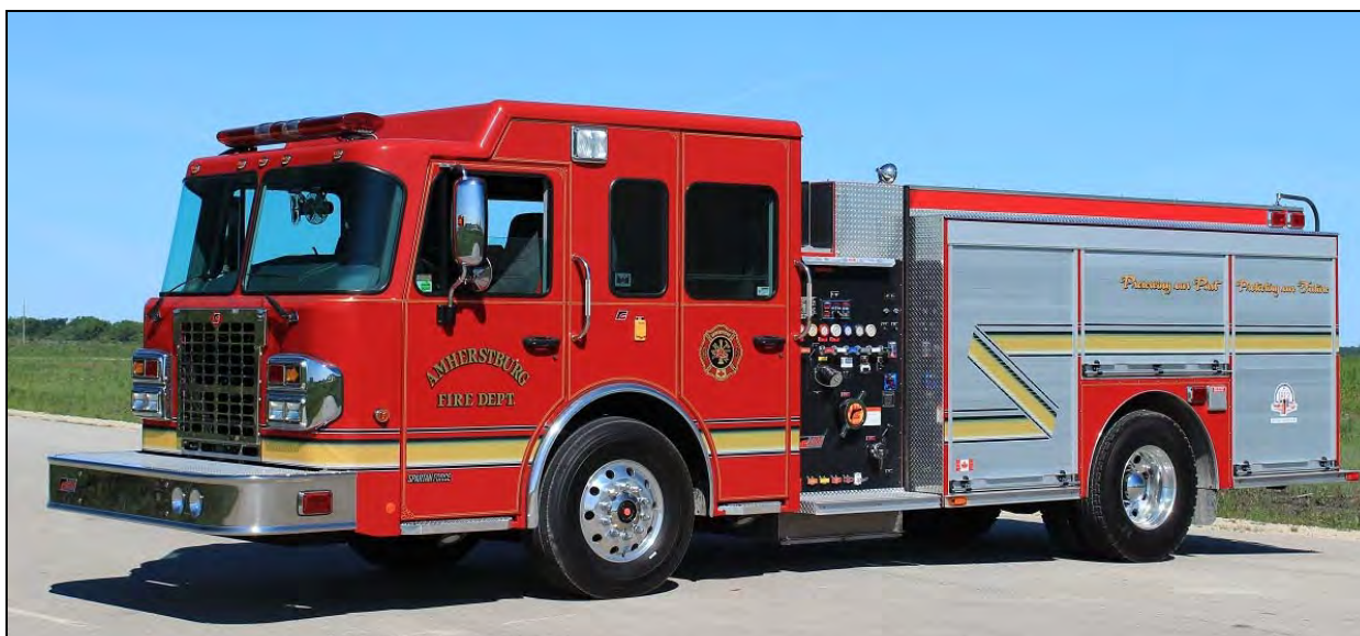
Delivered earlier this year is Amherstberg's new pumper from Fort Garry on a 2012 Spartan Force chassis. The bright red rig has a 1250igpm pump and an 800gwt, SN M280.. (Dave Stewardson photos)
