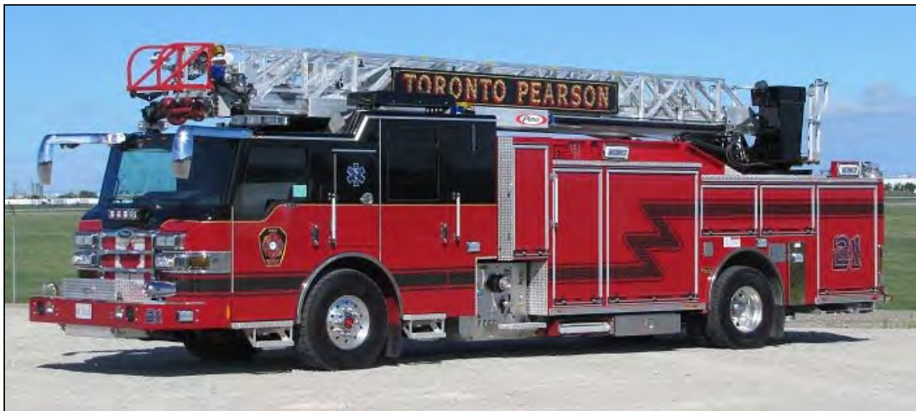
This Pierce Velocity 75' rearmount runs as Aerial 21 at Pearson, it has a 1250igpm pump and 400gwt.
