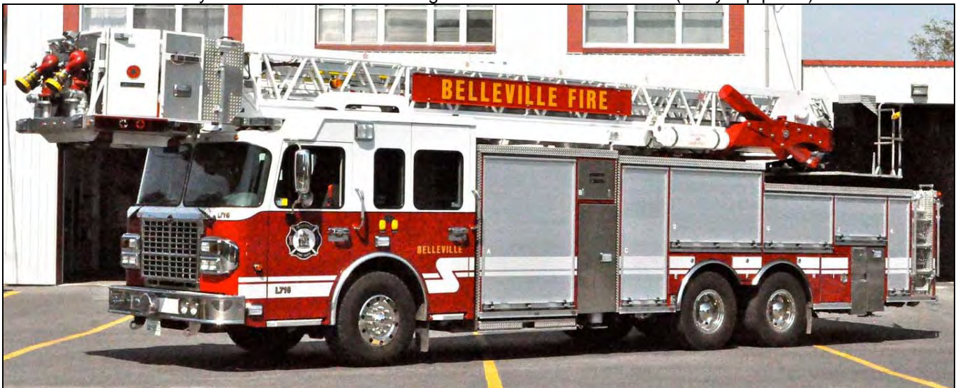
Above, Belleville's Ladder 716 is a 2011 Spartan Gladiator/DEV/Crimson tower, 1750/300/100'. (Terry Yip photo) Below, P711, a 2012 Spartan/Eastway 1250igpm with 500gwt & 30gft, both run from Station 1. (Neil McCarten photo)
