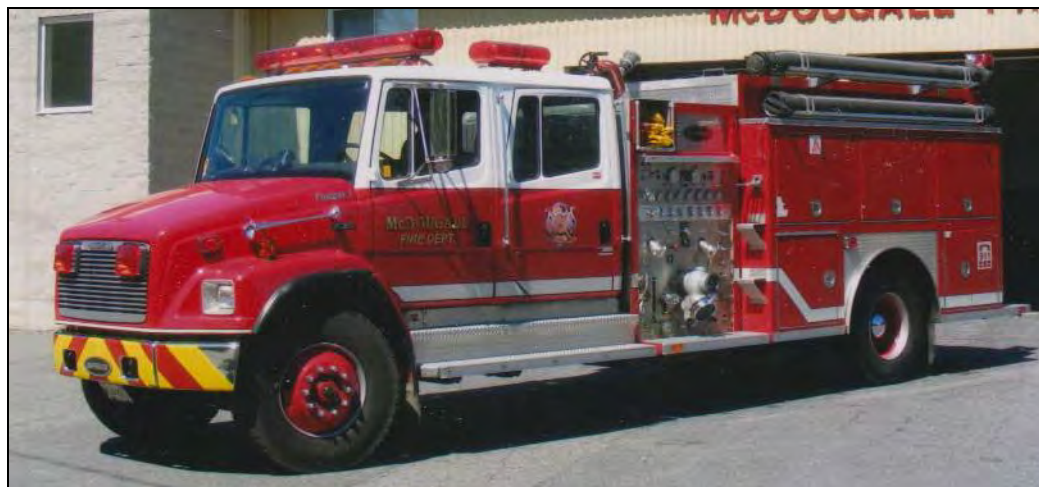
Above: McDougall Pump 1, a 1993 Freightliner FL80/Superior 1050igpm/800gwt. Below: McDougall Tanker 1, a 2008 Freightliner M2/Plastisol/Dependable 600igpm/3000gwt. (Photos by Brian Leduc)
