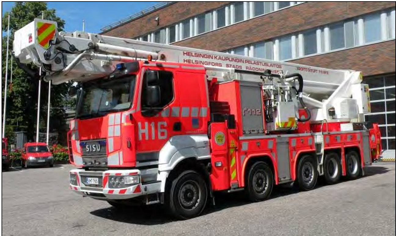
This monster, the tallest I've come across, can elevate to an incredible 61m. Stationed at Helsinki, Finland's HQ, this 2011 Bronto product was built on a SISU chassis (a local truck builder).
