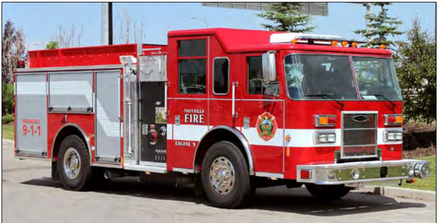
Foothills Fire Engine 9, a 2012 Pierce Sabre with a 1050igpm pump, 800gwt, and a 16gft. It also has a Husky 3 foam system. (John Bowerman photo).
