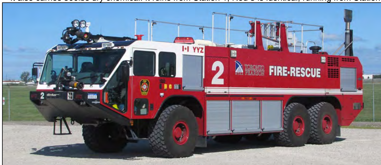
Red 2 is a 2007 Osh Kosh Stryker 3000, with a 1625gpm pump, 2400gwt and 420gft. Red 5, built in 2006, has the same specs, and runs from Station 1, Red 2 is at Station 2. (Desmond Brett photos)
