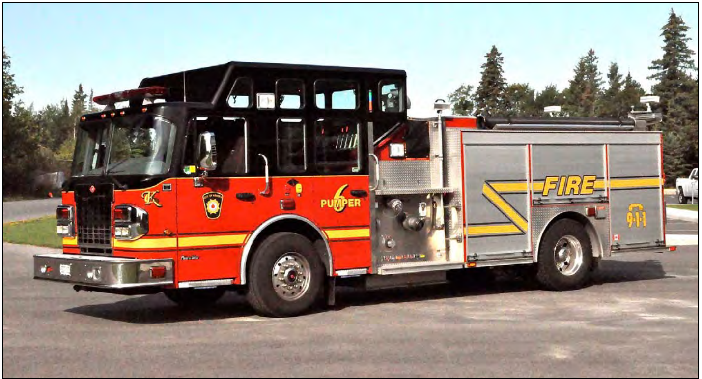
A couple more from the north, this is Thunder Bay Pumper 6, a 2011 Spartan Metro Star Fort Garry number with a 1250igpm pump, 800gwt and 30gft.
