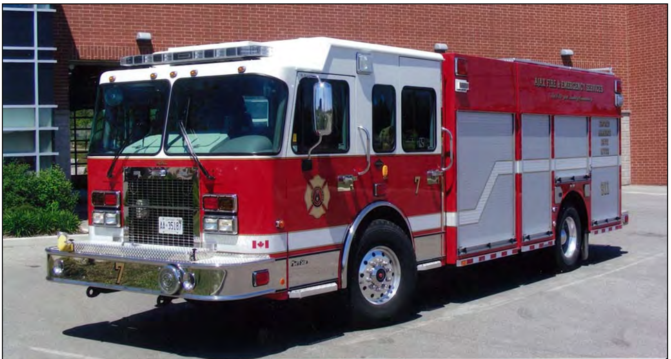
Ajax Pump 7, a 2010 Spartan Metro Star/SVI with a 1500igpm pump, 500gwt and a pair of 50gfts. (Neil McCarten photo)
