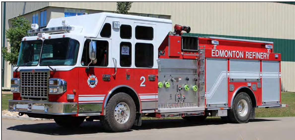
This 2012 Spartan Gladiator/Smeal pumper with a Hale 2000igpm pump, 1500gft and Chubb-National Foam input, recently went into service with Suncor's Edmonton Refinery.
