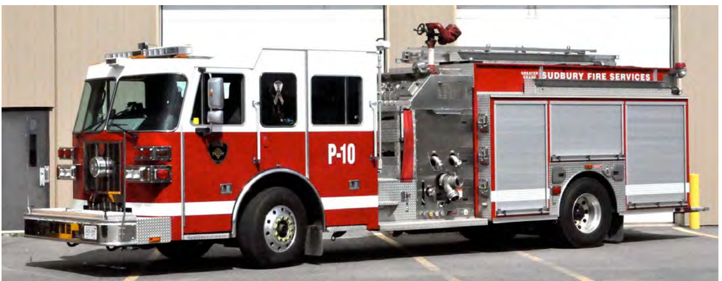
This 2009 Sutphen Shield 1250igpm/800gwt/20gft pumper runs from Sudbury's Azilda Station. (Terry Yip photos)
