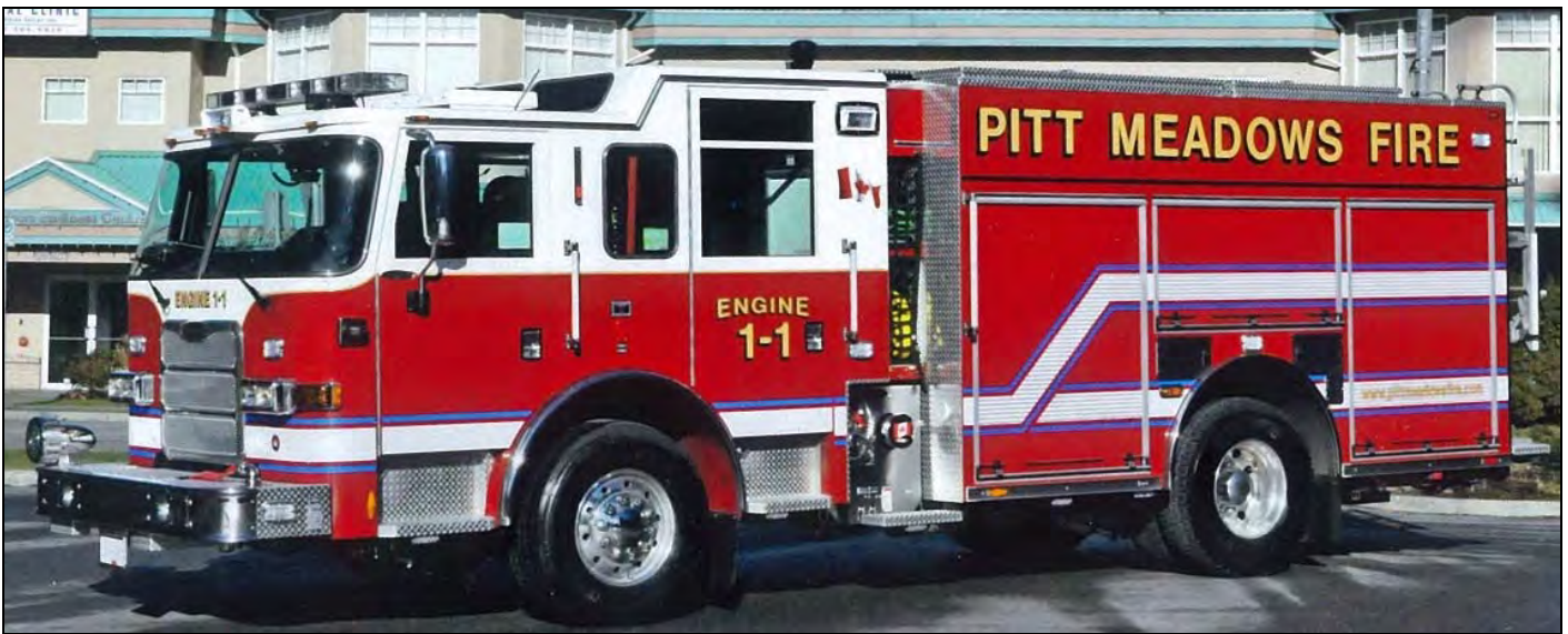
A couple from the left coast: Pitt Meadows BC Engine 1-1 is a 2011 Pierce Arrow XT 1250/650/30. Now in service as Sooke FRS Engine 204 is a 2006 E-One Typhoon 1250/500 with CAFS, formerly with Maricopa FD.
