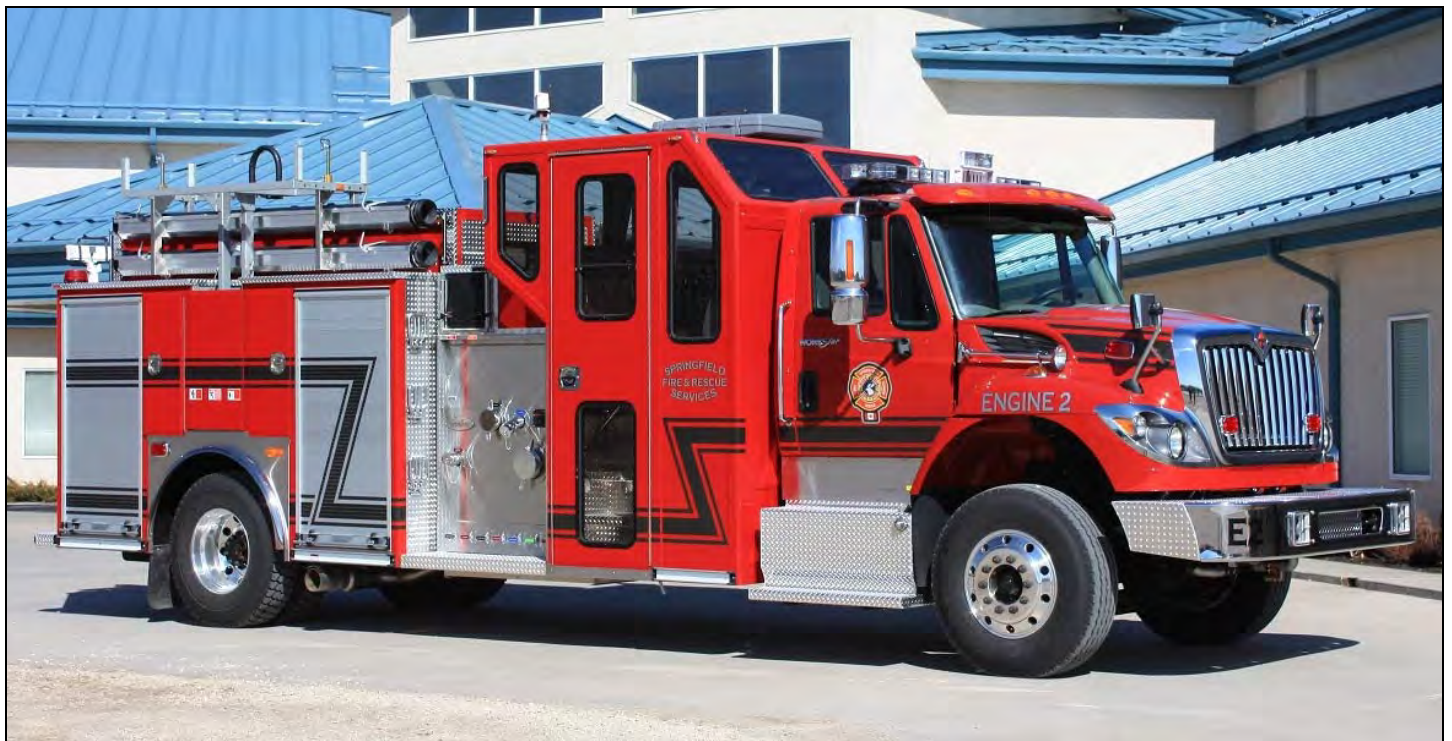
Another new Manitoba truck, this pumper went to Springfield, and is assigned to Engine 2. It's 2012 International 7400/Green Acres 1050/1000/30, with a fully enclosed, top mount pump panel.
