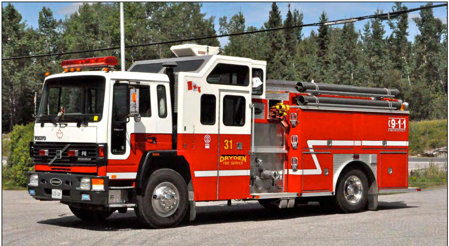
Dryden Pump 31 is a 1996 Volvo FE42, business end built by Superior. It has a 1050igpm pump, 800gwt and 35gft. (Terry Yip photos)
