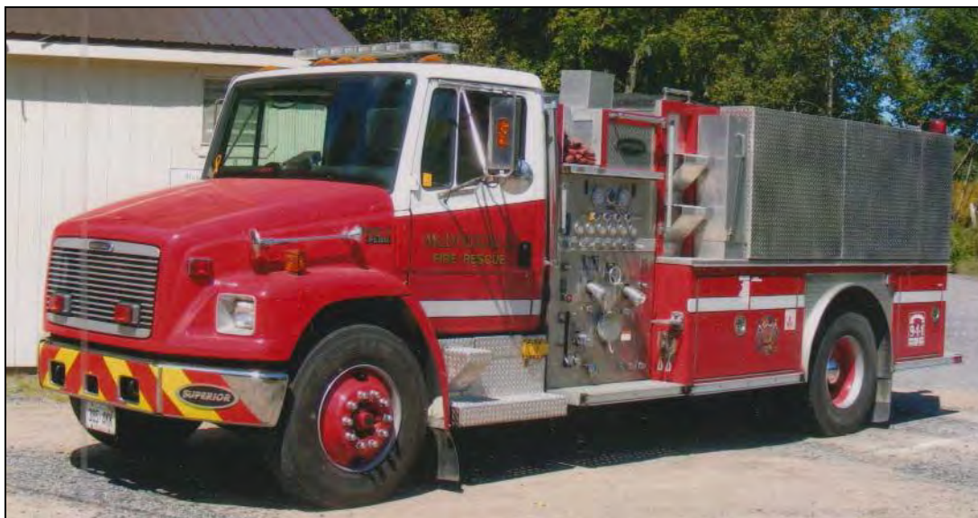
McDougall Tanker 2, a 2001 Freightliner FL80/Superior 1050igpm, 1200gwt
