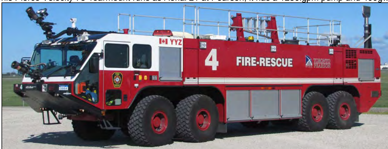
Also at Pearson is this 2009 Osh Kosh Stryker 4500. Red 4 has a 1625igpm pump, 3750gwt and 540gft. It also carries 500lbs dry chemical. It ruins from Station 1, Red 3 is identical, running from Station 2.
