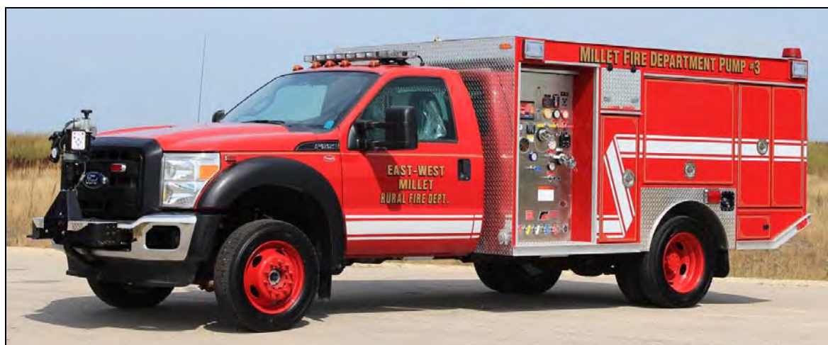
Millet, AB Pump 3, a 2012 Fort Garry/Ford F550 with 420igpm/300gwt/10gft.
