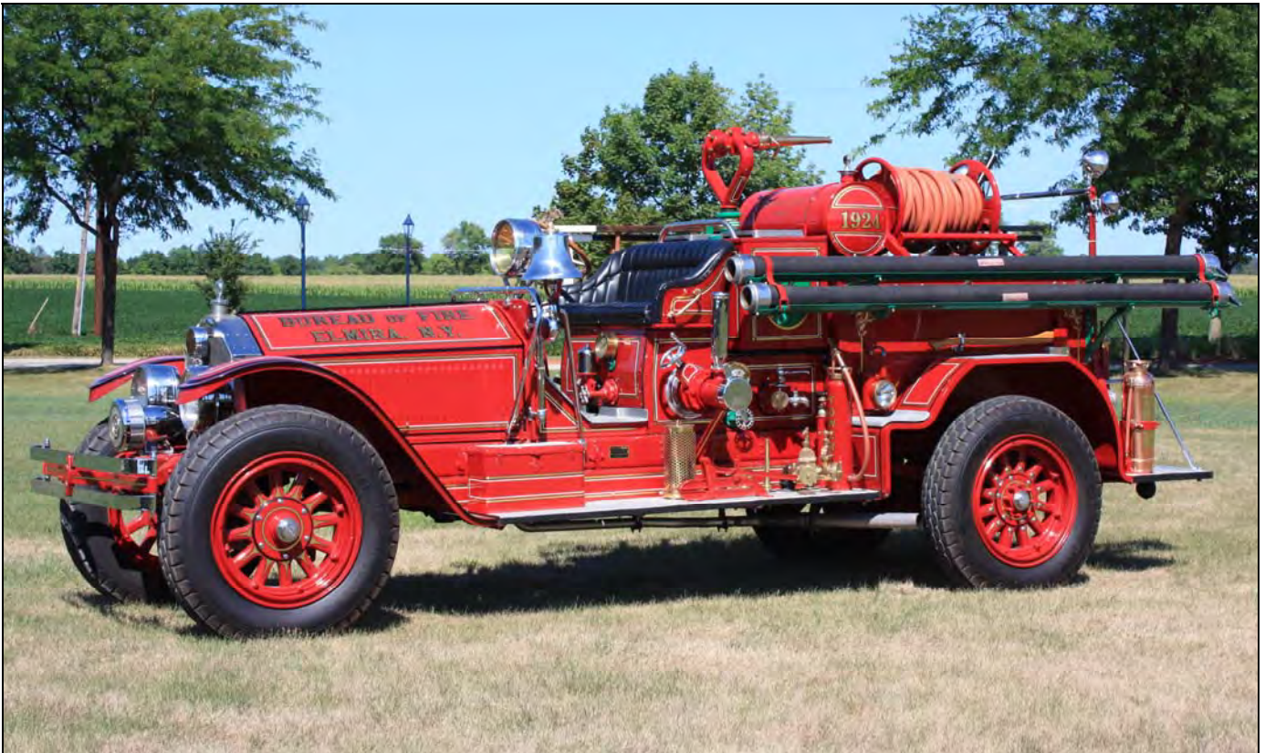
Another beautifully preserved rig, a 1924 American LaFrance Type 12 pumper with a 1000gpm pump and 60gwt. It was in service with Elmira, NY. Both rigs are privately owned. (Herb Galloway photos)
