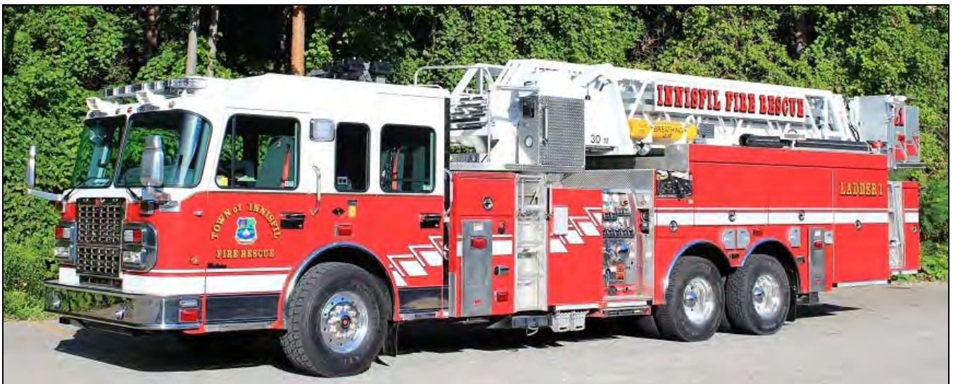
Innisfil recently received this 2011 Spartan Gladiator/Smeal 100' tower. It has a 1500igpm pump, 250gwt & 15gft. SN 3927 is assigned to Station 1 in Alcona. (Dave Stewardson photos)
