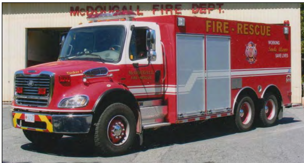
Above: McDougall Pump 1, a 1993 Freightliner FL80/Superior 1050igpm/800gwt. Below: McDougall Tanker 1, a 2008 Freightliner M2/Plastisol/Dependable 600igpm/3000gwt. (Photos by Brian Leduc)
