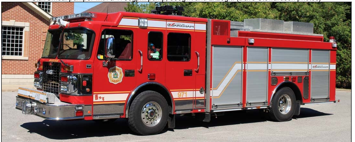
When he took the delivery shot of this rig for us last winter, Dave promised to reshoot it with the proper graphics and, true to his word, here is Thunder Bay Pumper 6, a 2015 Spartan Metro Star X/Fort Garry rig, in service. 1050igpm/600gwt #M597. Below is Markham 971, delivered last year. It's a 2014 Spartan Metro Star/Smeal pumper with a 1750gpm pump, 500gwt and 2x20gft. (Dave Stewardson photos)
