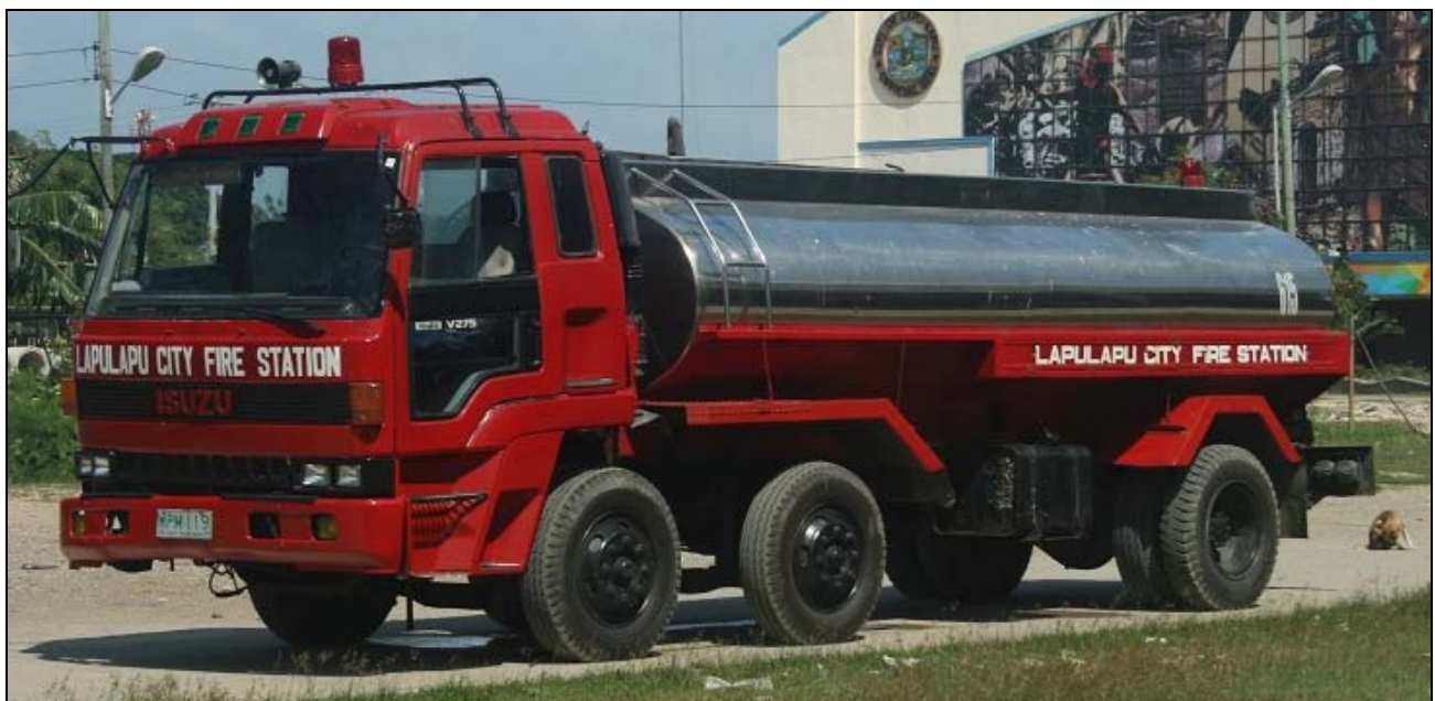
Also in Lapu-Lapu, Tanker 3 on an Isuzu V275 chassis has a 500gpm pump and 2000gwt.
