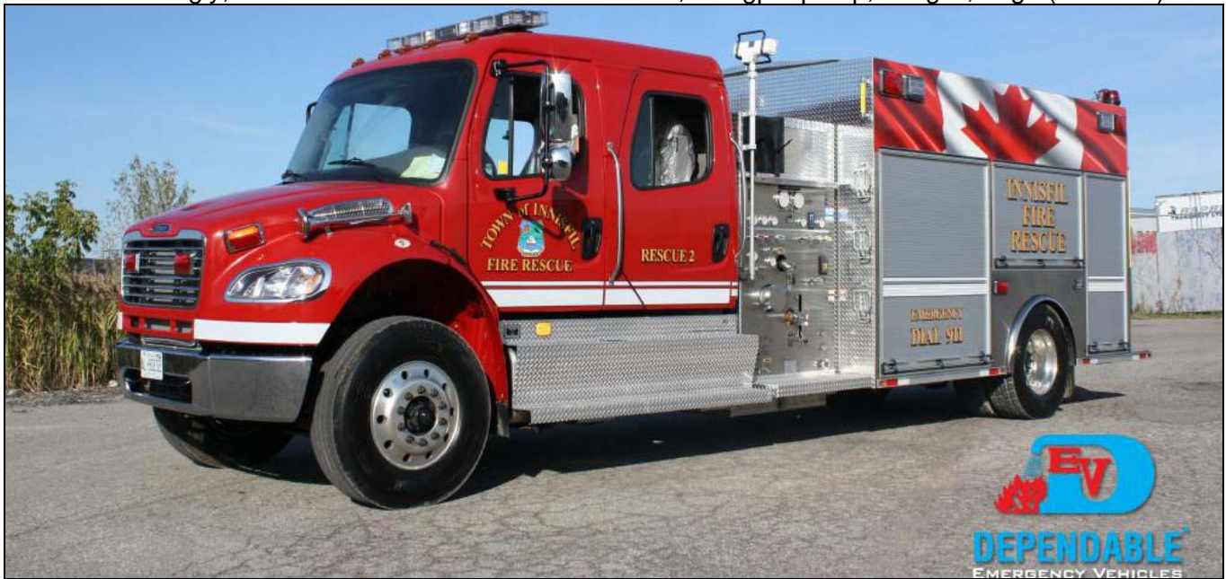
Innisfil, ON Rescue 2, a 2015 Freightliner M2-106/Dependable rig, has a 1500gpm Hale pump and a 1500gwt. (Photo credit: Dependable Emergency Vehicles)
