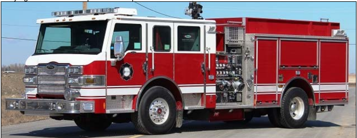
North West Redwater, AB recently put this 2015 Pierce Velocity pumper in service. It has a Waterous 1500gpm pump and 750gwt. It also has a Husky 12 foam system and 25gft. (John Bowerman photos))
