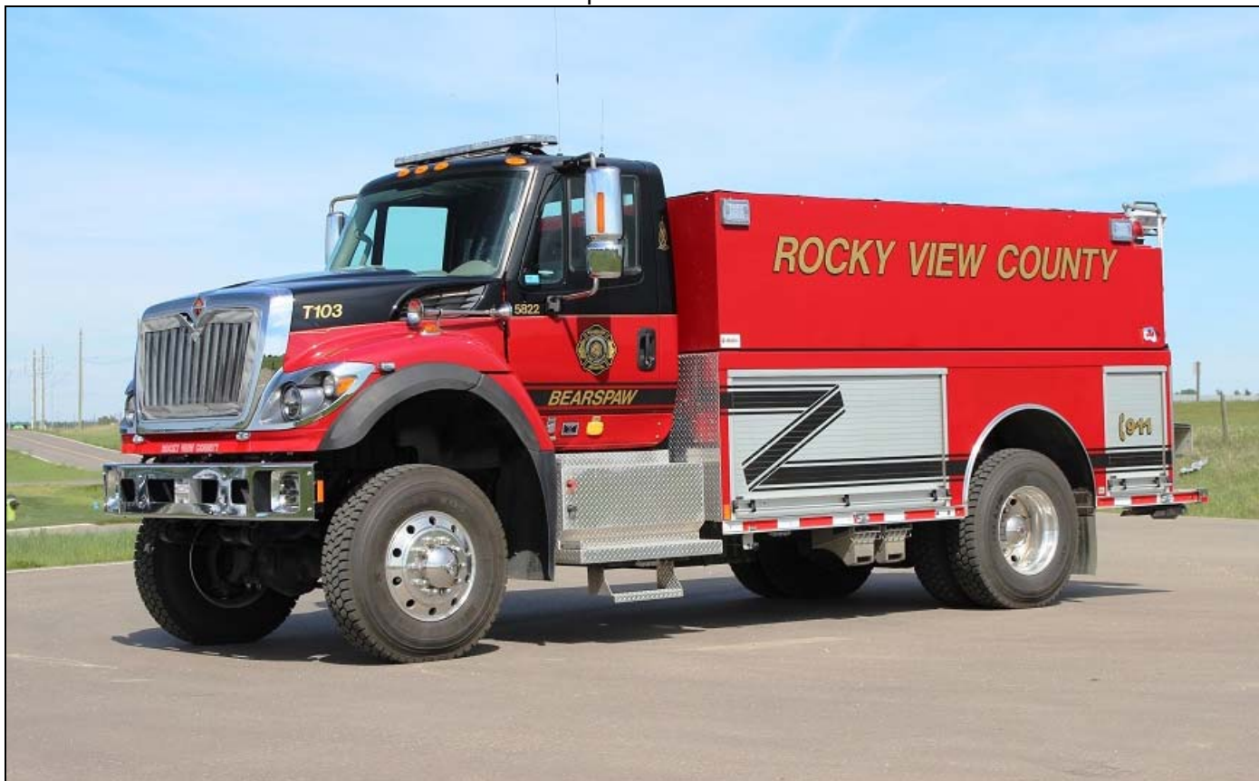
Rocky View, AB Tender103 was delivered with a matching pumper in the summer. It's a Rosenbauer product on a 2015 IHC 7400 4x4 chassis with a 625igpm pump and 1500gwt. (John Bowerman photo)
