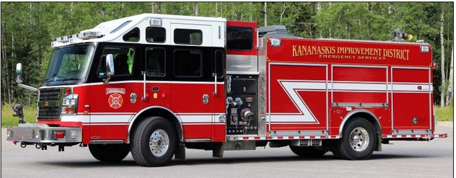
Kananaskis, AB recently put this 2015 Rosenbauer pump in service, it has a 1261igpm pump, 461gwt and 40gft. SN 16462 (John Bowerman photo)
