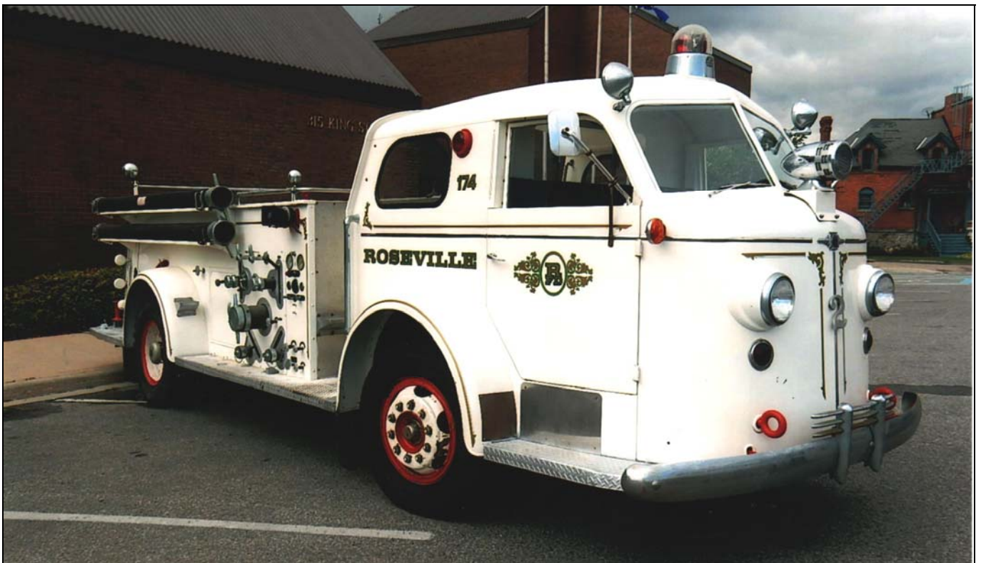
Two rigs from the Chatham Firefest; above is a 1947 American LaFrance 700 series 1000gpm engine originally with Roseville, MI. It's owned by Brent Denure Below is a 1970 Ward LaFrance (Rehabbed in 1990) from Chicago. Former Engine 39 (and 46) has a 2000gpm pump. Owned by Mike Kovac, it's done up as a twin to the truck from Backdraught . (Walt McCall photos)
