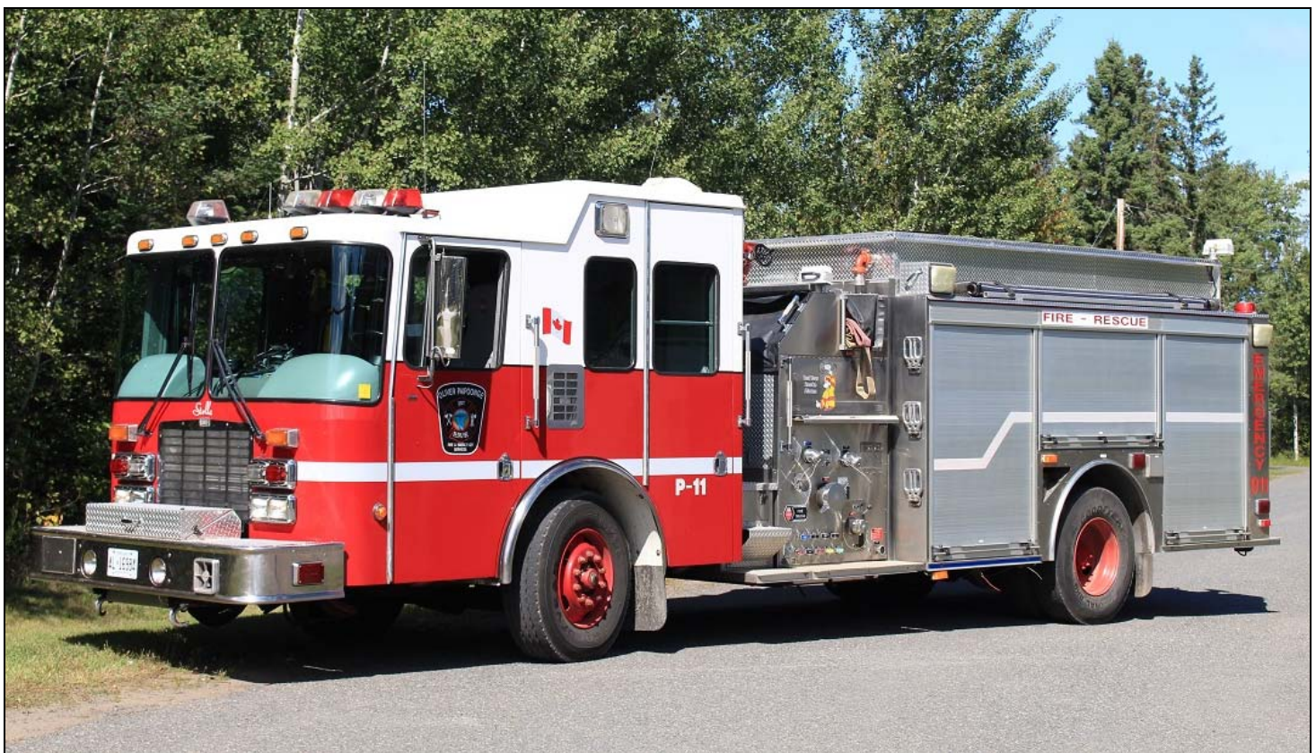
Off to a new home in Oliver Paipoonge, ON, this was Ottawa Pump 11, a 2003 HME 1871 Fort Garry pumper equipped with a 1250gpm pump and 500gwt. (Dave Stewardson photo)
