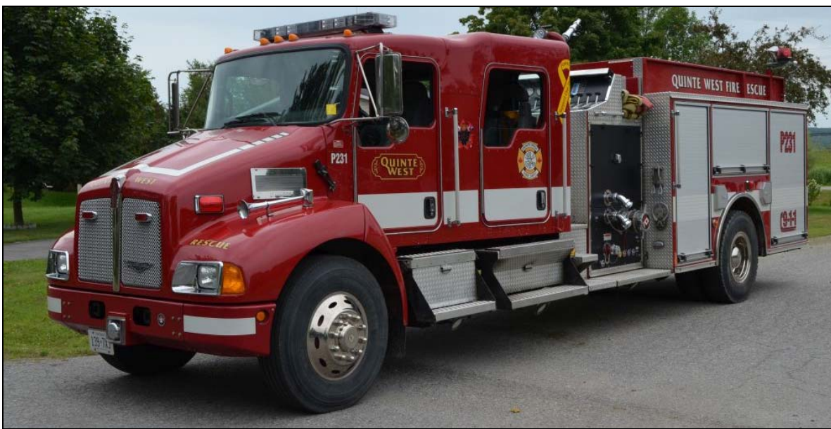
Quinte West Pumper 231, a 2007 Kenworth/Pierce with a 1050igpm pump and 835gwt. (Bob Rupert)
