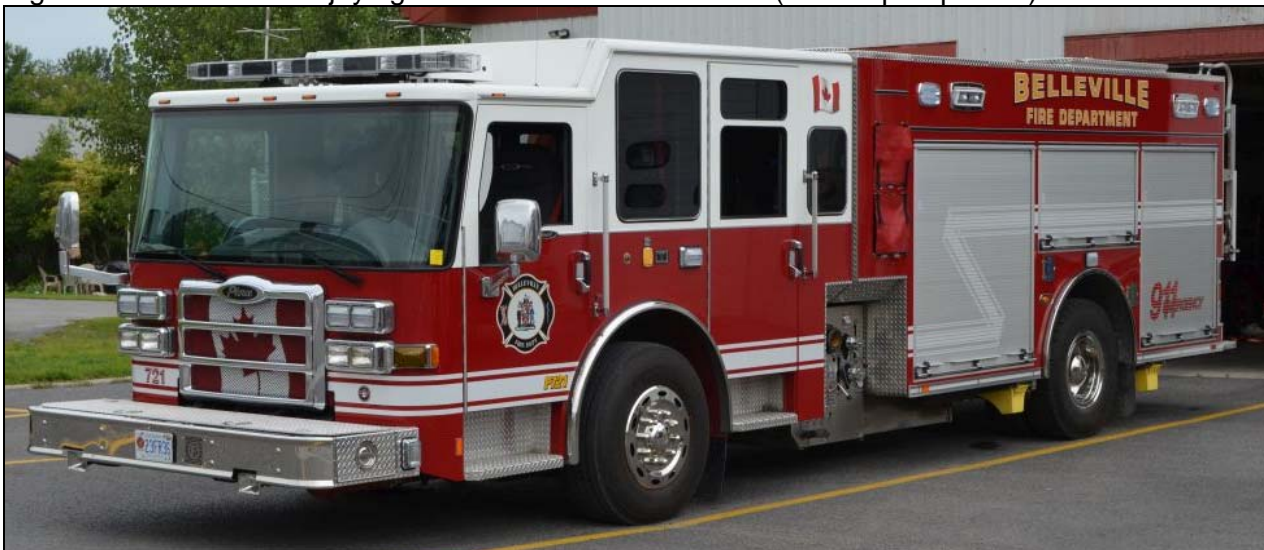
Belleville Pump 721, a Pierce Dash CF1331igpm pump, 537gwt, 5gft. Job#27047
