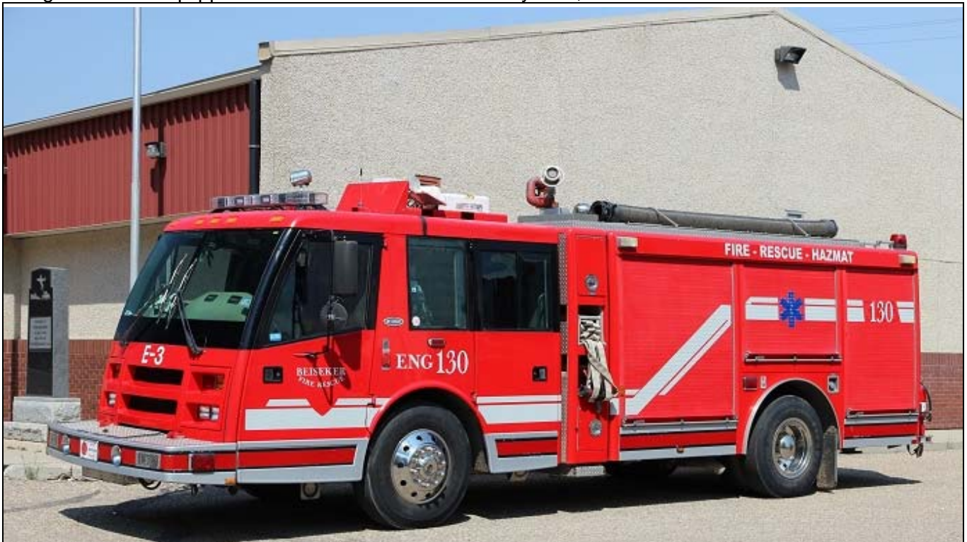
A unique find in Canada, this is an E-One Daytona pumper, operated by the Beiseker, AB FRS. Engine 130 was acquired through Fenton Fire in 2013, and was originally sold to the Port of Houston, and stationed in the Barbours Cut Container Terminal in 1998. It sports a rearmount 1500gpm Hale pump and a 500gwt. Around 10 of these were made and, apparently, this is the last of its kind still in service, all were originally sent to U.S. departments. (John Bowerman photos)
