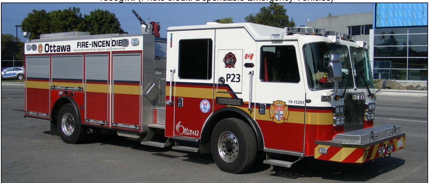
Ottawa Pump 23, one of 12 such rigs delivered this year, is a 2015 KME Predator Severe Service 1250igpm Waterous pump, 600gwt and 20gft. (Ken Walton photo)
