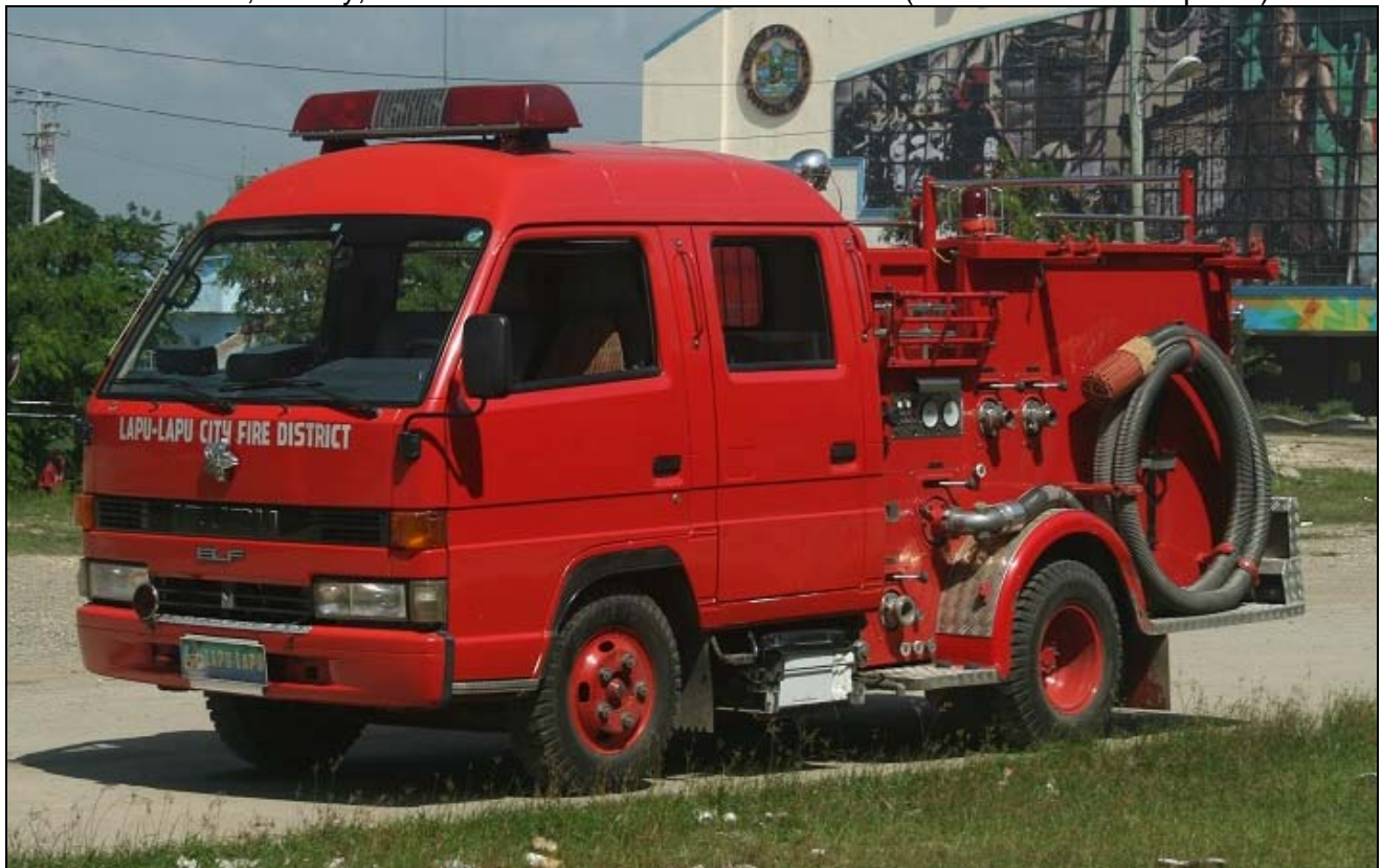
This former Japanese appliance is a 1990s vintage Isuzu/Ogawa pumper in service in Lapu-Lapu City in the Philippines since 2008. It has a 1000gpm pump and no tank. (Bob Dubbert photo)
