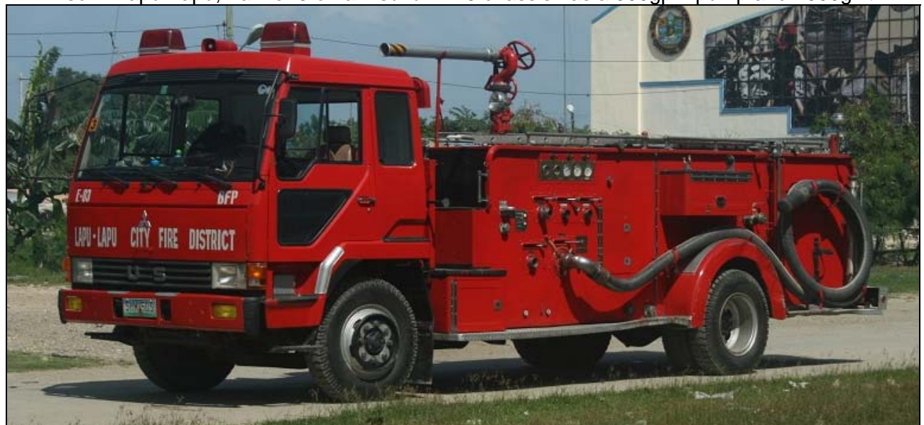
Lapu-Lapu Engine 3 is a 1985 Fuso/Morita pumper, 1000gpm and 700gwt.
