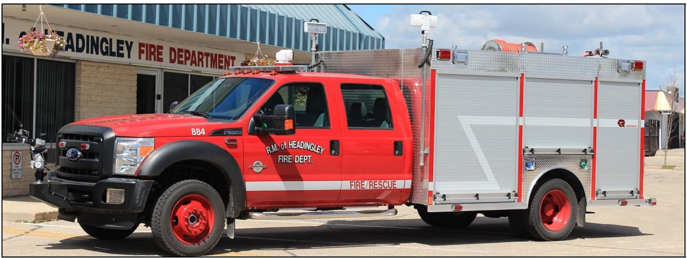
Headingly, MB 2015 Ford F550/Rosenbauer mini, 420igpm pump, 250gwt, 25gft (s/n 3796)
