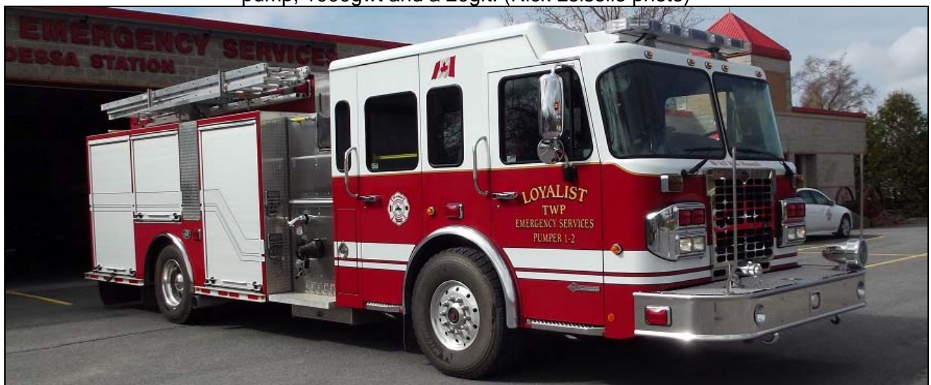
Below is Loyalist Township Pumper 2, a 2013 Spartan Metro Star/Dependable rig with 1050igpm pump, 1000gwt and a 20gft. (Rick Loiselle photo)
