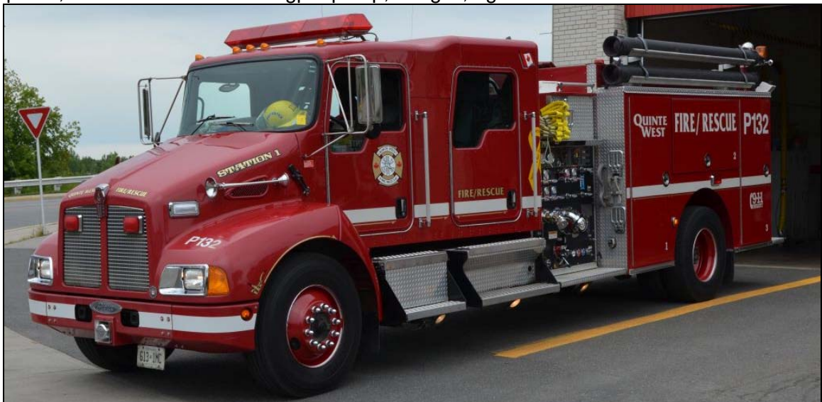
Quinte West Pump 132, a 2003 Kenworth T300/Pierce, 1750igpm pump, 800gwt. S #16327
