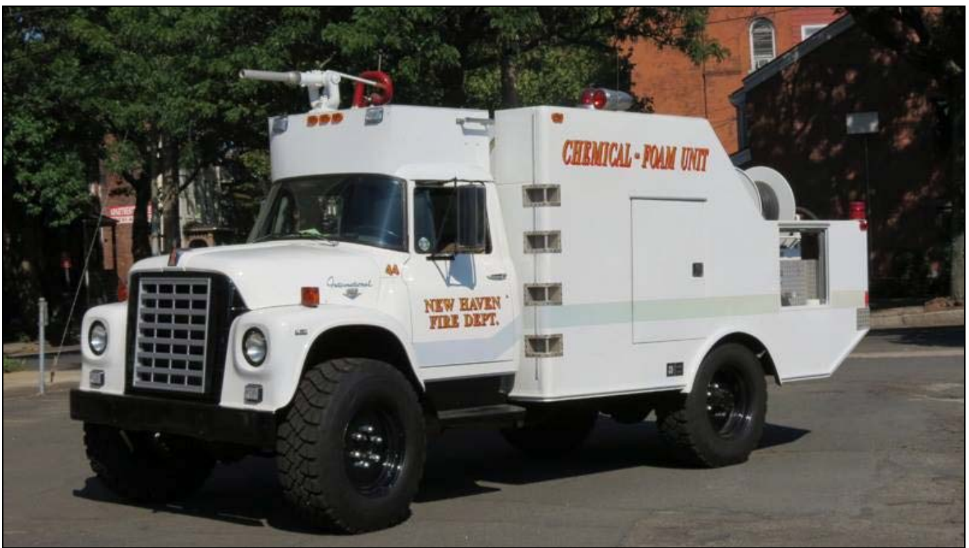
This unusual apparatus is the New Haven, CT FD Chemical/Foam Unit 44, seen at the 2015 IFBA convention. It is a 1970 IHC Loadstar 4x4/Amsul/Magnum 480 (480gft). (Herb Gallaway photo)
