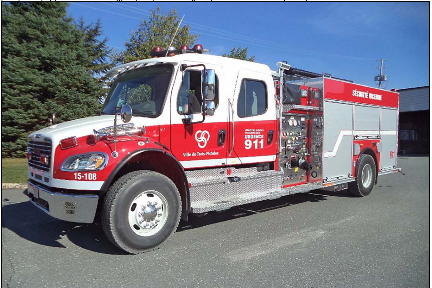
New to Trois Pistoles, QC, Unité 251 is a 2015 Freightliner M2-106/Maxi Métal pump with a 1050igpm pump and 1000gwt. (Photo from Maxi Métal)
