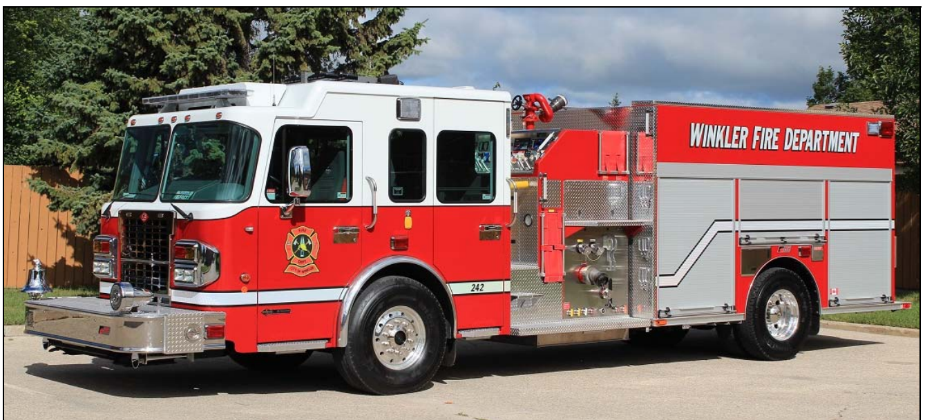
Winkler, MB recently received this 2015 Spartan Metro Star/Fort Garry 1250igpm/800gwt/2x20gft sn M623. It's assigned as Pumper 242. (Dave Stewardson photos)
