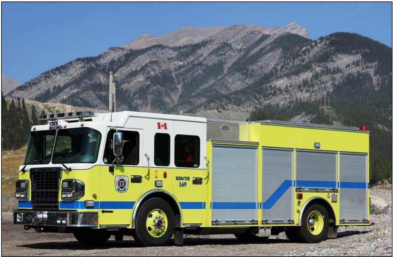
The Municipal District of Bighorn operates this 2014 Spartan Metro Star/Hub pumper from their hall in Exshaw, AB. Rescue 169 is their primary response rig, it has a 1050igpm Waterous pump, a 600gwt and a 30gft. It is also equipped with a Foam Pro 1600 foam system, SN 5520-1168.
