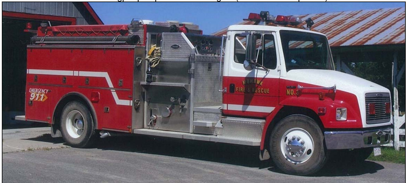
Below is Loyalist Township Pumper 2, a 2013 Spartan Metro Star/Dependable rig with 1050igpm pump, 1000gwt and a 20gft. (Rick Loiselle photo)
