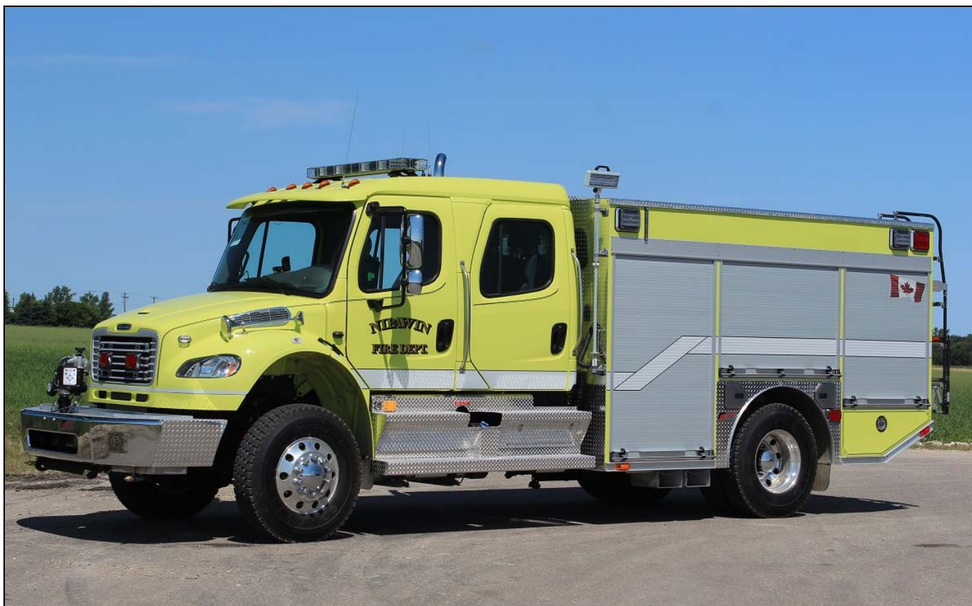
Nipawin, SK got this 2015 Freightliner M2-106 4x4/Fort Garry unit in the summer. It came with a 1050gpm Waterous pump, 1000gwt and 25gft. s/n M625 (Dave Stewardson photo)
