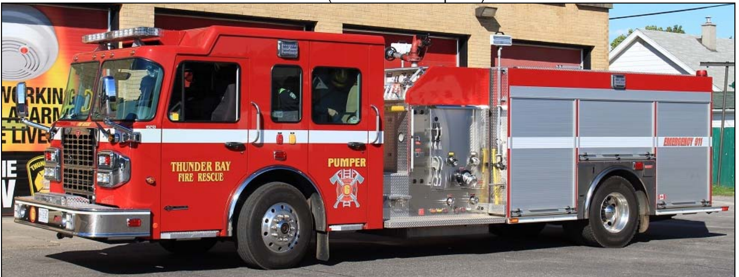
When he took the delivery shot of this rig for us last winter, Dave promised to reshoot it with the proper graphics and, true to his word, here is Thunder Bay Pumper 6, a 2015 Spartan Metro Star X/Fort Garry rig, in service. 1050igpm/600gwt #M597. Below is Markham 971, delivered last year. It's a 2014 Spartan Metro Star/Smeal pumper with a 1750gpm pump, 500gwt and 2x20gft. (Dave Stewardson photos)
