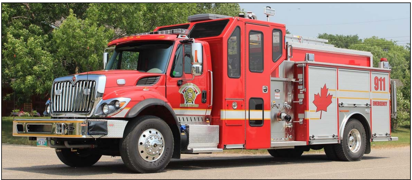
Boissevain, MB is now running this 2015 IHC Workstar 7500/Acres rig as Pumper 1, a 1050 igpm Waterous pump, 1000gwt and 25gft. SN 150521129. It replaced the 1993 Freightliner FL80/ Superior one below. That truck has a 1050igpm pump and an 800gwt, SN SE1375. (Dave Stewardson)
