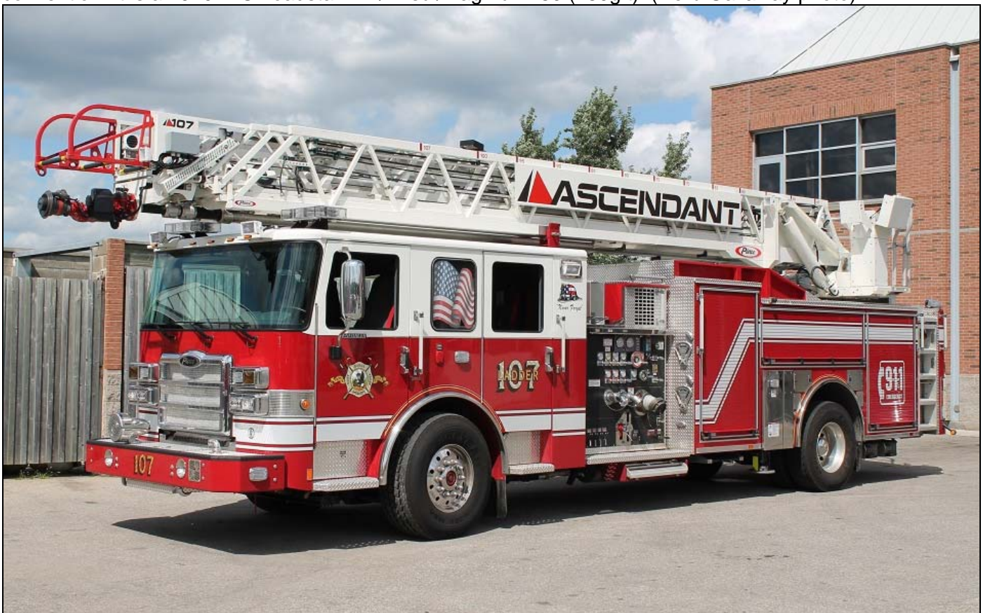
This is the new Pierce Ascendant; this particular demo was making the rounds in Southern Ontario and has now been purchased by Oakville. It packs a 107' ladder, 1250igpm pump and 417gwt, all on a single rear axle. The aerial can be raised in just 30 seconds, the jacks are just in front of the rear wheels and at the back. The rig will be restriped and numbered for Oakville before delivery. (Photo and info from Gary Dinkel)
