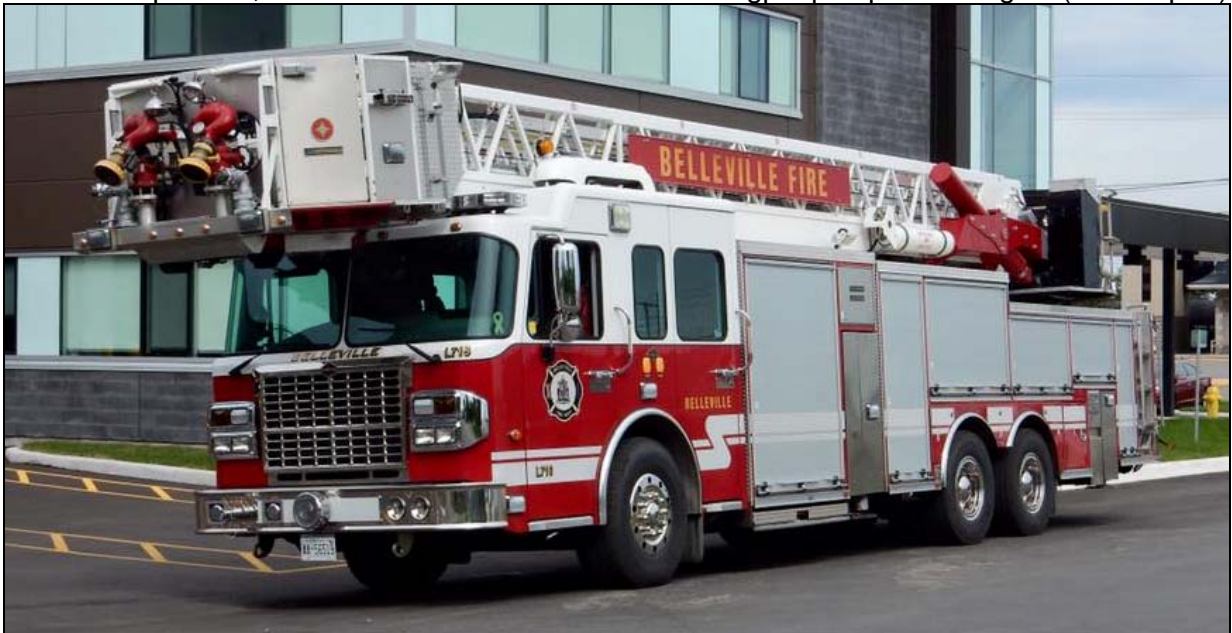
Belleville Ladder 716, a 2012 Spartan Gladiator MFD/Crimson/Dependable 100' Tower with a 2000gpm pump and 300gwt. (S/N J#2110097-01) (Ken Jansen). Below is Belleville Station 1. (Desmond Brett)
